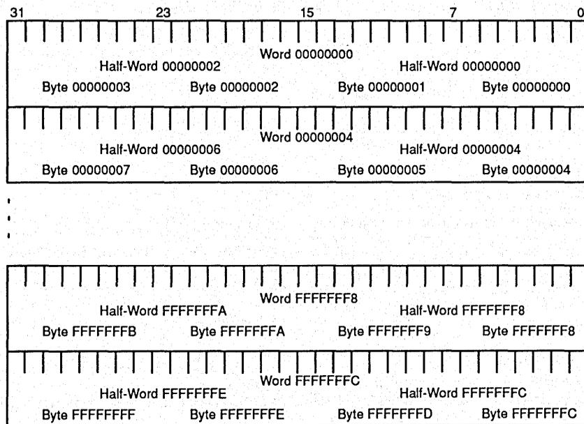
Figure 52. Byte and Half-Word Addressing with BO = 1
