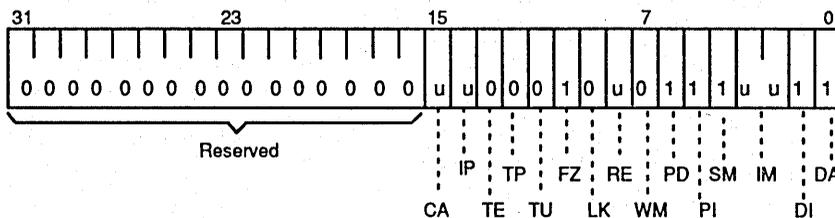
Figure 55. Current Processor Status after an Interrupt or Trap
