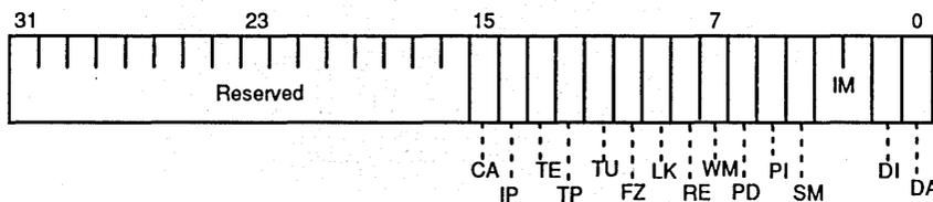
Figure 8. Current Processor Status Register
