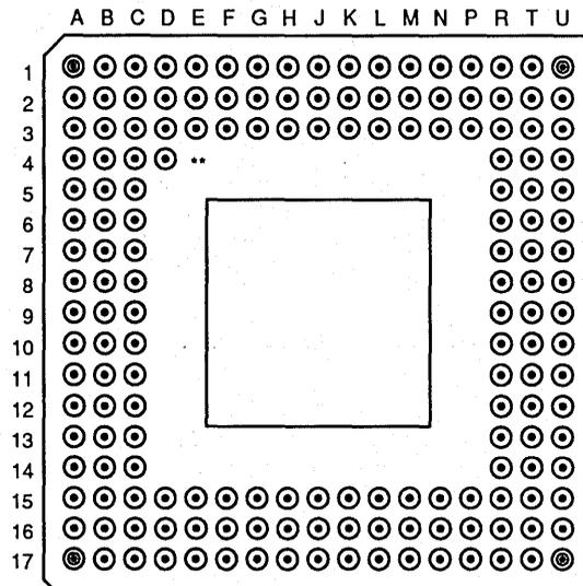
\* Pinout observed from pin side of package.
