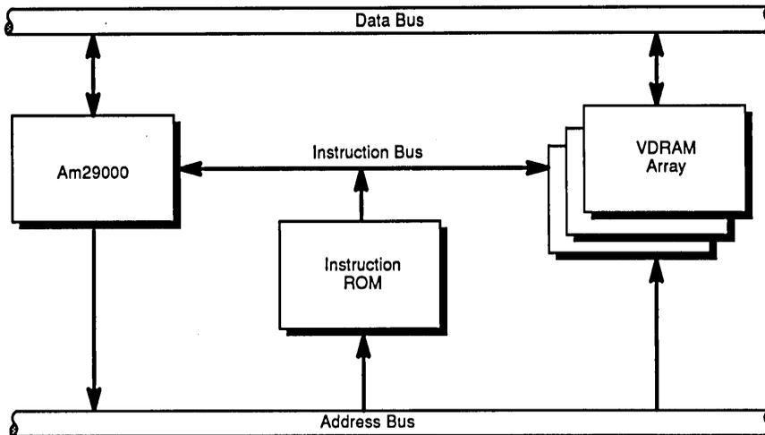
Figure 3. An Am29000 System with VDRAM
