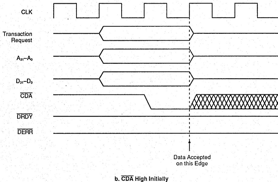
Note: Signals  $A_{31}-A_0$  and  $D_{31}-D_0$  are the Am29000 address and data buses, respectively.
