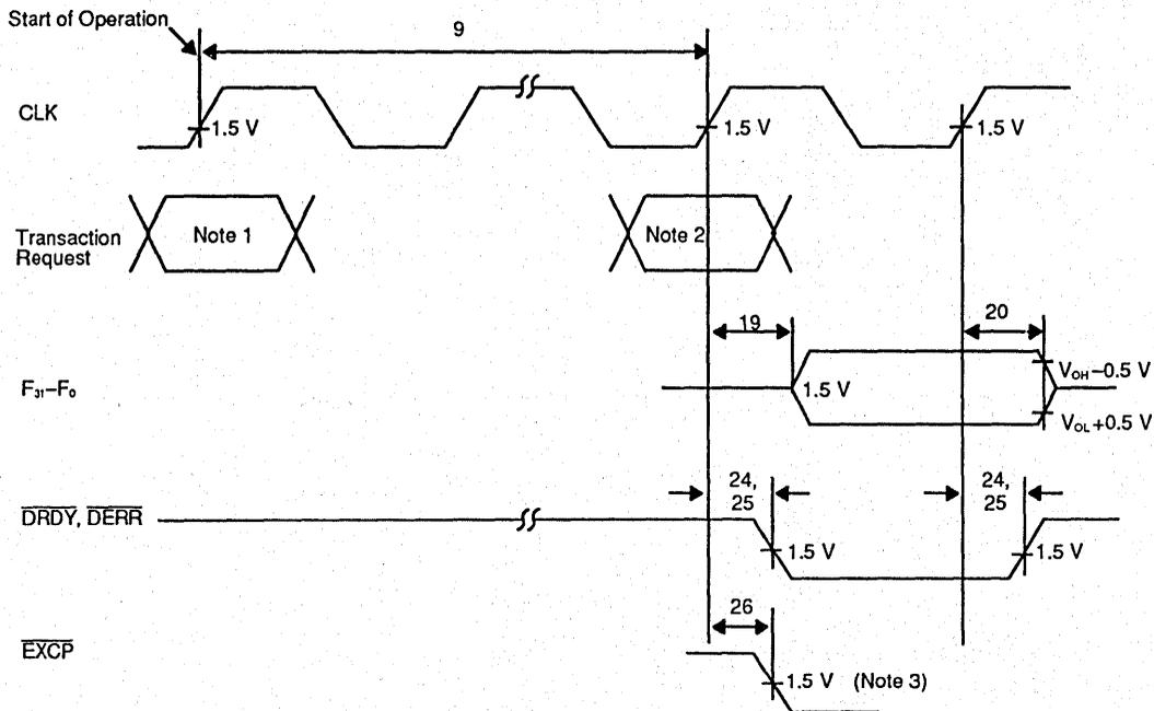
**Operation Timing for Pipeline Mode**
