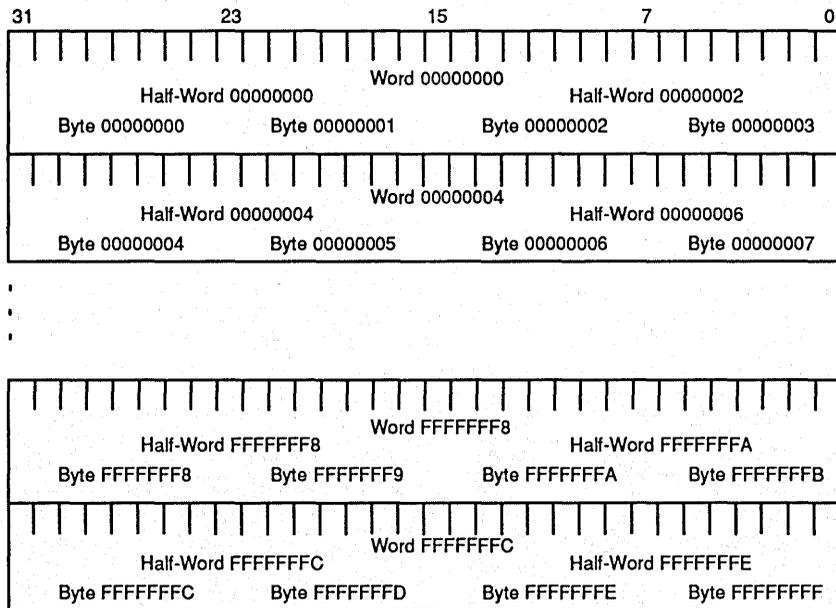
Figure 51. Byte and Half-Word Addressing with BO = 0
