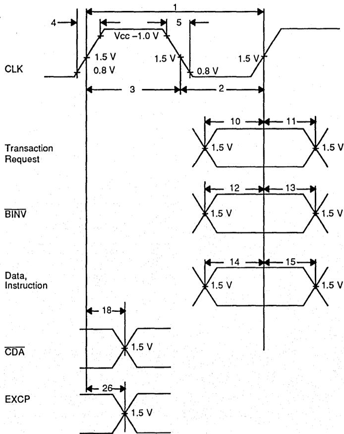
Input Signal Timing;  $\overline{\text{CDA}}$ , EXCP Timing
