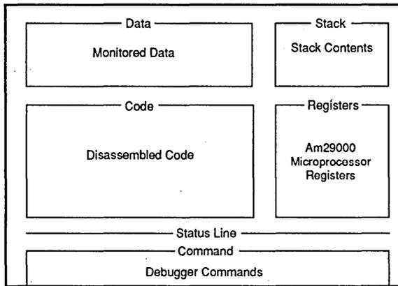
Figure 2. Standard Assembly-Level Screen
