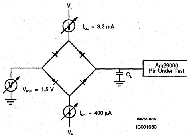
$C_L$  is guaranteed to 80 pF. For capacitive loading greater than 80 pF, refer to the Capacitive Output Delay table.
