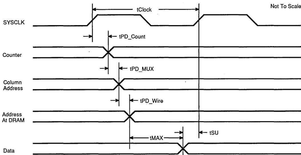
Figure 2. Single-Cycle Burst
