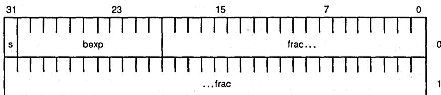
Figure 48. Double-Precision Floating-Point Format
