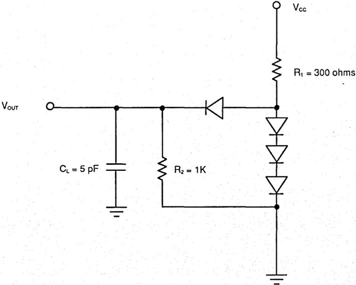
Three-State Output Inactive Test
