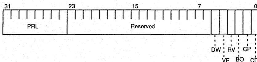
Figure 9. Configuration Register
