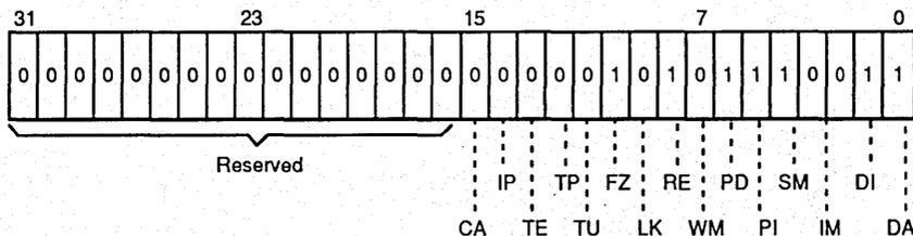
Figure 67. Current Processor Status Register in Reset Mode
