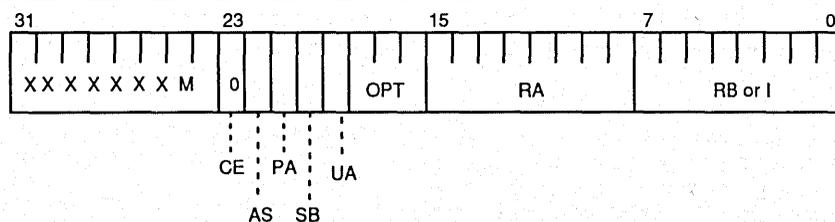
Figure 50. Non-Coprocessor Load/Store Format
