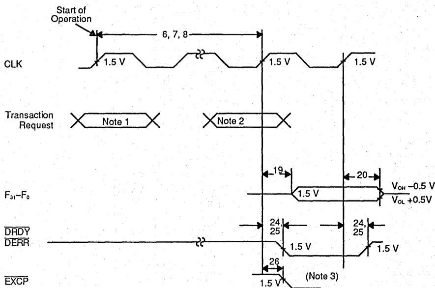
Operation Timing for Flow-Through Mode,  $\overline{DRDY}$ ,  $\overline{DERR}$  Not Advanced
