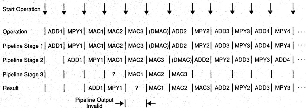
b. Pipeline invalidation timing for multiply-accumulate operations in pipeline mode.
