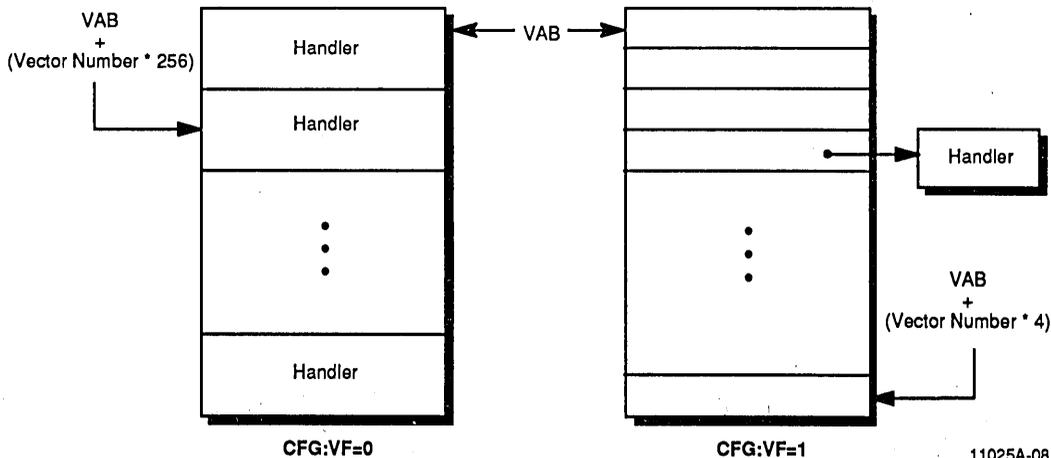
Figure 8. The Two Structures of the Vector Area
