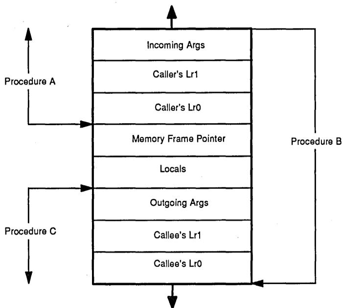
Figure 5. The Register Stack
