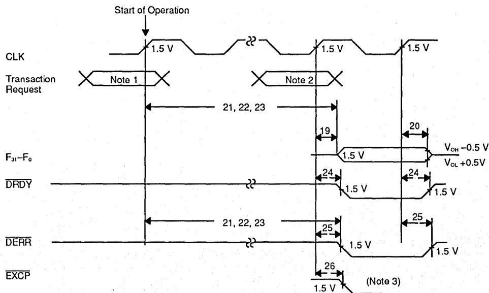
Operation Timing for Flow-Through Mode,  $\overline{\text{DRDY}}$ ,  $\overline{\text{DERR}}$  Advanced
