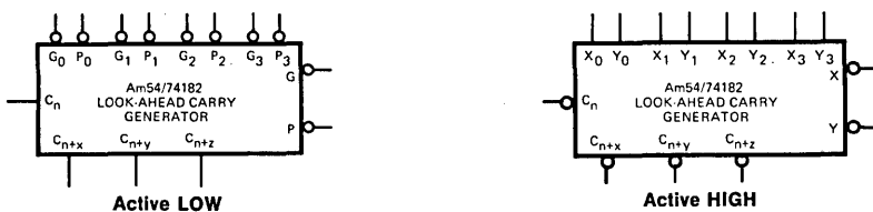
Figure 14. Am54/74182 (Am9342) Logic Symbol
