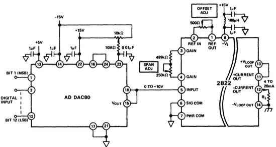
Figure 8. D/A Converter - Isolated 4 to 20mA Interface
