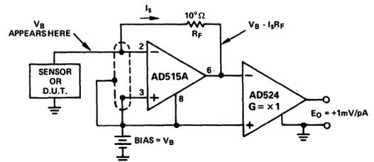
Figure 14. Current-to-Voltage Converters with Grounded Bias and Sensor
