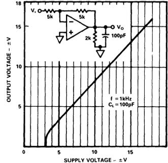
Figure 3. Output Voltage Swing vs. Supply Voltage
