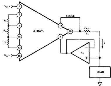
Figure 31. Voltage-to-Current Converter
