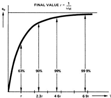
Figure 6. Step Response for Linear 6dB/Octave Amplifier
