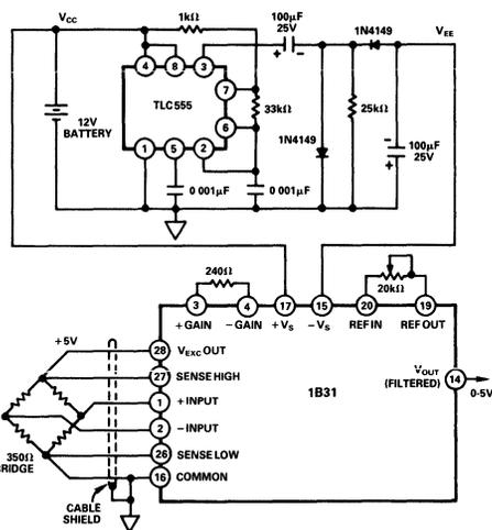
Figure 18. Negative Supply Generation for 1B31
