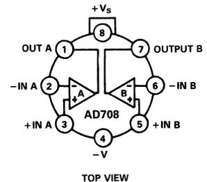
NOTE PIN 4 CONNECTED TO CASE
