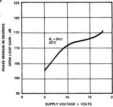
Figure 11. Open Loop Gain vs. Supply Voltage
