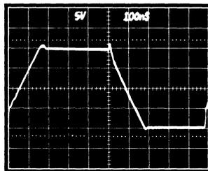
Figure 26b. Unity Gain Buffer Large Signal Response
