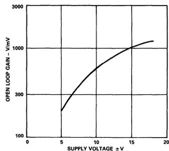
Figure 6. Open Loop Gain vs. Supply Voltage
