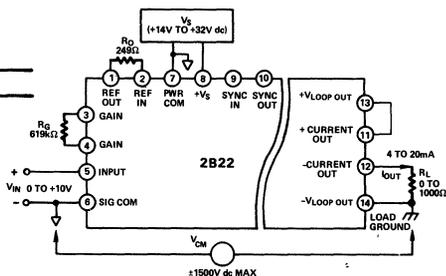
NOTE Resistors  $R_G$  and  $R_L$  are 1%, 50ppm/ $^{\circ}C$  Metal Film Type Values shown are for  $G = 1.6mA/V$ . For  $G = 16mA/V$ , use 10ppm/ $^{\circ}C$   $R_G$  and 50ppm/ $^{\circ}C$   $R_L$ .
