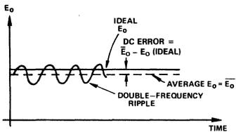
Figure 4. Typical Output Waveform for Sinusoidal Input
