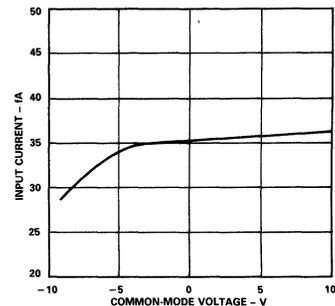
Figure 9. Input Bias Current vs. Common-Mode Voltage
