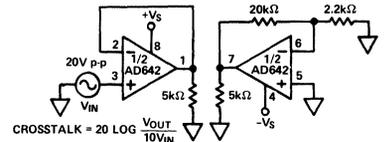
Figure 20. Crosstalk Test Circuit
