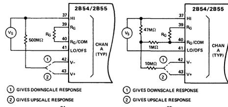
Figure 8. High Speed or Reversed Open Input Detection Output Filtering
