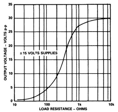
Figure 3. Output Voltage Swing vs. Resistive Load
