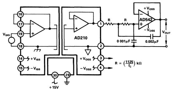
Figure 17. 2-Pole, Output Filter
