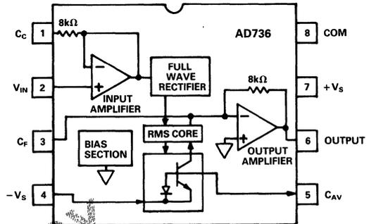
The AD736 allows the choice of two signal input terminals: a high impedance ( $10^{12}\Omega$ ) FET input which will directly interface with high Z input attenuators and a low impedance (8k $\Omega$ ) input which allows the measurement of 300mV input levels, while operating from the minimum power supply voltage of +2.8V, -3.2V. The two inputs may be used either singly or differentially.
