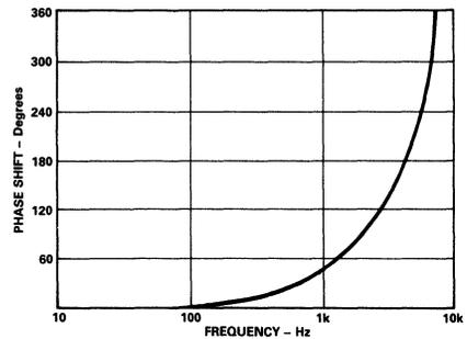
Figure 5. Typical AD295 - Phase Shift vs. Frequency
