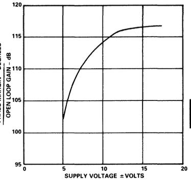
Figure 12. Open Loop Gain vs. Supply Voltage
