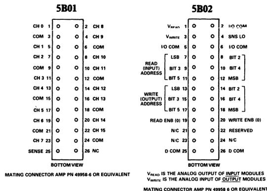
Figure 8. System Connector Pinout
