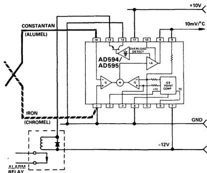
Figure 12. -ALM Driving A Negative Referenced Load
