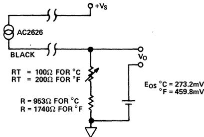
For most applications, a single point calibration is sufficient. With the probe at a known temperature, adjust R<sub>T</sub> so that V<sub>O</sub> corresponds to the known temperature.
