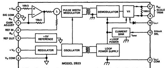
In data acquisition and control systems, the 2B23 may act as an isolated interface between the D/A converter output of a micro-computer analog I/O and standard 4 to 20mA or 0 to 20mA analog loops. In process control systems, the 2B23 may be used as a current output stage of a proportional controller to interface devices such as current-to-position converters and current-to-pneumatic transducers.
