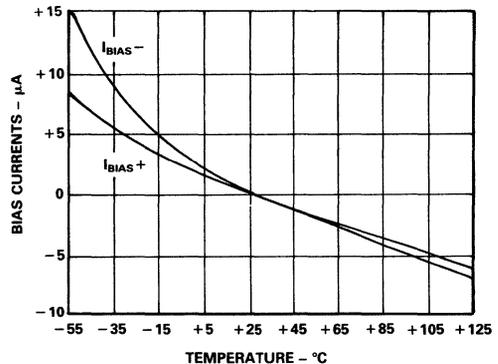
Figure 6. Bias Currents vs. Temperature
