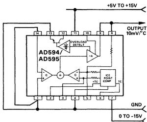
Figure 13. AD594/AD595 as a Stand-Alone Celsius Thermometer
