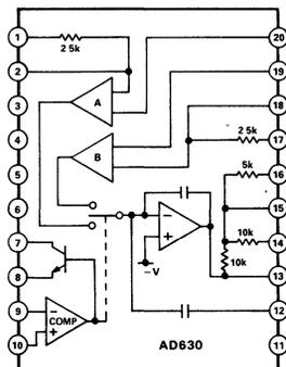
As a *lock-in amplifier*, it can recover a 0.1-Hz sine wave, transmitted as a modulation on a 400-Hz carrier, from a band-limited, clipped white-noise signal approximately 100,000 times larger – a dynamic range greater than 100dB.
