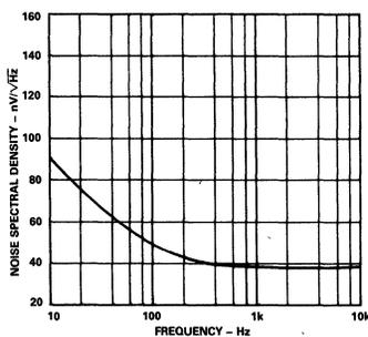
Figure 11. Input Voltage Noise vs. Frequency Spectral Density
