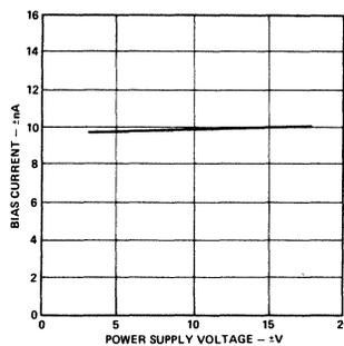
Figure 5. Input Bias Current vs. Supply Voltage
