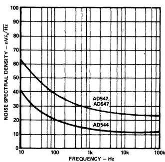
Figure 17. Input Noise Voltage Spectral Density
