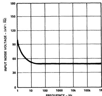
Figure 8. Input Voltage Noise vs. Frequency
