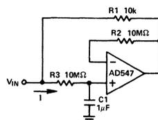
Figure 37. Capacitance Multiplier
