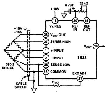
Figure 4. Constant Voltage Excitation: +10V to +15V Range.
