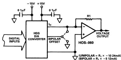
Figure 3. Inverting Unipolar or Bipolar Voltage Output
