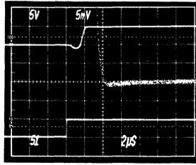
Figure 26. Gain Change Settling Time\*, Gain Change: 1 to 2
