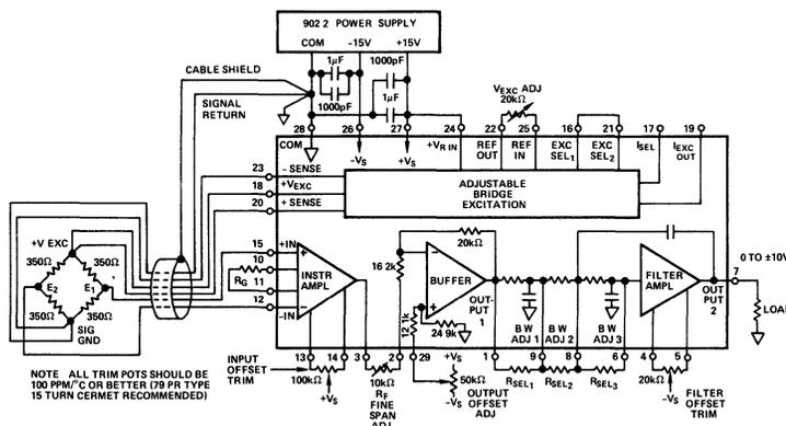
Figure 1. Typical Bridge Transducer Application Using 2B31
