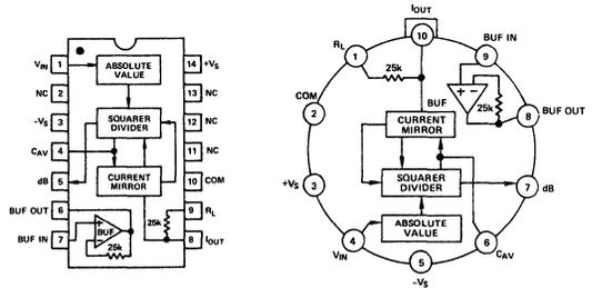
Figure 11. AD536A Pin Connections and Functional Diagram
