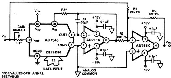
Figure 32. Bipolar Operation
