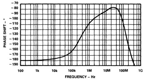
Small-Signal Output Phase Shift vs. Frequency ( $G = -10$ )
