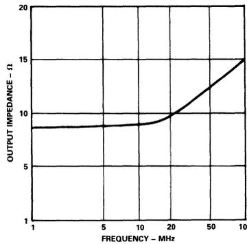
Figure 7. Output Impedance vs. Frequency
