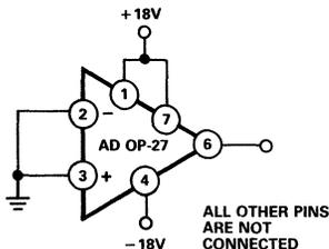
Figure 2. Burn-In Circuit
