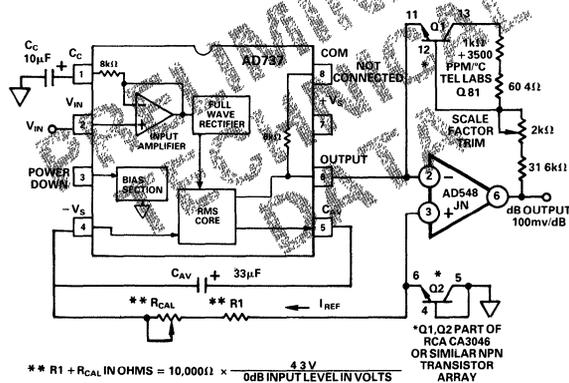
Figure 3. dB Output Connection
