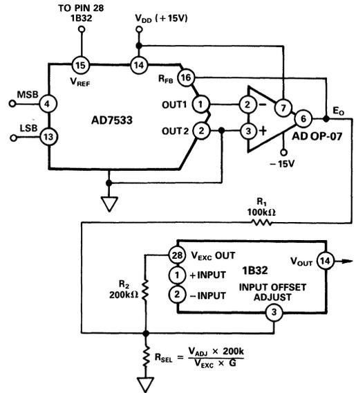
Figure 18. Output Offset Adjust Using a 10-Bit DAC
