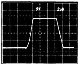
Transient Response  $R_L = 2k\Omega$   $C_L = 500pF$
