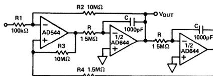
$$f_0 = \text{CENTER FREQUENCY} = 1/2\pi R_3 C$$
