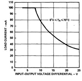
Figure 13. Maximum Load Current vs. Regulator Input-Output Voltage Differential
