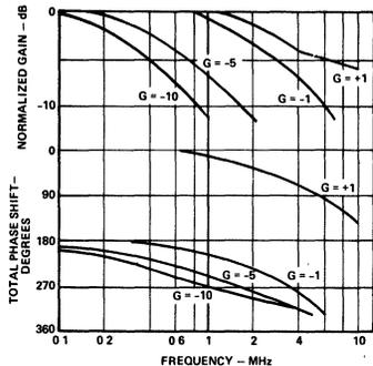
Figure 17. Closed Loop Gain & Phase vs. Frequency
