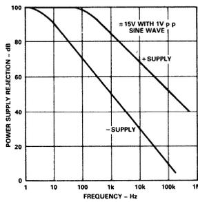
Figure 8. PSRR vs. Frequency
