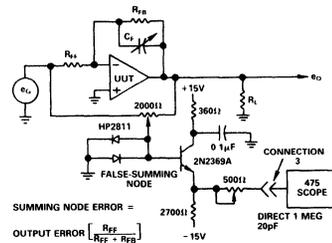
Figure 6. Settling Time Test Circuit for 0.1% Settling
