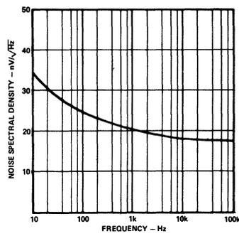
Figure 15. Noise Spectral Density
