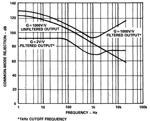
Figure 11. Common-Mode Rejection vs. Frequency and Gain
