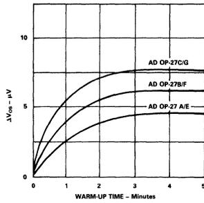
Input Offset Voltage Turn-On Drift vs. Time
