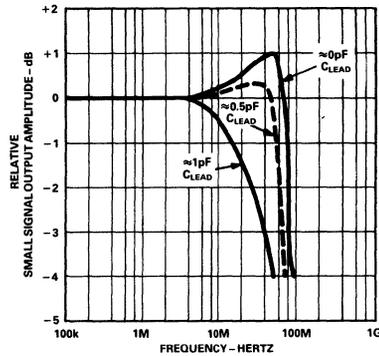
Figure 34. Response of the 20dB Video Amplifier
