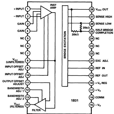
pair of thin-film  $20\text{k}\Omega$  resistors is connected across the excitation outputs. This assures temperature tracking of  $\pm 5\text{ppm}/^\circ\text{C}$  max and reduces part count.
