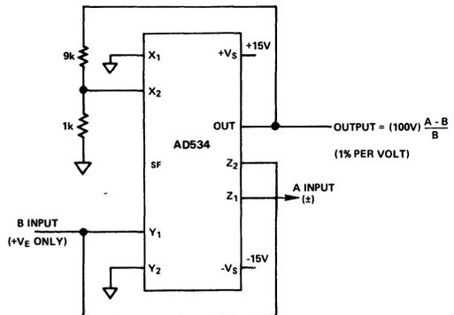
OTHER SCALES, FROM 10% PER VOLT TO 0.1% PER VOLT CAN BE OBTAINED BY ALTERING THE FEEDBACK RATIO
