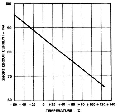
Figure 16. Short Circuit Current Limit vs. Temperature
