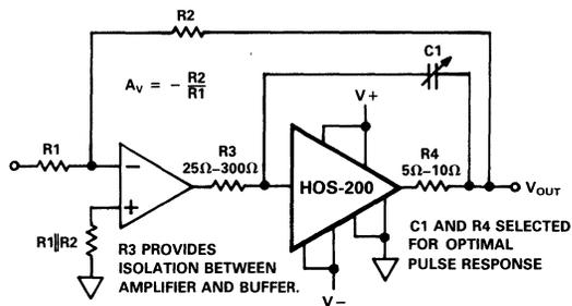
Figure 1. Increased Output Current Drive
