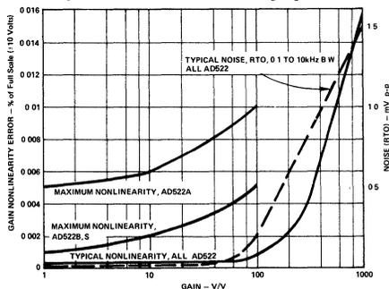
Figure 4. Gain Nonlinearity and Noise (RTO) vs. Gain
