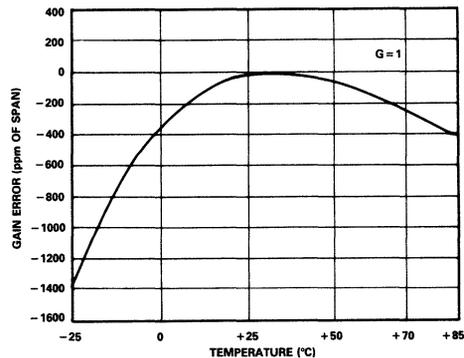
Figure 14. Gain vs. Temperature
