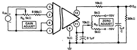
GAIN RESISTOR,  $R_1$ , 1%, 50ppm/°C METAL FILM TYPE IS RECOMMENDED FOR GAIN = 1V/V, LEAVE TERMINAL 2 OPEN.
