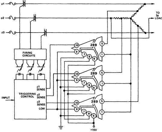
Figure 15. Isolating a 3 Phase Load Controller
