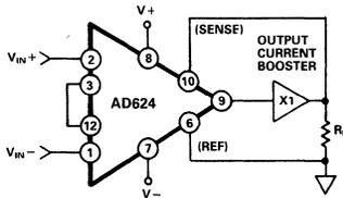
Figure 35. AD624 Instrumentation Amplifier with Output Current Booster
