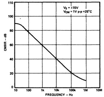
Figure 12. Common Mode Rejection Ratio vs. Frequency
