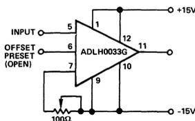
Figure 1. Offset Adjustment
