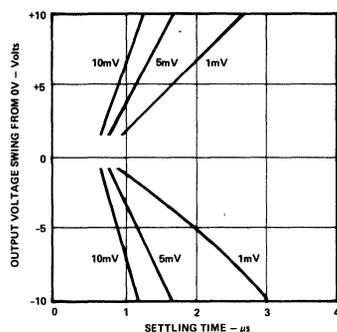
Figure 15. AD544 Output Settling Time vs. Output Swing and Error
