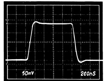
Figure 23c. Unity Gain Inverter Pulse Response (Small Signal)
