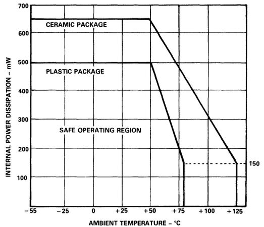
Figure 14. Excitation Source Internal Power Dissipation vs. Temperature
