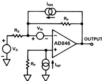
Figure 42. Op Amp Simplified Noise Model
