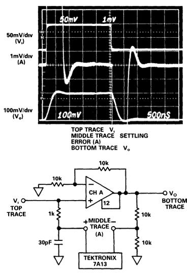
Figure 8. Small Signal Noninverting Step Response
