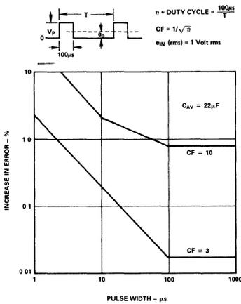
Figure 11. AD637 Error vs. Pulse Width Rectangular Pulse
