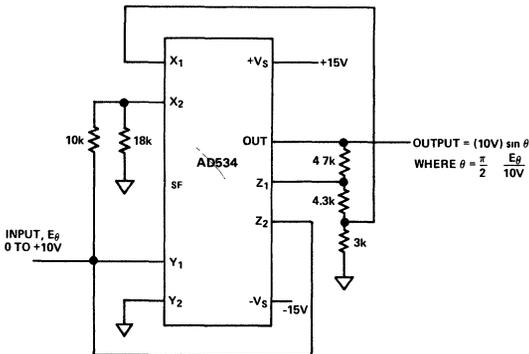
USING CLOSE TOLERANCE RESISTORS AND AD534L, ACCURACY OF FIT IS WITHIN ±0.5% AT ALL POINTS.  $\theta$  IS IN RADIANS.
