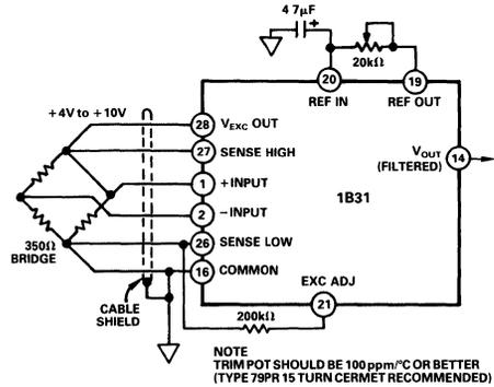
Figure 6. Constant Voltage Excitation: +4V to +10V Range
