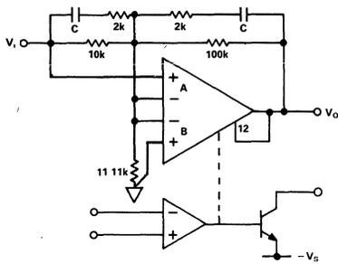
Figure 16. AD630 with External Feedback
