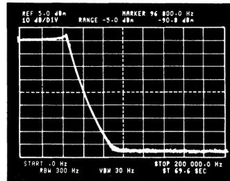
Figure 42. High Frequency Response for 9 Pole Chebychev Filter
