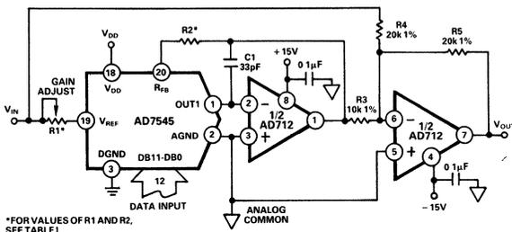
Figure 32. Bipolar Operation
