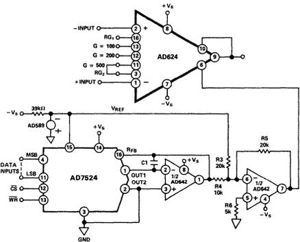
Figure 41. Software Controllable Offset
