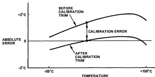
Figure 5. Effect of Scale Factor Trim on Accuracy
