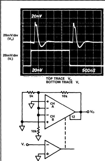
Figure 7. Channel-to-Channel Switch-Settling Characteristic
