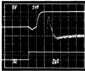
Figure 29. Gain Change Settling Time\*, Gain Change 1 to 16
