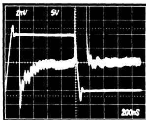
Figure 25b. Unity Gain Inverter Large Signal Response
