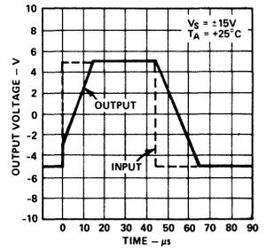
Figure 9. Voltage Follower Large Signal Pulse Response
