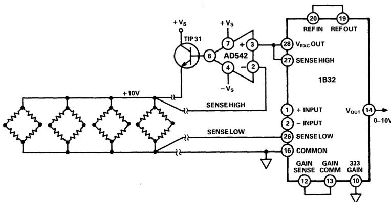
Figure 16. Multiple Load-Cell Application
