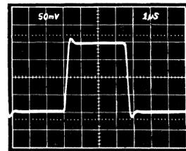
Figure 22c. Unity Gain Inverter Pulse Response (Small Signal)
