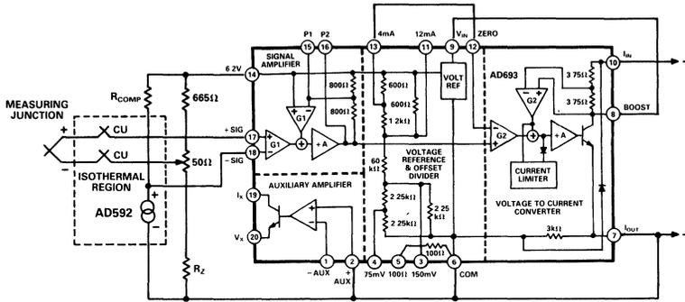
Figure 19. Thermocouple Inputs with Cold Junction Compensation
