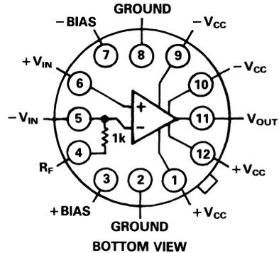
Current feedback is used instead of voltage feedback to provide dynamic performance that is relatively independent of gain settings. Flat gain and phase response combine with excellent noise and distortion performance to provide a unity-gain-stable amplifier especially well suited for use in digital communication systems. The AD9611 is an excellent choice for driving the newest generation of ultrahigh-speed flash converters when system SNR and effective number of bits are important.
