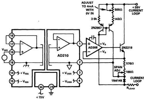
Figure 19. Isolated Voltage-to-Current Loop Converter
