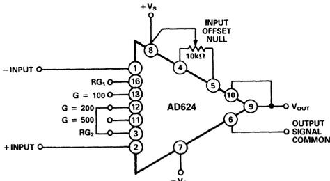
Figure 28. Operating Connections for  $G = 200$
