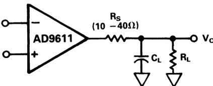
Figure 4. Isolating Capacitive Loads
