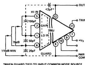
Figure 4. Model 286J Terminal Capacitance and CMR Ratings
