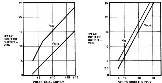
Figure 16. AD536A Input and Output Voltage Ranges vs. Supply
