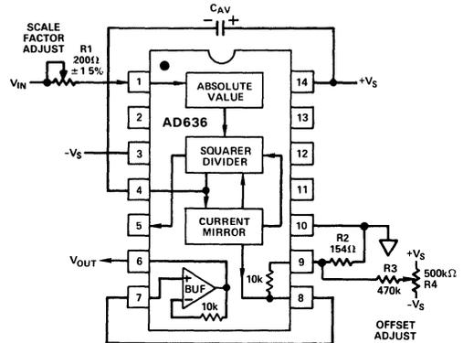
Figure 2. Optional External Gain and Output Offset Trims
