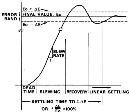
Figure 1. Settling Time
