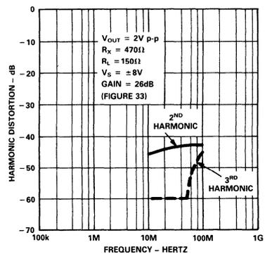
Figure 9. Harmonic Distortion vs. Frequency - High Gain
