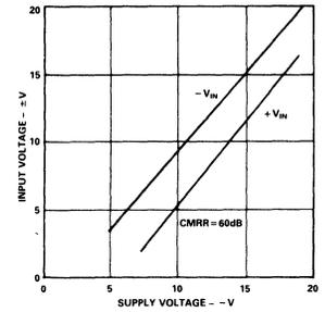
Figure 18. Input Voltage Range vs. Supply Voltage
