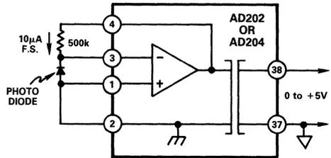
Figure 22. Photodiode Amplifier
