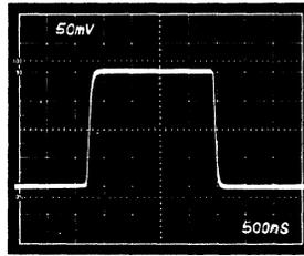
Figure 14. Small Signal Pulse Response,  $G=1$
