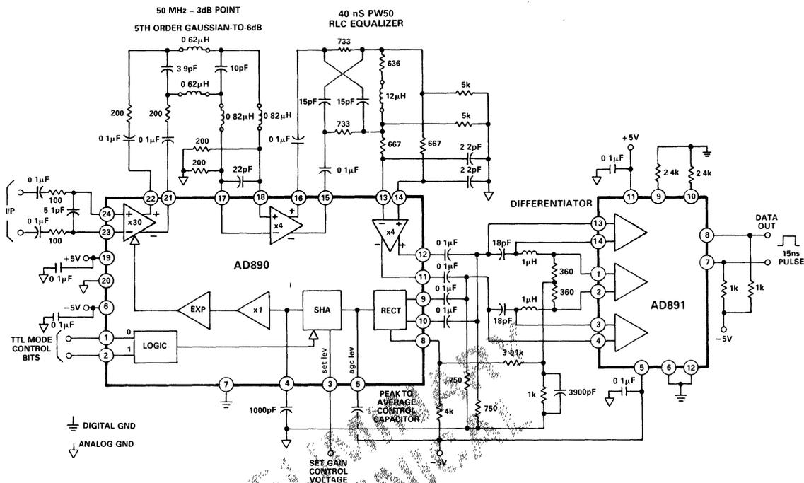
Figure 2. Typical AD890/AD891 Connection for a 30MHz Channel
