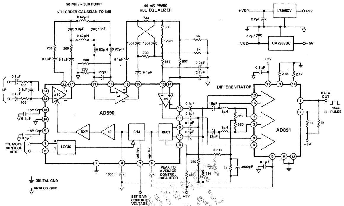
Figure 3. Typical AD890/AD891 Connection for a 30MHz Channel
