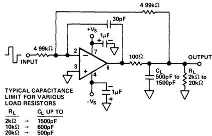
Figure 27. Circuit for Driving a Large Capacitance Load
