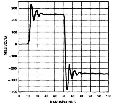
Figure 8. Small-Signal Settling ( $\pm 250\text{mV}$  Square Wave Input)
