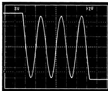
Figure 3. Output Function for Peak X-Input of  $\pm 18V$ , with  $U = 15V$ ,  $R_L = 600\Omega$  ( $\pm V_S = 18V$ )
