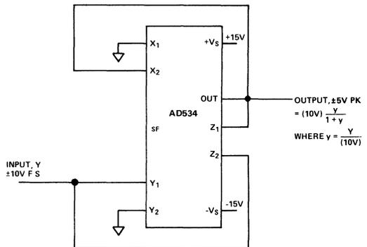
Figure 12. Bridge-Linearization Function
