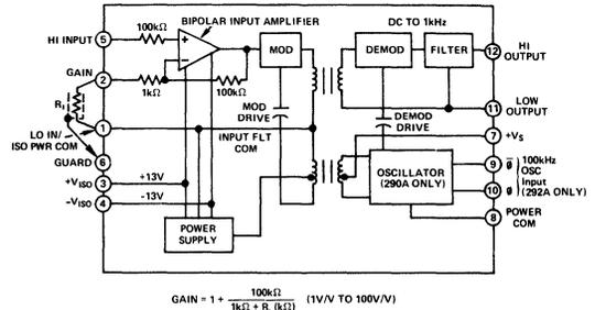
with 20V pk-pk input signal range at a gain of 1V/V operation. In portable single or multichannel designs, single power supply operation (+8V to +16V) enables battery operation.
