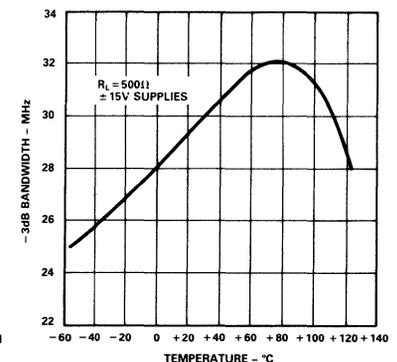
Figure 34. 3dB Bandwidth vs. Temperature
