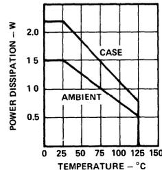
Figure 2. Power Dissipation vs. Temperature
