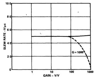
Figure 12. Slew Rate vs. Gain
