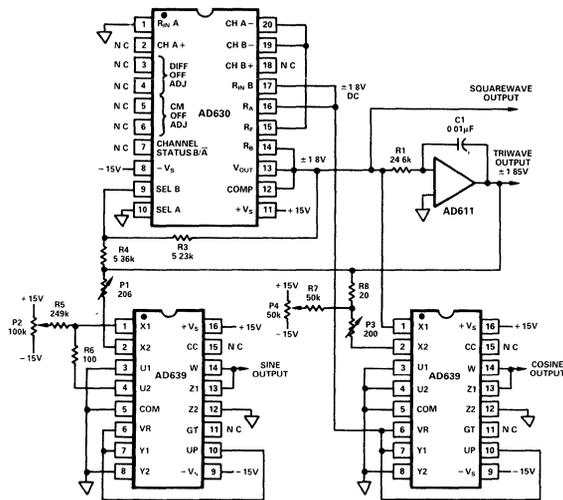
Figure 15. Quadrature Oscillator
