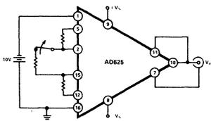
Figure 11. Overrange and Gain Switching Test Circuit ( $G=8$ ,  $G=1$ )
