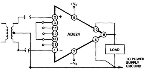
Figure 31a. Transformer Coupled
