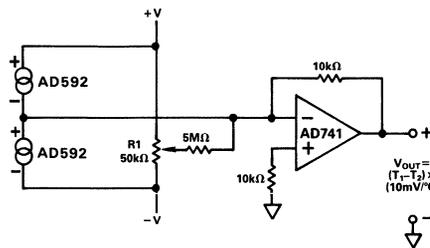
Figure 10. Differential Measurements
