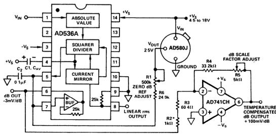
Figure 12. Temperature Compensated dB Output Circuit
