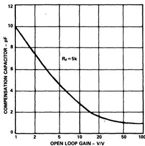
Figure 22. Recommended Compensation Capacitor vs. Closed Loop Gain
