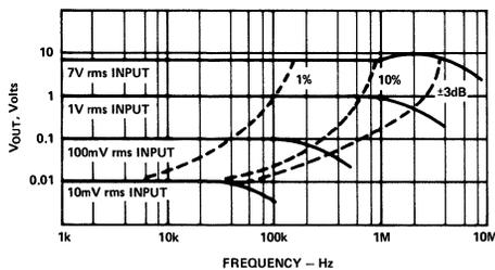
Figure 13. High Frequency Response
