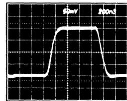
Figure 24c. Unity Gain Inverter Pulse Response (Small Signal)
