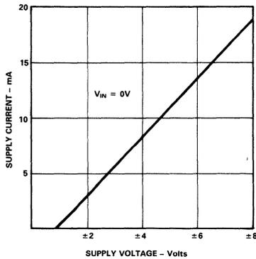
Figure 6. Supply Current vs. Supply Voltage
