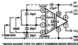
Figure 3. Model 284J Terminal Capacitance and CMR Ratings
