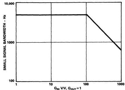
Figure 11. Typical AD295 - Small Signal Bandwidth vs. Gain
