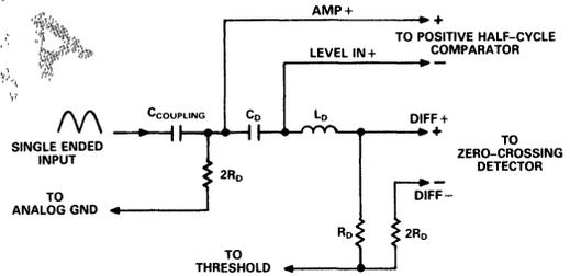
Figure 2b. Single-Ended Configuration of Passive Delay-Line Differentiator
