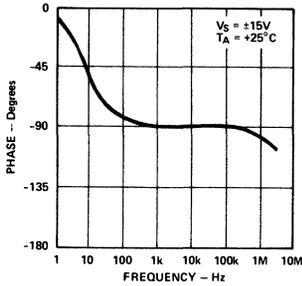
Figure 4. Open Loop Phase Response vs. Frequency
