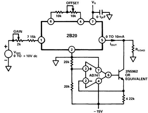
Figure 4a. 2B20 Configuration for 0 to 10mA Operation
