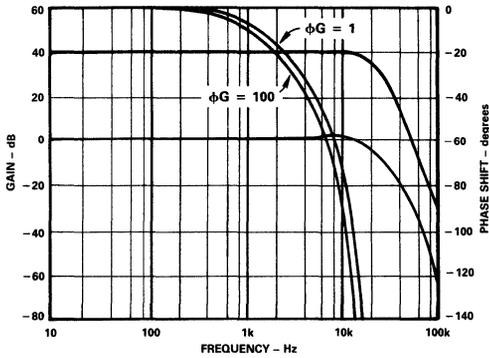
Figure 10. Phase Shift and Gain vs. Frequency
