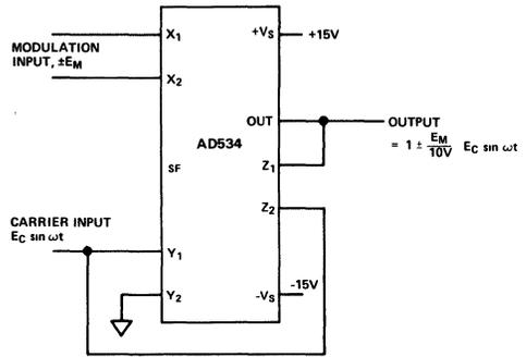
THE SF PIN OR A Z-ATTENUATOR CAN BE USED TO PROVIDE OVERALL SIGNAL AMPLIFICATION. OPERATION FROM A SINGLE SUPPLY IS POSSIBLE, BIAS  $Y_2$  TO  $V_S/2$ .
