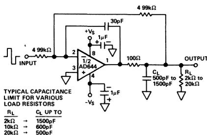
Figure 24. Circuit for Driving a Large Capacitive Load
