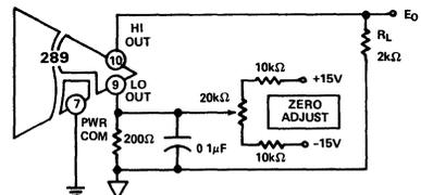
Figure 5b. Recommended Offset Adjustment for  $G = 1V/V$
