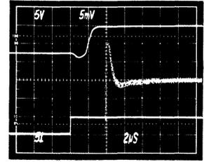
Figure 27. Gain Change Settling Time\*, Gain Change 1 to 4
