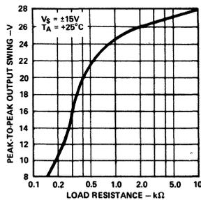
Figure 11. Output Voltage Swing vs. Load Resistance
