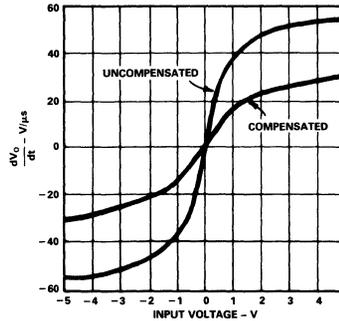
Figure 5.  $\frac{dV_O}{dt}$  vs. Input Voltage
