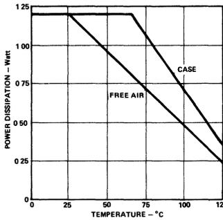
Figure 5. Permitted Dissipation vs. Temperature for AD382
