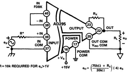
d. Output Gain Noninverting Configuration
