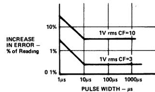
Figure 15. AD536A Error vs. Pulse Width Rectangular Pulse
