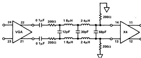
Figure 4. 5th Order Gaussian-to-6dB Transitional Filter
