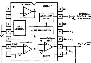
Figure 2. Standard rms Connection
