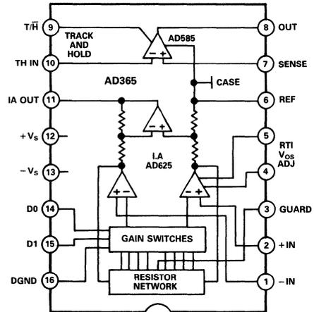
The input stage provides high common-mode rejection, low noise, fast settling at all gains, and low drift over temperature. The gains of 1, 10, 100, and 500 are digitally selected with the two gain control lines which are 5V CMOS compatible.
