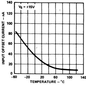
Figure 1. Offset Current vs. Temperature
