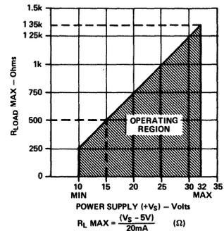
Figure 1. Maximum Load Resistance vs. Power Supply
