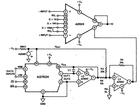
Figure 44. Software Controllable Offset
