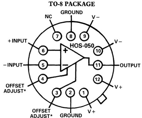
\*PINS FOR CONNECTING OPTIONAL OFFSET POTENTIOMETER. RECOMMENDED VALUE IS 10K OHMS, WITH CENTER ARM CONNECTED TO +15V.
