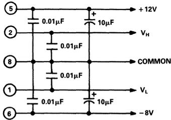
Figure 4. Basic Circuit Decoupling
