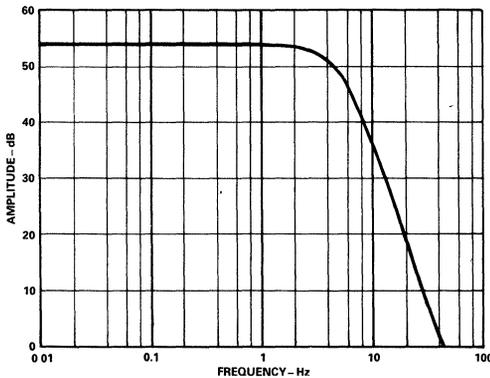
Figure 10. Filter Amplitude Response vs. Frequency,  $G = 500$
