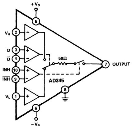
Figure 3. AD345 Block Diagram
