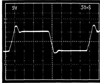
Figure 19b. Large Signal Pulse Response, Gain of 1
