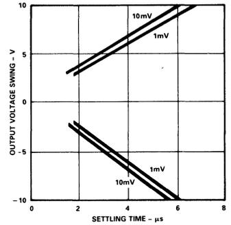
Figure 15. Output Settling Time vs. Output Swing and Error Voltage
