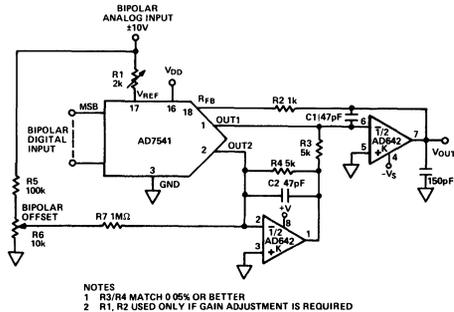
Figure 27a. AD642 Used as DAC Output Amplifier
