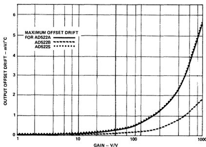
Figure 3. Output Offset Drift (RTO) vs. Gain
