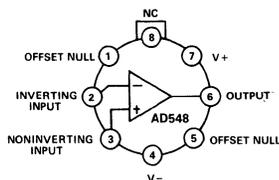
NOTE: PIN 4 CONNECTED TO CASE
