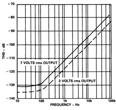
Figure 16. Total Harmonic Distortion vs. Frequency, Circuit of Figure 20 ( $G = 10$ )
