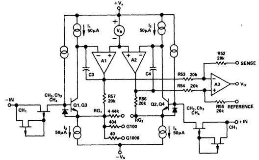
Figure 29. Simplified Circuit of Amplifier; Gain is Defined as  $((R56 + R57)/(R55)) + 1$ . For a Gain of 1,  $R_G$  is an Open Circuit
