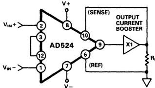
Figure 38. AD524 Instrumentation Amplifier with Output Current Booster
