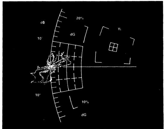
Figure 38. Differential Gain/Differential Phase Target with Generator Output Connected to Video Amplifier Input – Amplifier is Output Connected to Vector Scope Input
