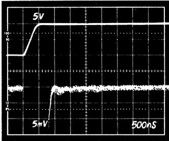
Figure 28a. Settling Characteristics 0 to +10V Step
