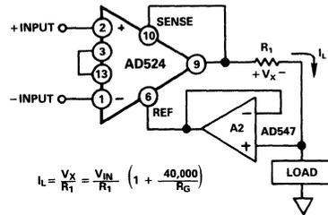
$$I_L = \frac{V_X}{R_1} = \frac{V_{IN}}{R_1} \left( 1 + \frac{40,000}{R_G} \right)$$
