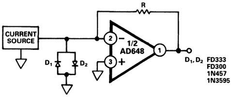
Figure 23c. I-to-V Converter with Diode Input Protection
