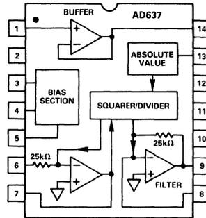
The AD637 is available in two accuracy grades (J, K) for commercial (0 to +70°C) temperature range applications and one (S) rated over the -55°C to +125°C temperature range. All versions are available in hermetically-sealed, 14-pin side-brazed ceramic DIPs as well as low-cost cerdip packages.
