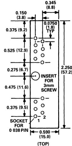
Figure 5. Module Footprint and Pinout
