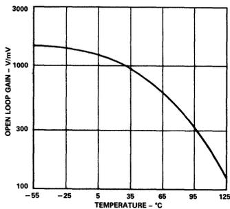
Figure 7. Open Loop Gain vs. Temperature
