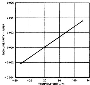
Figure 11. Nonlinearity vs. Temperature,  $Gain = 1$
