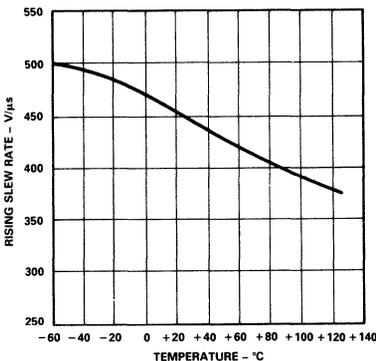
Figure 17. Slew Rate vs. Temperature
