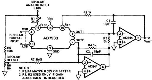
Figure 32a. AD544 Used as DAC Output Amplifiers
