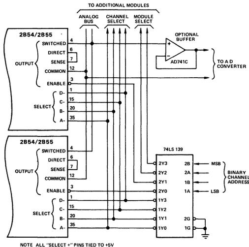
Figure 6. Expansion to More than Four Channels
