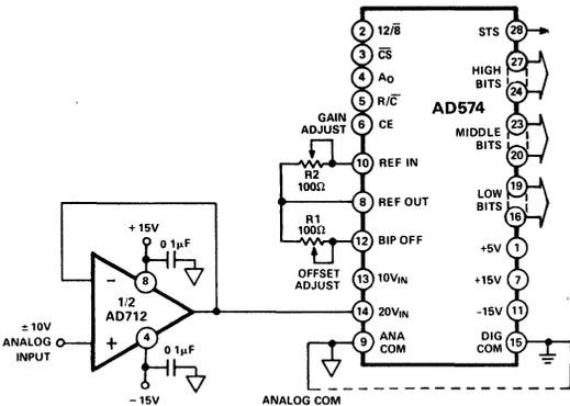
Figure 34. AD712 as ADC Unity Gain Buffer
