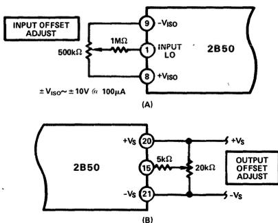
Figure 4. (A) Input and (B) Output Offset Adjustment
