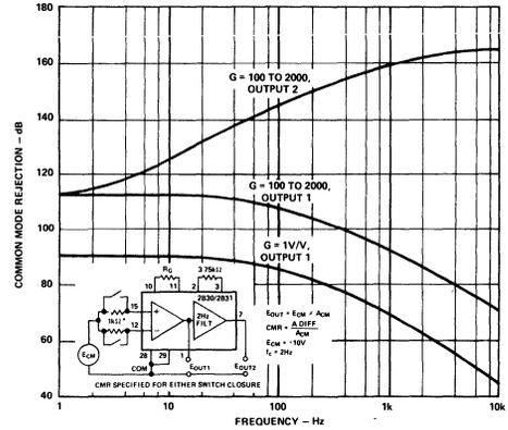
Figure 11. Common-Mode Rejection vs. Frequency and Gain
