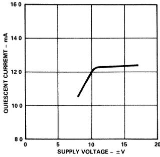
Figure 1. AD365 Quiescent Current vs. Supply Voltage
