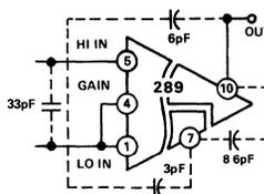
Figure 3. Model 289 Terminal Capacitance
