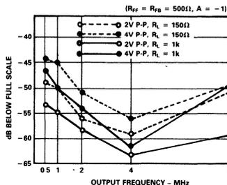
Figure 5. Harmonic Distortion - Inverting
