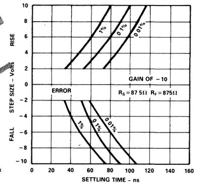
Figure 31. Settling Time vs. Step Size
