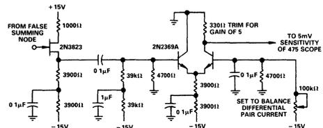
Figure 7. Settling Time Test Circuit for 0.01% Settling
