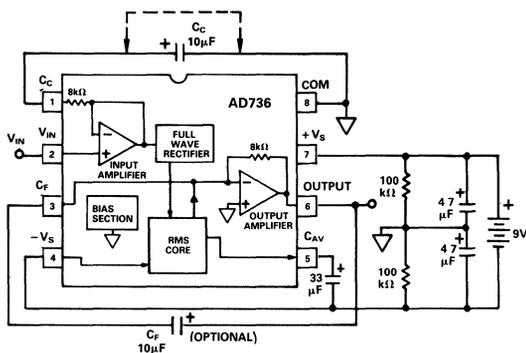
Figure 4. Connection for Battery Powered Operation.
