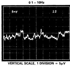
Figure 17. Low Frequency Noise -  $G = 1$  (System Gain = 1000)
