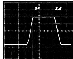
Figure 28. Transient Response  $R_L = 2k\Omega$   $C_L = 500pF$ –AD544
