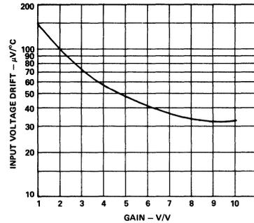
Figure 9. Input Offset Voltage Drift vs. Gain
