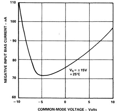
Figure 9. Negative Input Bias Current vs. Common-Mode Voltage
