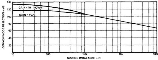
Figure 7. Typical 289 Common Mode Rejection vs. Source Impedance
