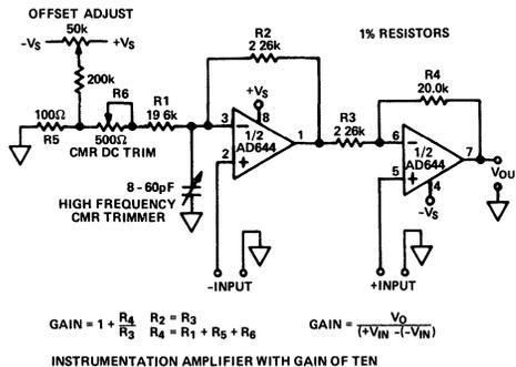
$$\text{GAIN} = 1 + \frac{R_4}{R_3} \quad R_2 = R_3 \quad R_4 = R_1 + R_5 + R_6$$
