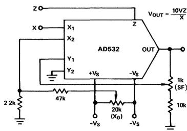
Figure 13. Divider Connection
