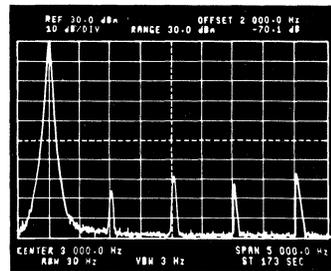
Figure 18. Spectrum of Cosine Output at 1kHz
