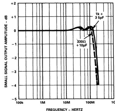
Figure 20. Response of the (Figure 17) Inverter Circuit With an  $R_{LAG}$  and  $C_{LAG}$  Compensation Network Employed
