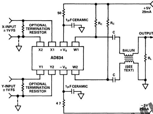
Figure 5. Using a Balun at the Output
