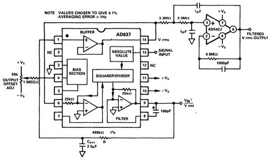
Figure 15. AD637 as a Low Frequency rms Converter
