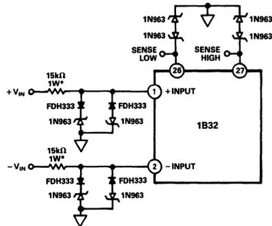
\*30kΩ 2W RESISTORS FOR 240V INPUT PROTECTION
