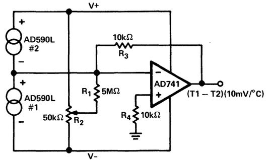
Figure 12. Differential Measurements
