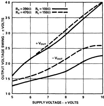
Figure 1. Output Voltage Swing vs. Supply Voltage
