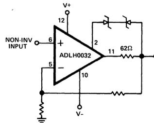
Figure 2. Output Short Circuit Protection
