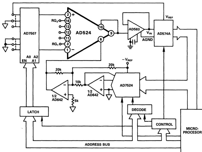
Figure 48. Microprocessor Controlled Data Acquisition System
