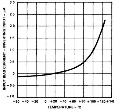
Figure 11. Negative Input Bias Current vs. Temperature
