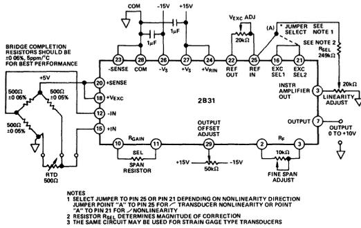
Figure 9. Transducer Nonlinearity Correction
