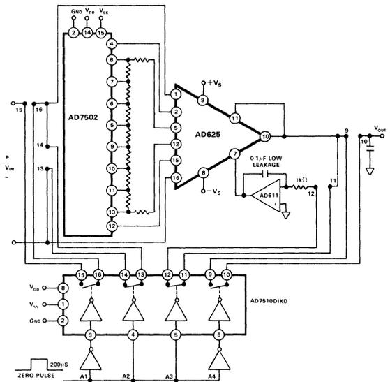
Figure 36. Auto-Zero Circuit
