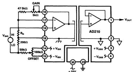
Figure 5. Adjustments for Noninverting Input
