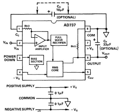
Figure 2. AD737 Average Responding Circuit
