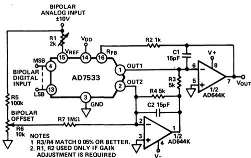
Figure 27a. AD644 Used as DAC Output Amplifiers
