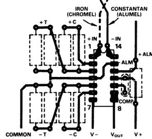
Figure 3. PCB Connections
