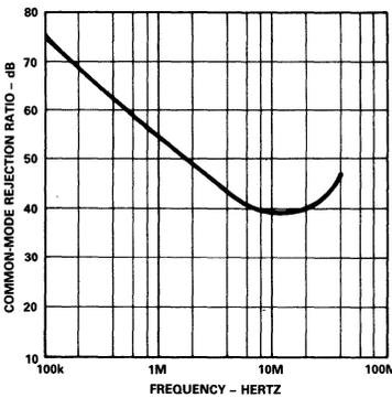
Figure 7. Common-Mode Rejection Ratio vs. Frequency
