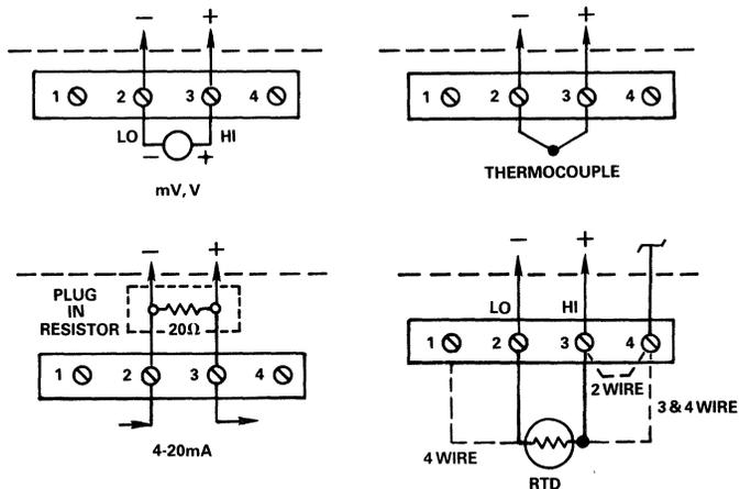
Figure 3. 5B Series Input Connections
