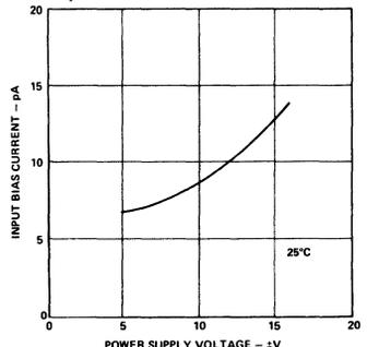
Figure 7. Input Bias Current vs. Supply Voltage
