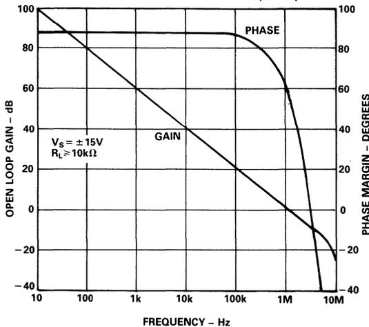
Figure 5. Open Loop Frequency Response
