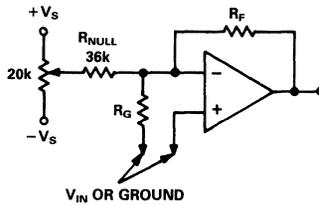
$$\text{OUTPUT NULL RANGE} \cong +V_S \left( \frac{R_F}{R_{\text{NULL}}} \right) \text{ TO } -V_S \left( \frac{R_F}{R_{\text{NULL}}} \right)$$
