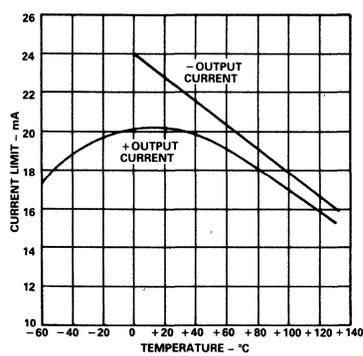
Figure 8. Short Circuit Current Limit vs. Temperature
