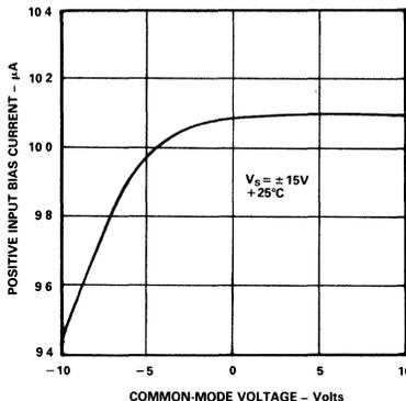
Figure 8. Positive Input Bias Current vs. Common-Mode Voltage
