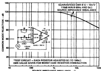
Figure 7. Common Mode Rejection vs. Source Impedance Imbalance
