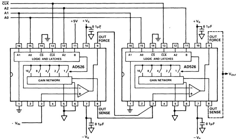
Figure 38. Cascaded Operation
