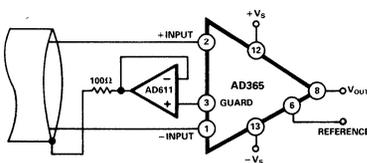
Figure 17. Common-Mode Shield Driver
