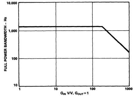
Figure 10. Typical AD295 - Full Power Bandwidth vs. Gain
