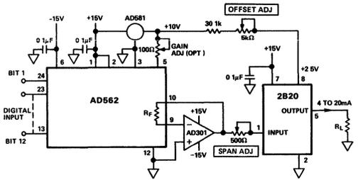
Figure 7. 12-Bit - 4 to 20mA Current Loop Interface
