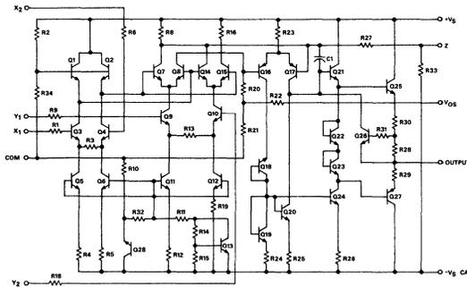
Figure 2. AD532 Schematic Diagram
