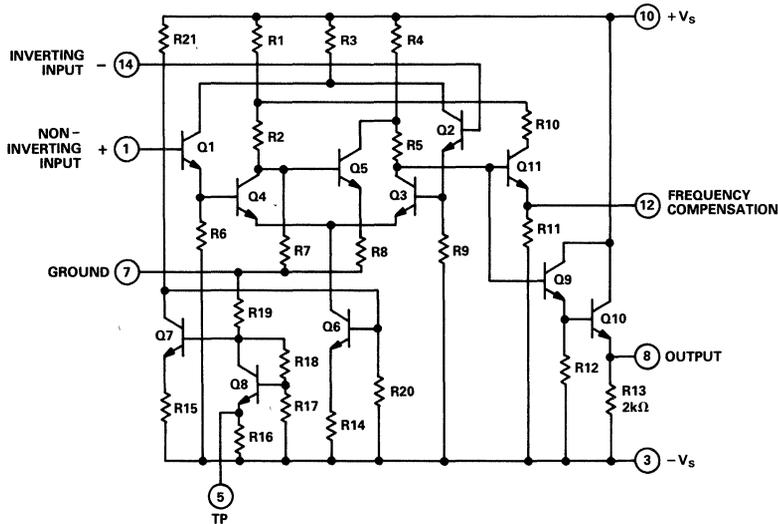
Figure 12. AD5539 Circuit
