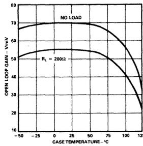
Figure 8. Gain vs. Temperature
