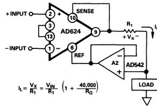
Figure 37. Voltage-to-Current Converter
