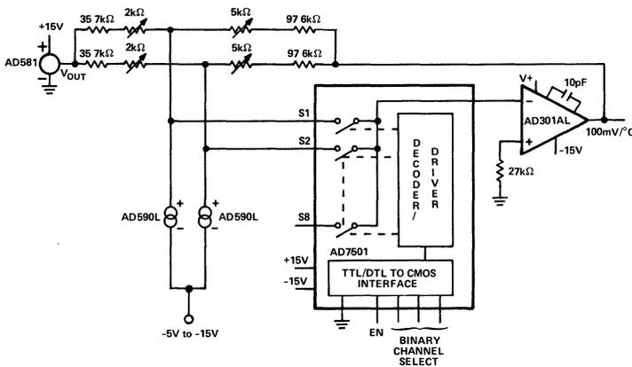
Figure 19. 8-Channel Multiplexer
