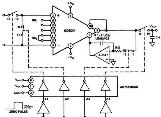
Figure 45. Auto-Zero Circuit
