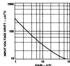
Figure 11. Input Offset Voltage Drift vs. Gain
