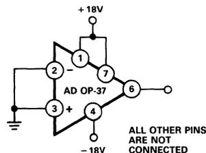
Figure 2. Burn-In Circuit
