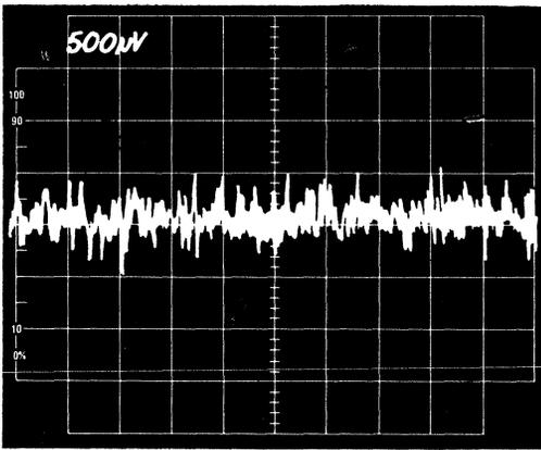
Figure 9. Voltage Noise, 0.1Hz to 10Hz,  $G = 1000$
