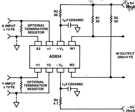
Figure 3. Basic Connections for Wideband Operation
