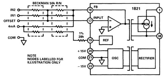
Figure 4. Low Tempco Resistor Network Configuration
