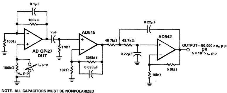
NOTE. ALL CAPACITORS MUST BE NONPOLARIZED
