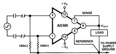
Figure 19b. Ground Returns for Bias Currents with ac Coupled Inputs
