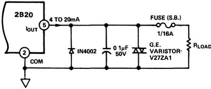
Figure 5. Output Protection Circuitry Connections
