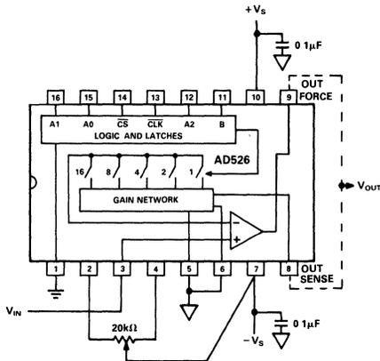
Figure 39. Offset Voltage Null Circuit
