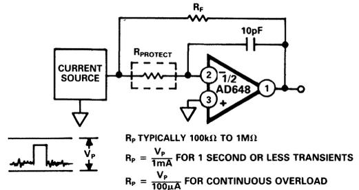
Figure 23a. Input Protection of I-to-V Converter
