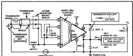
NOTE 1 GAIN RESISTOR,  $R_1$ , 1% 50ppm/°C METAL FILM TYPE IS RECOMMENDED FOR GAIN = 1V/V. LEAVE TERMINAL 2 OPEN FOR GAIN = 10V/V. SHORT TERMINAL 2 TO TERMINAL 1
