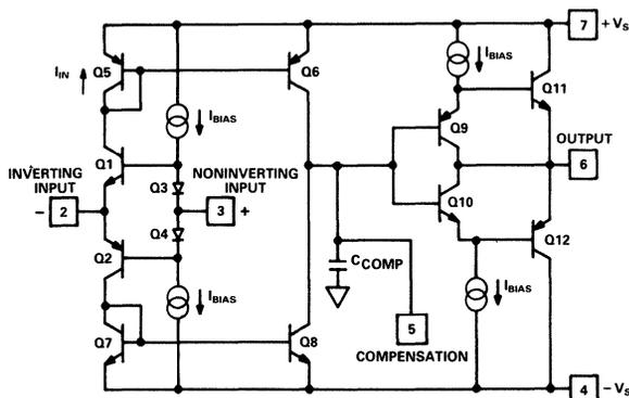
Figure 36. AD846 Simplified Schematic
