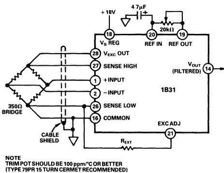
Figure 5. Constant Voltage Excitation: +10V to +15V Range
