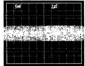
Figure 12. Wideband Output Noise,  $G = 16$  (Amplified by 10)
