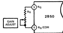
Figure 3. Gain Adjustment
