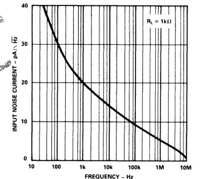
Figure 15. Input Noise Current Spectral Density
