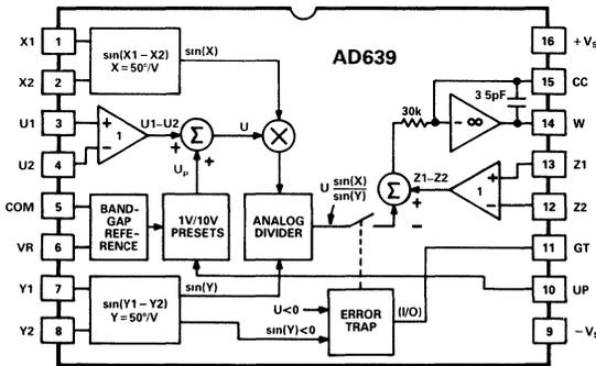
Figure 1. Equivalent Block Schematic of the AD639
