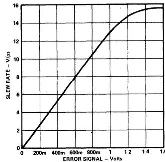
Figure 18. Slew Rate vs. Error Signal
