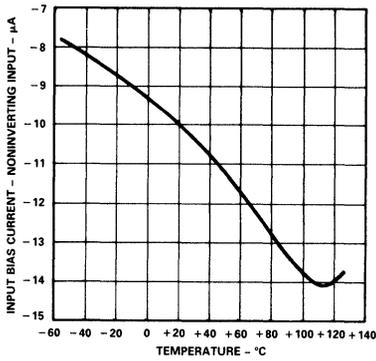
Figure 10. Positive Input Bias Current vs. Temperature
