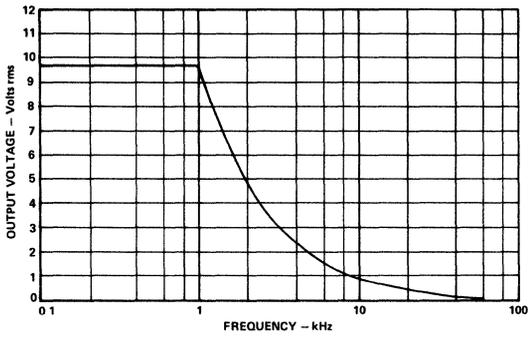
Maximum Undistorted Output vs. Frequency (Distortion  $\leq 1\%$ )
