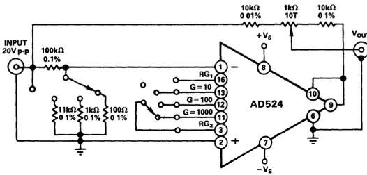
Figure 27. Settling Time Test Circuit
