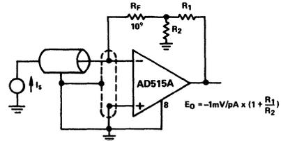
Figure 13. Picoampere to Voltage Converter with Gain
