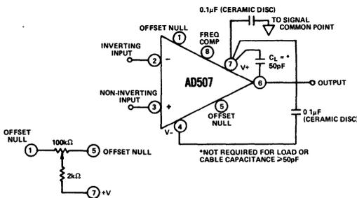
Figure 1. General Purpose Configuration to Closed Loop Gain > 10
