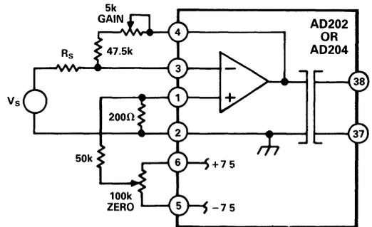
Figure 8b. Adjustments for Summing or Current Input
