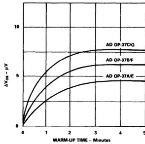
Input Offset Voltage Turn-On Drift vs. Time
