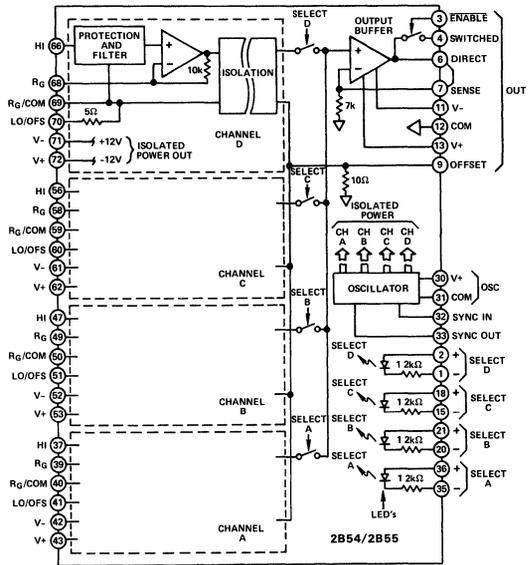
capacitor multiplexers in conditioning any thermocouple type. When cold junction compensation is required in measurement of temperature with thermocouples, the 2B54 may be used directly with the model 2B56 Universal Cold Junction Compensator.
