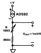
Figure 4. Basic Voltage Output (Single Temperature Trim)
