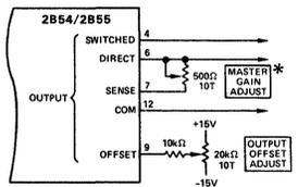
\* TO PRESERVE GAIN STABILITY THE OUTPUT GAIN ADJUSTMENT RANGE SHOULD NOT BE MORE THAN 10%
