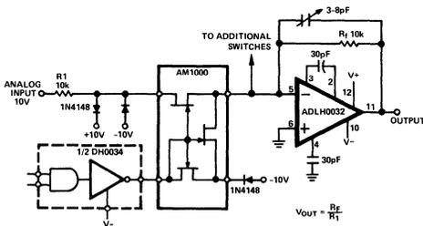
Figure 3. Current Mode Multiplexer
