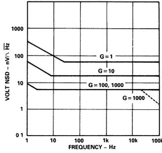
Figure 2. PGA RTI Noise Spectral Density vs. Gain
