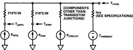
$$P_{CIRCUIT} = I_{CC} [ +V_{CC} - (-V_{CC}) ] \text{ WHERE } I_{CC} = 21\text{mA } (\text{at } \pm 15\text{V})$$
