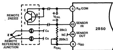
Figure 6. Remote Reference Junction Sensing
