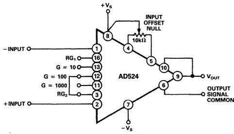
Figure 30. Operating Connections for  $G = 100$
