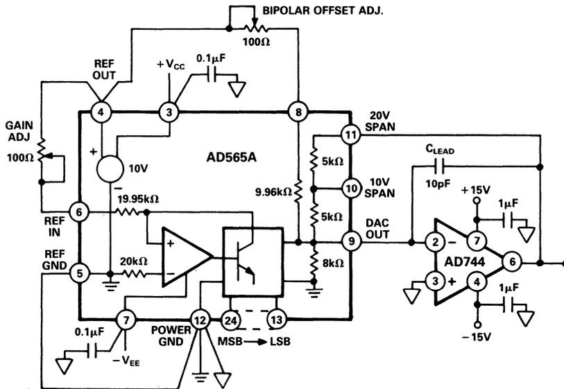
Figure 34.  $\pm 10V$  Voltage Output Bipolar DAC Using the AD744 as an Output Buffer
