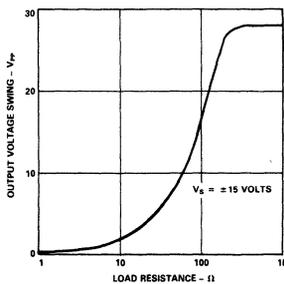
Figure 20. Output Voltage Swing vs. Load Resistance
