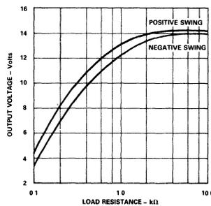
Output Swing vs. Resistive Load
