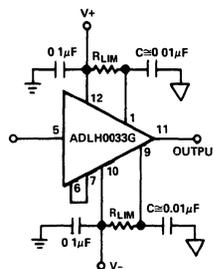
Figure 2. Short Circuit Protection Using Current Limiting Resistors ( $R_{LIM}$ )
