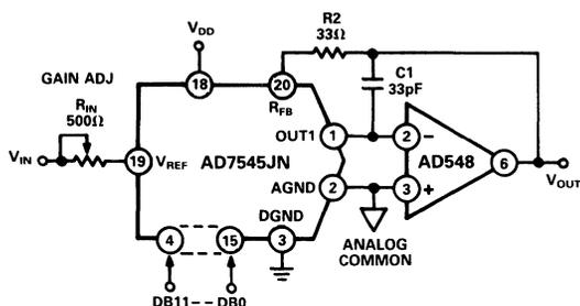
Figure 24. AD548 Used as DAC Output Amplifier
