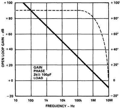
Figure 10. Open Loop Gain and Phase vs. Frequency
