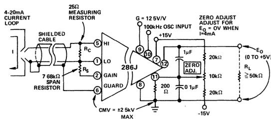
Figure 19. Isolated Analog Interface; 4 to 20mA is Converted to 0 to +5V at the Output, with Up to  $\pm 2500V$  of Isolation
