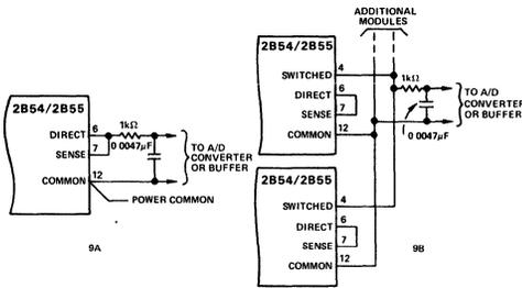
Figure 9. Output Filtering
