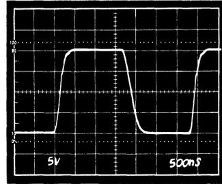
Figure 37. The Pulse Response of the 3 Op Amp Instrumentation Amplifier. Gain = 1, Horizontal Scale: 0.5μs/div, Vertical Scale: 5V/div. (Gain = 10)
