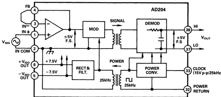
Figure 1b. AD204 Functional Block Diagram
