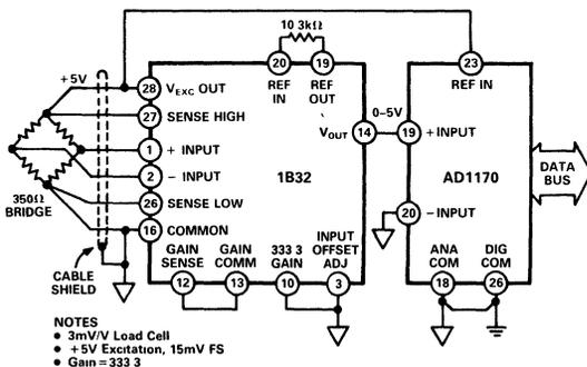
Figure 15. Auto-Calibrating Data Acquisition Using 1B32 and AD1170
