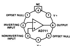
NOTE: PIN 4 CONNECTED TO CASE
