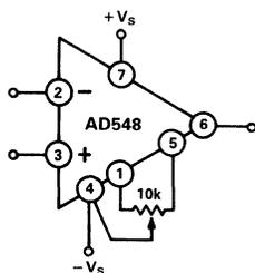
Figure 21. Offset Null Configuration
