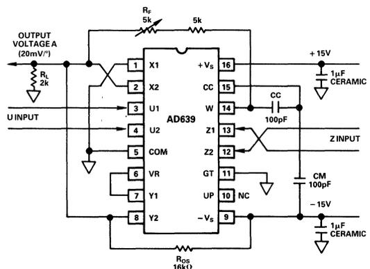
Figure 9. Connections for the General Arctangent Mode
