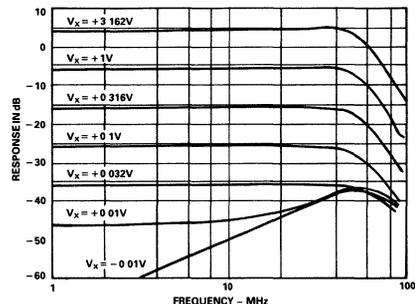
Figure 9a. AC Response of the VCA at Different Gains  $V_Y = 0.5\text{V RMS}$
