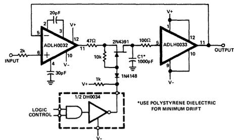
Figure 5. High Speed Sample and Hold
