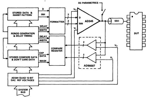
Figure 5. High-Speed Digital Test System Block Diagram
