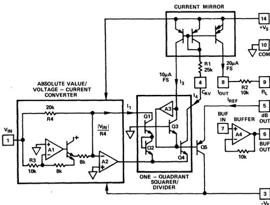
Figure 9. Simplified Schematic
