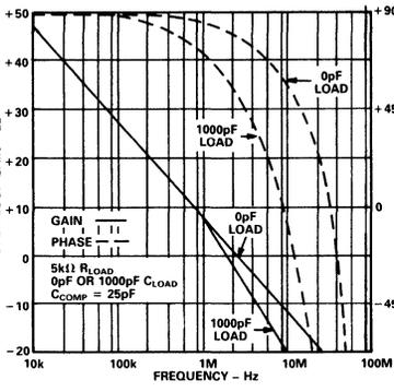
Figure 11. Open Loop Gain and Phase vs. Frequency  $C_{COMP} = 25pF$
