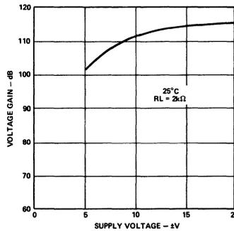
Figure 11. Open Loop Voltage Gain vs. Supply Voltage
