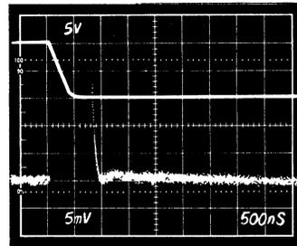
Figure 28b. Settling Characteristics 0 to -10V Step
