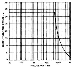
Figure 14. Large Signal Frequency Response
