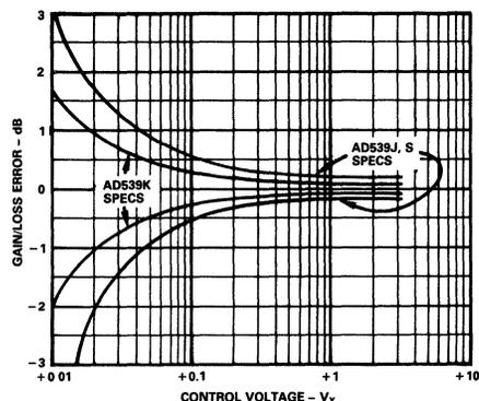
Figure 3a. Maximum ac Gain Error Boundaries
