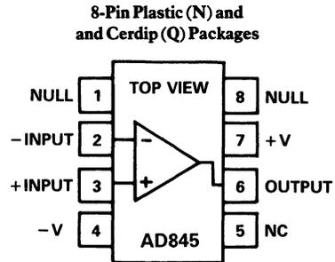
NOTE: PIN 4 CONNECTED TO CASE
