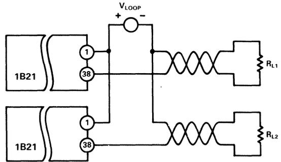
Figure 5. Multiple 1B21s with Single Loop Supply
