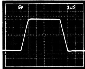
Figure 37. Transient Response  $R_L = 2k\Omega$ ,  $C_L = 500\text{pF}$
