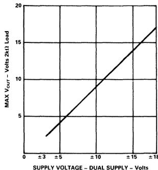
Figure 3. AD637 max  $V_{\text{OUT}}$  vs. Supply Voltage
