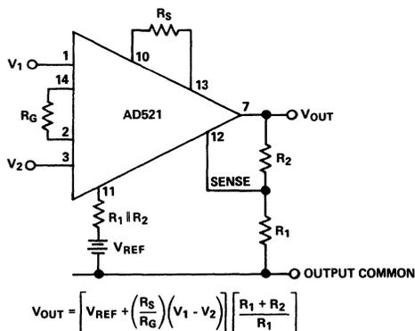
Figure 6. Circuit for utilizing some of the unique features of the AD521. Note that gain changes introduced by changing  $R_1$  and  $R_2$  will have a minimum effect on output offset if the offset is carefully nulled at the highest gain setting.
