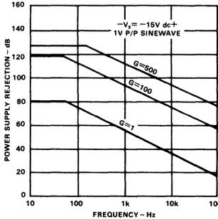
Figure 8. Negative PSRR vs. Frequency
