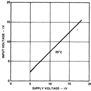
Figure 1. Input Voltage Range vs. Supply Voltage,  $G = 1$
