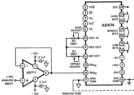
Figure 34. AD711 as ADC Unity Gain Buffer
