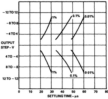
Figure 25. Settling Time Gain = 1000
