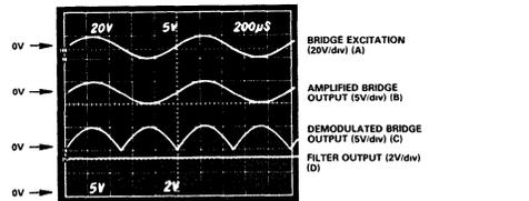
Figure 46. AC Bridge Waveforms
