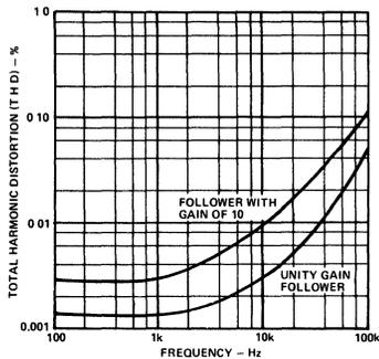
Figure 16. AD544 Total Harmonic Distortion vs. Frequency
