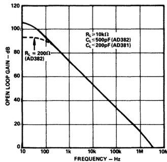
Figure 14. Open Loop Gain vs. Frequency
