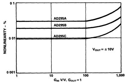
Figure 12. Typical AD295 - Gain Nonlinearity vs. Gain
