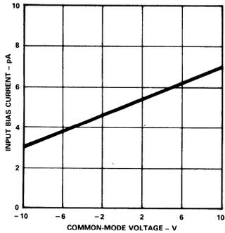
Figure 7. Input Bias Current vs. Common-Mode Voltage
