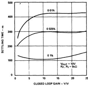
Figure 7. Settling Time vs. Closed Loop Gain
