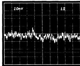
Figure 17. Low Frequency Voltage Noise -  $G = 1000$  (System Gain = 100,000)
