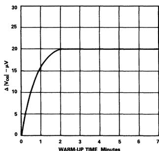
Figure 8. Change in Offset Voltage vs. Warm-Up Time
