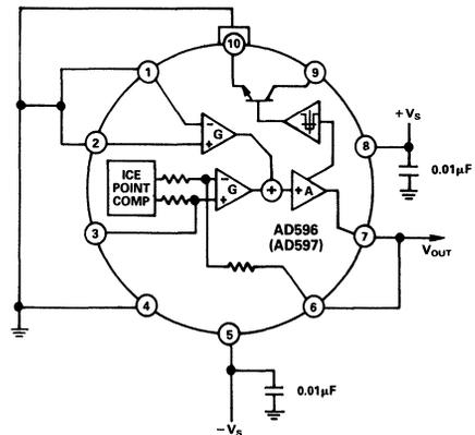
Figure 3. Stand-Alone Temperature Transducer Temperature Proportional Output Connection
