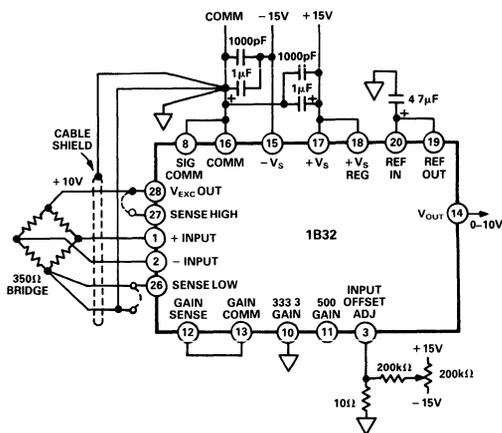
Figure 2. Internal Gain Strapping
