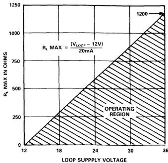
Figure 1. Maximum Load Resistance vs. Power Supply
