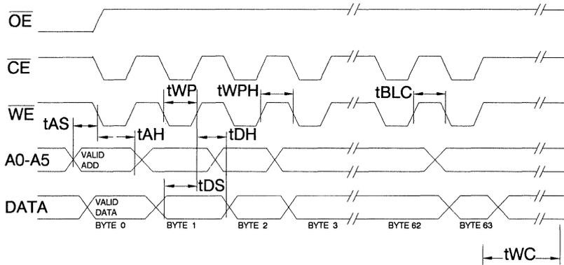
Note: A6 through A14 must specify the page address during each high to low transition of  $\overline{WE}$  (or  $\overline{CE}$ ).  $\overline{OE}$  must be high only when  $\overline{WE}$  and  $\overline{CE}$  are both low.
