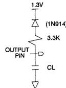
Note: C<sub>L</sub> = 100pF including jig capacitance.
