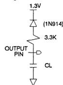
Note: C<sub>L</sub> = 100pF including jig capacitance.
