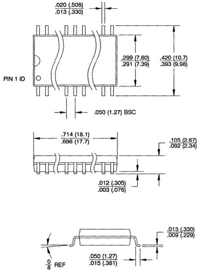
**28T, 28-Lead, 0.300" Wide, Wide Footprint Plastic Gull-Wing SOIC**
