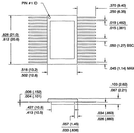
**24FW, 24-Lead, Windowed, Brazed Flat Package**
