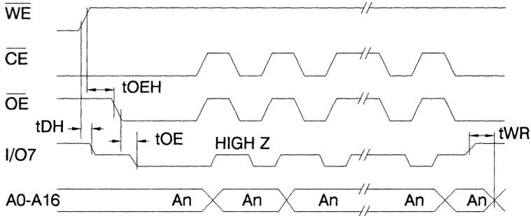
**Software Data Protection Enable Algorithm** <sup>(1)</sup>
