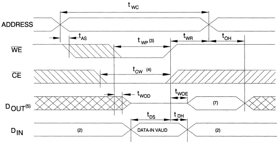
**A.C. Waveforms for Write Cycle 2 ( $\overline{\text{CE}}$  Write) <sup>(6)</sup>**
