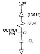
Note: C<sub>L</sub>=100pF including jig capacitance.
