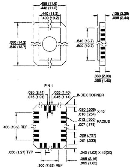
**44LW, 44-Pad, Windowed, Ceramic Leadless Chip Carrier**
