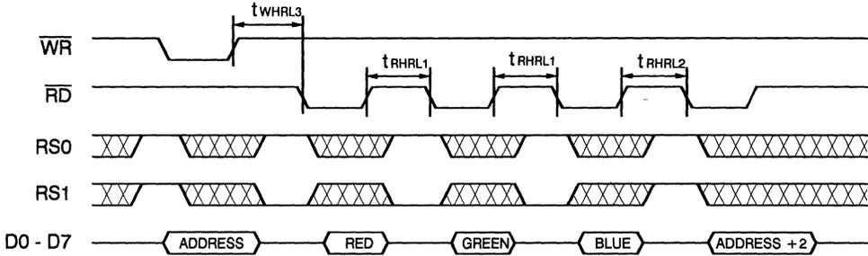
**A.C. Waveforms for Pixel Address (Write Mode) Write and Read Back**
