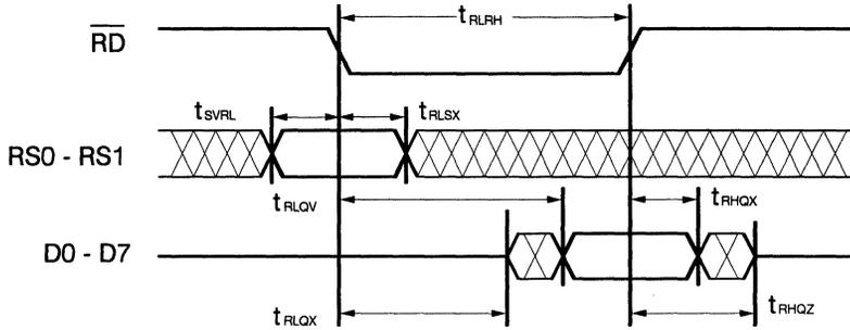
A.C. Waveforms for Color Value Write Followed by Any Write
