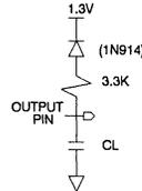
Note:  $C_L = 100\text{pF}$  including jig capacitance.
