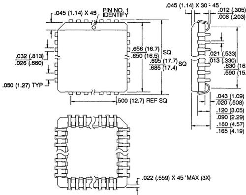
**68J, 68-Lead Plastic J-Lead Chip Carrier**
