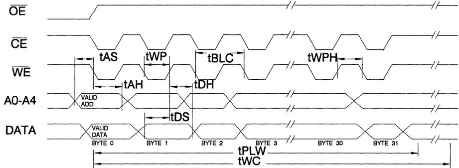
Note:  $A_5$  through  $A_{12}$  must specify the page address during each high to low transition of  $\overline{WE}$  (or  $\overline{CE}$ ).
