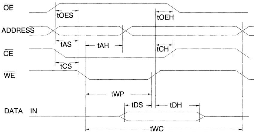
**A.C. Write Waveforms -  $\overline{CE}$  Controlled**
