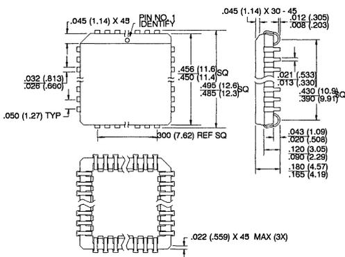
**32J, 32-Lead Plastic J-Lead Chip Carrier**
