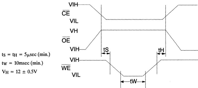
**Software Data Protection Enable Algorithm <sup>(1)</sup>**
