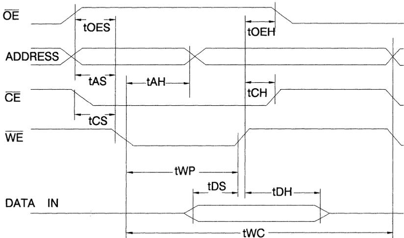
**A.C. Write Waveforms -  $\overline{CE}$  Controlled**
