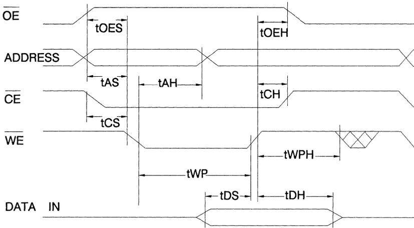
**A.C. Byte Load Waveforms -  $\overline{CE}$  Controlled**
