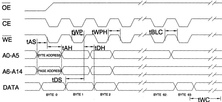
Notes: A6 through A14 must specify the page address during each high to low transition of  $\overline{WE}$  (or  $\overline{CE}$ ).
