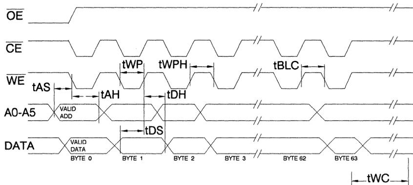
Note: A6 through A14 must specify the page address during each high to low transition of  $\overline{WE}$  (or  $\overline{CE}$ ).
