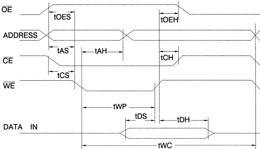
**A.C. Write Waveforms -  $\overline{CE}$  Controlled**
