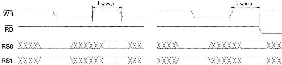
**A.C. Waveforms for Pixel Mask or Pixel Address Read**
