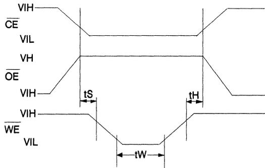
$$t_S = t_H = 1\mu\text{sec (min.)}$$
