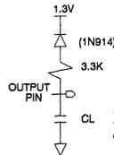
Note: C<sub>L</sub>=100pF including jig capacitance.
