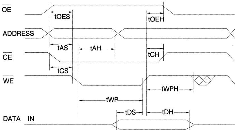
**A.C. Byte Load Waveforms -  $\overline{CE}$  Controlled**
