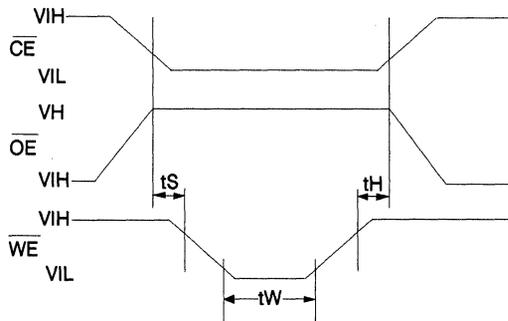
$t_S = t_H = 1\mu\text{sec (min.)}$
