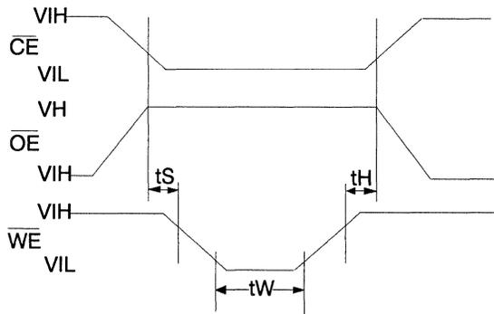
$$t_S = t_H = 1\mu\text{sec (min.)}$$
