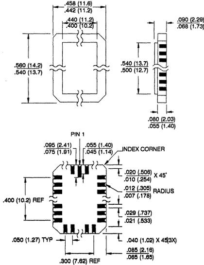
**44L, 44-Pad, Non-Windowed, Ceramic Leadless Chip Carrier**
