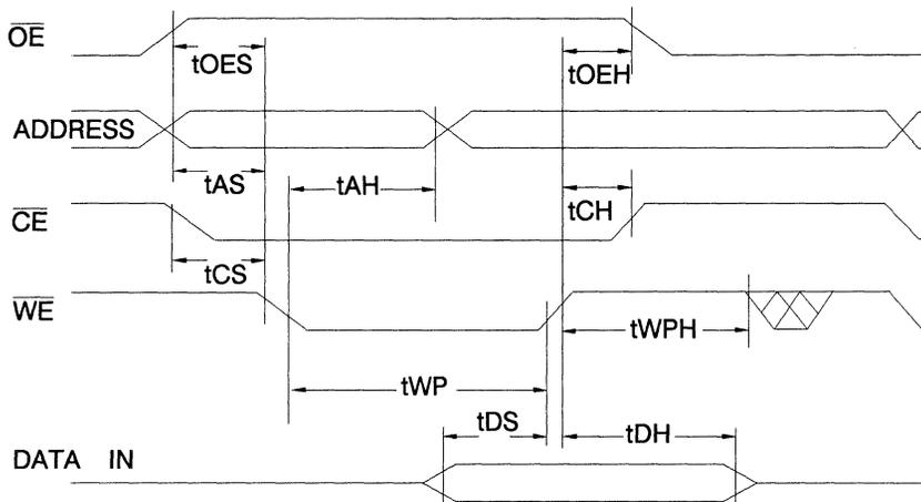
**A.C. Write Waveforms -  $\overline{CE}$  Controlled**
