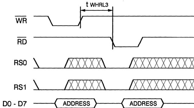
**A.C. Waveforms for Pixel Address (Read Mode) Write and Read Back**
