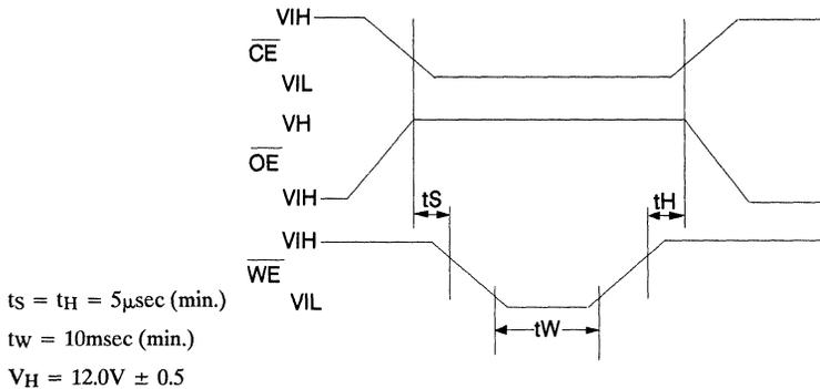
**Software Data Protection Enable Algorithm <sup>(1)</sup>**
