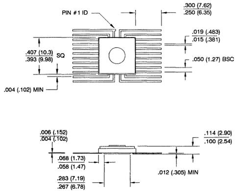
**28J, 28-Lead Plastic J-Lead Chip Carrier**
