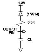
Note:  $C_L = 100\text{pF}$  including jig capacitance.
