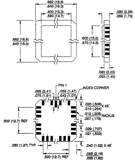
**28LW, 28-Pad, Windowed, Ceramic Leadless Chip Carrier**
