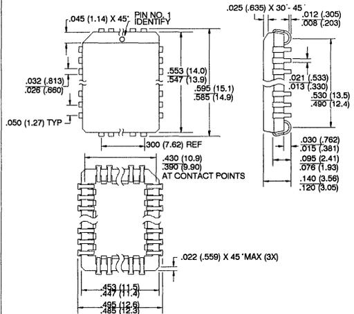
**44J, 44-Lead, Plastic J-Lead Chip Carrier**
