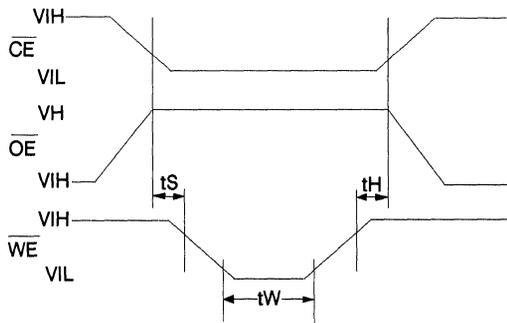
$$t_S = t_H = 1\mu\text{sec (min.)}$$
