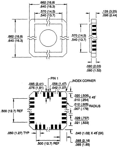
**32M, 32-Lead, Non-Windowed, 32D6 Compatible, Ceramic Module**
