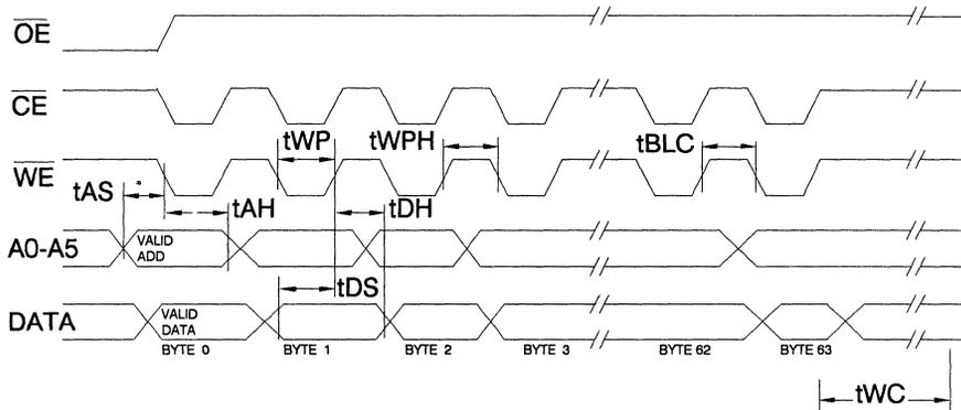
Note: A6 through A16 must specify the page address during each high to low transition of  $\overline{WE}$  (or  $\overline{CE}$ ).
