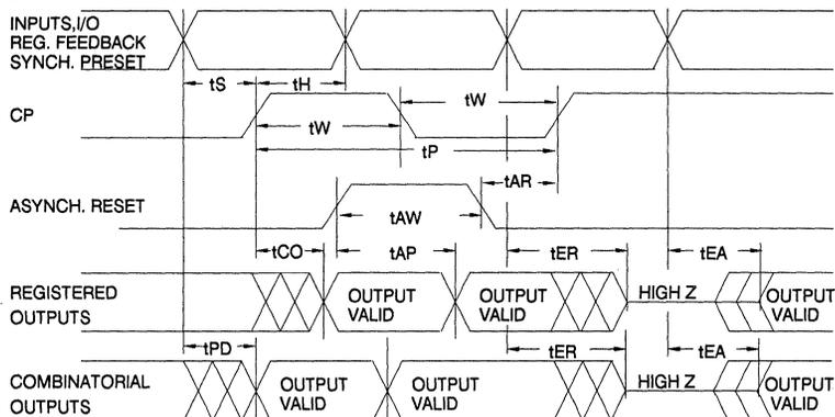
Note: 1. Timing measurement reference is 1.5V. Input AC driving levels are 0.0V and 3.0V, unless otherwise specified.
