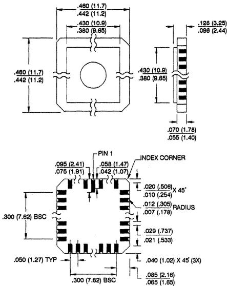
**32LW, 32-Pad, Windowed, Ceramic Leadless Chip Carrier**
