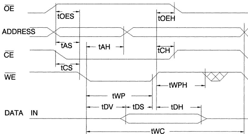
**A.C. Write Waveforms -  $\overline{CE}$  Controlled**
