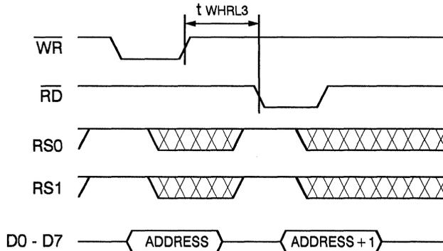
**A.C Waveforms for Pixel Mask Write Followed by Any Write or Read**
