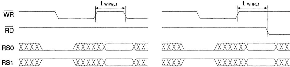
**A.C. Waveforms for Pixel Mask or Pixel Address Read Followed by Any Read or Write**
