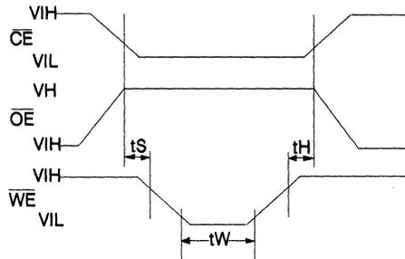
$t_S = t_H = 1\mu\text{sec (min.)}$
