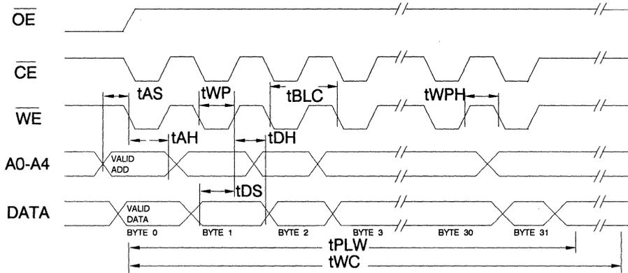
Note: A5 through A12 must specify the page address during each high to low transition of WE (or CE).
