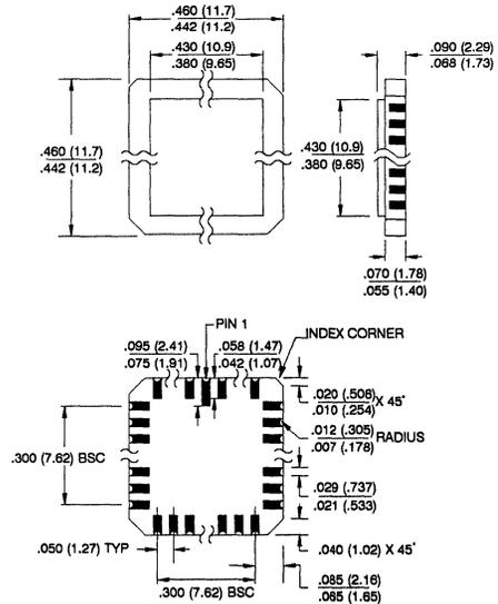
**32L, 32-Pad, Non-Windowed, Ceramic Leadless Chip Carrier**
