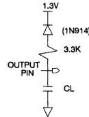
Note:  $C_L = 100\text{pF}$  including jig capacitance.
