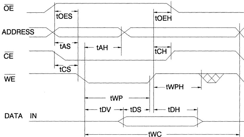
**A.C. Write Waveforms -  $\overline{CE}$  Controlled**
