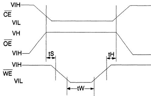
$t_S = t_H = 1\mu\text{sec (min.)}$
