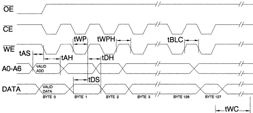
Note: A7 through A16 must specify the page address during each high to low transition of  $\overline{WE}$  (or  $\overline{CE}$ ).  $\overline{OE}$  must be high only when  $\overline{WE}$  and  $\overline{CE}$  are both low.
