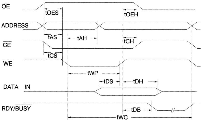
**A.C. Write Waveforms -  $\overline{CE}$  Controlled**
