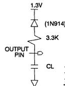
Note:  $C_L = 100\text{pF}$  including jig capacitance.
