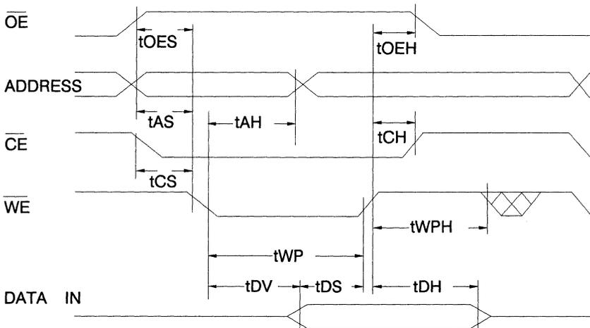
**A.C. Write Waveforms -  $\overline{CE}$  Controlled**
