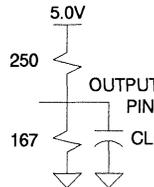
Note:  $C_L = 30\text{pF}$  including jig capacitance.
