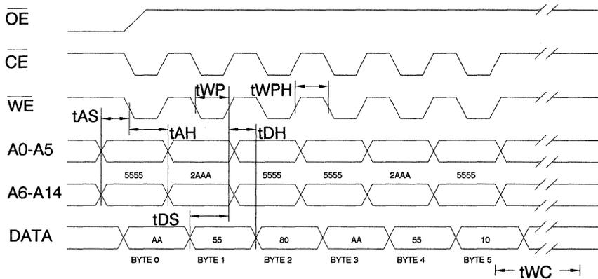
Note:  $\overline{OE}$  must be high only when  $\overline{WE}$  and  $\overline{CE}$  are both low.
