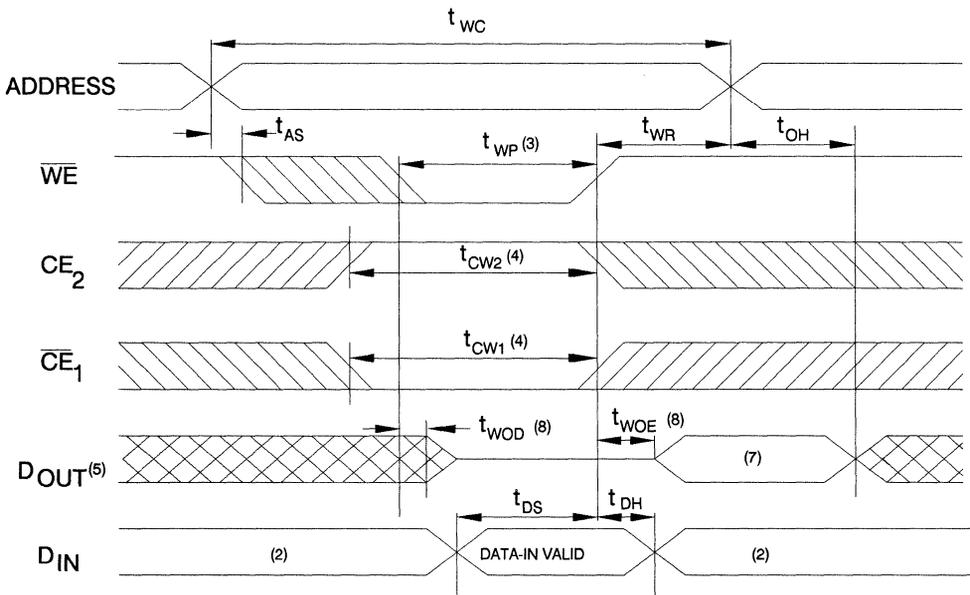
A.C. Waveforms for Write Cycle 2 ( $\overline{CE}$  Write)<sup>(6)</sup>
