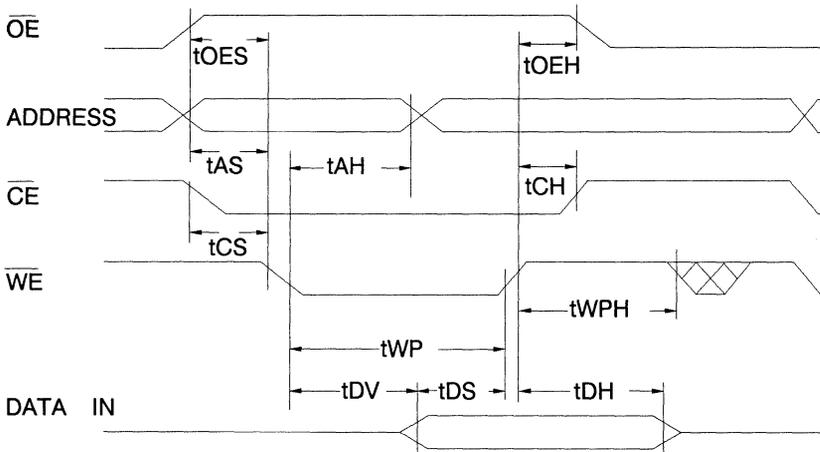
**A.C. Write Waveforms -  $\overline{CE}$  Controlled**
