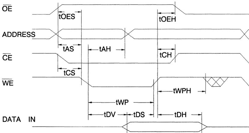
**A.C. Write Waveforms -  $\overline{CE}$  Controlled**
