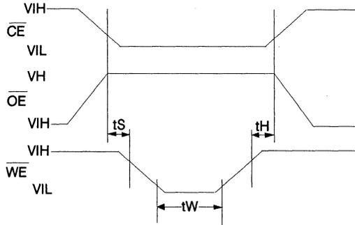
$$t_S = t_H = 1\mu\text{sec (min.)}$$
