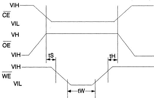
$$t_S = t_H = 1\mu\text{sec (min.)}$$
