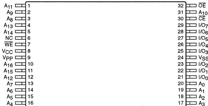
**TSOP Package (Reverse Pinout)**
