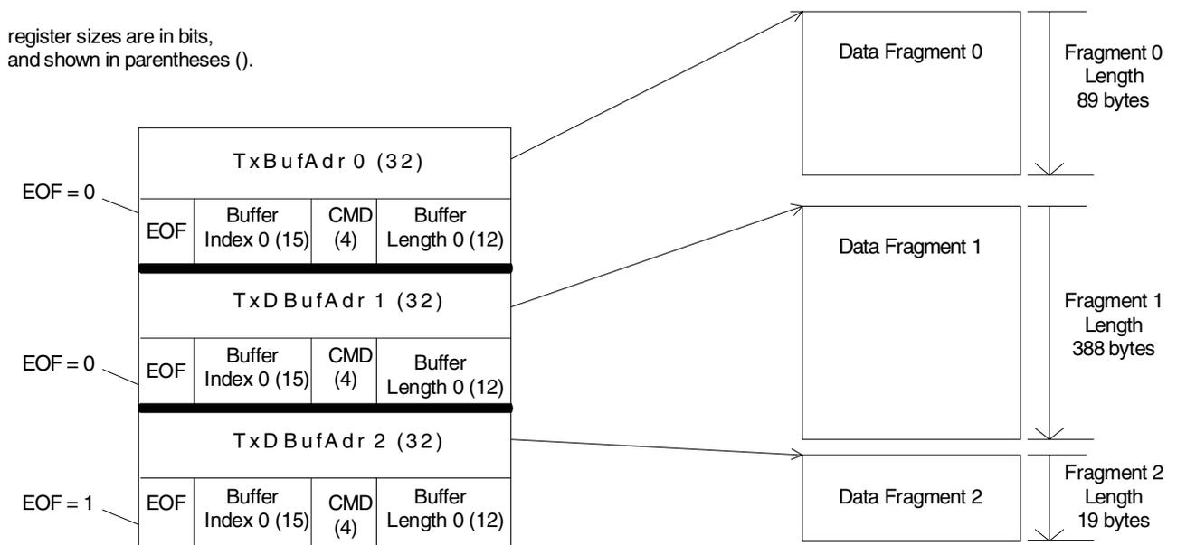
In the example shown in Figure 6-14, one frame is transmitted from three fragments. The MAC starts the frame by acquiring the medium and transmitting the preamble. Then, the fragments 0, 1, 2 are transmitted in order for a total of 446 bytes (39 + 388 + 19). Since the CRC bit in the first frame fragment is clear, the HW appends the 4 byte CRC. Thus, 4 more bytes are added to the frame for the CRC making the total frame length 450 bytes. Finally, the MAC sends the end-of-frame.
