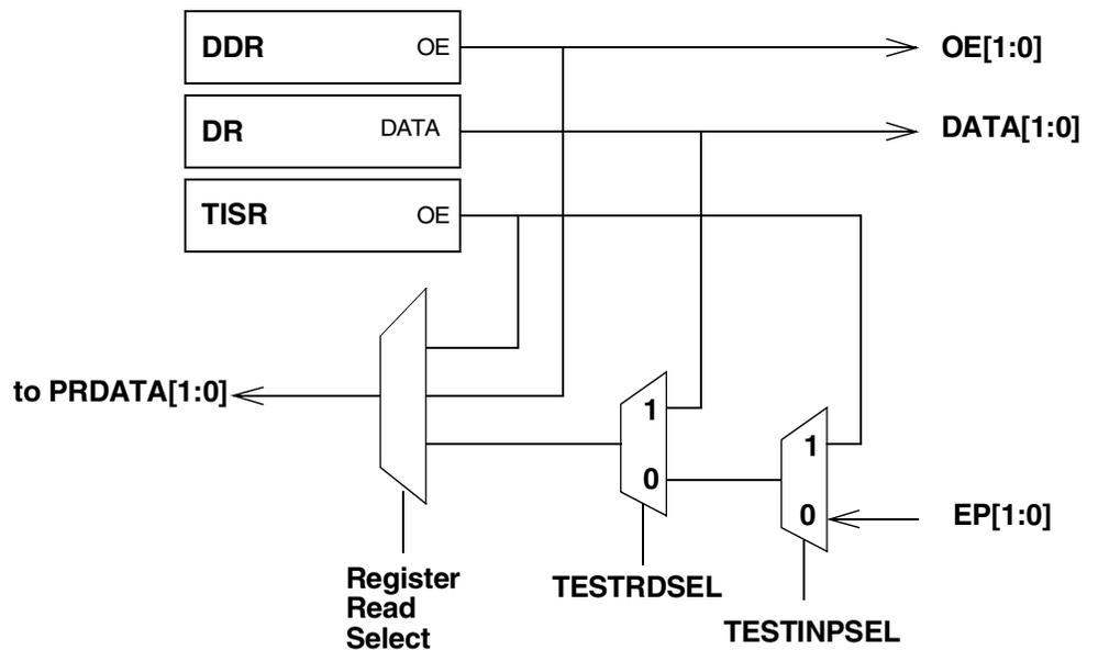
**Figure 21-4. Signal Connections Within GPIO Port G Control Logic**
