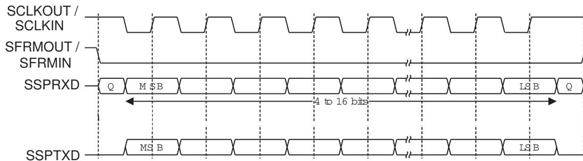
Note: Figure 19-8, Q is an undefined signal.
