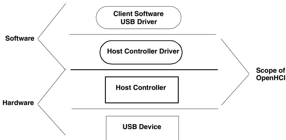
The Host Controller Driver and Host Controller work in tandem to transfer data between client software and a USB device. Data is translated from shared-memory data structures at the client software end to USB signal protocols at the USB device end, and vice-versa.
