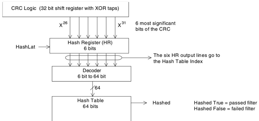
Whenever the hashed filter is passed on good frames, the output of the HR is presented on the Hash Table Index (RStatQ). A received good frame is
