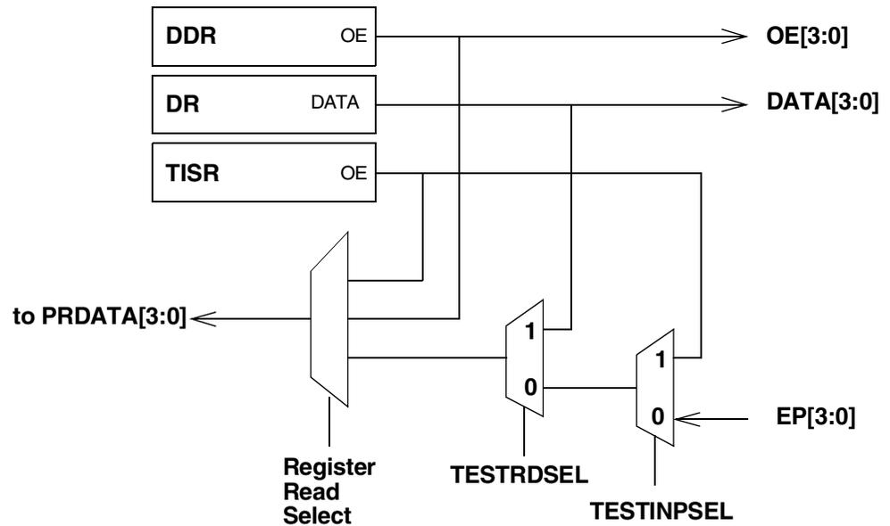
Figure 21-6. Signal Connections Within the Enhanced GPIO Port A and B Control Logic
