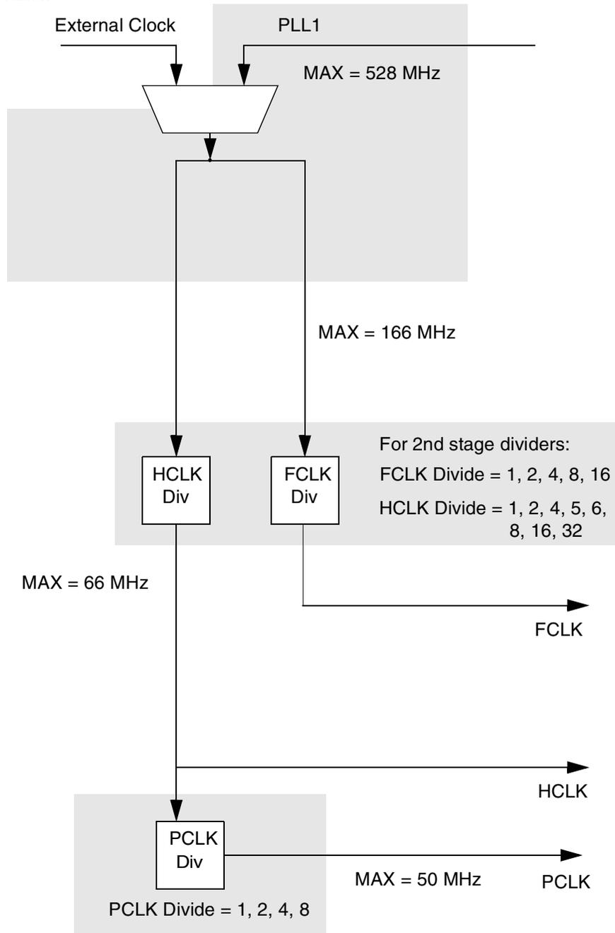
There are some limitations of each clock. FCLK must be  $\leq 166$  MHz, HCLK  $\leq 66$  MHz and PCLK  $\leq 50$  MHz and FCLK  $\geq$  HCLK  $>$  PCLK. Refer to register, “ClkSet1” on page 84, for the detailed configuration information regarding the divider bit fields.
