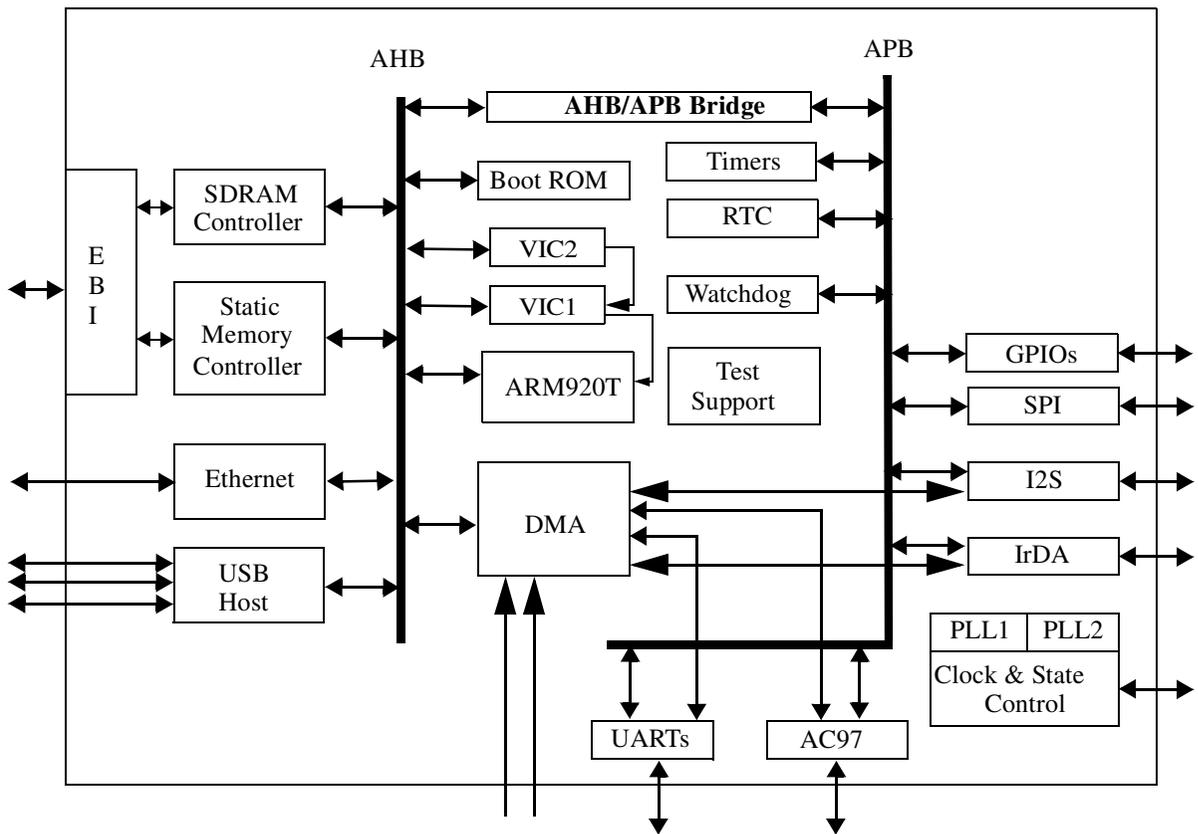
Before an AMBA-to-AHB transfer can commence, the bus master must be granted access to the bus. This process is started by the master asserting a request signal to the arbiter. Then the arbiter indicates when the master will be granted use of the bus. A granted bus master starts an AMBA-to-AHB transfer by driving the address and control signals. These signals provide information on the address, direction and width of the transfer, as well as indicating whether the transfer forms part of a burst.
