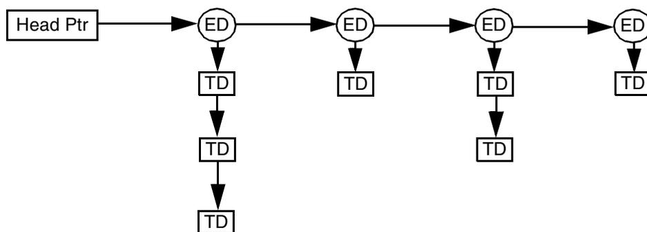
The head pointers to the bulk and control Endpoint Descriptor lists are maintained within the operational registers in the HC. The Host Controller Driver initializes these pointers prior to the Host Controller gaining access to them. Should these pointers need to be updated, the Host Controller Driver may need to halt the Host Controller from processing the specific list, update the pointer, then re-enable the HC.
