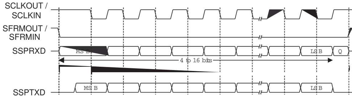
Note: In Figure 19-6, Q is an undefined signal.
