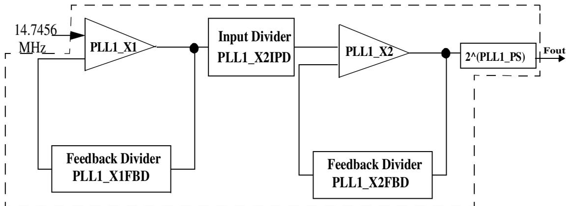
Both PLLs are software programmable (each value is defined in ClkSet1 and ClkSet2 registers respectively). The frequency of output clock  $F_{out}$  shows in the next equation:
