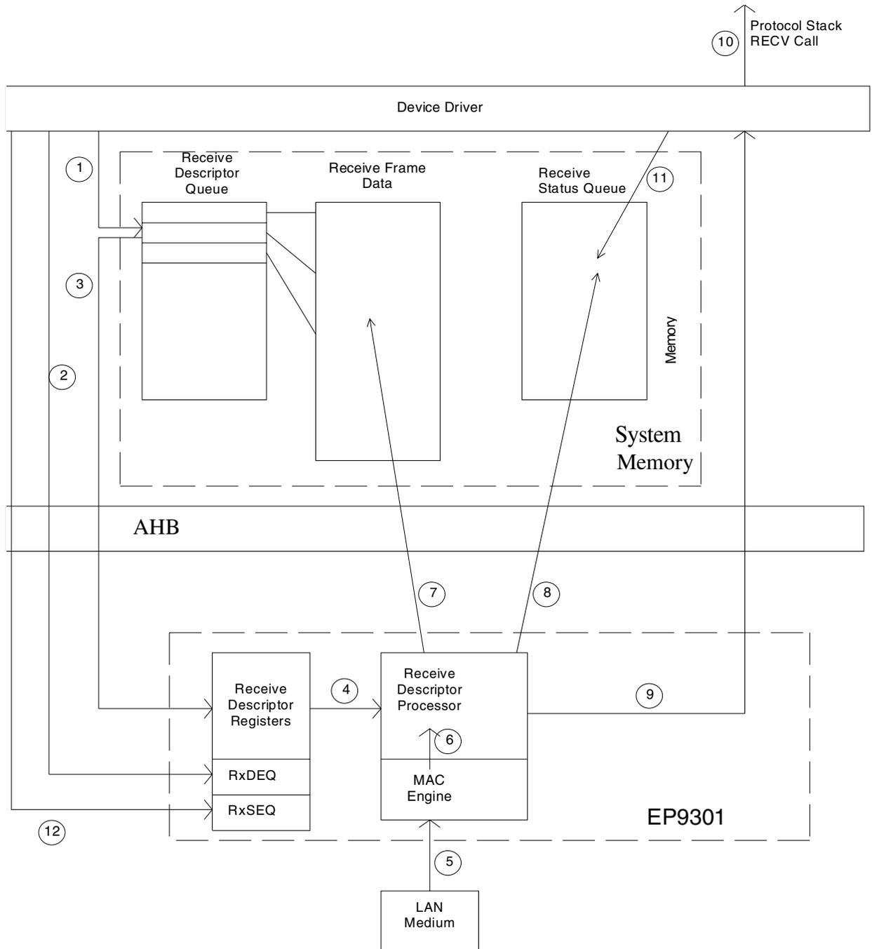
Refer to the circled numbers in Figure 6-9. The detailed receive flow is:
