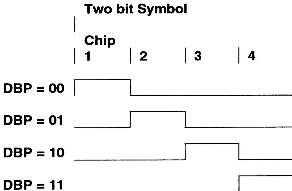
Figure 13-3. 4PPM Modulation Example
