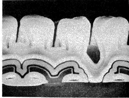
Fig. 13—SEM cross sectional view of 3D stacked capacitor cell.
