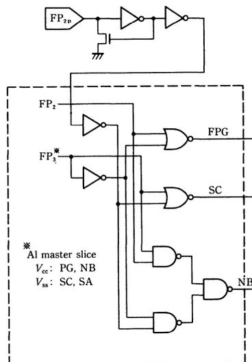
Fig. 16—Master slice/wire bond option control circuitry.
