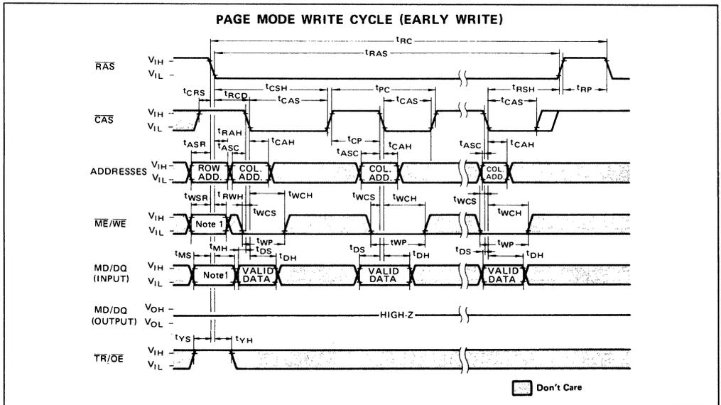
Note 1) When  $\overline{\text{ME/WE}} = \text{"H"}$ , all data on the MD/DQ can be written into the cell.
