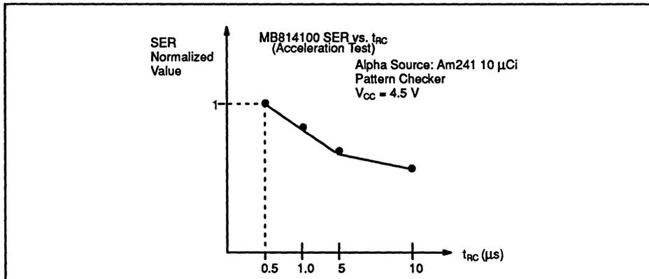
Figure 5. Soft Error Rate vs.  $t_{RC}$  (MB814100)
