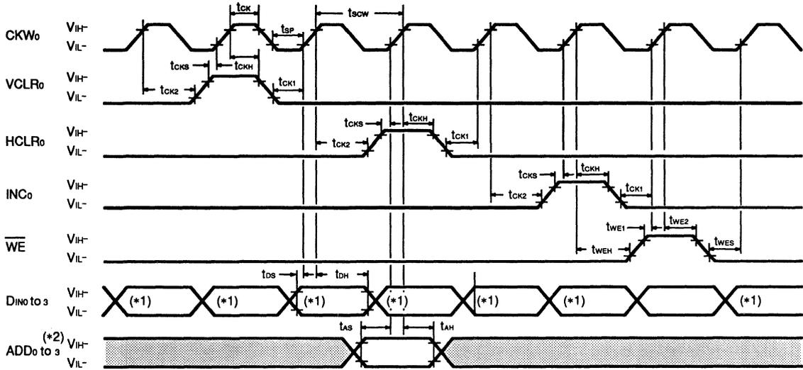
\*1 If VCLR<sub>0</sub> or HCLR<sub>0</sub> is received before the entire block (60 bits) is input, the block is canceled instead of written.
