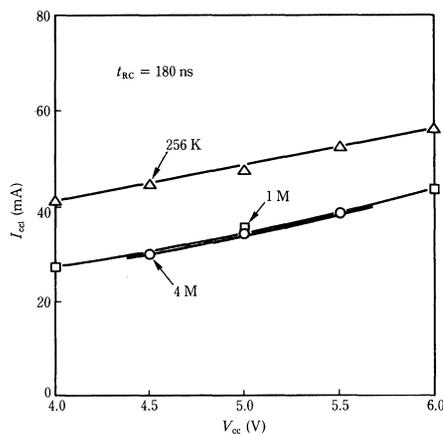
Fig. 23—Average  $V_{CC}$  current ( $I_{CC1}$ ) vs  $V_{CC}$  voltage.
