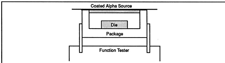
Figure 3. Alpha Source Acceleration Test
