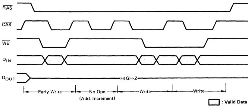
2) The case of first nibble cycle is delayed write (Read-Write)
