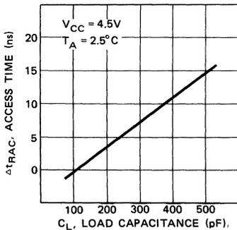
Fig. 29 – ACCESS TIME (SAM) vs LOAD CAPACITANCE
