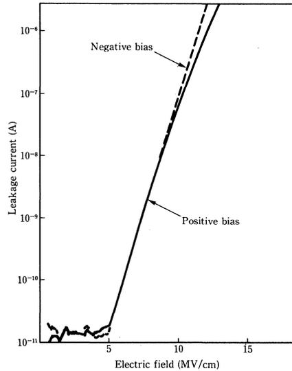
Fig. 14—Leakage current of capacitor film.
