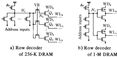
Fig. 18—Comparison of row decoder between nMOS and
