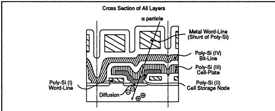
Figure 1. 4M DRAM Stacked Capacitor Cell
