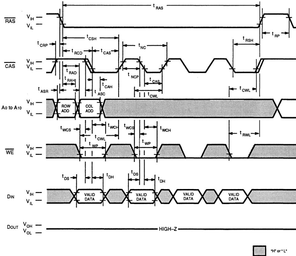
Fig. 10 –  $\overline{\text{RAS}}$ -ONLY REFRESH ( $\overline{\text{WE}}$ , DIN, A10 = "H" or "L")
