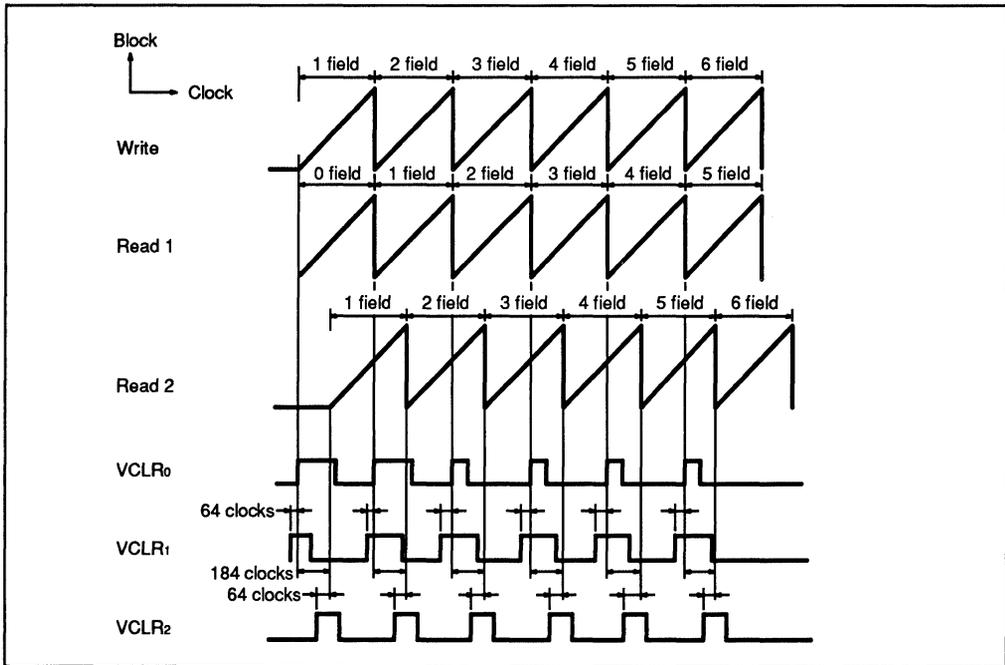
In the field memory (three ports) is used, stable output can be obtained, regardless of jitter from the write clock. In addition, the correlation between frames or lines can be calculated.
