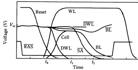
Fig. 5 - Operational waveforms of sense amplifier.
