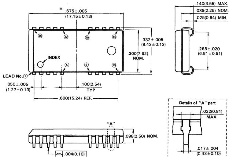
NOTE: 1. \*: This dimension includes resin protrusion. (Each side: .006(0.15) MAX)
