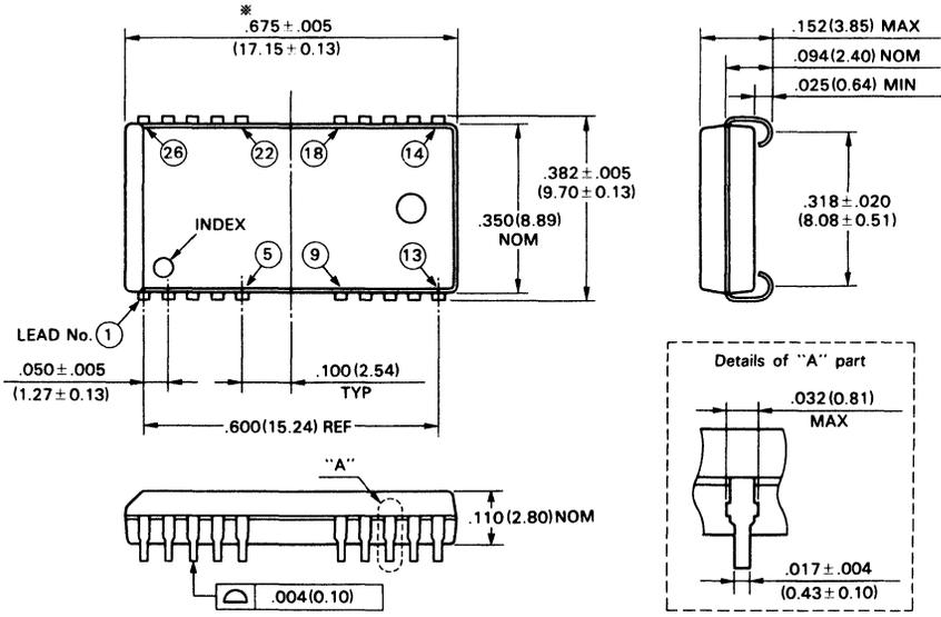
\*This dimension includes resin protrusion.(Each side:.006(0.15) MAX.)
