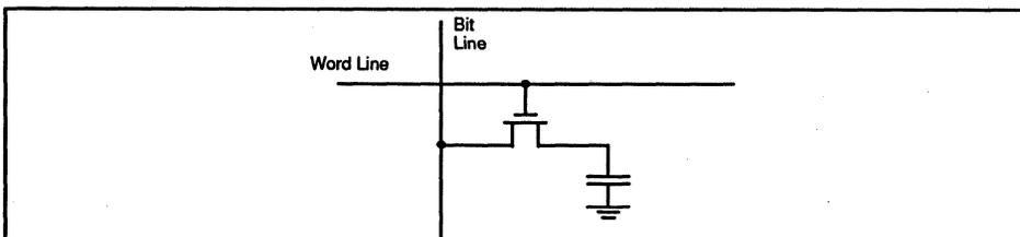
Figure 3. One Transistor (and One Capacitor) RAM Cell
