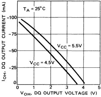
Fig. 33 – SD OUTPUT CURRENT vs SD OUTPUT VOLTAGE
