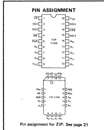
This device contains circuitry to protect the inputs against damage due to high static voltages or electric fields. However, it is advised that normal precautions be taken to avoid application of any voltage higher than maximum rated voltages to this high impedance circuit.
