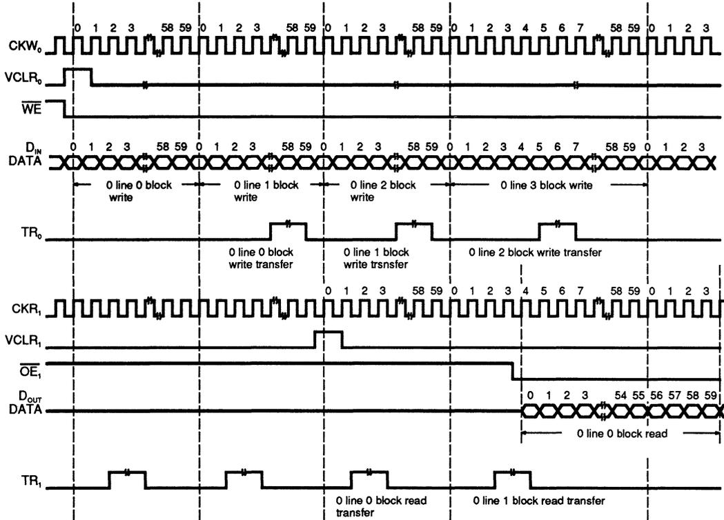
1) In order to get newly input data, it is necessary to get delay of VCLR<sub>1</sub> to VCLR<sub>0</sub> more than 120 clocks
