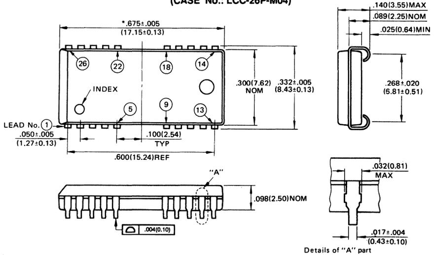
NOTE: 1. \*: This dimension includes resin protrusion. (Each side:  $.006$  (0.15) MAX)
