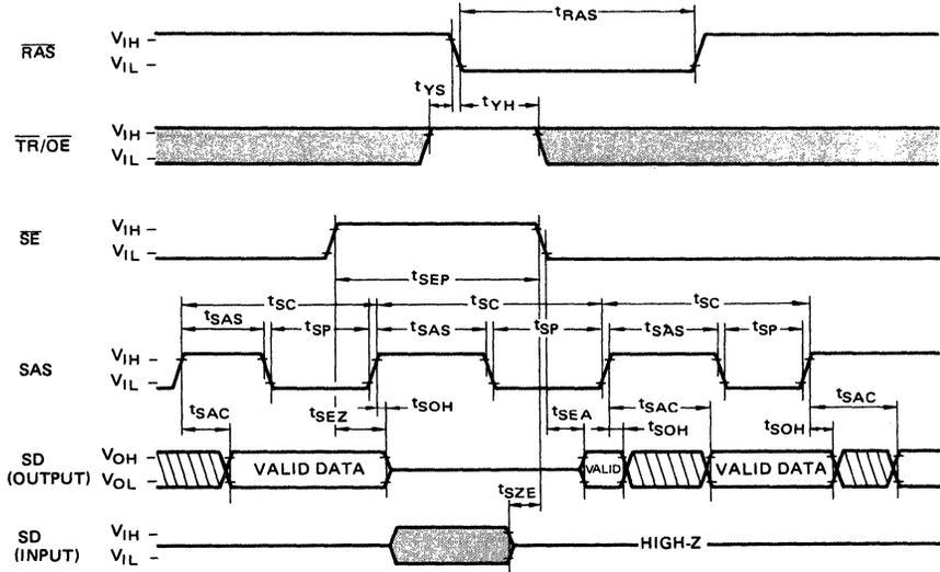
In the case of  $\overline{SE} = "L"$  while the operation;
