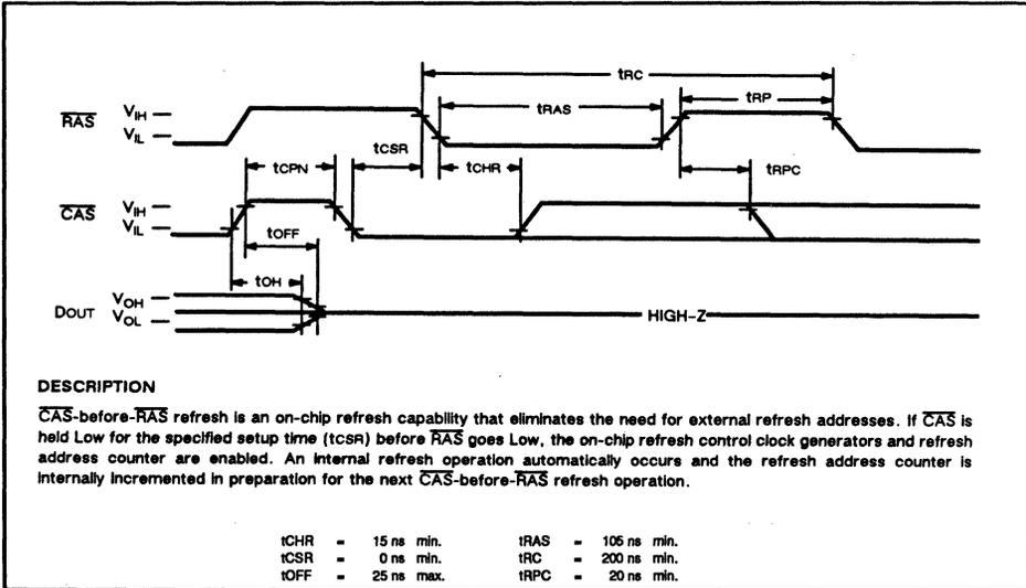
Figure 7.  $\overline{\text{CAS}}$  Before  $\overline{\text{RAS}}$  Refresh Cycle
