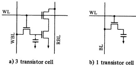
Fig. 3 - DRAM memory cell circuit.
