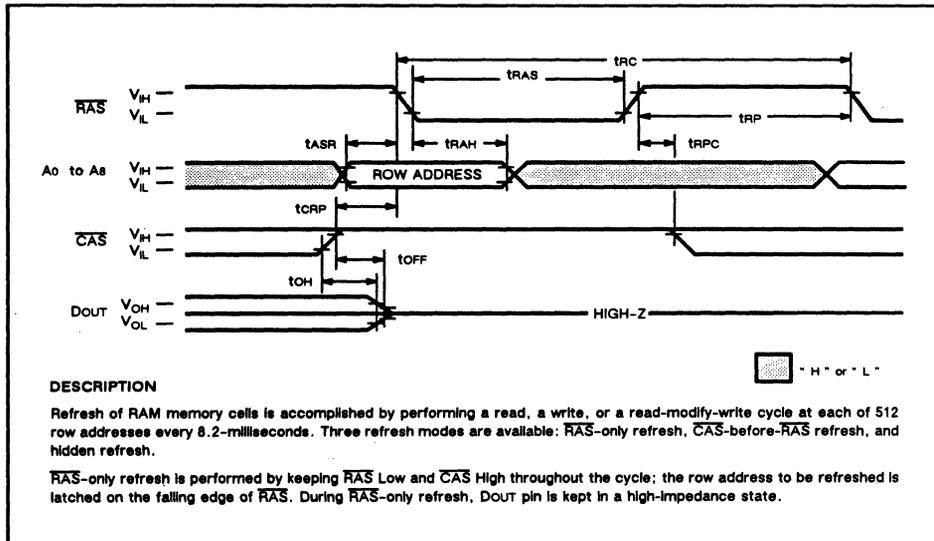
Figure 6. Typical  $\overline{\text{RAS}}$ -Only Refresh Cycle
