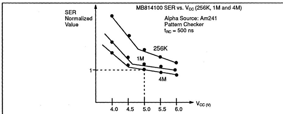
Figure 6. Relative Soft Error Rate vs. V<sub>CC</sub> (256K, 1M, 4M)
