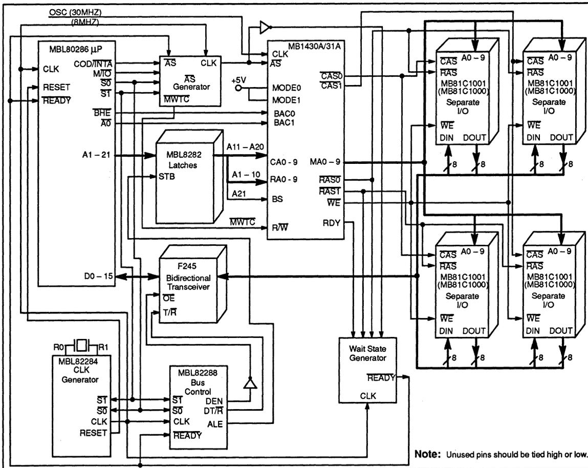
Figure 9. Schematic of 1 megabit x 32 DRAM with Zero Wait States
