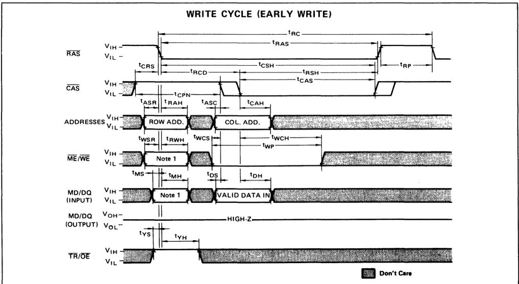
**Note 1)** When  $\overline{ME}/\overline{WE}$  = "H", all data on the MD/DQ can be written into the cell.
