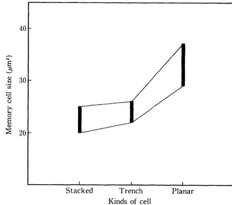
Fig. 8—Comparison of cell size for three types of cell structure.
