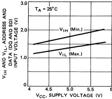
Fig. 25 – ADDRESS AND DATA (DQ AND SD) INPUT VOLTAGE vs SUPPLY VOLTAGE
