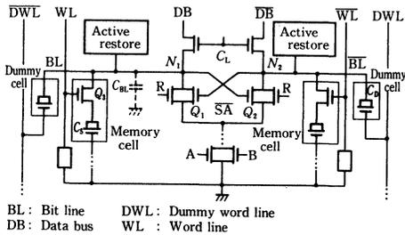
Fig. 4 - Sense amplifier circuitry of 254-K DRAM.
