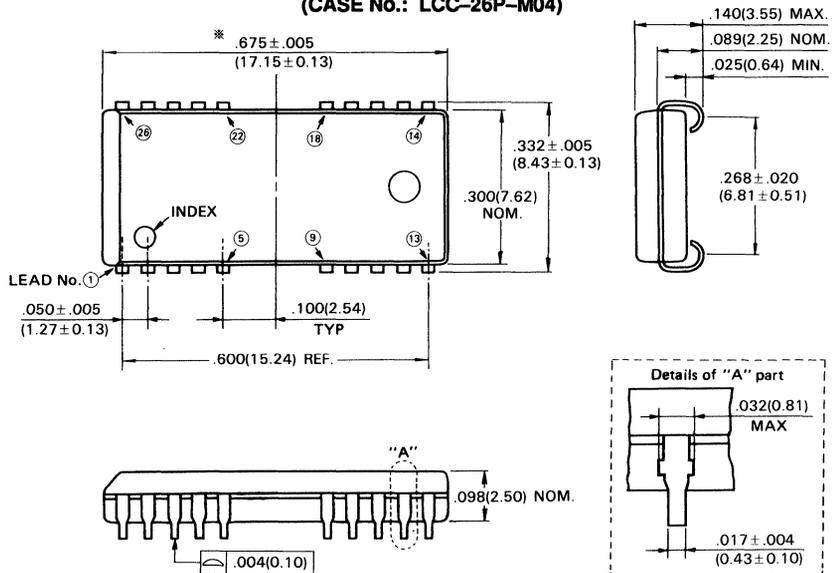
NOTE: 1. \*: This dimension includes resin protrusion. (Each side:  $.005$  (0.15) MAX)
