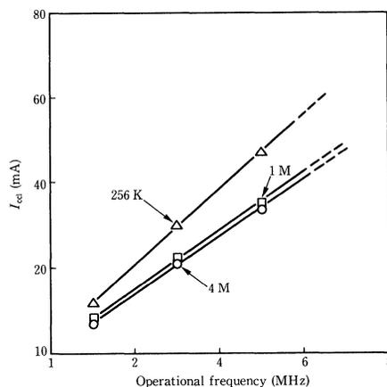
Fig. 24—Average  $V_{CC}$  current ( $I_{CC1}$ ) vs operational frequency.
