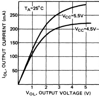
Fig. 23 – OUTPUT CURRENT vs OUTPUT VOLTAGE
