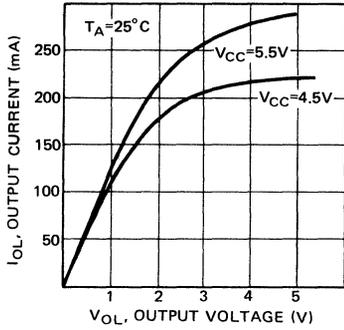
Fig. 22 – OUTPUT CURRENT vs OUTPUT VOLTAGE
