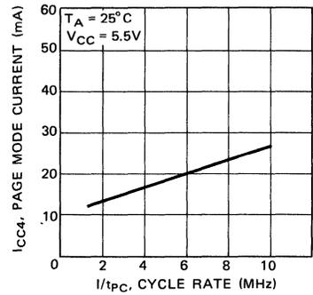
Fig. 13 – PAGE MODE CURRENT vs. CYCLE RATE
