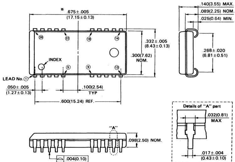
NOTE: 1. \*: This dimension includes resin protrusion. (Each side: .006(0.15) MAX)
