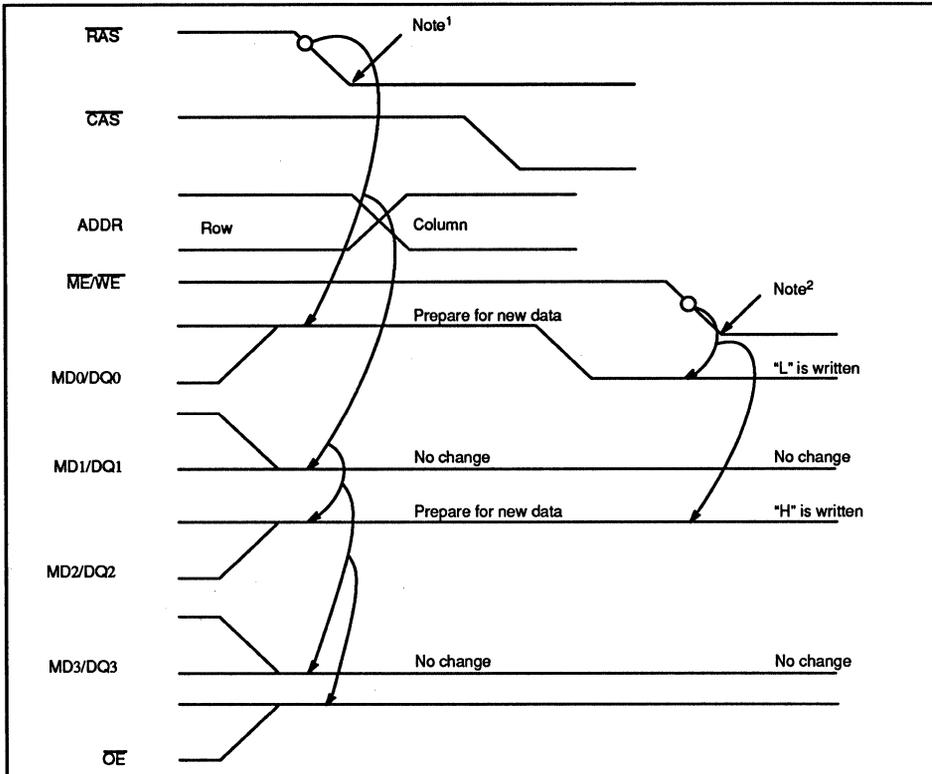
Figure 5. Bit Masking
