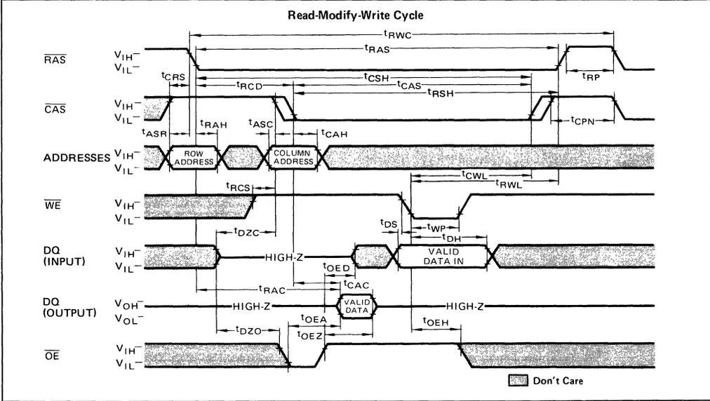
Note: 1) When  $\overline{OE}$  is kept high through a cycle, the DQ pins are kept high-Z state.
