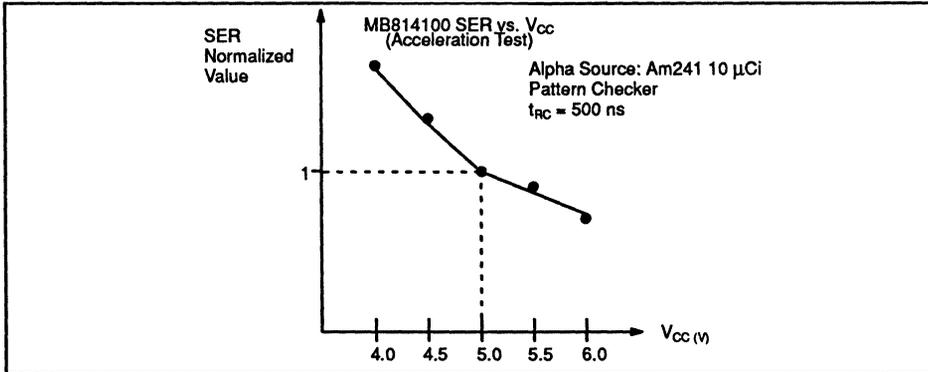
Figure 4. Soft Error Rate vs.  $V_{CC}$  (MB814100)
