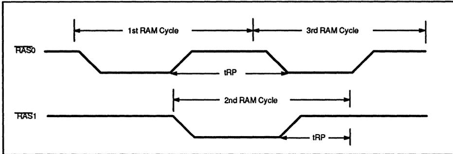
Figure 10. RAS Timing of Interleaving Memory
