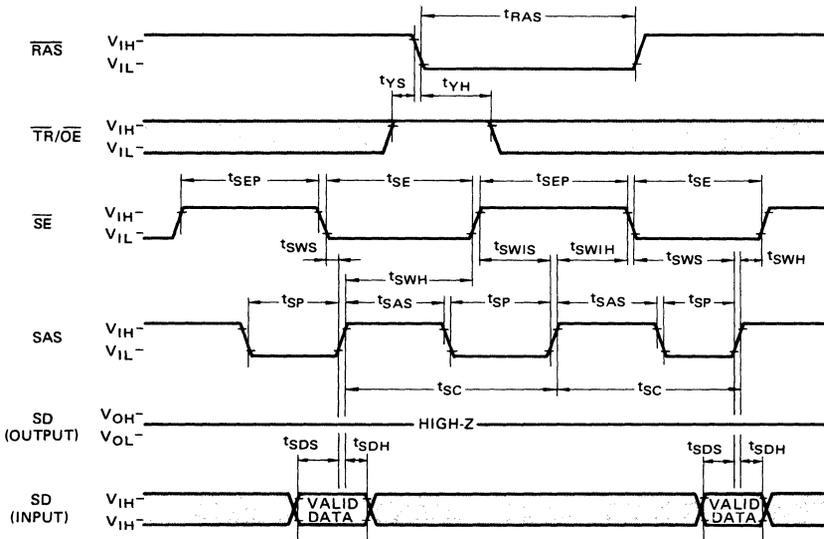
In the case of  $\overline{SE} = "L"$  while the operation;
