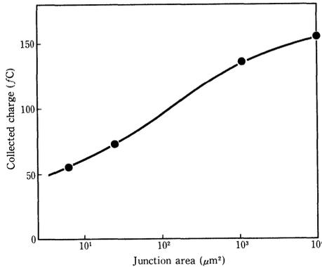
Fig. 10—Dependence of collected charge on junction area.
