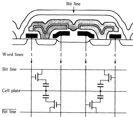
Fig. 7—3D stacked capacitor cell.
