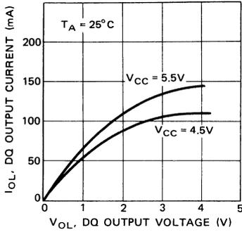
Fig. 31 – SD OUTPUT CURRENT vs SD OUTPUT VOLTAGE
