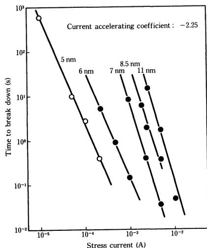
Fig. 15—Stress current on lifetime (0.1% cumulative failure).
