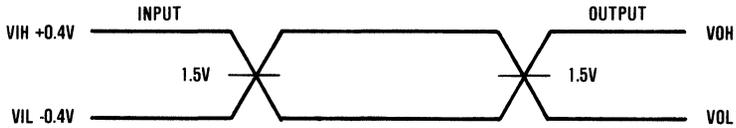
A.C. Testing: All input signals must switch between VIL -0.4V and VIH +0.4V. Input rise and fall times are driven at 1nsec per volt.
