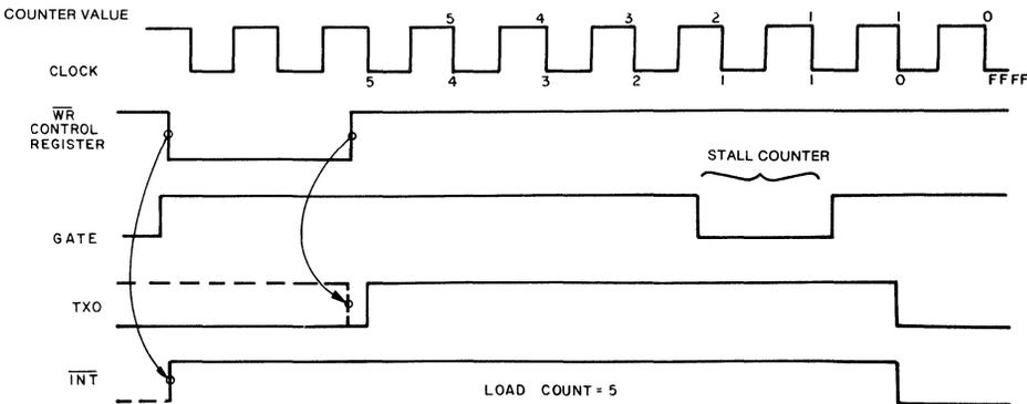
Fig. 2 - Timeout (mode 1) timing waveforms.
