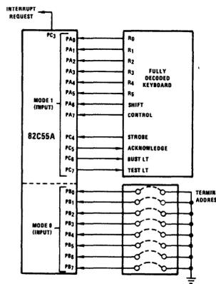
FIGURE 20. KEYBOARD AND TERMINAL ADDRESS INTERFACE
