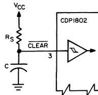
*The RC time constant should be greater than the oscillator start-up time (typically 20 ms).*
