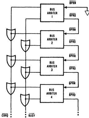
NOTE: The number of arbiters that may be daisy-chained together in the serial priority resolving scheme is a function of BCLK and the propagation delay from arbiter to arbiter. Normally, at 10MHz only 3 arbiters may be daisy-chained.
