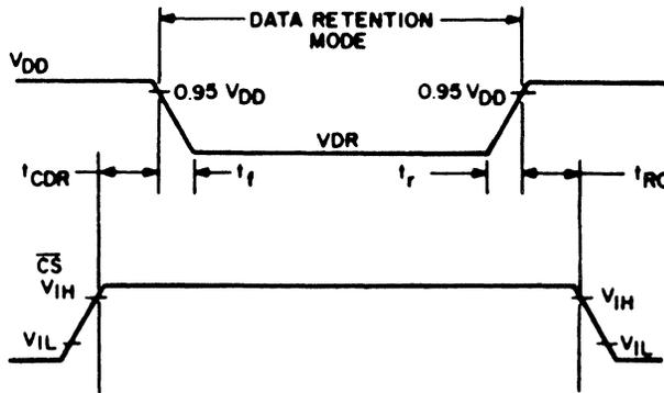
FIGURE 4. LOW  $V_{DD}$  DATA RETENTION WAVEFORMS AND TIMING DIAGRAM.
