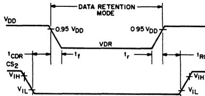
FIGURE 5. LOW  $V_{DD}$  DATA RETENTION TIMING WAVEFORMS
