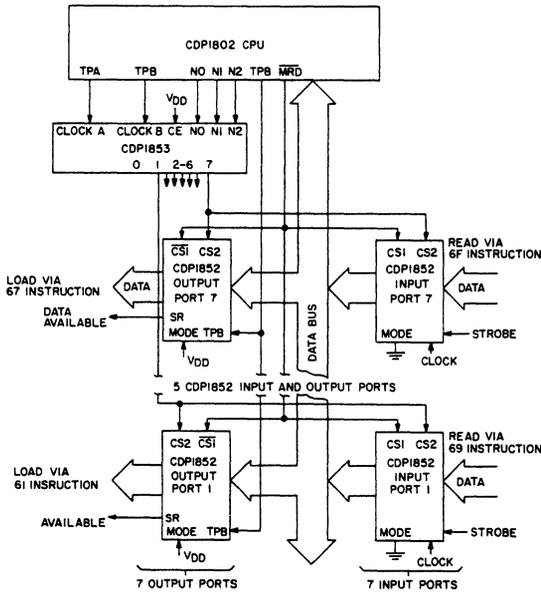
FIGURE 4. N-BIT DECODER IN A ONE-LEVEL I/O SYSTEM
