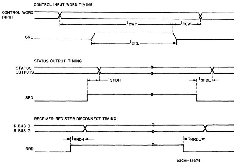
Fig. 9 – Mode 0 interface timing diagram.
