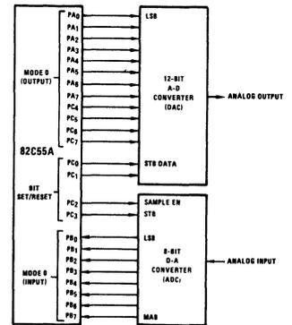
FIGURE 21. DIGITAL TO ANALOG, ANALOG TO DIGITAL
