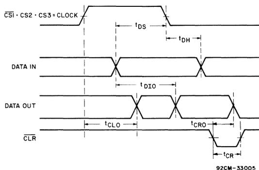
Fig. 5 - Timing waveforms for CDP1875C (output port).
