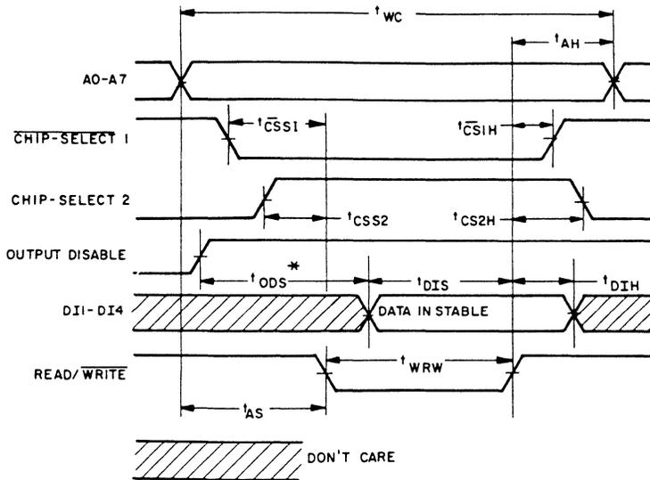
\*  $t_{ODS}$  is required for common I/O operation only; for separate I/O operations, output disable is don't care.
