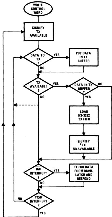
FIGURE 2. SIMPLE HS-3282 DRIVER ALGORITHM
