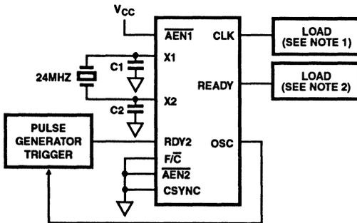
**TRYLCL, TRYHCH LOAD CIRCUIT (USING EF1)**
