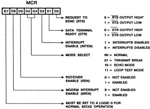
\*See Modem Status Register description for a description of register flag images with respect to output pins.
