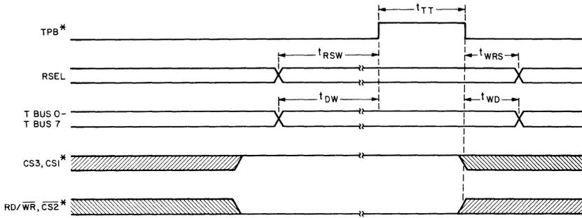
\* WRITE IS THE OVERLAP OF TPB, CSI, CS3=1 AND  $\overline{CS2}$ , RD/ $\overline{WR}$ =0
