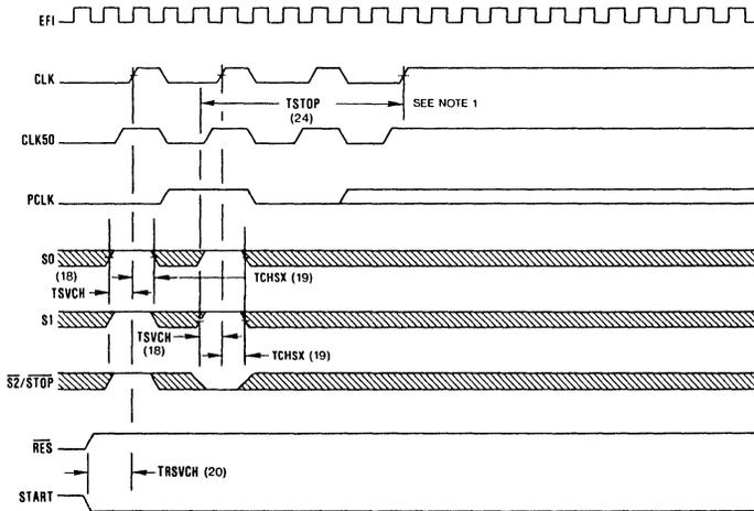
NOTE: 1. When  $F/\bar{C}$  is low, CLK and CLK50 stop high. When  $F/\bar{C}$  is high, CLK and CLK50 may stop either high or low.
