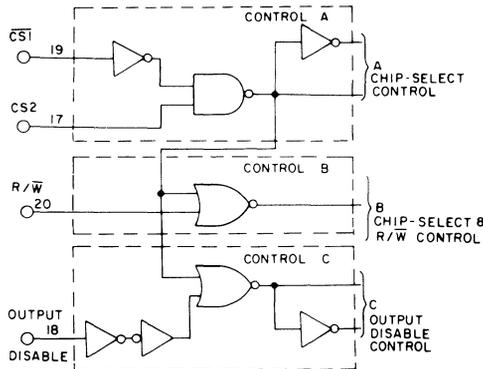
FIGURE 5. LOGIC DIAGRAM OF CONTROLS FOR MWS5101, MWS5101A
