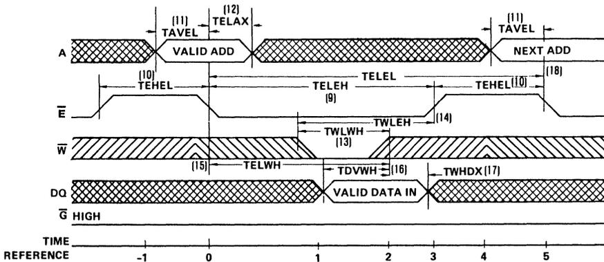
The write cycle is initiated on the falling edge of  $\bar{E}$  ( $T = 0$ ), which latches the address information in the on chip registers. If a write cycle is to be performed where the output is not to become active,  $\bar{G}$  can be held high (inactive). TDVWH and TWHDX must be met for proper device operation regardless of  $\bar{G}$ . If  $\bar{E}$  and  $\bar{G}$  fall before  $\bar{W}$  falls (read mode), a possible bus conflict may exist. If  $\bar{E}$  rises before  $\bar{W}$
