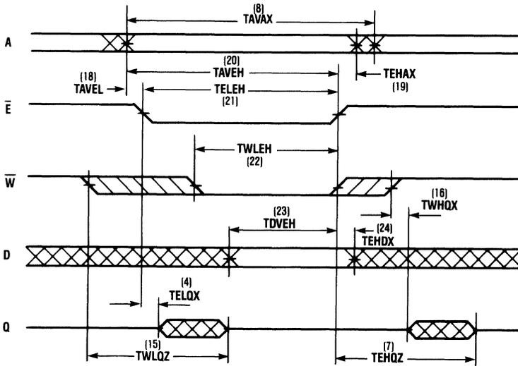
NOTE: In this mode,  $\bar{W}$  rises after  $\bar{E}$ . If  $\bar{W}$  falls before  $\bar{E}$  by a time exceeding  $TWLQZ$  (Max)  $TELQX$  (Min), and rises after  $\bar{E}$  by a time exceeding  $TEHQZ$  (Max)- $TWHQZ$  (Min), then  $Q$  will remain in the high impedance state throughout the cycle.
