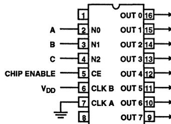
FIGURE 4. N-BIT DECODER USED AS A 1 OF 8 DECODER
