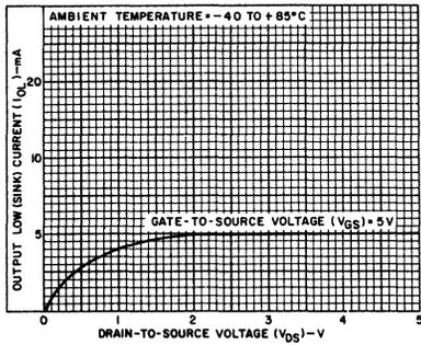
FIGURE 8. CDP1802BC MINIMUM OUTPUT LOW (SINK) CURRENT CHARACTERISTICS
