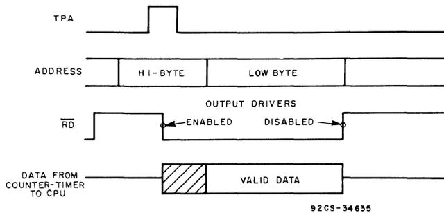
Fig. 9 - CDP1800-series memory-mapping read cycle timing waveforms.
