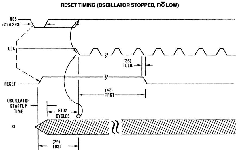
NOTE: 1. CLK, CLK50, PCLK Remain in the High State until  $\overline{RES}$  goes high and 8192 valid oscillator cycles have been registered by the 82C85 internal counter (TOST time period). After  $\overline{RES}$  goes high and CLK, CLK50, PCLK become active, the RESET output will remain high for minimum of 16 CLK cycles (TRST)
