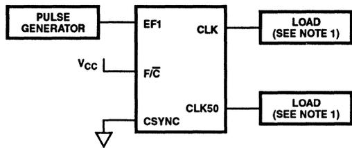
**TRYLCL, TRYHCH LOAD CIRCUIT (USING X1, X2)**
