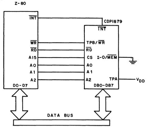
FIGURE 8. ZILOG CORPORATION Z-80<sup>®</sup> INTERFACE TO THE CDP1879
