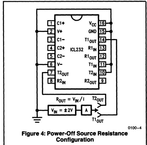
Figure 4: Power-Off Source Resistance Configuration
