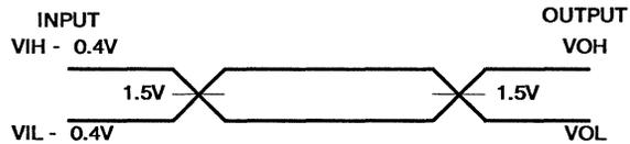
A.C. Testing: All input signals must switch between  $V_{IL} - 0.4V$  and  $V_{IH} + 0.4V$ . Input rise and fall times are driven at  $1ns/V$ .
