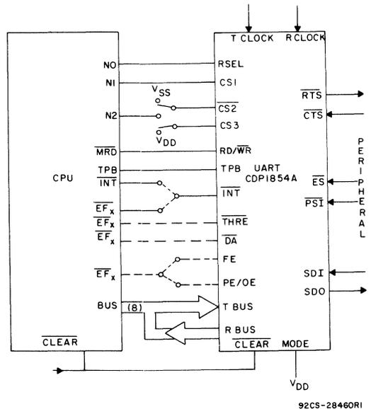
Fig. 2 - Recommended CDP1800-series connection, Mode 1 (non-interrupt driven system).
