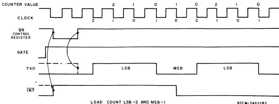
Fig. 6 - Variable-duty cycle (mode 5) timing waveforms.
