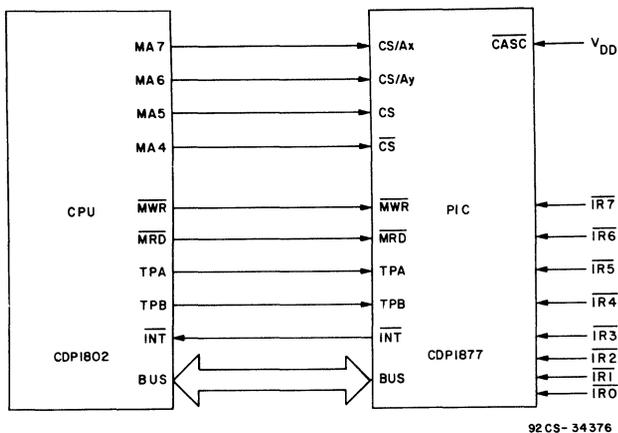
Fig. 2 - PIC and CPU connection diagram.
