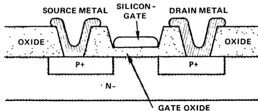
FIGURE 3. SILICON-GATE PFET STRUCTURE
