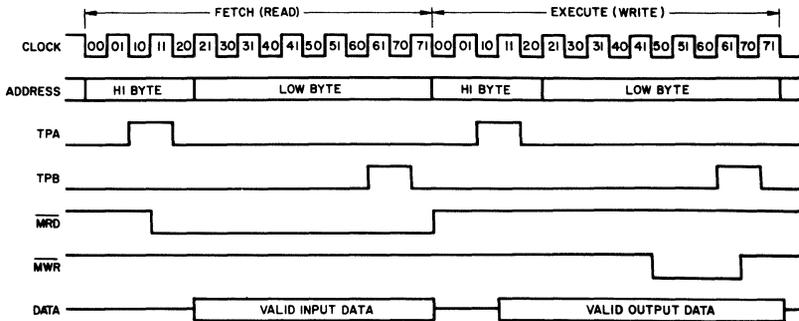
FIGURE 12. BASIC DC TIMING WAVEFORMS, ONE INSTRUCTION CYCLE
