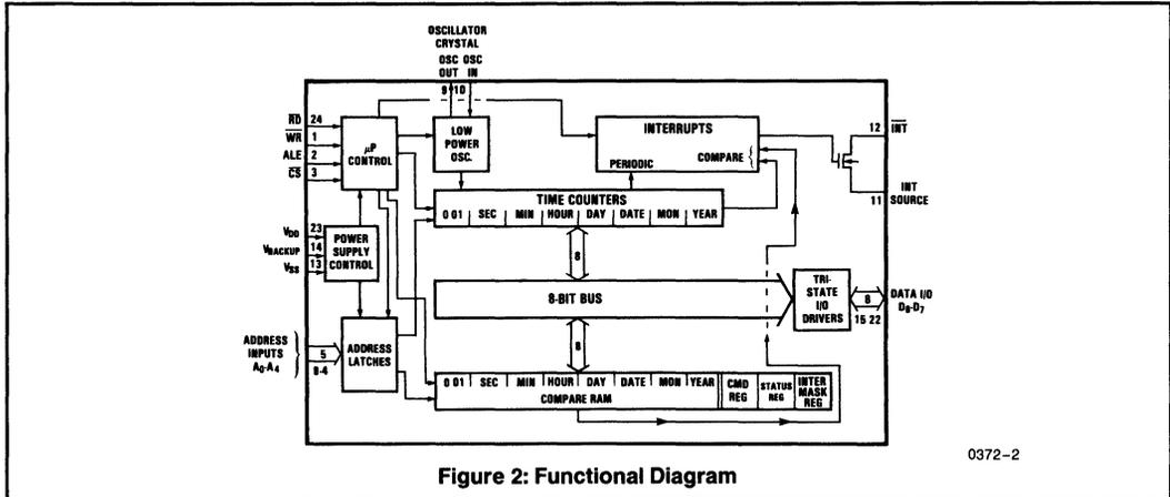
Figure 2: Functional Diagram
