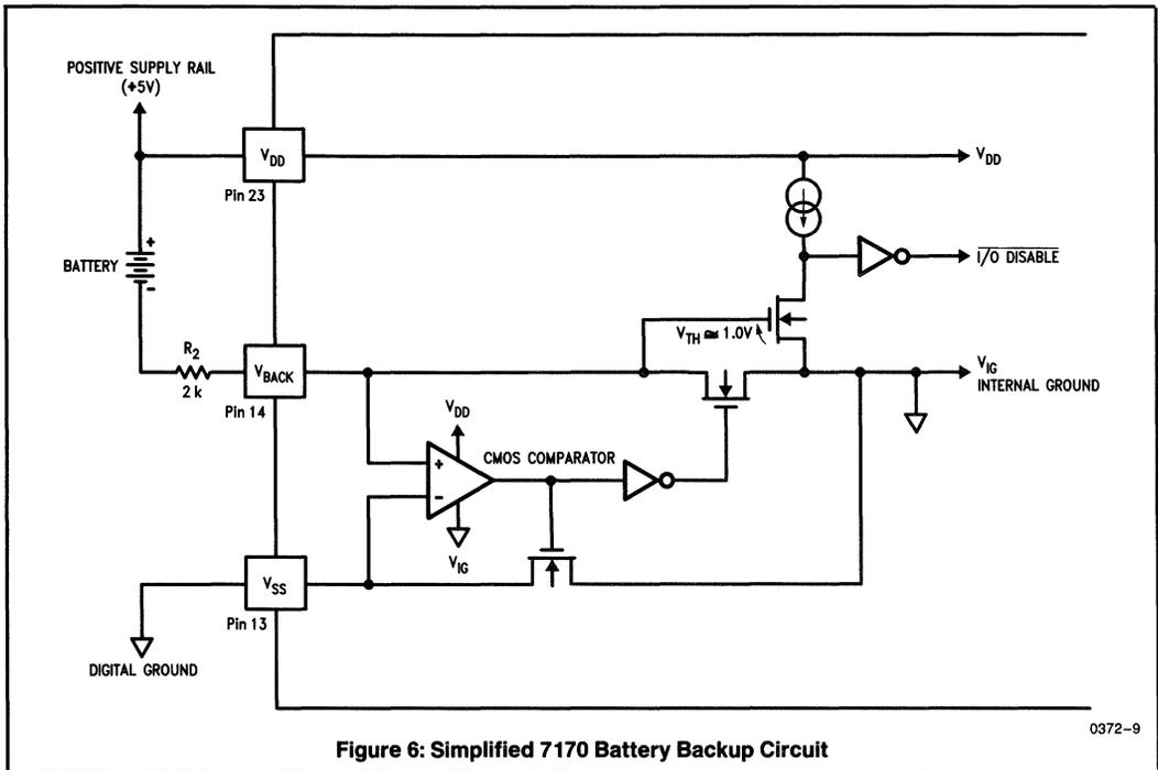
Figure 6: Simplified 7170 Battery Backup Circuit
