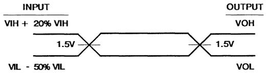
A.C. Testing: All input signals (other than CLK) must switch between  $V_{ILmax} - 50\% V_{IL}$  and  $V_{IHmin} + 20\% V_{IH}$ . CLK must switch between  $0.4V$  and  $V_{CC} - 0.4$ . Input rise and fall times are driven at  $1\text{ns}/V$ .
