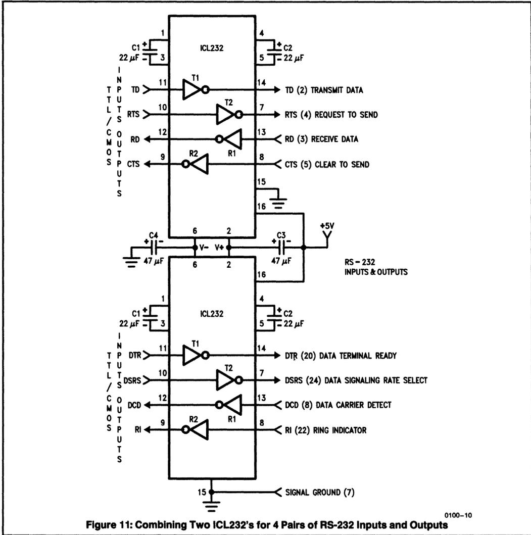
Figure 11: Combining Two ICL232's for 4 Pairs of RS-232 Inputs and Outputs
