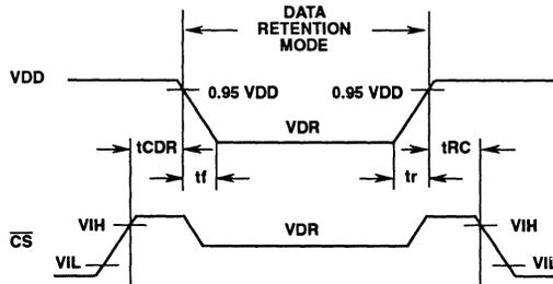
FIGURE 3. LOW VDD DATA RETENTION TIMING WAVEFORMS
