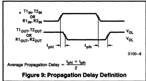
**Figure 9: Propagation Delay Definition**
