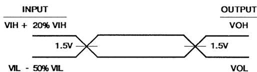
A.C. Testing: All input signals (other than CLK) must switch between  $V_{ILmax} - 50\% V_{IL}$  and  $V_{IHmin} + 20\% V_{IH}$ . CLK must switch between 0.4V and  $V_{CC} - 0.4V$ . Input rise and fall times are driven at 1ns/V.
