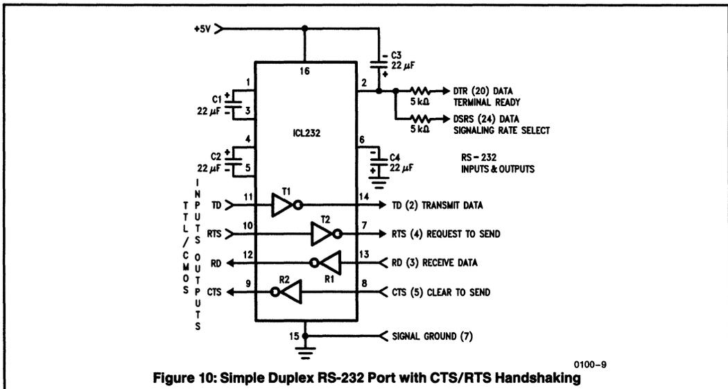
**Figure 10: Simple Duplex RS-232 Port with CTS/RTS Handshaking**
