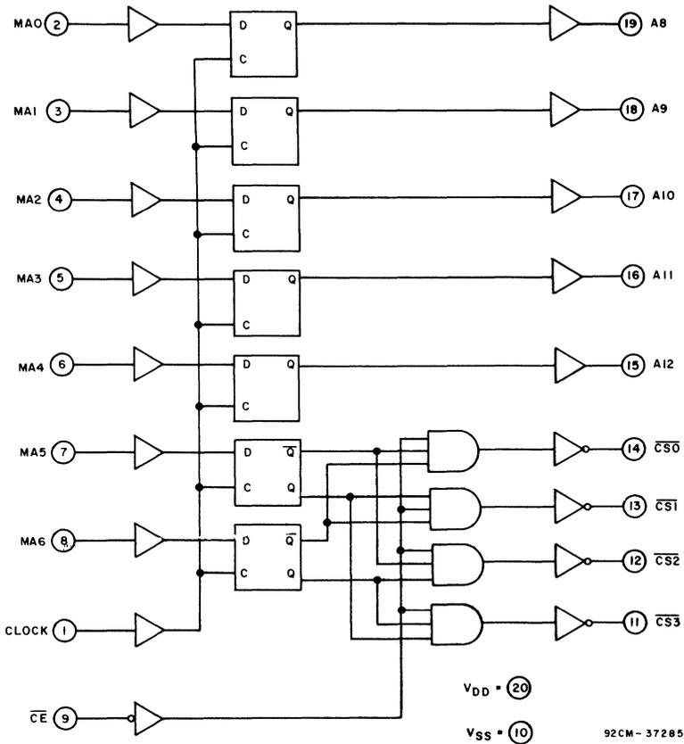
Fig 1 - Functional diagram for the CDP1883, CDP1883C
