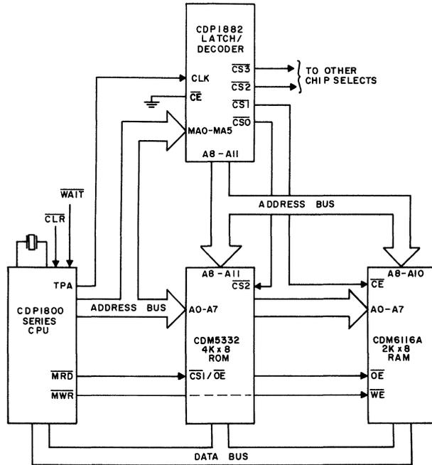
Fig. 5 - CDP1800-series system using the CDP1882.
