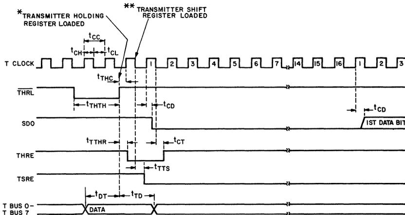
\* THE HOLDING REGISTER IS LOADED ON THE TRAILING EDGE OF  $\overline{\text{THRL}}$ .
