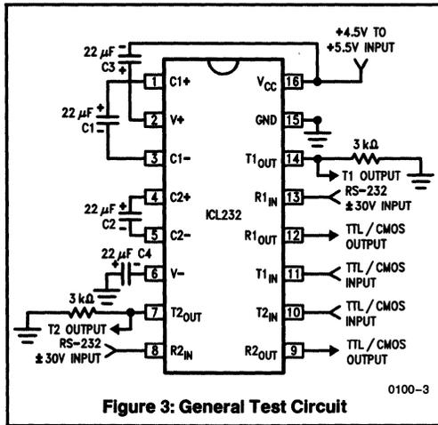
Figure 3: General Test Circuit
