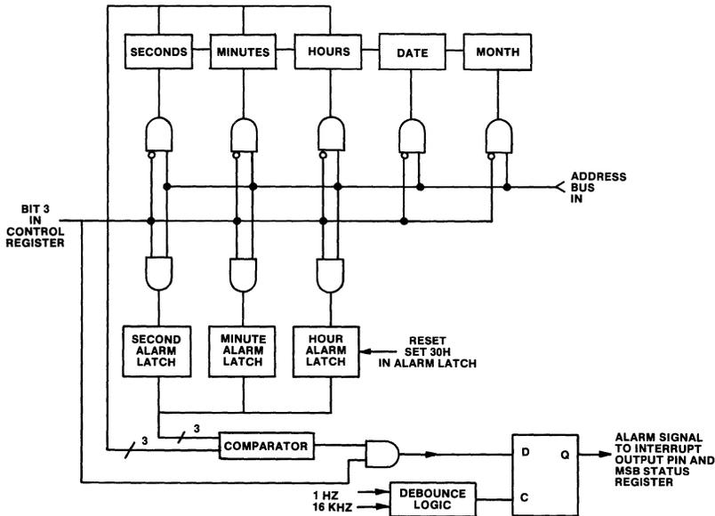
**FIGURE 19. SIMPLIFIED DIAGRAM OF COUNTER/ALARM LATCH ACCESS.**
