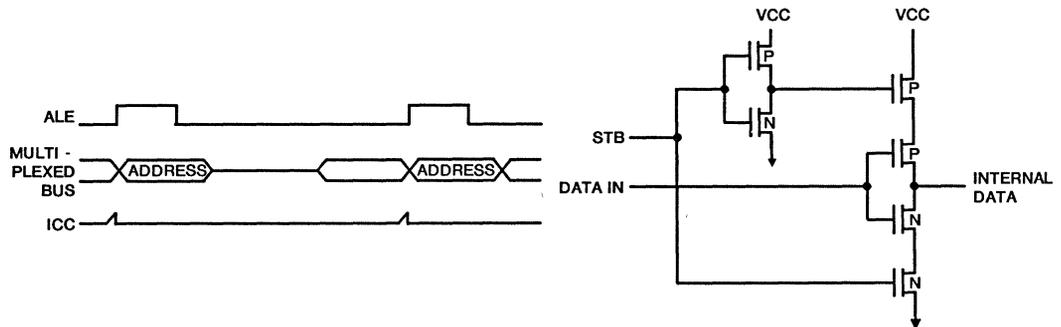
FIGURE 3. SYSTEM EFFECTS OF GATED INPUTS
