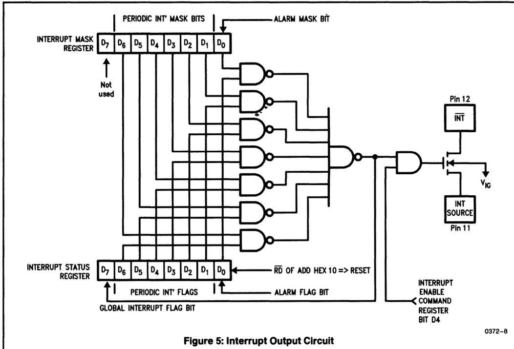
Figure 5: Interrupt Output Circuit
