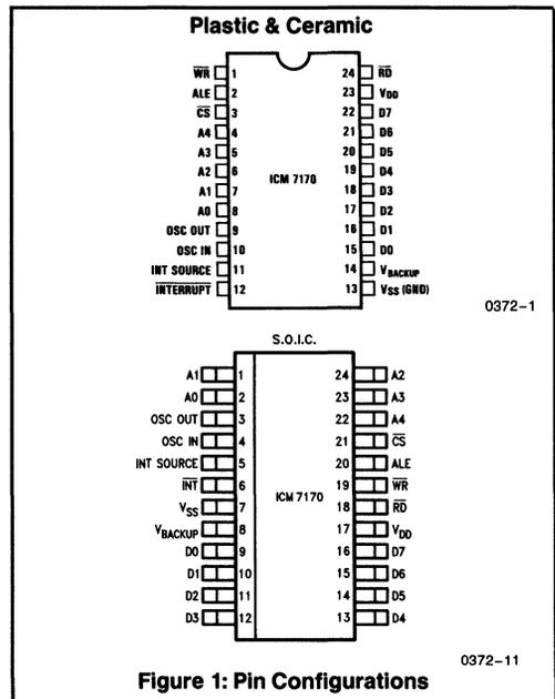
Figure 1: Pin Configurations
