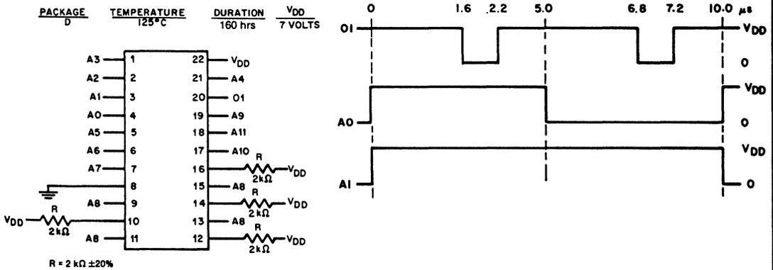
FIGURE 6. DYNAMIC/OPERATING BURN-IN CIRCUIT AND TIMING DIAGRAM
