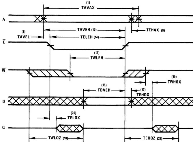
NOTE: In this mode,  $\bar{W}$  rises after  $\bar{E}$ . If  $\bar{W}$  falls before  $\bar{E}$  by a time exceeding TWLQZ (Max) TELQX (Min), and rises after  $\bar{E}$  by a time exceeding TEHQZ (Max)-TWHQZ (Min), then Q will remain in the high impedance state throughout the cycle.
