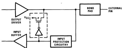
FIGURE 20B. BUS HOLD CIRCUITRY — PINS 4-6, 68
