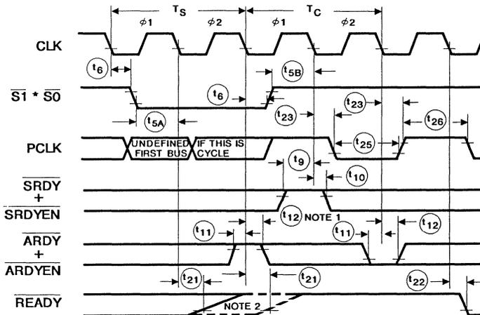
NOTES. 1. This is an asynchronous input. The setup and hold times shown are required to guarantee the response shown.
