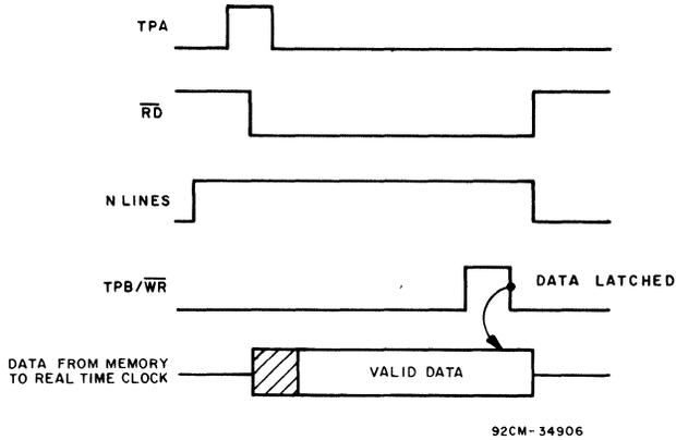
Fig. 15 - CDP1800-series input/output-mapping timing waveforms with output instruction.
