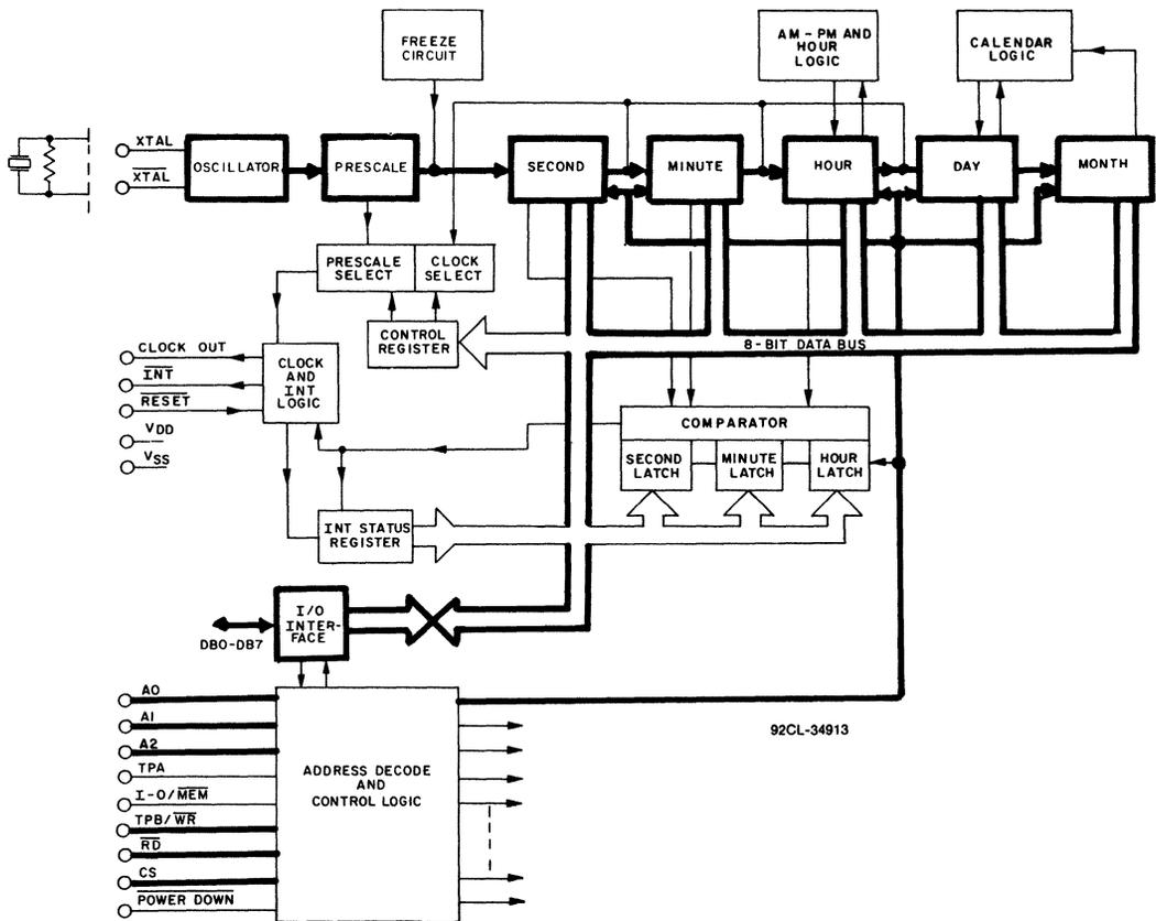
Fig. 2 - Functional diagram - time counters highlighted.
