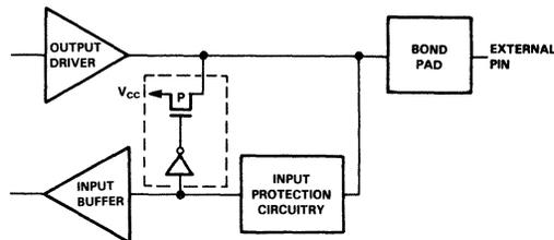
FIGURE 6B. BUS HOLD CIRCUITRY PIN 26-32, 34
