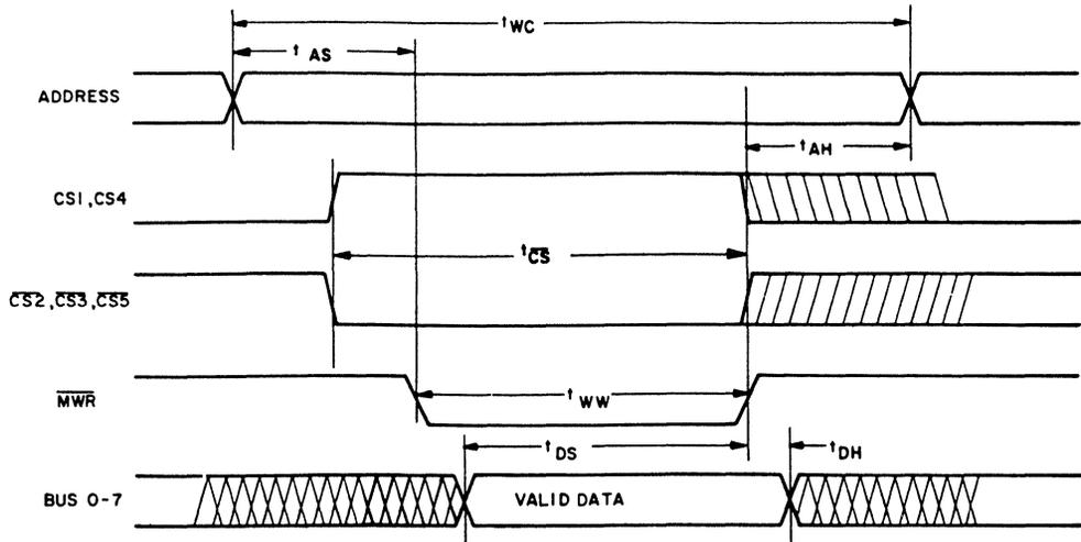
NOTE:  $\overline{MRD}$  must be high during write operation
