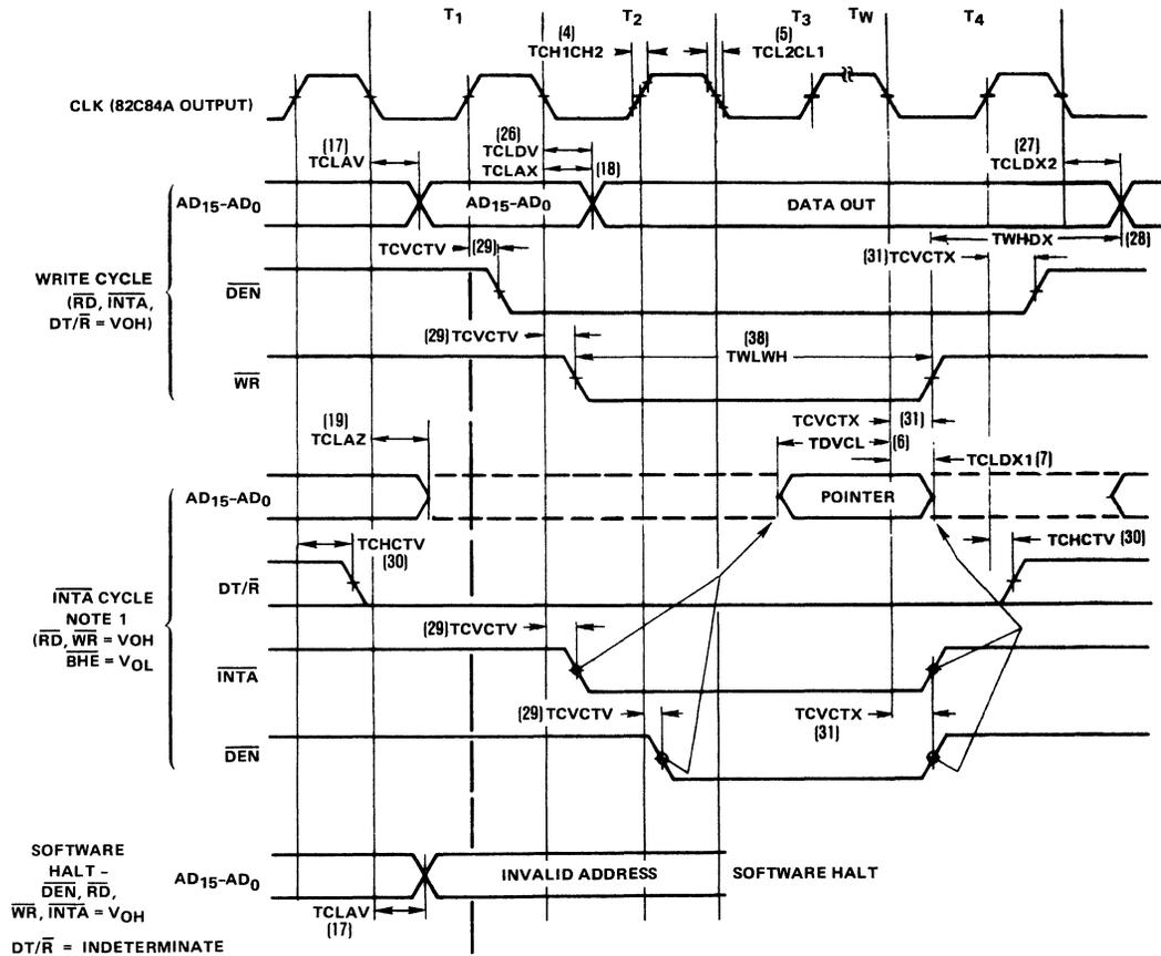
NOTE: 1. Two INTA cycles run back-to-back. The 80C86 local ADDR/DATA bus is floating during both INTA cycles. Control Signals are shown for the second INTA cycle.
