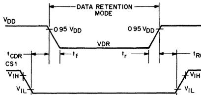
Fig 8 - Low  $V_{DD}$  data retention timing waveforms
