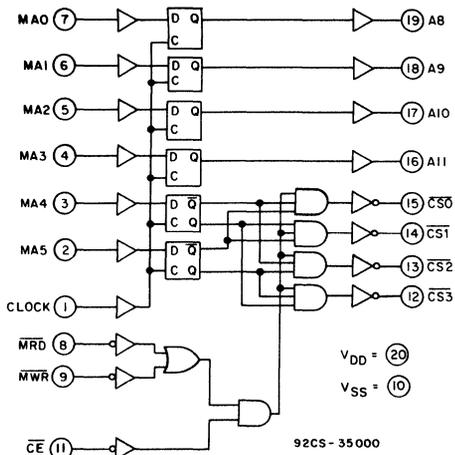
Fig. 1 - Functional diagram for the CDP1881, CDP1881C.
