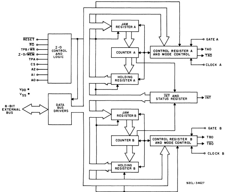
Fig. 1 - Functional diagram CDP1878 and CDP1878C.
