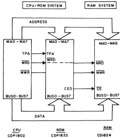
Fig 5 - CDP1824 (128 x 8) minimum system (128 x 8)
