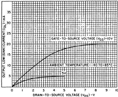
FIGURE 6. MINIMUM OUTPUT LOW (SINK) CURRENT CHARACTERISTICS
