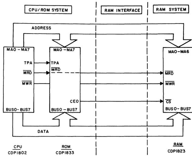
Fig. 5 - CDP1823 (128 x 8) minimum system (128 x 8)
