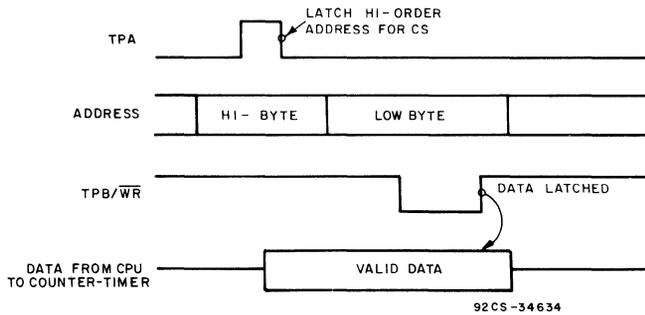
Fig. 8 - CDP1800-series memory-mapping write cycle timing waveforms.
