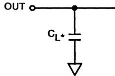
\* Includes stray and jig capacitance,  $C_L = 50\text{pF}$
