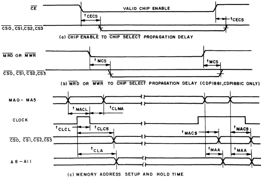
Fig. 3 - CDP1881 and CDP1882 timing waveforms.
