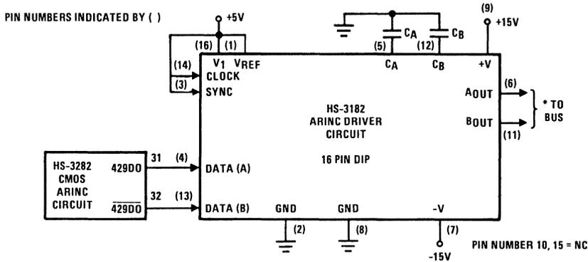
\* The rise and fall time of the outputs are set to ARINC specified values by  $C_A$  and  $C_B$ . Typical  $C_A = C_B = 75\text{pF}$  for high speed and  $300\text{pF}$  for low speed operation. The output HI and low levels are set to ARINC specifications by  $V_{REF}$ .
