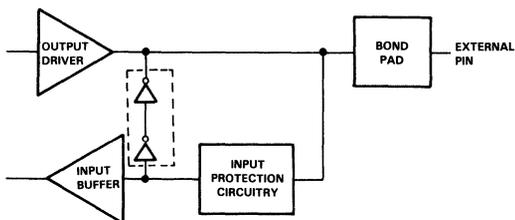
FIGURE 6A. BUS HOLD CIRCUITRY PIN 2-16, 35-39
