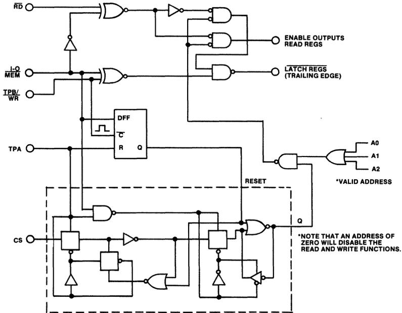
**FIGURE 4. I/O-CONTROL AND DEVICE-ENABLE SCHEMATIC**
