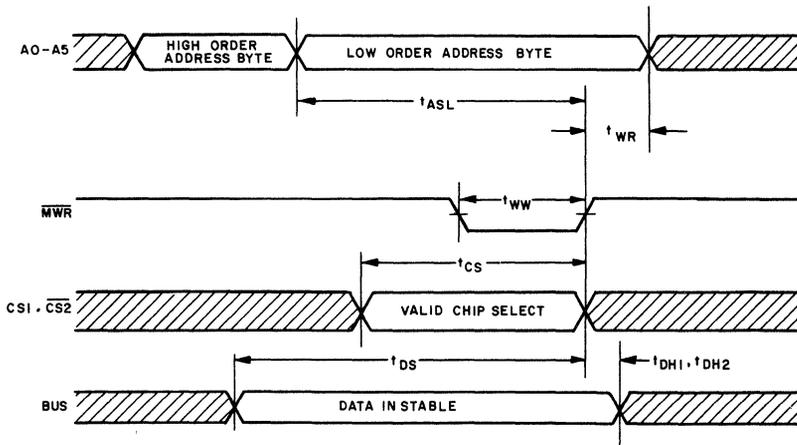
Fig. 7 - Timing waveforms for Write-cycle 2 [TPA=High].
