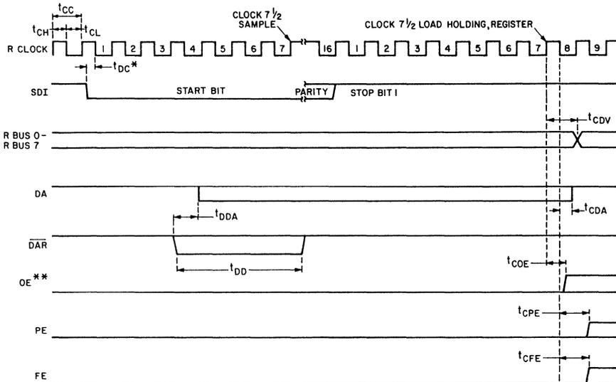
\* IF A START BIT OCCURS AT A TIME LESS THAN  $t_{DC}$  BEFORE A HIGH-TO-LOW TRANSITION OF THE CLOCK, THE START BIT MAY NOT BE RECOGNIZED UNTIL THE NEXT HIGH-TO-LOW TRANSITION OF THE CLOCK THE START BIT MAY BE COMPLETELY ASYNCHRONOUS WITH THE CLOCK
