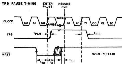
NOTE: PAUSE (IN CLOCK WAVEFORM) WHILE REPRESENTED HERE AS ONE CLOCK CYCLE IN DURATION, COULD BE INFINITELY LONG.
