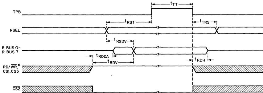
\* READ IS THE OVERLAP OF CSI, CS3, RD/ $\overline{WR}$ =1 AND  $\overline{CS2}$ =0
