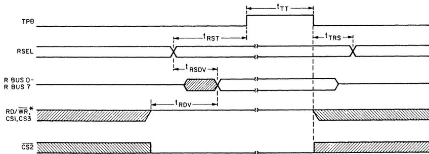
\* READ IS THE OVERLAP OF CSI, CS3, RD/WR=1 AND  $\overline{CS2}$ =0
