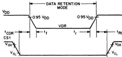
Fig 3 - Low  $V_{DD}$  data retention timing waveforms
