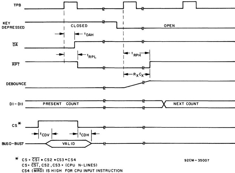
Fig 4 — CDP1871A dynamic timing diagram (repeat)
