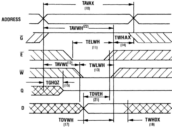
In this write cycle  $\bar{G}$  has control of the output after a period,  $T_{GHQZ}$ .  $\bar{G}$  switching the output to a high impedance state allows data in to be applied without bus contention after
