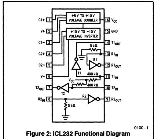
Figure 2: ICL232 Functional Diagram
