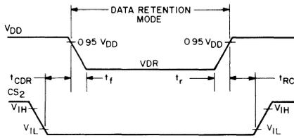
FIGURE 3. LOW  $V_{DD}$  DATA RETENTION TIMING WAVEFORMS
