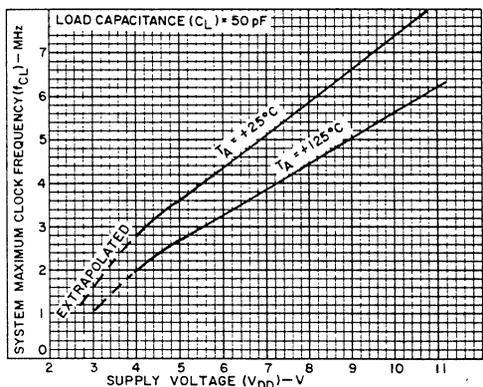
**FIGURE 3. TYPICAL MAXIMUM CLOCK FREQUENCY AS A FUNCTION OF SUPPLY VOLTAGE**
