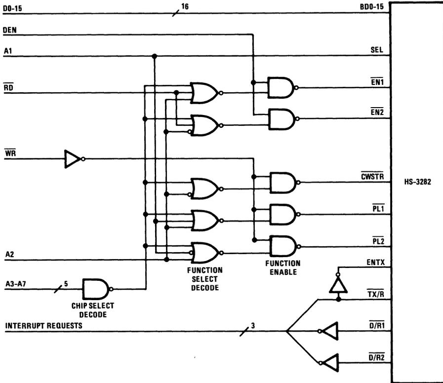
FIGURE 1. TYPICAL HOST TO HS-3282 INTERFACE LOGIC
