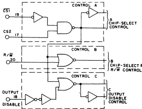
Fig. 6 - Logic diagram of controls for CDP1822 and CDP1822C.
