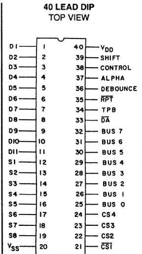
FIGURE 2. TERMINAL DIAGRAM
