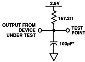
**$\overline{\text{BPRO}}$ ,  $\overline{\text{BREQ}}$  LOAD CIRCUIT**
