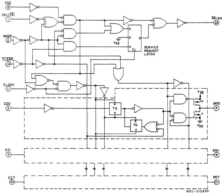
**FIGURE 2. CDP1852/3 LOGIC DIAGRAM**
