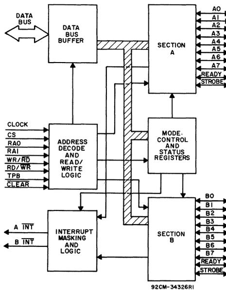
Fig. 1 - Functional diagram for CDP1851 and CDP1851C.
