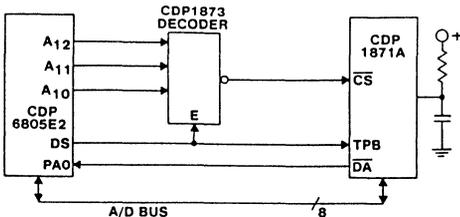
**FIGURE 7. APPLICATION OF THE CDP1871A AND CDP6805 PROCESSOR**
