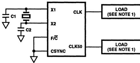
**TCHCL, TCLCH LOAD CIRCUIT (USING EF1)**
