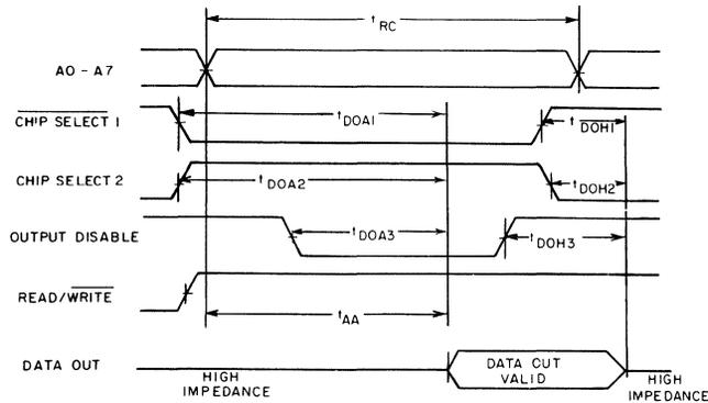
Fig. 1 - Read cycle timing waveforms.
