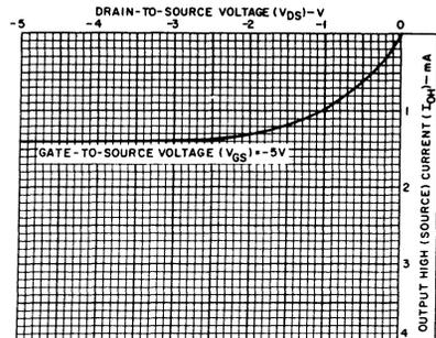
FIGURE 7. CDP1802BC MINIMUM OUTPUT HIGH (SOURCE) CURRENT CHARACTERISTICS
