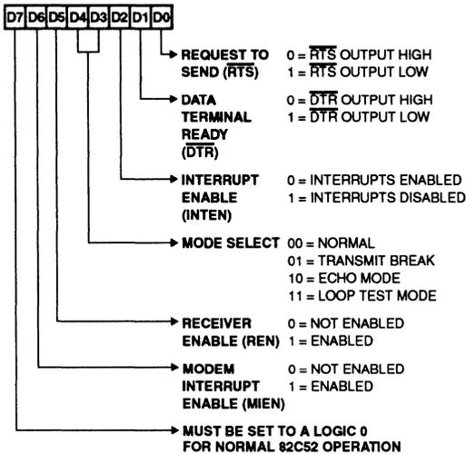
**FIGURE 5. MCR FORMAT**
