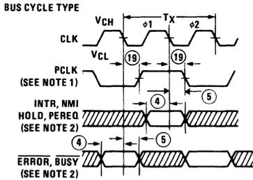
80C286 RESET INPUT TIMING AND SUBSEQUENT PROCESSOR CYCLE PHASE
