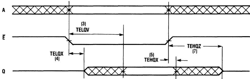
NOTE:  $\bar{W}$  is high for entire cycle and D is ignored. Address is stable by the time  $\bar{E}$  goes low and remains valid until  $\bar{E}$  goes high.
