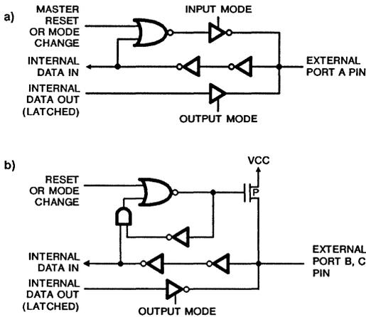
FIGURE 2. PORT A, PORT C BUS-HOLD CONFIGURATION
