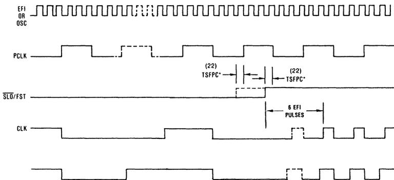
\* IF TSFPC is not met on one edge of PLCK, SLO/FST will be recognized on the next edge of PLCK.
