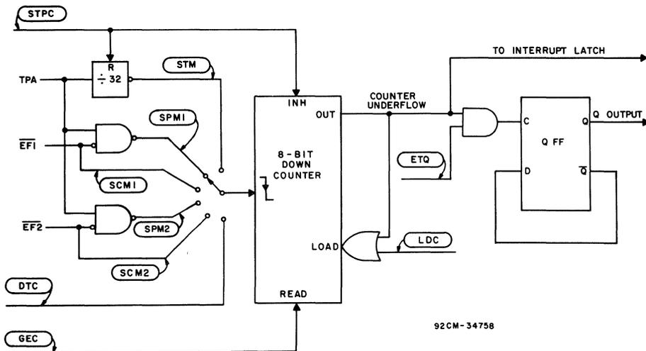
Fig. 6 - Timer/Counter diagram for CDP1805AC and CDP1806AC.
