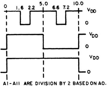
FIGURE 4. DYNAMIC/OPERATING BURN-IN CIRCUIT AND TIMING DIAGRAM
