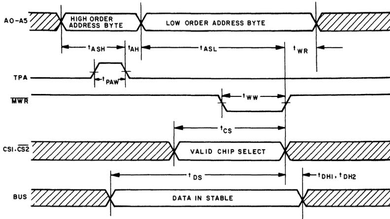
Fig 6 - Timing waveforms for Write-cycle 1.
