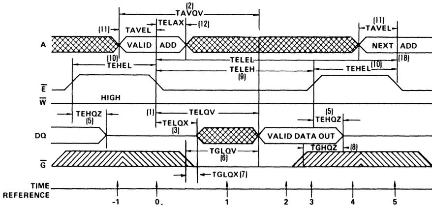
The address information is latched in the on chip registers on the falling edge of  $\bar{E}$  ( $T = 0$ ), minimum address setup and hold time requirements must be met. After the required hold time, the addresses may change state without affecting device operation. During time ( $T = 1$ ), the outputs become enabled but data is not valid until time ( $T = 2$ ),  $\bar{W}$  must
