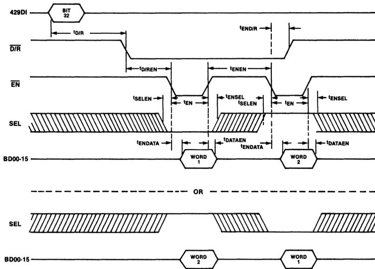
FIGURE 2. RECEIVER TIMING
