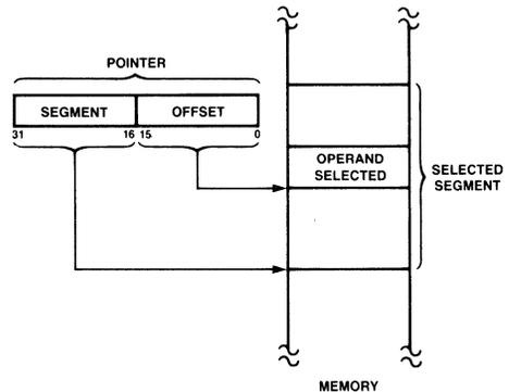
FIGURE 4. TWO COMPONENT ADDRESS
