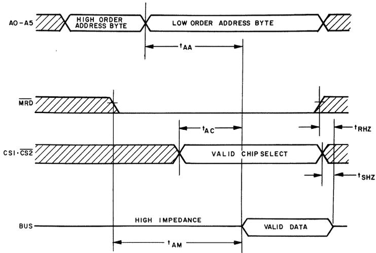
Fig 5 - Timing waveforms for Read-cycle 2 [TPA-High].
