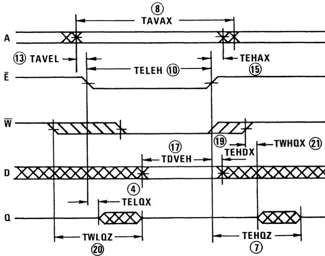
NOTE: In this mode,  $\bar{W}$  rises after  $\bar{E}$ . If  $\bar{W}$  falls before  $\bar{E}$  by a time exceeding  $TWLQZ$  (Max) -  $TELQX$  (Min), and rises after  $\bar{E}$  by a time exceeding  $TEHQZ$  (Max) -  $TWHQX$  (Min), then Q will remain in the high impedance state throughout the cycle. The address must remain stable whenever  $\bar{E}$  and  $\bar{W}$  are both low.
