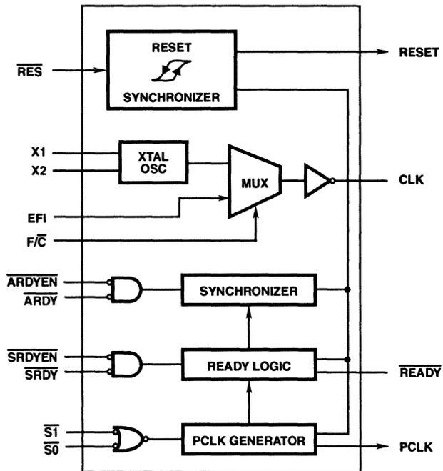
**Pin Description** The following pin function descriptions are for the 82C284 clock generator.
