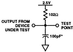
**$\overline{\text{AEN}}$  LOAD CIRCUIT**
