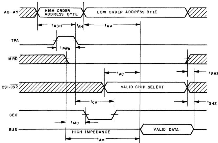
Fig. 4 - Timing waveforms for Read-cycle 1
