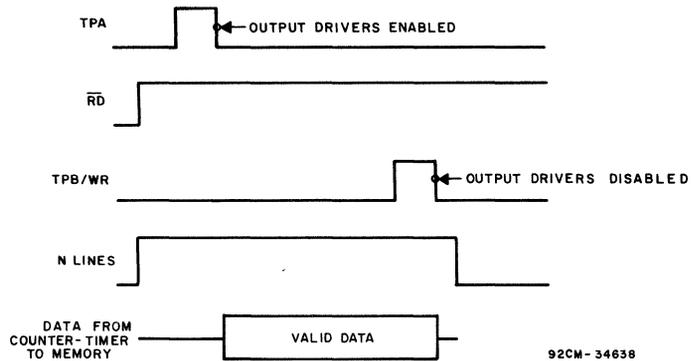
Fig. 12 - CDP1800-series input/output-mapping timing waveforms with input instruction.
