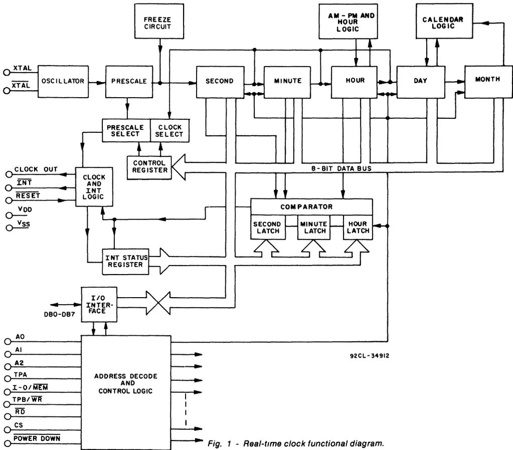
Fig. 1 - Real-time clock functional diagram.
