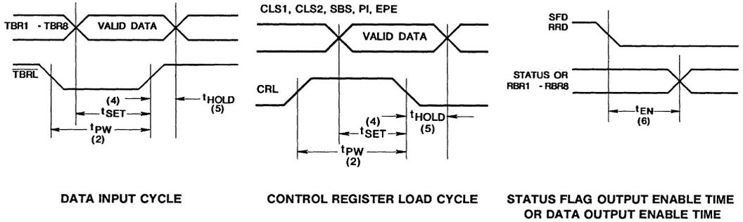
**A.C. Testing Input, Output Waveform**
