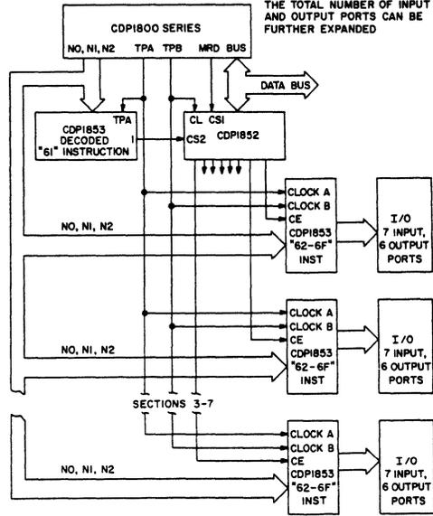
FIGURE 5. TWO-LEVEL I/O USING CDP1853 AND CDP1852
