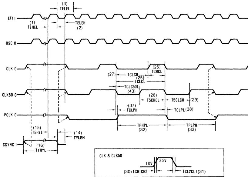
NOTE: All Timing Measurements are made at 1.5 Volts Unless Otherwise Noted.
