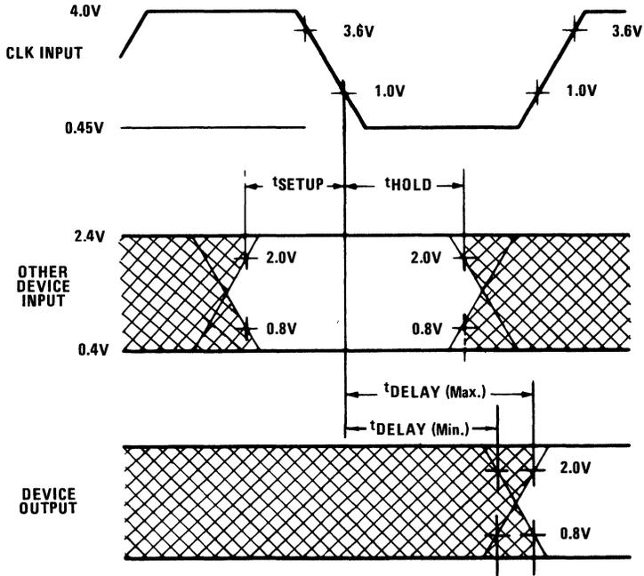
NOTE: For A.C. testing, input rise and fall times are driven at 1 ns per volt.
