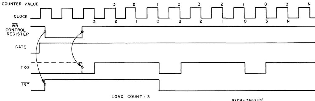
Fig. 5 - Rate generators (mode 4) timing waveforms. 92CM-34631R2
