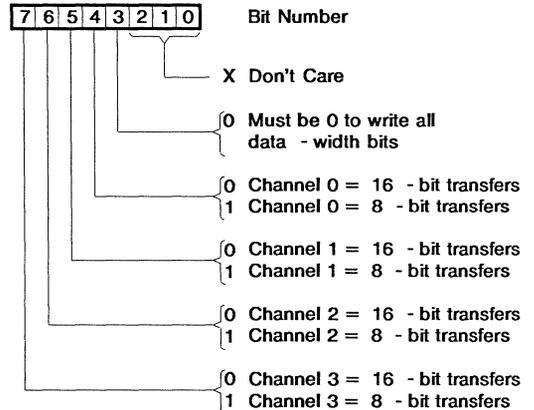
**Mask Register** - In 16-bit transfer mode this register operates the same as the previous Mask register description with the exception of bit 3 when writing the instruction to separately set or clear a mask bit. Bit 3 of the data must be "1" when writing a single mask bit. Bits 4-7 are ignored when this instruction is written. Refer to the following diagram for writing single mask bits.
