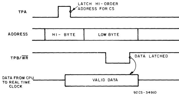
Fig. 12 - CDP1800-series memory-mapped write-cycle timing waveforms.
