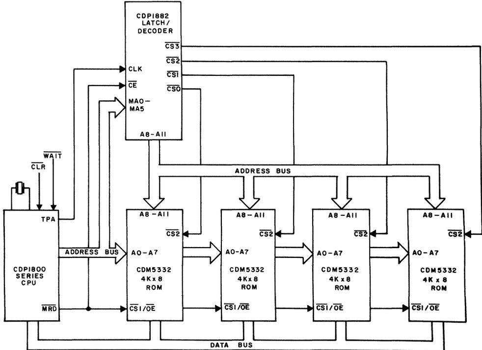
Fig. 6 - 16K-byte ROM systems using the CDP1882.
