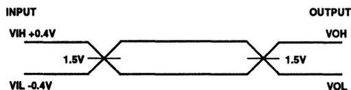
A.C. Testing: All input signals (other than CLK) must switch between  $V_{IL} -0.4V$  and  $V_{IH} +0.4V$ . CLK must switch between 0.4V and  $V_{CC} -0.4V$ . Input rise and fall times are driven at 1ns/V.
