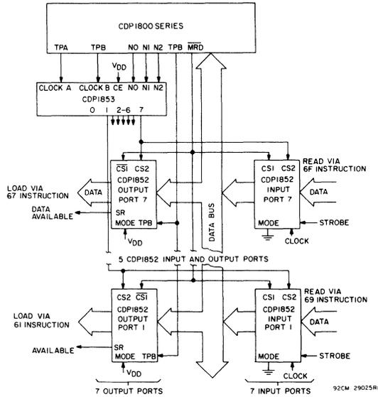
Fig. 5 - N-bit decoder in a one-level I/O system
