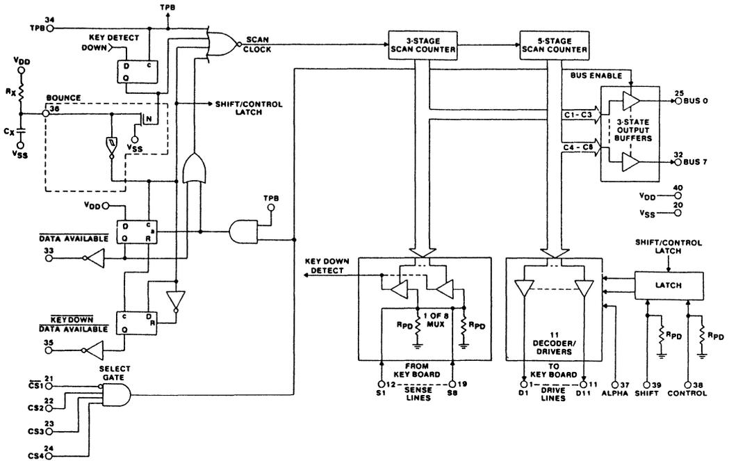
FIGURE 3. CDP1871A CONTROL SCHEMATIC
