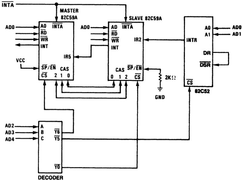
FIGURE 15. EXAMPLE 2: CASCADED 82C59As
