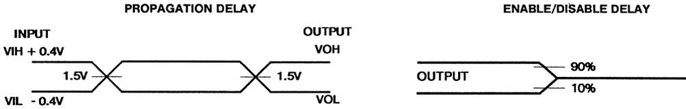
AC Testing: All input signals (except IX and RST) must switch between  $V_{IL} - 0.4V$  and  $V_{IH} + 0.4V$ . Input rise and fall times are driven at 1nsec per volt.
