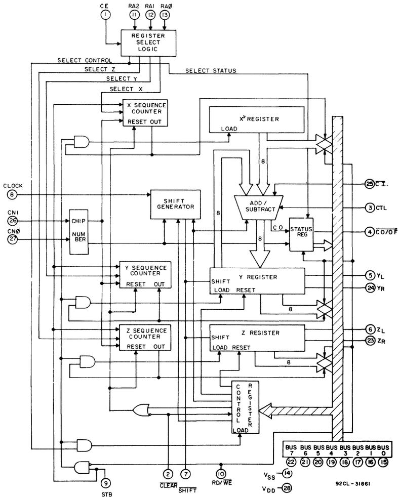
Fig. 2 - Block diagram of CDP1855 and CDP1855C.
