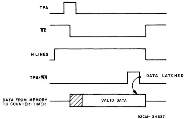
Fig. 11 - CDP1800-series input/output-mapping timing waveforms with output instruction.
