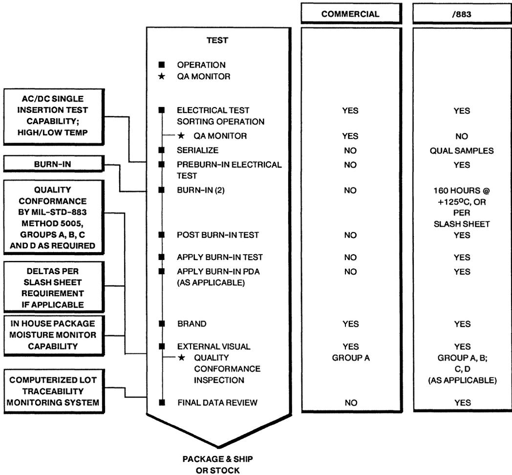
(2) Burn-in test temperatures can be increased and time reduced per regression tables in Mil-Std-883, Method 1015
