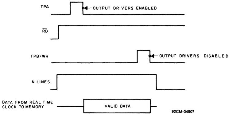
Fig. 16 - CDP1800-series input/output-mapping timing waveforms with input instruction.
