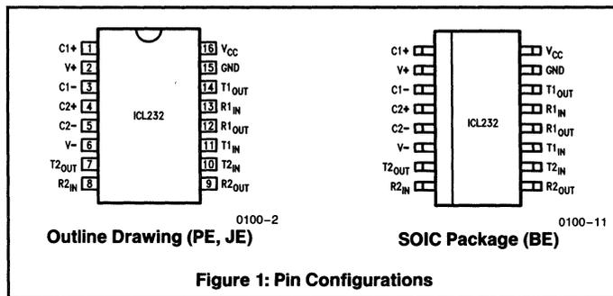
Figure 1: Pin Configurations
