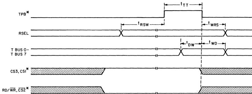
\* WRITE IS THE OVERLAP OF TPB, CSI, CS3=1 AND  $\overline{CS2}$ , RD/WR=0
