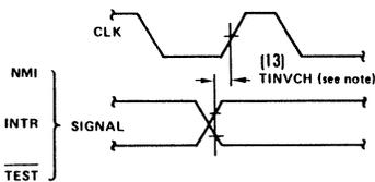
NOTE: Setup requirements for asynchronous signals only to guarantee recognition at next CLK
