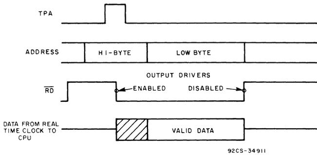
Fig. 13 - CDP1800-series memory-mapped read-cycle timing waveforms.
