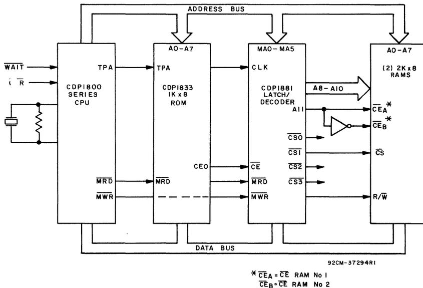
Fig. 4 - Minimum 1800-system using the CDP1881
