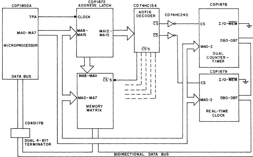
**FIGURE 5. REAL-TIME CLOCK AND COUNTER-TIMER IN MEMORY-MAPPED INTERFACE**
