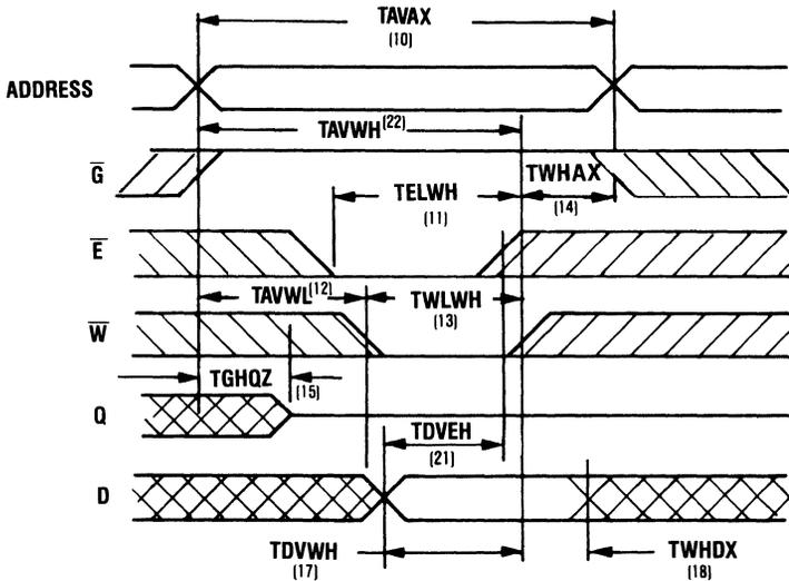
In this write cycle  $\bar{G}$  has control of the output after a period,  $T_{GHOZ}$ .  $\bar{G}$  switching the output to a high impedance state allows data in to be applied without bus contention after
