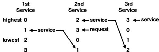
With Rotating Priority in a single chip DMA system, any device requesting service is guaranteed to be recognized after no more than three higher priority services have occurred. This prevents any one channel from monopolizing the system.
