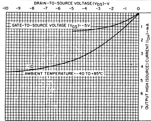
FIGURE 5. MINIMUM OUTPUT HIGH (SOURCE) CURRENT CHARACTERISTICS
