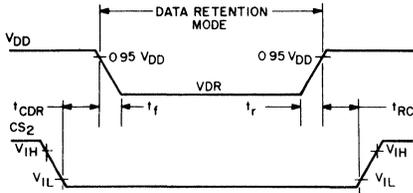
Fig. 3 - Low V<sub>DD</sub> data retention timing waveforms.
