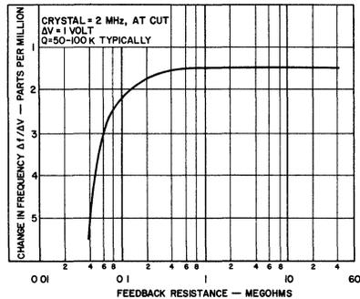
**FIGURE 4. STABILITY OF CDP1802 CRYSTAL OSCILLATOR AS A FUNCTION OF FEEDBACK RESISTOR VALUE.**
