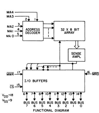
Fig 4 - Functional diagram.
