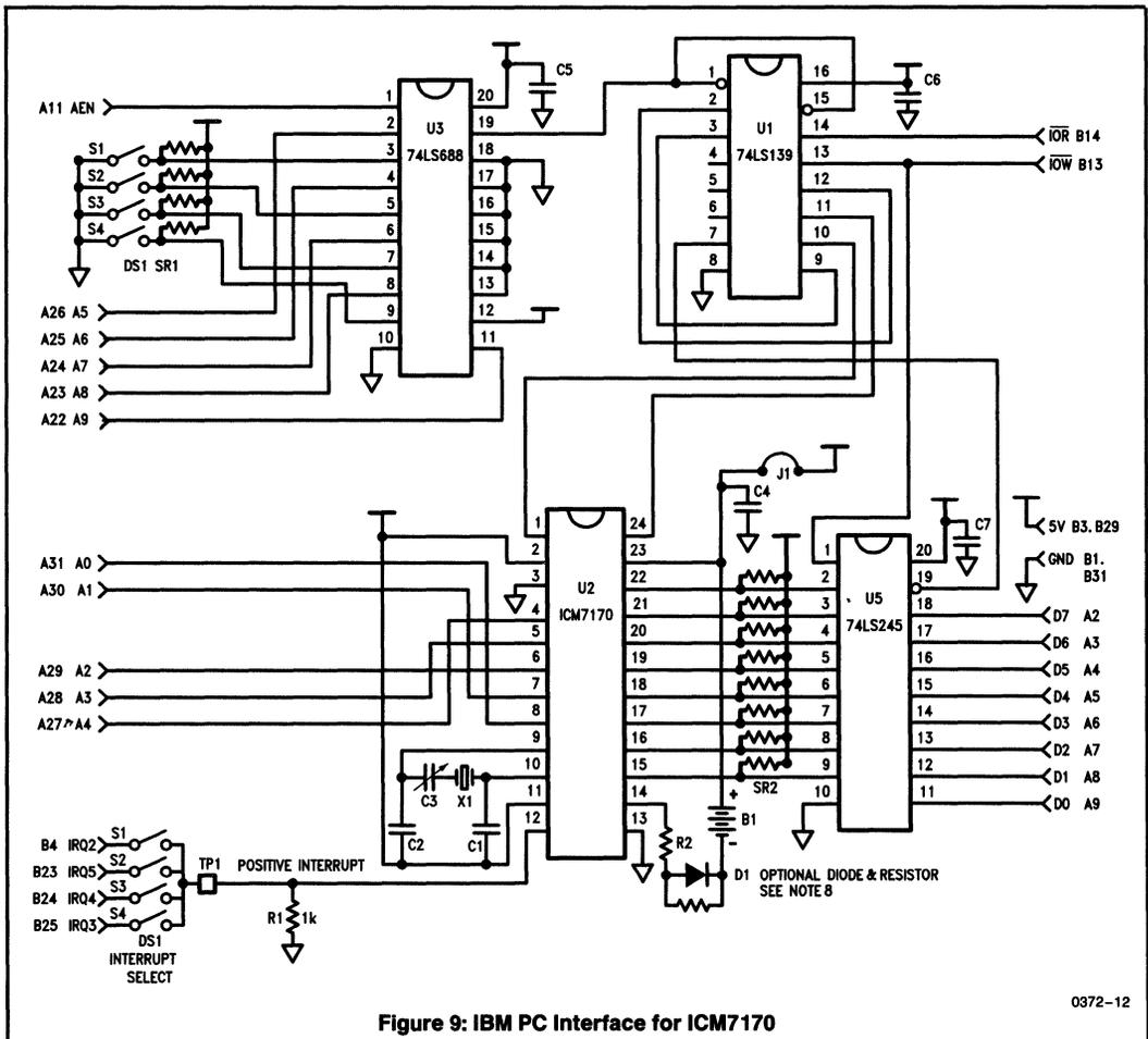
Figure 9: IBM PC Interface for ICM7170
