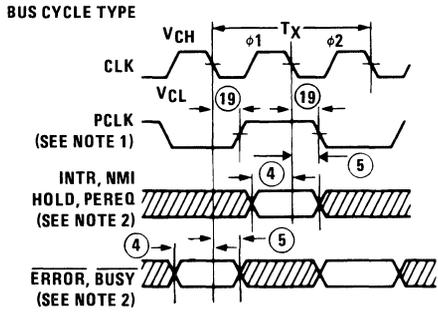
80C286/883 RESET INPUT TIMING AND SUBSEQUENT PROCESSOR CYCLE PHASE
