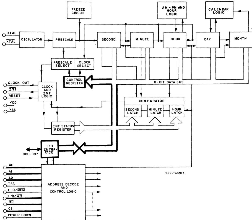
Fig. 4 - Functional diagram - control register highlighted.
