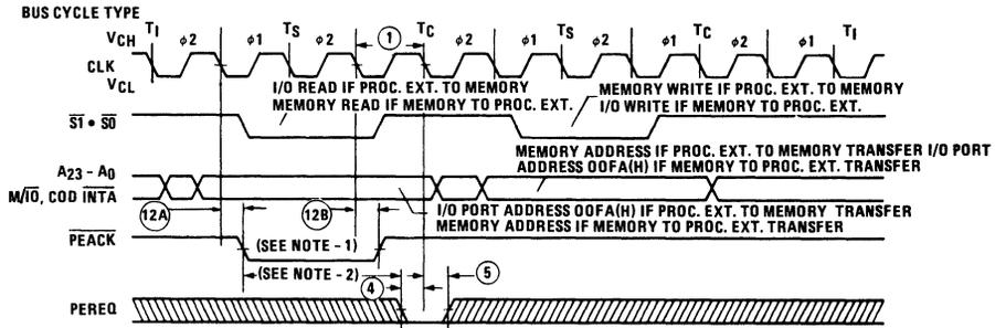
ASSUMING WORD-ALIGNED MEMORY OPERAND. IF ODD ALIGNED, 80C286 TRANSFERS TO/FROM MEMORY BYTE-AT-A-TIME WITH TWO MEMORY CYCLES.
