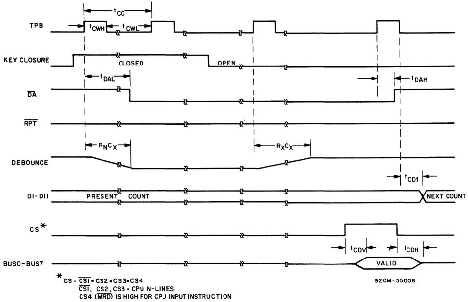
Fig 3 — CDP1871A dynamic timing diagram (non-repeat)
