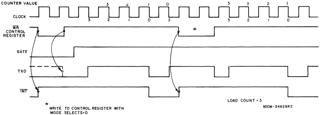
Fig. 3 - Timeout strobe (mode 2) timing waveforms.
