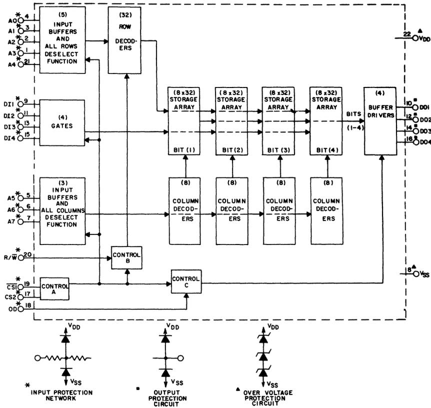
Fig. 5 - Functional block diagram for CDP1822 and CDP1822C.
