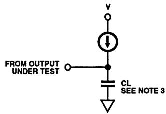
$I_{OL} = 5\text{mA}$ ,  $I_{OH} = -5\text{mA}$  for CLK and CLK50 outputs
