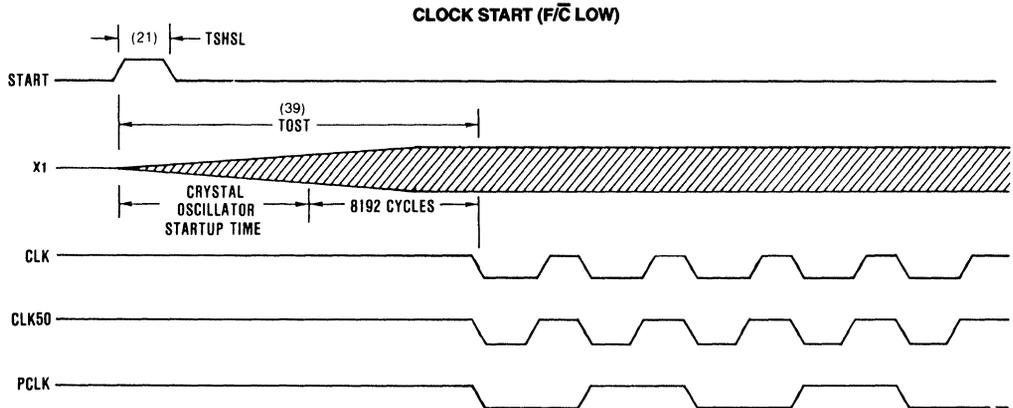
NOTE: Start up count begins when the crystal oscillator reaches a suitable threshold level.
