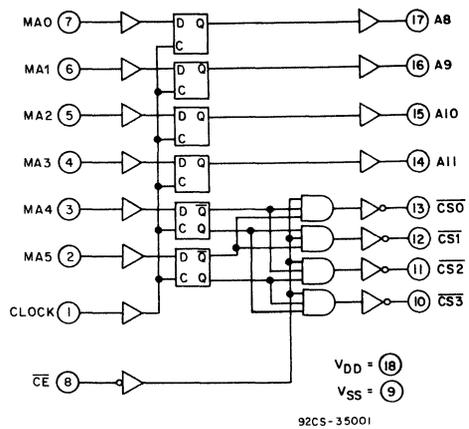
Fig. 2 - Functional diagram for the CDP1882, CDP1882C.
