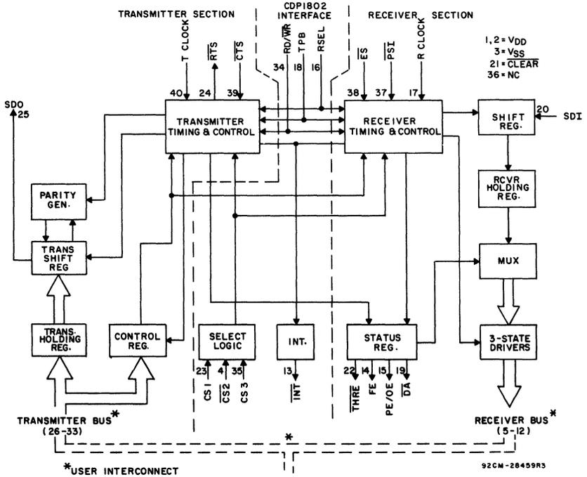
Fig. 1 - Mode 1 block diagram (CDP1800-series microprocessor compatible).
