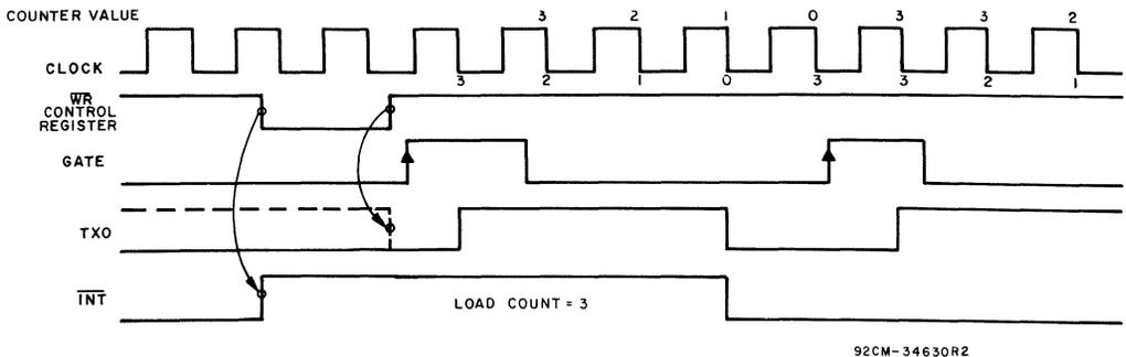
Fig. 4 - Gate controlled one-shot (mode 3) timing waveforms.
