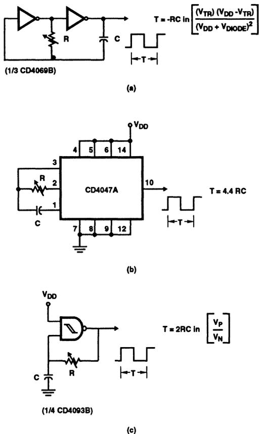
FIGURE 5. THREE SIMPLE RC-CONTROLLED OSCILLATOR CIRCUITS SUITABLE FOR USE AS EXTERNAL CLOCK FOR CDP1802 MICROPROCESSOR (OUTPUT CONNECTED TO PIN 1 THROUGH EVALUATION KIT P2-W).
