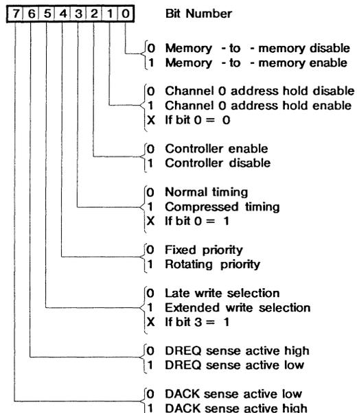
**Mode Register** - Each channel has a 6-bit Mode register associated with it. When the register is being written to by the microprocessor in the Program Condition, bits 0 and 1 determine which channel Mode register is to be written. When the processor reads a Mode register, bits 0 and 1 will both be ones. See the following diagram and Figure 4 for Mode register functions and addresses.
