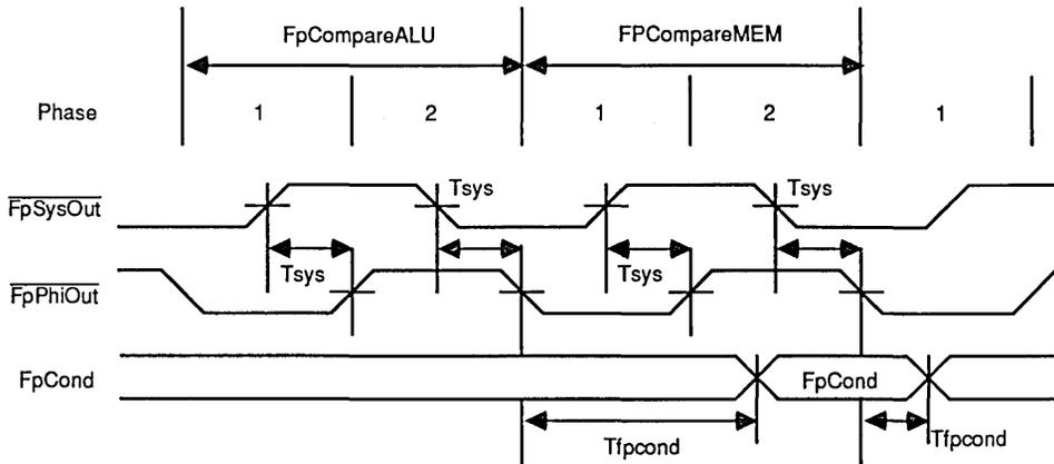
Figure 11. Floating Point Condition Timing
