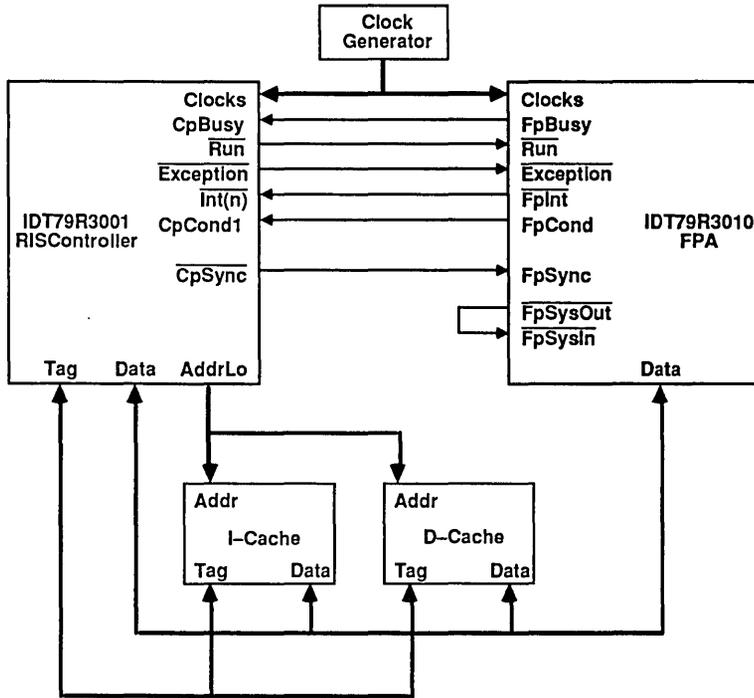
Figure 8. IDT79R3001 Interface to IDT79R3010 Floating Point Co-Processor
