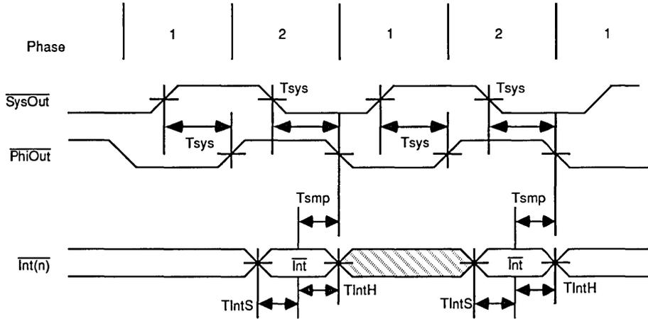
Figure 18. Interrupt Timing
