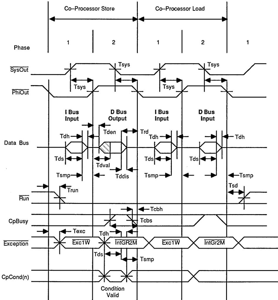
Figure 17. Co-Processor Load/Store Timing
