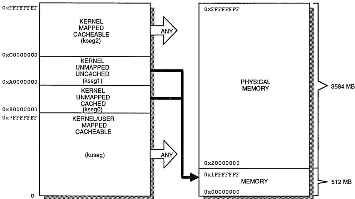
Figure 6. IDT79R3000 Virtual Address Mapping
