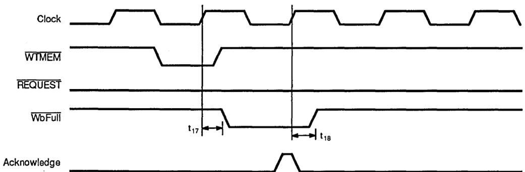
Figure 10.  $\overline{WbFull}$  Signal Timing Specifications
