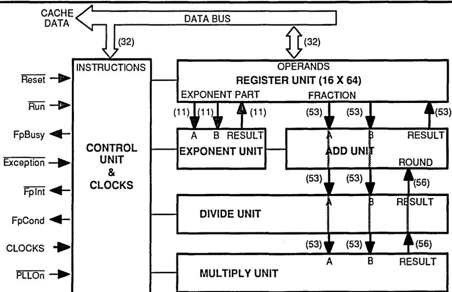
Figure 1. IDT79R3010 Functional Block Diagram
