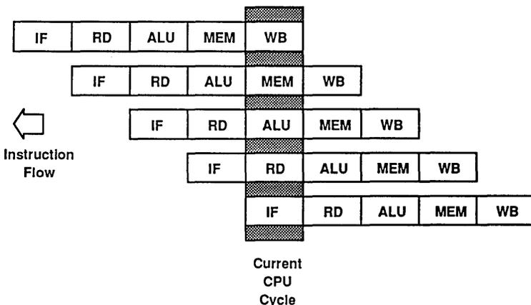
Figure 3. Instruction Execution in IDT79R3001 Pipeline
