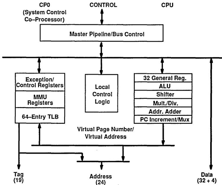
Figure 1. IDT79R3001 Block Diagram
