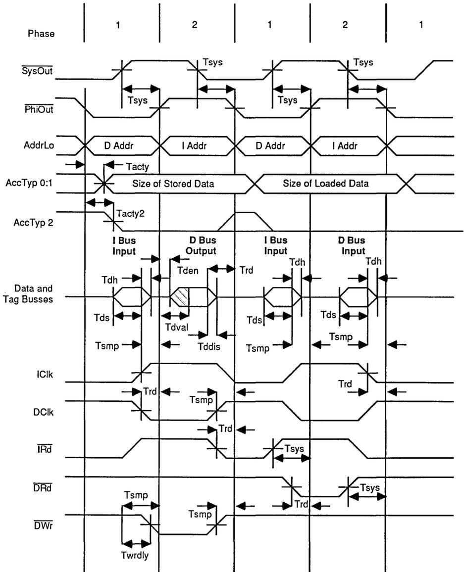
Figure 18. Synchronous Memory (Cache) Timing
