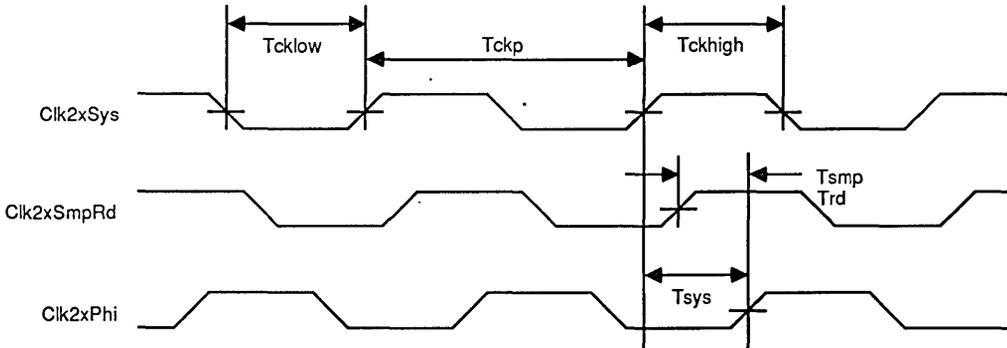
Figure 16. Input Clock Timing
