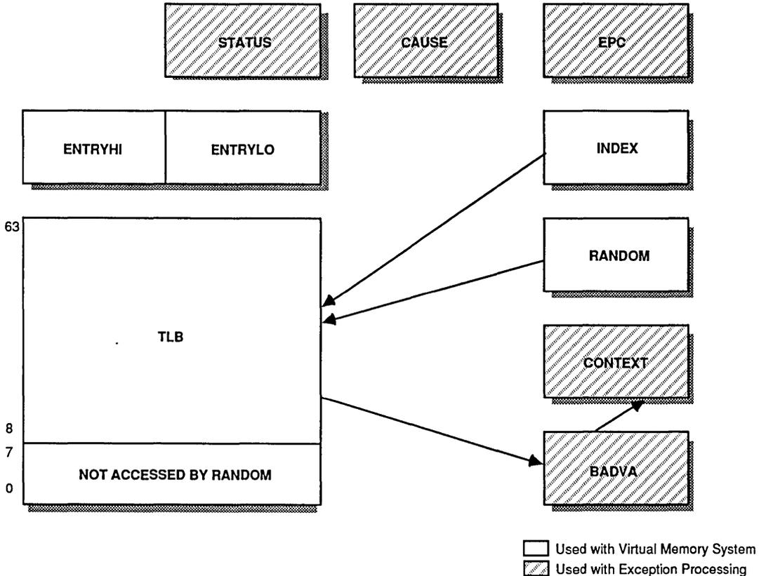
Figure 4. The System Coprocessor Registers
