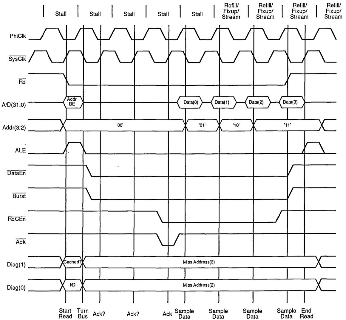
Figure 7. IDT R3051 Family Burst Read Operation (Two Bus Wait Cycles)
