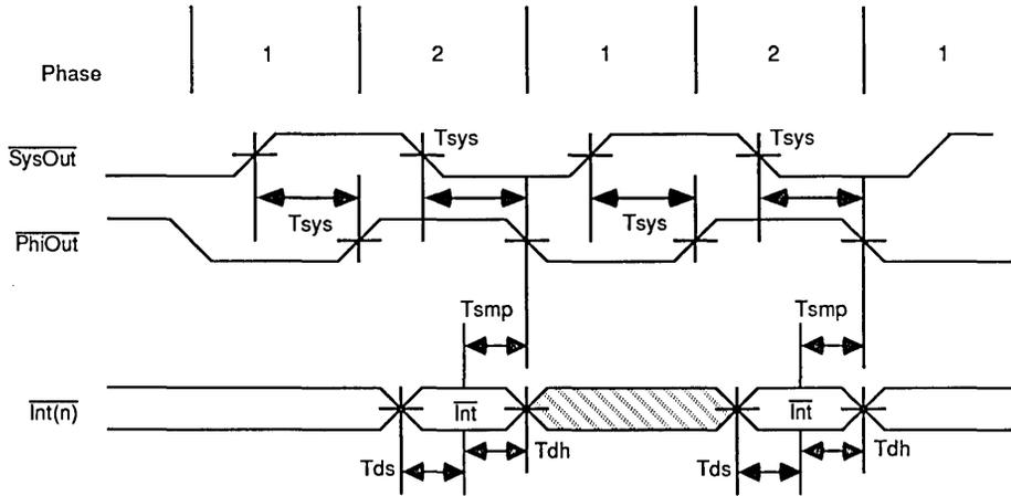
Figure 18. Interrupt Timing
