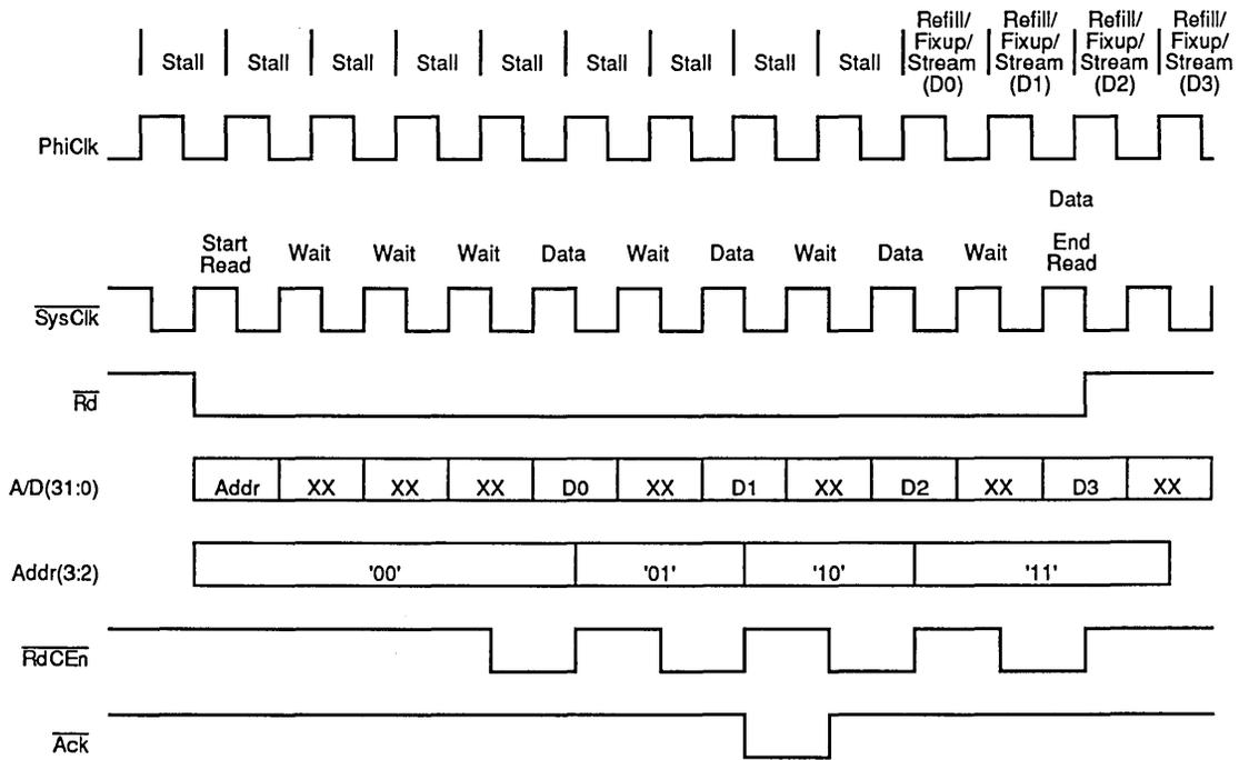
Figure 8. IDT R3051 Family Throttled Quad Read Operation (Three Bus Wait Cycles, One Bus Wait Cycle Between Words)
