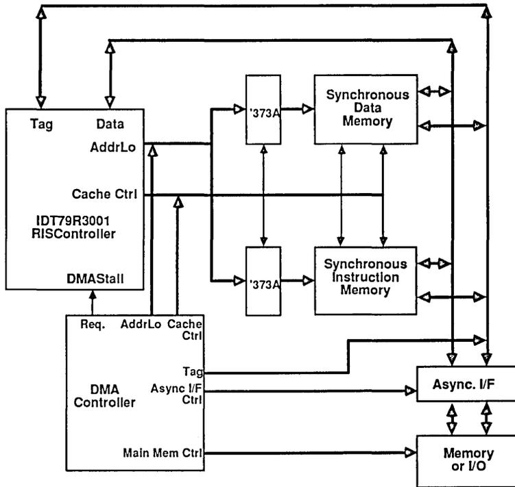
Figure 9. IDT79R3001 DMA Interface
