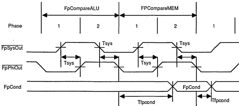
Figure 11. Floating Point Condition Timing
