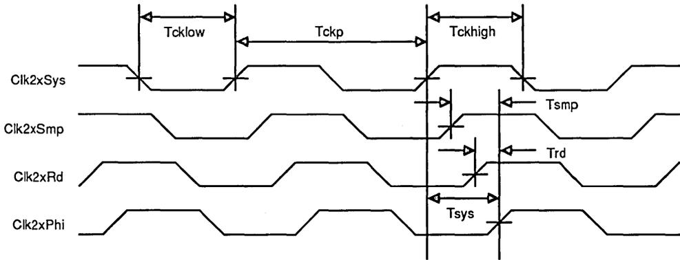
Figure 12. Input Clock Timing
