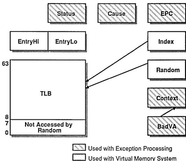
Figure 12. System Control Co-processor (CP0) Registers
