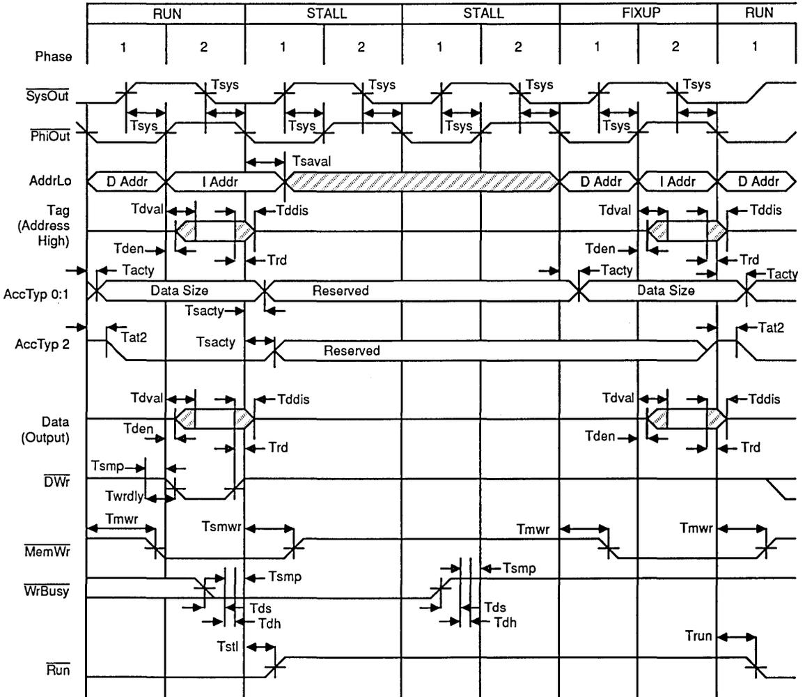
Figure 19. Memory Write Timing
