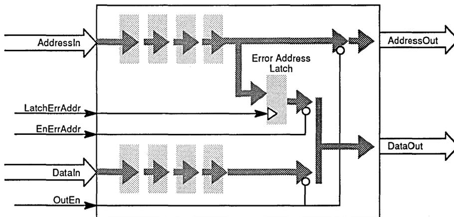
Figure 8. The Write Buffer Error Address Latch
