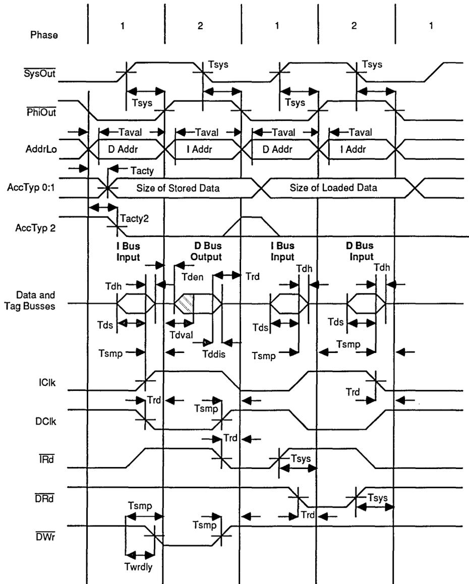
Figure 14. Synchronous Memory (Cache) Timing
