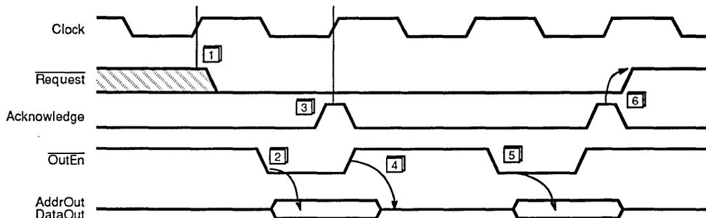
Figure 6. Write Buffer — Main Memory Interface Timing
