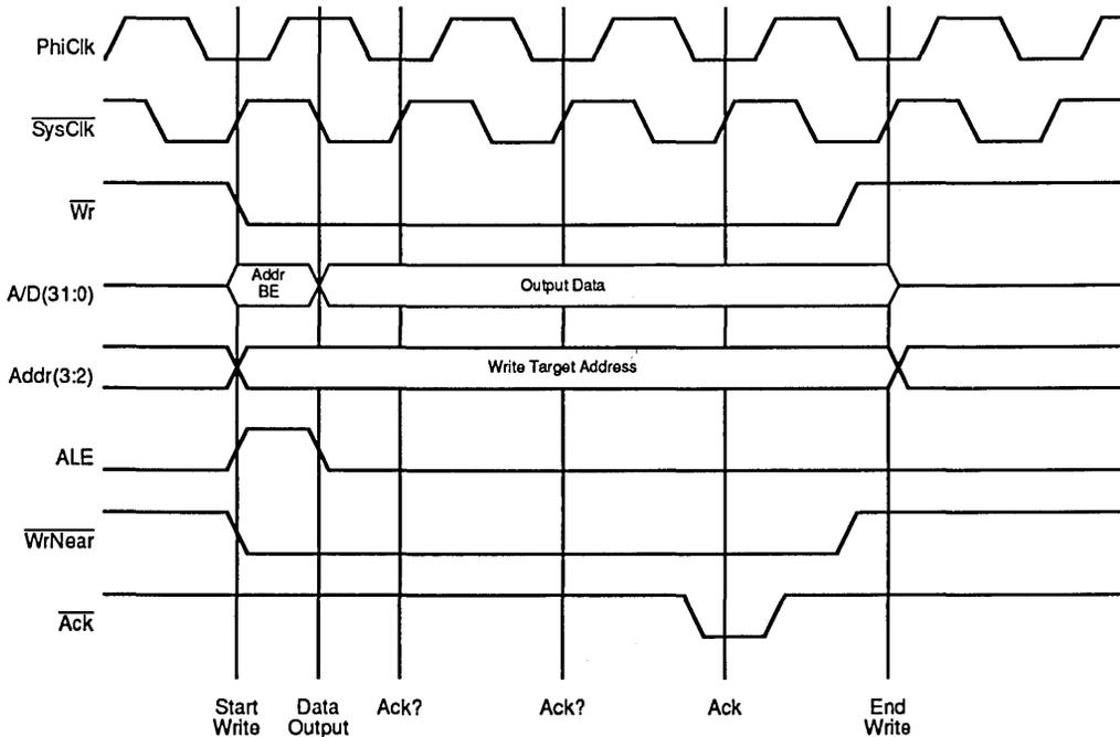
Figure 5. IDT R3051 Family Write Operation (Two Bus Wait Cycles)
