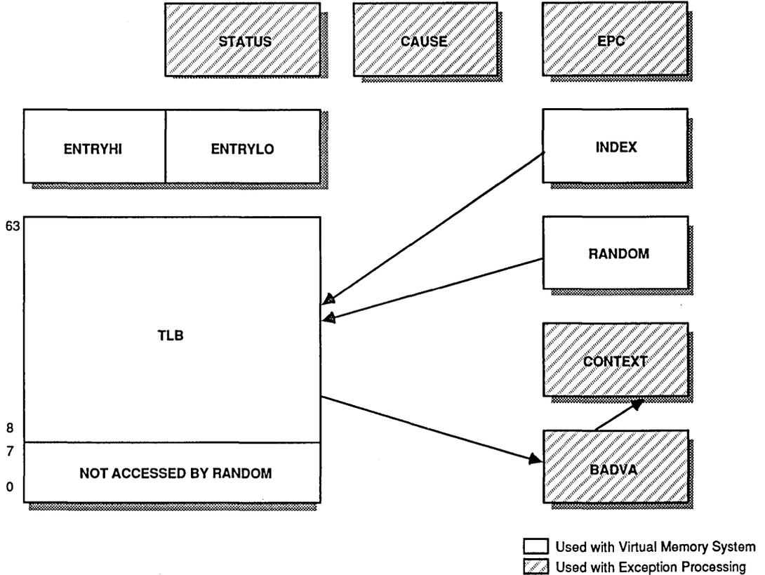
Figure 4. The System Coprocessor Registers
