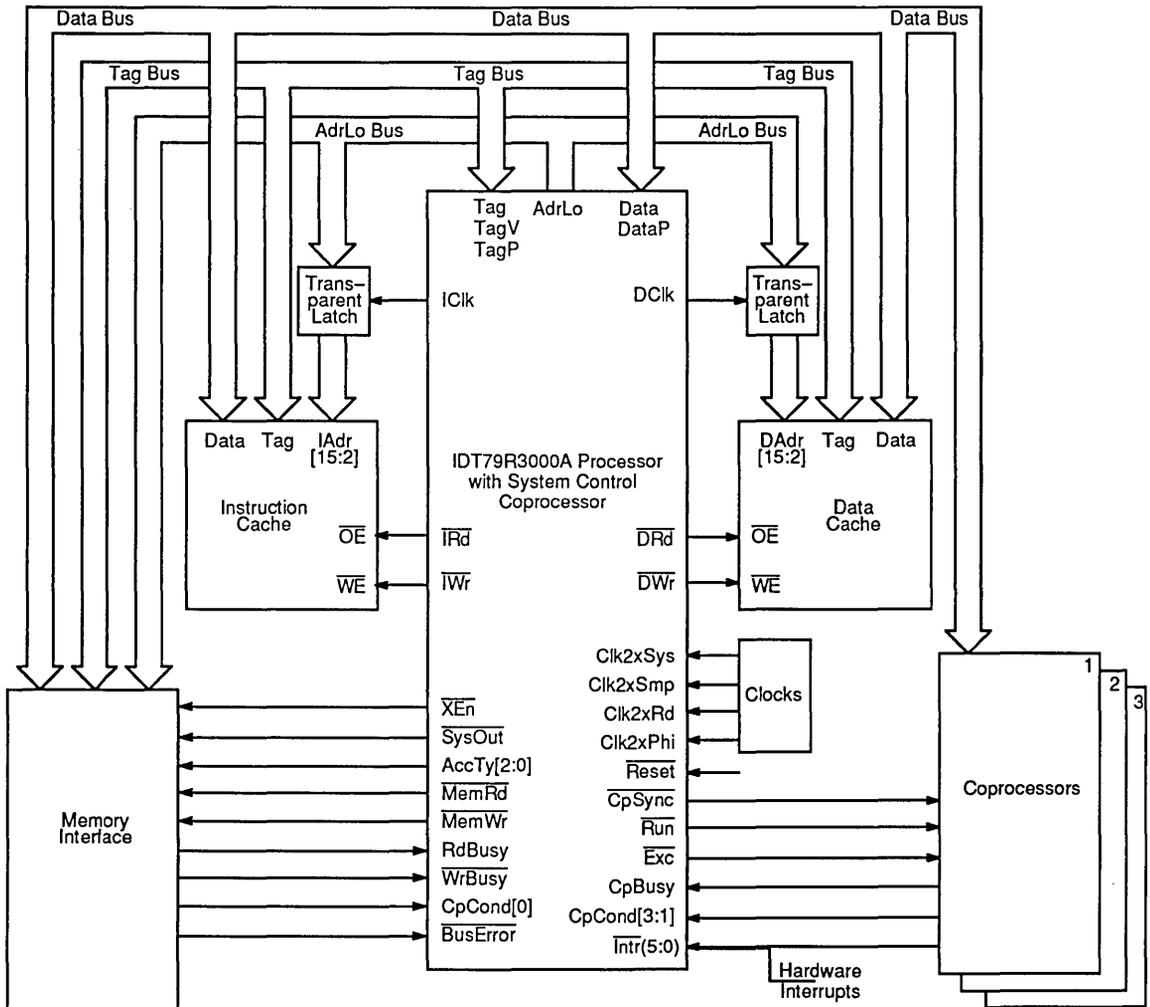
Figure 11. IDT79R3000A Subsystem Interfaces Example; 64 KB Caches
