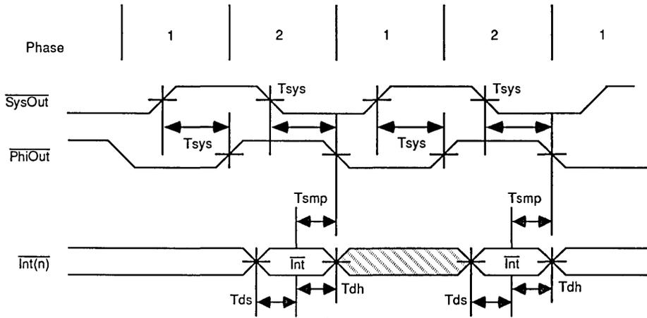
Figure 22. Interrupt Timing
