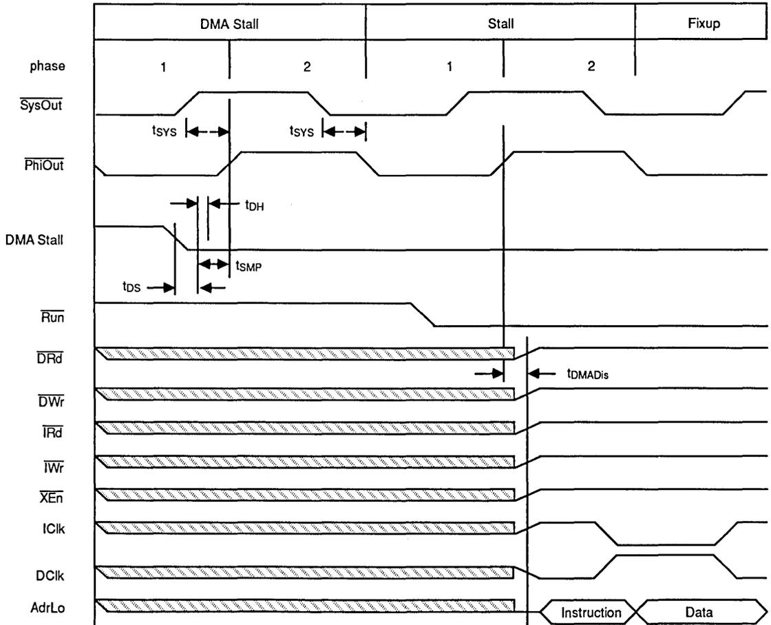
Figure 24. Entering DMA Stall
