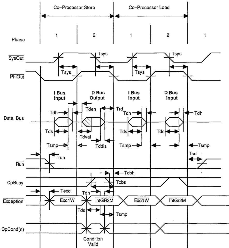
Figure 21. Co-Processor Load/Store Timing
