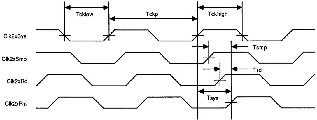
Figure 6. Input "2x" Clock Timing
