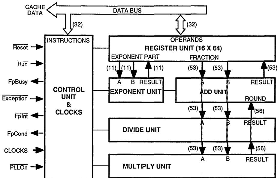
Figure 1. IDT79R3010A Functional Block Diagram
