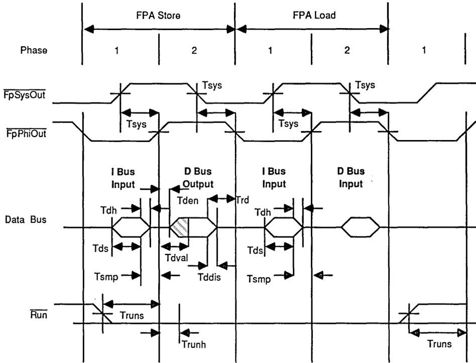
Figure 8. Floating Point Load/Store Timing
