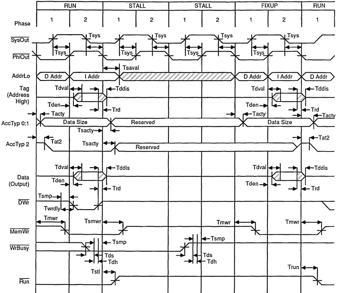
Figure 15. Memory Write Timing
