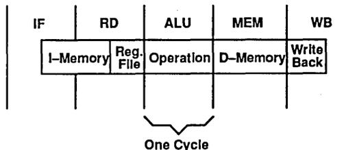
Figure 2. IDT79R3001 Five-Stage Pipeline
