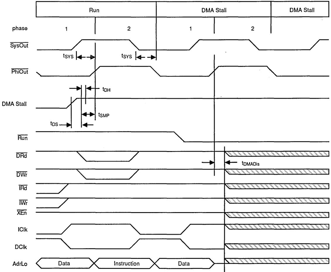
Figure 25. Completing DMA Stall
