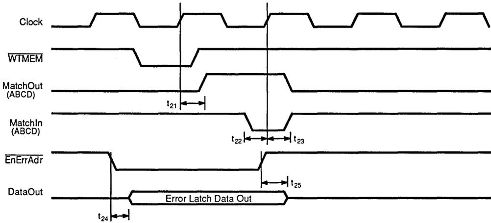
Figure 12. Match and Error Latch Timing Specifications
