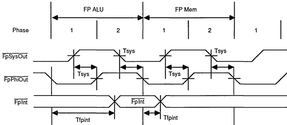
Figure 10. Floating Point Interrupt Timing
