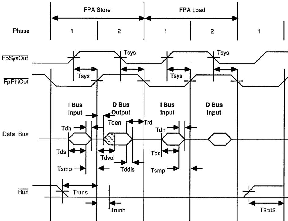
Figure 8. Floating Point Load/Store Timing
