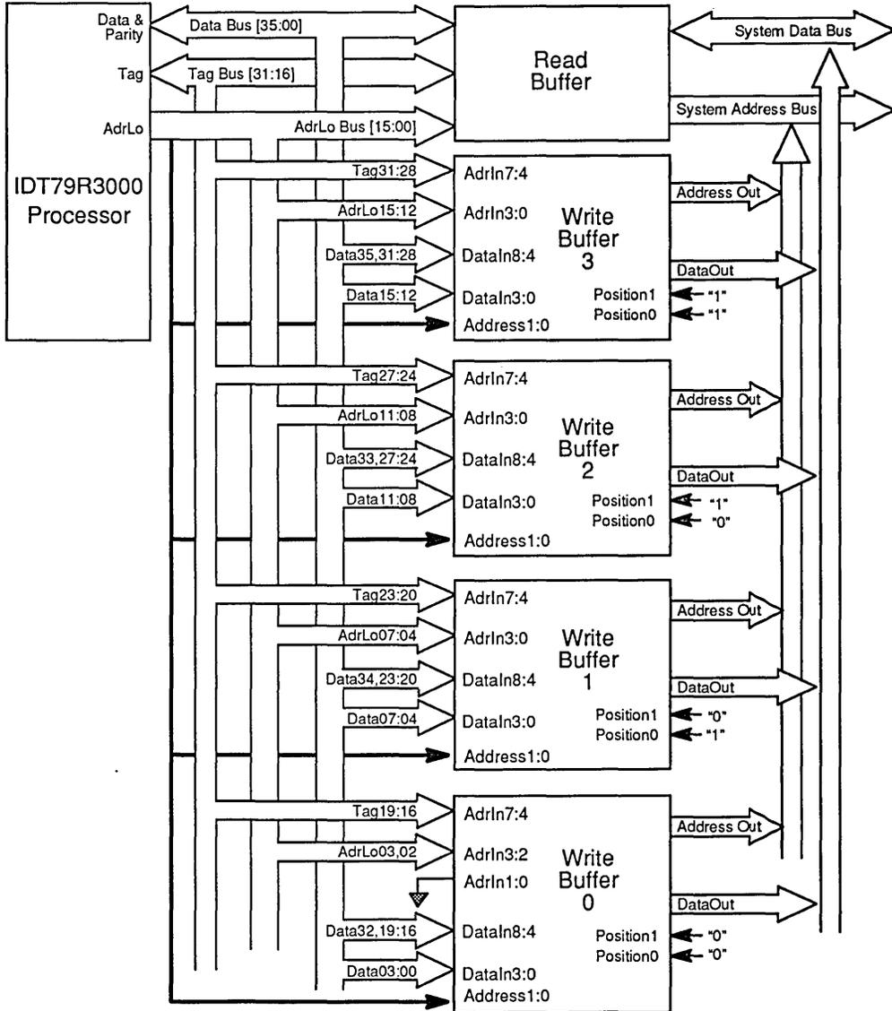
Figure 3. Write Buffer Data and Address Line Connections
