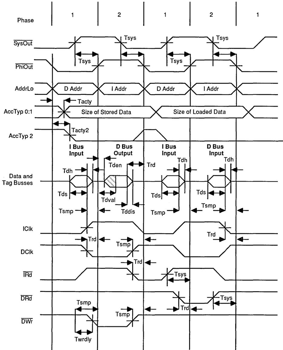
Figure 14. Synchronous Memory (Cache) Timing
