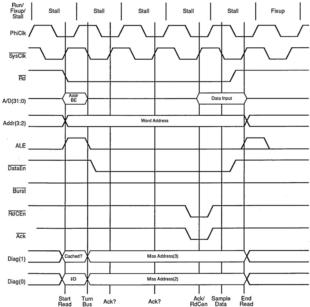
Figure 6. IDT R3051 Family Single Word Read Operation (Two Bus Wait Cycles)
