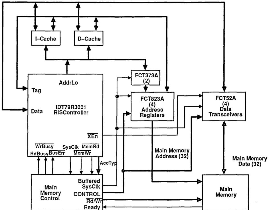
Figure 7. IDT79R3001 Asynchronous Interface
