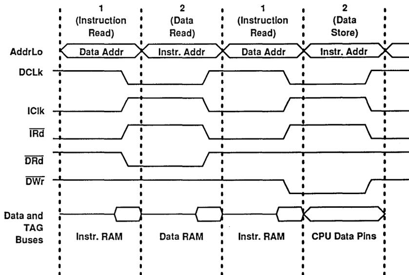
Figure 4. Synchronous Memory Control Timing
