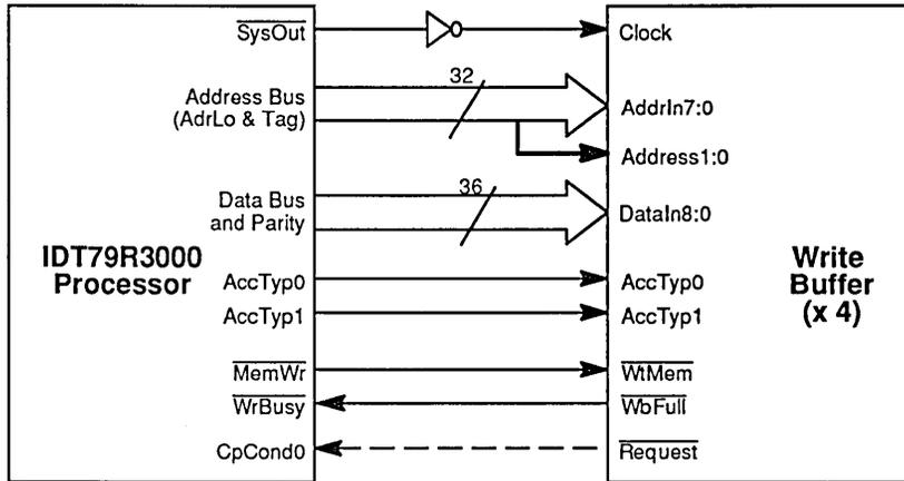
Figure 2. Write Buffer — IDT79R3000 Processor Interface
