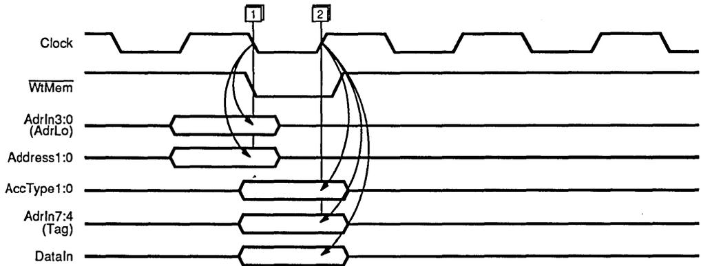
Figure 4. Processor — Write Buffer Interface Timing
