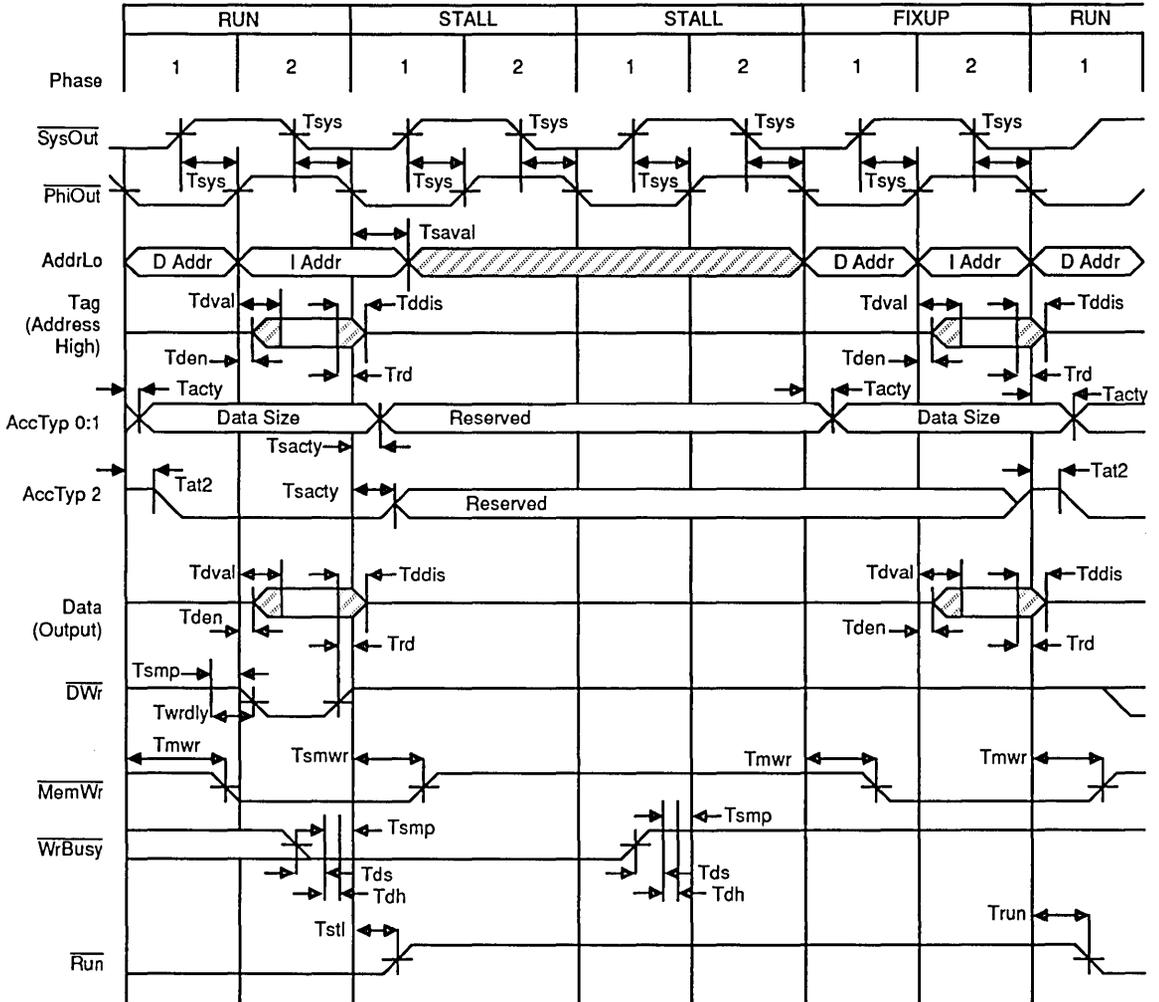
Figure 15. Memory Write Timing
