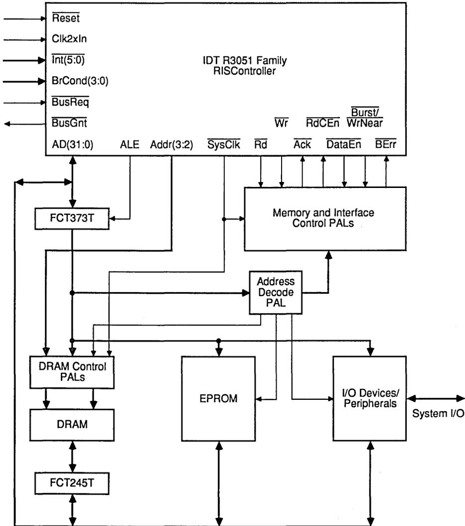
Figure 9. Typical R3051 Family Based System
