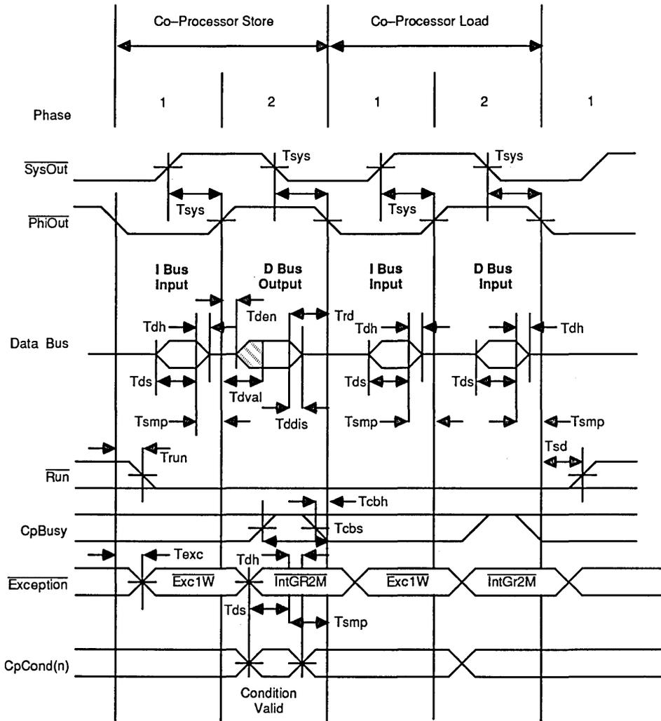
Figure 17. Co-Processor Load/Store Timing
