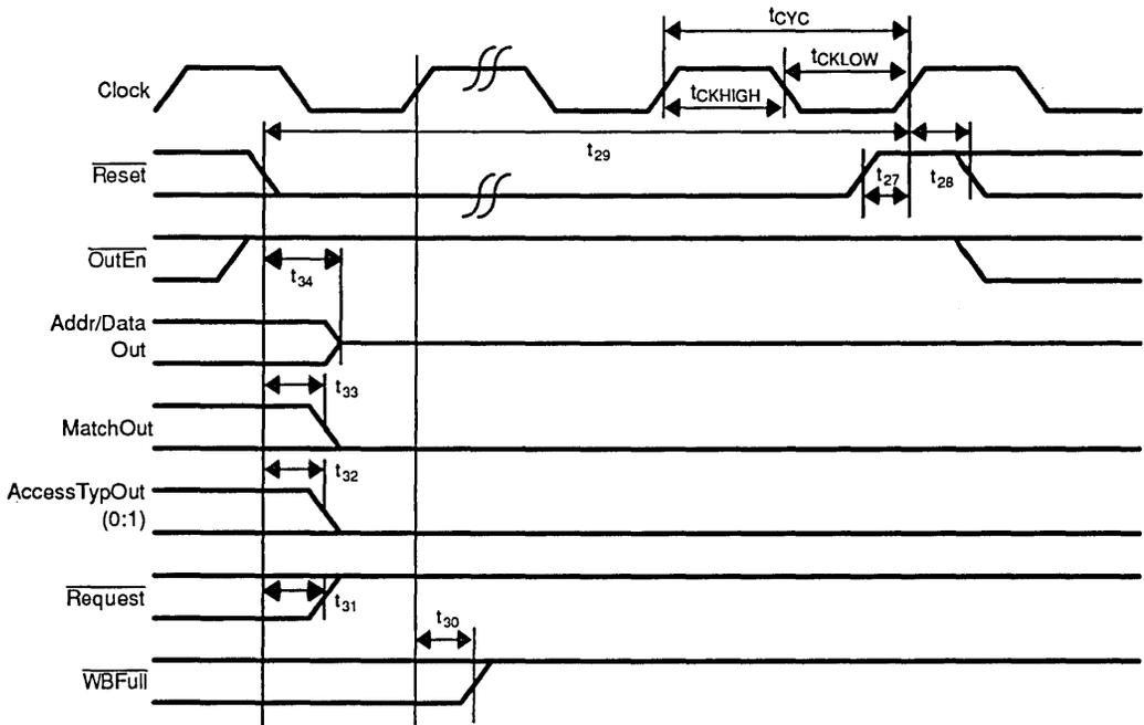
Figure 14. Reset Timing
