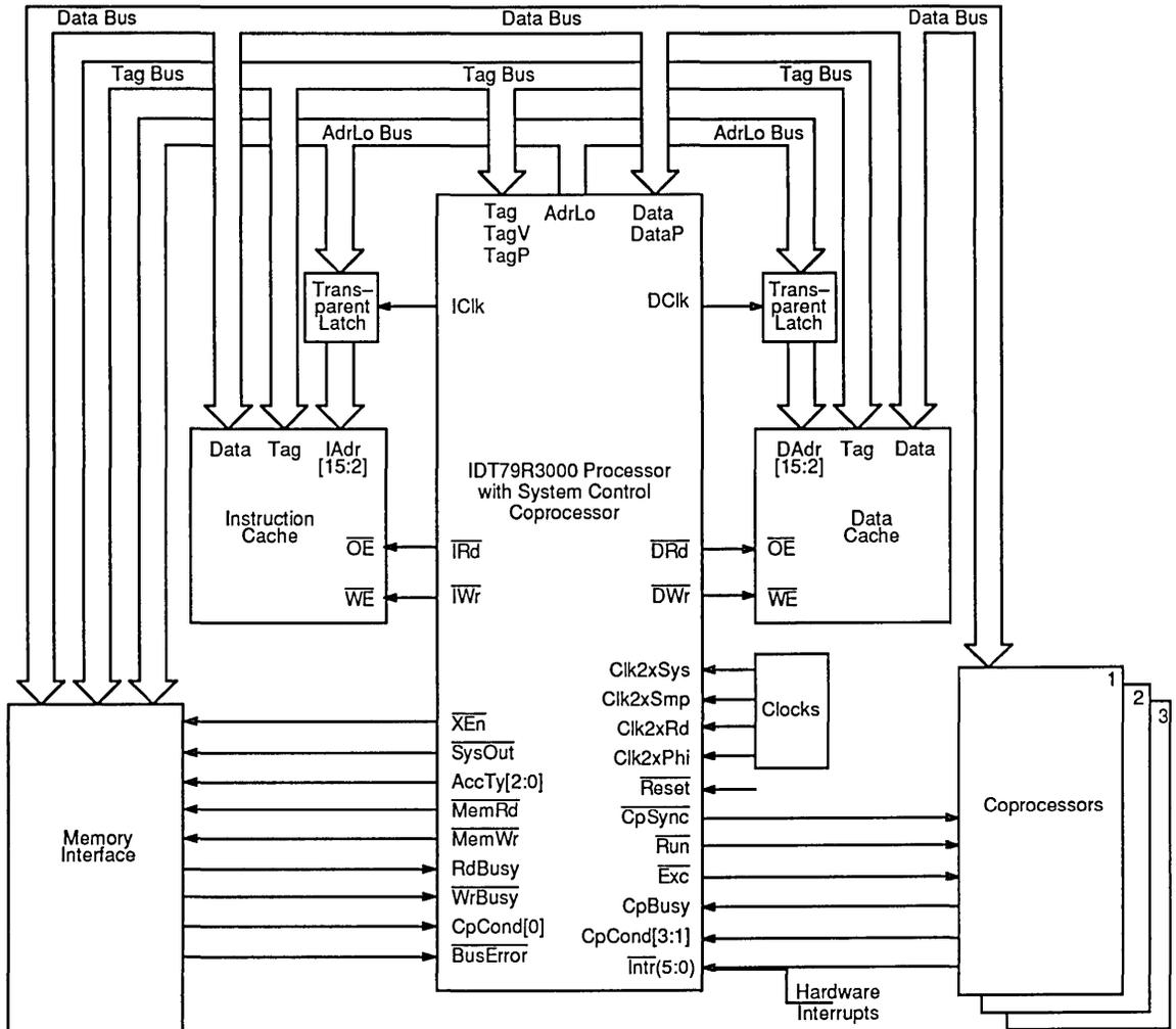
Figure 11. IDT79R3000 Subsystem Interfaces Example; 64 KB Caches
