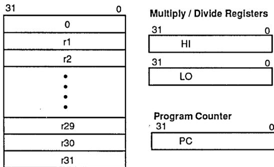
Figure 2. IDT79R3000A CPU Registers
