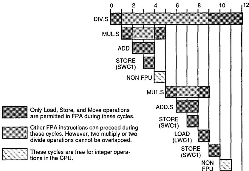
Figure 3. Examples of Overlapping Floating Point Operation
