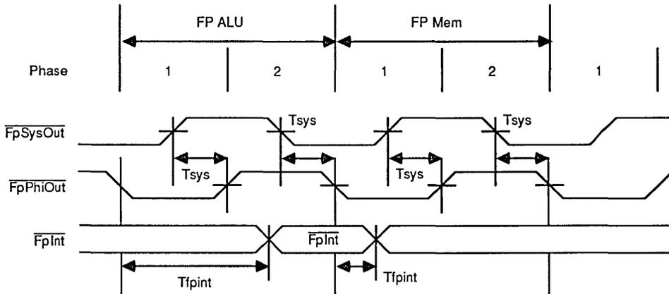
Figure 10. Floating Point Interrupt Timing
