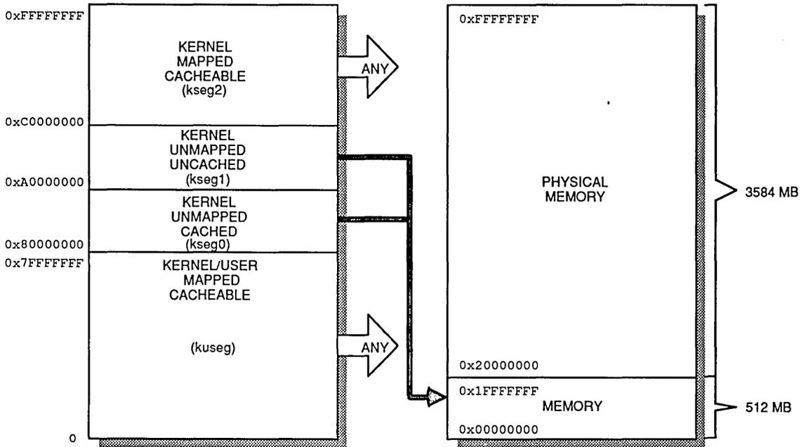
Figure 6. IDT79R3000A Virtual Address Mapping
