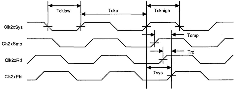
Figure 12. Input Clock Timing
