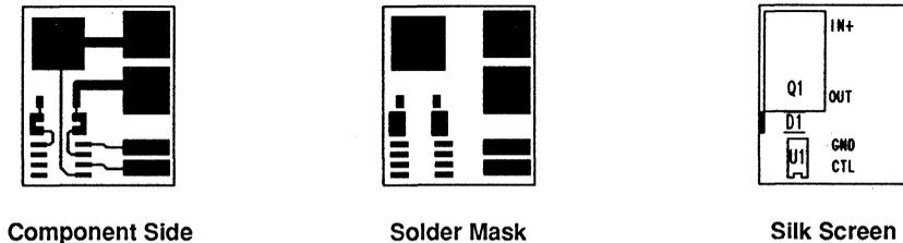
Figure 6. MIC5011 DB-1 Board Layout
