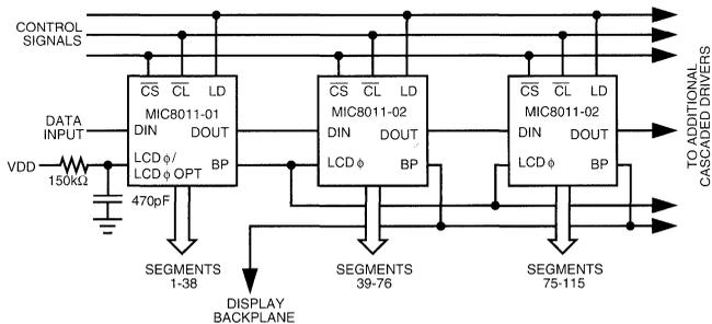
Figure 3. Cascading with Internal Clock Oscillator - Option -01
