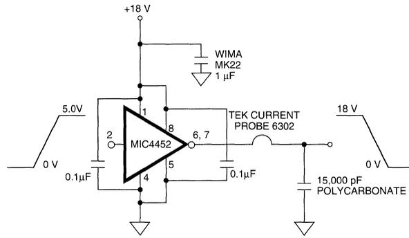
Figure 6. Peak Output Current Test Circuit
