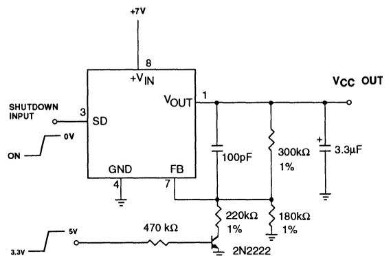
PIN 3 LOW= ENABLE OUTPUT. Q1 ON = 3.3V, Q1 OFF = 5.0V.
