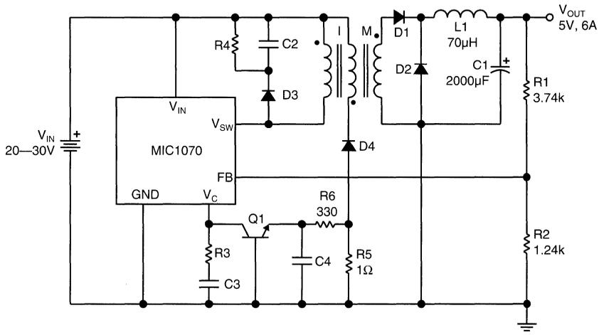
Figure 17. Forward Converter
