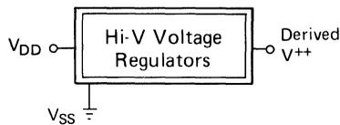
Extra high voltage ( $V^{++}$ ) is normally derived using a voltage "doubler."  $V^{++}$  is needed to power the level shifters used to pull the N-channel DMOS gates above  $V_{DD}$ . An external clamping zener diode holds  $V^{++}$  at 15V to 20V above  $V_{DD}$  (for  $V_{DD} \geq 20V$ ). This zener diode gives over voltage protection to the level shifters, while holding  $V^{++}$  at 18V to 20V above  $V_{DD}$ .
