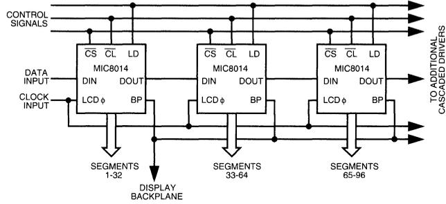
Figure 3. Cascading with External Clocking Source - 02 Option
