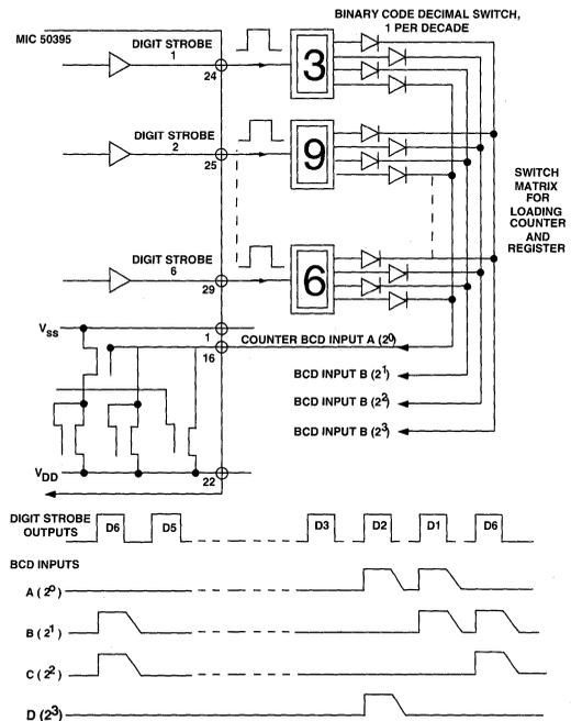
NOTE: THAT INPUT LINES ARE ALL PULLED TO  $V_{DD}$  DURING INTERDIGIT BLANKING
