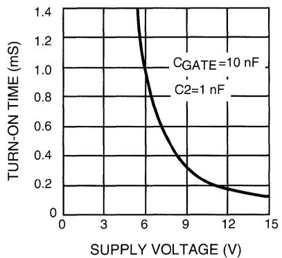
\* Time for gate to reach  $V^+ + 5V$  in test circuit with  $V_S = V^+ - 5V$ .
