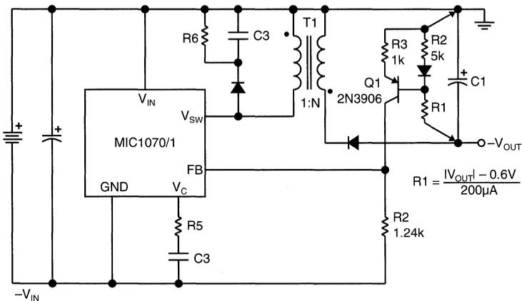
Figure 16. Negative Input-Output Flyback Converter
