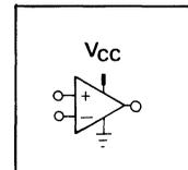
All of the linear macro implementations, with the exception of the linear buffer, are intended to drive light loads (i.e. another op amp, a comparator, a gate, etc.) and so they are tested with high impedance loads on the order of a megaohm. Gain degradation should be expected at loads of 100K ohms or less.
