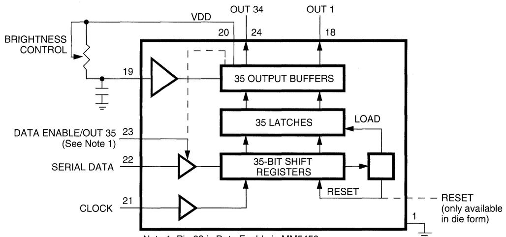
Note 1: Pin 23 is Data Enable in MM5450
