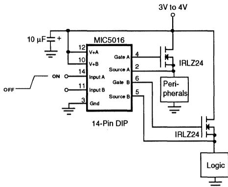
Figure 2: 3 to 4 V Dual Sleep Mode Switch
