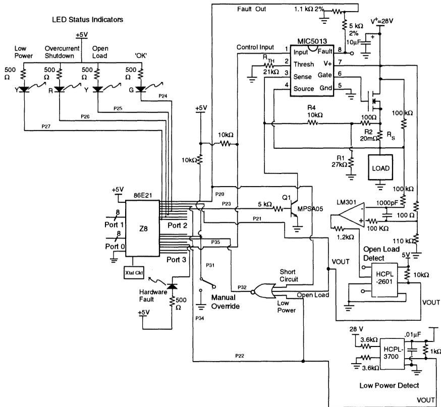
Figure 5: Z8 Based Power Controller
