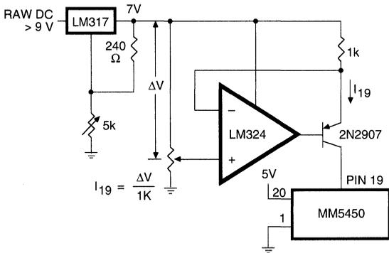
Figure 10. Typical Application of Constant Current Brightness Control
