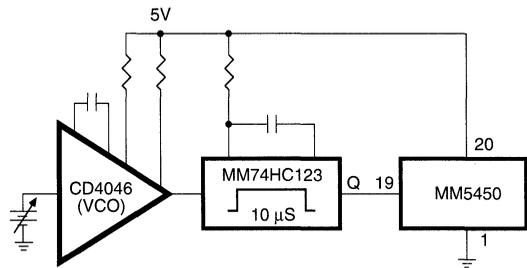
Figure 11. Brightness Control Varying the Duty Cycle
