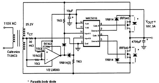
Figure 14: High Efficiency 60 Hz Synchronous Rectifier
