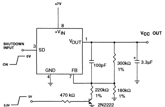
PIN 3 LOW= ENABLE OUTPUT. Q1 ON = 3.3V, Q1 OFF = 5.0V.
