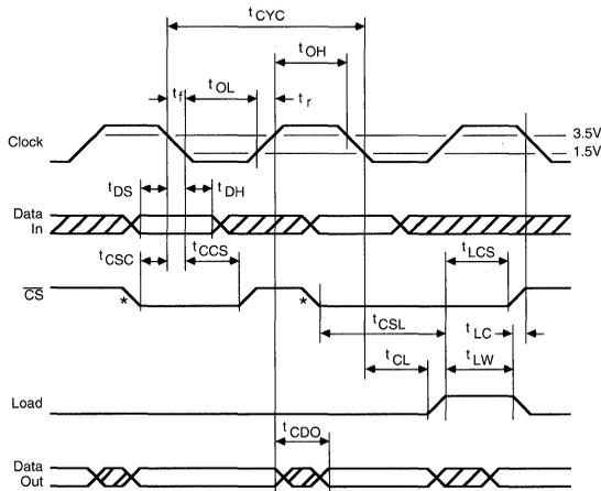
\* The CS high-to-low transition will generate a clock pulse.
