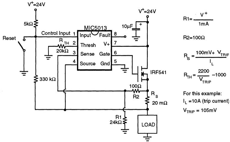
Figure 1: Basic Circuit Breaker/Switch Configuration
