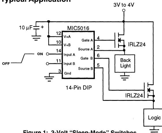
Figure 1: 3-Volt "Sleep-Mode" Switches with Logic Level FETs
