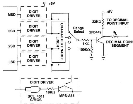
**FIG. 11: CLOCKING DECIMAL POINT INPUT FOR COMMON-CATHODE LED'S**
