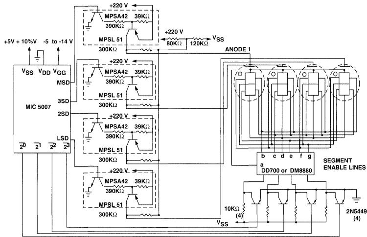
**FIG. 9: INTERFACING WITH FILAMENT DISPLAYS
