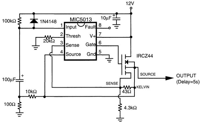
**Figure 12. Time-Delay Relay with 30A Over-Current Protection**
