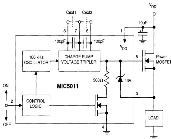
Figure 3. MIC5011 Block Diagram and Typical Application
