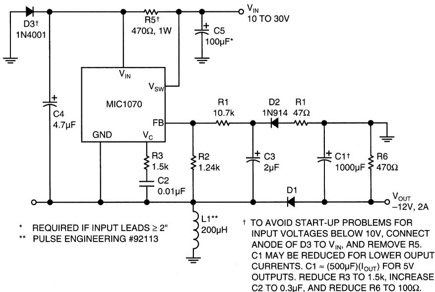
Figure 7. Positive to Negative Buck-Boost Converter
