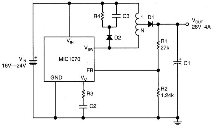
Figure 10. Current Boosted Boost Converter
