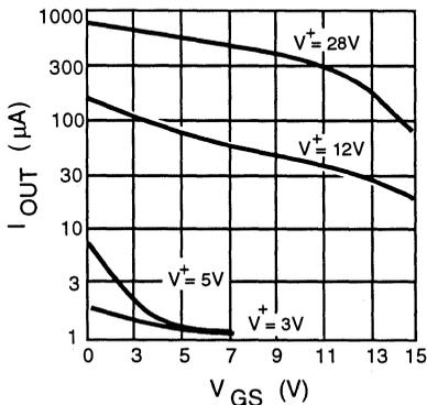
**Charge Pump Output Current, VGS = Ground**
