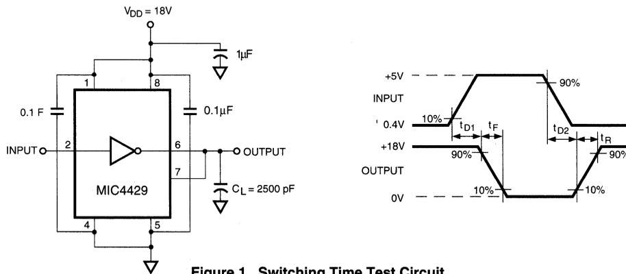
**Figure 1. Switching Time Test Circuit**
