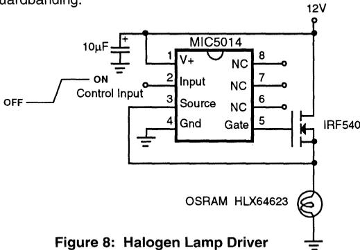
Figure 8: Halogen Lamp Driver
