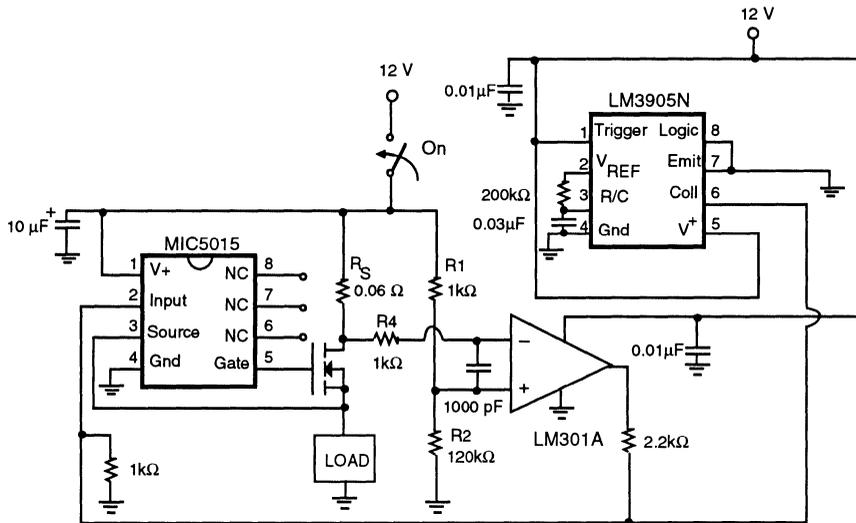
Figure 5: High Side Driver With Delayed Overcurrent Shutdown
