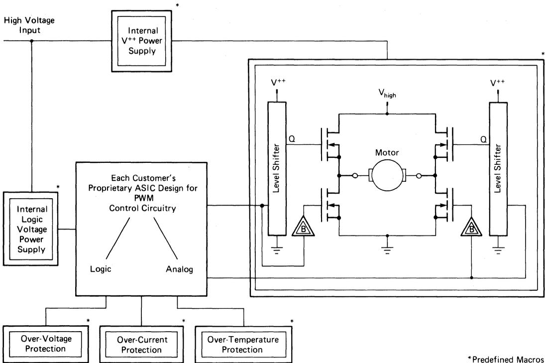
The above motor control application shows how a mixture of predefined macros and customer proprietary ASIC control circuits are used to make a circuit optimally fit an application. Each transistor in the bridge can be a single DMOS FET, or 2 to 4
