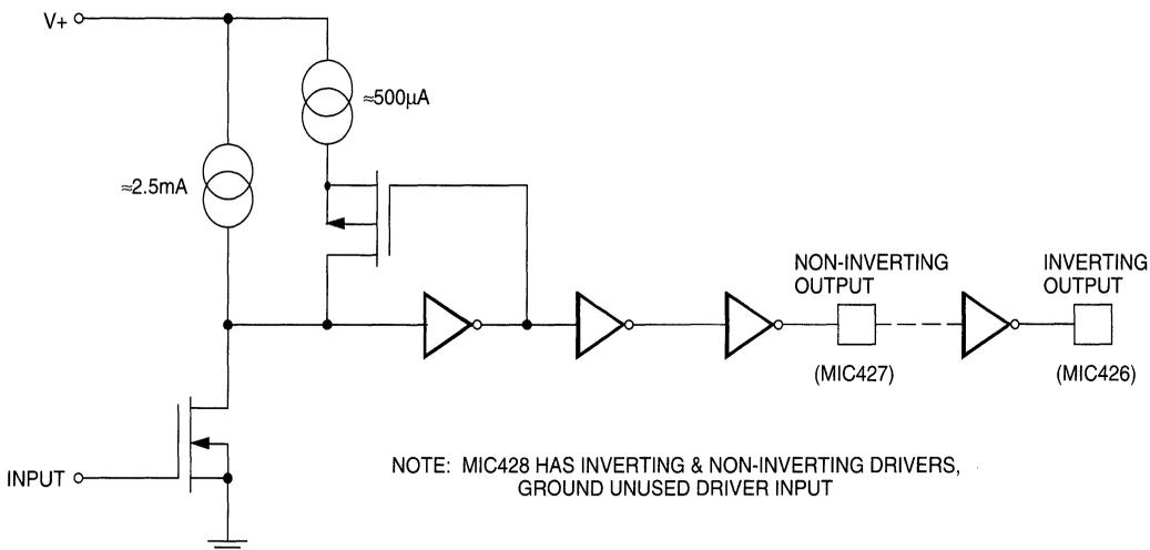
Quiescent power supply current is 8mA maximum. The MIC426 requires 1/5 the current of the pin compatible bipolar DS0026 device. This is important in DC to DC converter applications with power efficiency constraints and high frequency switch mode power supply applications. Quiescent current is typically
