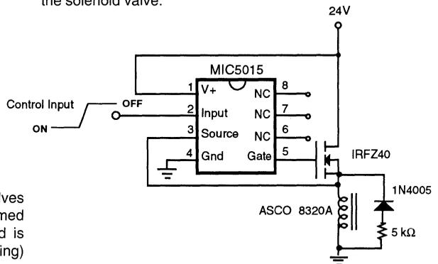
Figure 7: Solenoid Valve Driver
