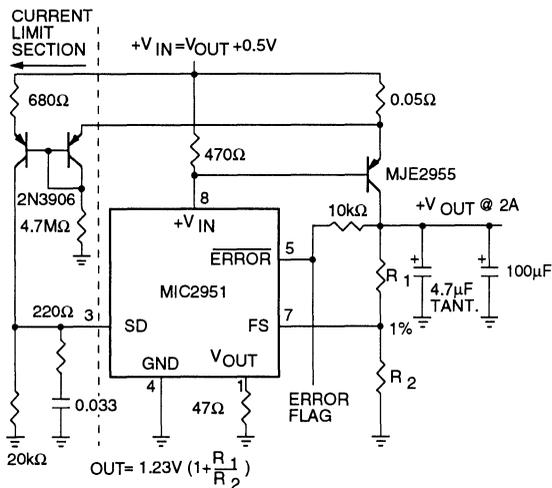
FOR 5  $V_{OUT}$ , USE INTERNAL RESISTORS. WIRE PIN 6 TO 7, AND WIRE PIN 2 TO  $+V_{OUT}$  BUS.
