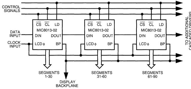
Figure 3. Cascading with External Clocking Source - 02 Option
