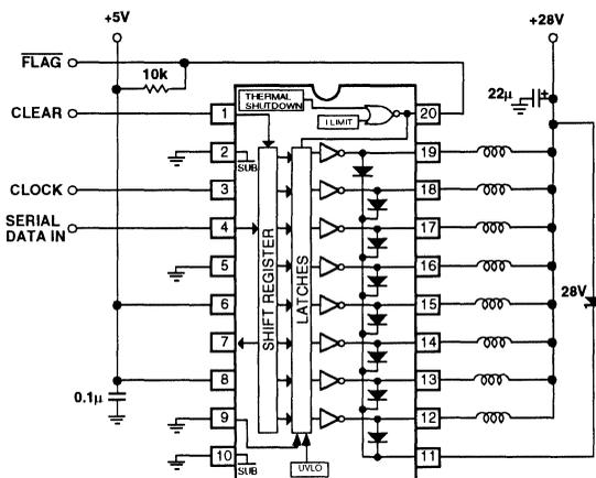
Protected Level Shifting Lamp Driver with Darlington Emitters Tied To a Negative Supply
