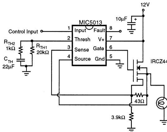
$$R_S = \frac{SR(V_{TRIP} + 100mV)}{R_L - (V_{TRIP} + 100mV)}$$
