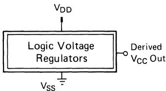
Internal regulators can generate local low level digital/analog voltages ( $V_{CC}$ ) from a single  $V_{DD}$  high voltage supply of 20 Volts to 100 Volts or extra high ( $V^{++}$ ) voltages above  $V_{DD}$ .
