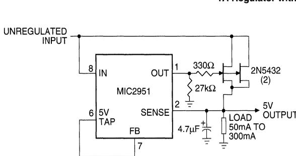
300 mA Regulator with 0.75 V Dropout
