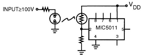
HIGH VOLTAGE INPUT (POSITIVE OR NEGATIVE POLARITY)
