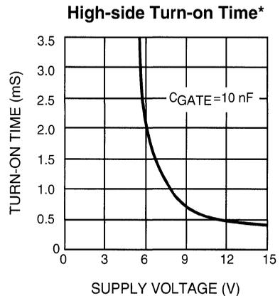
\* Time for gate to reach  $V^+ + 5V$  in test circuit with  $V_S = V^+ - 5V$  (prevents gate clamp from interfering with measurement).
