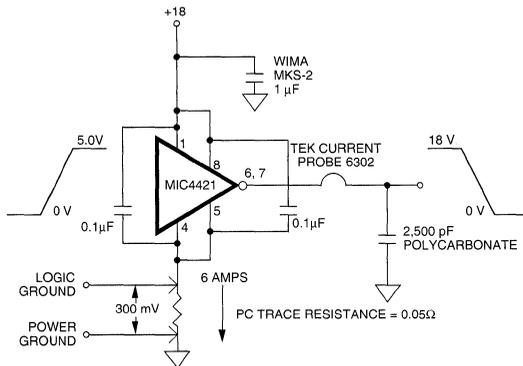
**Figure 5. Switching Time Degradation Due to Negative Feedback**
