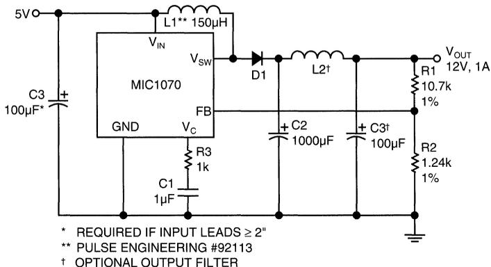
Figure 1. Boost Converter (5V to 12V)
