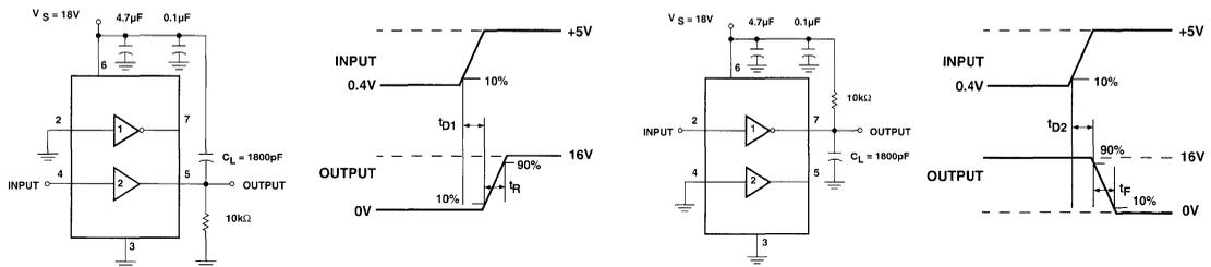
Figure 1. MIC4403 Switching time test circuit.
