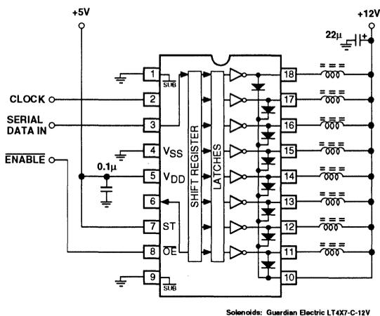
**MIC5841 Level Shifting Lamp Driver with Darlington Emitters Tied to a Negative Supply**
