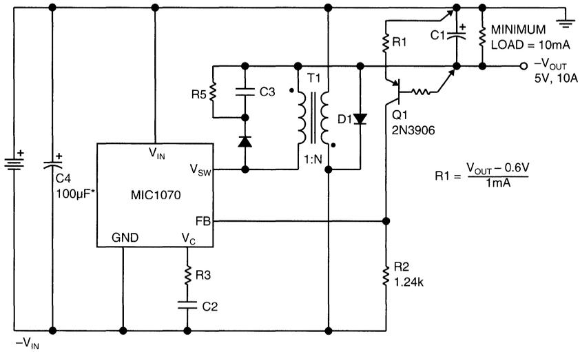
Figure 12. Negative Current Boosted Buck Converter
