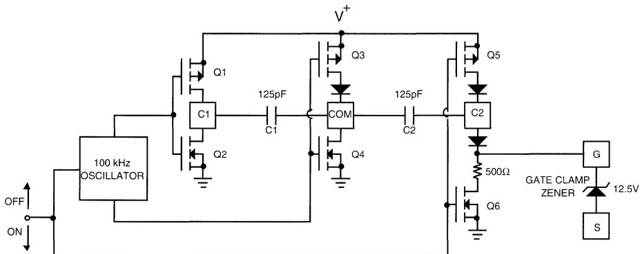
Figure 14. Gate Control Circuit Detail
