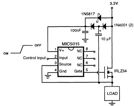
**Figure 1. Low Voltage Bootstrapped High Side Switch**
