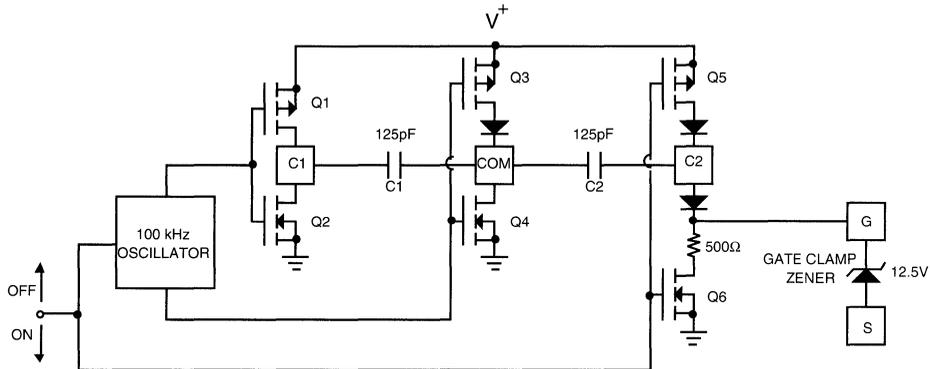
Figure 14. Gate Control Circuit Detail
