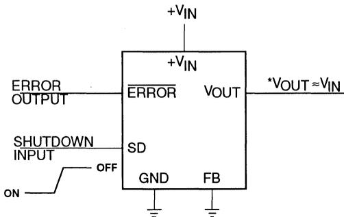
\*MINIMUM INPUT-OUTPUT VOLTAGE RANGES FROM 40mV TO 400mV, DEPENDING ON LOAD CURRENT.
