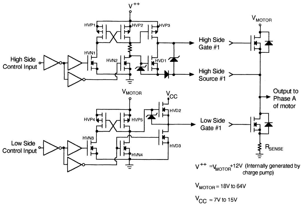
Figure 1. MPD8020-0011 Output Stage (one of three)
