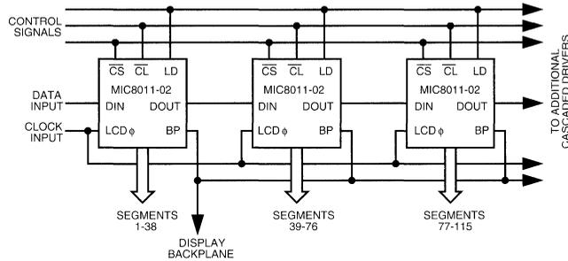
Figure 2. Cascading with External Clocking Source - Option -02
