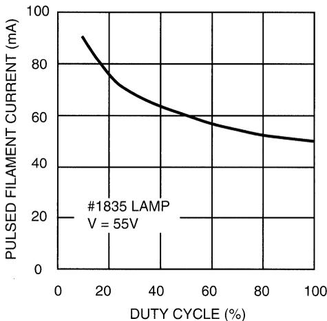
Figure 3. Pulsed Filament Current vs. Duty Cycle
