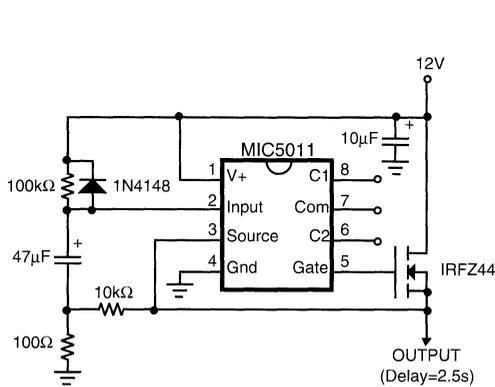
**Figure 9. 30 Ampere Time-Delay Relay**
