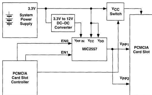
**Figure 4. MIC2557 Palmtop application. Note that the  $V_{PP1}$  and  $V_{PP2}$  pins are combined. Although this does not fully satisfy PCMCIA specifications, it simplifies the circuitry and is acceptable in certain applications.**
