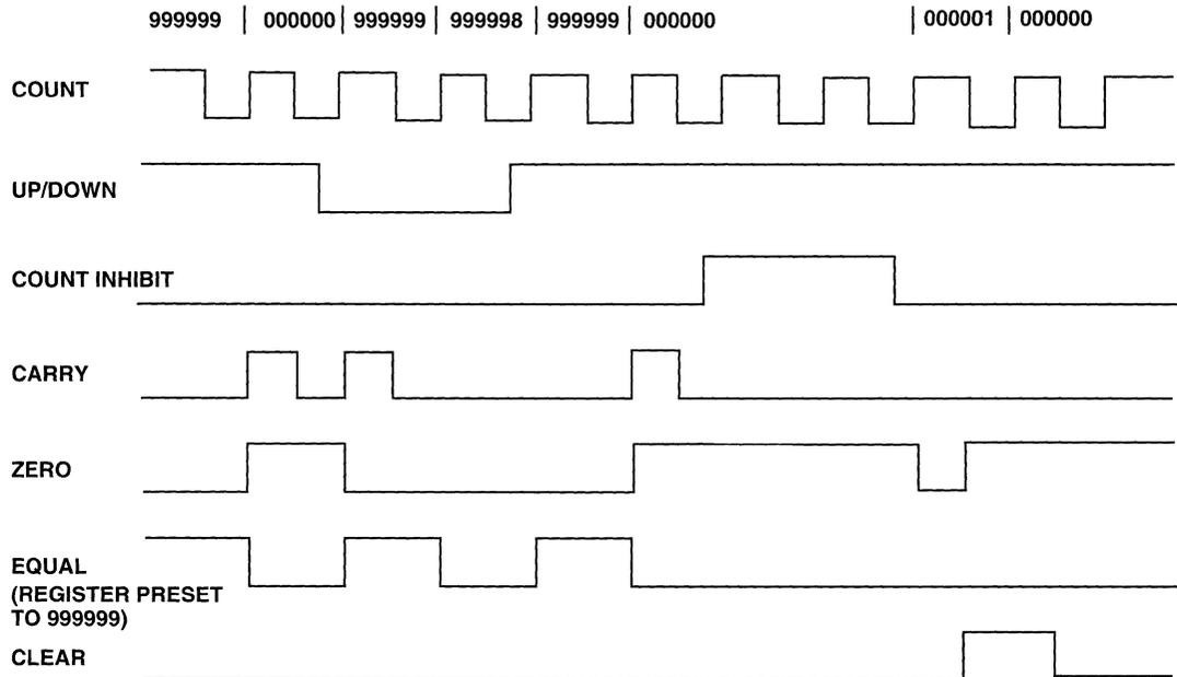
Figure 2: Up/Down Count Timing
