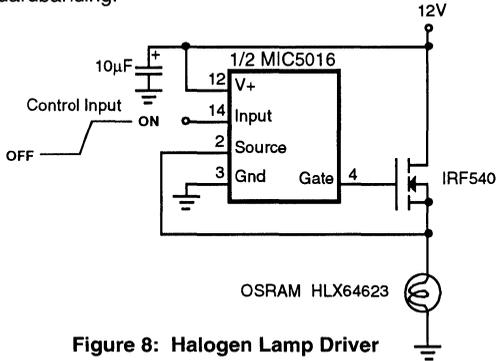
Figure 8: Halogen Lamp Driver
