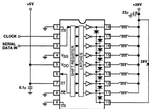
**MIC5841 Solenoid Driver with Output Enable**
