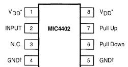
\* Pins 1 and 8 must be externally connected for proper operation.
