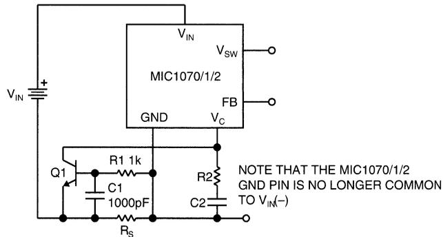
Figure 5. External Current Limit
