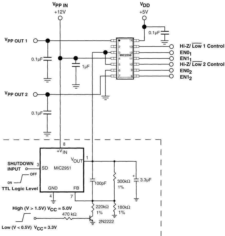
**V<sub>CC</sub> Switching and Control Block**
