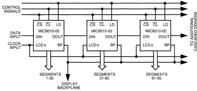
Figure 3. Cascading with External Clocking Source - 02 Configuration
