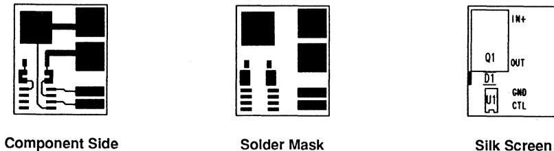
Figure 6. MIC5011 DB-1 Board Layout
