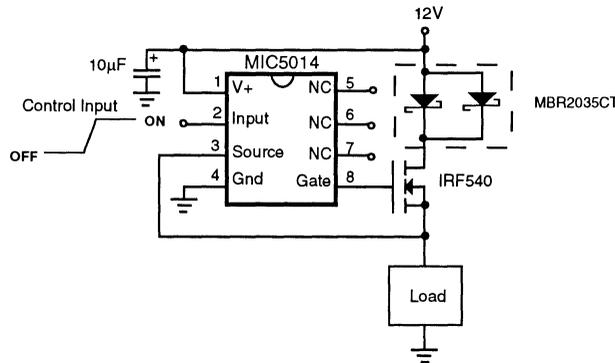
**Figure 12: High Side Driver With Load Protection**
