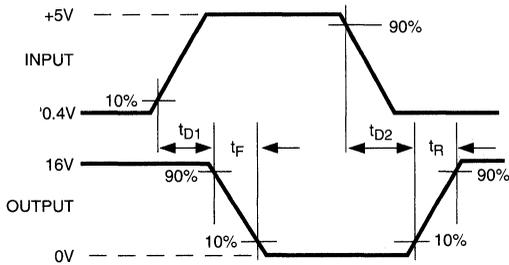
**Figure 1. Inverting Driver Switching Time**
