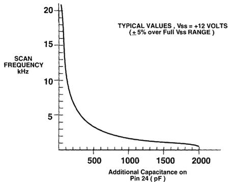
Figure 7: Scan Frequency vs. External
