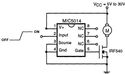
Figure 6: DC Motor Speed Control/Driver
