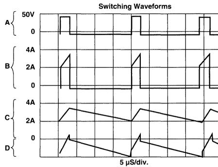
$$V_{OUT} = 5V \quad V_{IN} = 45V$$
