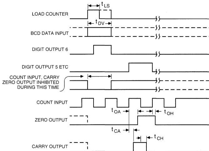
$t_{LS}$  2.0  $\mu$ S min NOTE: REF. TO POSITIVE TRANSITION OF DIGIT OUTPUT
