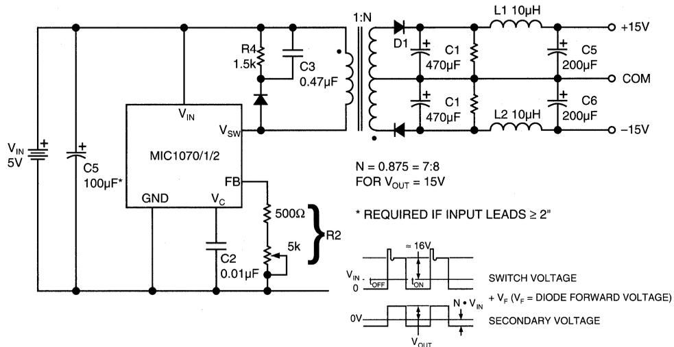
Figure 6. Totally Isolated Converter
