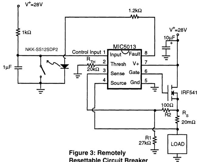
**Figure 3: Remotely Resettable Circuit Breaker**
