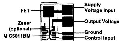
Figure 2. MIC5011 DB-1 Low Voltage Logic Controlled Power Switch
