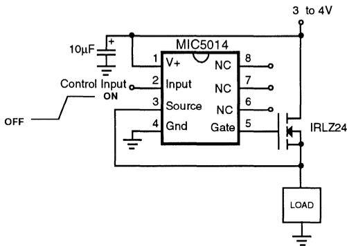
Figure 1. 3 Volt "Sleep-mode" Switch with a Logic Level FET
