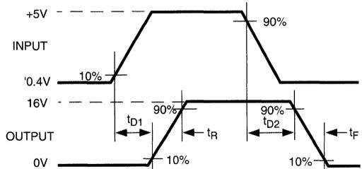
**Figure 2. Non-Inverting Driver Switching Time**
