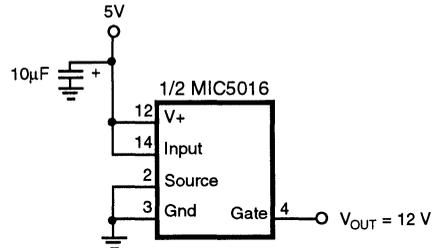
Figure 11. DC - DC Converter
