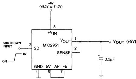
(Note: no external resistors are necessary)
