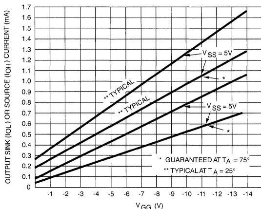
(I<sub>OL</sub> @ V<sub>0</sub> = V<sub>SS</sub> - 0.75V; T<sub>A</sub> = 25°C and T<sub>A</sub> = 75°C
