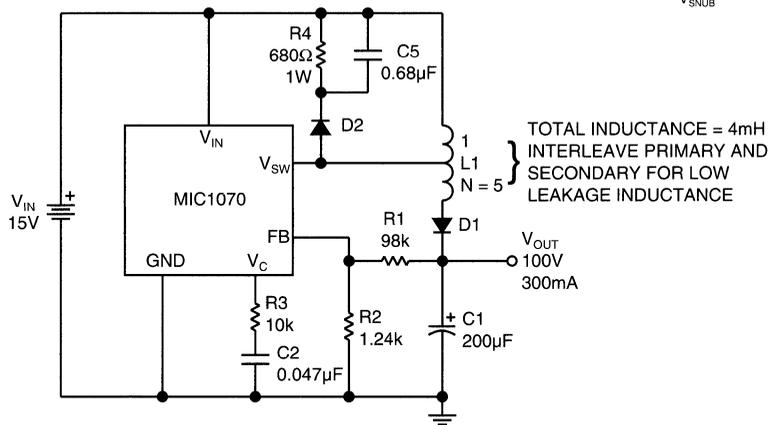
Figure 9. Voltage Boosted Boost Converter
