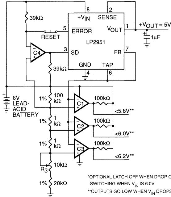
\*OPTIONAL LATCH OFF WHEN DROP OUT OCCURS. ADJUST R3 FOR C2 SWITCHING WHEN  $V_{IN}$  IS 6.0V
