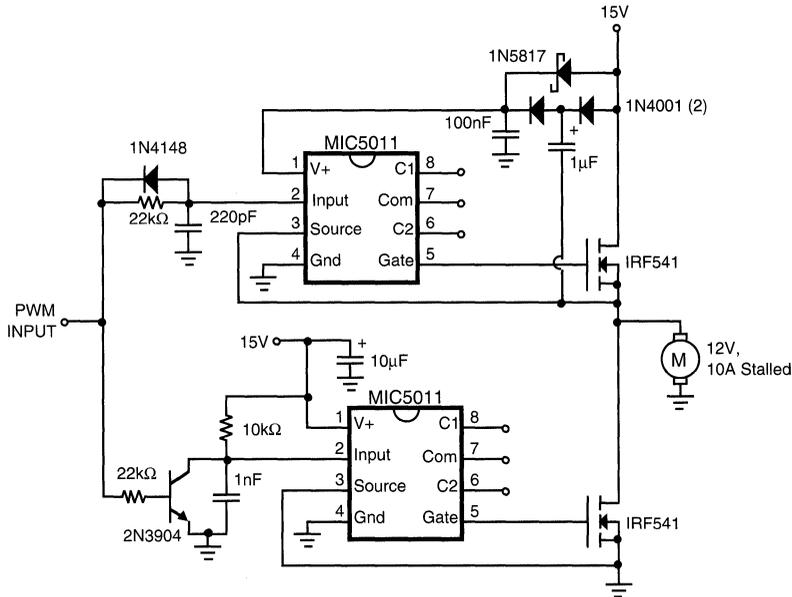
**Figure 8. Half-Bridge Motor Driver**
