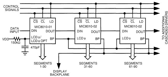
Figure 2. Cascading with Internal Clock Oscillator - 01 Configuration
