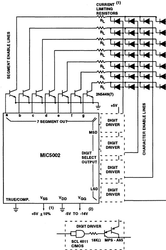
**FIG. 7: INTERFACING WITH COMMON CATHODE LED'S**
