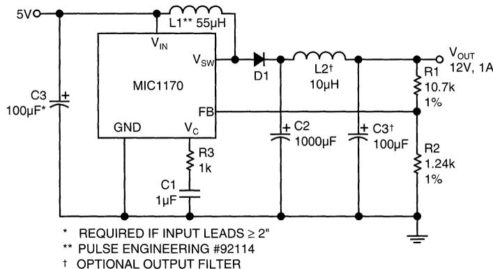
Figure 1 Boost Converter (5V to 12V)
