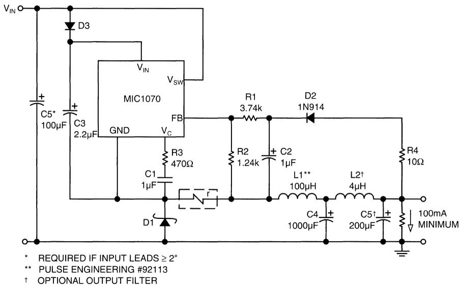
Figure 13. Positive Buck Converter
