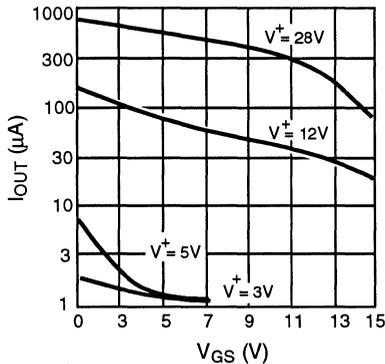
**Charge Pump Output Current, VS = Ground**
