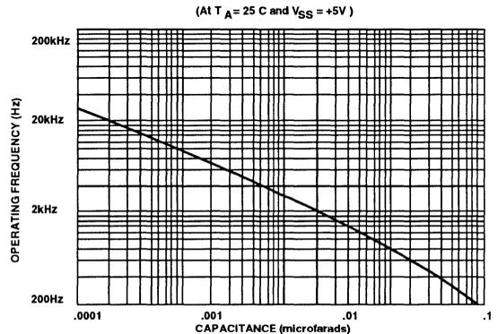
**FIG.12: CAPACITOR ON COUNT INPUT**
