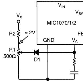
Figure 3. External Current Limit
