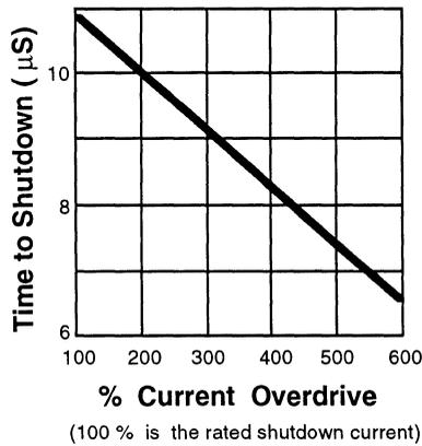
Figure 2: Shutdown Time vs. % Current Overdrive
