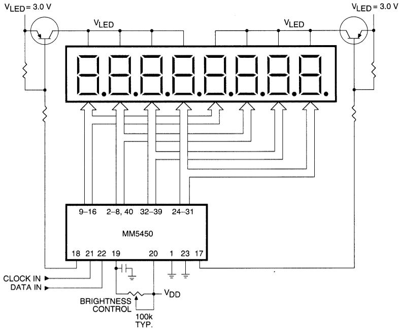
Figure 13. Duplexing 8 Digits with One MM5450.
