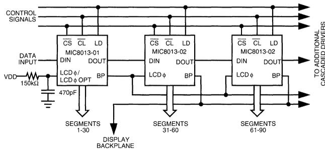
Figure 2. Cascading with Internal Clock Oscillator - 01 Option
