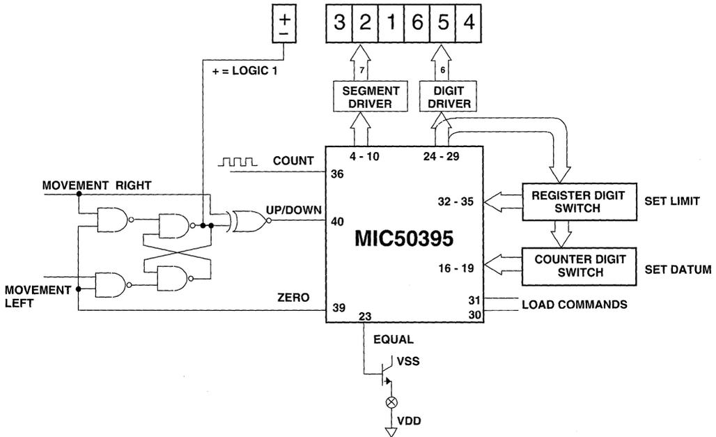
Figure 10: Positional Measurement
