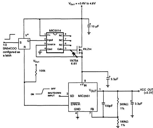
Figure 3: Low Battery Shutdown Switch
