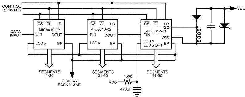
Figure 2. Cascading with MIC8010/12
