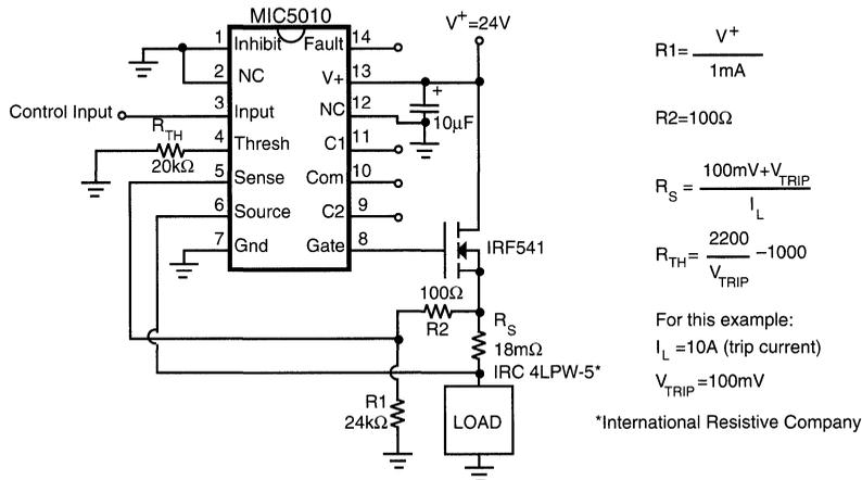
**Figure 3. High-Side Driver with Current Shunt**
