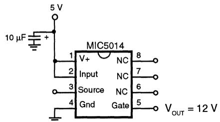
Figure 11. DC - DC Converter
