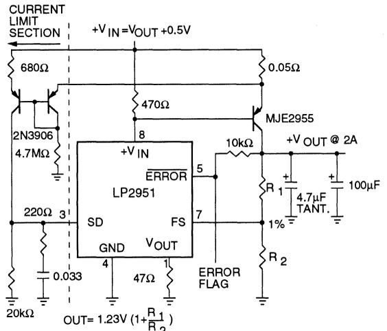
FOR 5  $V_{OUT}$ , USE INTERNAL RESISTORS. WIRE PIN 6 TO 7, AND WIRE PIN 2 TO  $+V_{OUT}$  BUS.
