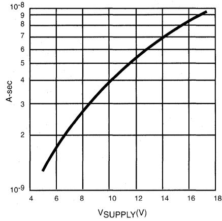
**Note 1:** The values on this graph represent the loss seen by both drivers in a package during one complete cycle. For a single driver divide the stated values by 2. For a single transition of a single driver, divide the stated value by 4.
