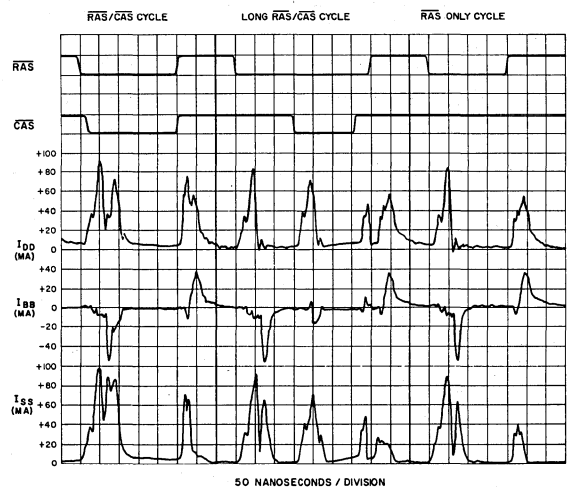
Fig. 5 Typical Current Waveforms
