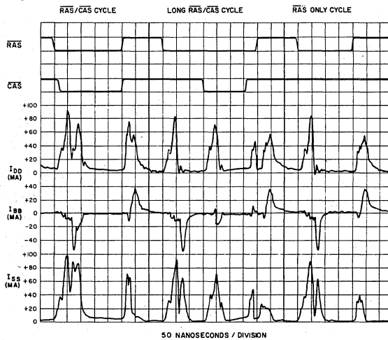
Fig. 5 Typical Current Waveforms for the MK 4116
