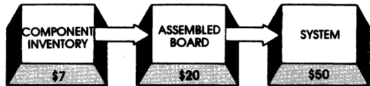
Typical costs for detection and replacement of IC failures at various manufacturing stages. Figure 1
