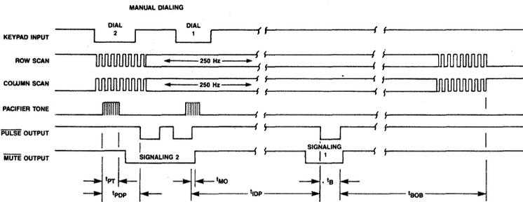
Figure 4A. MK5376 Timing Diagram — Pulse Mode Off-Hook Operation
