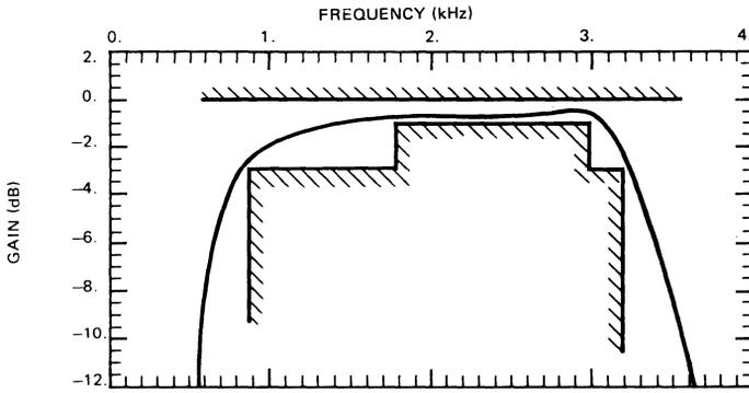
**Rx BAND-PASS AND REJECTION FILTER TYPICAL RESPONSE AND LIMITS CHART**
