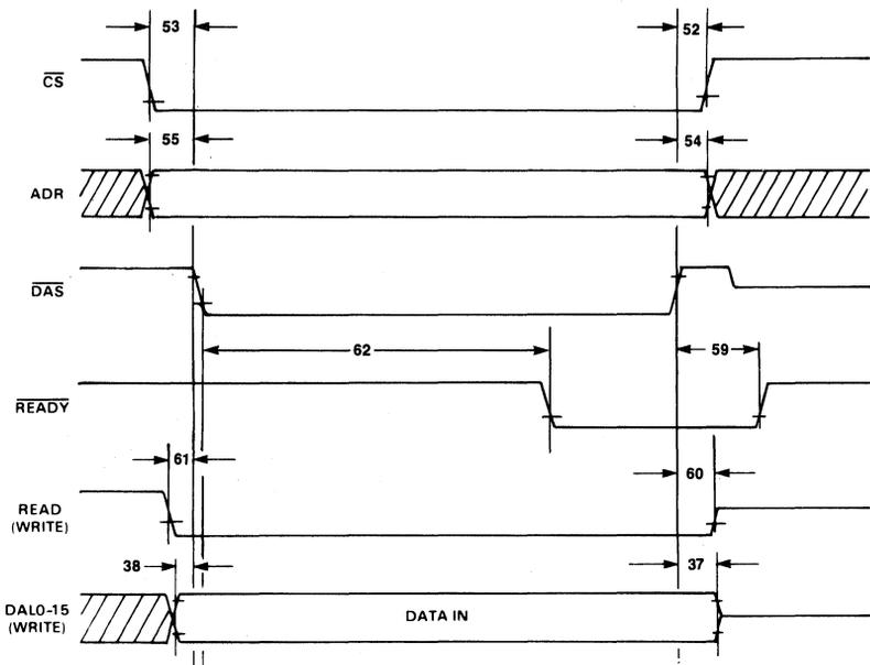
Figure 10. MK5025 Bus Slave Timing Diagram (Write)
