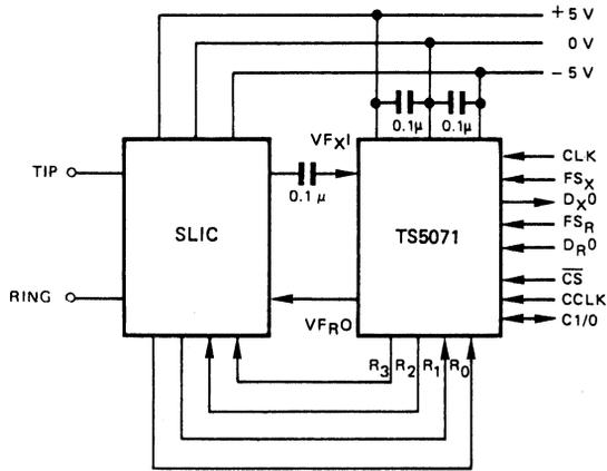
FIGURE 3 - TYPICAL APPLICATION WITH MONOLITHIC SLIC
