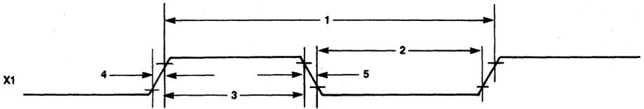
Figure 6. External X1 Timing Diagram
