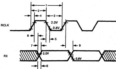
Figure 17a. RCLK and RX Timing
