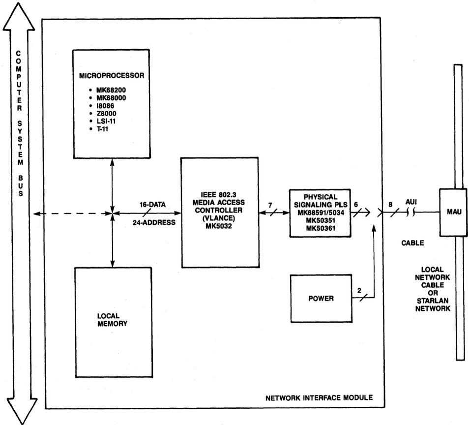
Figure 2. Ethernet Local Area Network System Block Diagram
