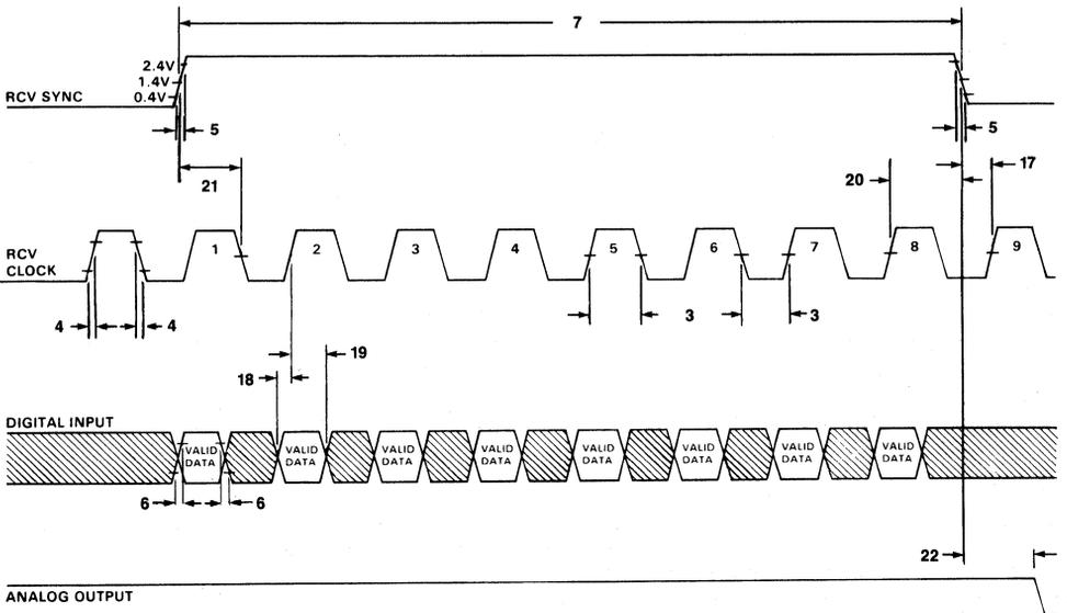
NOTE: All rise and fall times are measured from 0.4V and 2.4V. All delay times are measured from 1.4V.
