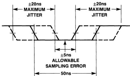
Figure 7. Maximum Jitter Impact On Sampling
