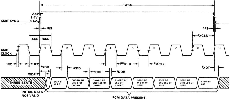
NOTE: All rise and fall times are measured from 0.4V and 2.4V.
