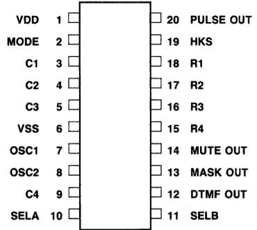
Figure 1. MK53721 Pinout
