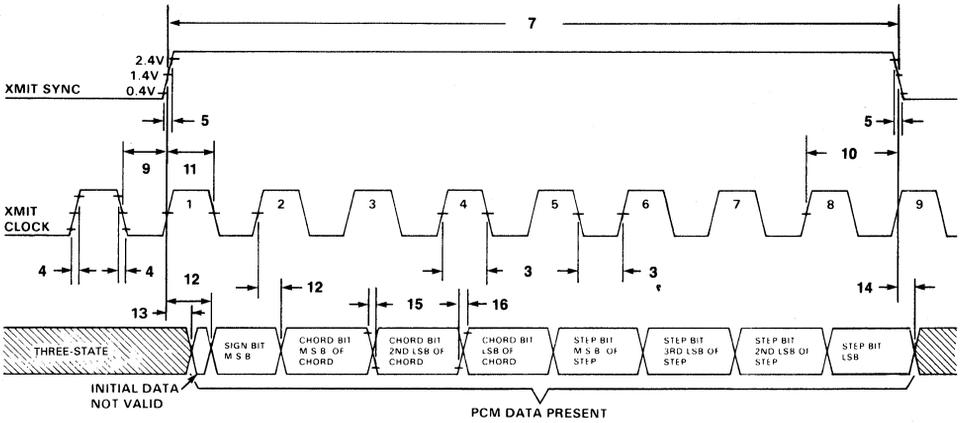
NOTE: All rise and fall times are measured from 0.4V and 2.4V. All delay times are measured from 1.4V.
