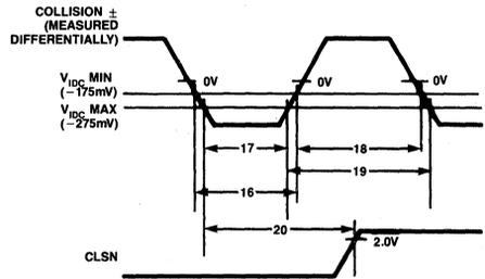
Figure 16b. Collision  $\pm$  Input Pulse Width Timing
