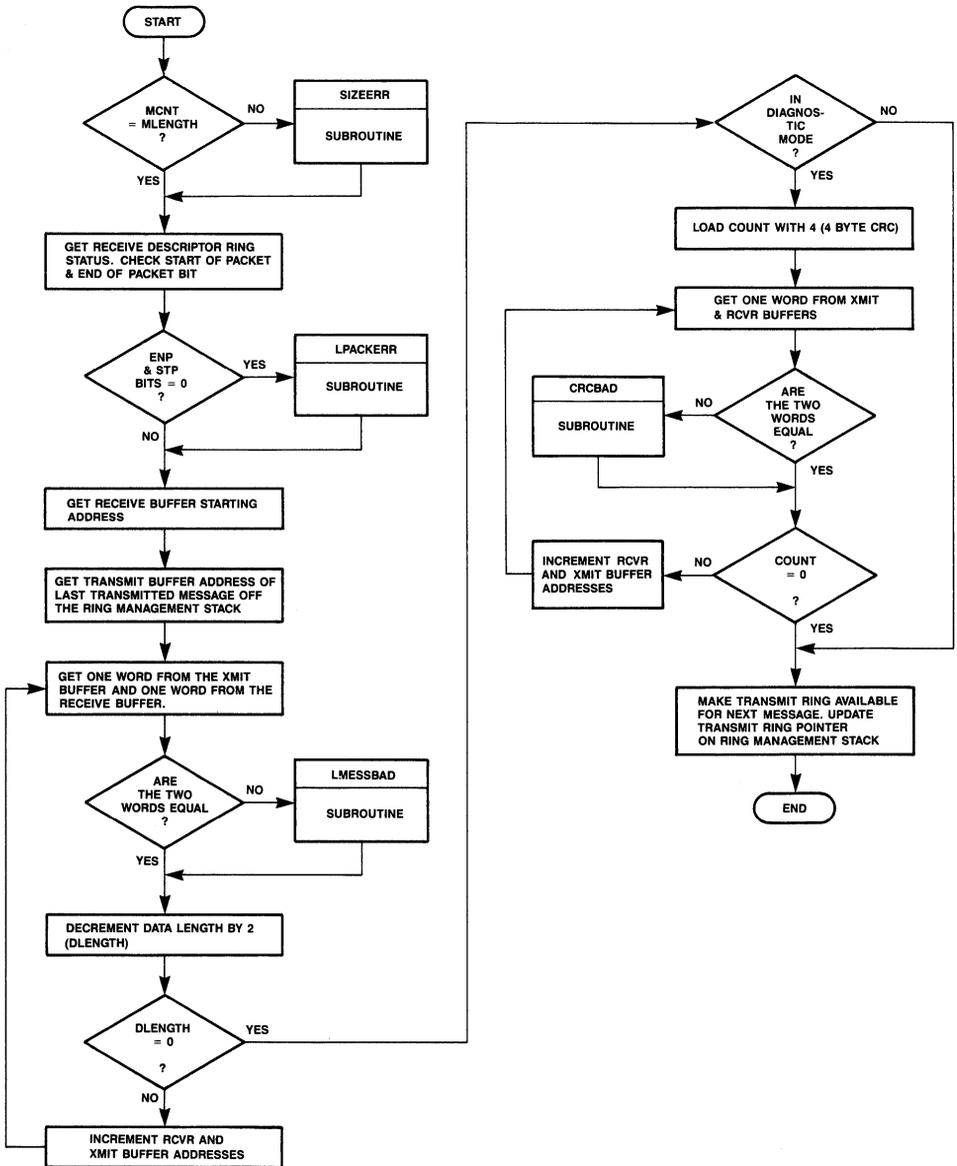
Figure 35. Loopback Service Routine [LANC.E. LEXCEPT. RVCR. LOOPBACK]
