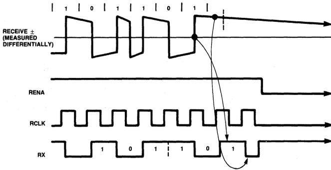
Figure 12. Receiver Timing — End of Packet (Last Bit = 1)
