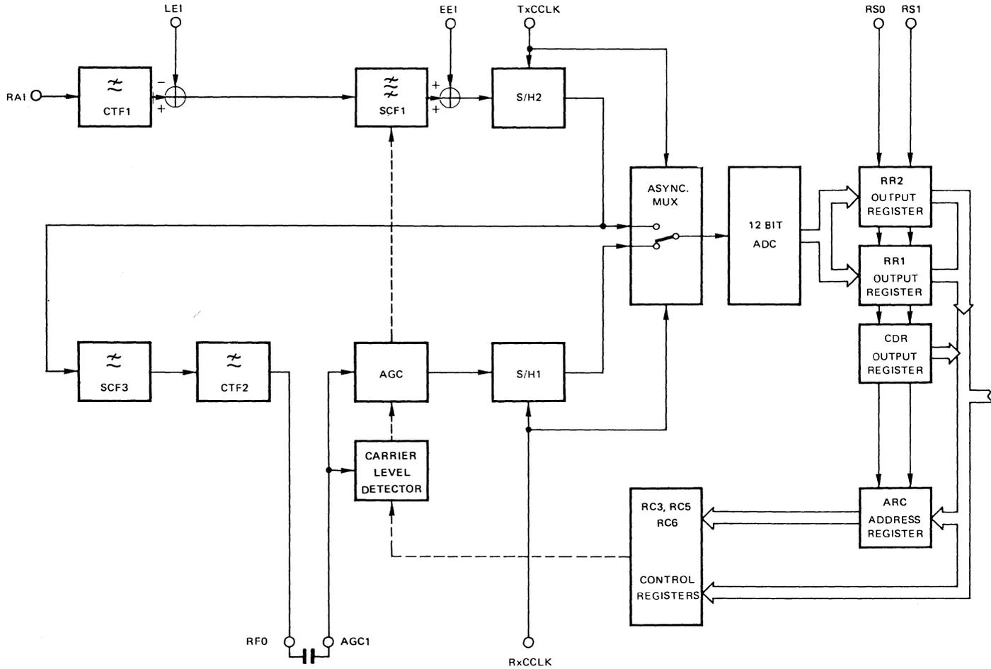
FIGURE 2 - TWO-WIRE ECHO CANCELLING ANALOG SIGNAL TREATMENT
