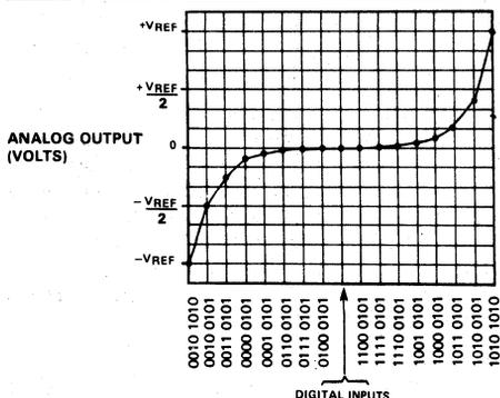
Figure 7. D/A Converter (A-Law Decoder) Transfer Characteristic
