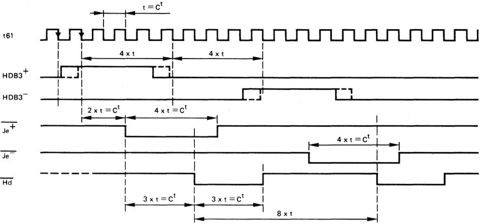
2 - EXTERNAL SIGNALS WITH  $HDB3^+$  AND  $HDB3^-$  SIGNAL PERIOD  $6 \times t$
