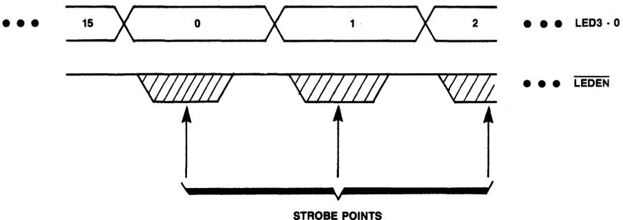
Figure 6. Scan Display Timing
