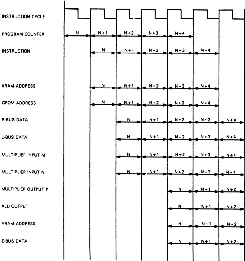
FIGURE 4.1.B. - PIPELINE THROUGHPUT
