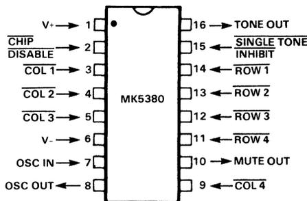
D-to-A conversion for synthesis of the tones is accomplished on chip by a sinusoidally tapped resistor tree.
