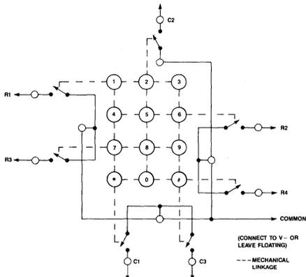
Figure 2B. Keyboard Schematics-Standard Telephone-Type Keypad
