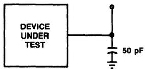
Figure 18. Test Load For RX, RENA, and TCLK
