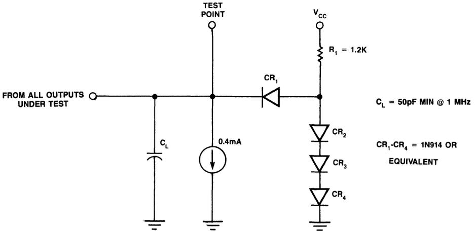
Figure 9. Output Load Diagram
