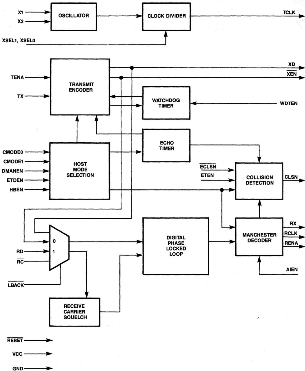
Figure 2. Manchester Encoder/Decoder Block Diagram
