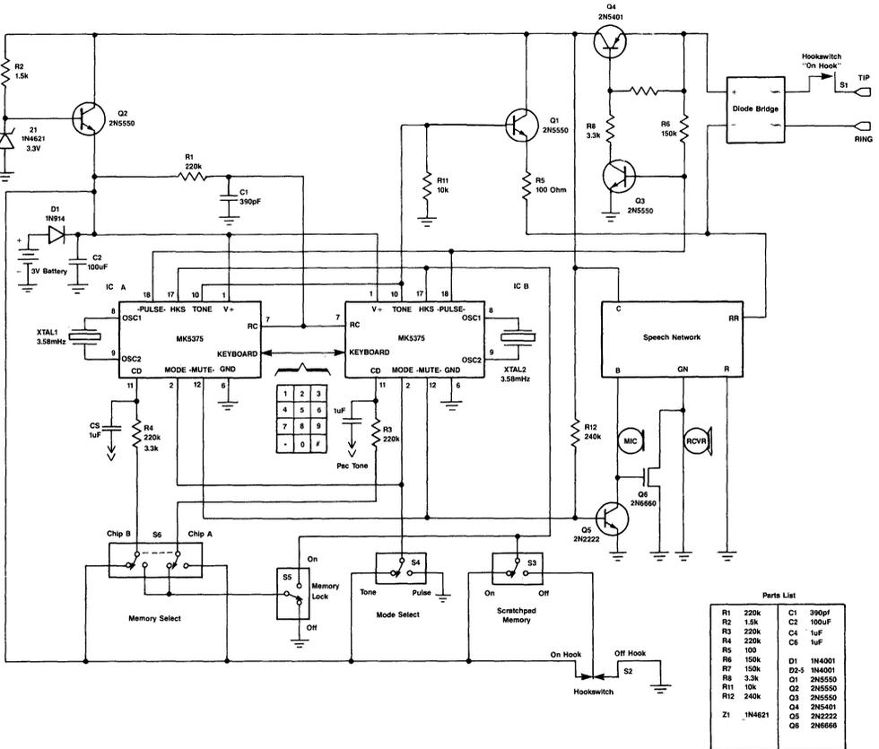
Figure 8. MK5375 Application Circuit Schematic
