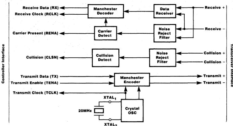
Figure 3. MK68591/2 Block Diagram
