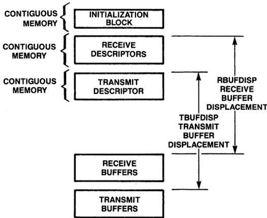
Figure 23. Buffer Displacement Diagram
