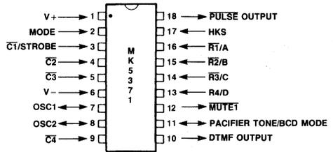
Figure 1. Pin Connection
