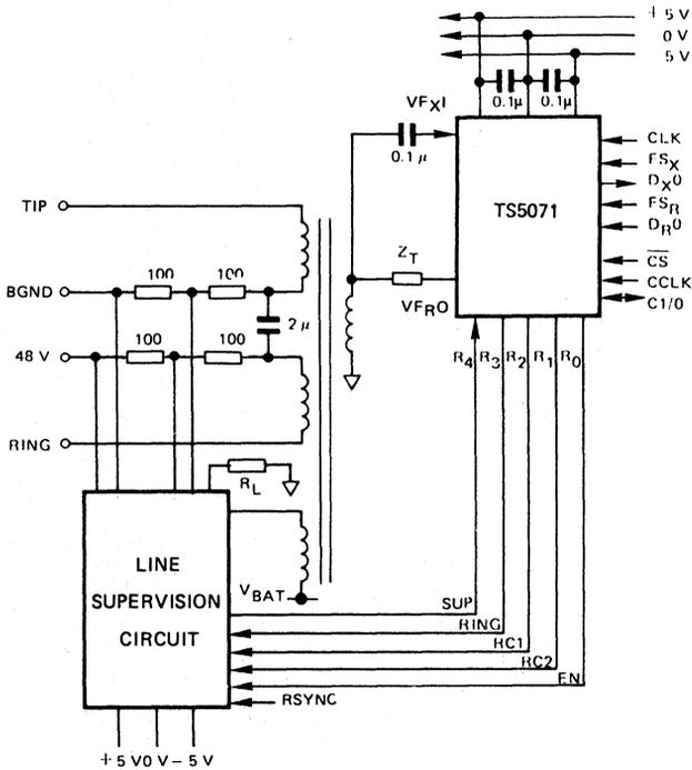
FIGURE 2 - TYPICAL APPLICATION WITH TRANSFORMER SLIC
