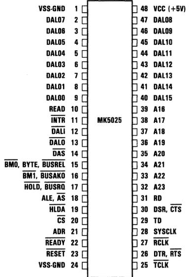
Figure 1. Pin Connection
