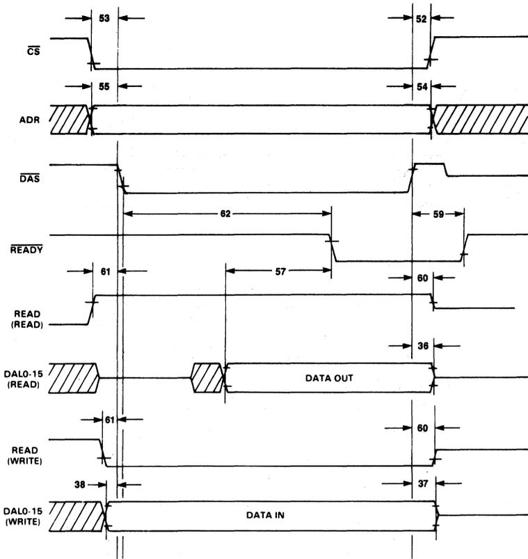
Figure 8. MK5025 Bus Slave Timing Diagram
