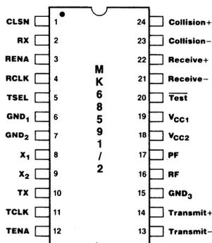
Figure 1. Pin Assignments
