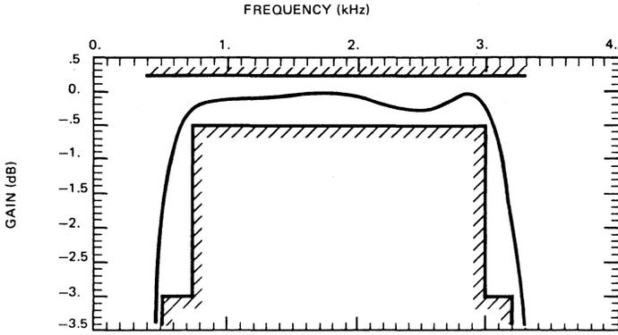
**Rx BAND-PASS FILTER TYPICAL RESPONSE AND LIMITS CHART**
