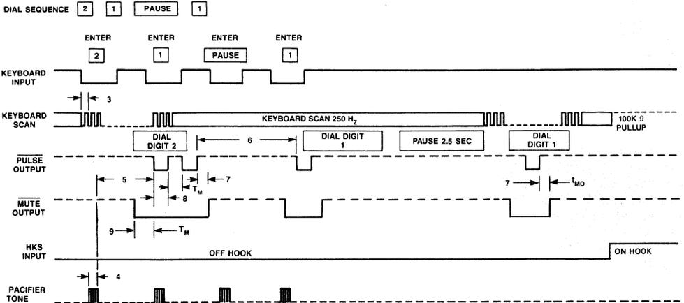
**Figure 8. Pulse Mode Timing**
