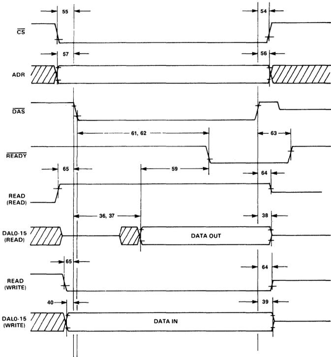
Figure 9. LANCE Bus Slave Timing Diagram
