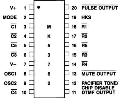
Figure 1. Pin Connection
