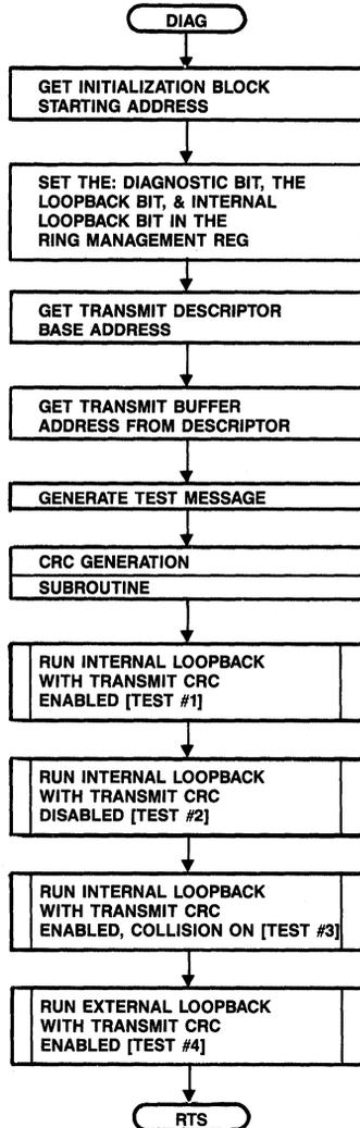
Figure 26. Diagnostics' Subroutine [LANCE. INITIAL. DIAG]
