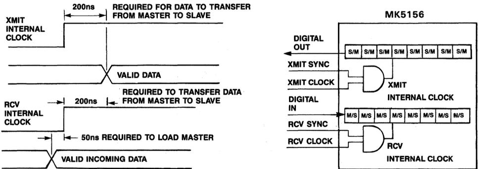
Figure 5. Data Input/Output Timing
