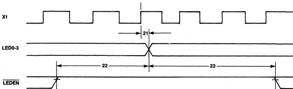
Figure 13. Status Display Timing Diagram
