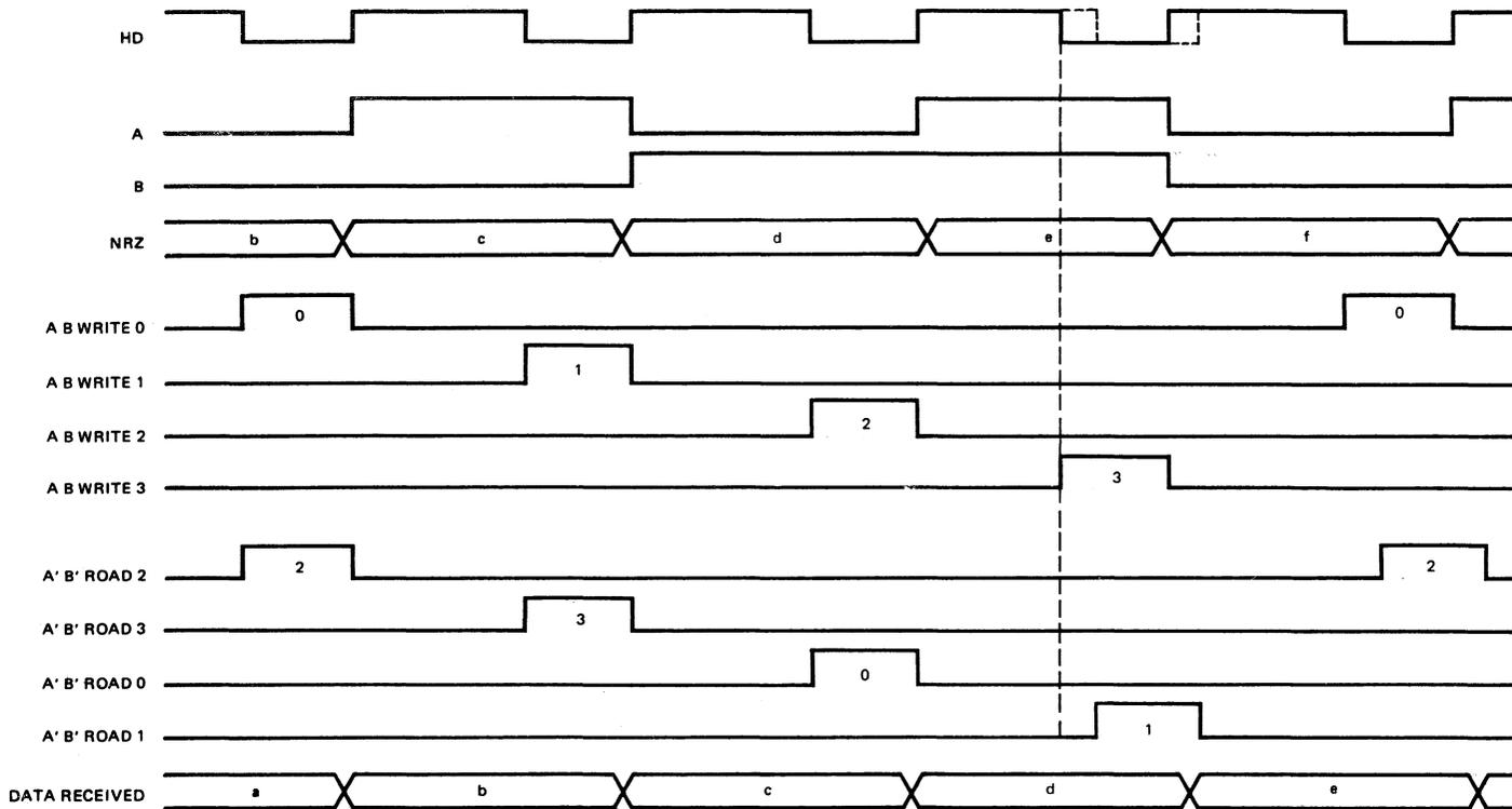
FIGURE 8 — APPLICATION TIMING DIAGRAM — 72321 WITH SLAVED OSCILLATOR
