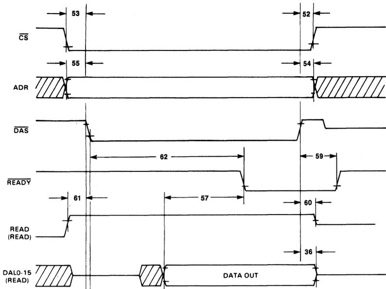
Figure 9. MK5025 Bus Slave Timing Diagram (Read)
