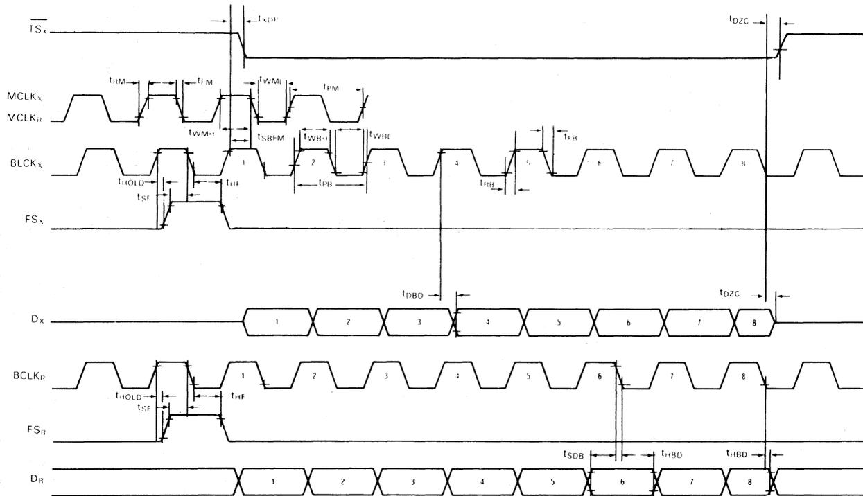
FIGURE 3 - SHORT FRAME SYNC TIMING
