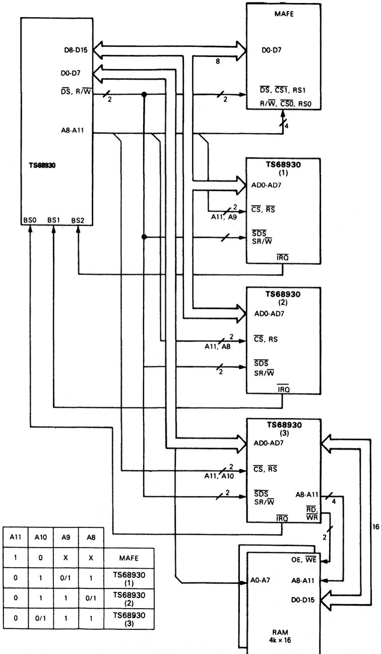
FIGURE 6.7.C. - CONFIGURATION EXAMPLE: 4 TS68930 + MAFE + RAM
