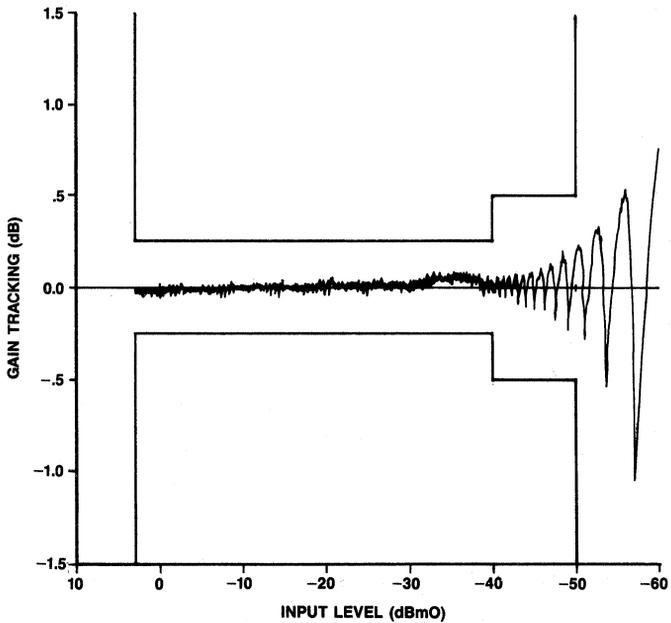
Figure 15. MK5156 Single-Ended Gain Tracking
