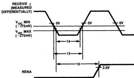
Figure 16a. Receive  $\pm$  Input Pulse Width Timing
