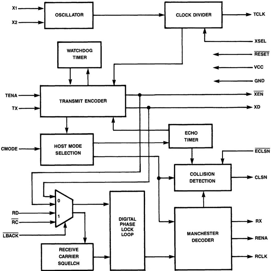
Figure 2. StarLAN Encoder Decoder. MK5035
