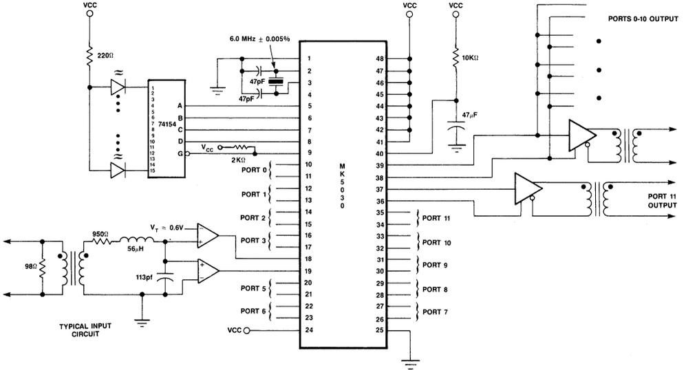
Figure 9. MK5030 External Component Diagram
