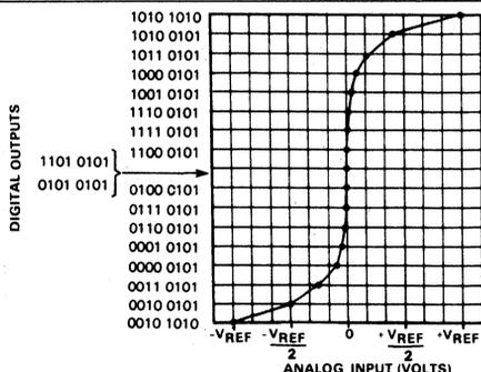
Figure 6. A/D Converter (A-Law Encoder) Transfer Characteristic
