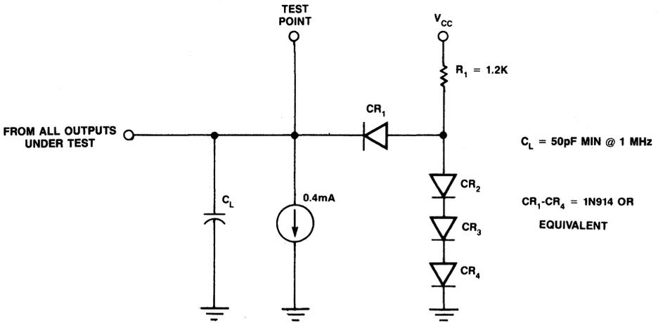
Figure 9. Output Load Diagram
