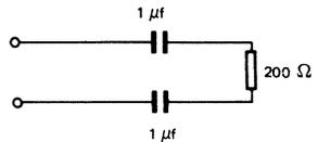
**Note 3: Receiving mode - Test diagram**
