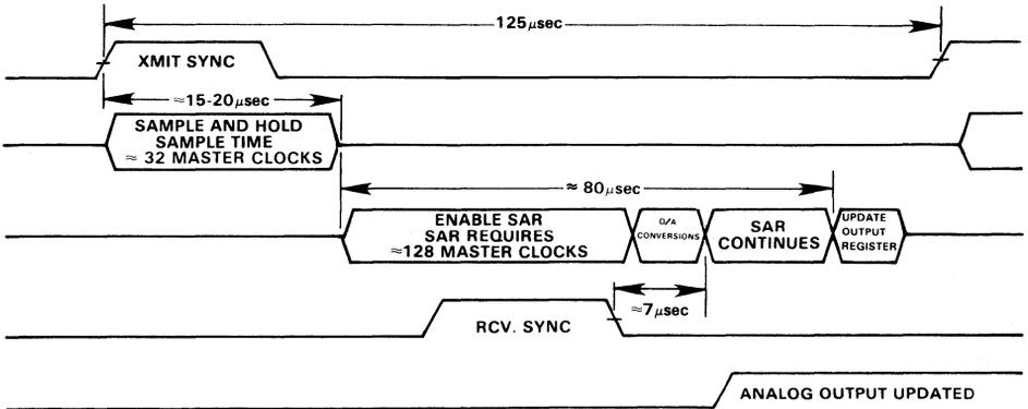
Figure 4. A/D, D/A Conversion Timing
