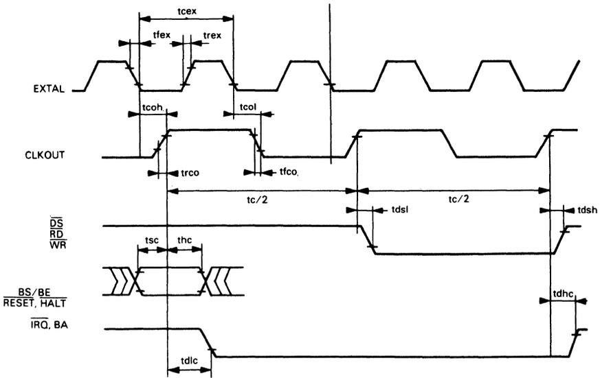
FIGURE 9.1. - CLOCK AND CONTROL PINS TIMING
