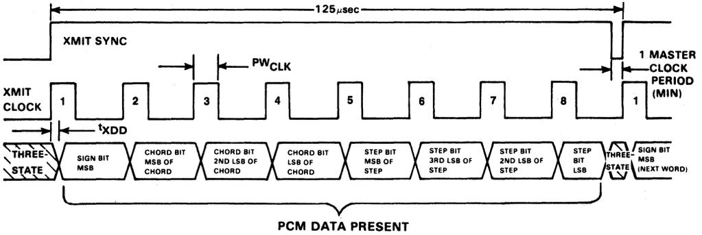
NOTE: All rise and fall times are measured from 0.4V and 2.4V. All delay times are measured from 1.4V.
