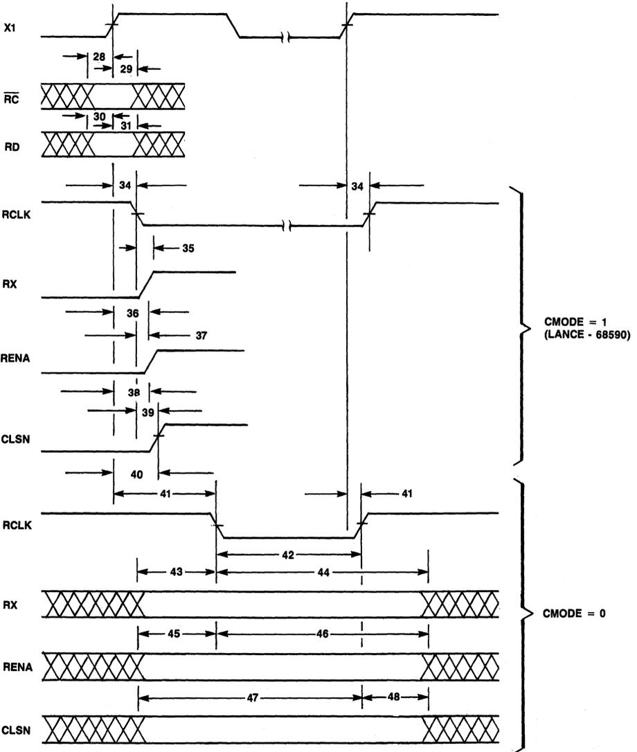
Figure 8. Receiver Timing Diagram
