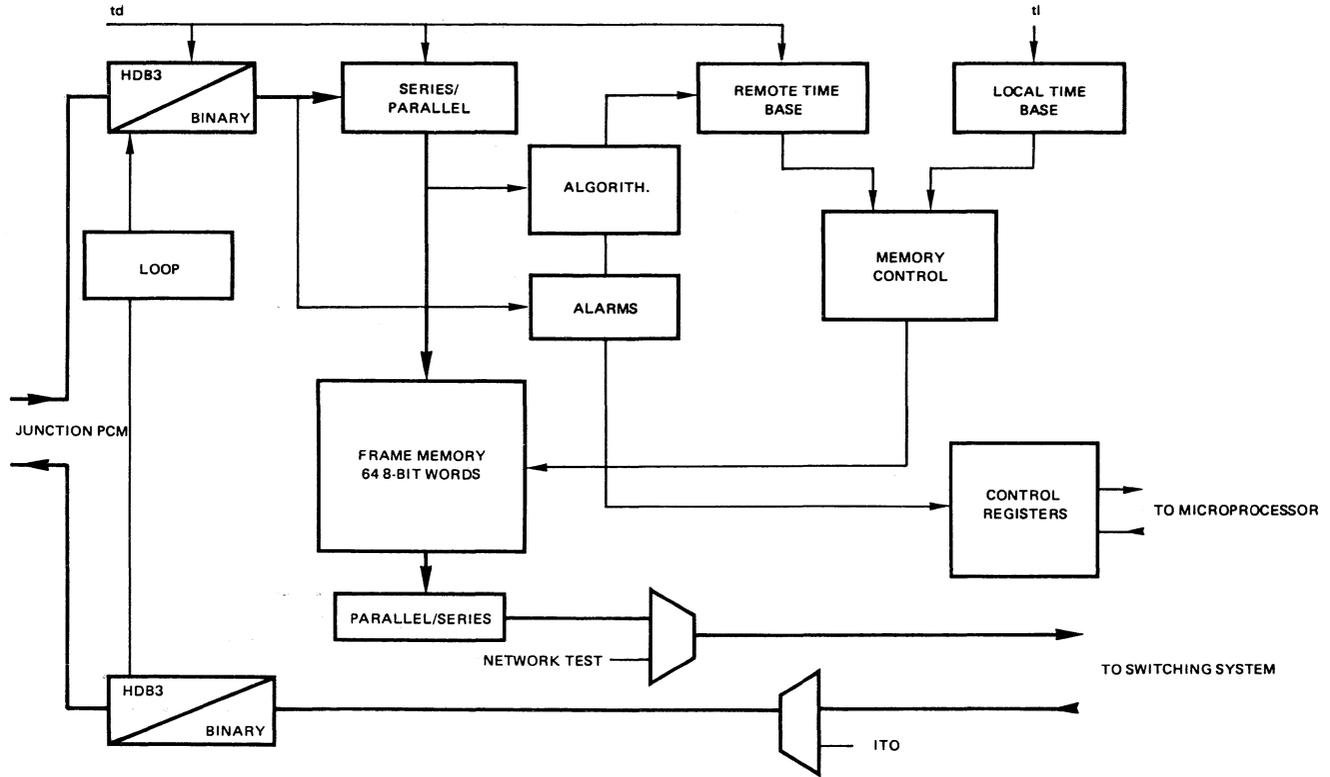
FIGURE 9 - SWITCHING TERMINAL MODULE
