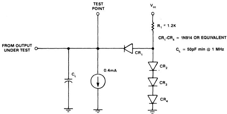
Figure 5. Output Load Diagram
