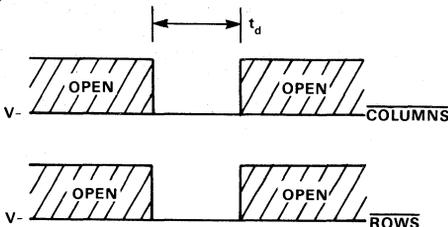
NOTE:  $t_d$  is minimum tone duration plus oscillator start up time ( $t_{RISE}$ )
