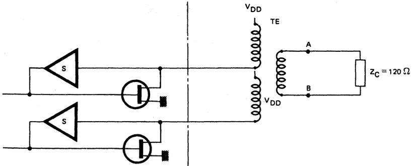
FIGURE 4 -- MEH CIRCUIT BUILT-IN TRANSMIT AMPLIFIER
