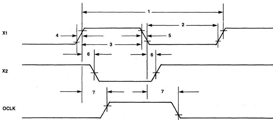
Figure 10. Oscillator Timing Diagram
