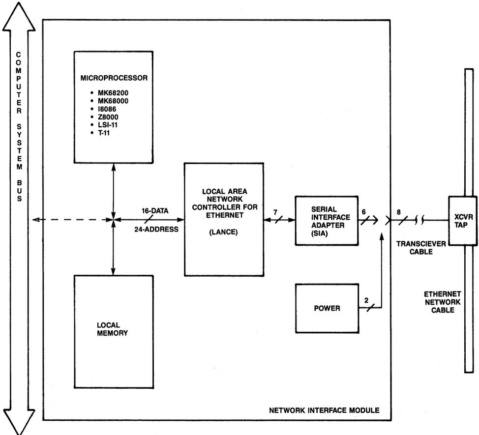
Figure 3. Ethernet Local Area Network System Block Diagram
