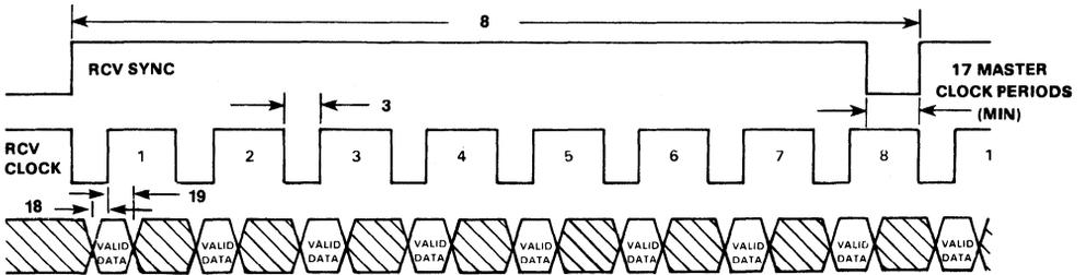
NOTE: All rise and fall times are measured from 0.4V and 2.4V. All delay times are measured from 1.4V.
