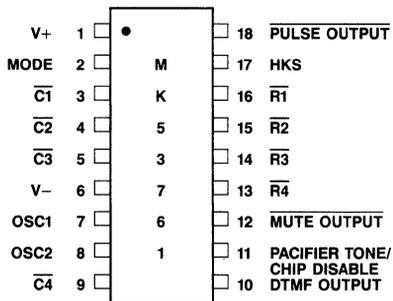
Figure 1. Pin Connection
