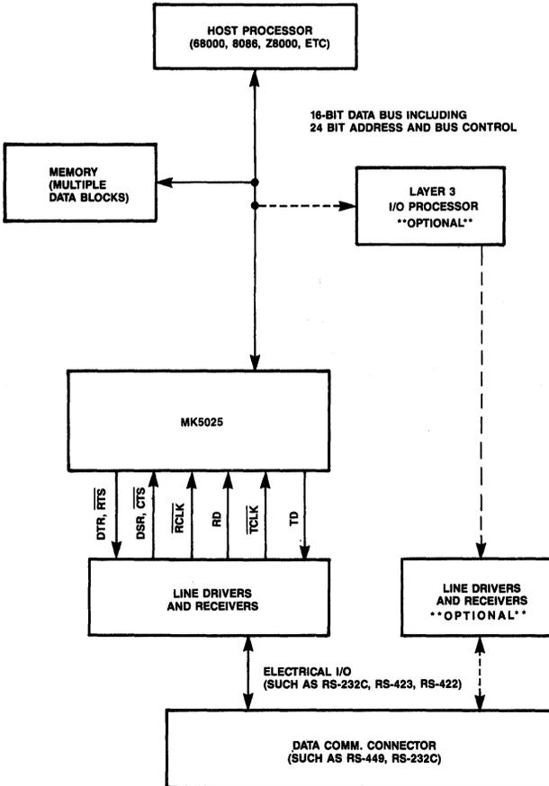
Figure 2. Possible System Configuration for the MK5025
