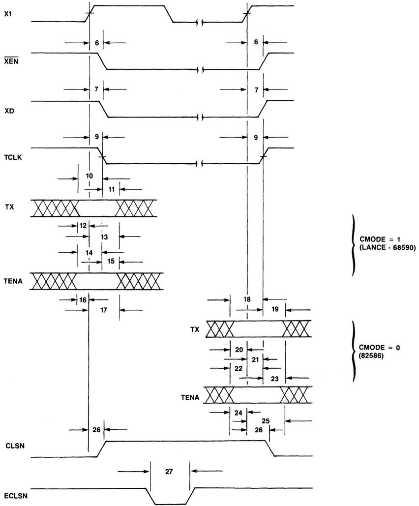
Figure 7. Transmit Timing Diagram
