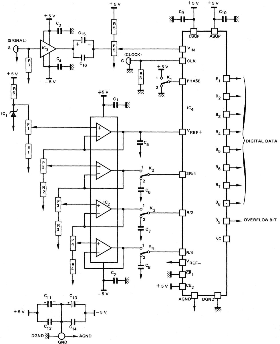
**8 BIT RESOLUTION CONFIGURATION 20 MHZ SAMPLING RATE**
