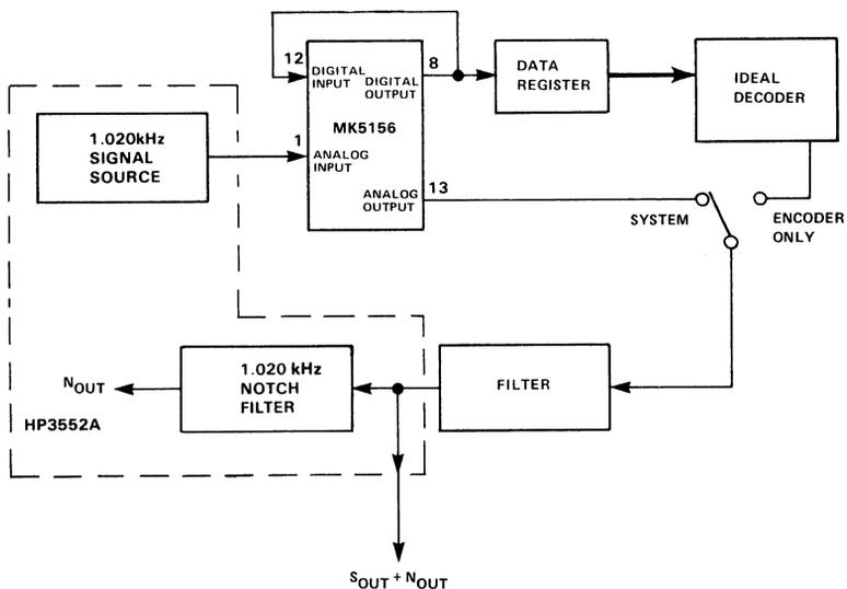
**NOTE:** The ideal decoder consists of a digital decompander and a 13-bit precision DAC.
