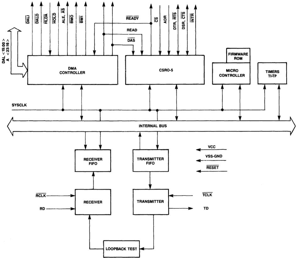
Figure 2. MK5025 Simplified Block Diagram
