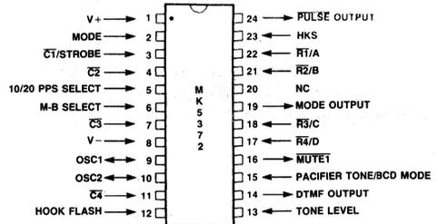
Figure 2. Pin Connection
