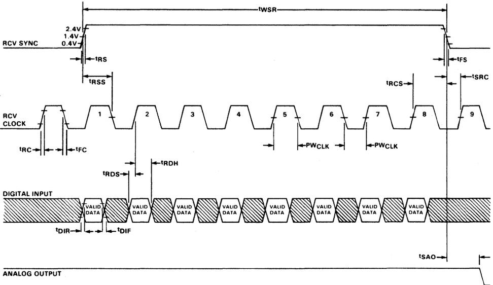
NOTE: All rise & fall times are measured from 0.4V and 2.4V. All delay times are measured from 1.4V.
