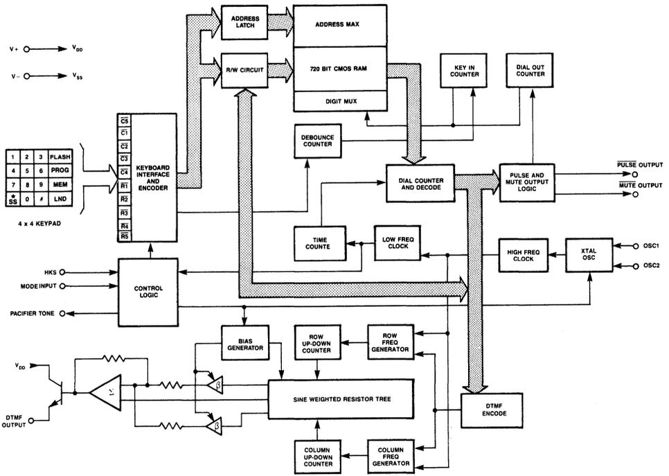
Figure 3. MK53761 Functional Block Diagram
