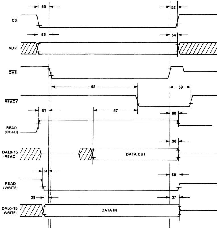
Figure 8. MK5025 Bus Slave Timing Diagram
