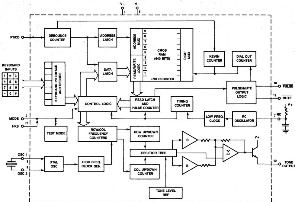
Figure 2. MK5375 Functional Block Diagram
