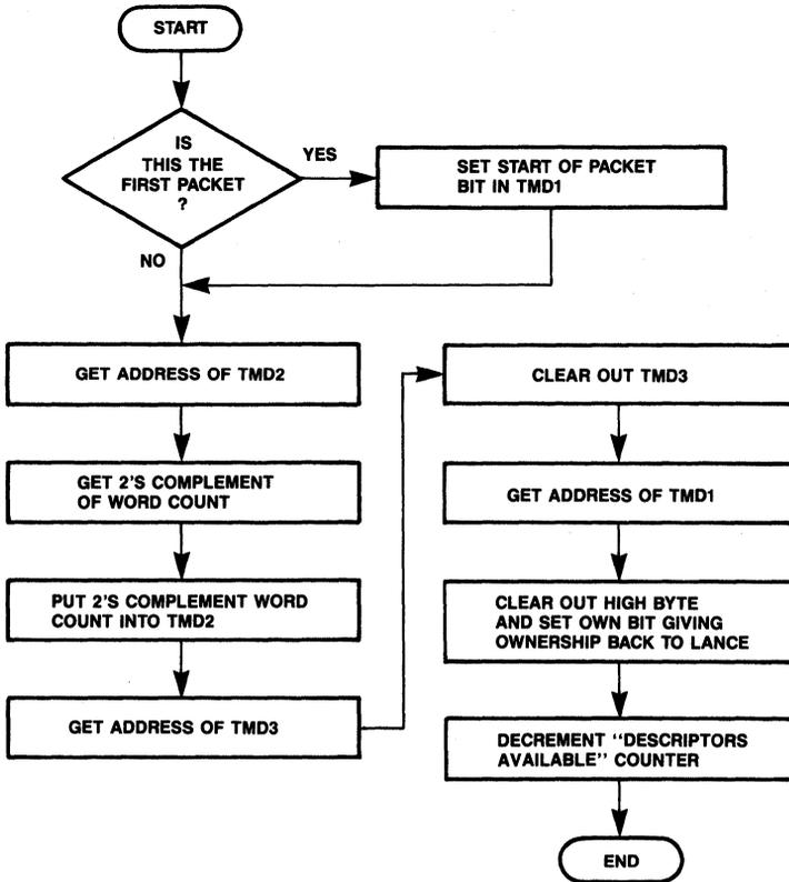
Figure 39. Transmit Ring Update Submodule [MESSAGE. XMIT RING UPDATE]
