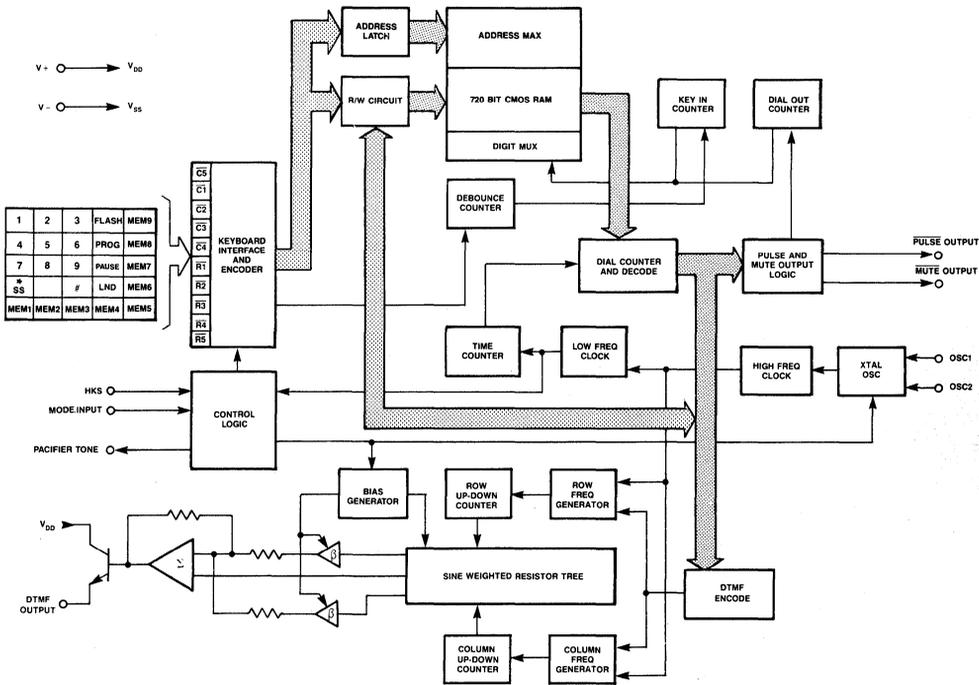
Figure 3. MK53762 Functional Block Diagram
