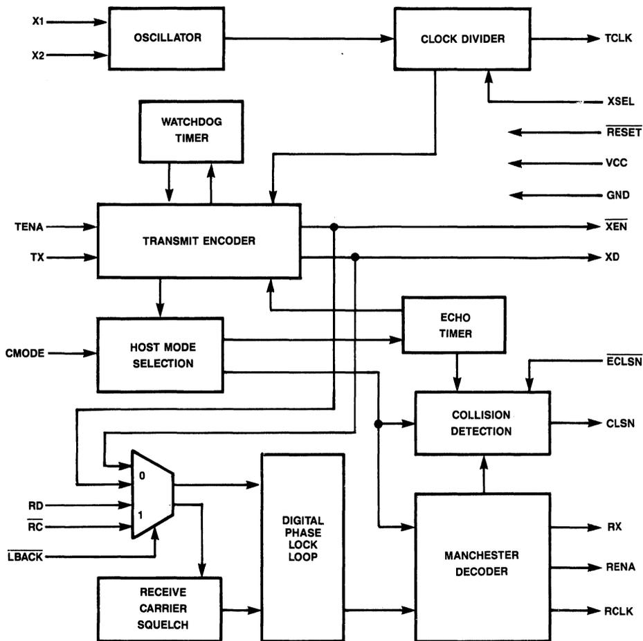
Figure 2. StarLAN Encoder Decoder. MK50351
