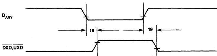
Figure 12. Retimer Disabled (MODE3 = 0) Timing Diagram
