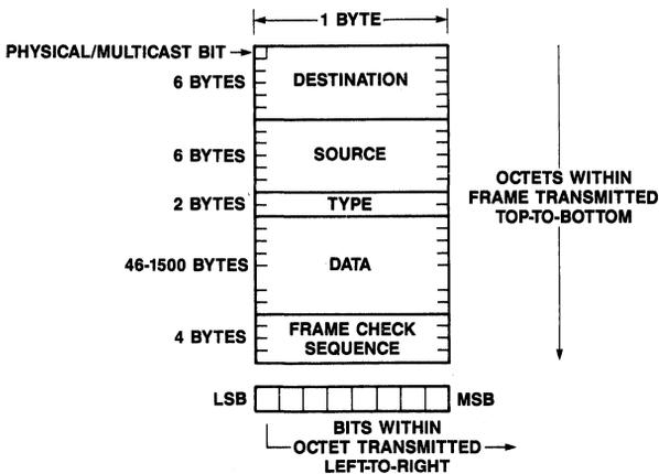
Figure 3. Ethernet and Packet Bit Transmission Sequence
