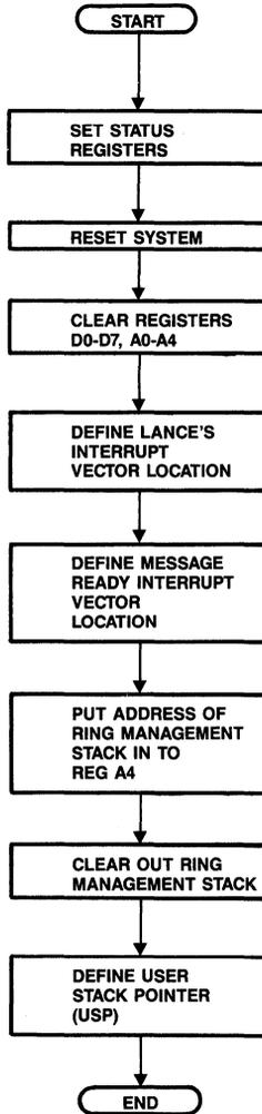
Figure 21. Clear Submodule [LANCE. INITIAL. CLEAR]
