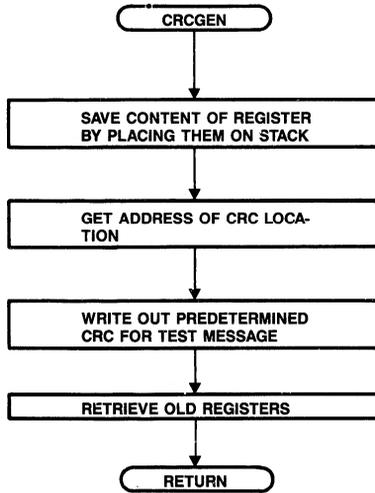
Figure 28. Cycle Redundancy Check Generation Subroutine [CRCGEN]
