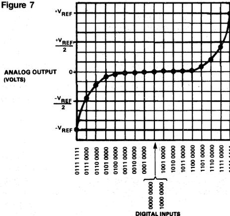
CLOCK to clock the serial data into its input register. RCV SYNC goes low to indicate the end of serial input data. The 8 bits of the input data have the same functions described for the DIGITAL OUTPUT. The transfer characteristic of the D/A converter ( $\mu$ -Law Decoder) is shown in Figure 7.
