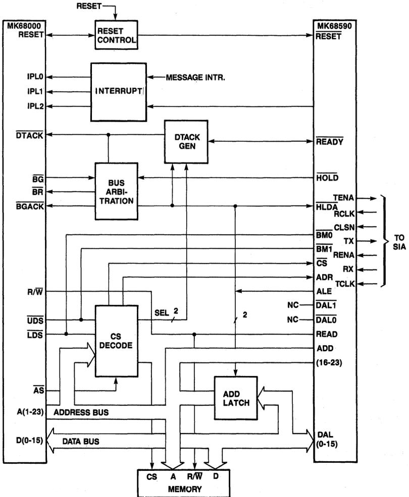
Figure 5. 68000/68590 Block Diagram
