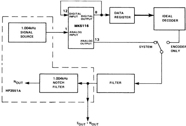
NOTE: The ideal decoder consists of a digital decomander and a 13-bit precision DAC.
