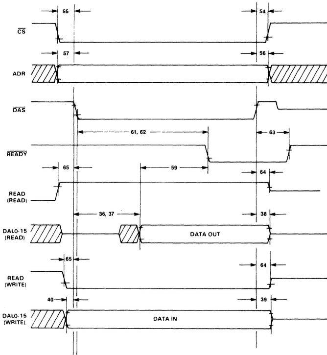
Figure 8. MK5032 Bus Slave Timing Diagram
