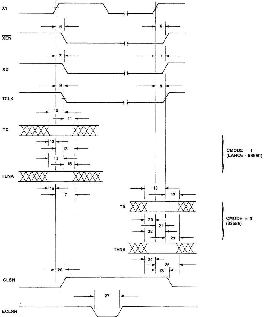
Figure 7. Transmit Timing Diagram
