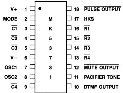
Figure 1. Pin Connection
