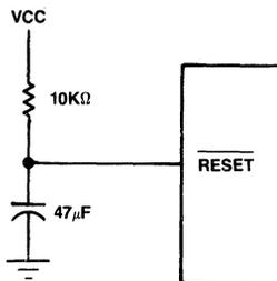
Figure 5. Typical RC Connection For Power-On Reset
