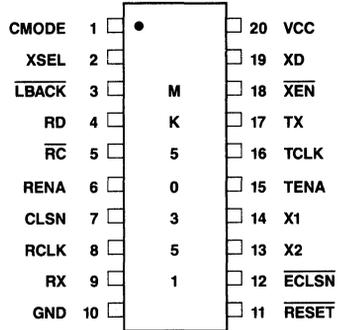
Figure 1. MK50351 Pin Assignment
