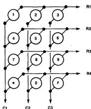
Figure 2A. Keyboard Schematics-Calculator-Type Keypad
