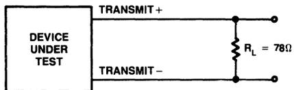
Figure 19. Transmit  $\pm$  Output Test Circuit
