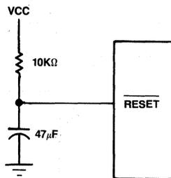
Figure 8. Typical RC Connection For Power-On Reset
