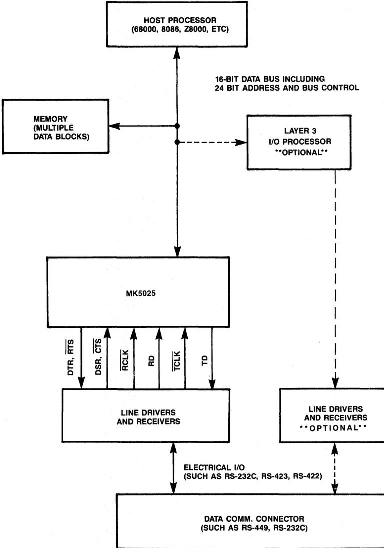
Figure 1. Possible System Configuration for the MK5025
