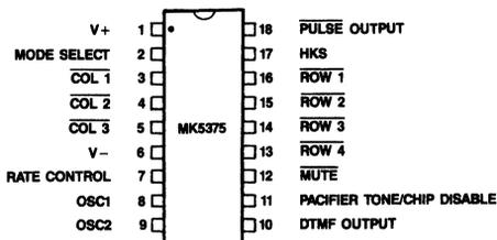
Figure 1. Pin Connections
