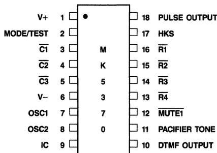
Figure 1. Pin Connection
