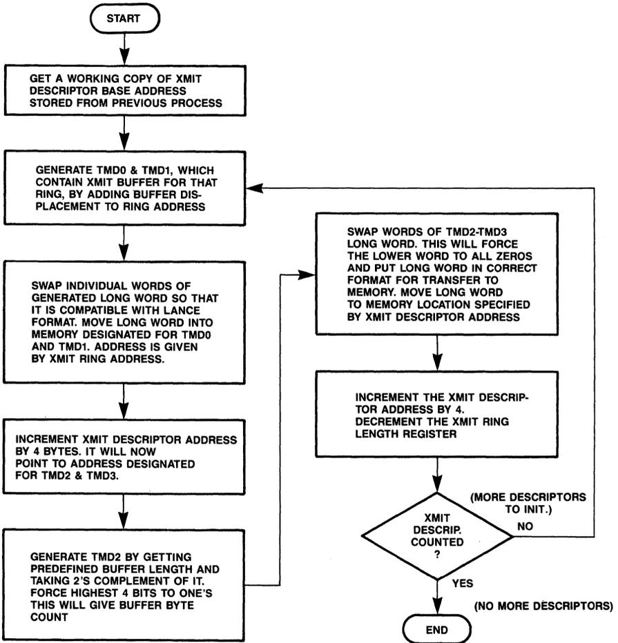
Figure 25. Transmit Ring Initialization Submodule [LANCE. INITIAL. TRINGINIT]
