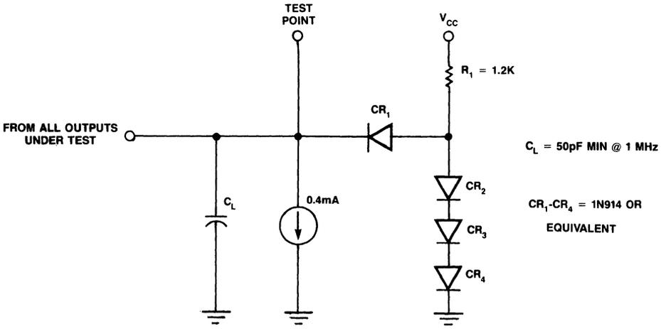
Figure 9. Output Load Diagram
