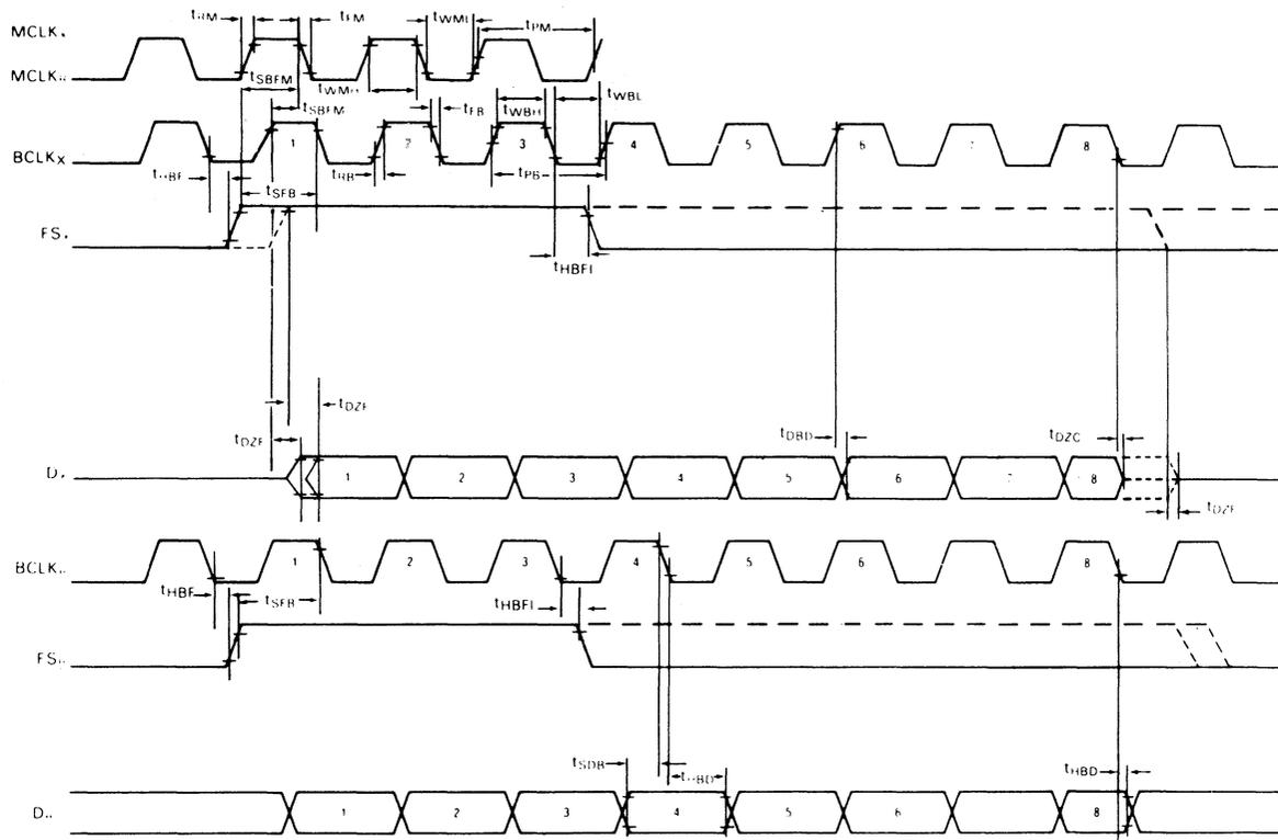
FIGURE 4 - LONG FRAME SYNC TIMING
