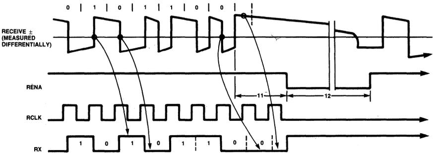
Figure 11. Receiver Timing — End of Packet (Last Bit = 0)
