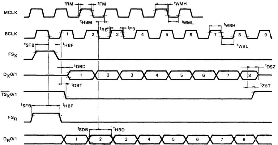
FIGURE 5 - DELAYED DATA TIMING
