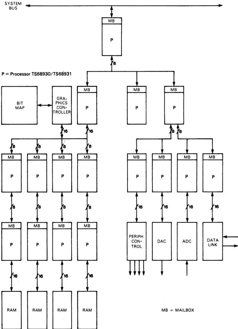
FIGURE 6.F. - MULTIPROCESSING MACHINE
