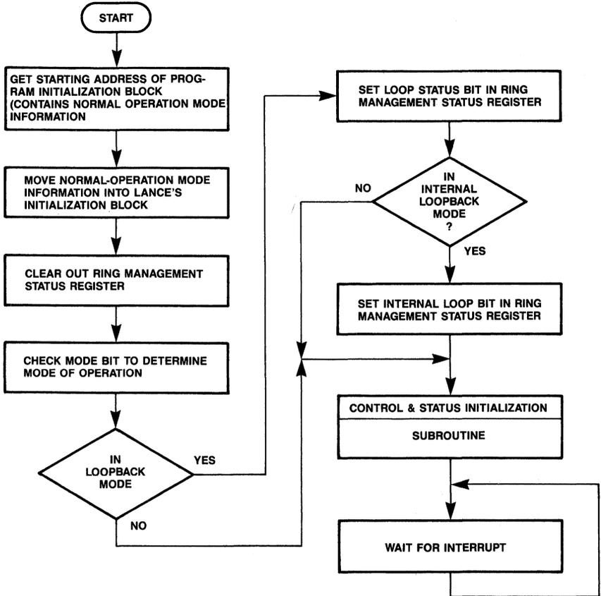
Figure 30. Normal Operation Initialization Submodule [LANCE. INITIAL. NORM]
