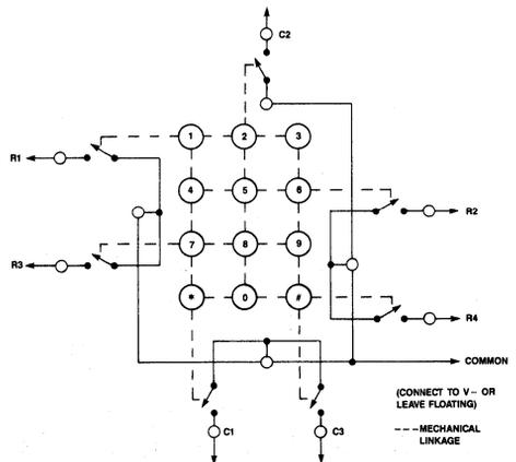
**Figure 3. Keypad Schematics**
