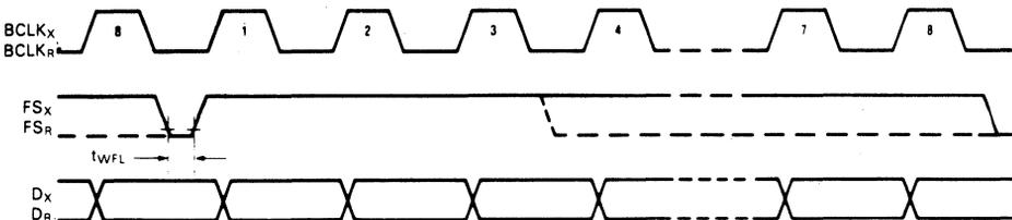
FIGURE 2 - 64 k bits/s TIMING DIAGRAM (See next page for complete timing)
