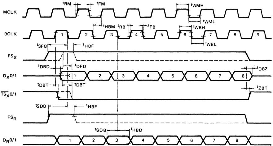
FIGURE 4 - NON DELAYED DATA TIMING
