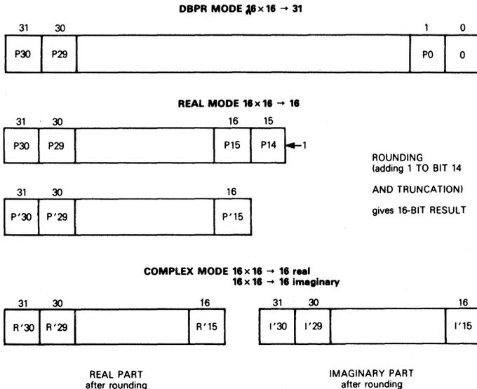
FIGURE 5.3.1. - MULTIPLICATION OUTPUT REGISTER (P) FORMATS
