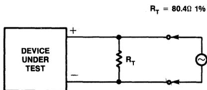
Figure 20. Receive  $\pm$  and Collision  $\pm$  Input Test Circuit
