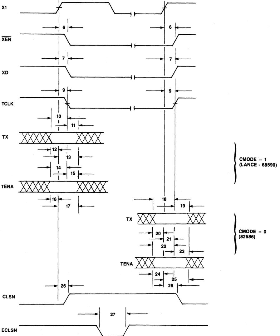
Figure 7. Transmit Timing Diagram
