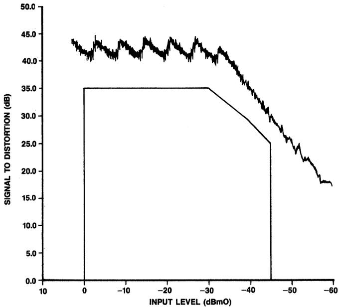
Figure 14. MK5156 Single-Ended Signal To Distortion
