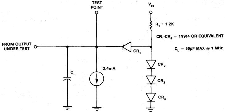
Figure 5. Output Load Diagram
