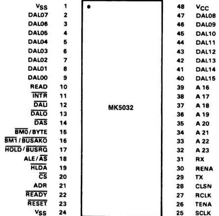
Figure 1. MK5032 Pin Assignment
