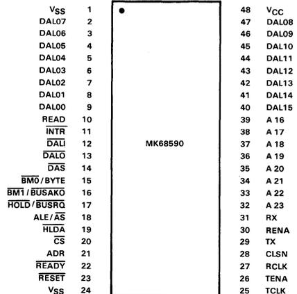
Figure 2. LANCE Pin Assignment
