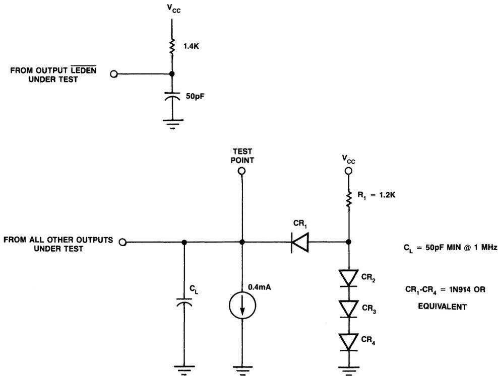
Figure 14. Output Load Diagram
