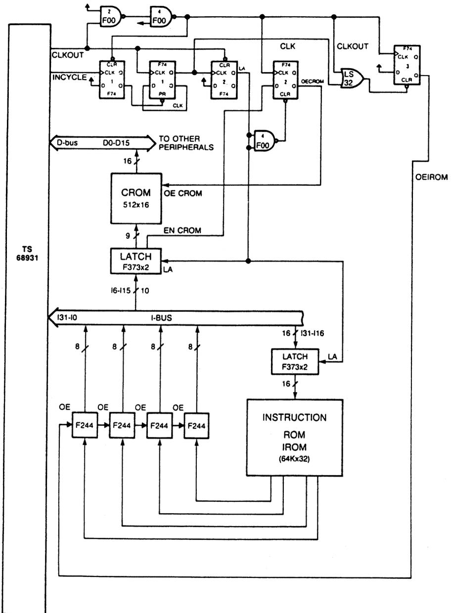
FIGURE 6.7.D. - I-BUS INTERFACE (TS68931)
