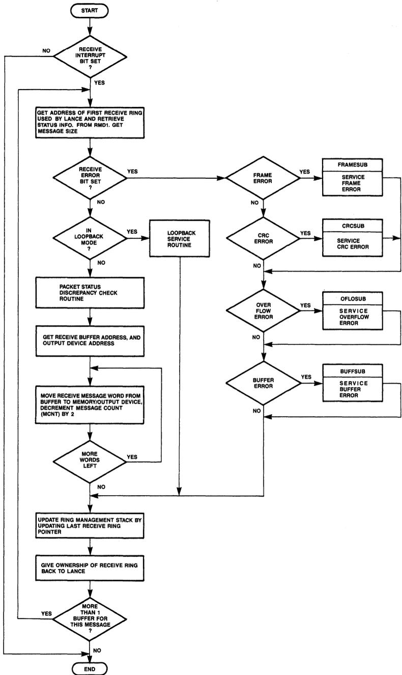
Figure 34. Receive Interrupt Handling Submodule [LANCE, LEXCEPT, RVCR]
