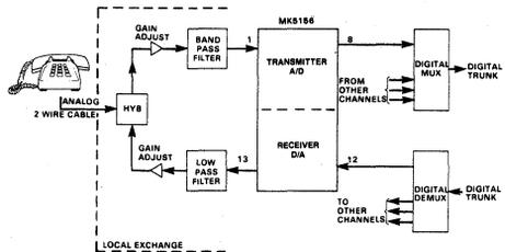
Figure 2. PCM System Block Diagram
