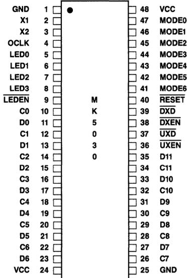
Figure 1. MK5030 Pin Assignment
