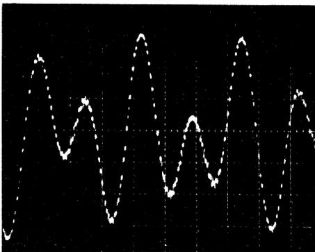
Figure 4B. Typical Dual-Tone Waveform (Row 1, Col 1)
