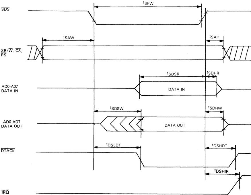
FIGURE 9.3. - SYSTEM BUS TIMING DIAGRAM
