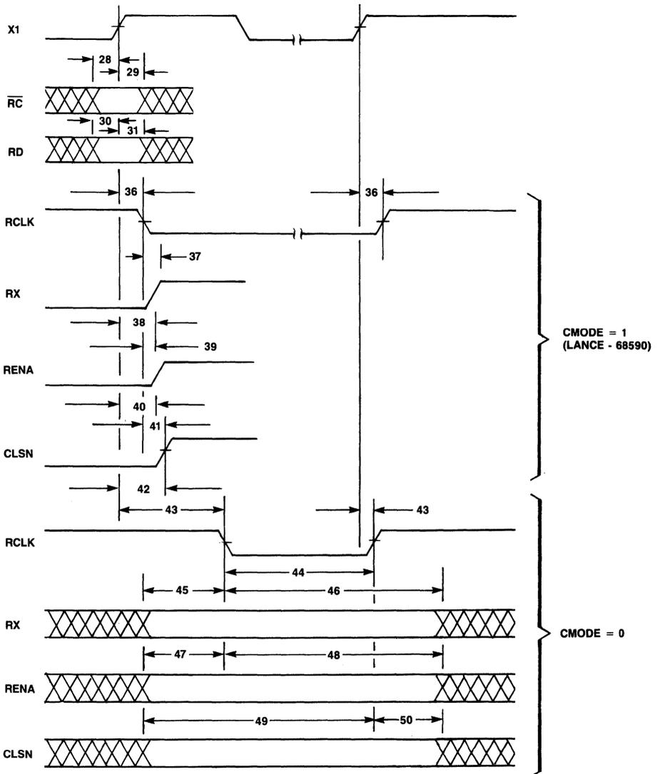
Figure 8. Receiver Timing Diagram
