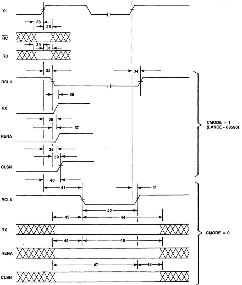
Figure 8. Receiver Timing Diagram
