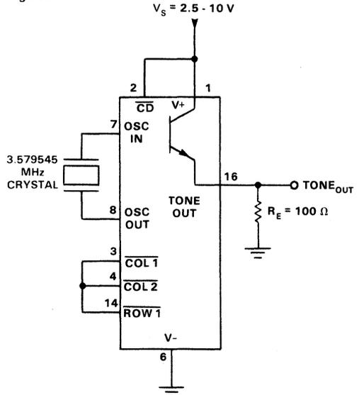
NOTE: The above circuit connections are for a Row 1 single tone test. For a Col 1 single-tone test, connect Row 1 (Pin 14) and Row 2 (Pin 13) to Col 1 (Pin 3).
