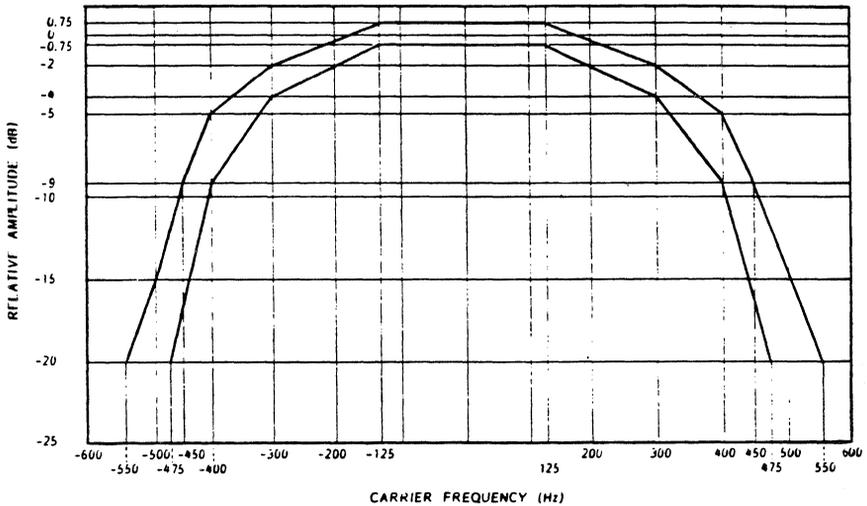
Figure 7 - Amplitude limits of signal transmitted on-line (without equalization)
