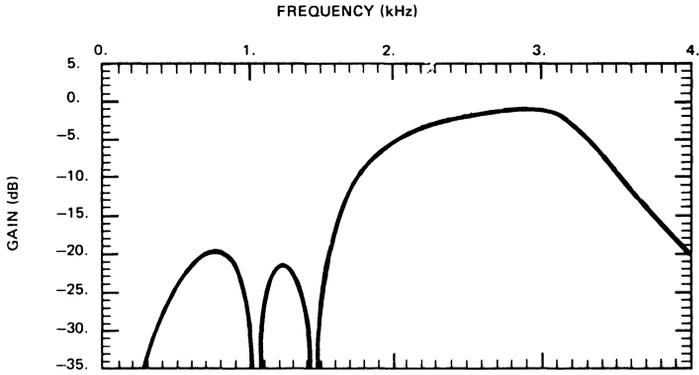
**Rx BAND-PASS FILTER TYPICAL RESPONSE FOR V.22 MODE (HIGH CHANNEL)**
