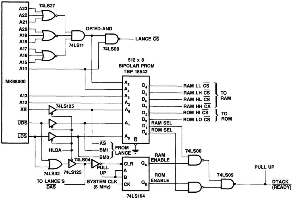
Figure 10. Chip Select Decode and DTACK Circuit
