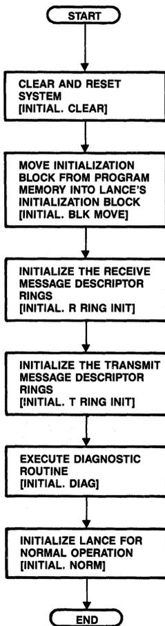
Figure 20. Initialization Software Module [LANCE. INITIAL]
