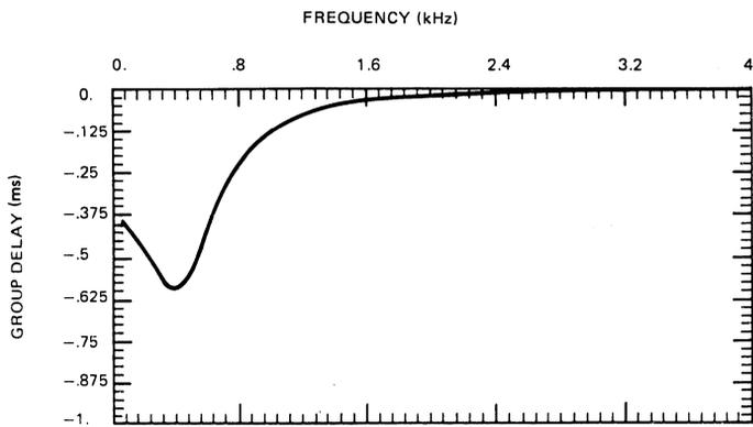
**Rx HIGH-PASS FILTER TYPICAL GROUP DELAY TIME AND LIMITS CHART ( $F_s=72\text{kHz}$ )**
