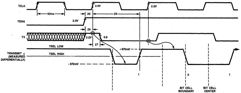
Figure 13. Transmitter Timing — Start of Transmission (TSEL Low, TSEL High)
