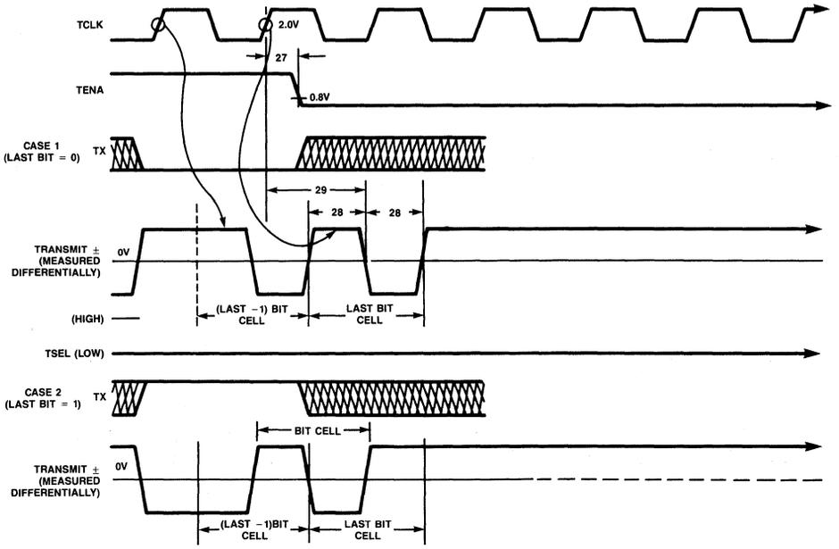
Figure 14b. Transmitter Timing — End of Transmission (TSEL Low)
