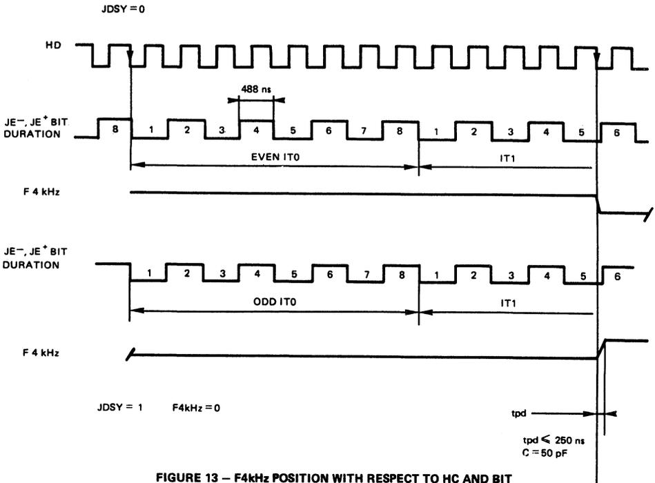
FIGURE 13 — F4kHz POSITION WITH RESPECT TO HC AND BIT DURATION OF JE+/JE—
