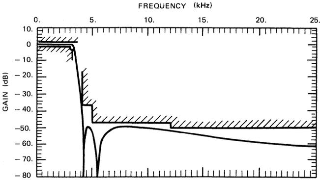
TRANSMIT LOW-PASS FILTER TYPICAL RESPONSE AND LIMITS CHART
