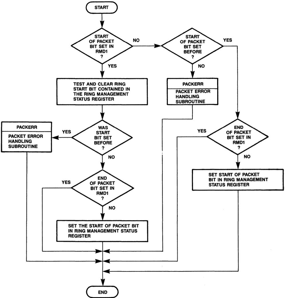
Figure 36. Packet Status Discrepancy Check Routine [LANC.E. LEXCEPT. RCVR. PACKCHECK]
