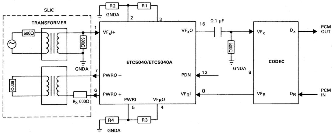
**Note 1 :** Transmit voltage gain =  $\frac{R1 + R2}{R2} \times \sqrt{2}$  (The filter itself introduces a 3 dB gain) ( $R1 + R2 \geq 10 \text{ k}\Omega$ )
