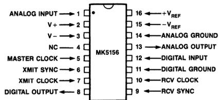
Figure 1. Pin Connections
