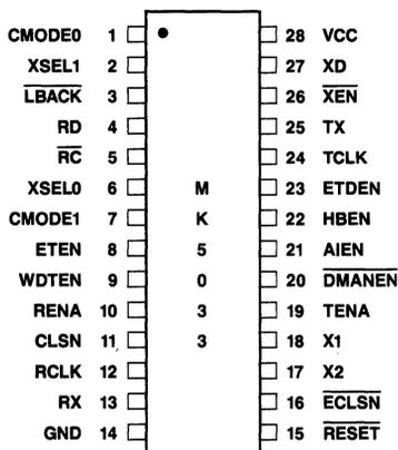
Figure 1. MK5033 Pin Assignment
