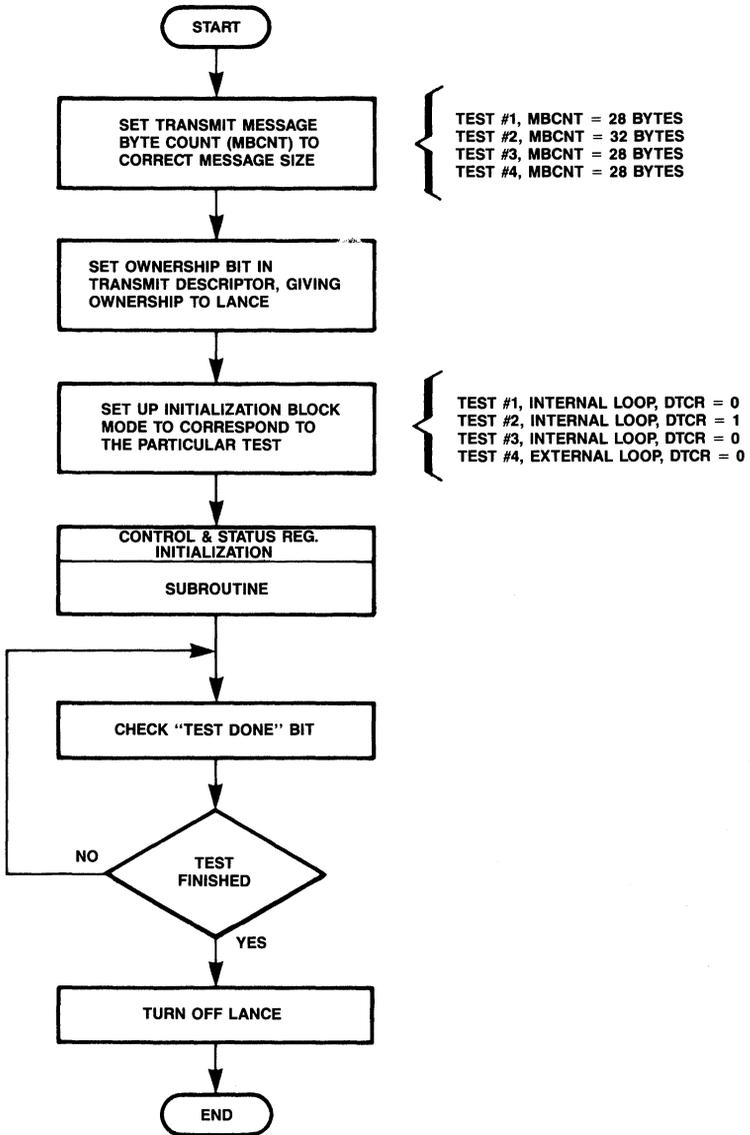
Figure 27. Loopback Diagnostic Test Routine
