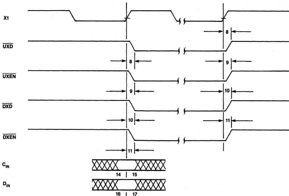
Figure 11. Retimer Enabled (MODE3 = 1) Timing Diagram
