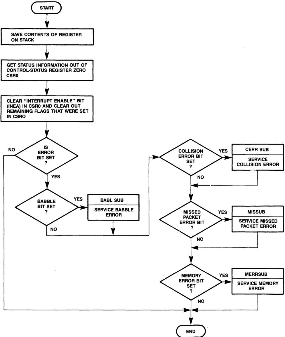
Figure 32. Interrupt Error Determination Submodule [LANCE. LEXCEPT. ERROR]
