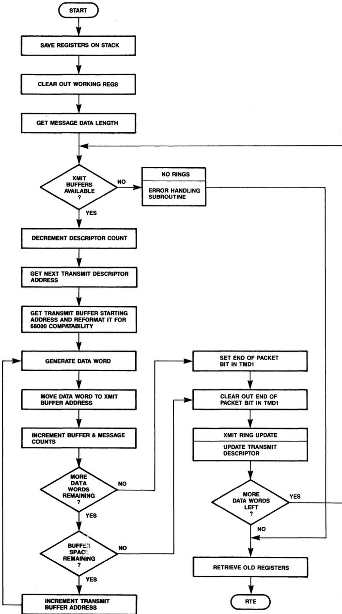
Figure 38. Message Interrupt Software Module [LANCE.MESSAGE]
