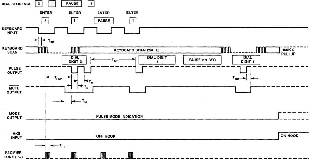
Figure 10. Pulse Mode Timing
