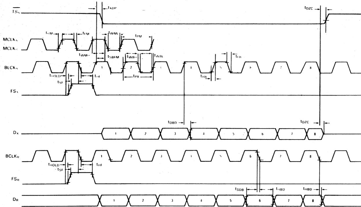
FIGURE 3 - SHORT FRAME SYNC TIMING
