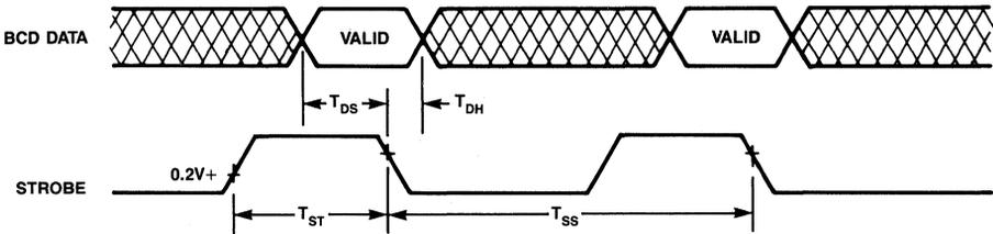
Figure 5. BCD Mode Strobe Interface Timing
