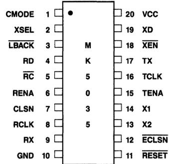
Figure 1. MK5035 Pin Assignment
