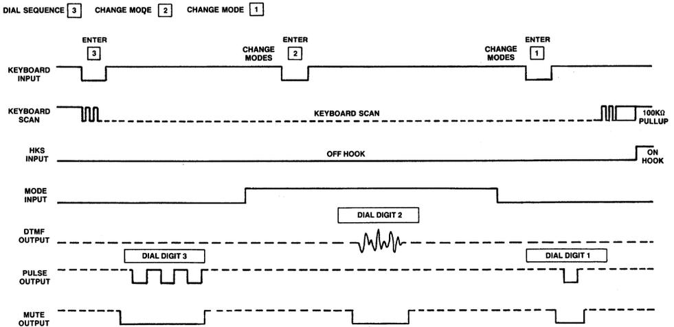
Figure 9. Pulse and Tone Mode Timing
