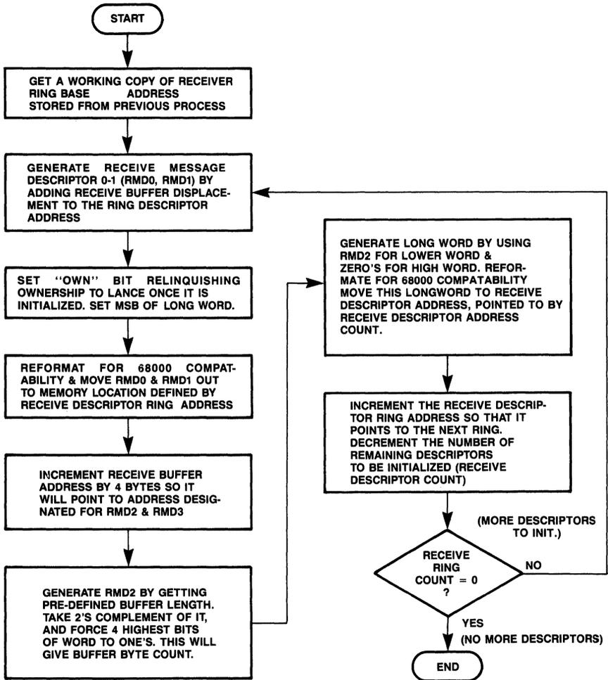
Figure 24. Receive Ring Initialization Submodule [LANCE. INITIAL. RRINGINIT]
