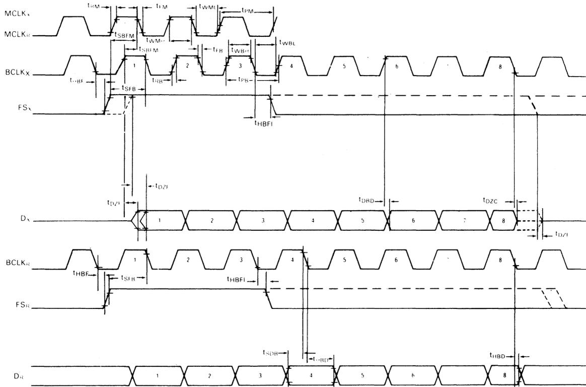
FIGURE 4 - LONG FRAME SYNC TIMING
