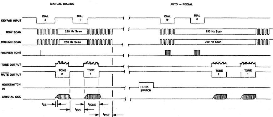
Figure 4B. MK5376 Timing Diagram — Tone Mode
