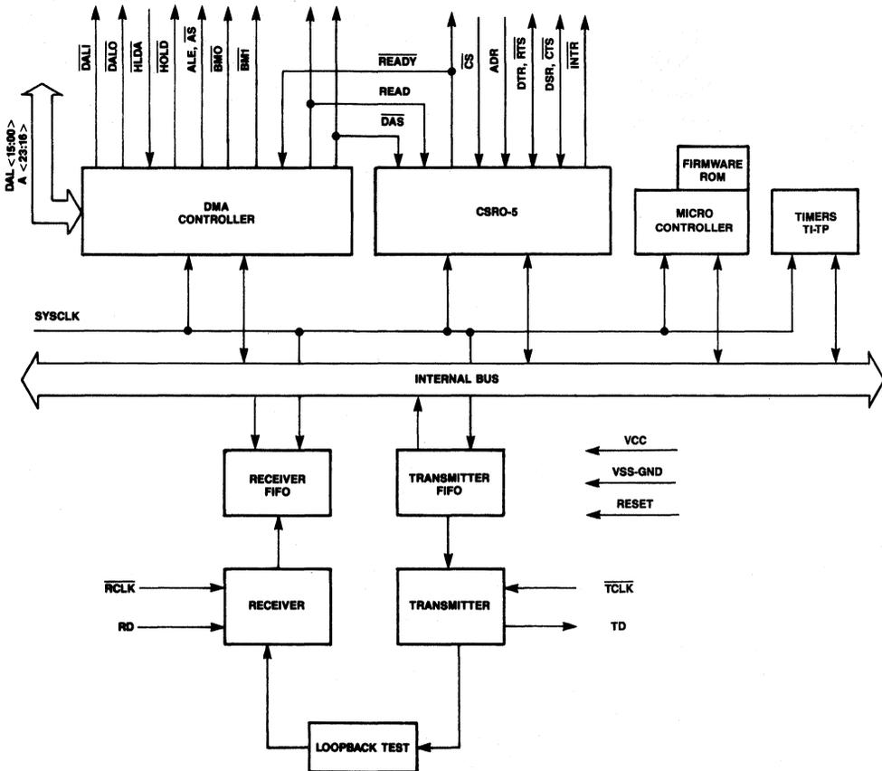
Figure 3. MK5025 Simplified Block Diagram
