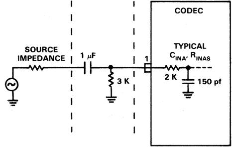
**Figure 9. Recommended Analog Input Circuit**
