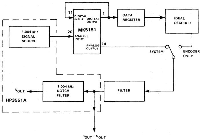
NOTE: The ideal decoder consists of a digital decomposer and a 13-bit precision DAC.
