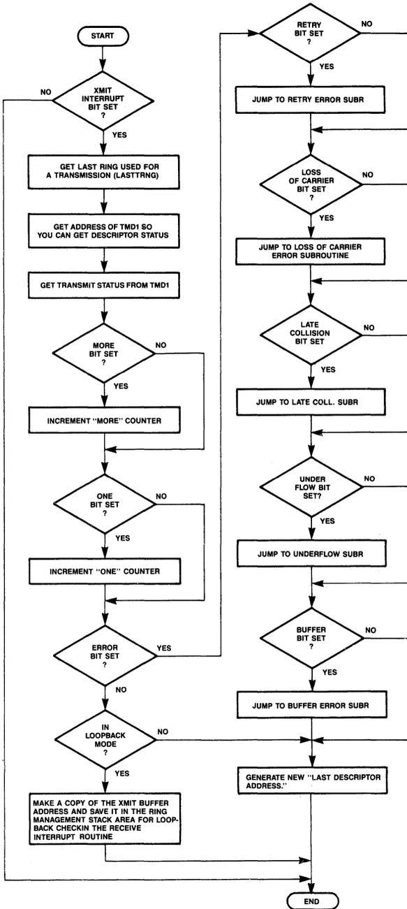
Figure 33. Transmit Interrupt Handling Submodule [LANC.E. LEXCEPT. XMIT]
