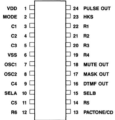
Figure 1. MK53763 Pinout
