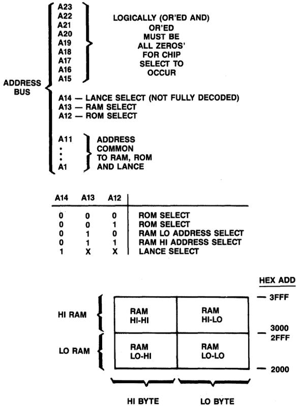
Figure 11. Chip Select Decode Description
