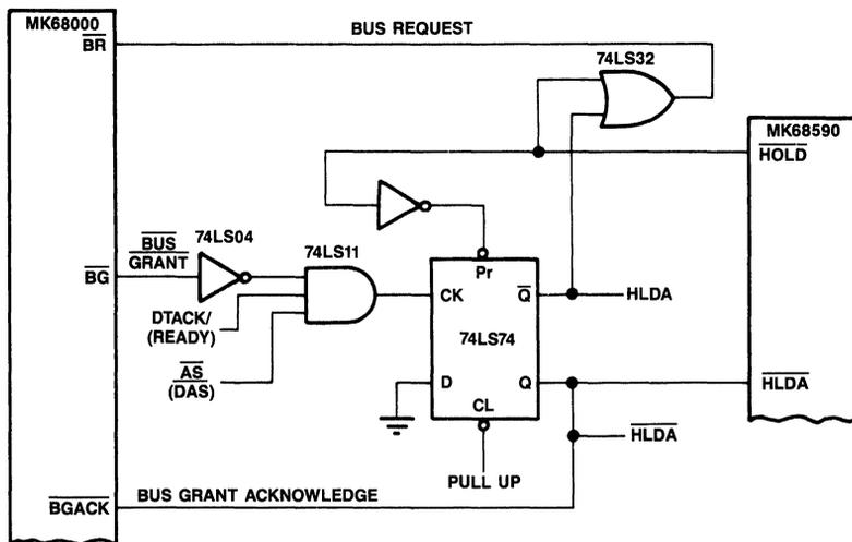
Figure 16. Bus Arbitration Circuit
