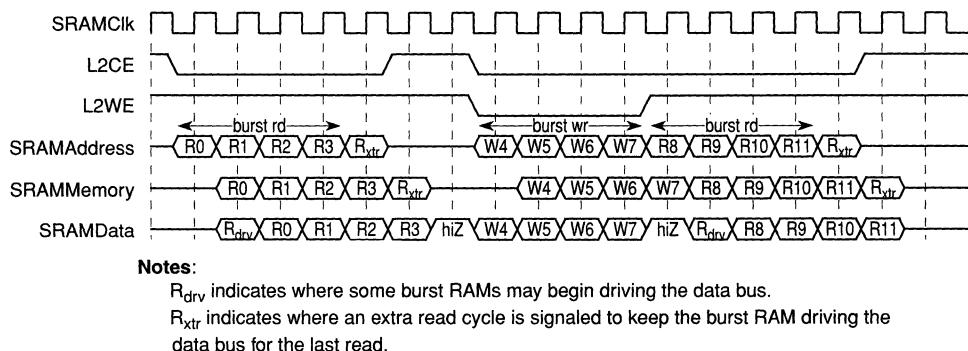
**Figure 9-5. Burst Read-Write-Read L2 Cache Access (Pipelined)**
