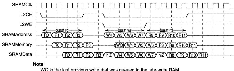
**Figure 9-8. Burst Read-Write-Read L2 Cache Access (Late-Write SRAM)**
