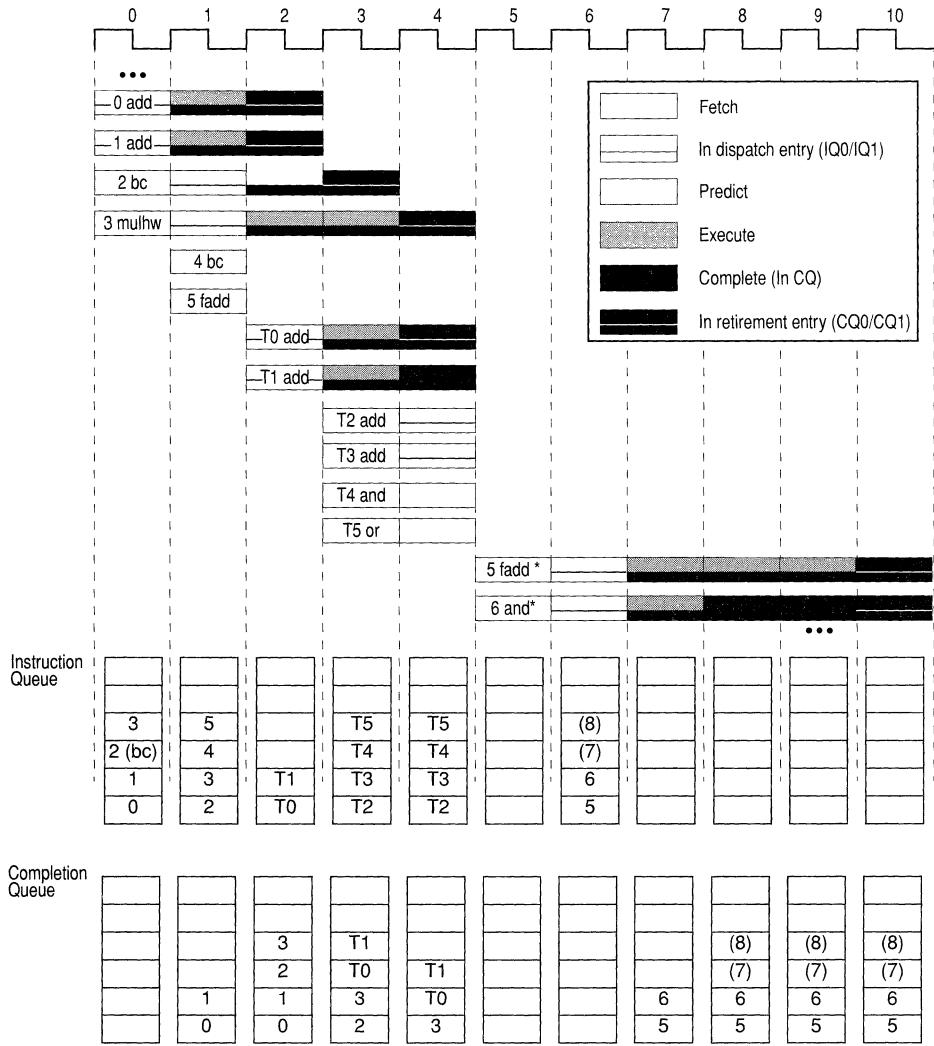
\* Instructions 5 and 6 are not in the IQ in clock cycle 5. Here, the fetch stage shows cache latency.
