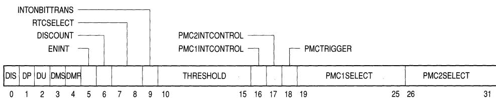
Figure 2-5. Monitor Mode Control Register 0 (MMCR0)
