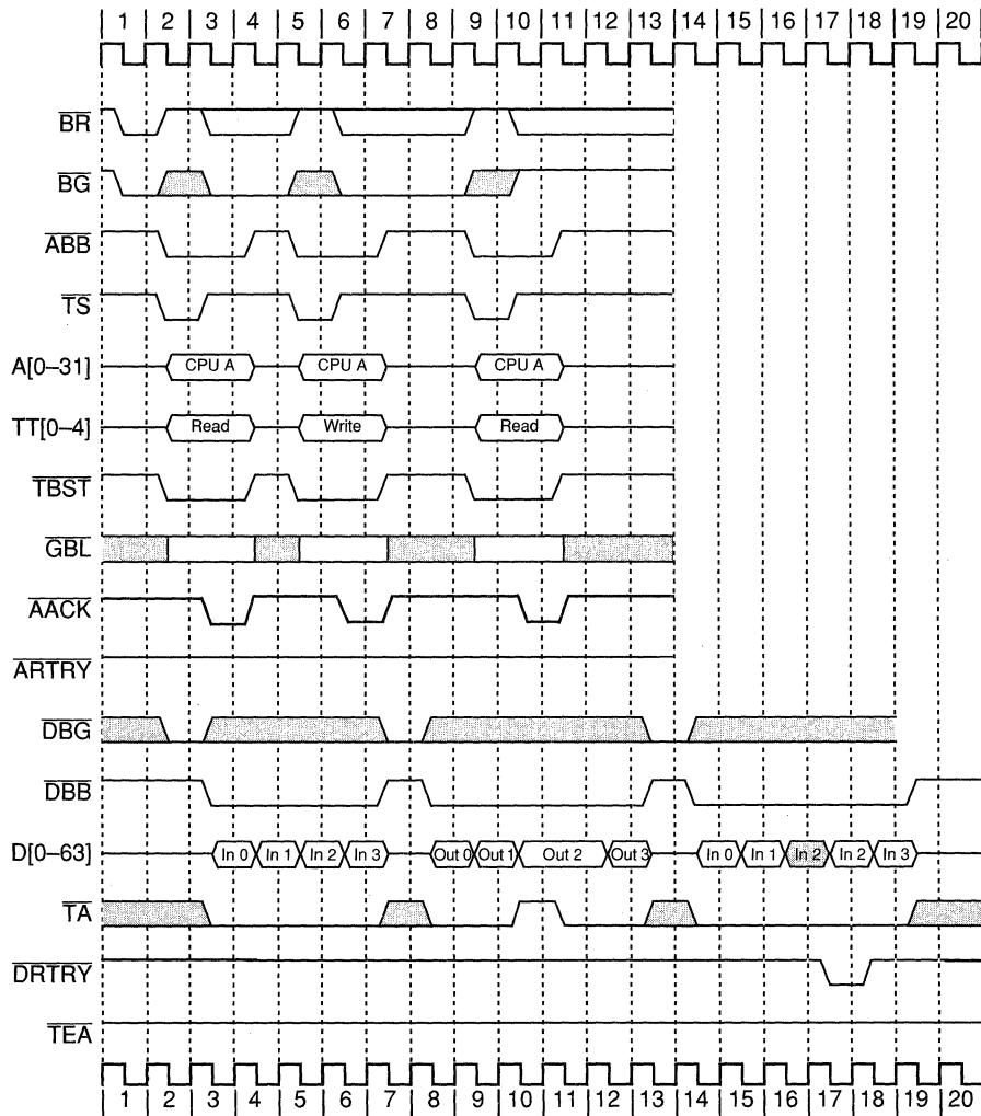
**Figure 8-19. Burst Transfers with Data Delay Controls**
