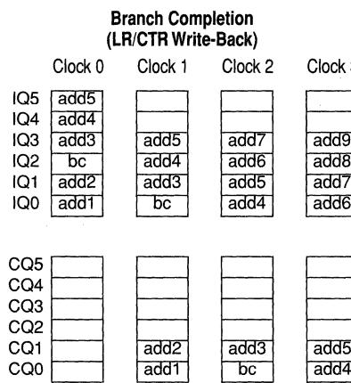
**Figure 6-9. Branch Completion**
