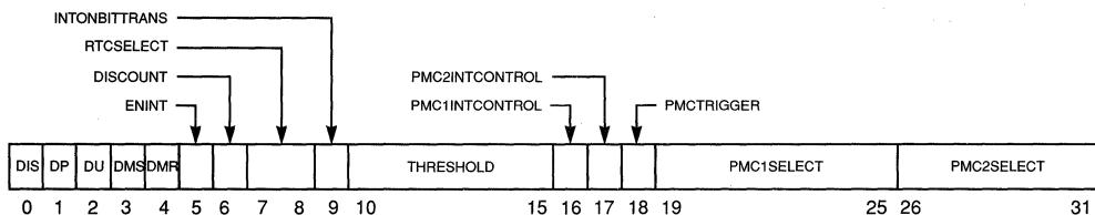
**Figure 11-1. Monitor Mode Control Register 0 (MMCR0)**
