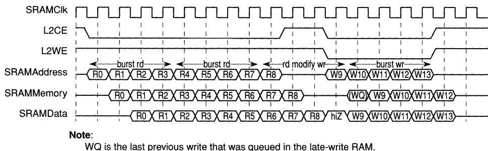
**Figure 9-9. Burst Read-Modify-Write L2 Cache Access (Late-Write SRAM)**
