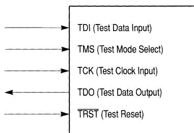
Figure 8-21. IEEE 1149.1a-1993 Compliant Boundary Scan Interface
