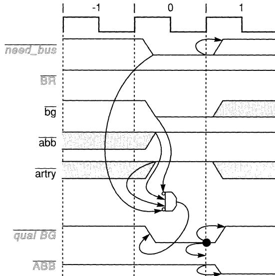
**Figure 8-5. Address Bus Arbitration Showing Bus Parking**
