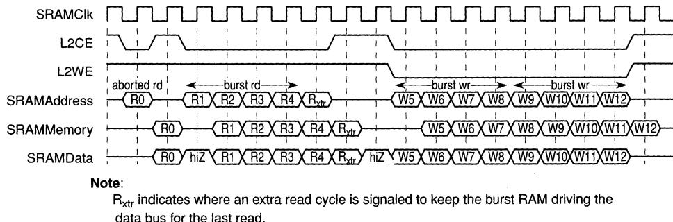
**Figure 9-4. Burst Read-Write-Write L2 Cache Access (Flow-Through)**
