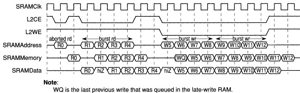
**Figure 9-10. Burst Read-Write-Write L2 Cache Access (Late-Write SRAM)**
