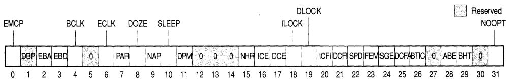
**Figure 2-3. Hardware Implementation-Dependent Register 0 (HID0)**
