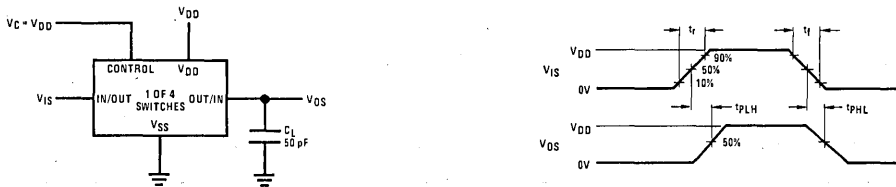
FIGURE 1. tPHL, tPLH Propagation Delay Time Signal Input to Signal Output
