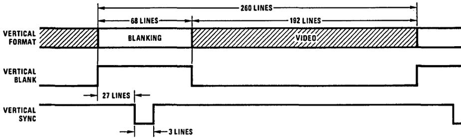
FIGURE 24. DP8352 60 Hz Refresh Rate Frame Signals
