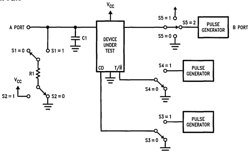
FIGURE A. A Port Test Load
