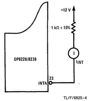
FIGURE 3. INTA Test Circuit (For RST 7)
