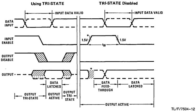
\*When the Input Enable makes a positive transition the output will be indeterminate for a short duration. The positive transition of the Input Enable normally occurs during a don't care timing state at the output.
