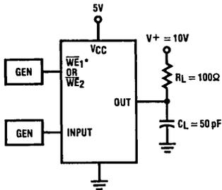
\* $\overline{WE}_1 = 0V$  When the Input =  $\overline{WE}_2$
