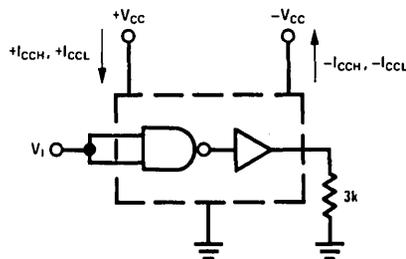
FIGURE 5. I<sub>CCH+</sub>, I<sub>CCH-</sub>, I<sub>CCL+</sub>, I<sub>CCL-</sub>
