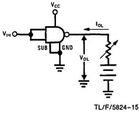
Both inputs are tested simultaneously.
