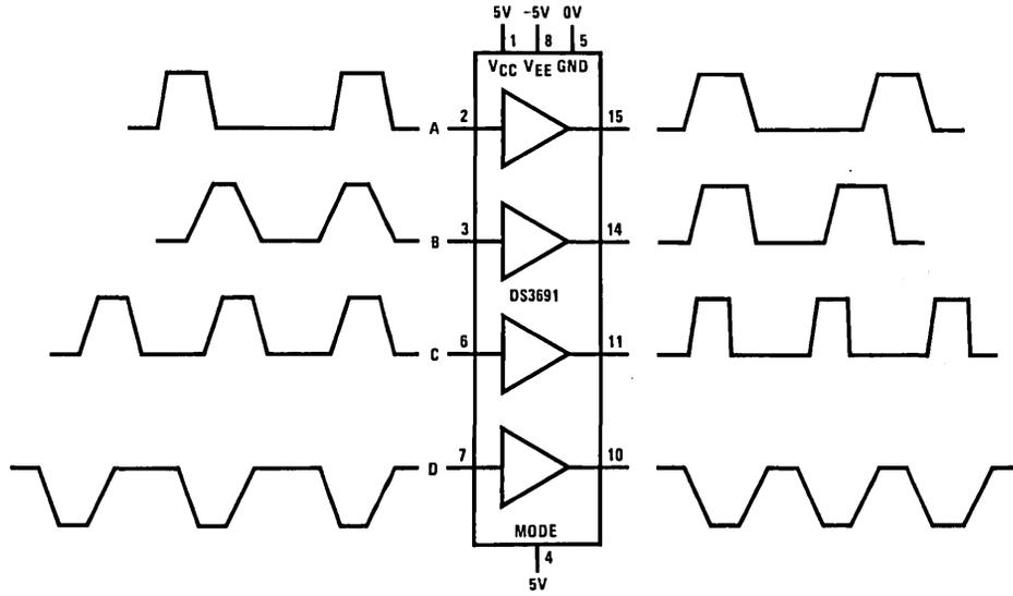
FIGURE 9. DS3691 Connected for Unbalanced Mode Operation
