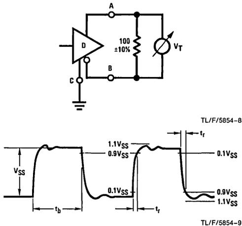
$t_b$  = Time duration of the unit interval at the applicable modulation rate.
