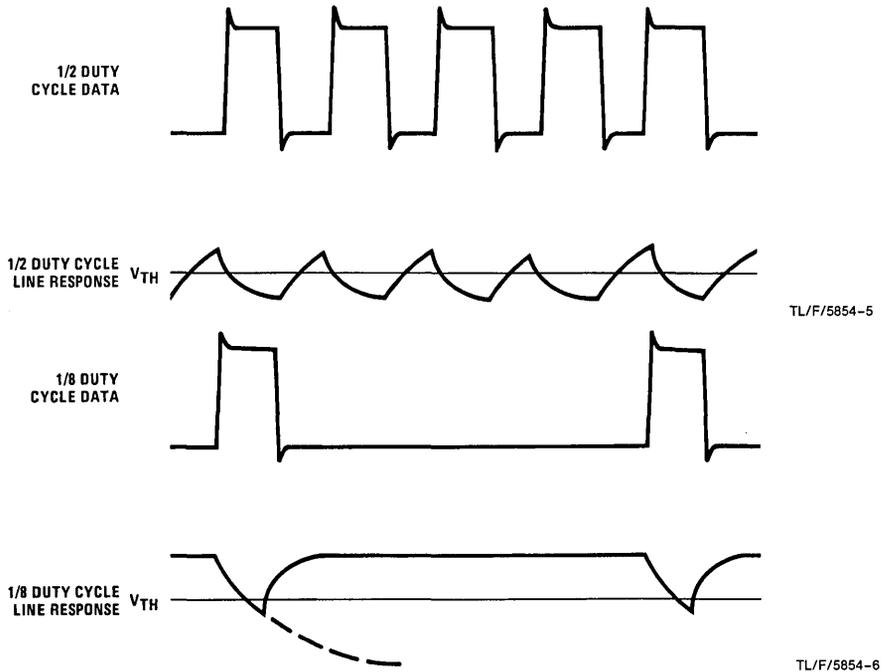
FIGURE 3b. Signal Distortion Due to Duty Cycle
