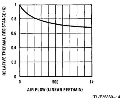
FIGURE 14. Thermal Resistance vs Air Velocity
