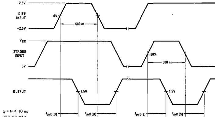
Note: Optimum switching response is obtained by minimizing stray capacitance on Response Control pin (no external connection).
