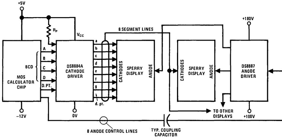
FIGURE 4. BCD Data Interfacing Directly With MOS Output
