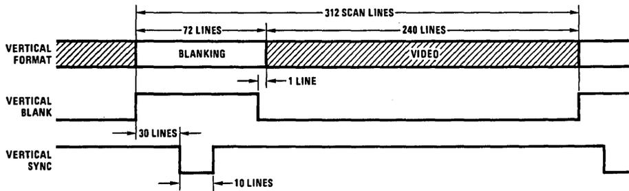
FIGURE 21. DP8350 50 Hz Refresh Rate Frame Signals
