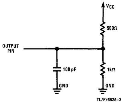
FIGURE 2. Test Load
