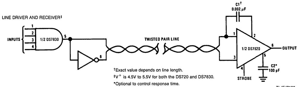
FIGURE 19. Interconnection of the Line Driver and Line Receiver
