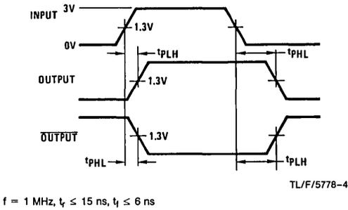
FIGURE 2. Propagation Delays
