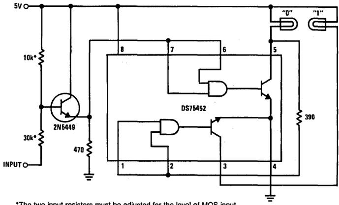
\*The two input resistors must be adjusted for the level of MOS input.
