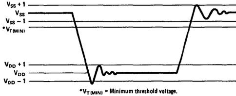
**FIGURE 6. Clock Waveform**
