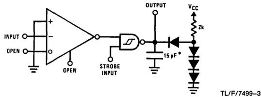
\*Includes probe and test fixture capacitance
