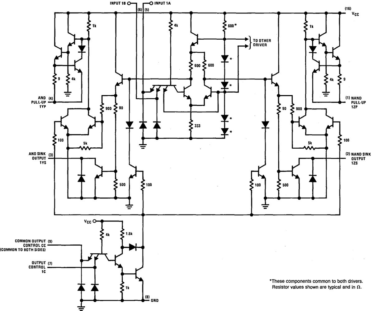
\*These components common to both drivers. Resistor values shown are typical and in  $\Omega$ .
