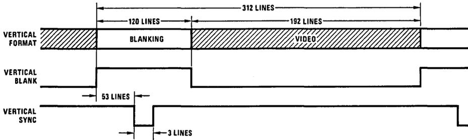
FIGURE 25. DP8352 50 Hz Refresh Rate Frame Signals
