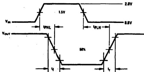
$t_r$  and  $t_f$  are measured between 10% and 90% of the output waveform.
