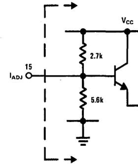
$I_{ADJ}$  may be programmed by a voltage source or by resistors.
