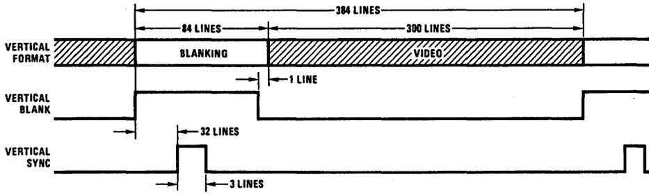
FIGURE 30. DP8353 50 Hz Refresh Rate Frame Signals
