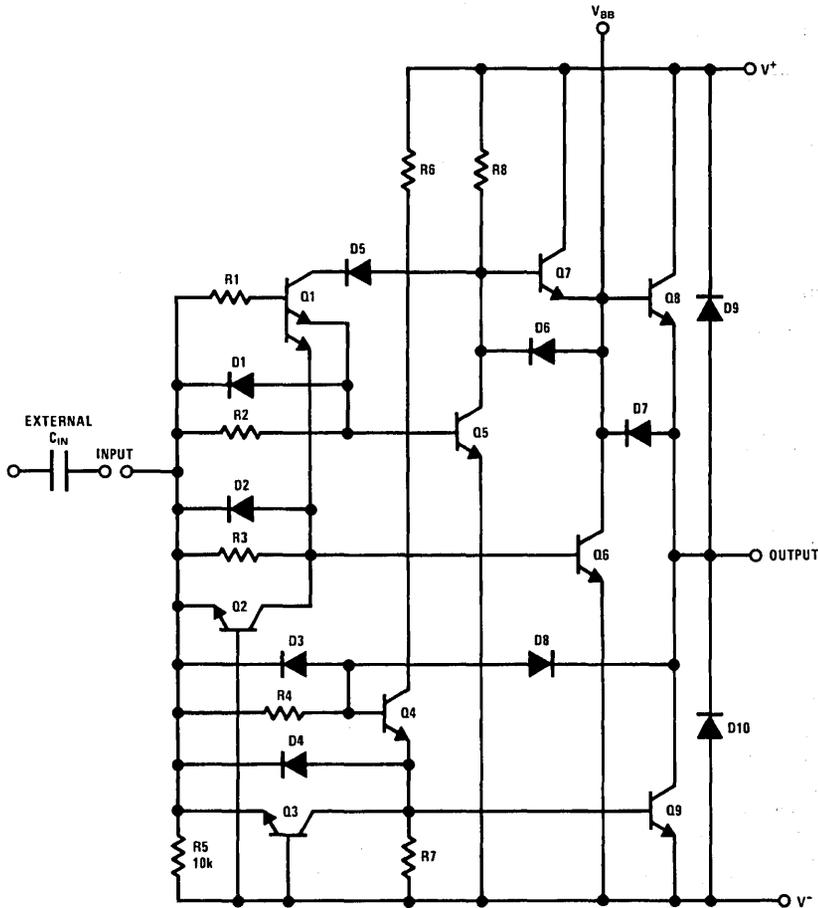
**FIGURE 7. Schematic of 1/2 DS0056**
