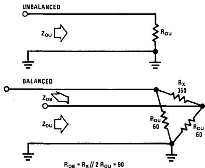
FIGURE 16. Impedance Measurement
