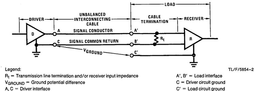
FIGURE 1b. RS-423 Unbalanced Digital Interface Circuit
