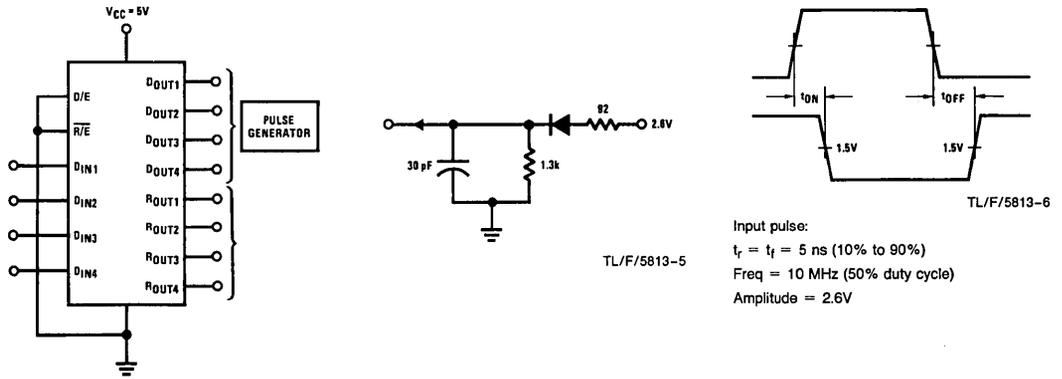
FIGURE 1. Propagation Delay ( $D_{OUT}$  to  $R_{OUT}$ )
