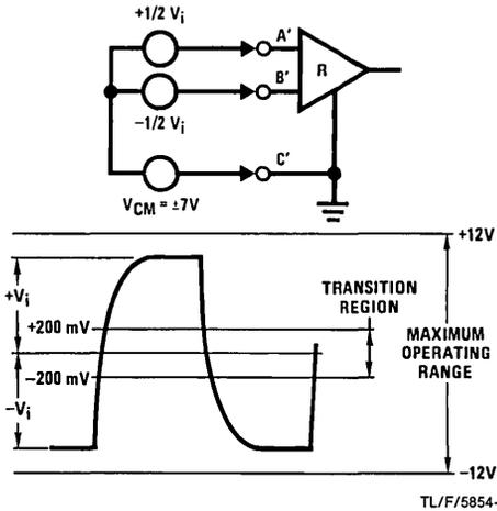
**FIGURE 6. Receiver Input Sensitivity Measurement**
