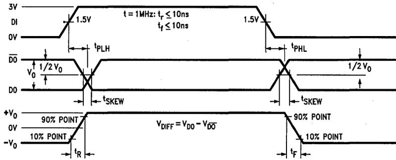
FIGURE 5. Driver Propagation Delays
