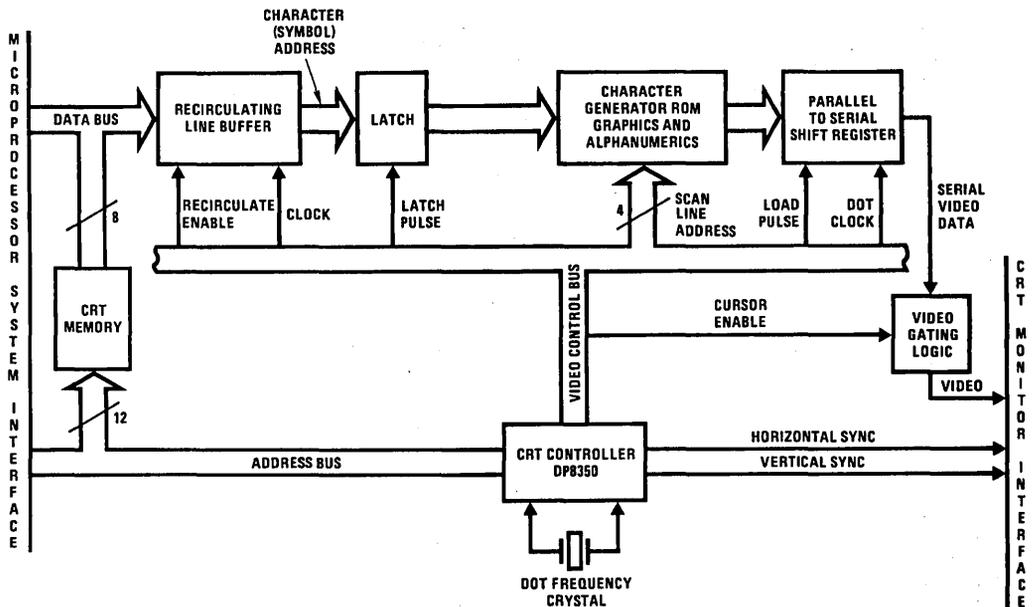
FIGURE 5. Character Generator Graphics (with line buffer)
