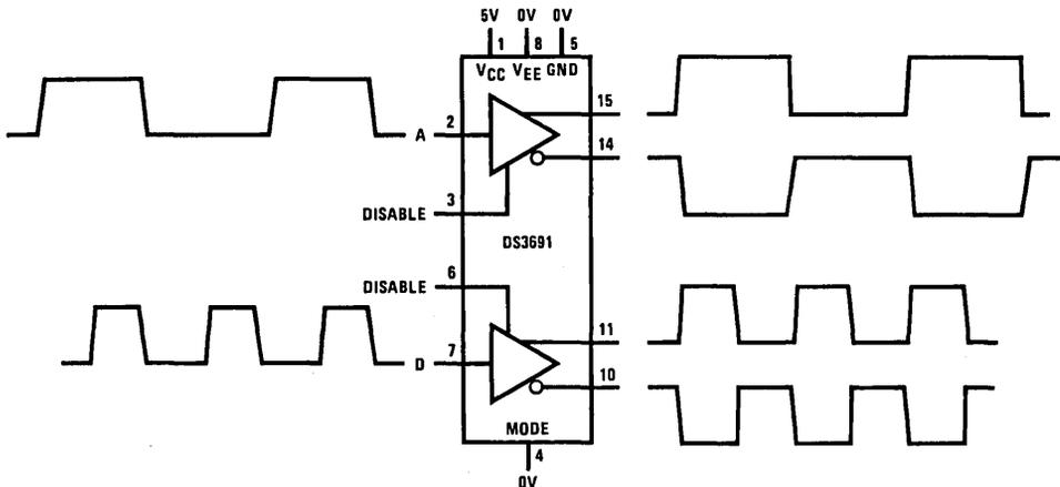
**FIGURE 8. DS3691 Connected for Balanced Mode Operation**
