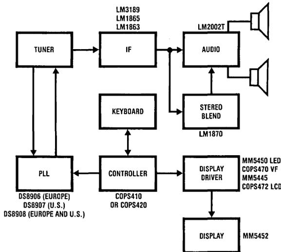
**FIGURE 12. AM-FM Digitally Tuned Radio System**
