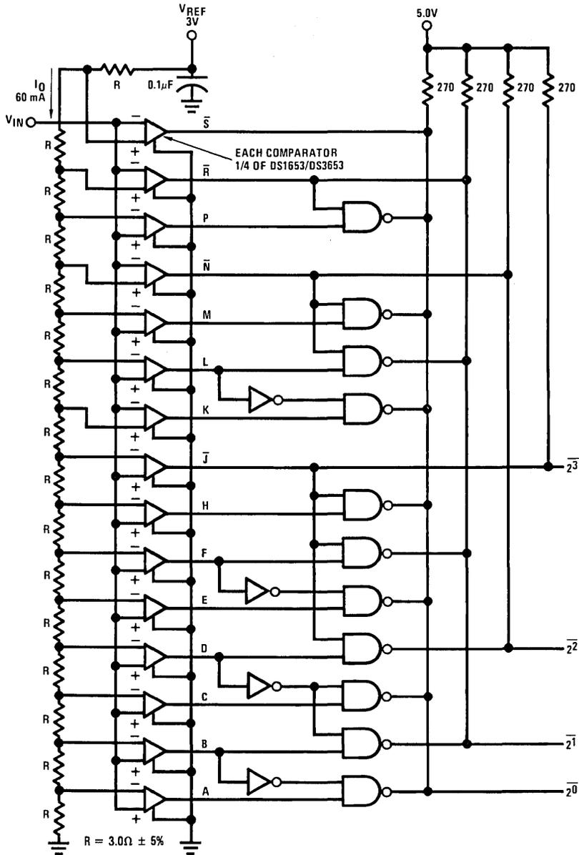
$$2^0 = (\bar{A} + B) (\bar{C} + D) (\bar{E} + F) (\bar{H} + J) (\bar{K} + L) (\bar{M} + N) (\bar{P} + R) (\bar{S})$$
