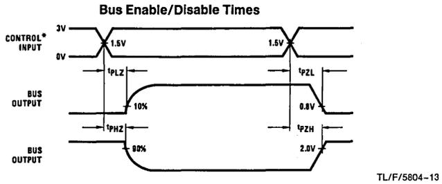
\*Input signal:  $f = 1.0 \text{ MHz}$ , 50% duty cycle,  $t_r = t_f \leq 5 \text{ ns}$
