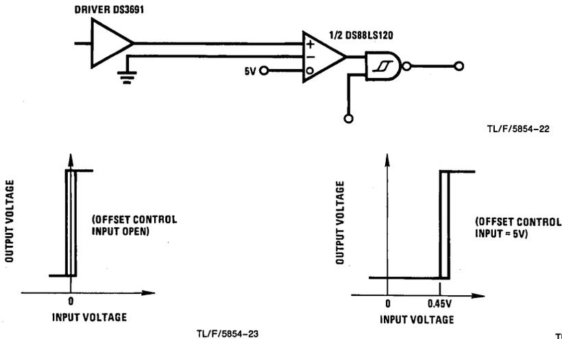
**FIGURE 16. Fail-Safe Using the DS88LS120 Threshold Offset for Unbalanced Lines**
