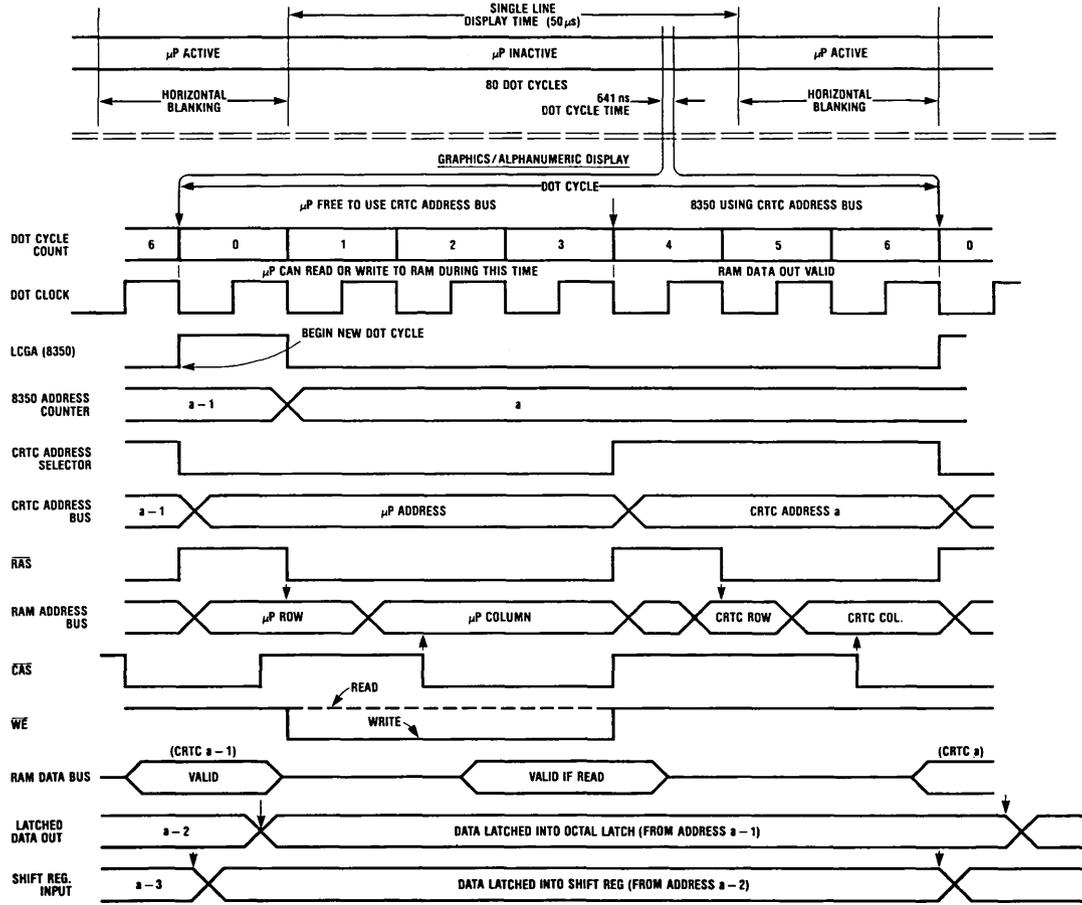
FIGURE 11. Memory Control Logic Timing Diagram
