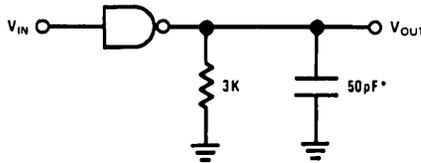
\* $C_L$  includes probe and jig capacitance.
