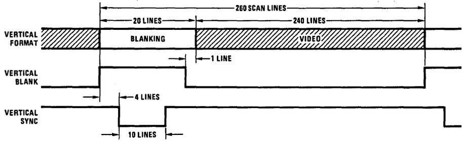
FIGURE 20. DP8350 60 Hz Refresh Rate Frame Signals
