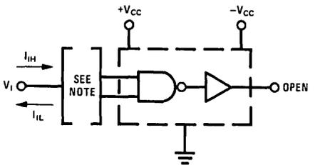
FIGURE 3. I<sub>IH</sub>, I<sub>IL</sub>
