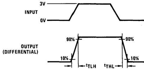
Input pulse;  $f = 1\text{MHz}$ , 50%;  $t_r = t_f < 6\text{ns}$ .
