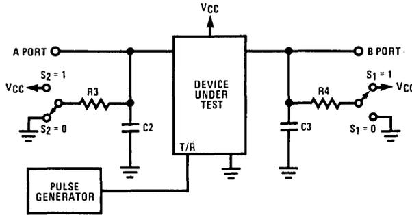
Note: C2 and C3 include test fixture capacitance.
