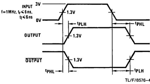
FIGURE 2. Propagation Delays
