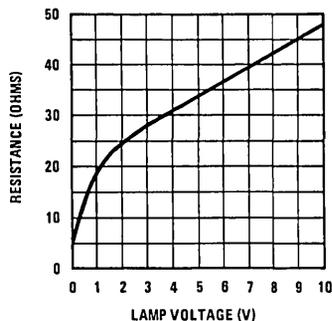
FIGURE 20. DC Characteristics of an Incandescent Lamp
