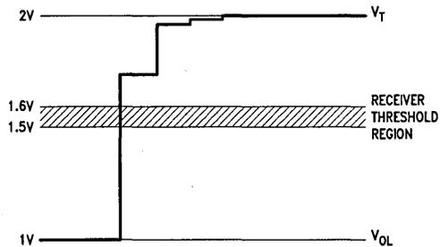
FIGURE 5. P896 Signaling Levels and the Worst-Case Bus Waveform
