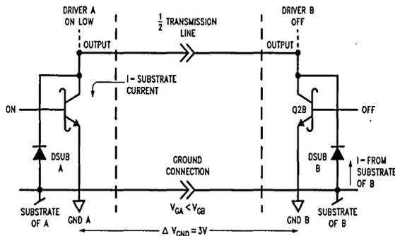
FIGURE 2b. Two DCEs Separated by a Ground Drop
