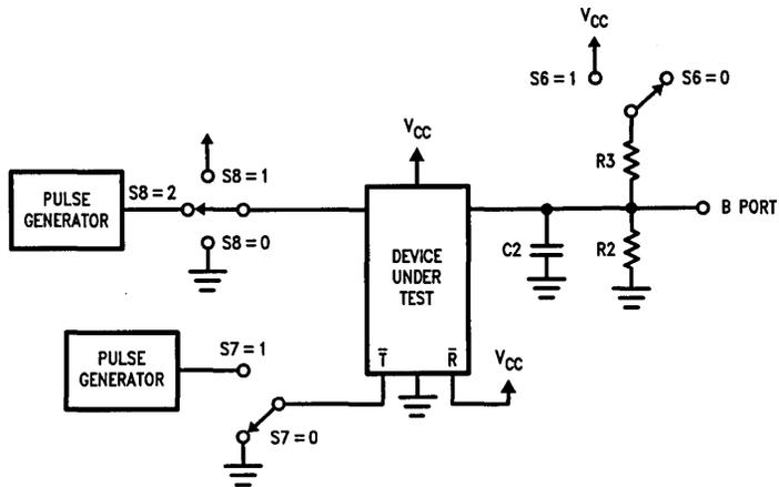
FIGURE B. B Port Test Load
