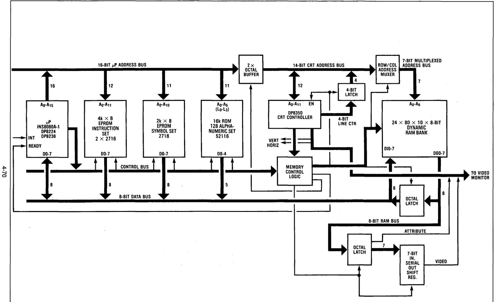
FIGURE 14. Complex Alphanumeric/Graphics/Symbol Display Terminal
