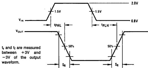
$t_r$  and  $t_f$  are measured between  $+3\text{V}$  and  $-3\text{V}$  of the output waveform.
