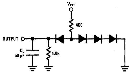
FIGURE 2. Receiver Output Load
