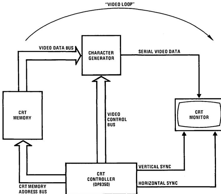
FIGURE 1. Elements of the "Video Loop"
