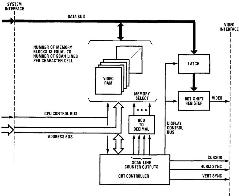
FIGURE 17. Dot-By-Dot Graphics Block Diagram
