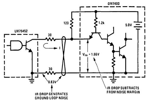
FIGURE 9. Unbalanced Method
