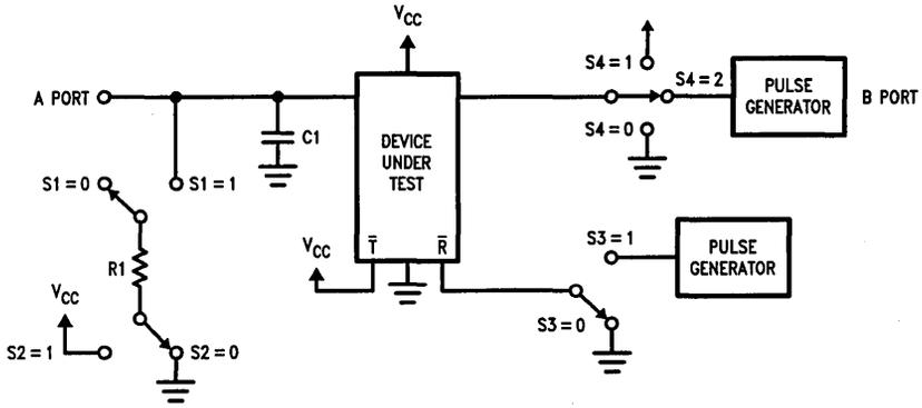
FIGURE A. A Port Test Load
