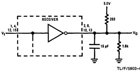
Note:  $t_r = t_f = 15$  ns. Pulse width = 500 ns measured between 1.7V levels.  $f = 1$  MHz.
