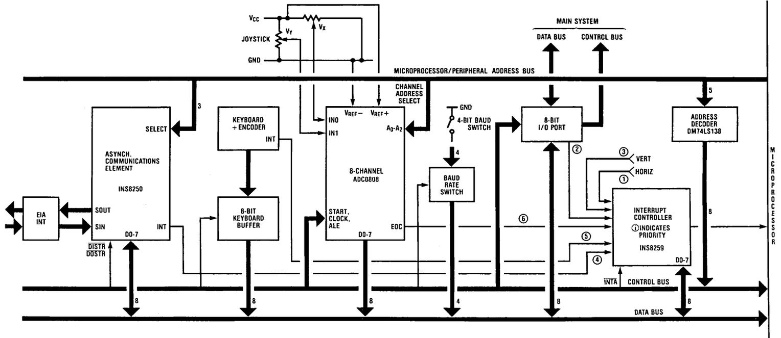
FIGURE 13. Interfacing to Various Peripheals
