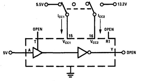
All four line receivers are tested simultaneously.
