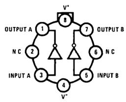
Note: Pin 4 connected to case.
