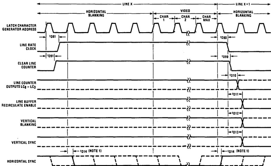
**Note 1:** Actual polarity and position of the horizontal sync start and stop points is a function of the particular device format.
