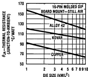
FIGURE 7. Thermal Resistance vs Lead Frame Material
