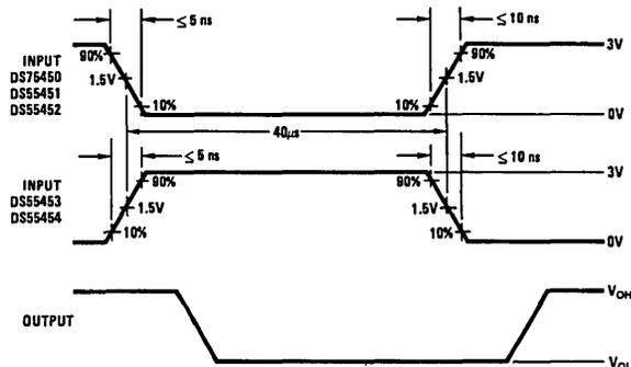
**Note 1:** The pulse generator has the following characteristics: PRR = 12.5 kHz,  $Z_{OUT} \approx 50\Omega$ .
