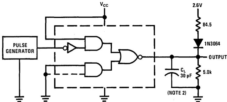
**Note 1:** The pulse generator has the following characteristics:  $Z_{OUT} \approx 50\Omega$ ,  $t_W = 200$  ns, duty cycle = 50%
