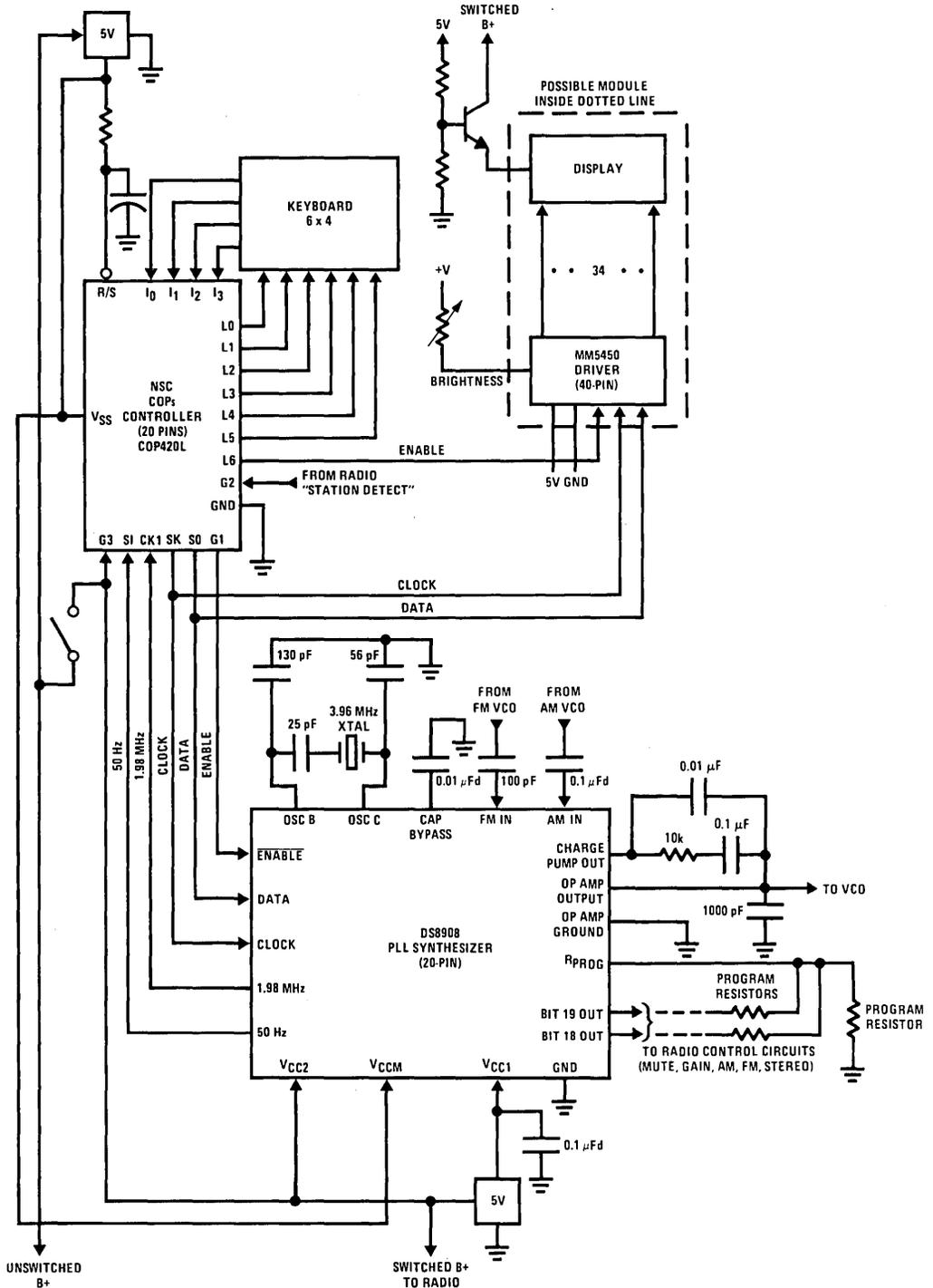
AM/FM PLL/Synthesizer (Serial Data 20-Pin Package)
