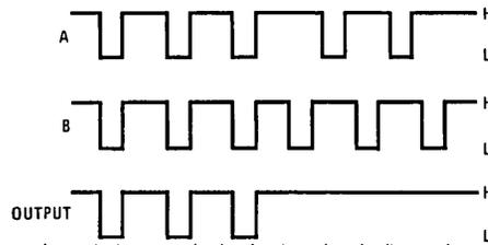
Low output occurs only when inputs are low simultaneously.
