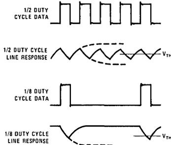
FIGURE 7. Signal Distortion Due to Duty Cycle
