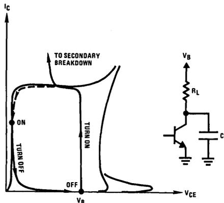
FIGURE 6. Capacitive Load Transfer Characteristics
