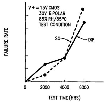
In order to achieve reliability performance comparable to DIPs—SO packages are designed and built with materials and processes that effectively compensate for their small size.
