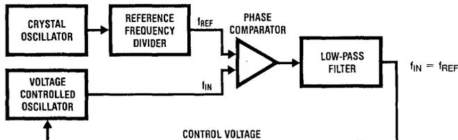
FIGURE 3. Basic Phase-Locked-Loop
