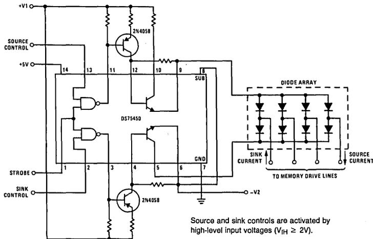
Source and sink controls are activated by high-level input voltages ( $V_{IH} \geq 2V$ ).
