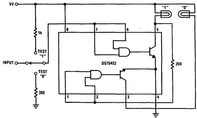
FIGURE 30. TTL or DTL Positive Logic-Level Detector
