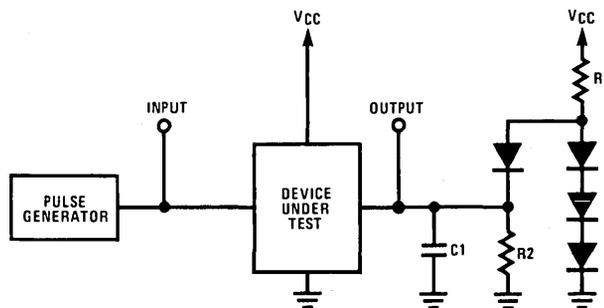
**Note:** C1 includes test fixture capacitance.
