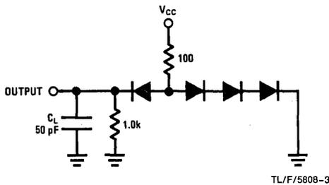
FIGURE 1. Driver Output Load
