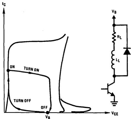
FIGURE 5. Inductive Load Transfer Characteristics Clamped by Diode
