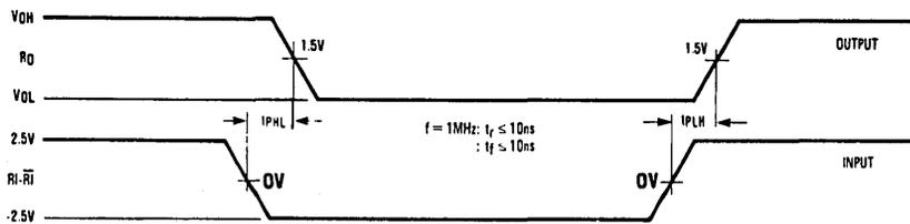
Note: Differential input voltage may be realized by grounding  $\bar{R}_I$  and pulsing  $R_I$  between +2.5V and -2.5V
