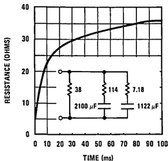
FIGURE 19. Transient Response of an Incandescent Lamp
