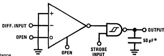
\*Includes probe and test fixture capacitance
