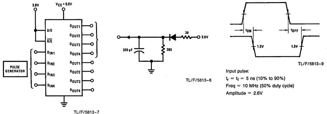
FIGURE 2. Propagation Delay ( $D_{IN}$  to  $D_{OUT}$ )
