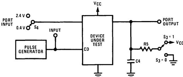
Note: C4 includes test fixture capacitance.
