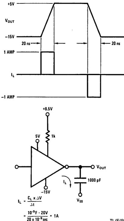
FIGURE 8. Clock Waveforms (Voltage and Current)
