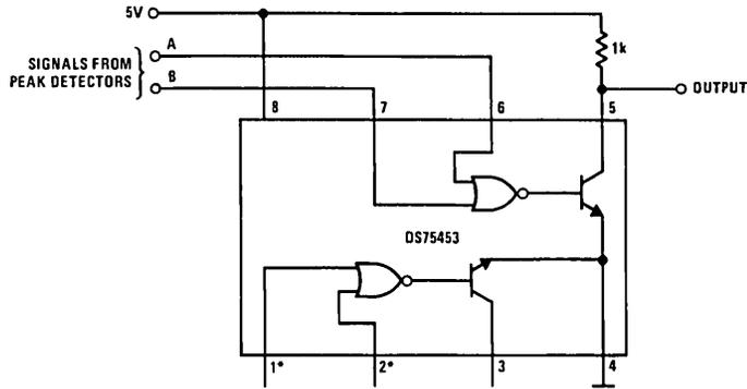
\*If inputs are unused, they should be connected to +5V through a 1k resistor.
