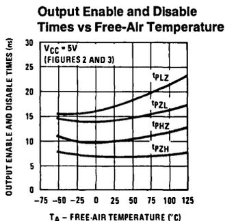
\*Data for temperatures below 0°C and above 70°C and for supply voltages below 4.75V and above 5.25V are applicable to DS55113 circuits only. These parameters were measured with the active pull-up connected to the sink output.
