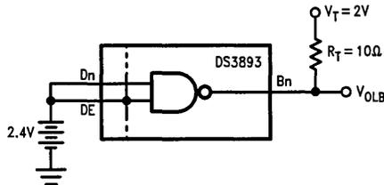
FIGURE 2. Driver Output Low Voltage
