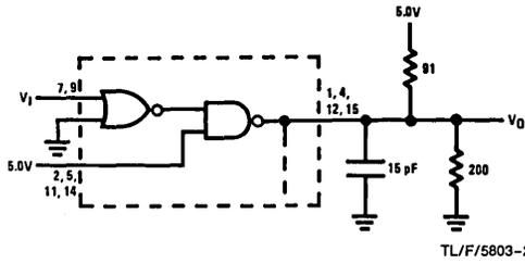
Note:  $t_r = t_f = 2.5$  ns. Pulse width = 500 ns measured between 1.5V levels.  $f = 1$  MHz.
