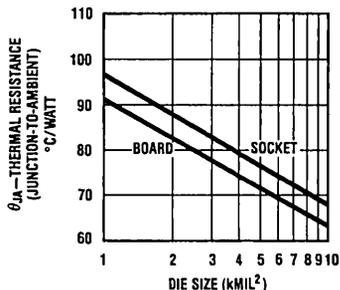
FIGURE 8. Thermal Resistance vs Board or Socket Mount
