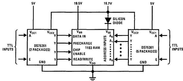
FIGURE 2. Interconnection of DS75361 Devices with 1103 RAM
