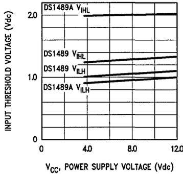
**FIGURE 5. Input Threshold vs Power Supply Voltage**
