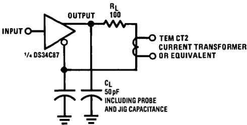
FIGURE 4. Differential Rise and Fall Times
