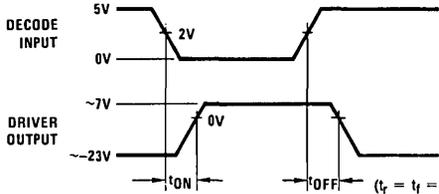
Duty Cycle =  $\frac{t_{ON}}{t_p}$
