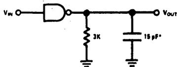
\* $C_L$  includes probe and jig capacitance.
