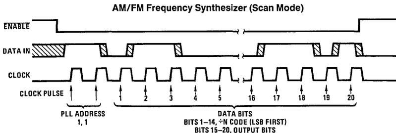
NEGATIVE TRANSITION ON ENABLE CLEARS PREVIOUS ADDRESS. CLOCK MUST BE LOW DURING TRANSITION.
