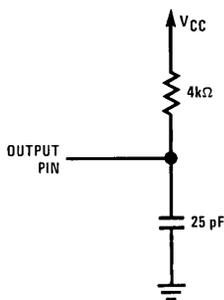
FIGURE 1. Test Load
