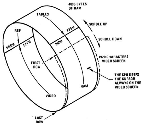
FIGURE 9. Drum Analogy for the RAM
