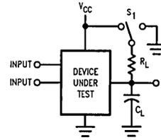
$C_L$  includes load and test jig capacitance.
