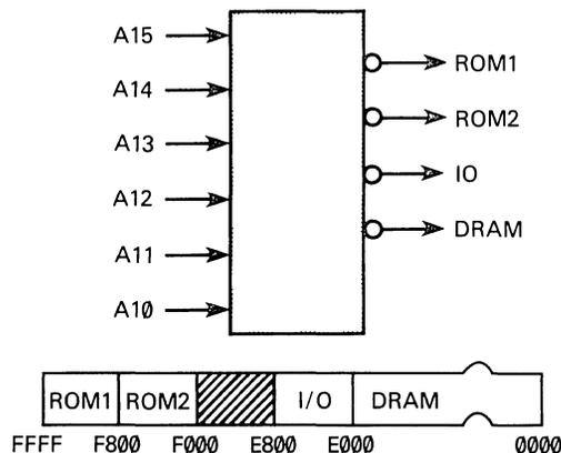
**Figure 6.3.2** Block Diagram: 6809 Memory Address Decoder
