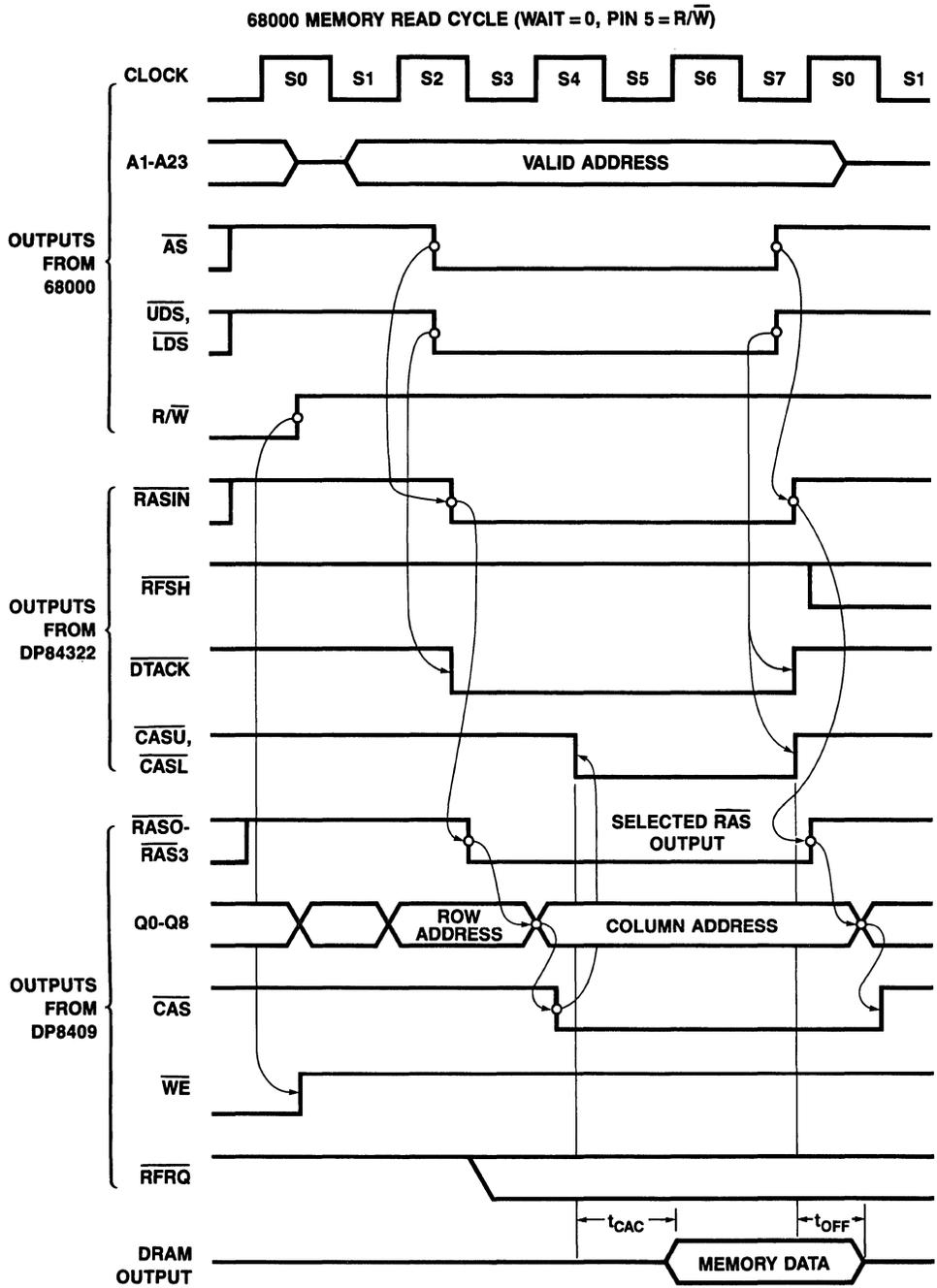
Figure 8.12.4 Timing Diagram; 68000 Memory Read Cycle
