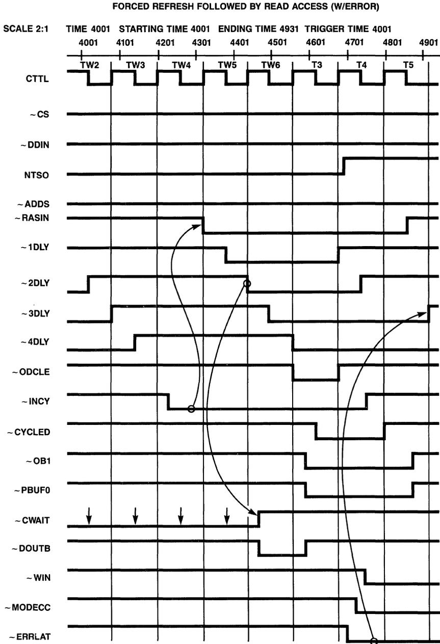
**Figure 8.14.13** Simulation Timing Diagram; Forced Refresh Followed by Read Access (With Error)
