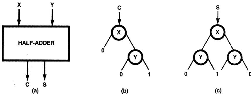
**Figure A.2.4** (a) A Half-adder; (b) Binary Decision Diagram for  $C = X \cdot Y$ ; (c) Binary Decision Diagram for  $S = X \oplus Y$
