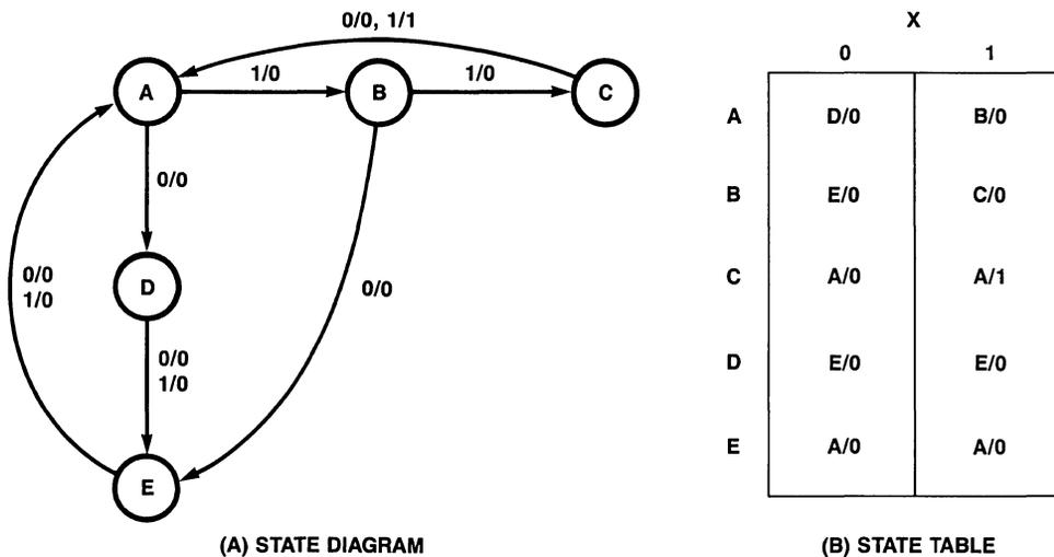
Figure 5.7.11 (A) State Diagram (B) State Table
