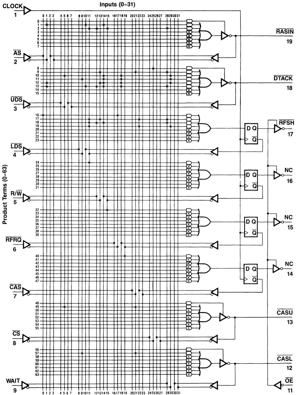
Figure 8.12.12 DP84322 Logic Diagram PAL Device 16R4
