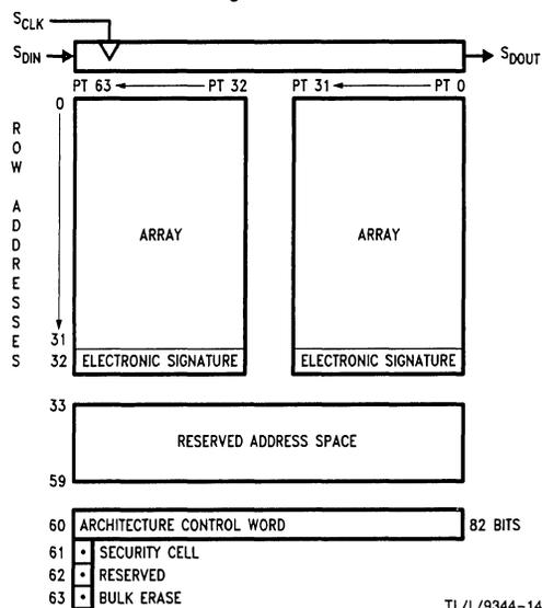
FIGURE 1. GAL16V8 Row Address Map Block Diagram
