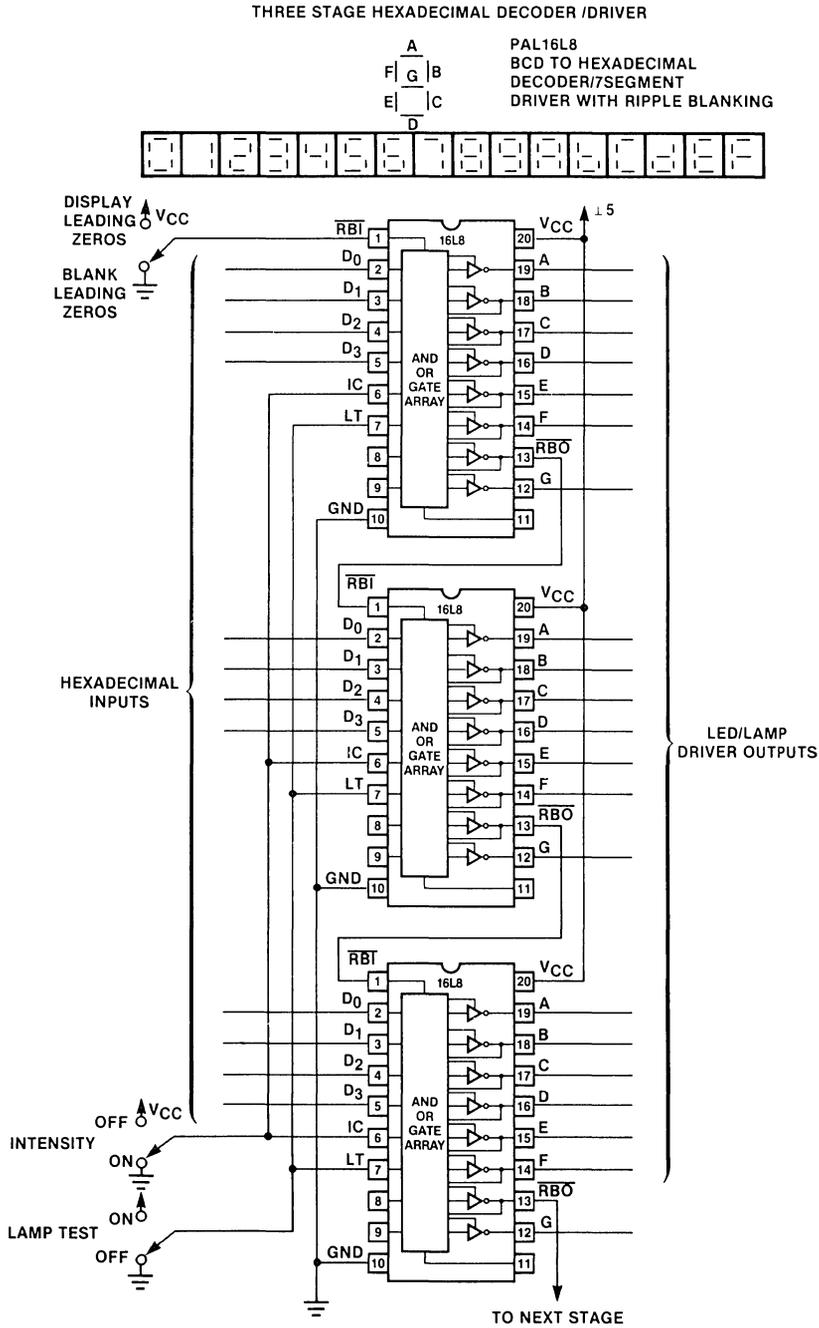
Figure 8.4.1 Hex Display Decoder-Driver, Combinational Logic Diagram
