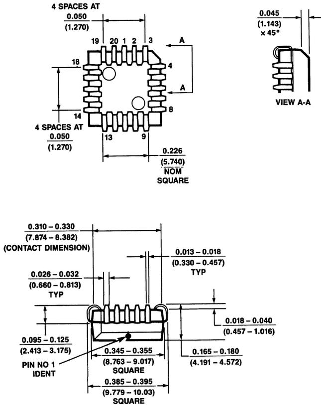
Figure 13.9 NS Package PCC-20 20-Lead Plastic Leaded Chip Carrier (V)
