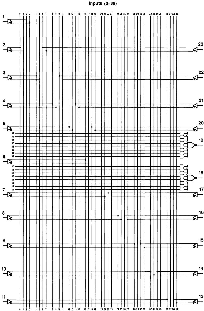
Figure 4.4.18 Logic Diagram PAL20L2
