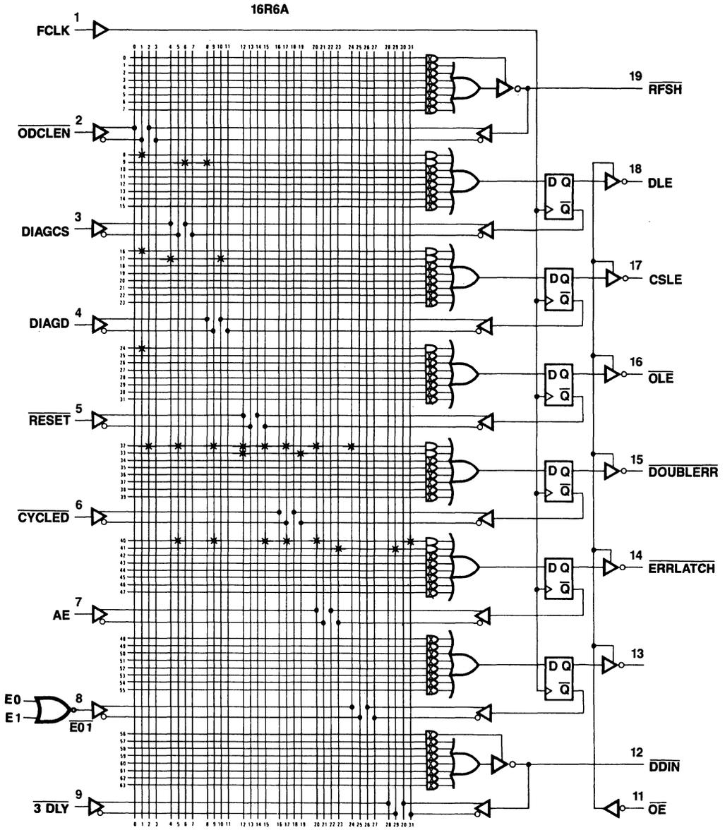
Figure 8.14.17 Logic Diagram of PAL Device #4
