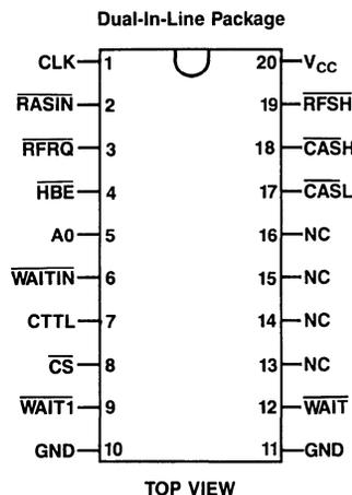
Figure 8.11.1 Connection Diagram
