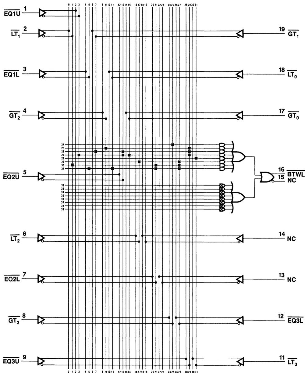
Figure 8.5.2 Logic Diagram PAL16C1
