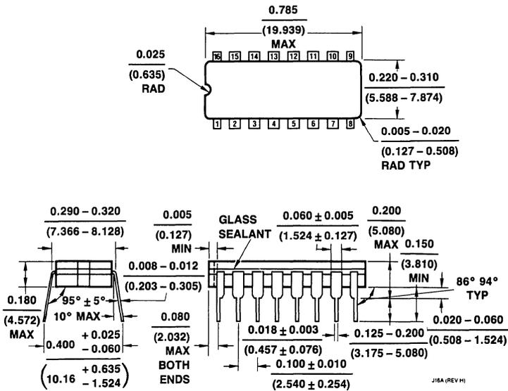
**Figure 13.1** NS Package J16A 16-Lead Cavity DIP (J)
