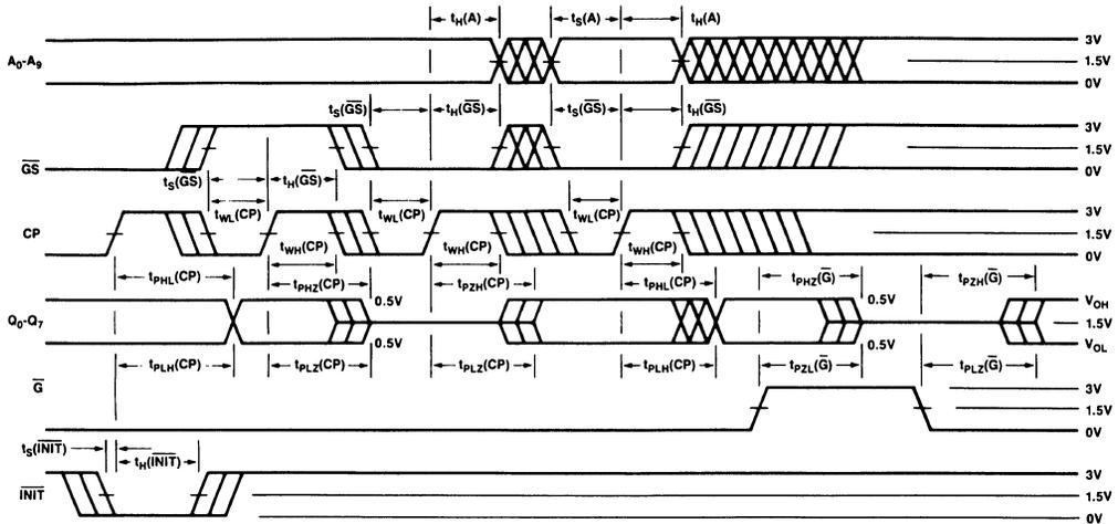
Figure 11.4.3 Switching Waveforms, Registered PROM
