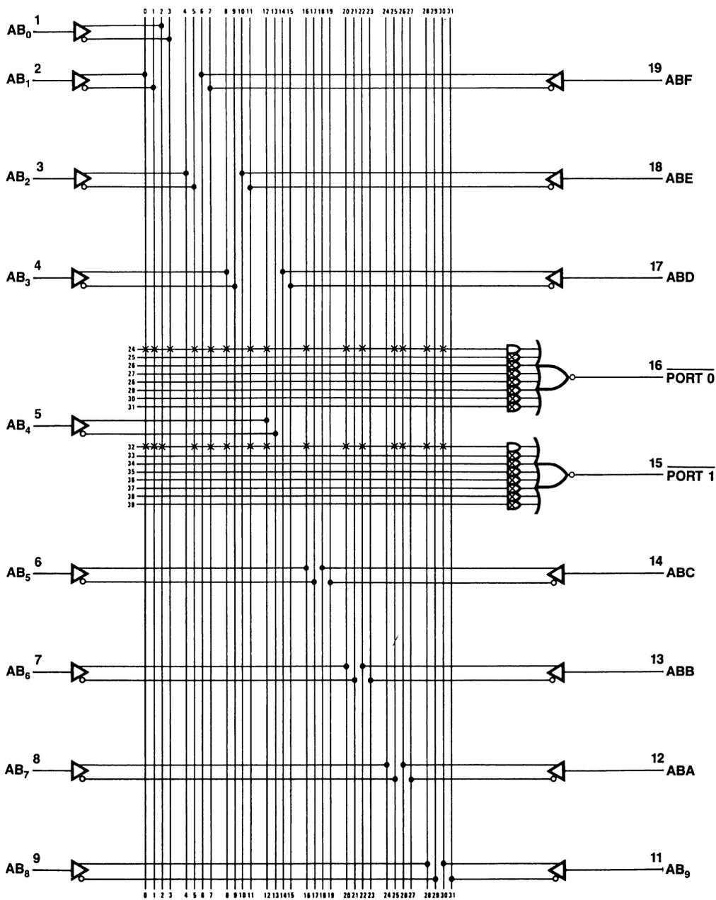
Figure 8.3.2 Logic Diagram PAL16L2
