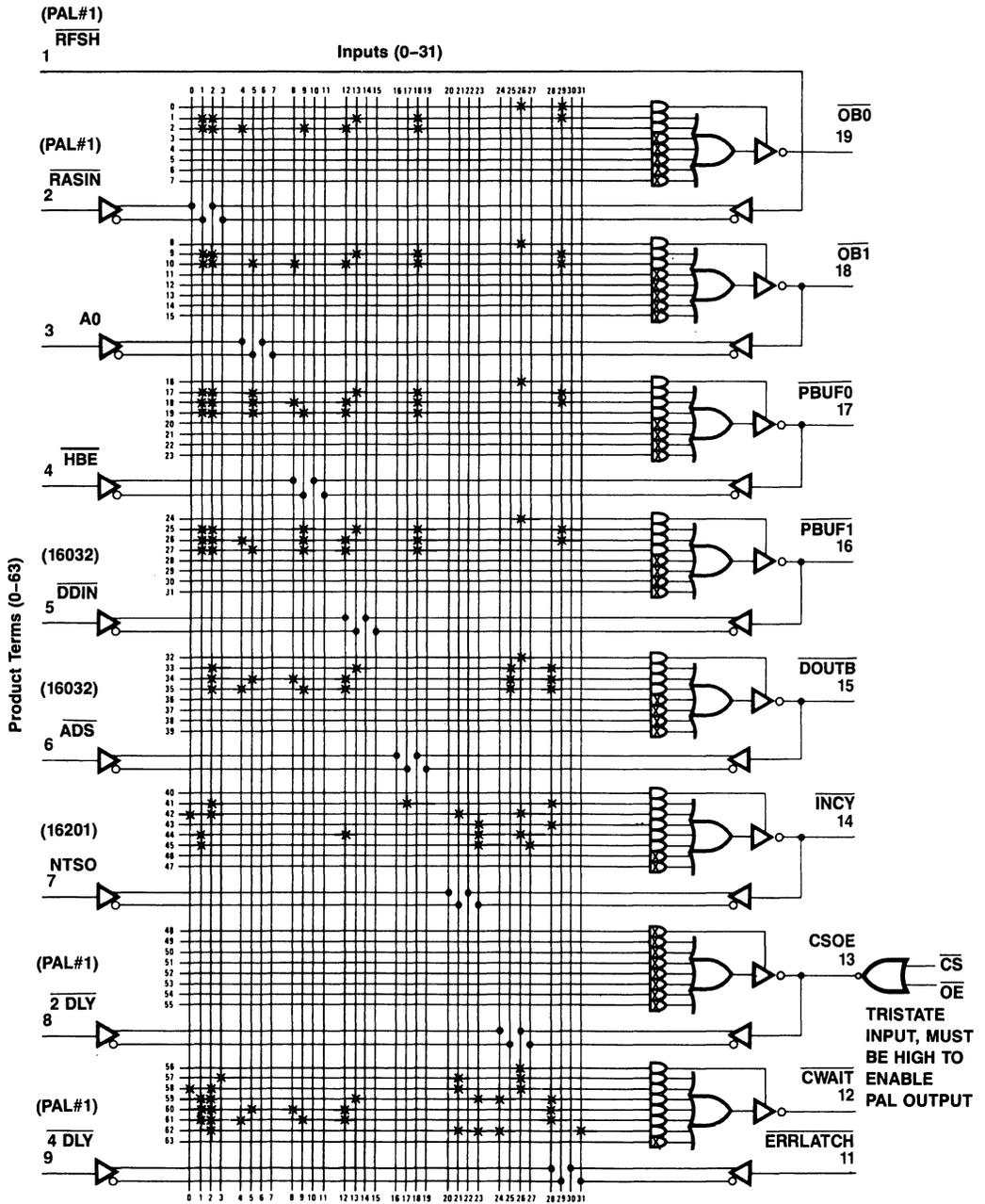
Figure 8.14.15 Logic Diagram of PAL Device #2
