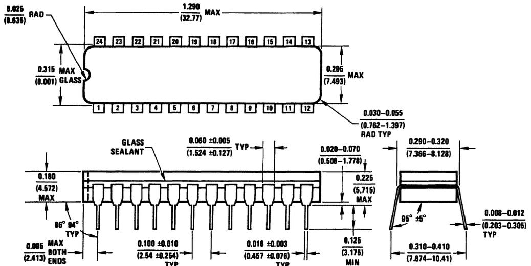
24-Pin Narrow Ceramic Dual-In-Line Package (J)
