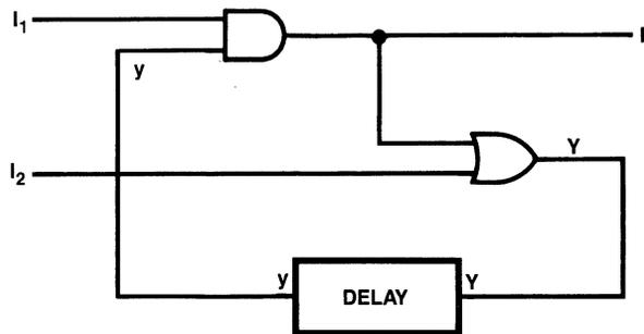
**Figure 3.6.1** A Typical Sequential Circuit
