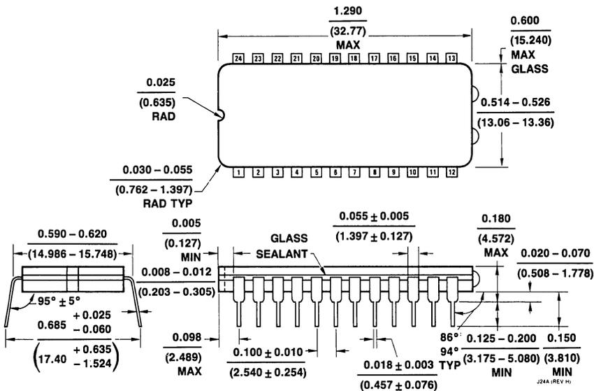
Figure 13.7 NS Package J24A 24-Lead Cavity DIP (J)
