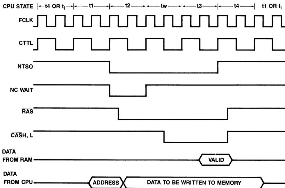
Figure 8.11.4 Timing Diagram; Read, or Write Memory Cycle With One Wait
