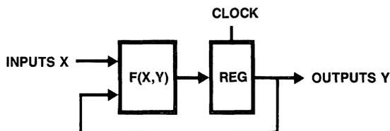
Figure 7.5.2 Sequential Circuit
