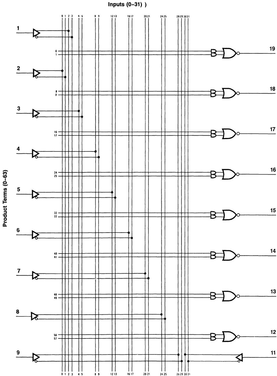
Figure 4.4.6 Logic Diagram PAL10L8
