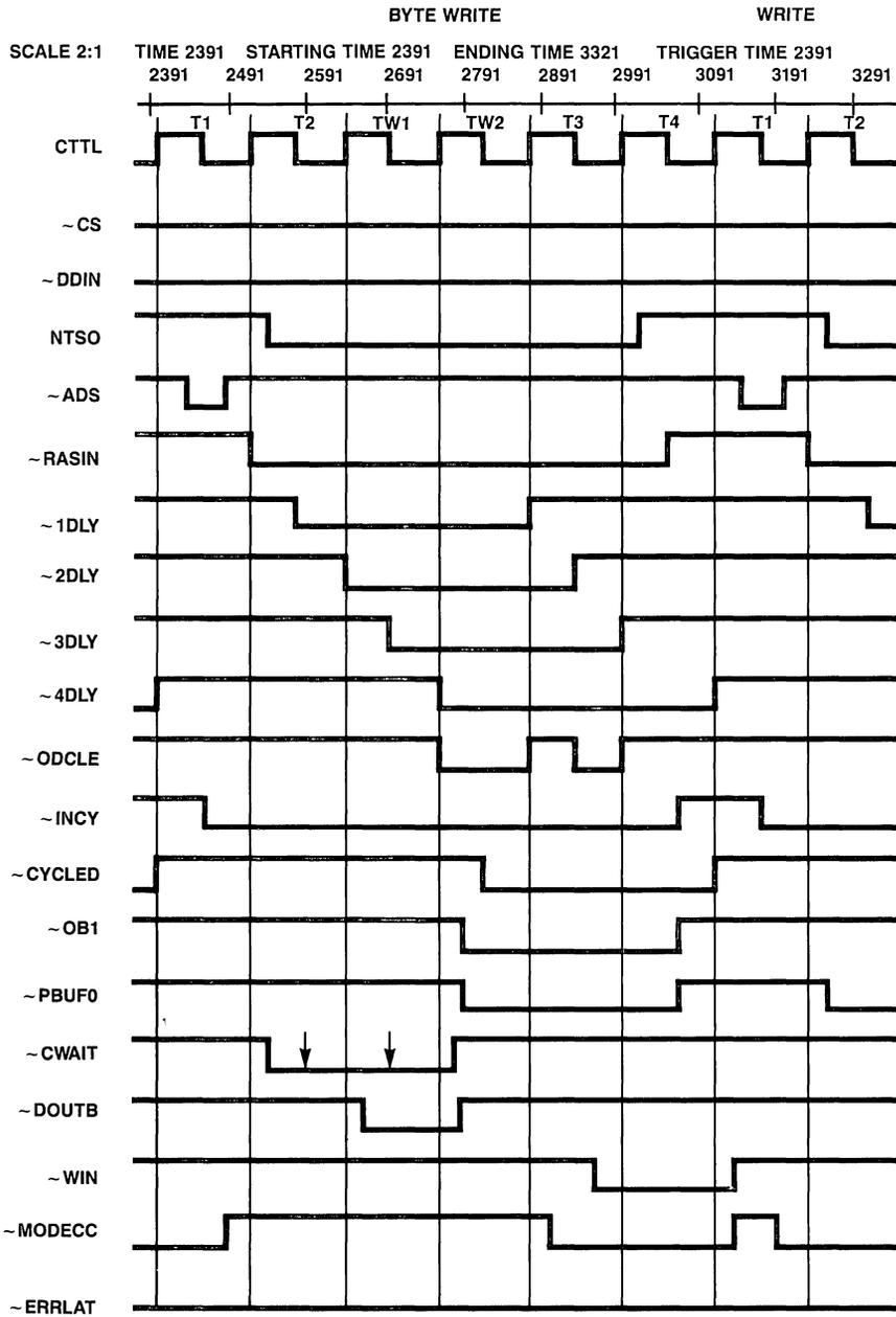
Figure 8.14.10 Simulation Timing Diagram; Byte Write
