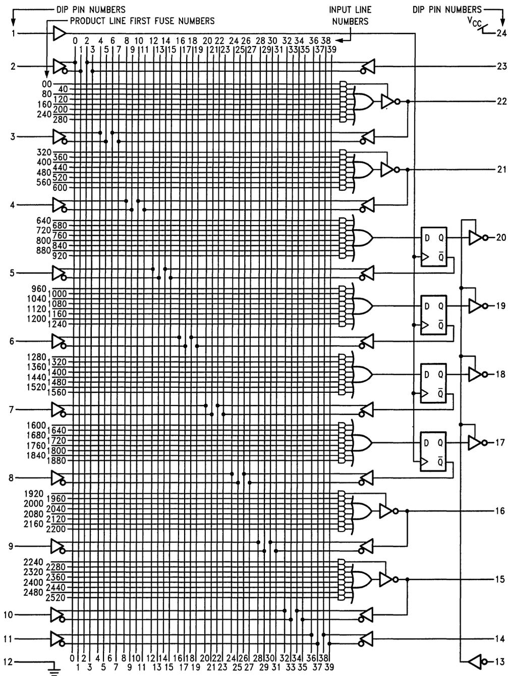
JEDEC Logic Array Fuse Number = Product Line First Fuse Number + Input Line Number
