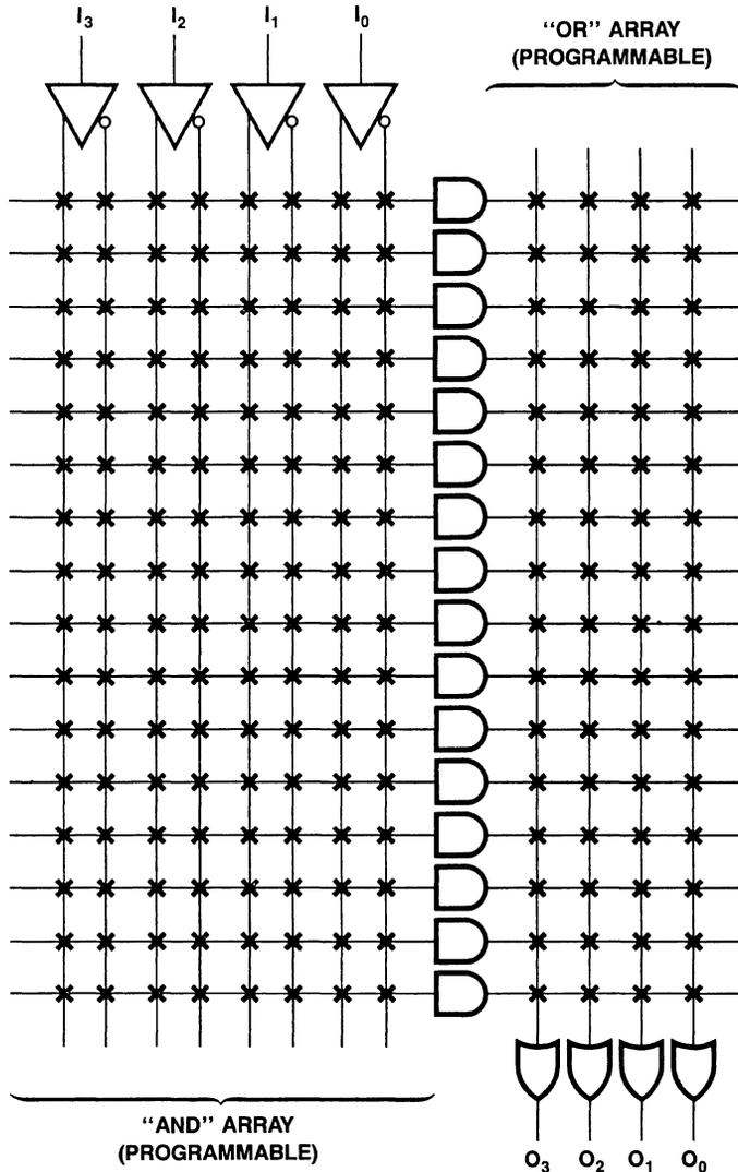
Figure 2.3.4 FPLA with 4 Inputs, 4 Outputs, and 16 Products
