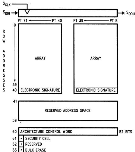
FIGURE 1. GAL20V8 Row Address Map Block Diagram
