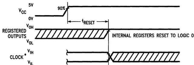
\*The clock input should not be switched from low to high until after time  $t_{RESET}$ .
