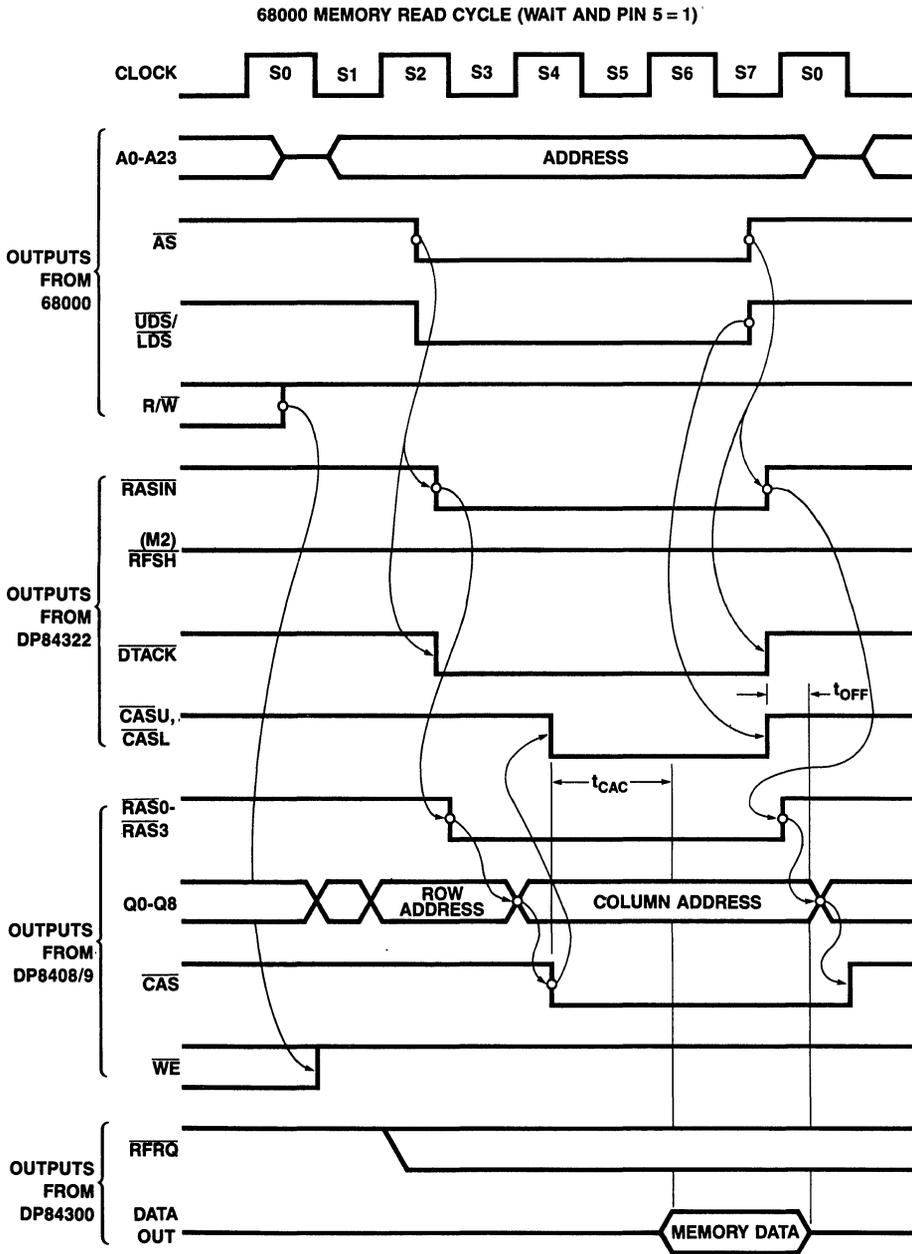
Figure 8.12.10 Timing Diagram; 68000 Memory Read Cycle
