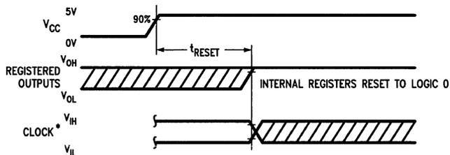
\*The clock input should not be switched from low to high until after time  $t_{RESET}$ .
