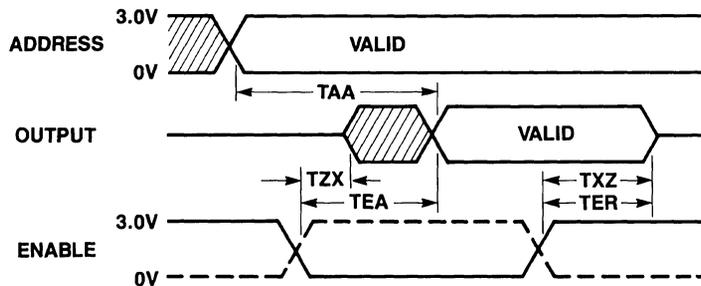
Figure 11.4.2 Switching Time Waveforms Non-Registered PROMs
