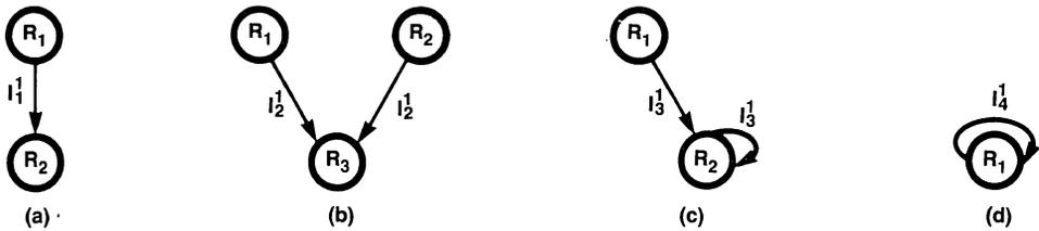
**Figure A.2.3** Representations of Microprocessor Instruction —  $I_1$ , (a) Transfer Instruction,  $R_2 \leftarrow R_1$ ; (b) Add Instruction,  $R_3 \leftarrow R_1 + R_2$ ; (c)  $I_3$ , OR Instruction,  $R_2 \leftarrow R_1 \text{ OR } R_2$ ; (d)  $I_4$  Rotate Left Instruction.
