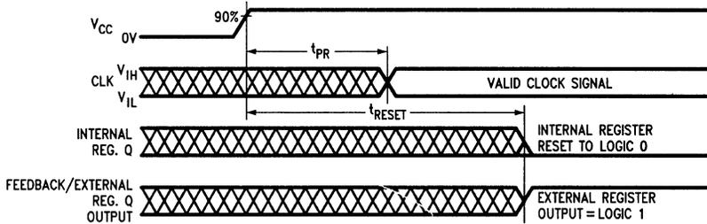
FIGURE 5. Power-Up Reset Waveforms
