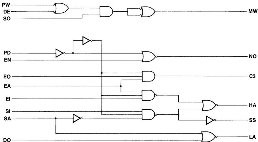
Figure 8.10.1 Control Logic for 8086 CPU Board
