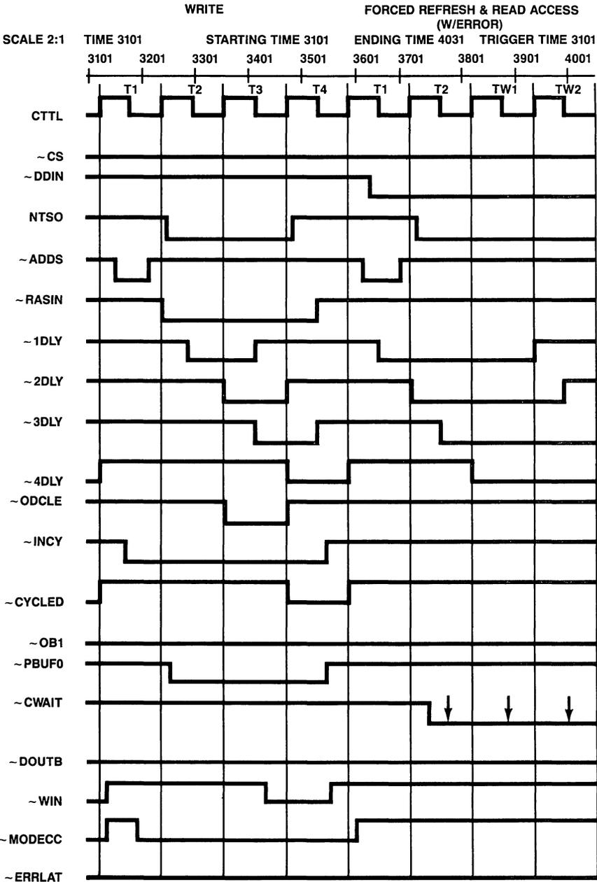
Figure 8.14.12 Simulation Timing Diagram; Write, Forced Refresh and Read Access
