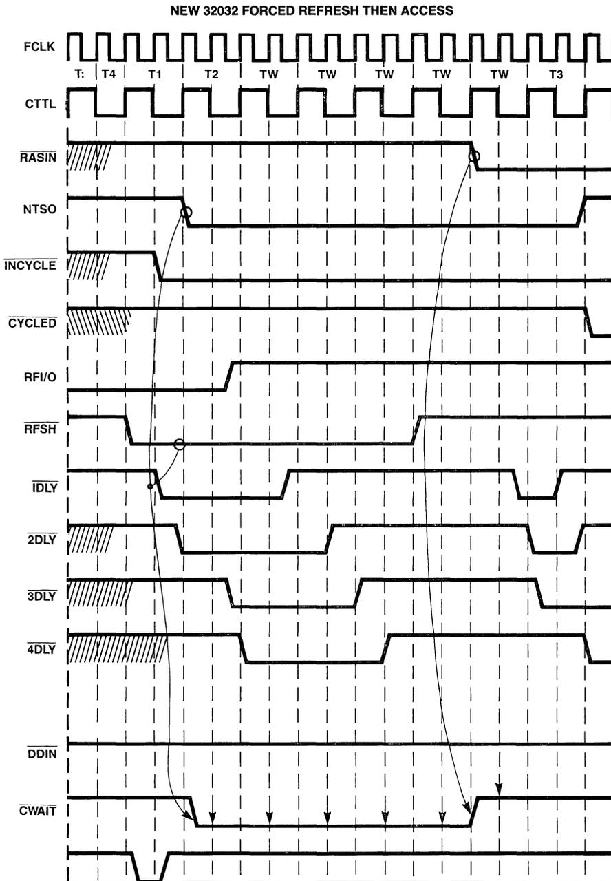
Figure 8.14.6 Timing Diagram; Forced Refresh Then Access
