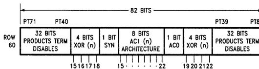
FIGURE 2. GAL20V8 Architecture Control Word Diagram
