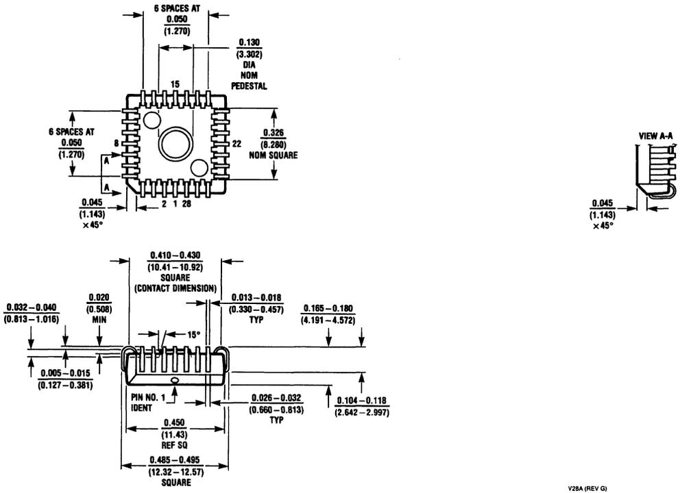
28-Lead Plastic Chip Carrier (V)
