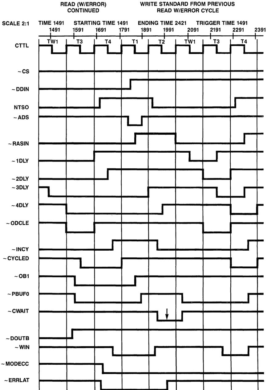
Figure 8.14.9 Simulation Timing Diagram; Read With Error and Write Cycle
