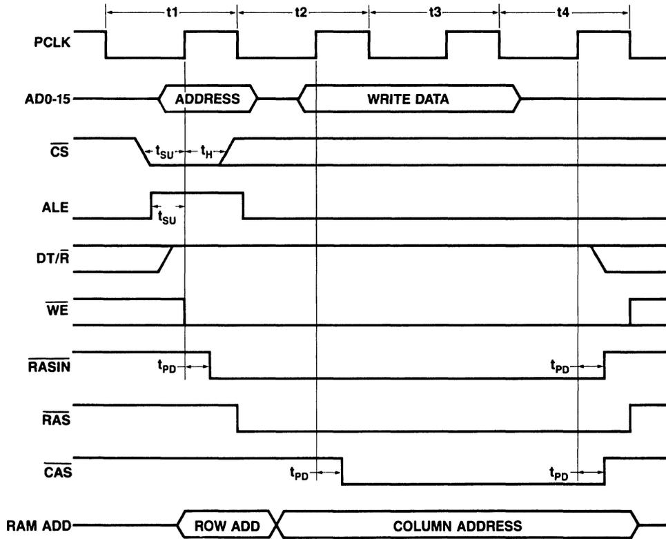
Figure 8.13.7 Timing Diagram; Write Timing
