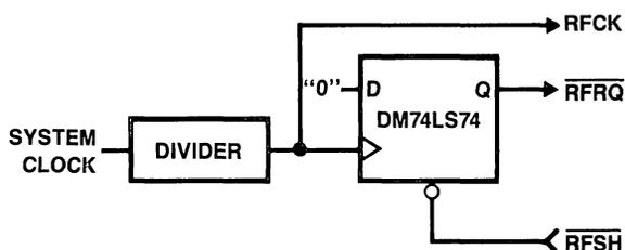
**Figure 8.13.4** Using a Flip-Flop and a Counter for Refresh Request Logic
