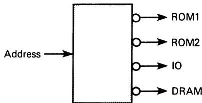
**Figure 6.3.3** Simplified Block Diagram: 6809 Memory Address Decoder
