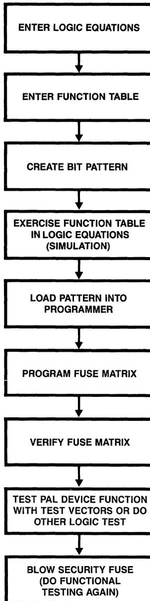
Figure 7.5.5 PAL Device Programming Procedures
