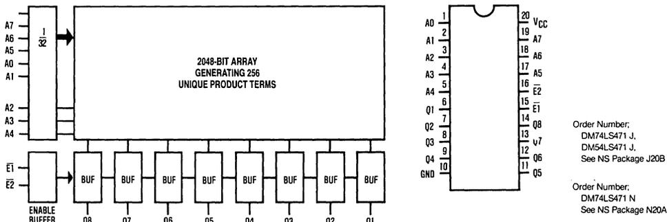
**Figure 11.7.1** Block and Connection Diagram
