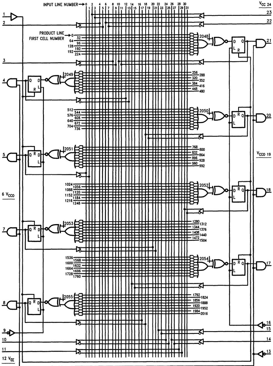
JEDEC logic array cell number = product line first cell number + input line number.
