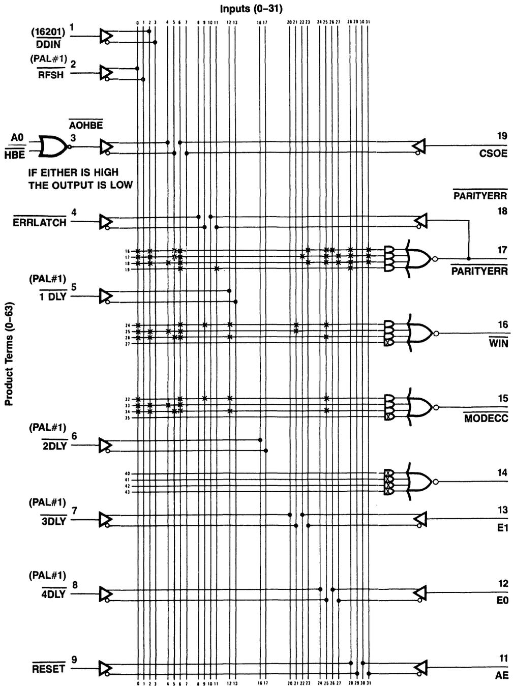
Figure 8.14.16 Logic Diagram of PAL Device #3
