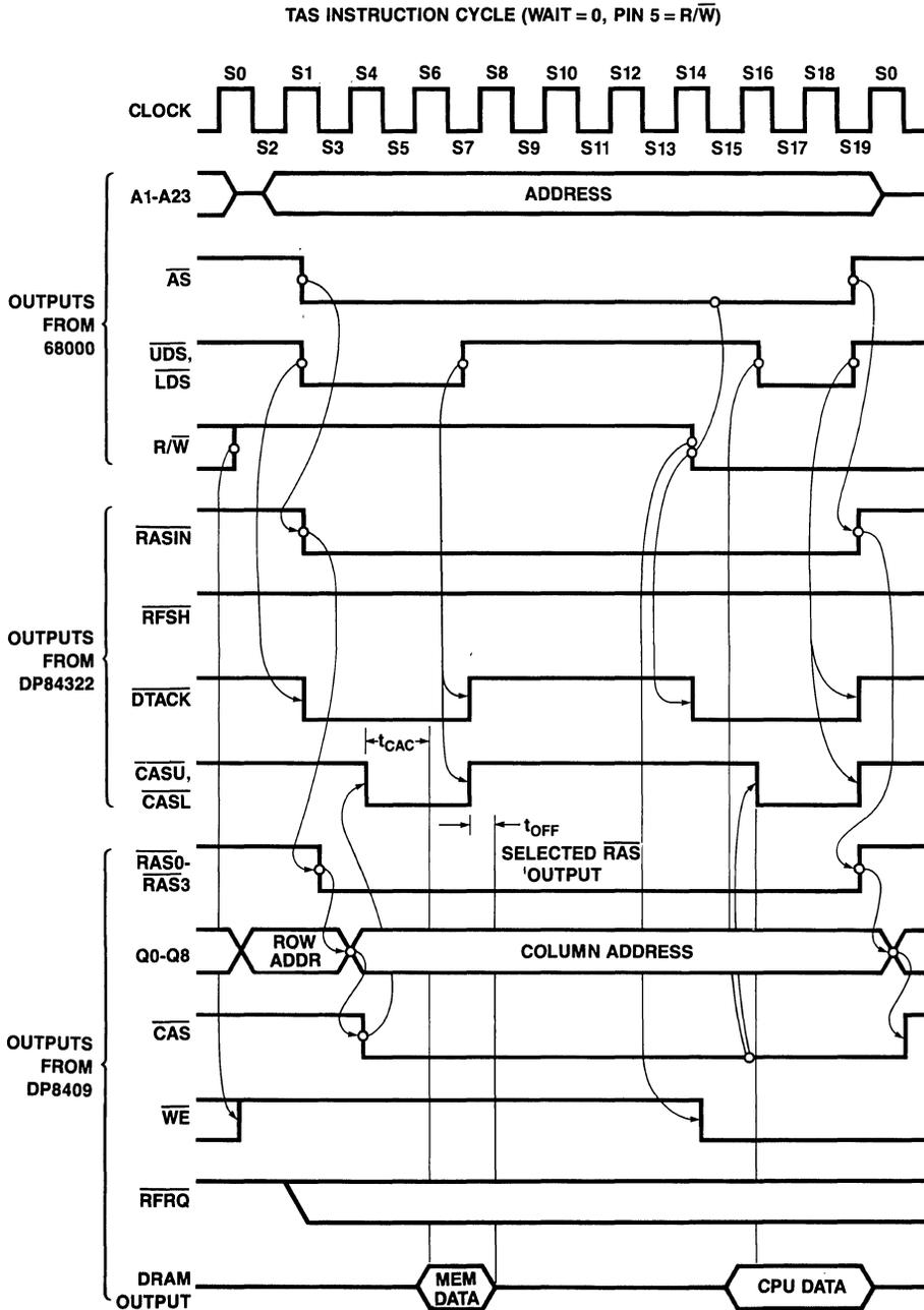
Figure 8.12.6 Timing Diagram; TAS Instruction Cycle
