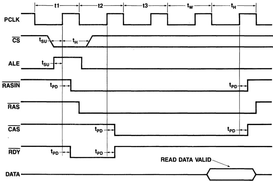
Figure 8.13.8 Timing Diagram; Memory Cycle With 1 Wait State
