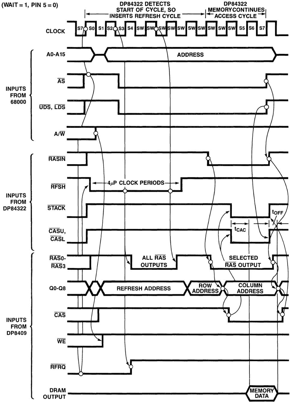
Figure 8.12.8 Timing Diagram; Memory Read Cycle and Forced Refresh
