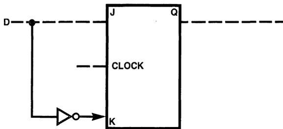
**Figure 3.5.2** Implement D Flip-Flop by Using J-K
