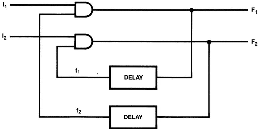
**Figure 3.6.5** Example of Circuit with Unpredictable Output States
