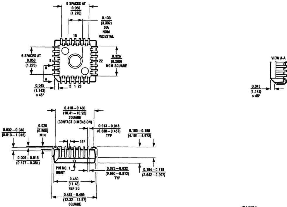
28-Lead Plastic Chip Carrier Package (V)
