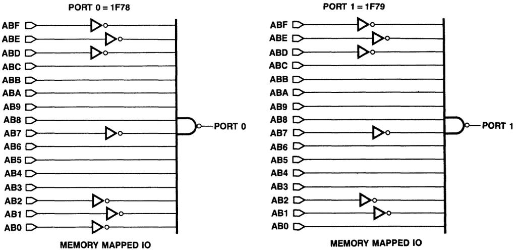
Figure 8.3.1 Memory Mapped I/O Logic Diagram
