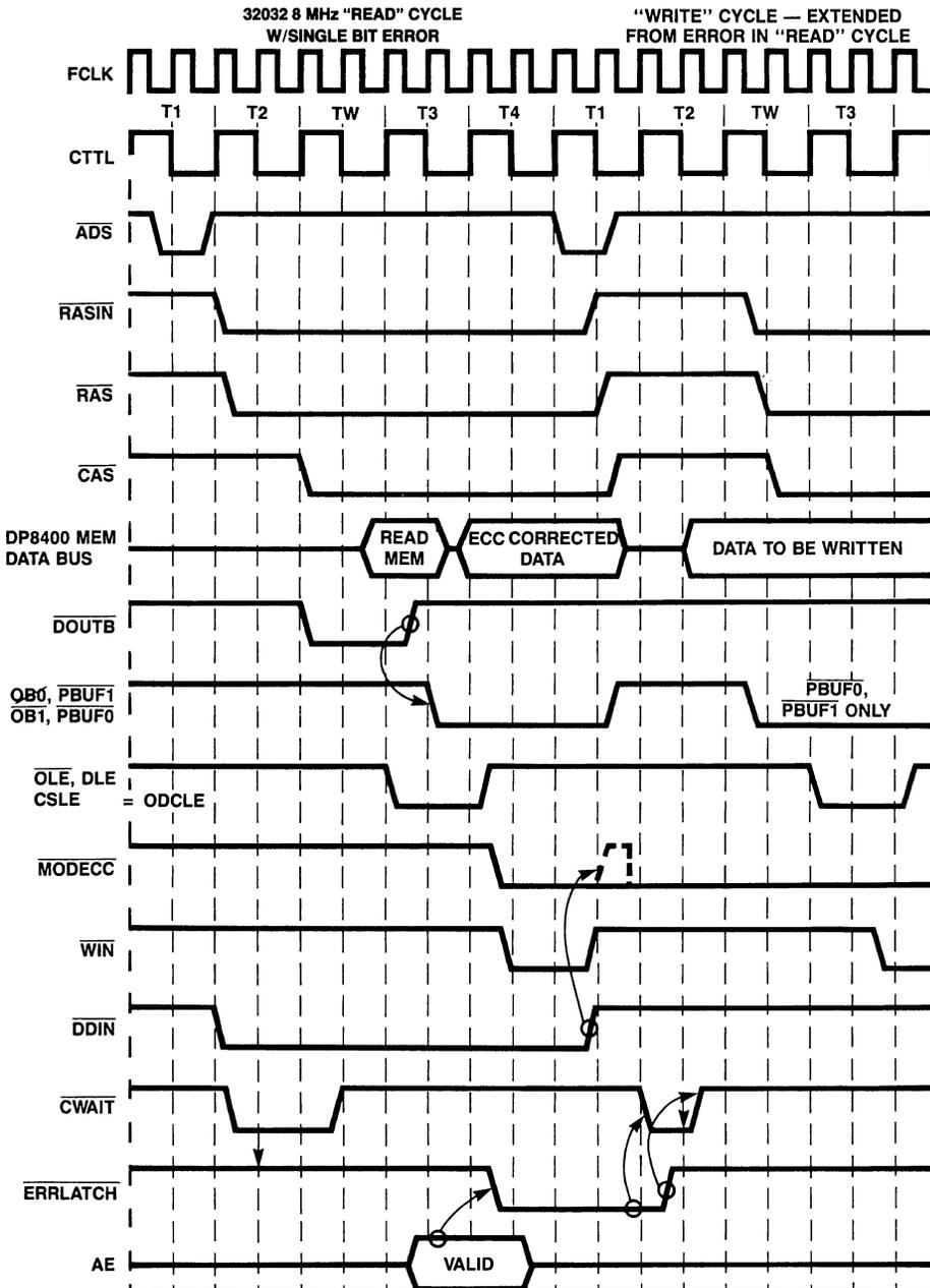
Figure 8.14.4 Timing Diagram; Read Cycle With Simple Bit Error
