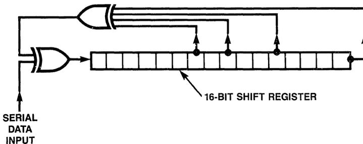
**Figure A.3.5** The 16-bit Linear Feedback Shift Register Used in Signature Analysis
