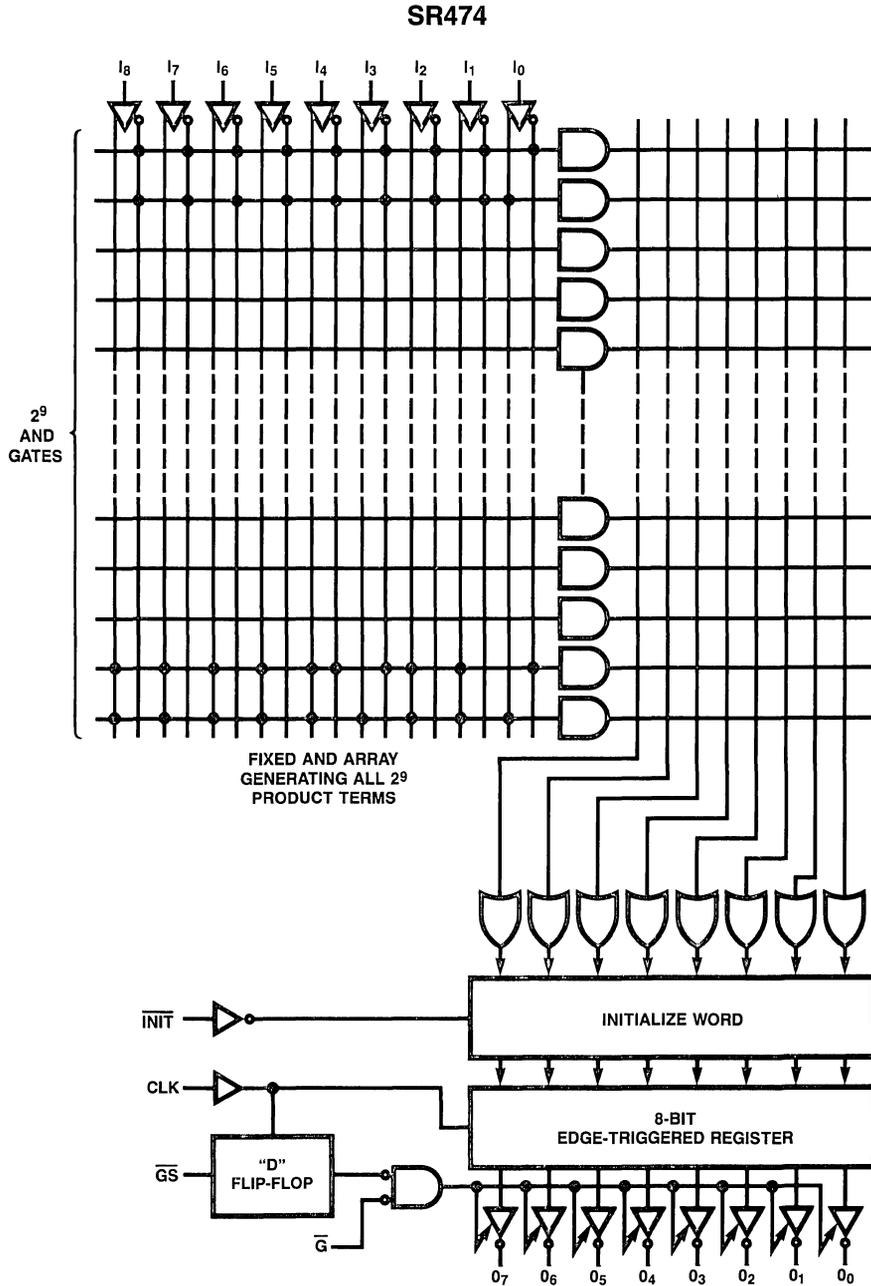
Figure 4.4.32 512 × 8 Registered PROM Logic Diagram
