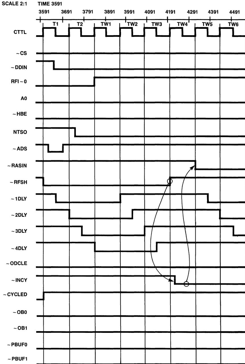
Figure 8.14.11 Simulation Timing Diagram; Forced Refresh Then Access
