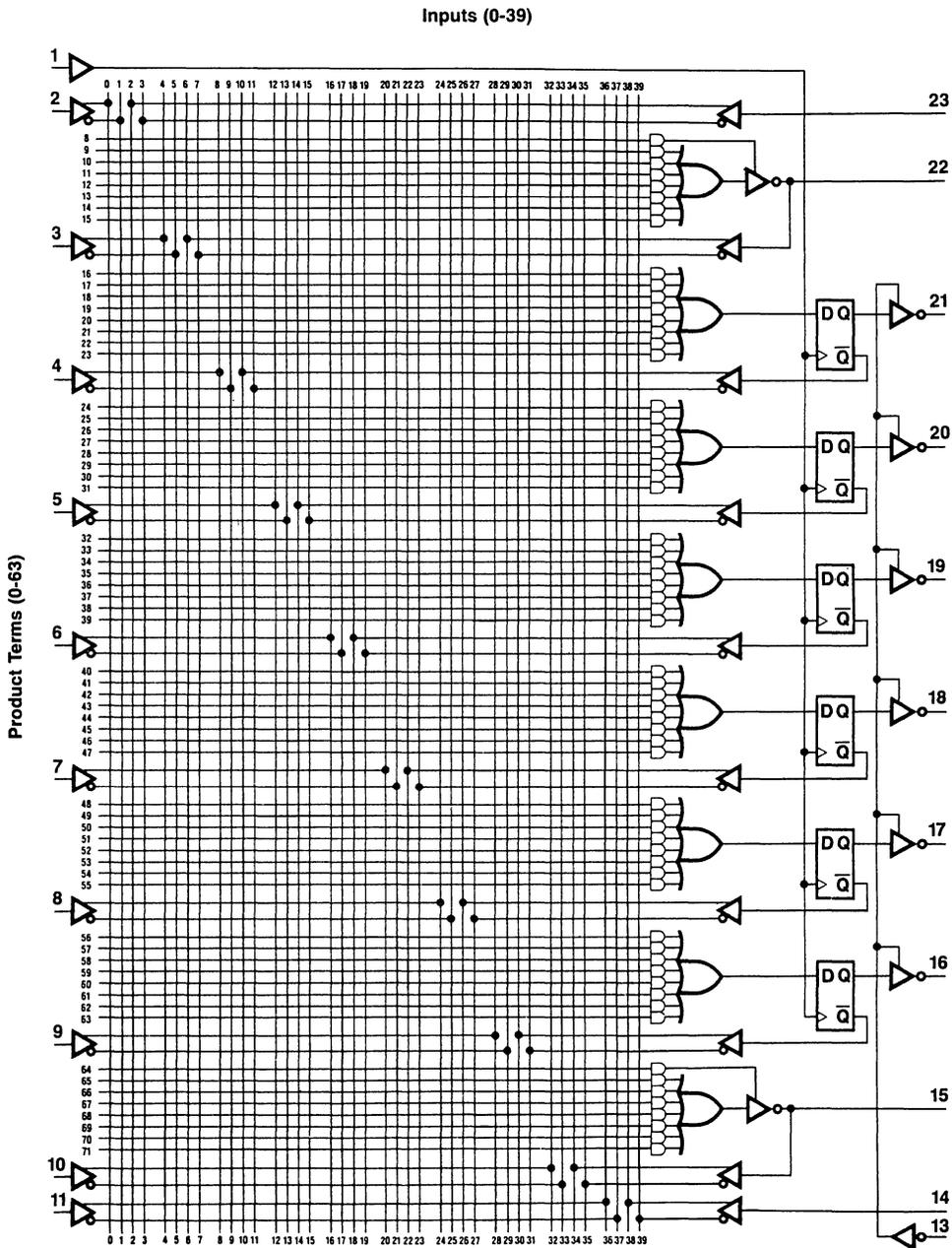
Figure 4.4.26 Logic Diagram PAL20R6
