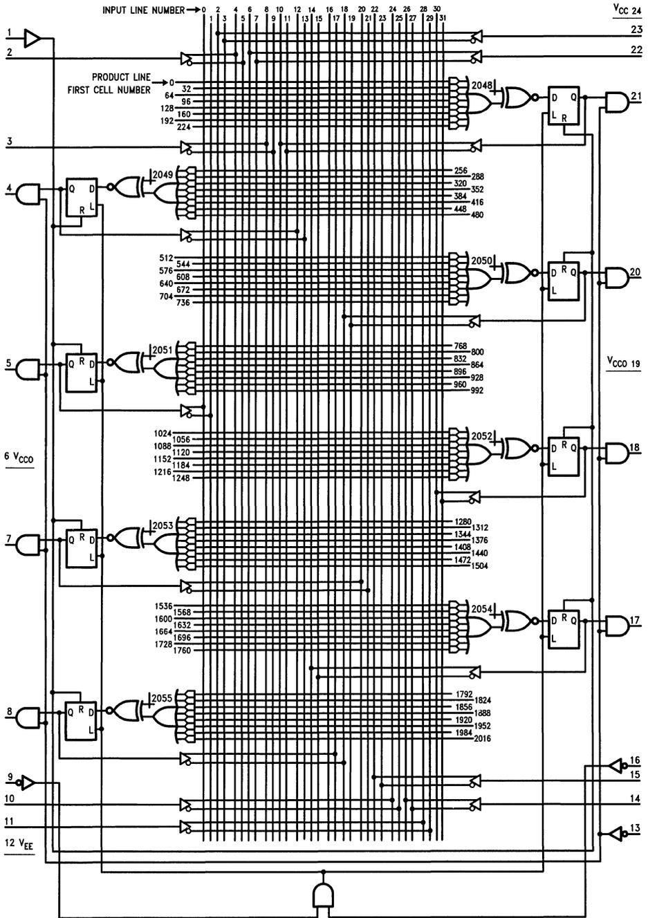
JEDEC logic array cell number = product line first cell number + input line number.
