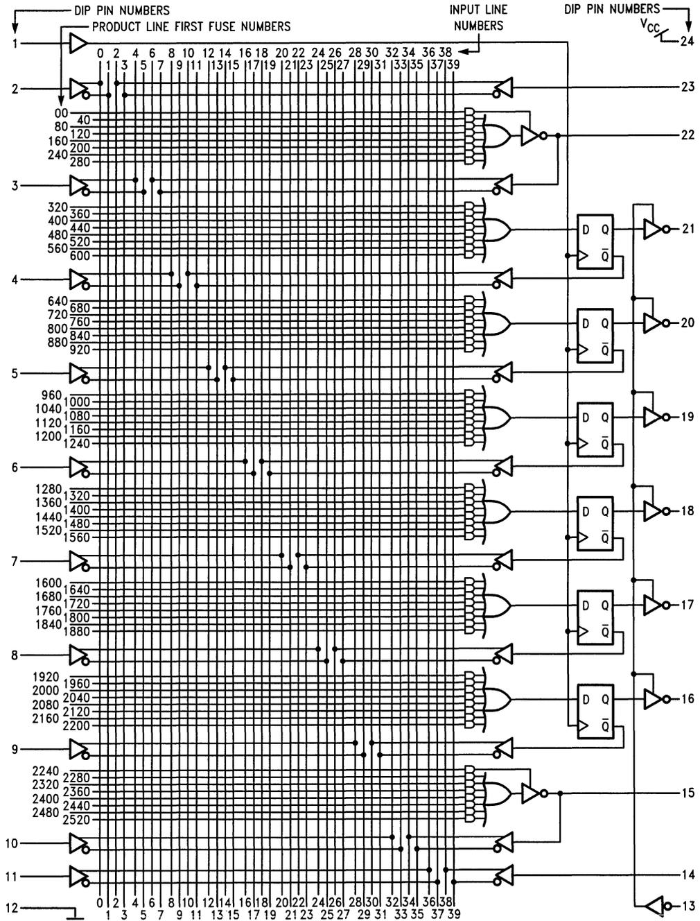
JEDEC Logic Array Fuse Number = Product Line First Fuse Number + Input Line Number
