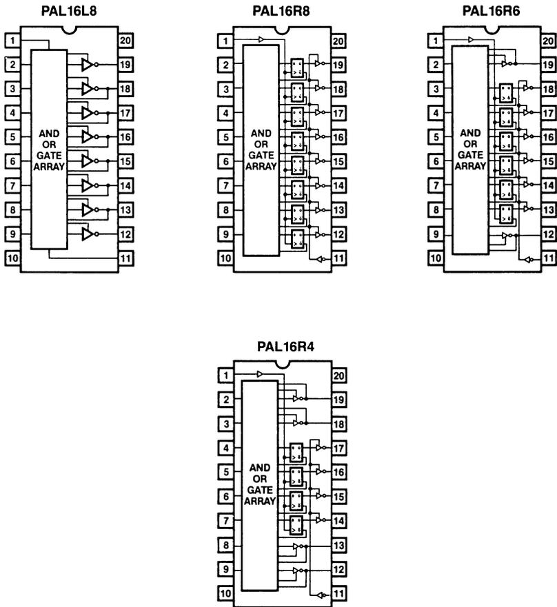
Figure 4.2.4 PAL Device Logic Symbols — Series 20 (Contd.)
