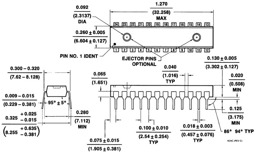
Figure 13.6 NS Package N24C 24-Lead Molded DIP (N)
