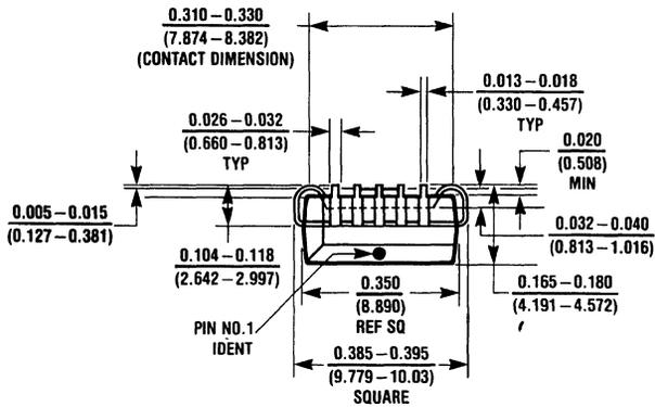
**Ceramic Dual-In-Line Package (V)**
