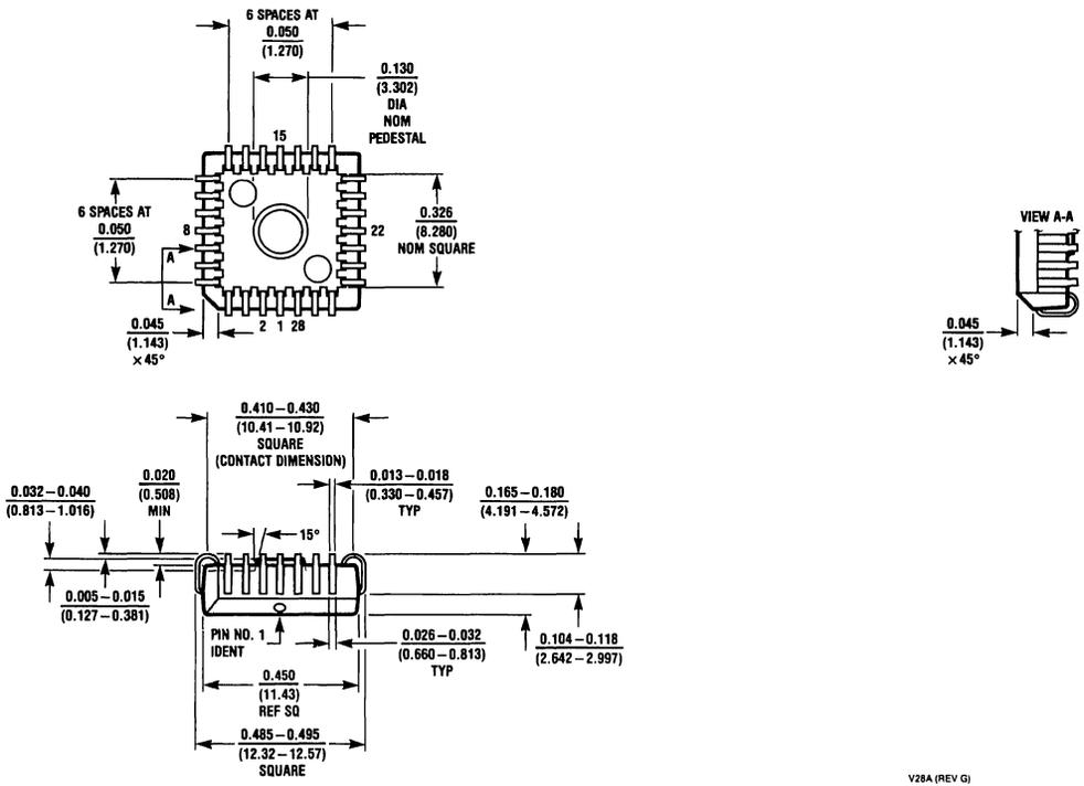
28-Lead Plastic Chip Carrier (V)
