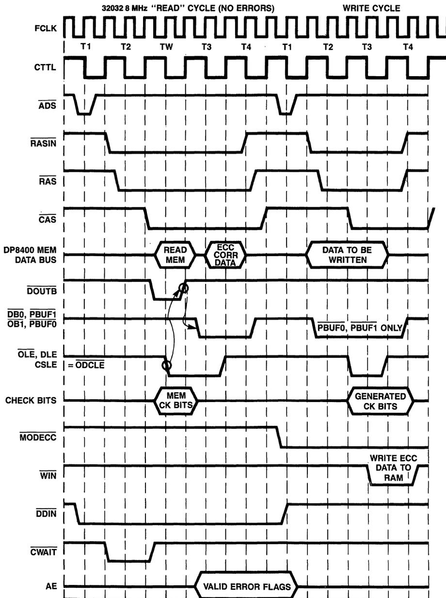
Figure 8.14.3 Timing Diagram; Read Cycle and Write Cycle
