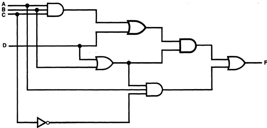
Figure 3.3.1 A Random Logic Circuit
