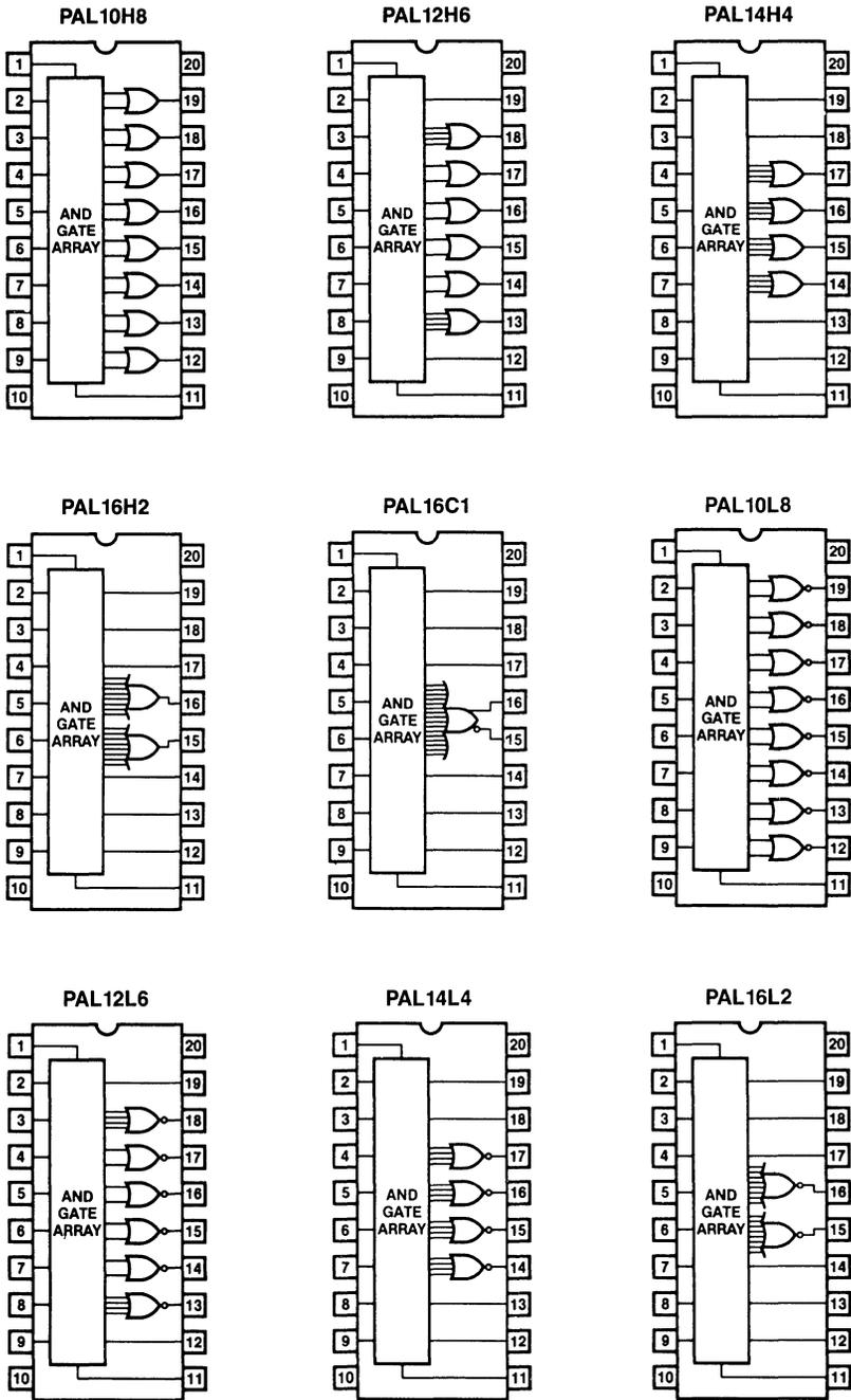
Figure 4.2.4 PAL Device Logic Symbols — Series 20
