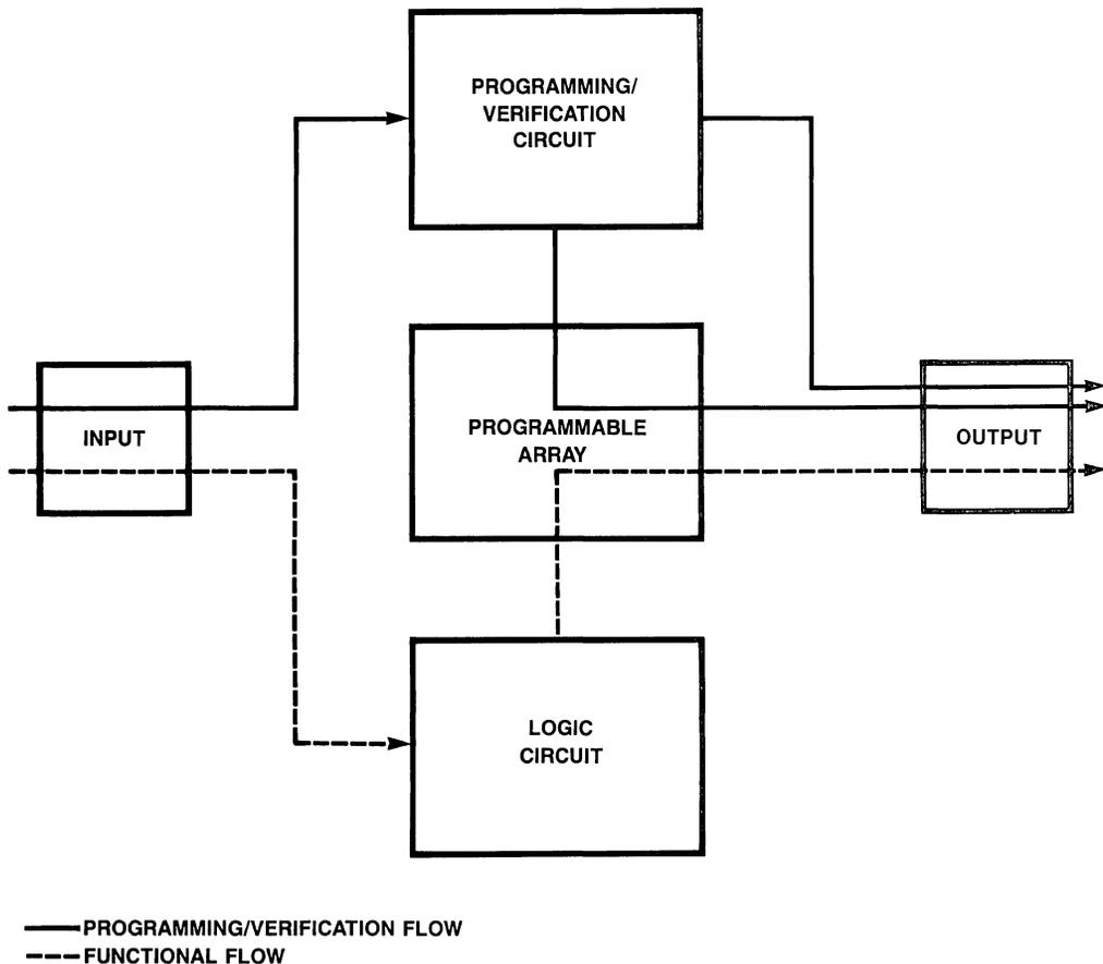
Figure 7.2.1 PAL Device's Architecture
