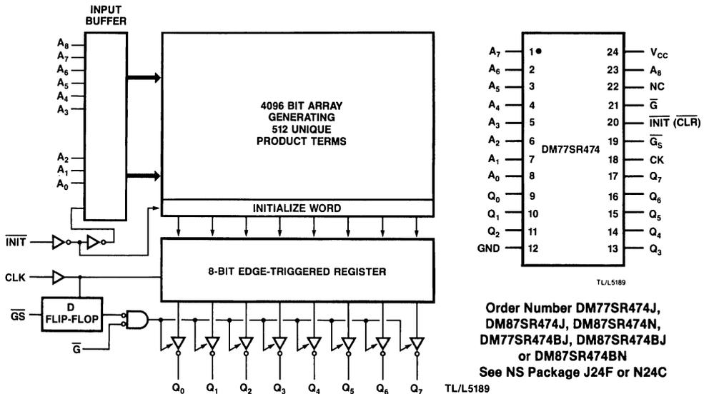
Figure 11.10.1 Block and Connection Diagrams
