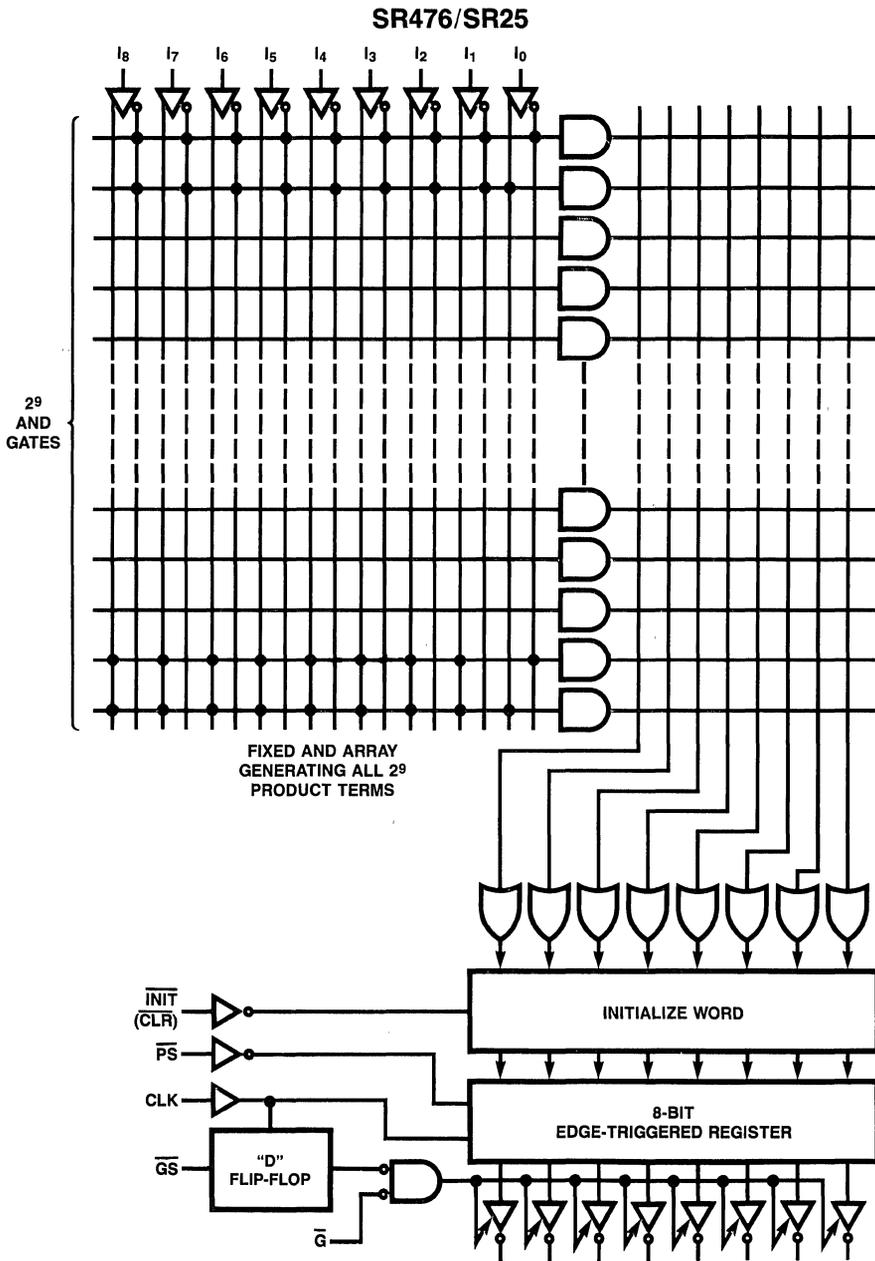
**Figure 4.4.31** 512 × 8 Registered PROM Logic Diagram
