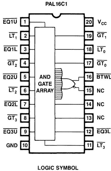
Figure 8.5.1 PAL Device 16C1 Limit Checker
