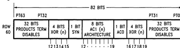
FIGURE 2. GAL16V8 Architecture Control Word Diagram
