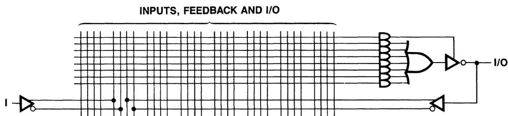
Figure 4.2.2 PAL Device Bidirectional Circuit, Logic Diagram
