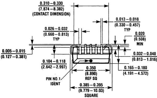
20-Lead Plastic Chip Carrier Package (V)
