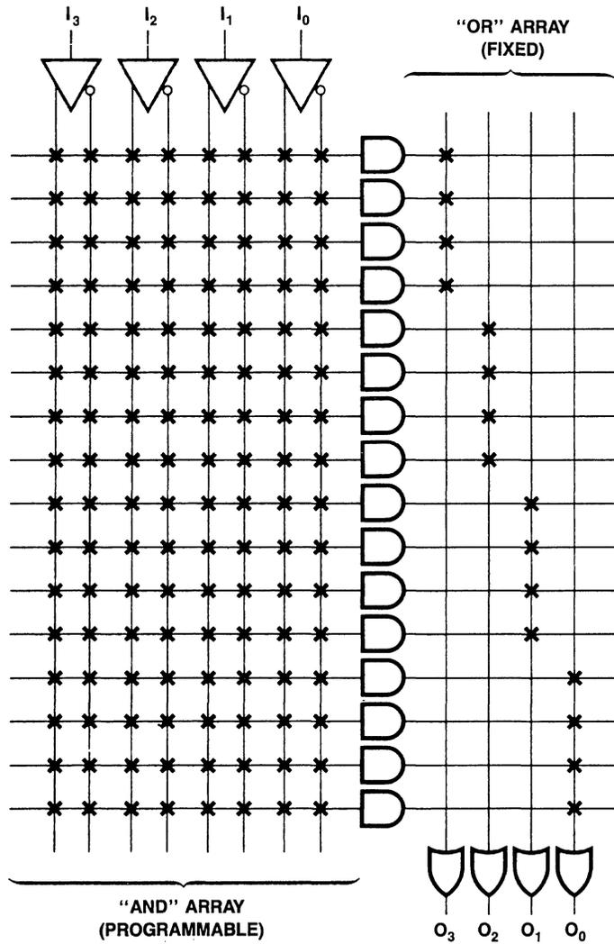
Figure 2.3.5 PAL Device Having 4 Inputs, 4 Outputs, and 16 Products
