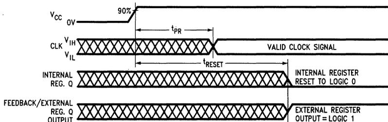
FIGURE 5. Power-Up Reset Waveforms
