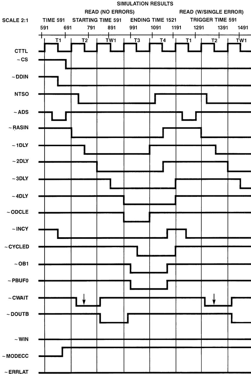
Figure 8.14.8 Simulation Timing Diagram; Read/Write Without Errors
