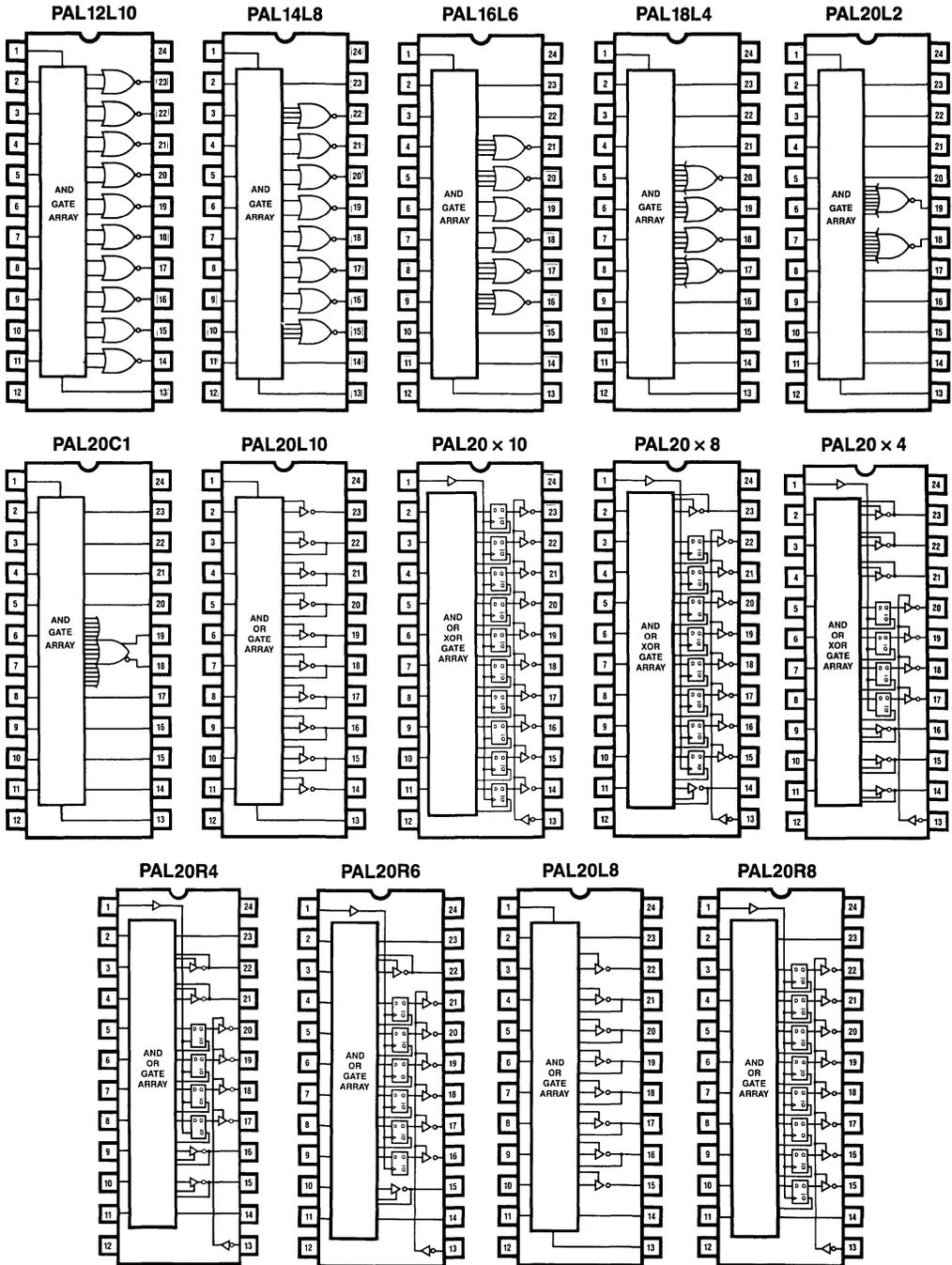
Figure 4.2.5 PAL Device Logic Symbols — Series 24
