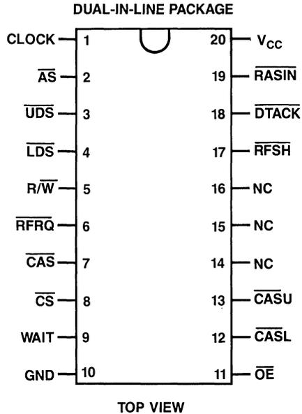
**Figure 8.12.1** Connection Diagram
