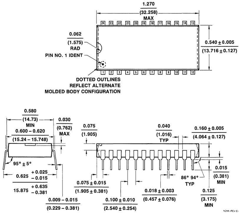
Figure 13.8 NS Package N24A 24-Lead Molded DIP (N)
