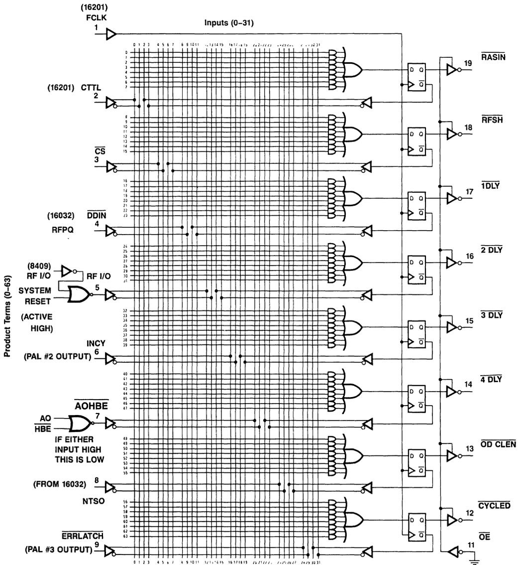
Figure 8.14.14 Logic Diagram of PAL Device #1
