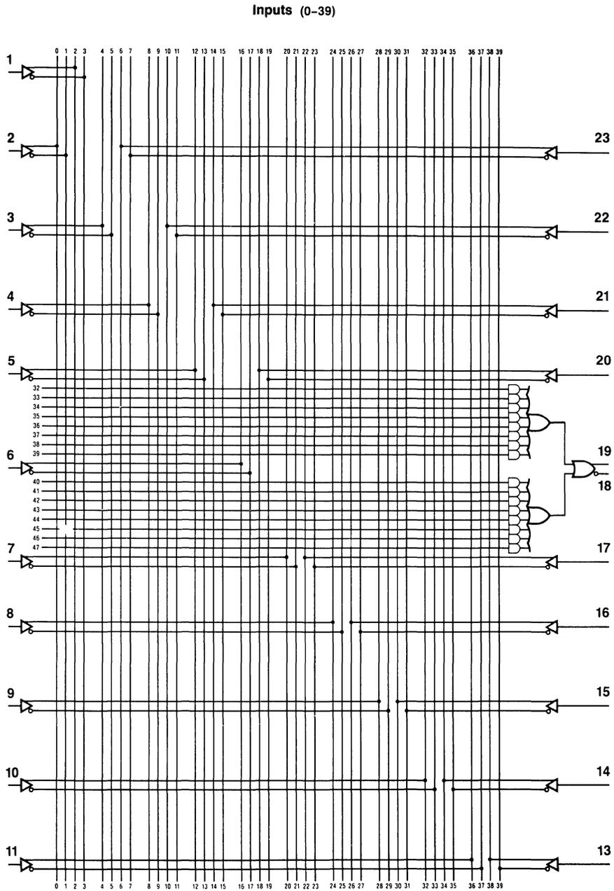
Figure 4.4.19 Logic Diagram PAL20C1
