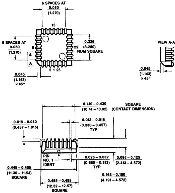
Figure 13.10 NS Package PCC-28 28-Lead Plastic Leaded Chip Carrier (V)
