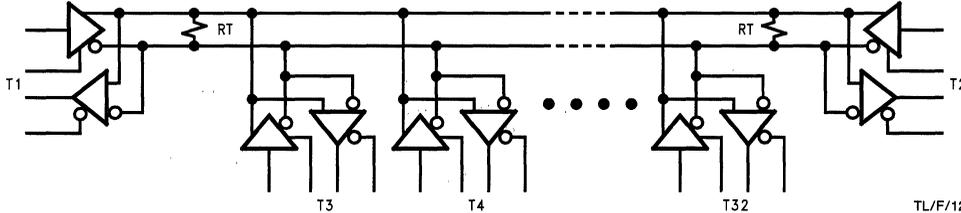
FIGURE 18. Typical RS-485 Bus Interface
