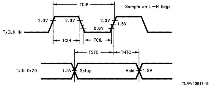
FIGURE 7. DS90CR563 (Transmitter) Setup/Hold and High/Low Times
