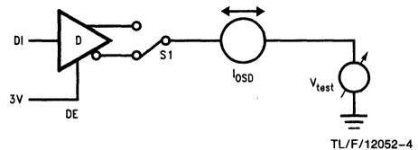
V<sub>test</sub> = -7V to +12V
