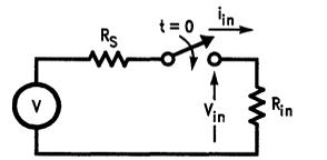
FIGURE 1b. Thevenin Equivalent for Initial Wave
