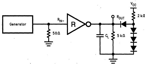
FIGURE 4. Receiver Propagation Delay Test Circuit (Note 6)
