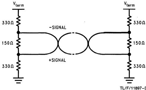
**FIGURE 3. The SCSI Differential Termination**
