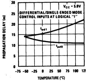
Propagation Delay from Input to Output (Channel 2)
