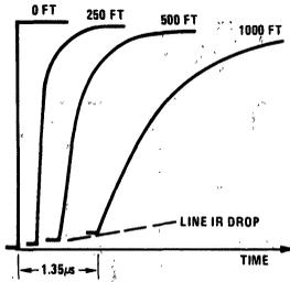
**FIGURE 5. Signal Response at Receiver** TL/F/8826-5
