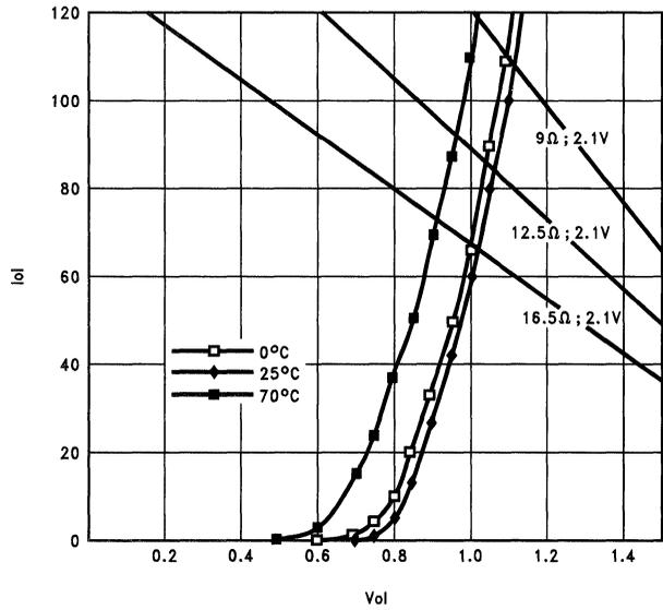
FIGURE 4. IO<sub>L</sub> vs VO<sub>L</sub> and Load Line
