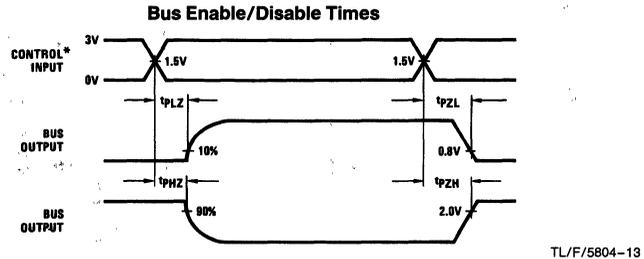
\*Input signal:  $f = 1.0 \text{ MHz}$ , 50% duty cycle,  $t_r = t_f \leq 5 \text{ ns}$
