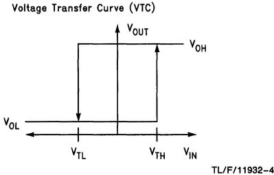
FIGURE 3. Threshold Voltages
