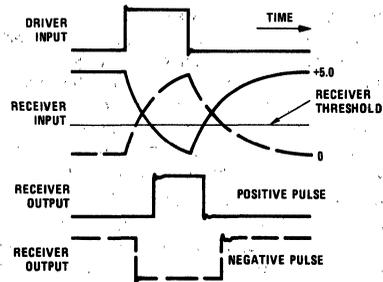
**FIGURE 8. Slicing Level Distortion** TL/F/8826-8
