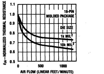
FIGURE 9. Thermal Resistance vs Air Flow
