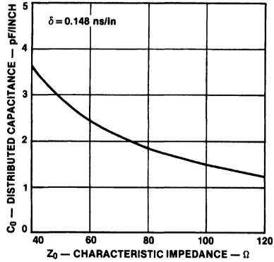
**FIGURE 2-3. Microstrip Distributed Capacitance Versus Impedance, G-10 Epoxy**
