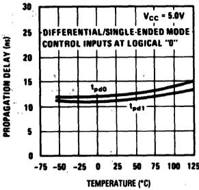
Propagation Delay from Input to Output (Channel 1)
