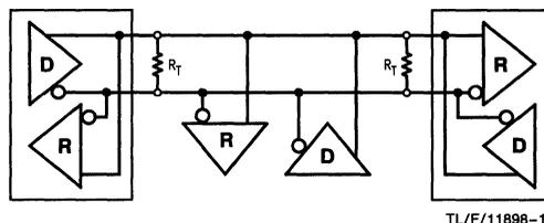
**FIGURE 11. Bi-Directional Termination Configuration**
