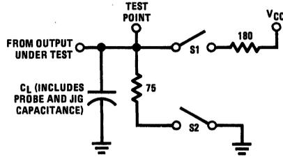
Note: S1 and S2 of load circuit are closed except where shown.
