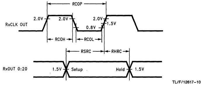
FIGURE 8. DS90CR564 (Receiver) Setup/Hold and High/Low Times
