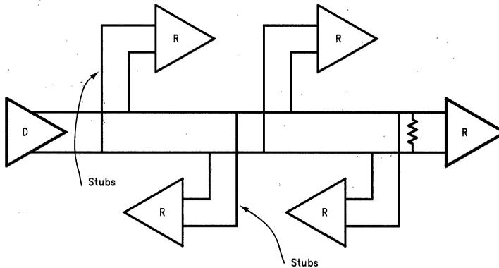
FIGURE 9. Multi-Drop Configuration for LVDS
