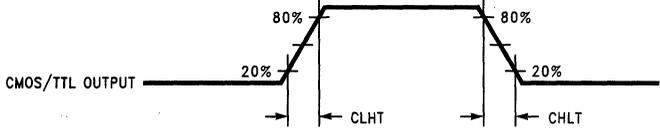
FIGURE 4. DS90CF582 (Receiver) CMOS/TTL Output Load and Transition Timing
