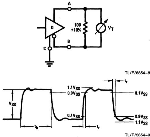
$t_b$  = Time duration of the unit interval at the applicable modulation rate.
