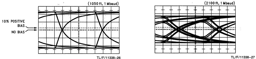
$$\text{ISOCRONOUS DISTORTION (ID)} = \frac{t_{cs}}{t_{ui}} \times 100\%$$
