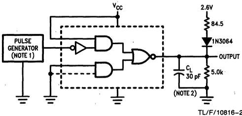
**Note 1:** The pulse generator has the following characteristics:  $Z_{OUT} \approx 50\Omega$ ,  $t_W = 200$  ns, duty cycle = 50%,  $t_r = t_f = 5.0$  ns.
