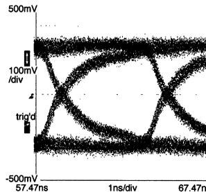
FIGURE 10b. Eye Pattern at Receiver Inputs
