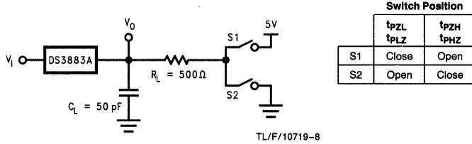
**FIGURE 6. Receiver Enable/Disable Set-Up**
