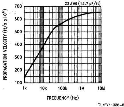
FIGURE 5. Propagation Velocity vs Frequency
