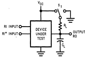
FIGURE 2. Test Circuit for Switching Characteristics
