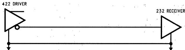
FIGURE 4. RS-422 to RS-232—Direct Connection
