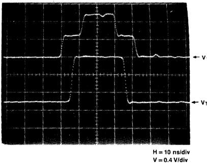
**FIGURE 1-7. Series Terminated Line and Waveforms**
