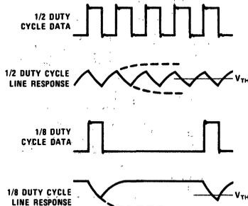
**FIGURE 7. Signal Distortion Due to Duty Cycle** TL/F/8826-7
