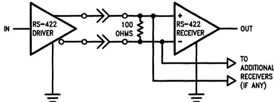
FIGURE 1a. An RS-422 Configuration
