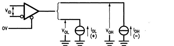
FIGURE 3. Receiver  $V_{OH}$  and  $V_{OL}$
