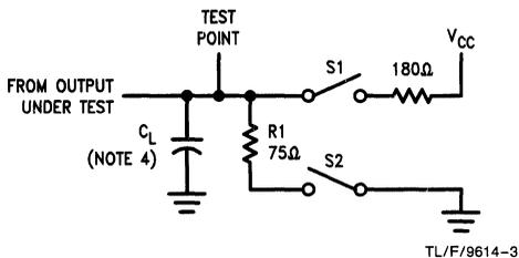
FIGURE 2. AC Load Test Circuit for TRI-STATE Outputs
