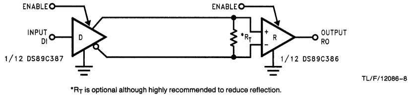
**FIGURE 5. Two-Wire Balanced System, RS-422**
