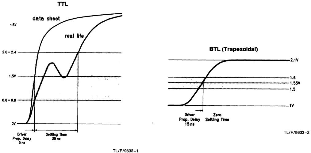
FIGURE 1. Settling Times
