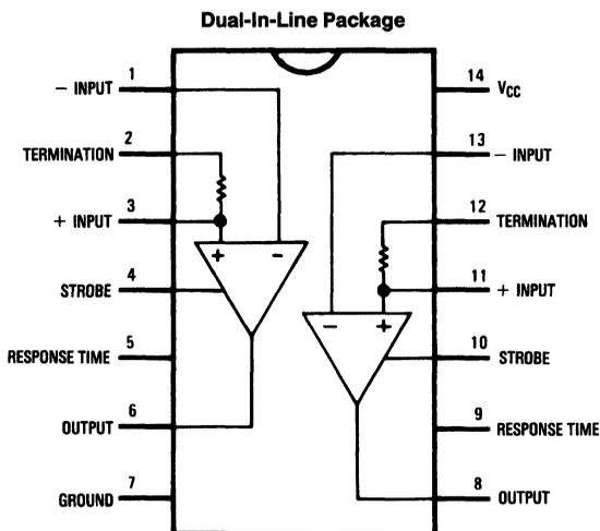
Note: Pin 7 connected to bottom of cavity package.
