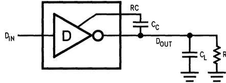
FIGURE 9. External Slew Rate Control Capacitor Connection
