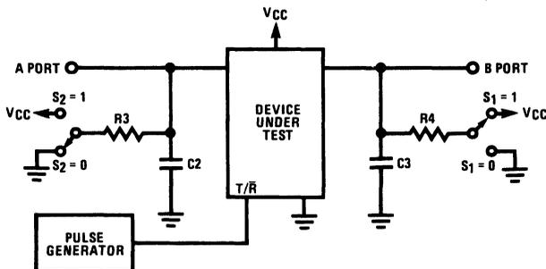
Note: C2 ad C3 include test fixture capacitance.
