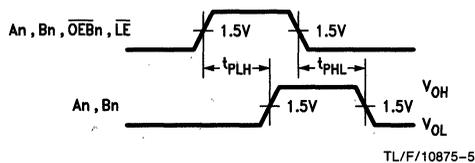
**Waveform 1: Propagation Delay for Data to Output**
