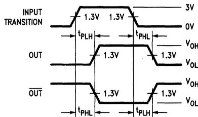
FIGURE 3. Propagation Delay (Notes 1 and 3)
