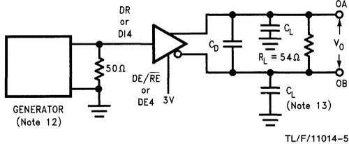
FIGURE 3. Driver Differential Propagation Delay Load Circuit
