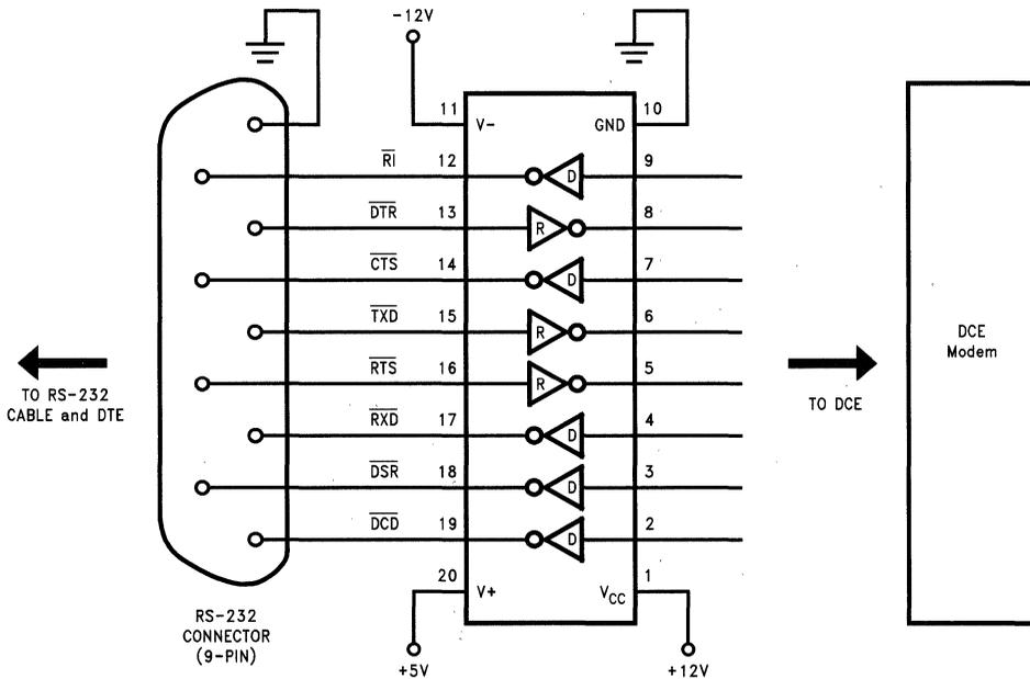
FIGURE 5. Typical DCE Application
