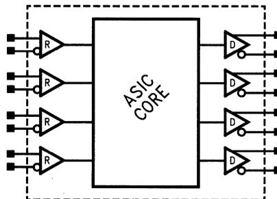
FIGURE 11. ASIC Cell Implementation of LVDS
