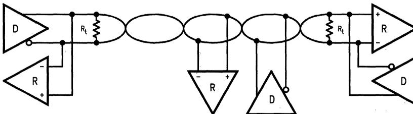
FIGURE 6. Example of Multi-Point Configuration
