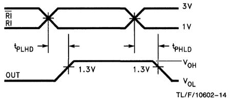
FIGURE 6. Receiver Differential Propagation Delay Timing
