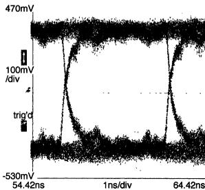
FIGURE 10a. Eye Pattern at Driver Output
