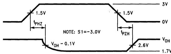
FIGURE 6. Receiver TRI-STATE® Delay Timing ( $t_{PZH}$ ,  $t_{PZH}$ )
