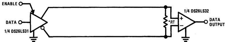
\*R<sub>T</sub> is optional although highly recommended to reduce reflection.
