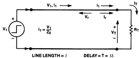
**FIGURE 1-1. Assigned Polarities and Directions for Determining Reflections**
