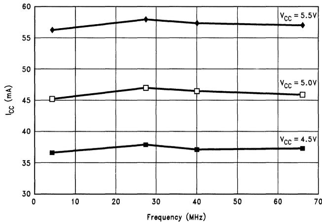
**FIGURE 7. DS3886A I<sub>CC</sub> vs Switching Frequency (A<sub>n</sub> to B<sub>n</sub>) (All Channels Switching at Room Temperature)**
