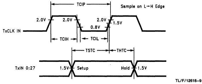
FIGURE 7. DS90CR583 (Transmitter) Setup/Hold and High/Low Times
