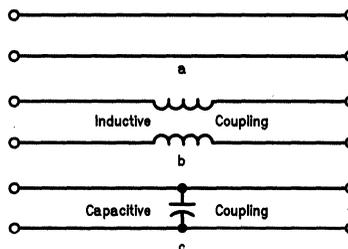
FIGURE 5. Cable-to-Cable Coupling
