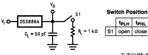
FIGURE 5. Receiver Propagation Delay Set-up
