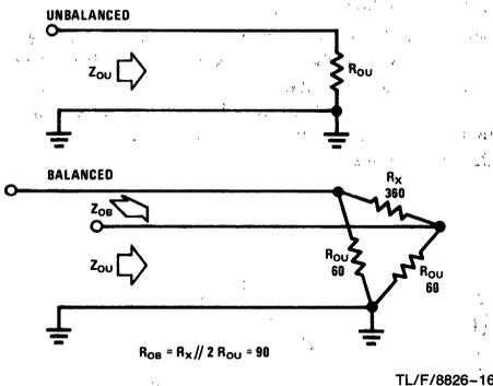
**FIGURE 16. Impedance Measurement**
