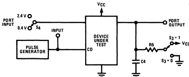
Note: C4 includes test fixture capacitance. Port input is in a fixed logical condition. See AC table.
