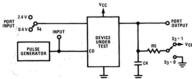
Note: C4 includes test fixture capacitance.
