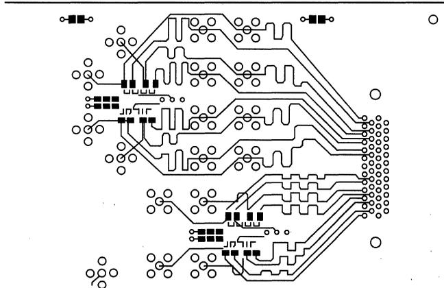
FIGURE 3. Trace Mitering on LVDS Lines
