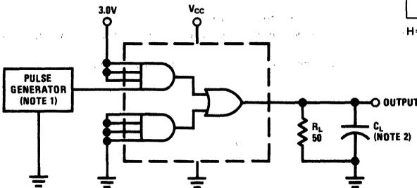
**Note 1:** The pulse generators have the following characteristics:  $Z_{OUT} \approx 50\Omega$ ,  $t_w = 200 \text{ ns}$ , duty cycle = 50%.
