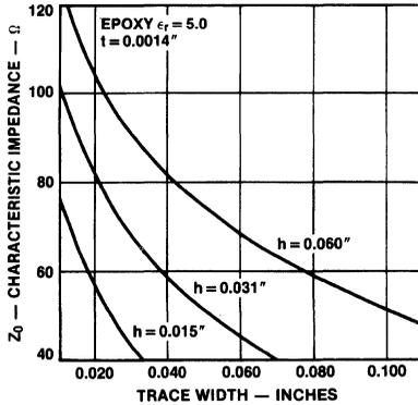
**FIGURE 2-2. Microstrip Impedance Versus Trace Width, G-10 Epoxy**
