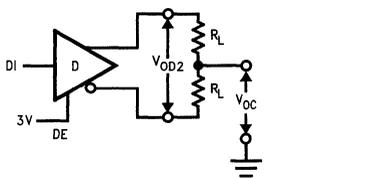
FIGURE 1. Driver V<sub>OD2</sub> and V<sub>OC</sub>
