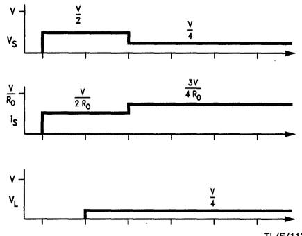
FIGURE 7.  $R_L = \frac{R_0}{3}$
