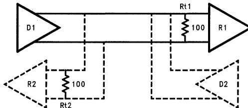
FIGURE 8. Bi-Directional Application over One Pair of Twp
