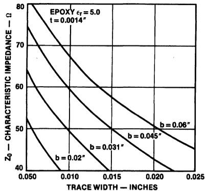
**FIGURE 2-4. Stripline Impedance Versus Trace Width, G-10 Epoxy**
