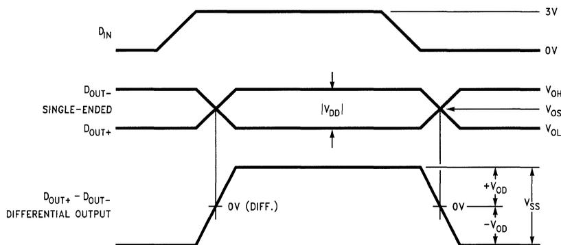
FIGURE 7. Driver Output Levels
