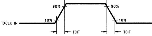
FIGURE 5. DS90CR581 (Transmitter) Input Clock Transition Time
