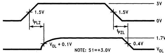
FIGURE 7. Receiver TRI-STATE® Delay Timing ( $t_{PLZ}$ ,  $t_{PLZ}$ )
