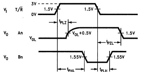
**FIGURE 9. T/R to Bn ( $t_{pHL}$  and  $t_{pLH}$  only), T/R to An ( $t_{pZL}$  and  $t_{pLZ}$  only)**
