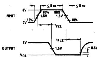
FIGURE 3.  $t_{PZL}$  and  $t_{PLZ}$
