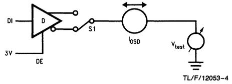
$V_{test} = -7V$  to  $+12V$
