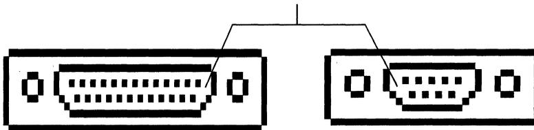
FIGURE 8. Example of Protected Connectors
