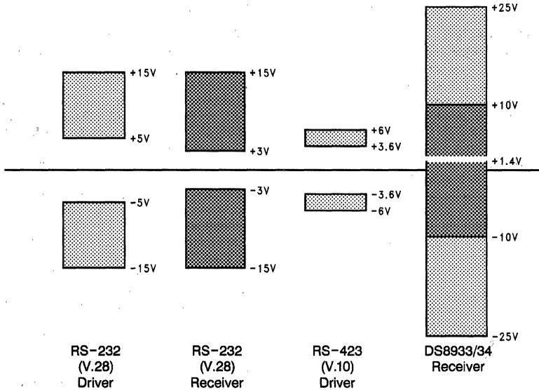
FIGURE 4. Signaling Levels
