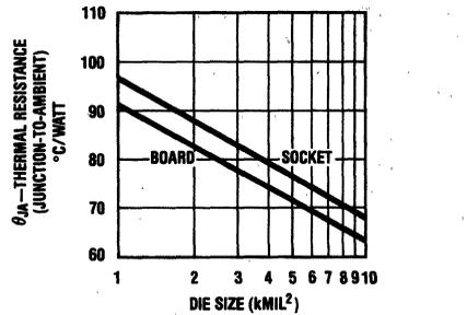
FIGURE 8. Thermal Resistance vs Board or Socket Mount
