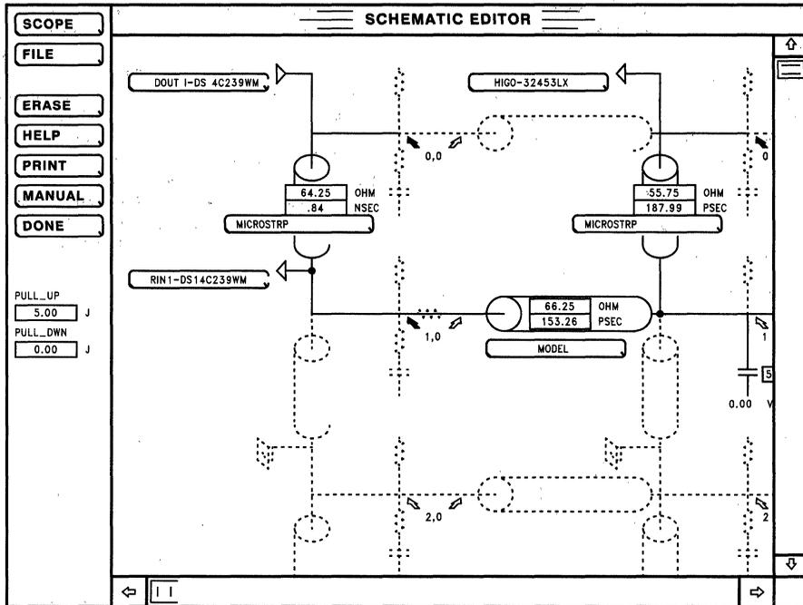
FIGURE 5. Schematic Editor of LineSim PRO
