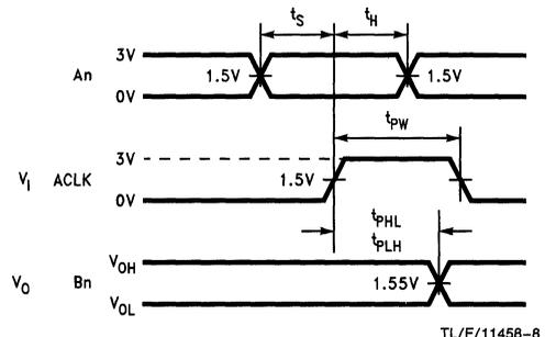
FIGURE 4. Driver: ACKL to Bn, t<sub>s</sub>, t<sub>h</sub>, t<sub>pw</sub>
