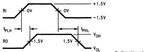
**FIGURE 14. Receiver Propagation Delays**
