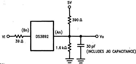
Note:  $t_{\text{R}} = t_{\text{F}} < 2 \text{ ns}$  from 10% to 90%
