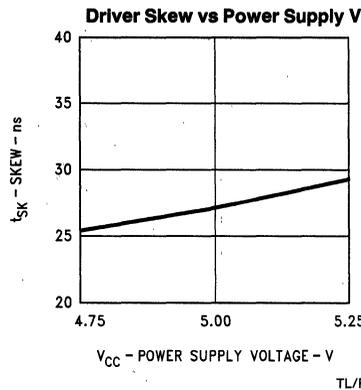
\*V defined as  $V_{CC} = |V_{EE}|$
