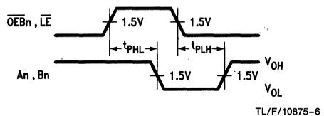
**Waveform 2: Propagation Delay for Data to Output**
