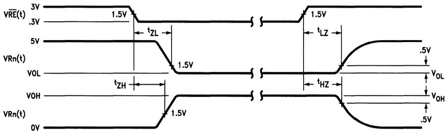
Note:  $t_{\text{r}} = t_{\text{f}} \leq 4 \text{ ns}$  From 10% to 90%
