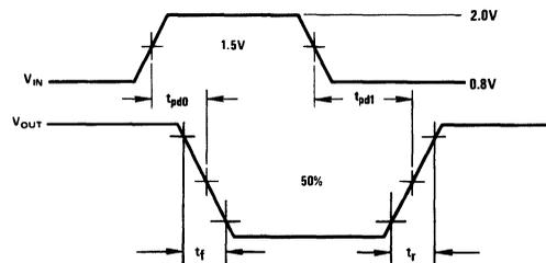
$t_r$  and  $t_f$  are measured between 10% and 90% of the output waveform.
