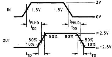
$$t_{SKW} = |t_{PLHD} - t_{PHLD}|$$
