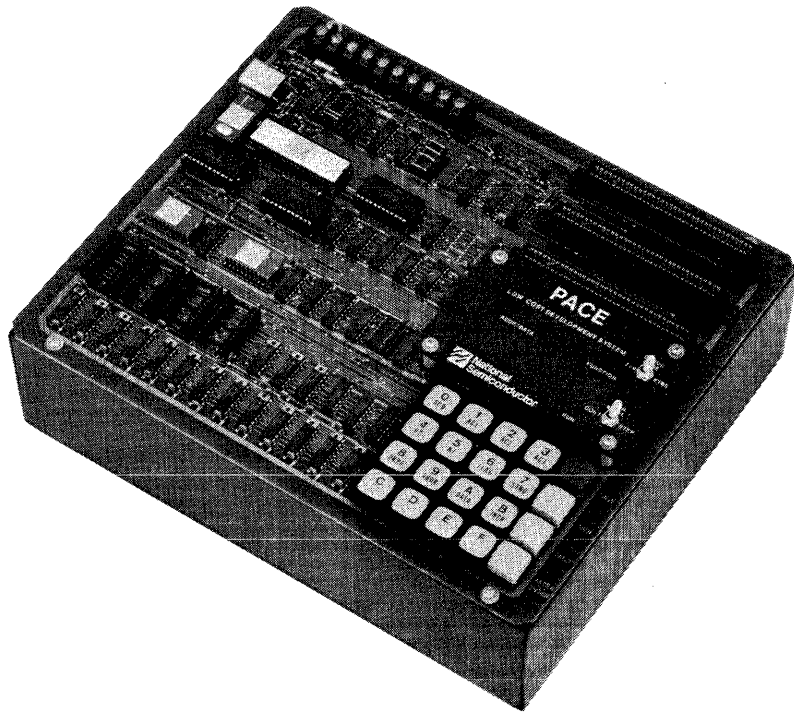
Figure 1-3. PACE Low Cost Development System (LCDS)
