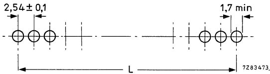
Fig. 2 Hole pattern for single-row bottom-entry sockets; see Table 1 for dimension L.
