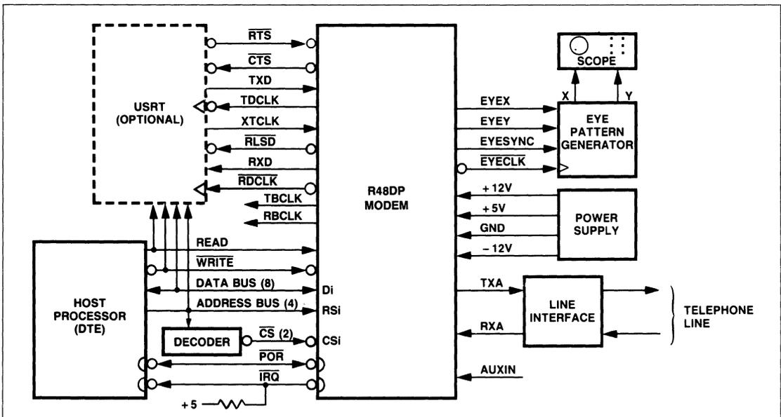
Figure 1. R48DP Functional Interconnect Diagram
