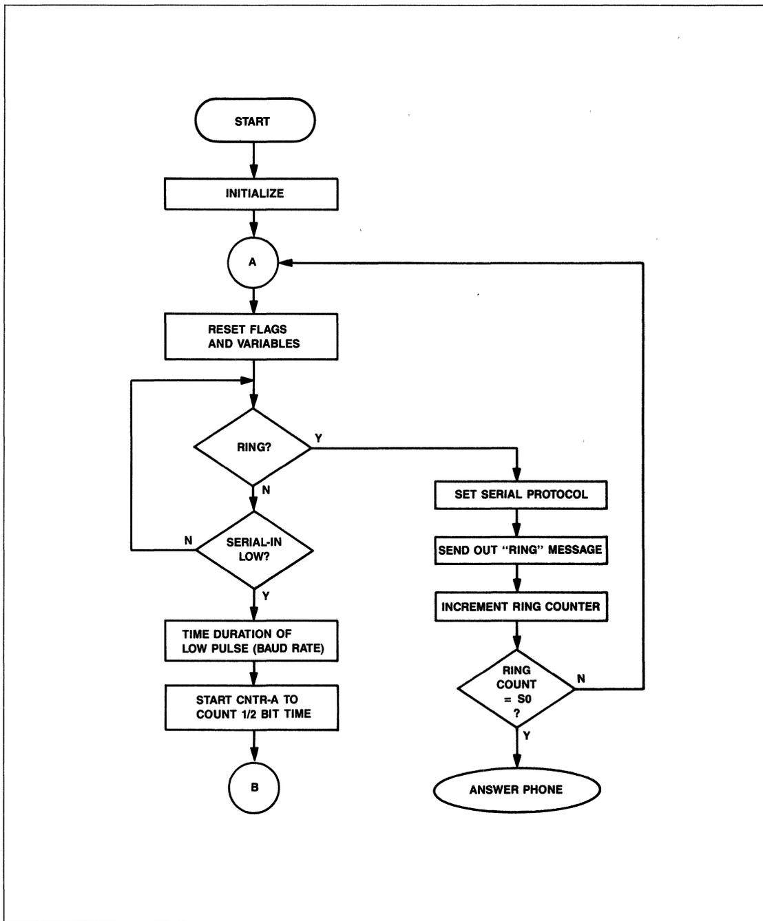
Figure 5. Command Mode Flowchart
