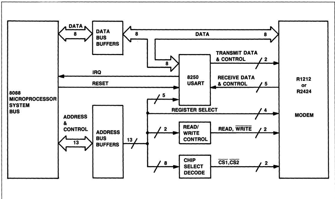
Figure 1. IBM PC to R1212/R2424 Modem Interface
