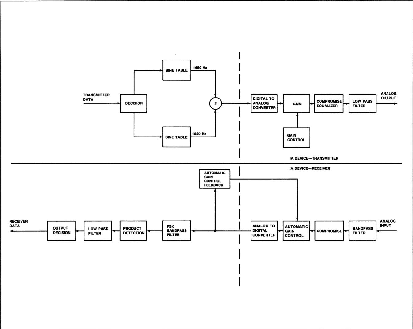
Figure 4. R96FAX FSK Processing Flow Diagram
