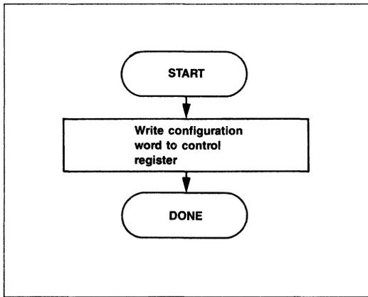
Figure 7. Flowchart — Basic Devices Setup: 82C55
