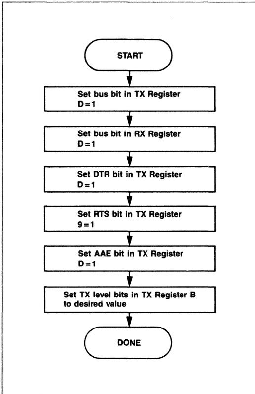
Figure 8. Flowchart — Basic Devices Setup: R2424
