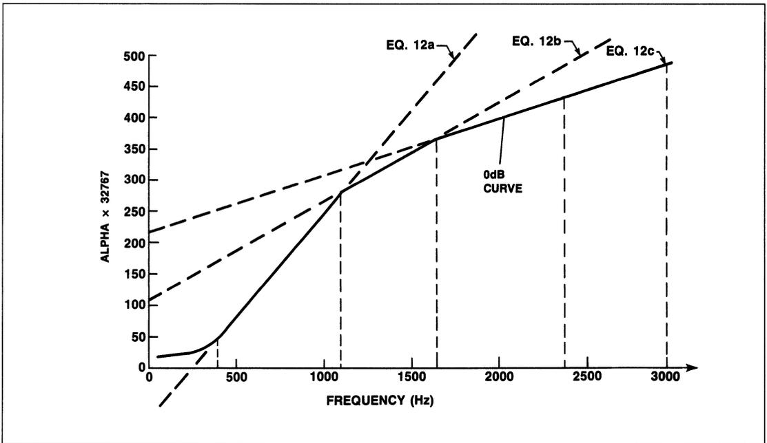
Figure 6.  $\alpha$  versus Center Frequency for  $|H(f_o)| = 0\text{dB}$
