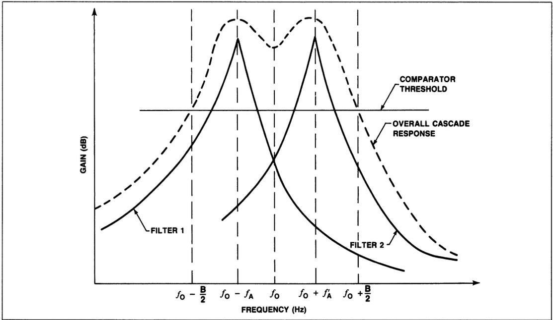
Figure 5. Graphical Representation of Bandwidth (B) and Offset Frequencies ( $f_A$  and  $f_o$ )
