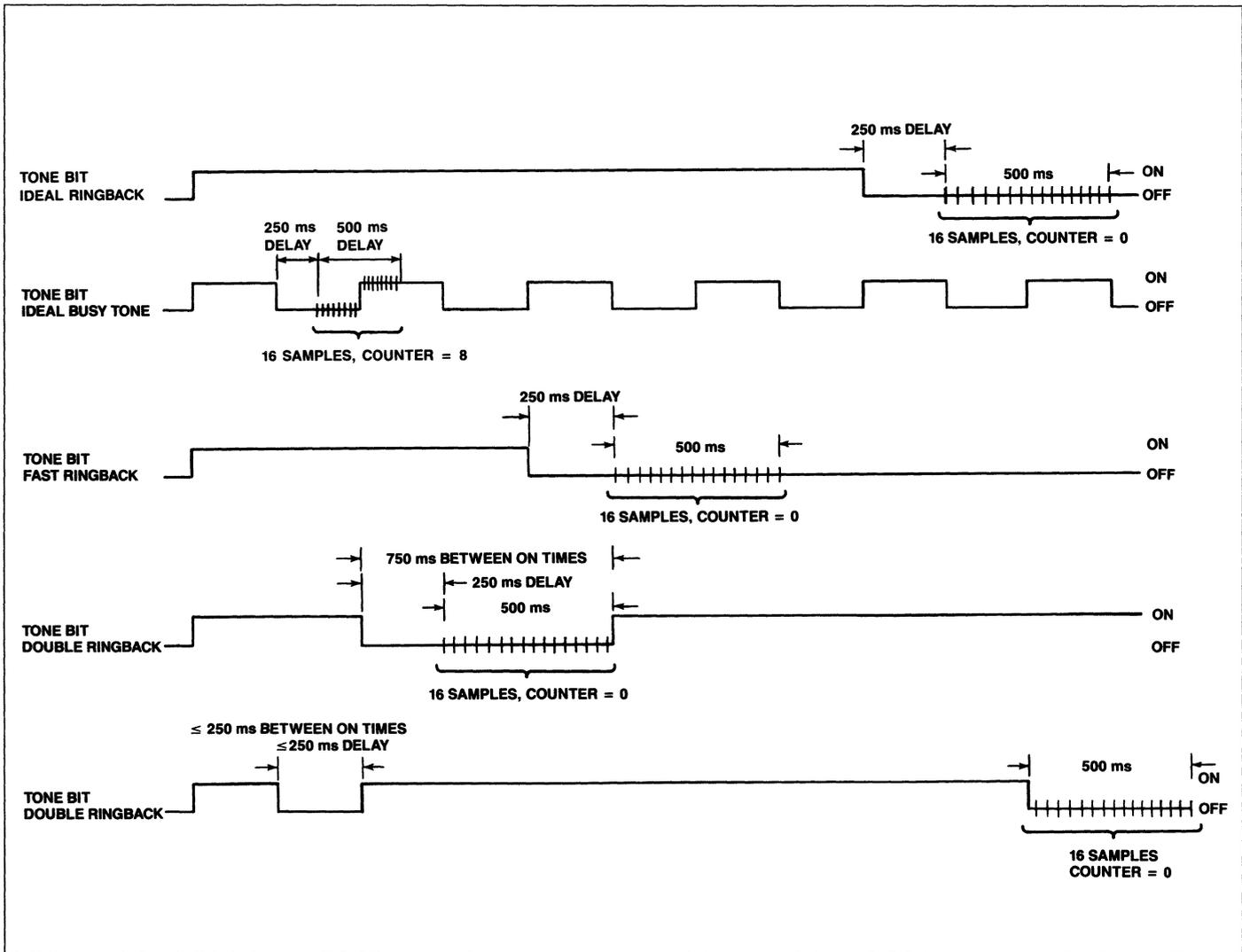
Figure 6. Timing for Call Progress Tone Detection Routine
