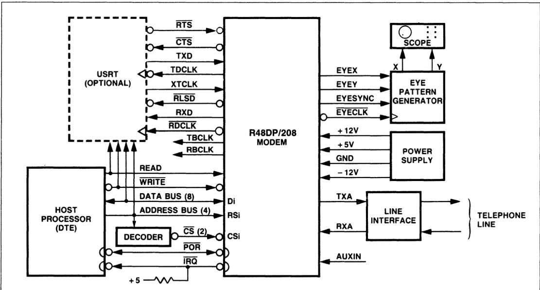
Figure 1. R48DP/208 Functional Interconnect Diagram
