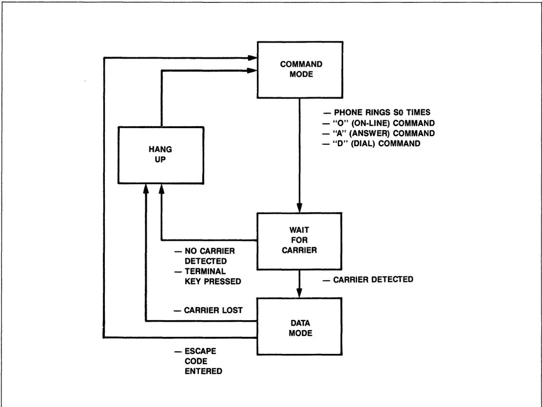
Figure 4. Modem Software Functional State Diagram
