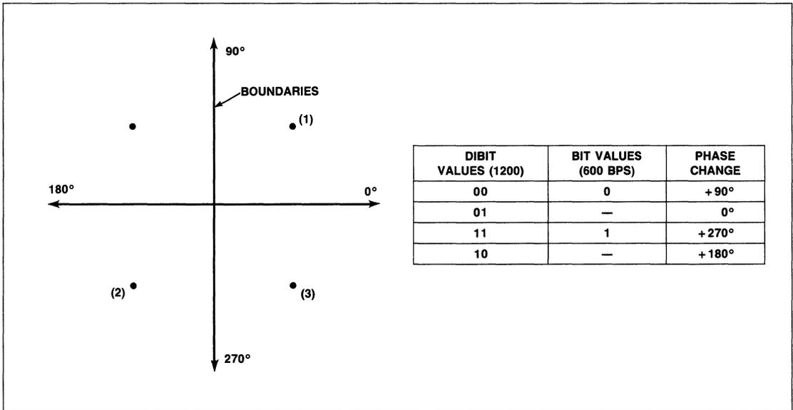
Figure 9. V.22 A/B 1200 bps/600 bps
