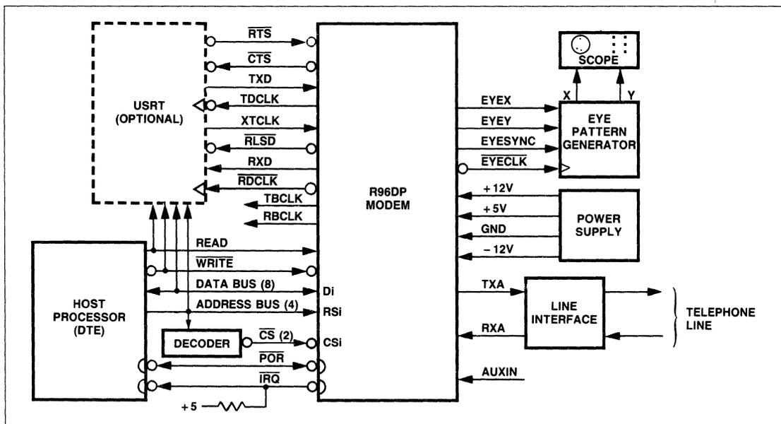
Figure 1. R96DP Functional Interconnect Diagram
