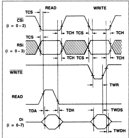
Figure 2. Microprocessor Interface Timing Diagram
