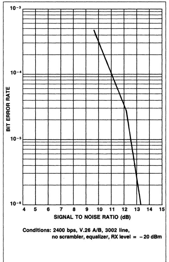
Figure 5. Typical BER Performance 3002 Unconditioned Line.
