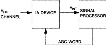
$V_{INT} = \frac{(A/D \text{ Sample Word})_{16}}{(40)_{16}} \times \frac{3}{256} \text{ Volts}$ $V_{EXT} = V_{INT} \div \text{LOG}_{10}^{-1} \left[ \frac{\text{AGC Gain (dB)}}{20} \right]$
