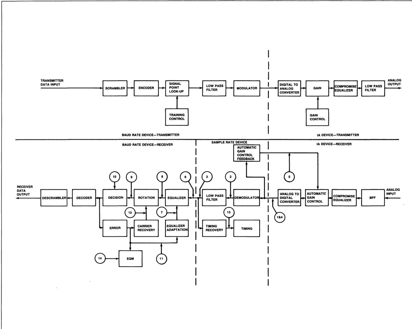
Figure 2. R48DP/R96DP/R96FT/R96FAX (Group 3) Processing Flow Diagram
