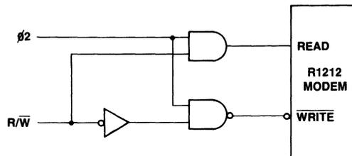
Figure 3. R/W to READ WRITE Conversion Logic
