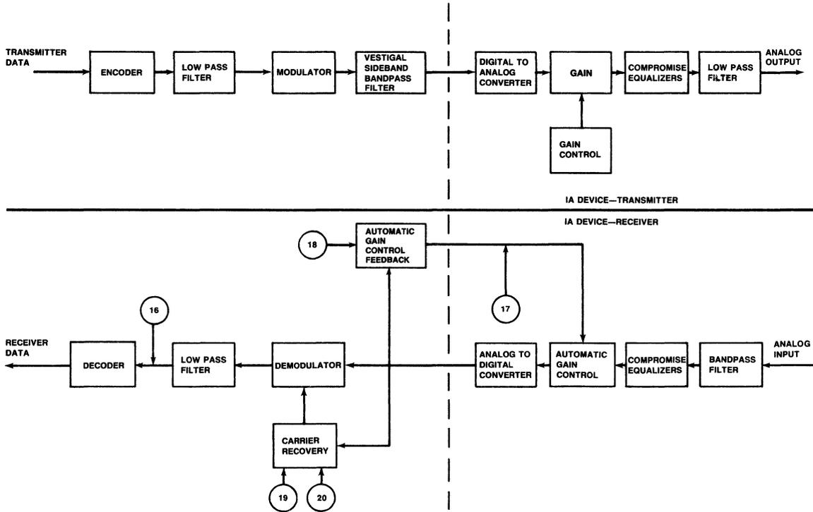
Figure 3. R96FAX (Group 2) Processing Flow Diagram
