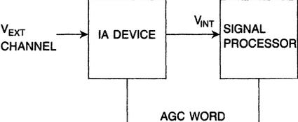
$V_{INT} = \frac{(A/D \text{ Sample Word})_{16}}{40_{16}} \times \frac{3}{256} \text{ Volts}$ $V_{EXT} = V_{INT} \div \text{LOG}_{10}^{-1} \left[ \frac{\text{AGC Gain (dB)}}{20} \right]$
