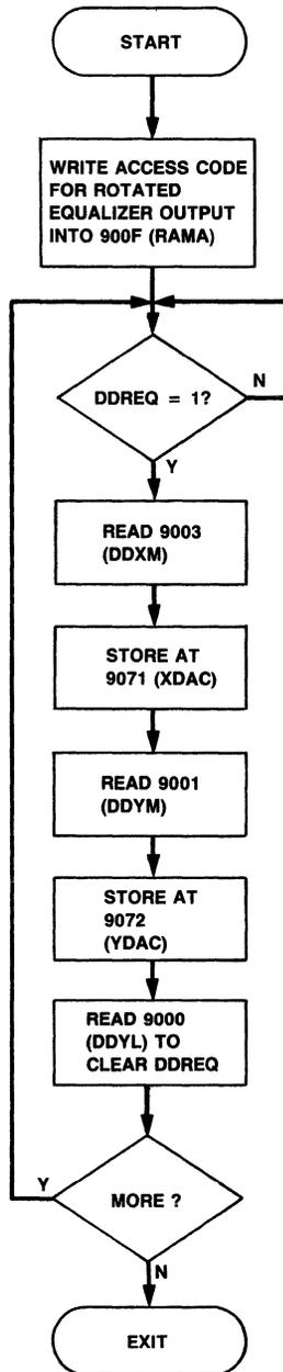
Figure 7. Eye Pattern Generation Flowchart
