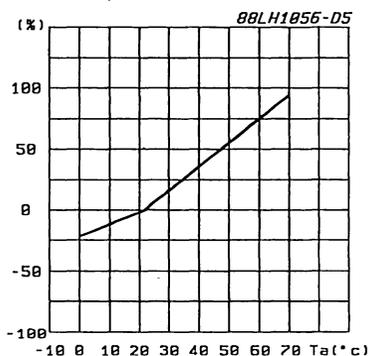
**Figure 11 :** Normalized Current Limit vs. Temperature.
