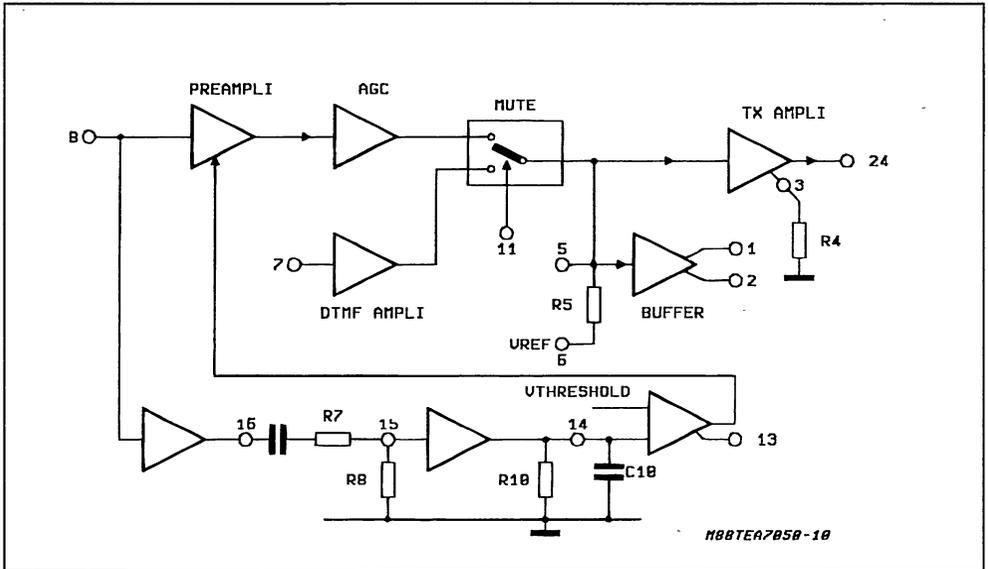
2.1. A.G.C. IN TRANSMISSION. The transmission gain between Microphone Input (pin 8) and Vline (pin 24) is internally decreased of 6dB when the line current varies from 27mA to 42mA with a constant AC load of 600ohms.
