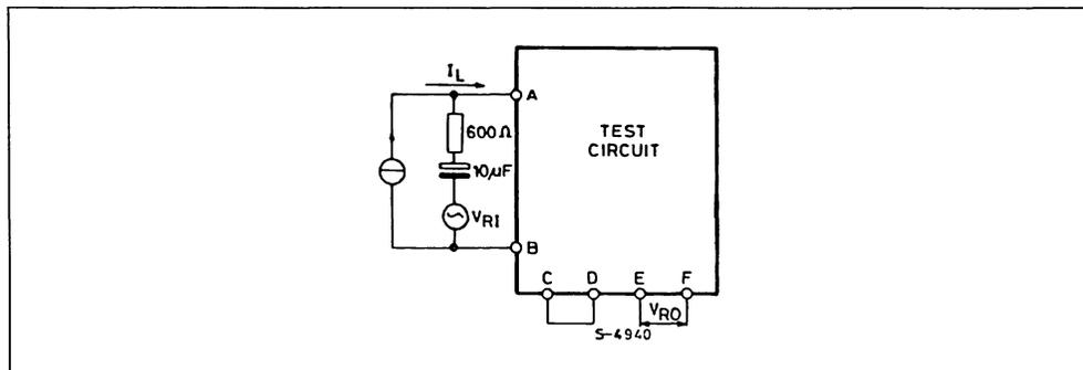
**ELECTRICAL CHARACTERISTICS** (Refer to test circuits,  $T_{amb} = -25$  to  $+50$  °C,  $f = 200$  to  $3400$  Hz,  $I_L = 15$  to  $100$  mA,  $R_7 = 17.3$  k $\Omega$ ,  $R_8 = 17.1$  k $\Omega$ , S1 in A, S2 in A, unless otherwise specified)
