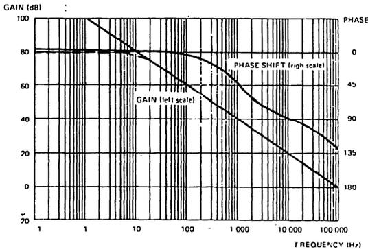
OPEN LOOP FREQUENCY RESPONSE AND PHASE SHIFT
