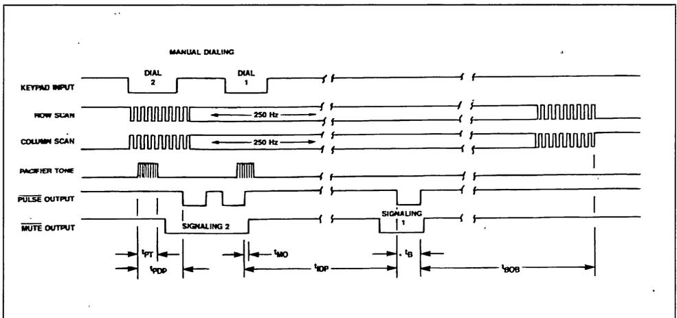
Figure 3B : MK5376 Timing Diagram - Tone Mode.
