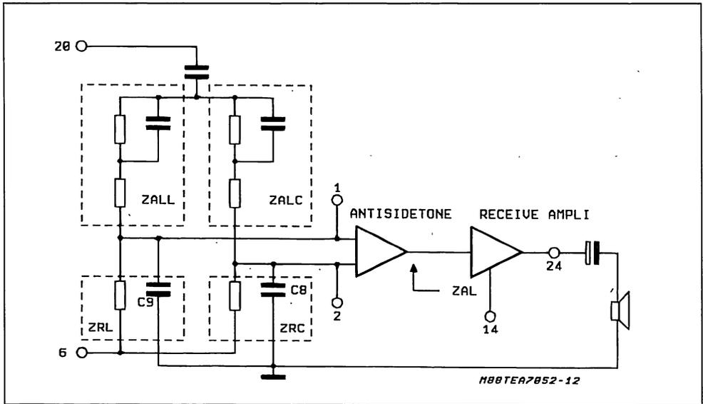
3.1. A.G.C. IN RECEIVE. As described for the transmission chain, also the receiving gains  $G_r$ , from pins 1 and 2 to pin 24, have a reduction of 6dB when line moves from 27mA to 42mA.
