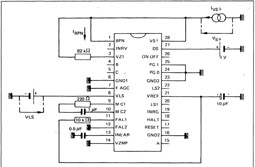
Figure 8 : Test Power Supply in Ring Mode - VB + MAX.
