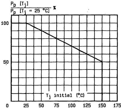
Fig.3 - Allowable power dissipation versus junction temperature.
