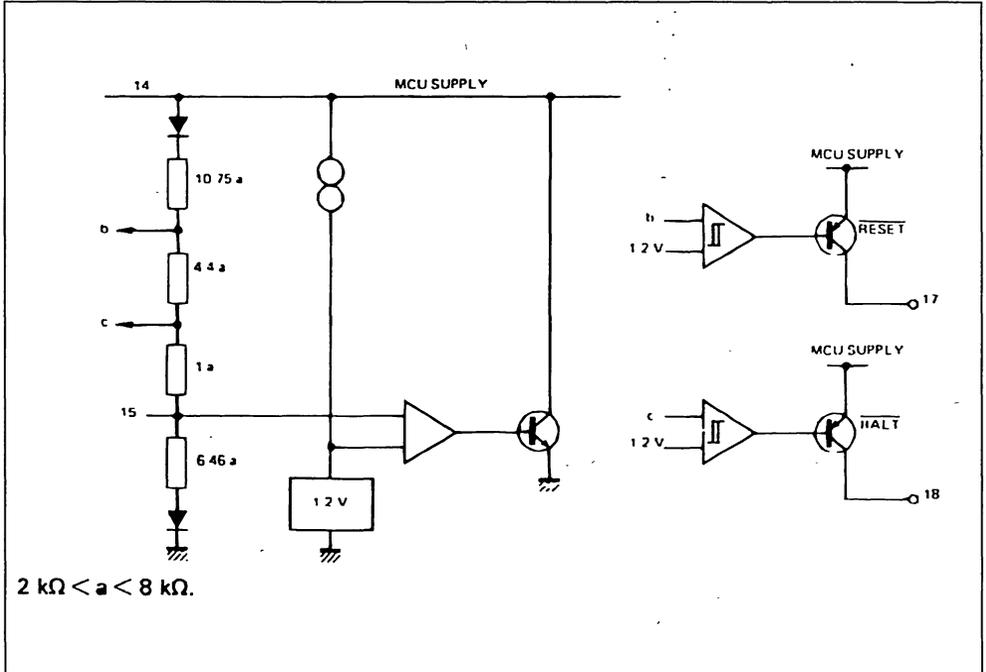
Note : Reset and Halt outputs, which are open collector outputs, require external resistors to zero volt.
