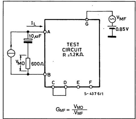
**ELECTRICAL CHARACTERISTICS** (refer to the test circuits, S1 and S2 in (a),  $T_{amb} = -25$  to  $+50$  °C,  $f = 200$  to  $3400$  Hz, unless otherwise specified)
