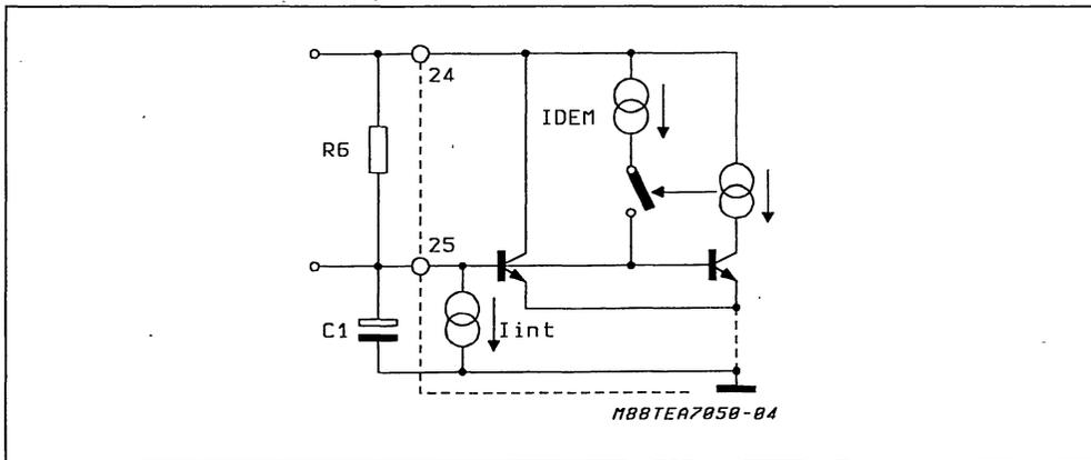
At "Off-hook", with only DC voltage applied to the line terminals, C1 fixes the timing of the line current profile at :
