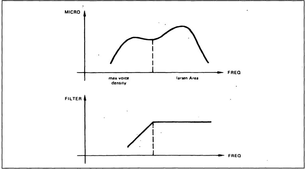
To extract the larsen component, the microphone signal is first filtered by a second order filter (formed
