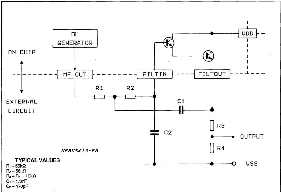
The filter components shown have been chosen to give a second order Butterworth response with a cut-off frequency of about 3.5KHz. The pass-band insertion loss is nominally 0.5dB.
