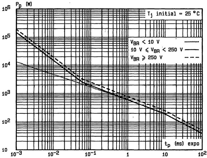
Fig.1 - Peak pulse power versus exponential pulse duration.
