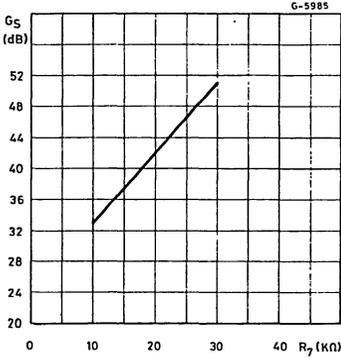
Figure 9 : Receiving Gain vs.  $R_8$  Value (AGC OFF).
