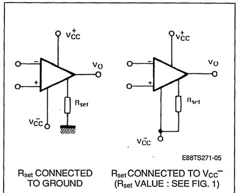
Figure 1 :  $R_{set}$  Connected to  $V_{CC}^-$ .
