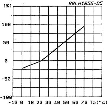
**Figure 11 :** Normalized Current Limit vs. Temperature.
