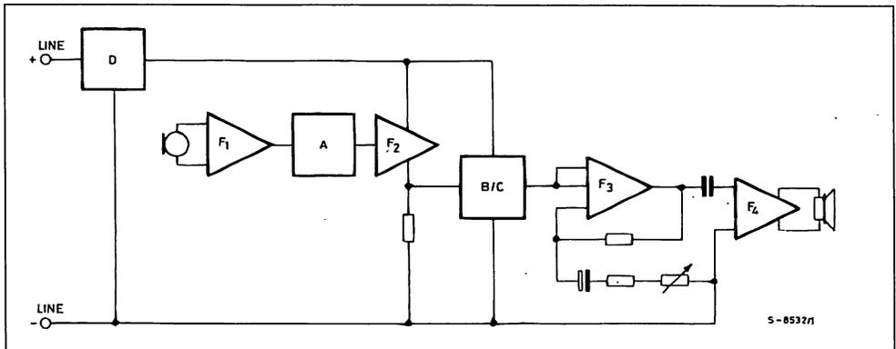
In this case an extra 20 dB amplification is added to the receiving part. A potentiometer provides the
