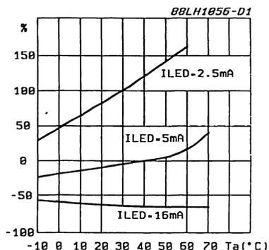
**Figure 7 : Normalized Turn-off Time vs. Temperature.**
