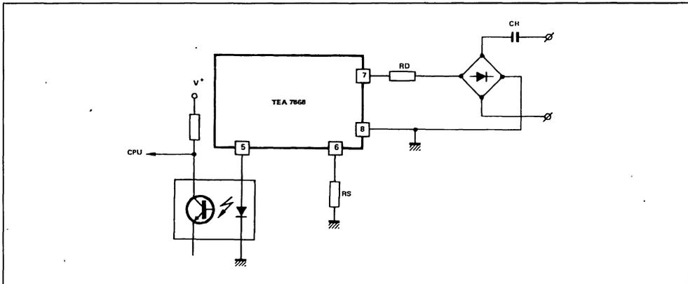
The ringing signal coming from the line is rectified by the diode bridge ; the circuit compares the peak amplitude of the signal to a predetermined detection level fixed by  $R_S$ . On the output transistor of the optocoupling device a logic signal is generated which frequency is twice the frequency of the ringing signal.
