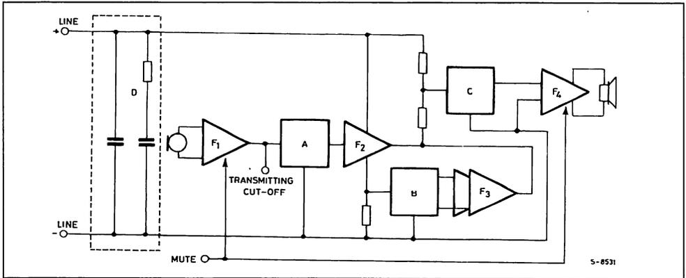
A, B, C and D are RC links with the following functions :
