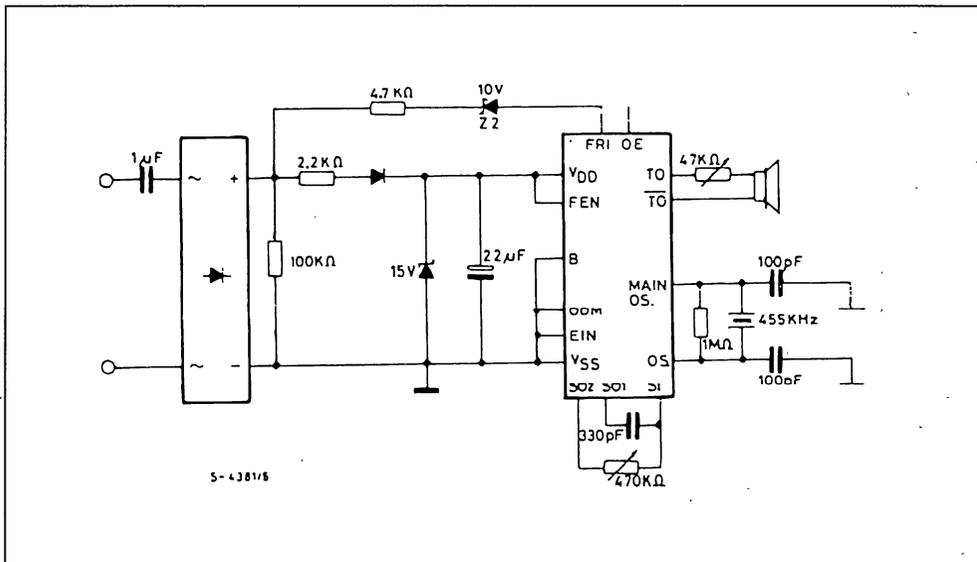
If pin EIN is connected to V<sub>DD</sub> the ringer is activated by frequencies upper than 20 Hz.
