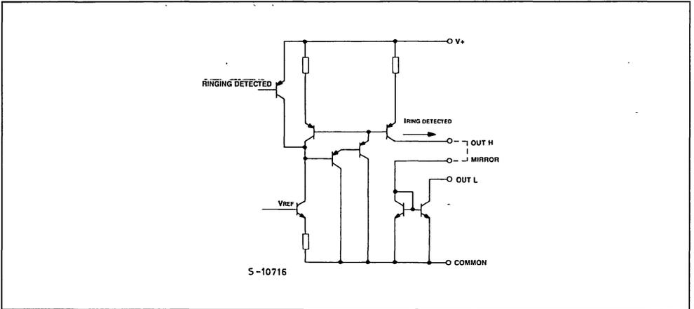
Figure 12 : Typical Application for Interface Direct to Logic.
