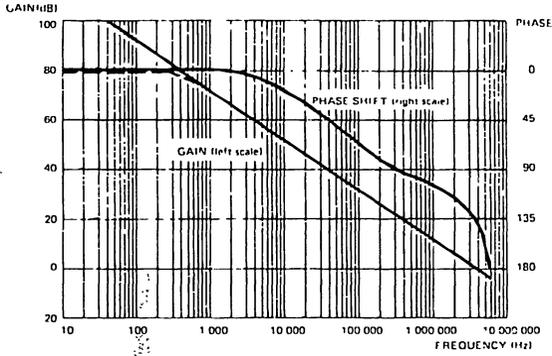
OPEN LOOP FREQUENCY RESPONSE AND PHASE SHIFT
