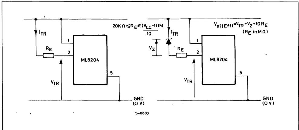
Oscillation of the ML8204 may be inhibited for voltages in the range  $V_{si} < V_s \leq V_{s(max)}$  by sinking the current from D<sub>1</sub>, starving Q<sub>1</sub> of base current. This is achieved by either a) grounding pin 2 (fig. 6a), or b) applying a voltage  $V_{INH}$  via a resistor R<sub>1</sub> to pin 2 (fig. 6b) to ensure that :
