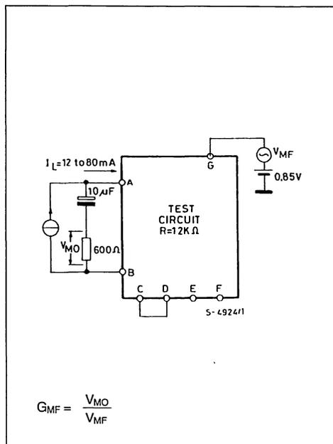
**ELECTRICAL CHARACTERISTICS** (refer to the test circuits,  $V_G = 1$  to 2 V,  $I_L = 12$  to 80 mA, S1, S2 and S3 in (a),  $T_{amb} = -25$  to  $+50$  °C,  $f = 200$  to 3400 Hz, unless otherwise specified)
