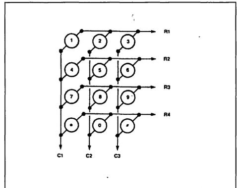
**Figure 1B : Keyboard Schematics Standard Telephone Type Keypad.**
