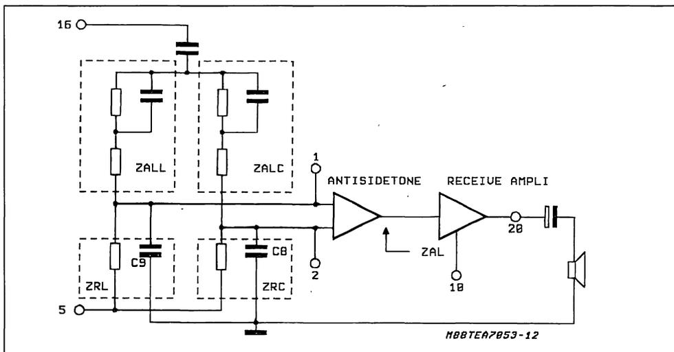
**3.1. A.G.C. IN RECEIVE.** As described for the transmission chain, also the receiving gains  $G_r$ , from pins 1 and 2 to pin 20, have a reduction of 6dB when  $I_{line}$  moves from 27mA to 42mA.
