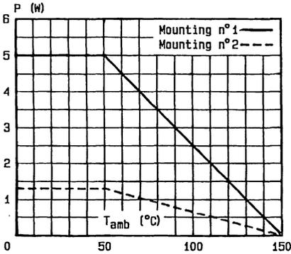
Fig. 1 - Power dissipation versus ambient temperature.
