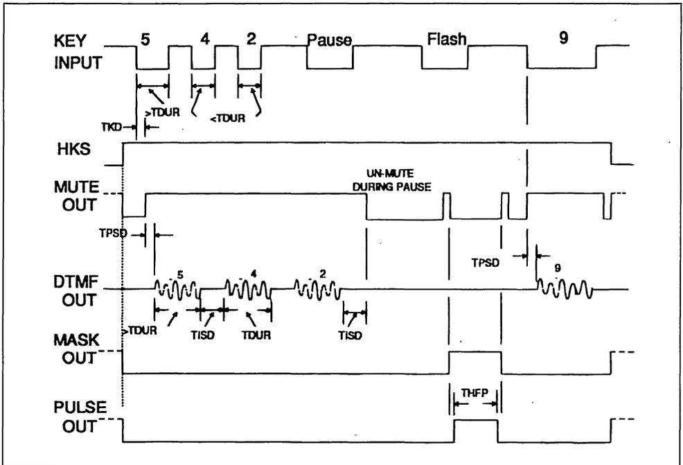
Figure 2 : Pulse Mode Timing.
