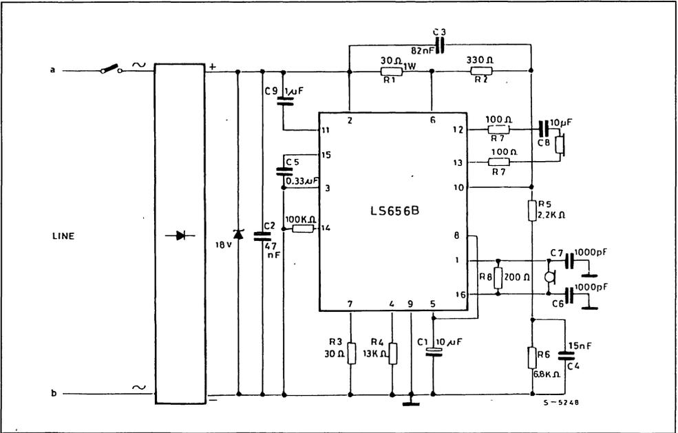
Figure 14 : Application Circuit with Gain Controlled by Line Voltage (french standard).
