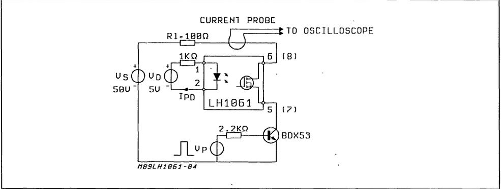
Figure 13 : Current spike ( $R_L = 100\Omega$ ,  $V_S = 50V$ ).
