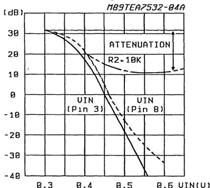
$$\text{ATTENUATION} = \frac{Z_{in2} (1.2 K)}{Z_{in2} (1.2 K) + R_2 (E X T)}$$
