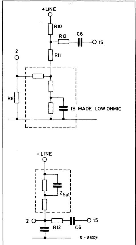
Figure 9 : 20dB Extra Amplifier (cannot be used in all version).
