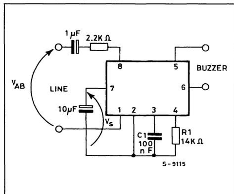
**Figure 2 : Typical Application with Balanced Output.**
