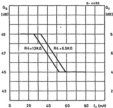
Figure 13 : Balance Network Impedance vs. Line Current.
