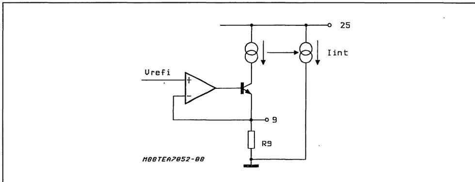
Vline must be externally adjusted (with R6) to guarantee both DC and AC characteristic in accordance to the french standards. At this purpose it is suggested that Vline equals 5.6 volts at Iline = 16mA. This typical value is obtained with R6 = 13Kohm.
