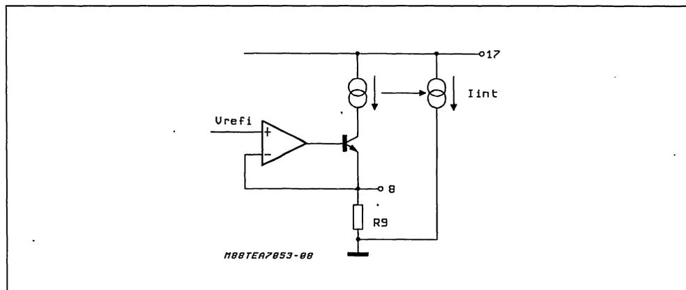
1.4. HIGH VOLTAGE CONTROL STAGE (pin 13). The behaviour of "HV control" is determined by several conditions, both internal (I<sub>line</sub> sensor) and external (pins 12 and 17) with the purpose to accomplish the different DC characteristics and transitory conditions imposed by the French specification :
