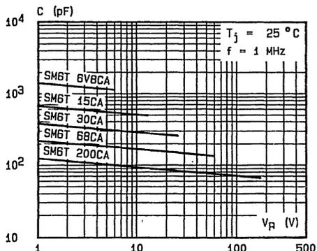
Fig. Bb - Capacitance versus reverse applied voltage for bidirectional types (typical values).
