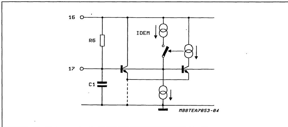
At "Off-hook", with only DC voltage applied to the line terminals,  $C1$  fixes the timing of the line current profile at :
