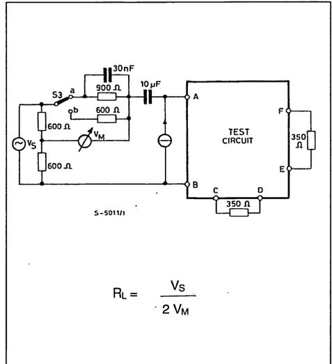
**ELECTRICAL CHARACTERISTIC** (refer to the test circuit,  $T_{amb} = 25\text{ }^{\circ}\text{C}$ ,  $f = 300\text{ Hz}$  to  $3400\text{ Hz}$ , S1, S2 in "a" unless otherwise specified)
