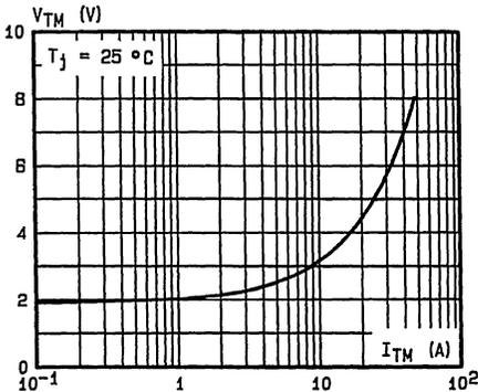
Fig.5 - On-state voltage versus on-state current (typical values).
