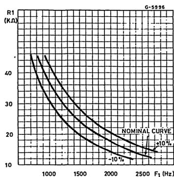
$$R_1 \approx \frac{3.56 \times 10^4}{F_1 \text{ (HZ)}} \times (1 - 0.16 \times \ln \frac{F_1}{2543})$$
