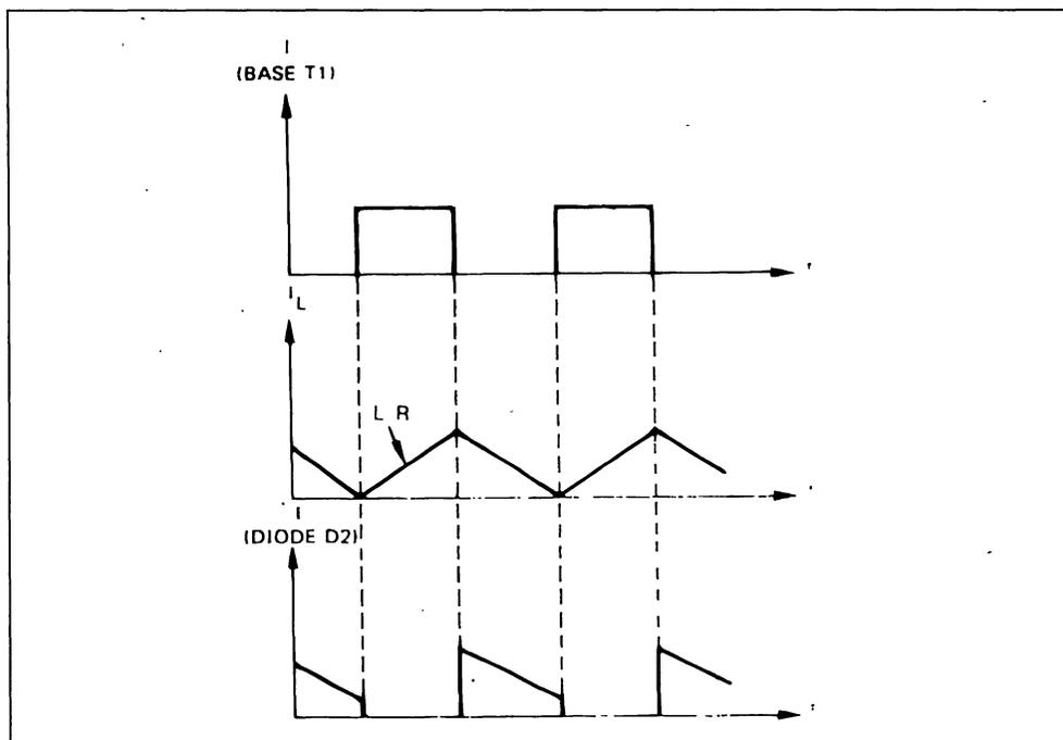
Internal conditions during switching converter operation :
