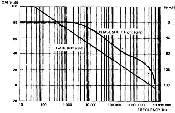
OPEN LOOP FREQUENCY RESPONSE AND PHASE SHIFT
