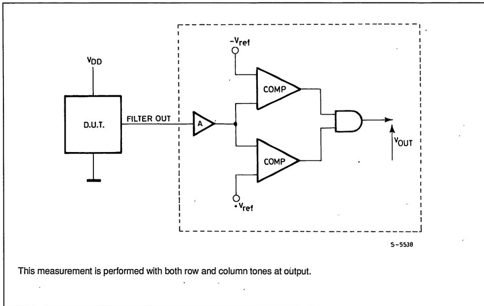
Figure 2 : Out Tone Level Measurement Test Set.
