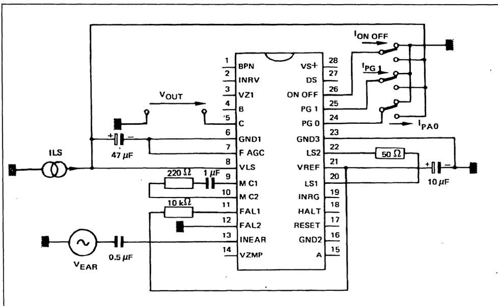
Figure 6 : Test Antiacoustic System Efficiency.
