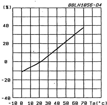
**Figure 10 :** Normalized Threshold Current vs. Temperature.
