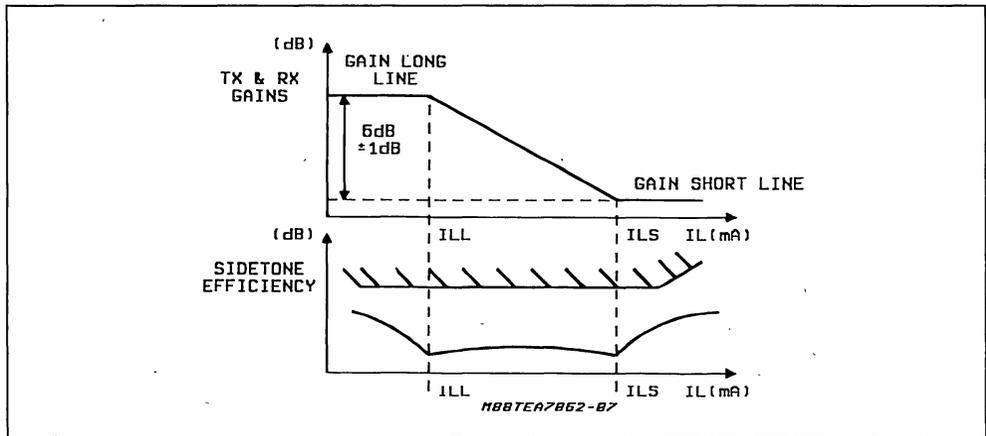
**4.1 PROGRAMMABLE CONTROLS.** AGC and sidetone attack and disconnect points (or currents) are programmable externally through two independent pins, I-start (pin 19) and I-slope (pin 13).
