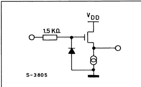
The following equivalent circuit should be applied during filter design :
