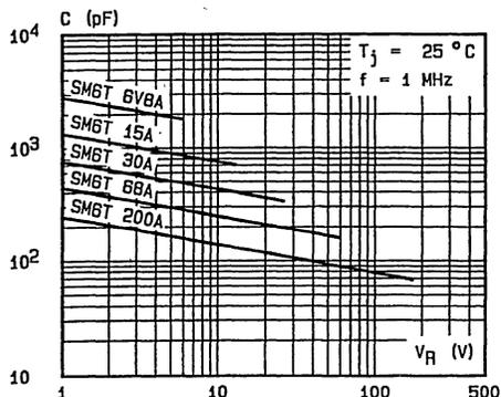
Fig. Ba - Capacitance versus reverse applied voltage for unidirectional types (typical values).
