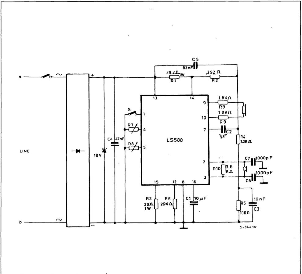
Figure 11 : Anticlippping Application.
