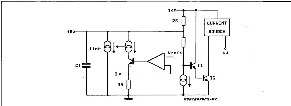
**1.2 V<sub>LINE</sub> (pin 14).** The line voltage (pin 14) is determined by the value of the external resistor R6 and by the internal current, I<sub>int</sub>, flowing between Vc (pin 15) and Ground (see also paragr. 1.1) :
