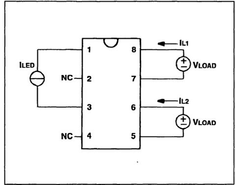
Figure 4 :  $\tau_{ON}/\tau_{OFF}$  Test Circuit and Waveform.
