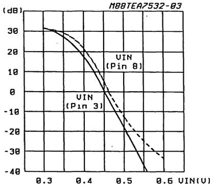
**Figure 2 : AC Output Voltage versus Amplifier Gain.**
