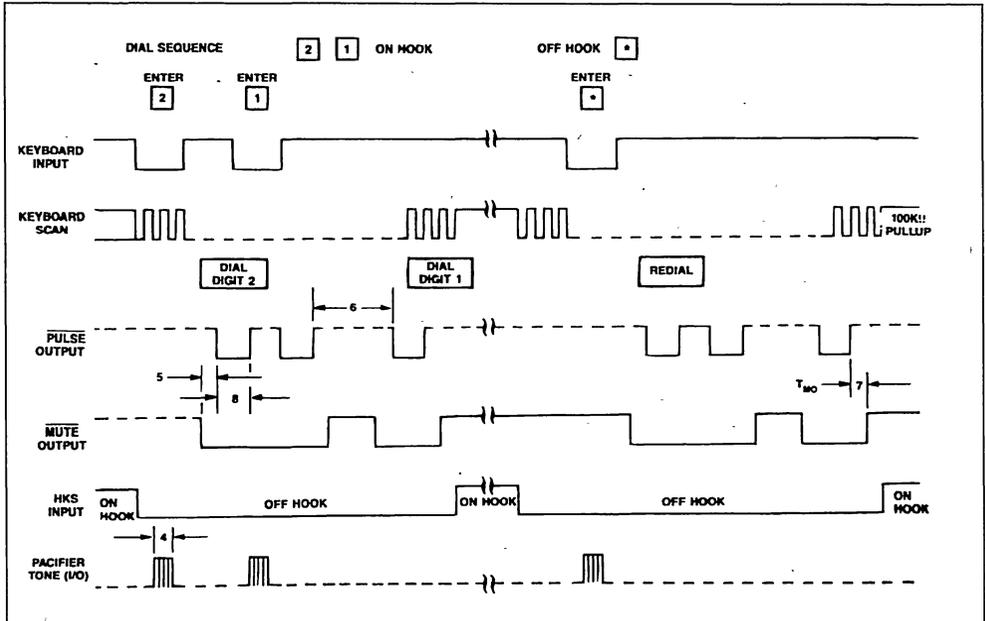
Figure 6 : Pulse and Tone Mode Timing.
