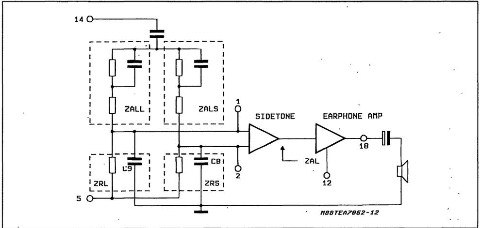
**3.1 A.G.C. IN RECEIVE.** As described for the transmission chain, also the receiving gains  $G_r$ , from pins 1 and 2 to pin 24, have a reduction of 6dB when  $I_{line}$  moves from ILL to ILS (see also paragr. 4).
