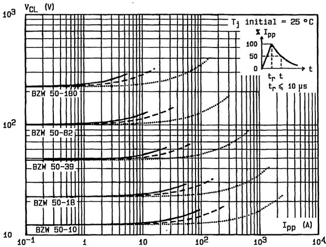
Fig.2 - Clamping voltage versus peak pulse current.
