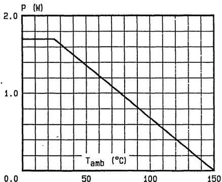
Fig. 4 - Power dissipation versus ambient temperature.
