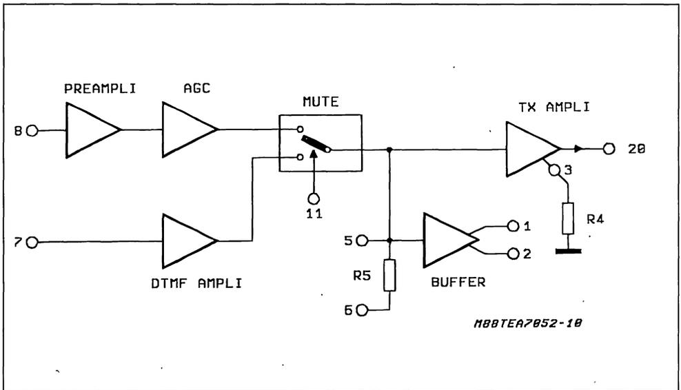
2.1. A.G.C. IN TRANSMISSION. The transmission gain between Microphone Input (pin 8) and Vline (pin 20) is internally decreased of 6dB when the line current varies from 27mA to 42mA with a constant AC load of 600 ohms.
