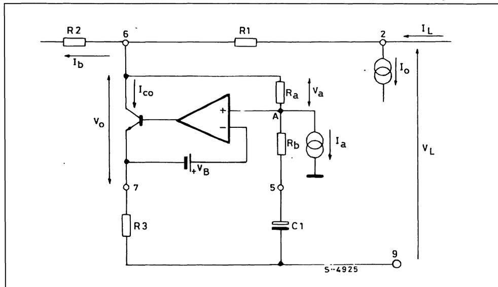
It is important to note that the DC voltage at pin 5 is proportional to the line current ( $V_5 = V_7 + V_B = (I_L - I_0) R_3 + V_B$ ).
