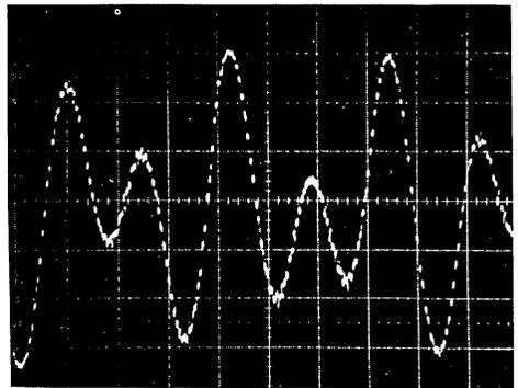
**Figure 2C** : Spectral Analysis of Waveform in Fig.5 (Vert.10 dB/div. Horizontal - 600 Hz/div.).
