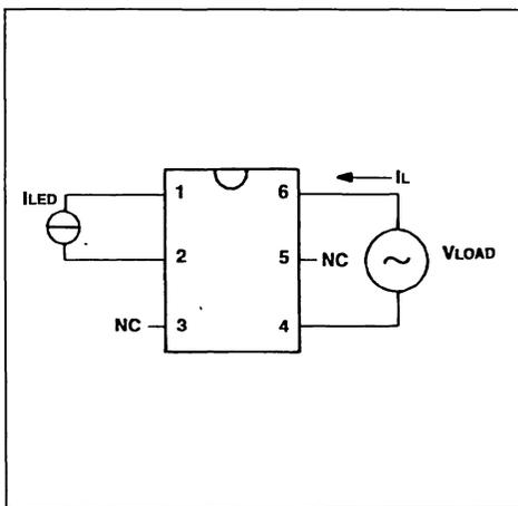
Figure 4 :  $\tau_{ON}/\tau_{OFF}$  Test Circuit and Waveform.
