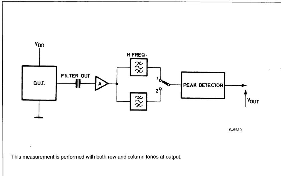
Figure 3 : THD Measurement Test Set.
