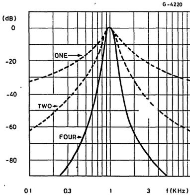
**Figure 19** : Bandwidth of Band-pass Filter.
