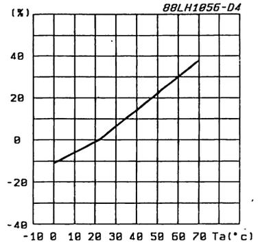
**Figure 10 :** Normalized Threshold Current vs. Temperature.
