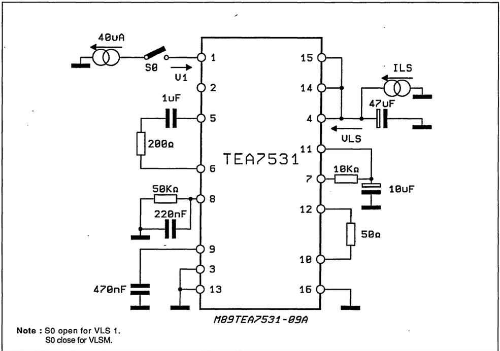
Figure 7 : Loudspeaker Amplifier : Gain/Distortion/Output Offset.
