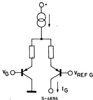
b) When gains have to be related to the voltage at the line terminals of the telephone set, it is necessary to obtain  $V_G$  from a resistive divider directly connected to the end of the line.
