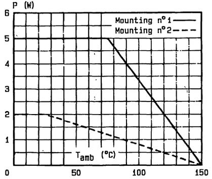
Fig. 4 - Power dissipation versus ambient temperature.
