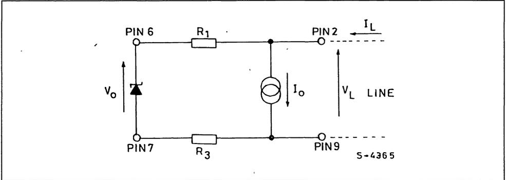
**Figure 6 :** Circuit Configuration of the Shunt Regulator.
