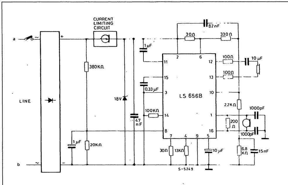
Figure 15 : Application Circuit with Fixed Gain Operation.
