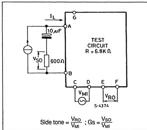
$$\text{Side tone} = \frac{V_{RO}}{V_{MI}} ; G_s = \frac{V_{SO}}{V_{MI}}$$
