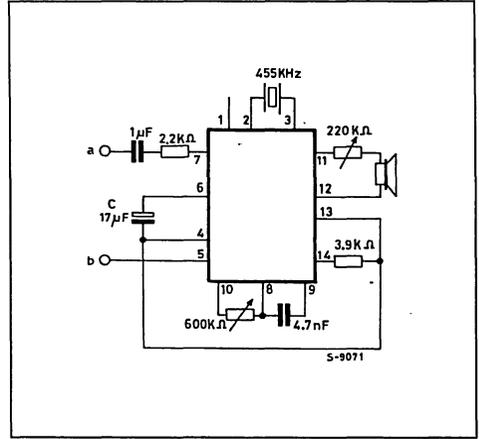
**Figure 4 :** Circuit Connection Scheme for Repetition Frequency Adjustment Described in Section 5.
