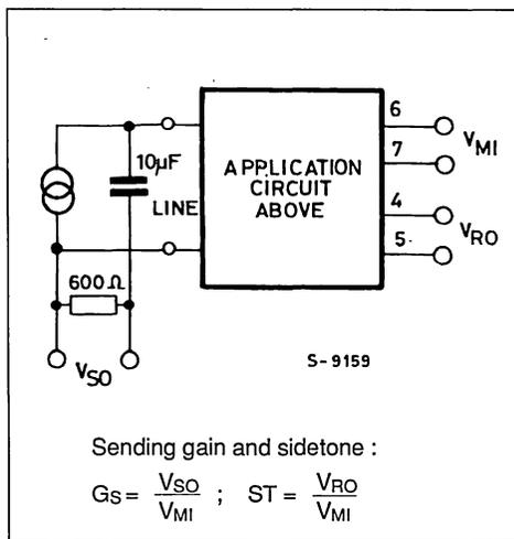
**ELECTRICAL CHARACTERISTICS** ( $T_{amb} = 25\text{ }^{\circ}\text{C}$  ; frequency = 1 Khz ;  $I_L = 20\text{ mA}$  : mute low ;  $R1$  (pin 14) =  $43\text{ }\Omega$  unless otherwise spec.)
