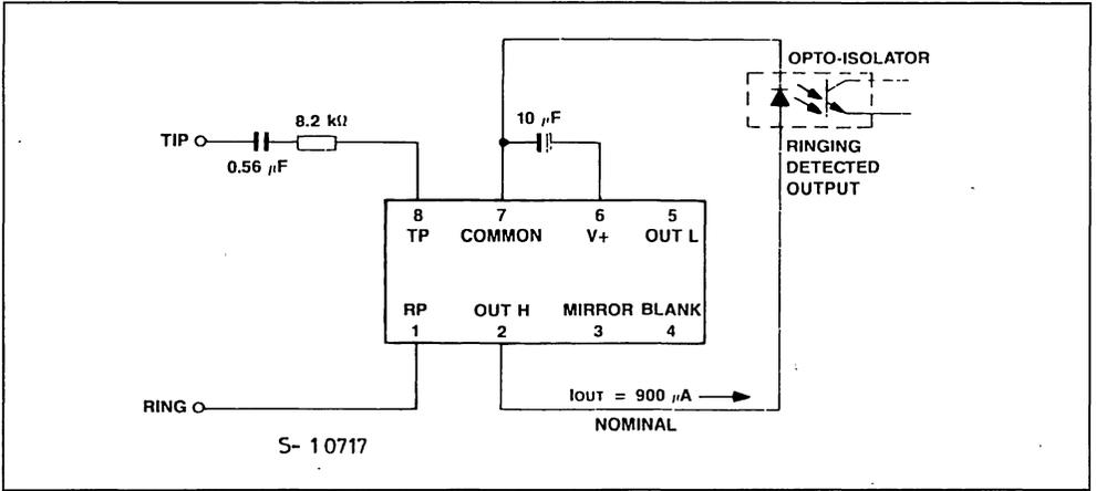
Figure 11 : Typical Application for Opto-isolator Drive.
