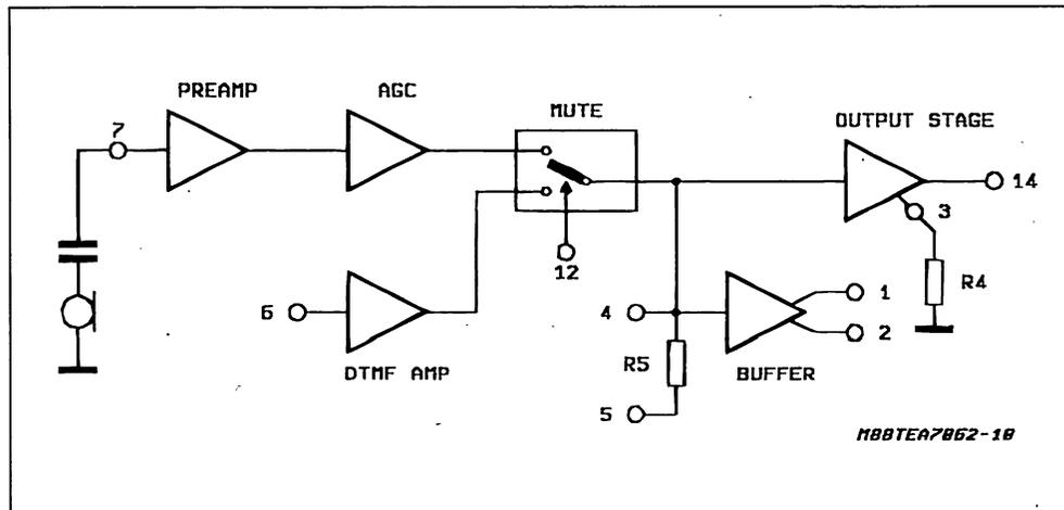
**2.1 A.G.C. IN TRANSMISSION.** The transmission gain between Microphone Input (pin 7) and Vline (pin 14) is internally decreased of 6dB when the line current varies from ILL to ILS with a constant AC load of 600Ω.
