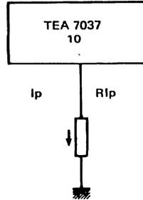
$$R_{lp} \text{ in MW} = \frac{7.8}{I_{p\mu A}}$$
