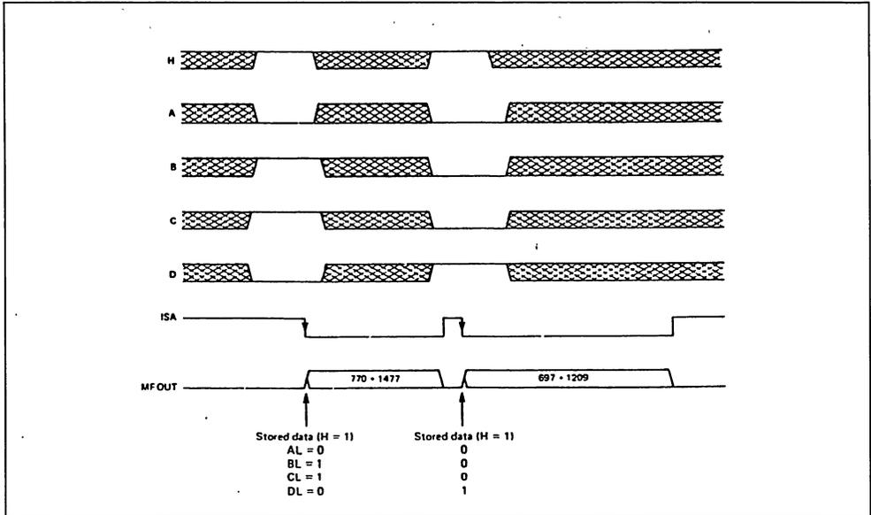
**Note :** If the circuit operates permanently in parallel mode, then the H input may be left floating (internally pulled-up to V\*) or tied to logic 1. With ISA at logic 0, H,A,B,C, and D inputs cannot modify the generated DTMF pair.
