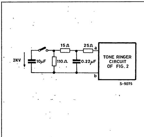
Figure 7 : Test Circuit which Activates the Output Signal Generator (see also frequency specification).
