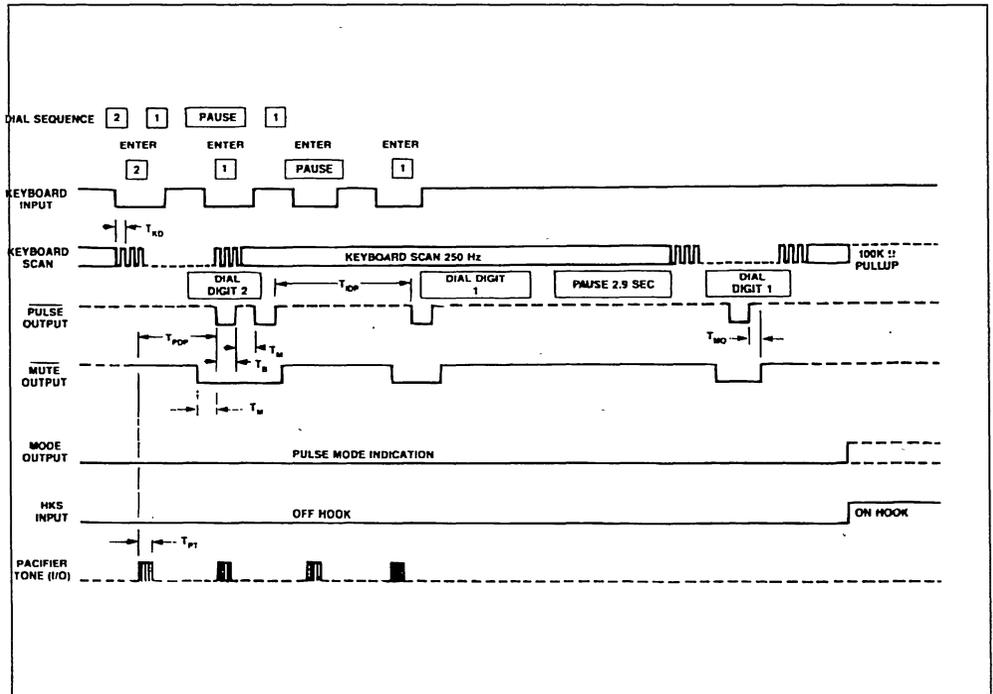
Figure 7 : Pulse And Tone Mode Timing.
