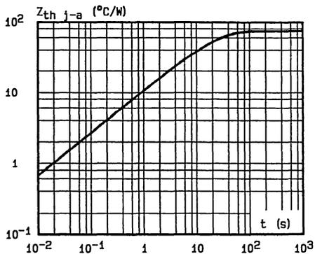
Fig. 6 - Transient thermal impedance junction-ambient versus pulse duration.
