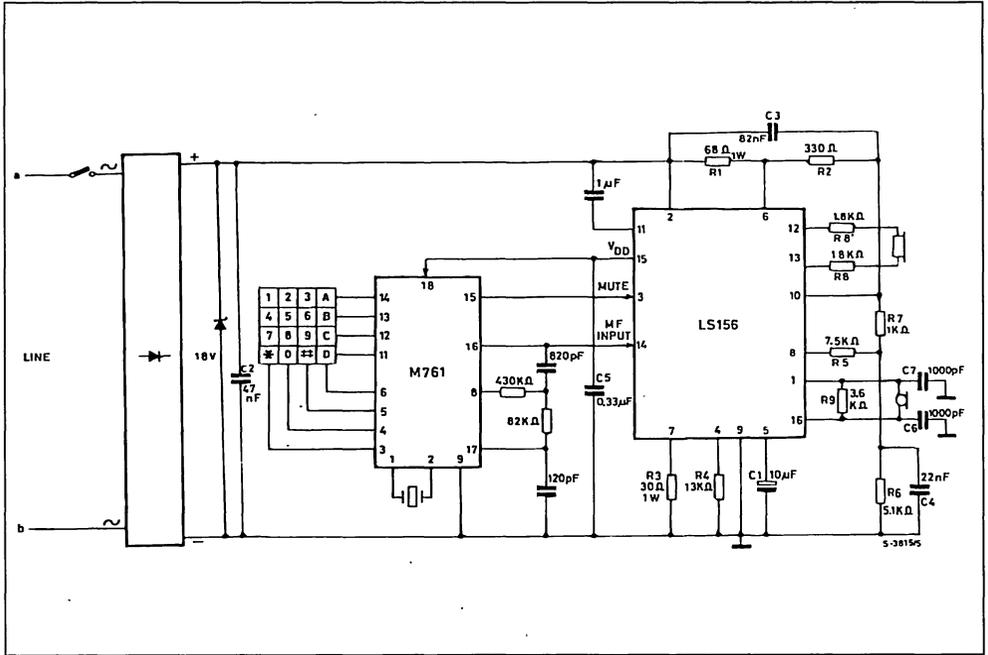
Figure 9 : Application Circuit with Multifrequency (EUROP I std.).
