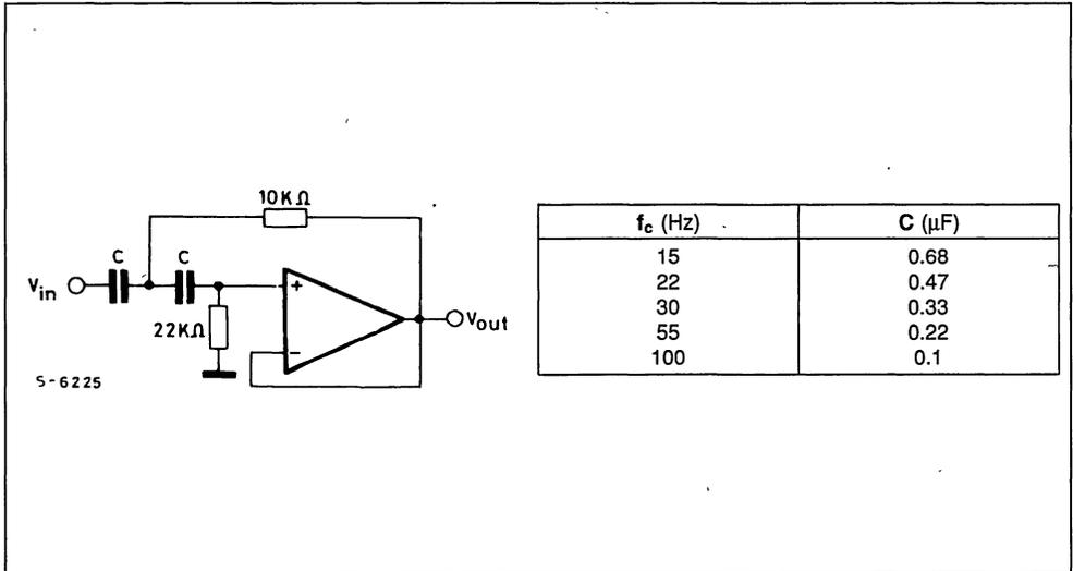
Figure 22 : High Cut Filter ( $G_v = 0$  dB).
