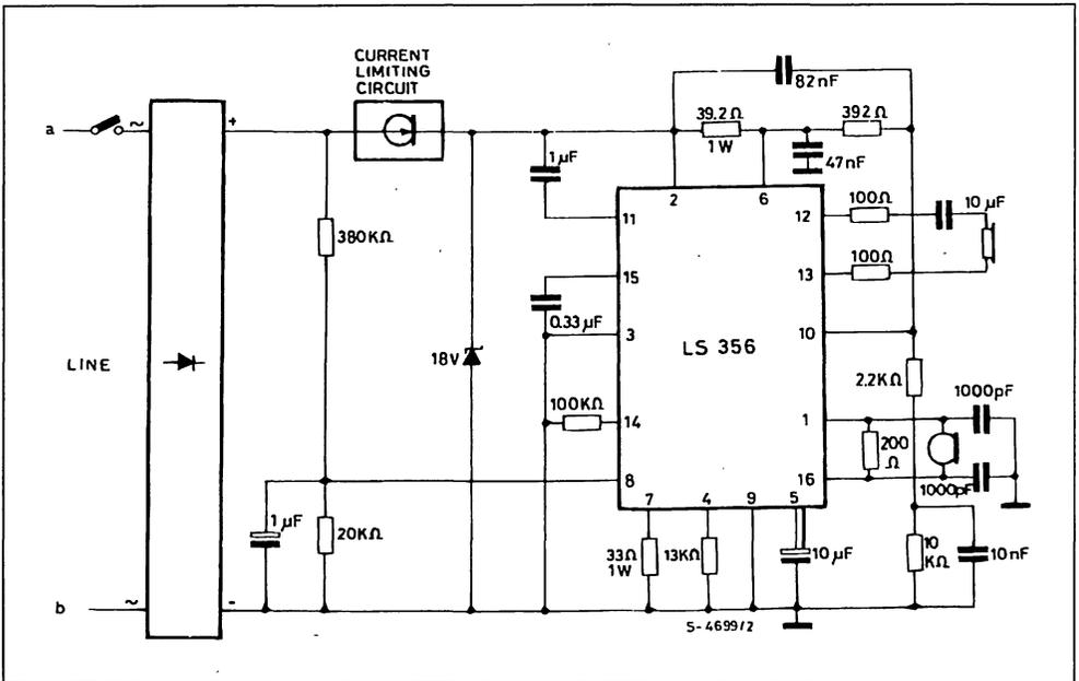
**Figure 14 : Application Circuit with Fixed Gain Operation.**
