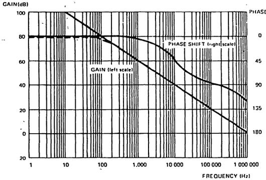
OPEN LOOP FREQUENCY RESPONSE AND PHASE SHIFT
