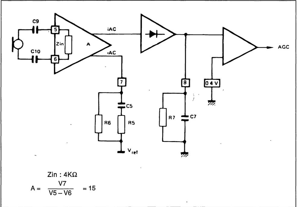
The first filter is generated by the capacitors on pins 5 and 6 ; the second filter by the R-C network on pin 7.
