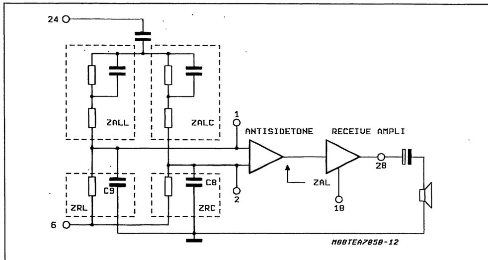
3.1. A.G.C. IN RECEIVE. As described for the transmission chain, also the receiving gains Gr, from pins 1 and 2 to pin 28, have a reduction of 6dB when Iline moves from 27mA to 42mA.
