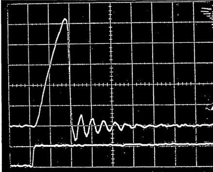
Figure 14 : Current limiting ( $V_S = 50V$ ,  $R_L = 100\Omega$ ).
