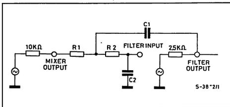
It is evident that R1 and R2 should be kept high to avoid undue influence of Mixer and Filter output impedances.
