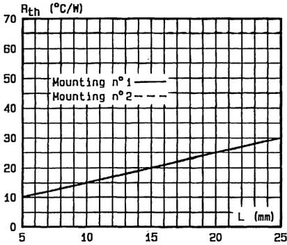
Fig. 5 - Thermal resistance versus lead length.
