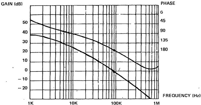
OPEN LOOP FREQUENCY RESPONSE AND PHASE SHIFT
