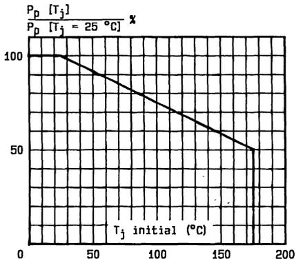
Fig.3 - Allowable power dissipation versus junction temperature.
