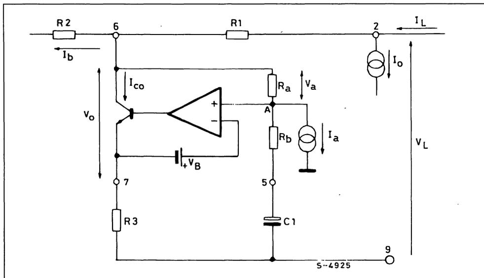
The difference  $I_L - I_o$  flows through the shunt regulator being  $I_b$  negligible.
