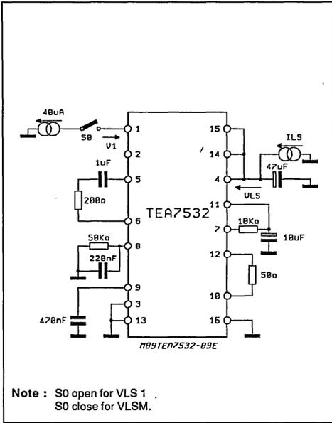
Figure 8 : Loudspeaker Amplifier : Gain/Distortion/Output Offset.
