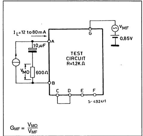
**ELECTRICAL CHARACTERISTICS** (refer to the test circuits,  $V_G = 1$  to  $2$  V,  $I_L = 12$  to  $80$  mA, S1 and S2 in (a),  $T_{amb} = -25$  to  $+50$  °C,  $f = 200$  to  $3400$  Hz, unless otherwise specified)
