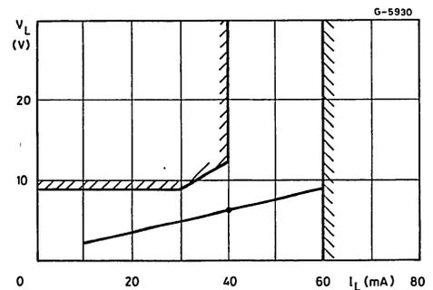
voltage also will go down. It is not recommended, though, to set the PBL3726 to DC voltages below 2.5V. If in some circumstances the DC characteristics of PBL3726 is too low, they can be raised by inserting an extra diode in series with the rectifier bridge as in fig. 14.
