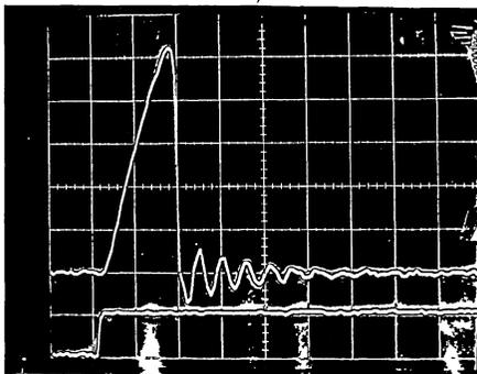
**Figure 14 :** Current limiting ( $V_S = 22V$ ,  $R_L = 100\Omega$ ).
