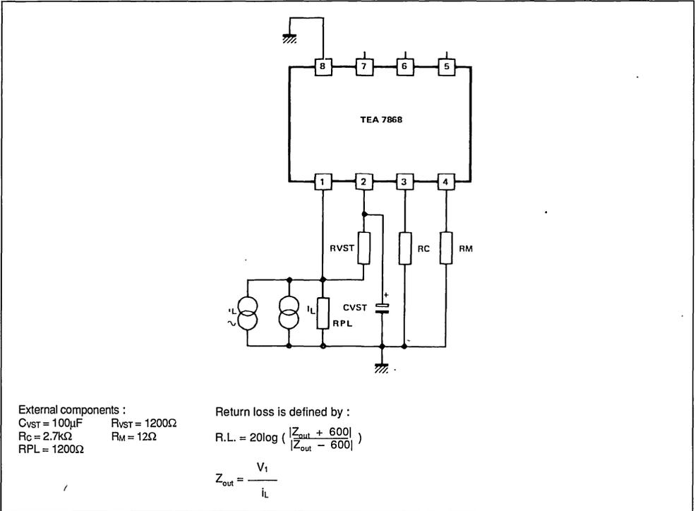
Figure 3 : Ring Detection Level and Impedance.
