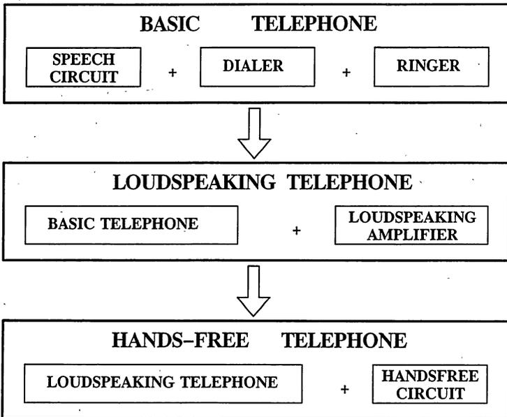
**MODULAR APPROACH.** The SGS-THOMSON telephone product range includes a basic, telephone kit for each national standard plus add-on function ICs that turn a basic phone into a feature phone.
