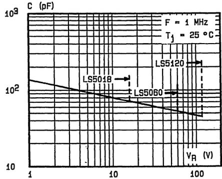
Fig.4 - Junction capacitance versus reverse applied voltage.
