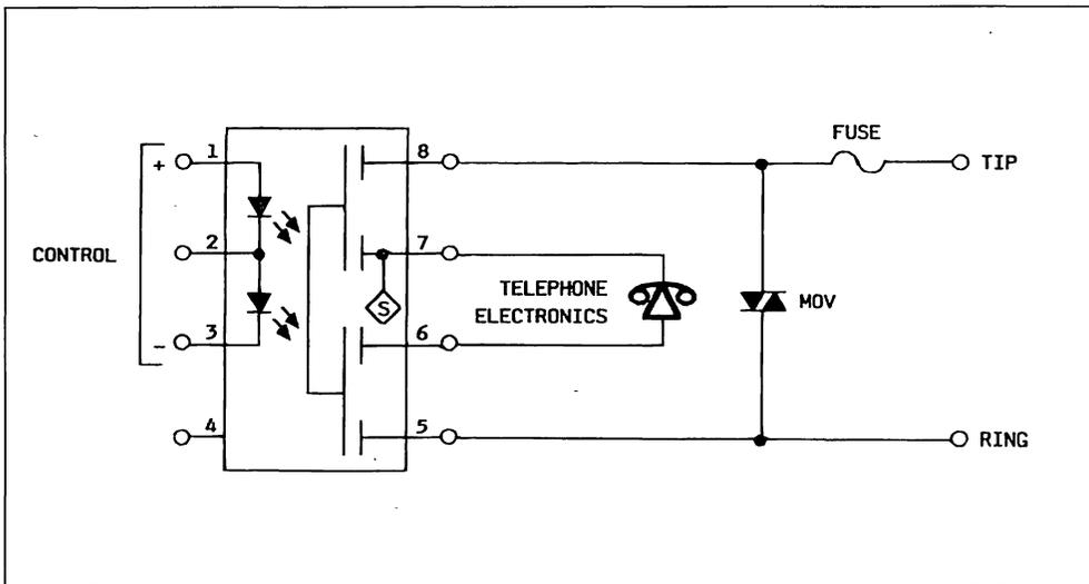
Figure 16 : Balanced Two-line Multiplexer Application.
