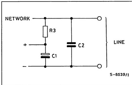
as in the example for British Telecom (fig. 12), this can also be achieved by copying the mathematical model of the desired impedance.
