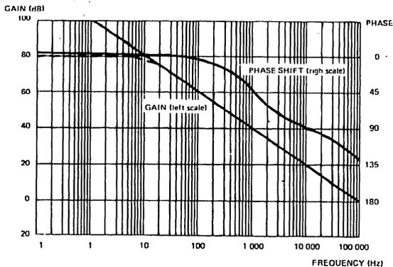
OPEN LOOP FREQUENCY RESPONSE AND PHASE SHIFT
