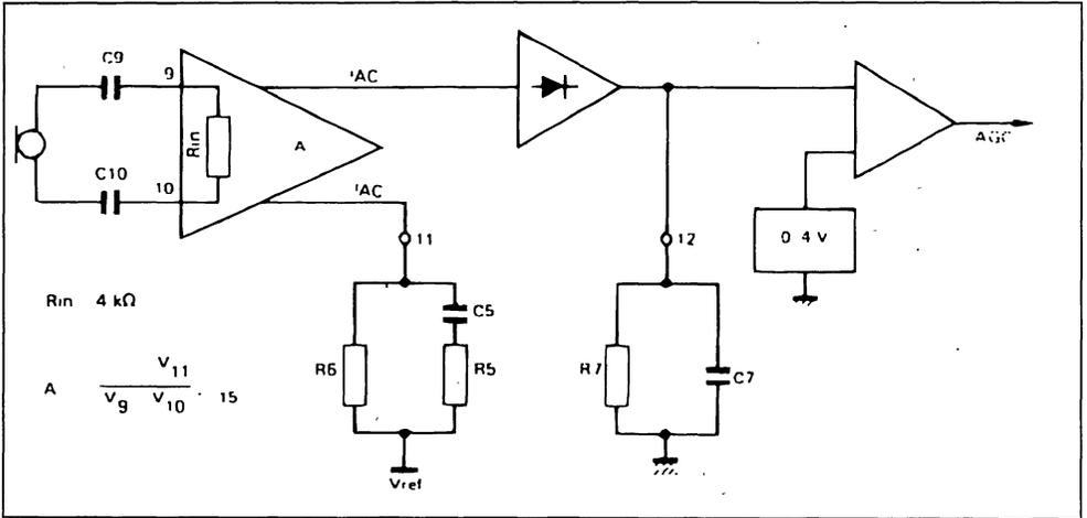
$$i_{AC} = \frac{V_{pin\ 11}}{Z_{pin\ 11}} \quad \text{with} \quad \frac{1}{Z_{pin\ 11}} = \frac{1}{R6} + \frac{1}{R5 + \frac{1}{C5j\omega}}$$
