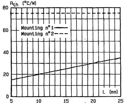
Fig. 2 - Thermal resistance versus lead length.
