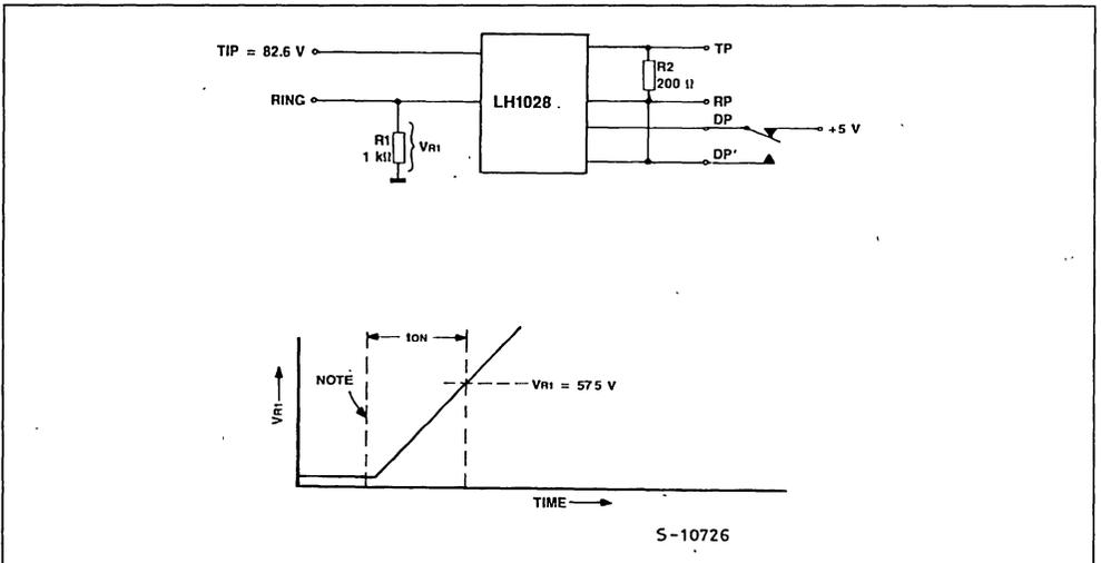
Figure 7 : Turn-off Time Test Method.
