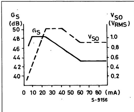
**Figure 6 :** DC Characteristic Measured between Line and GND.
