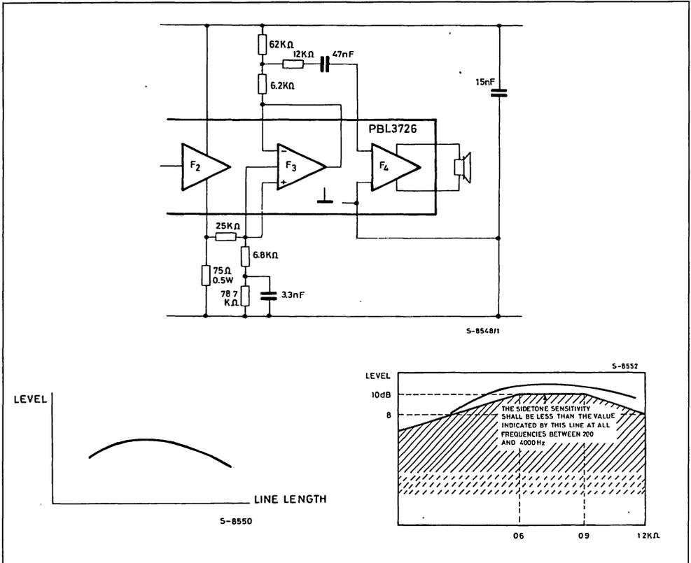
Figure 25 : Regulated Sidetone Network.
