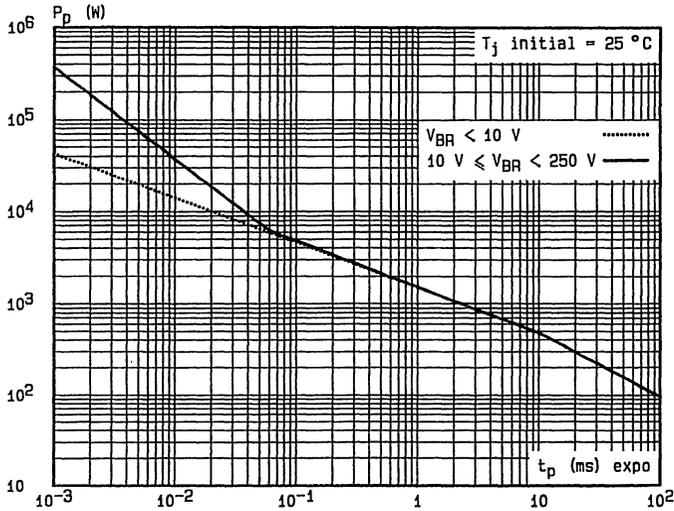
Fig.1 - Peak pulse power versus exponential pulse duration.
