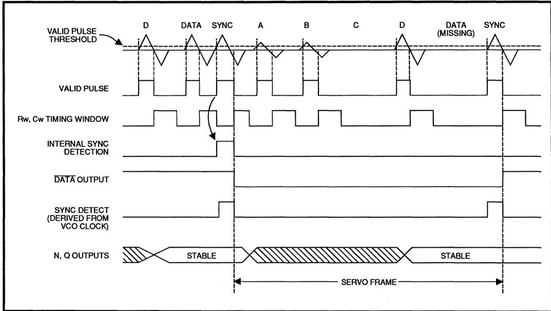
**FIGURE 5 : SYNC AND DATA PULSE DETECTION**
