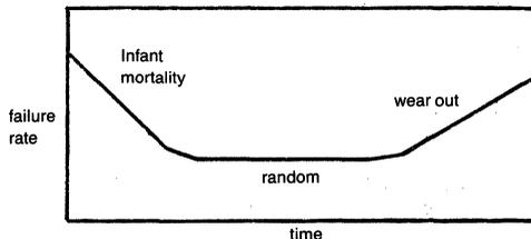
The bath tub curve above, implies that the useful life of the product extends until some basic design limitation is experienced. At SSI the Arrhenius Model is used to extrapolate a failure rate at an accelerated temperature test condition to a normal use temperature condition.
