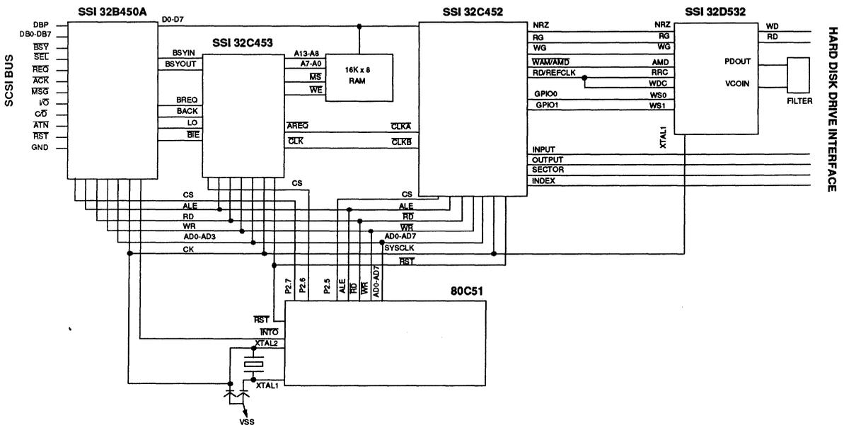
FIGURE 8: SCSI PERIPHERAL CONTROLLER CHIP SET
