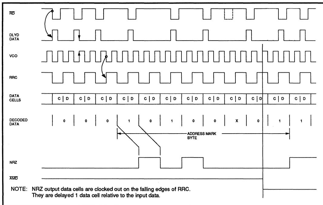
**FIGURE 2: Address Mark Detection and NRZ Waveform Diagram**
