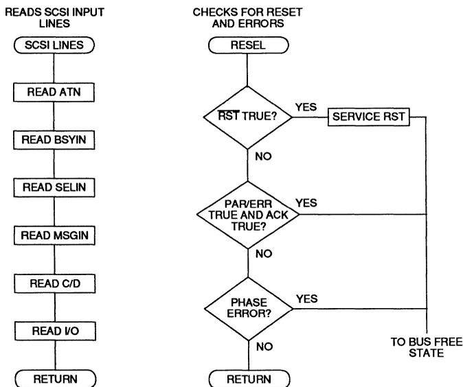
FIGURE 9: SCSI Background Routines Using SSI 32B451
