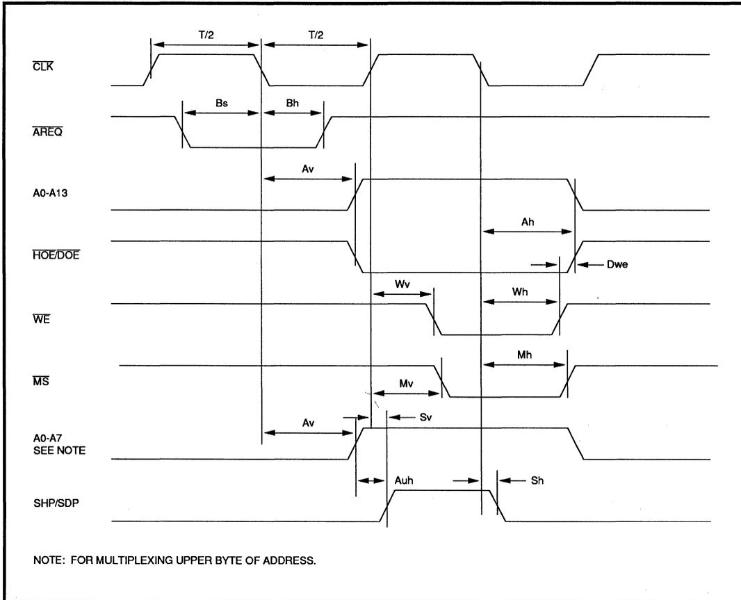
FIGURE 1: Peripheral Device to Buffer Interface Timing
