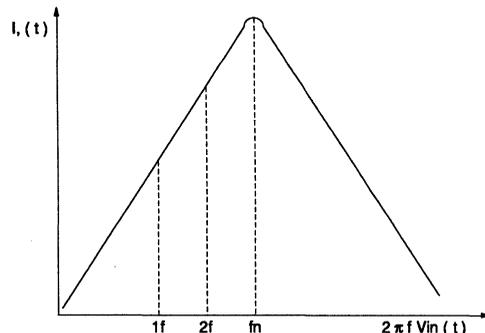
As with the previous Rex, Cex example, care must be taken to insure a 90° phase shift at the frequencies of interest (1f and 2f or 1.25 MHz and 2.5 MHz). This requirement is modified by any need to compensate for phase distortion caused by preceding signal processing.
