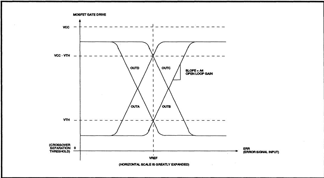
**FIGURE 4(B): SIMPLIFIED TRANSFER FUNCTION OF SSI 32H569
