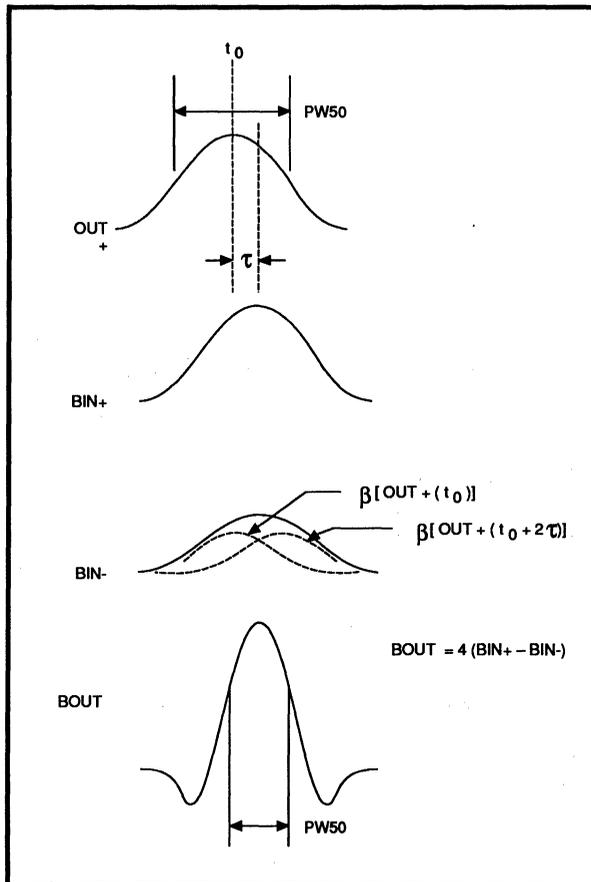
The  $PW50$  reduction is dependent on the amplitude of  $\tau$  and the attenuation ( $\beta$ ) between  $EF3$  and  $BIN-$ .
