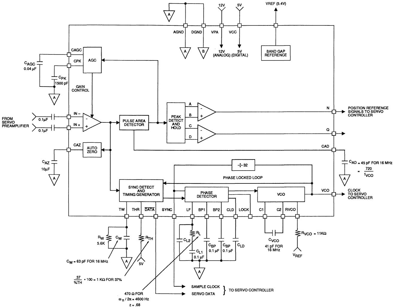
FIGURE 6: DESIGN EXAMPLE FOR 500 KHz FRAME RATE
