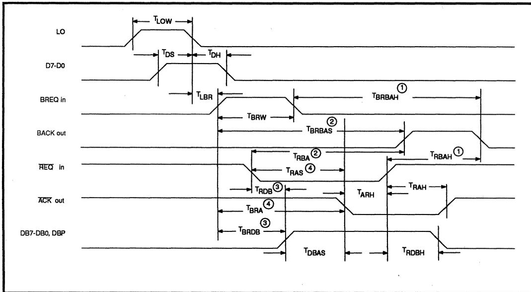
FIGURE 3: DATA TRANSFER INTERFACE TIMING - INITIATOR OUT
