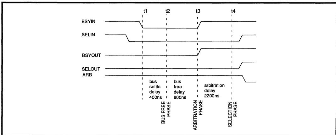
FIGURE 7: SSI 32C453 SCSI Arbitration Logic Timing
