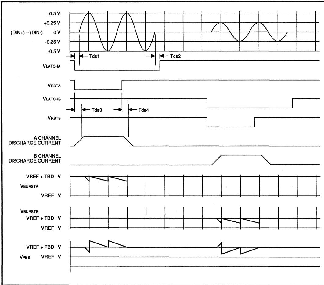
FIGURE 4: Servo Read Mode II Timing Diagram
