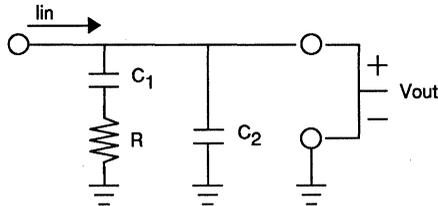
The role of C1 is as an integrating element. The larger this capacitance, the longer the acquisition time; the smaller the capacitance, the greater the ability to track high frequency jitter. The resistor R reduces the phase shift induced by C1. The capacitor C2 will suppress high frequency transients and will have minimal effect on the loop response if it is small relative to C1 (typically  $C_2 = C_1/10$ )
