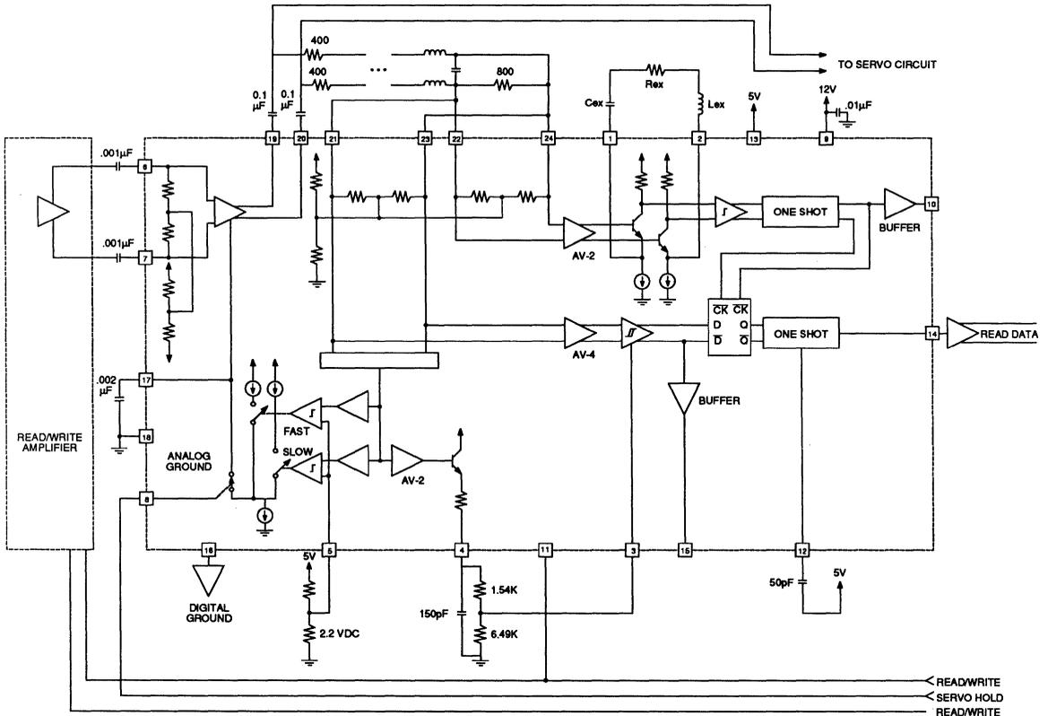
NOTE: Circuit traces for the 12V bypass capacitor and the AGC Hold Capacitor should be as short as possible with both capacitors returned to the Analog Ground Pin.
