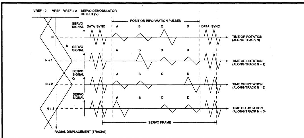
FIGURE 3: PRE-RECORDED SERVO SIGNAL AND SERVO DEMODULATOR OUTPUT VS. RADIAL DISPLACEMENT
