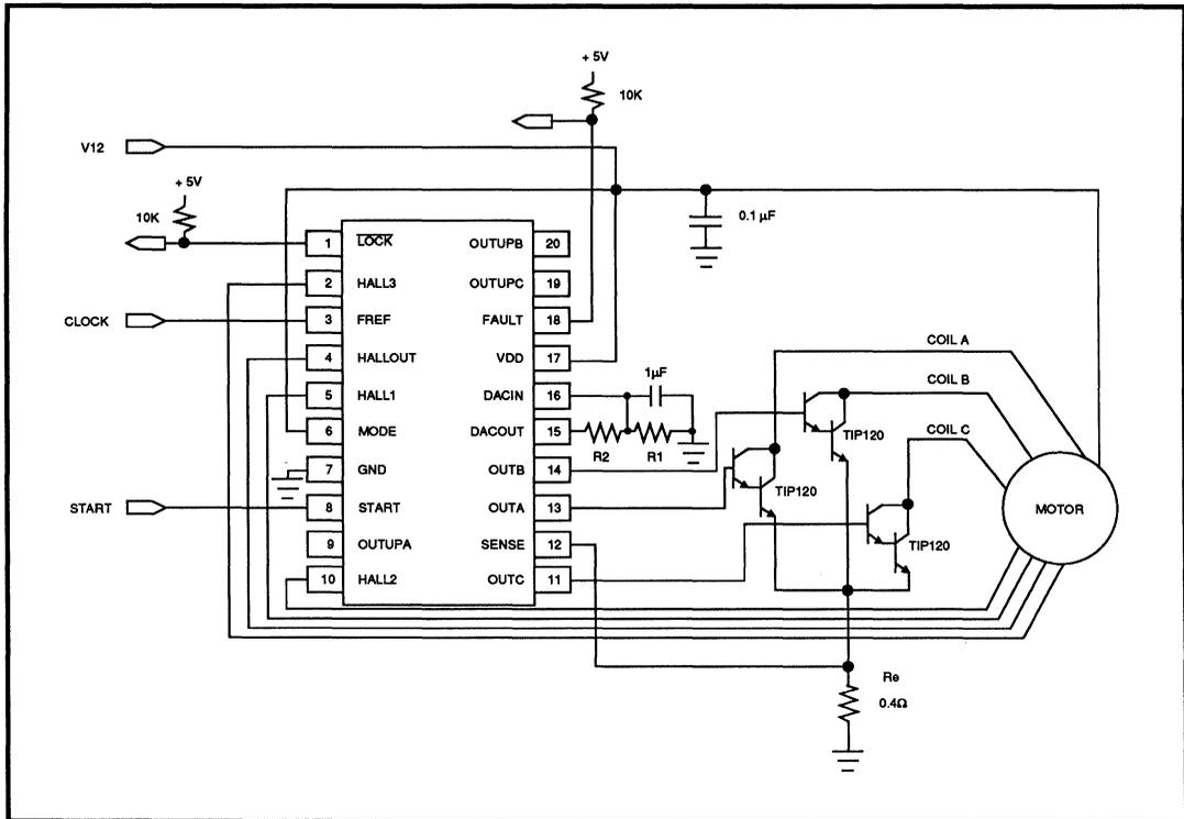
Typical Three-Phase, 8-Pole, Unipolar,
