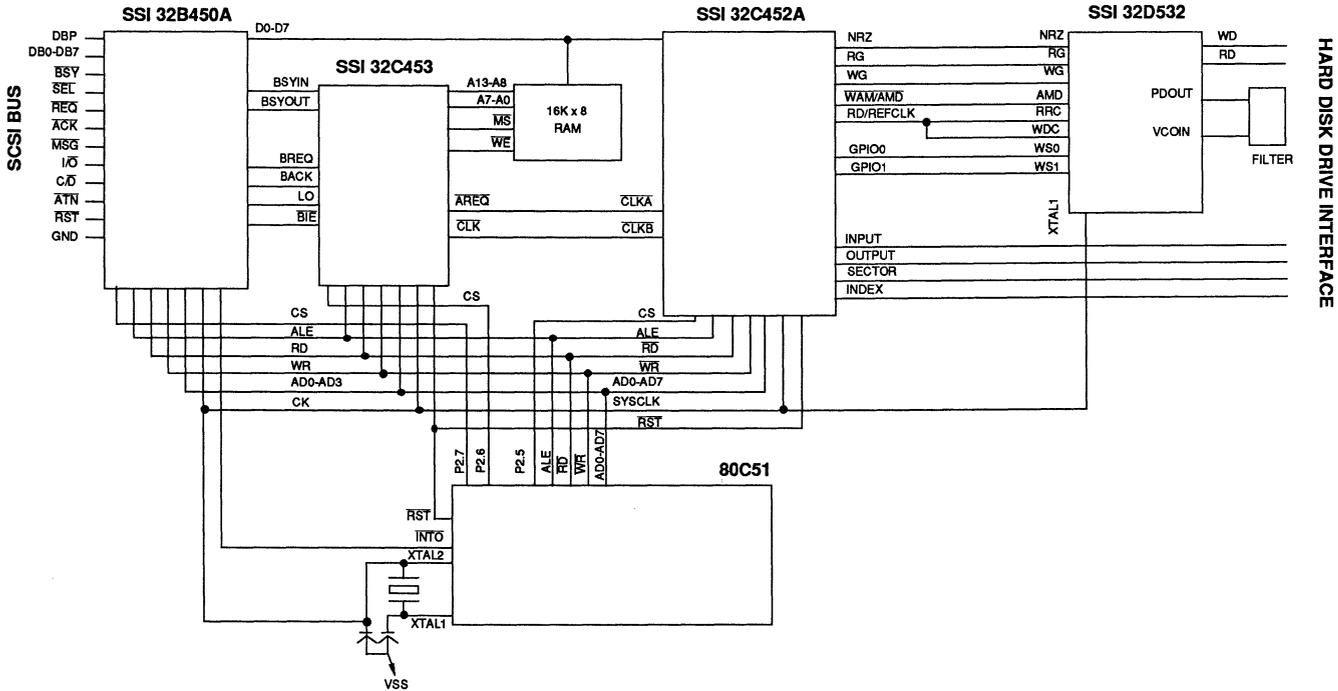
FIGURE 8: SCSI PERIPHERAL CONTROLLER CHIP SET
