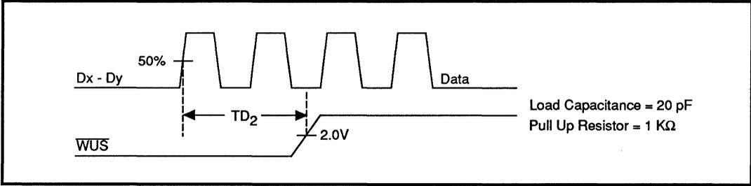
FIGURE 2: Unsafe to Safe Timing
