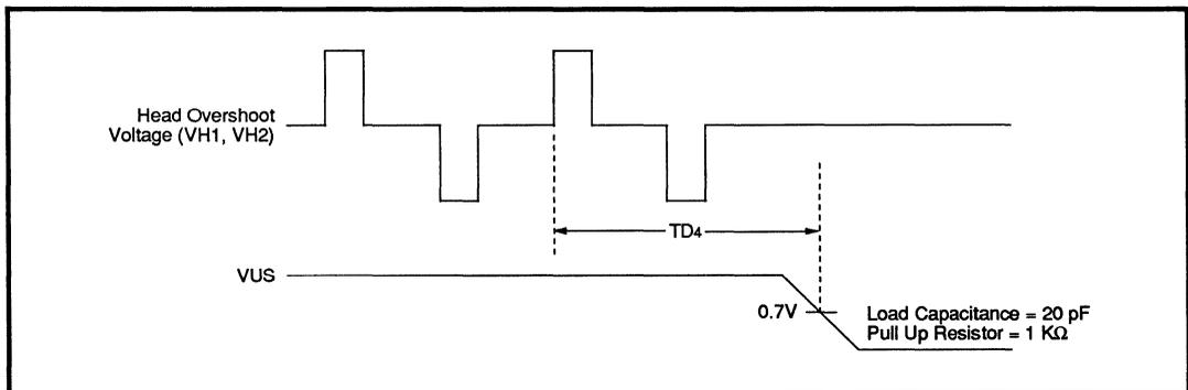
FIGURE 2B: Safe to Unsafe Timing
