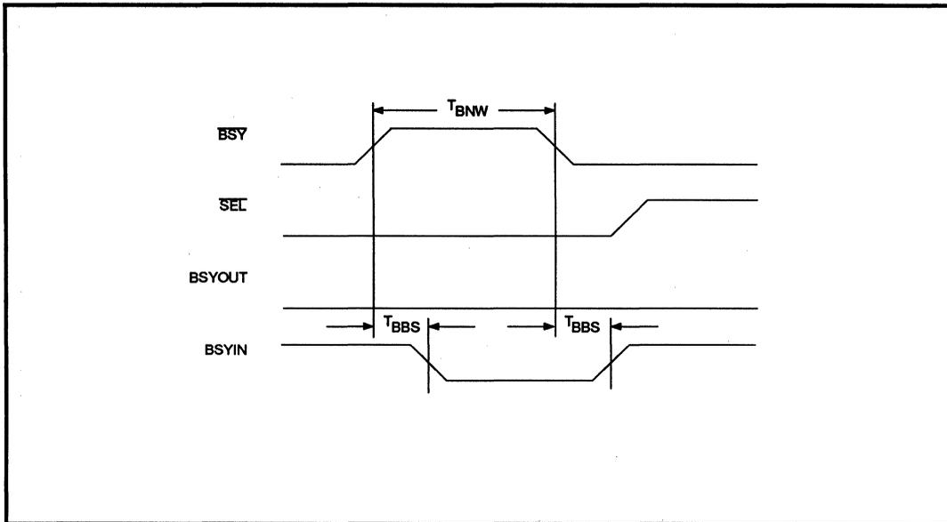
FIGURE 7: BSYIN AND BSYOUT TIMING - SSI 32B450A NOT ARBITRATING
