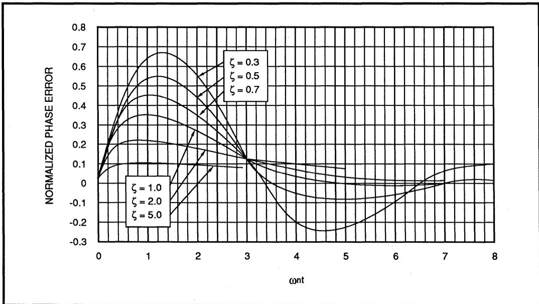
FIGURE 14: TRANSIENT PHASE ERROR  $\theta_e(t)$  DUE TO A STEP IN FREQUENCY  $\Delta\omega$
