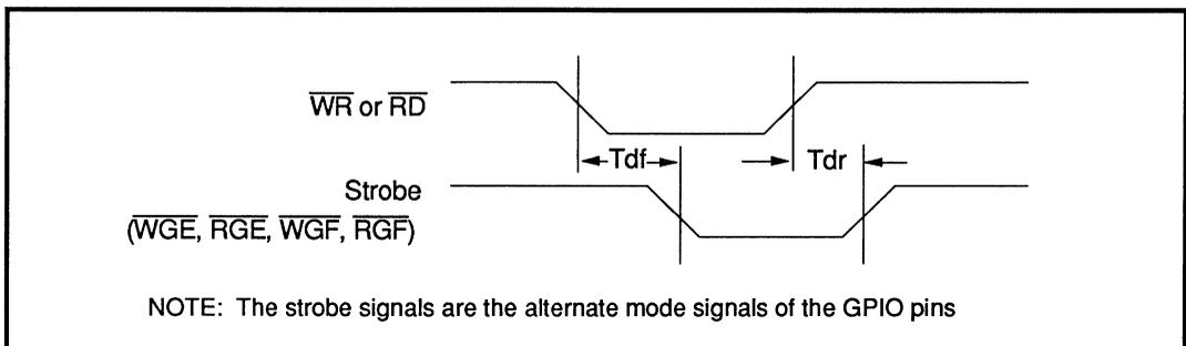
FIGURE 7: ADDRESS DECODE 6E AND 6F TIMING
