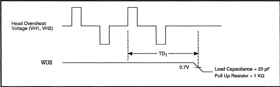
FIGURE 1: Safe to Unsafe Timing
