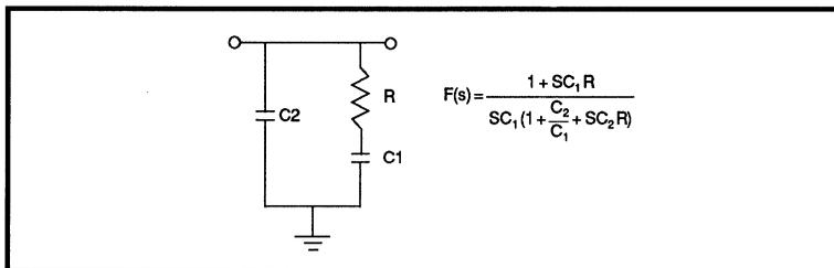
FIGURE 6 : Loop Filter Example
