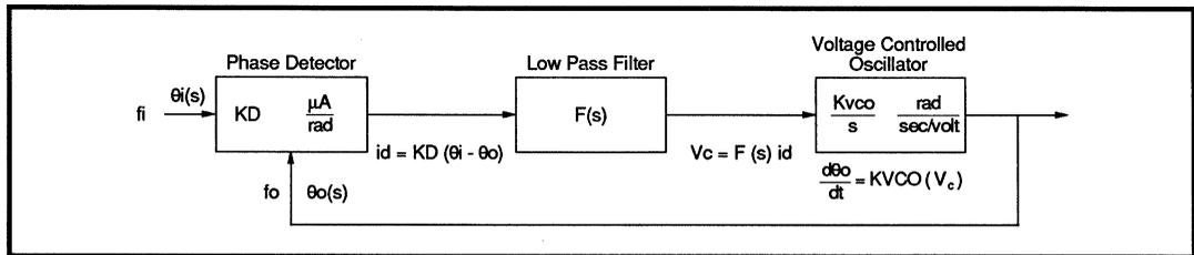
FIGURE 5 : Phase Locked Loop
