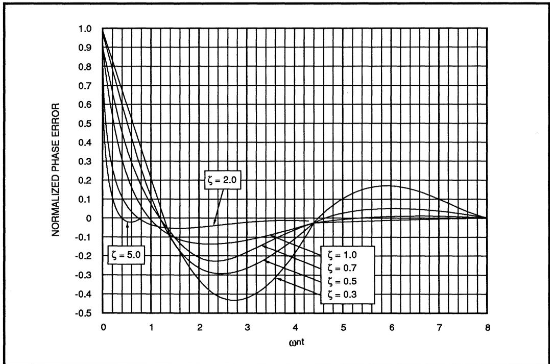
FIGURE 13: TRANSIENT PHASE ERROR  $\theta_e(t)$  DUE TO A STEP IN PHASE  $\Delta\theta$
