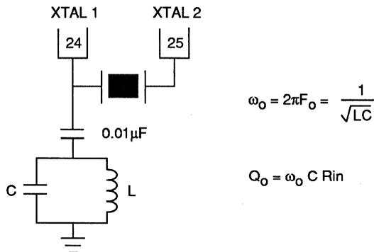
The typical input impedance looking into XTAL1 is approximately  $R_{in} = 250\Omega$ . It is recommended to design the value of  $Q_0$  at approximately 10 to 15. Therefore, a resonant frequency of  $F_0 = 20$  MHz would result in  $L \cong 0.16$   $\mu$ H and  $C \cong 380$  pF.
