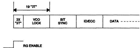
In hard sector operation the SSI 32D536's Address Mark Detection circuitry is not enabled by a AMENB signal and  $\overline{AMD}$  remains inactive. A hard sector read operation does not require an address mark search but starts with a preamble search as with soft sector and sequences identically. In all respects, with exception to the address mark search sequence, hard sector read operation is the same as soft sector read.
