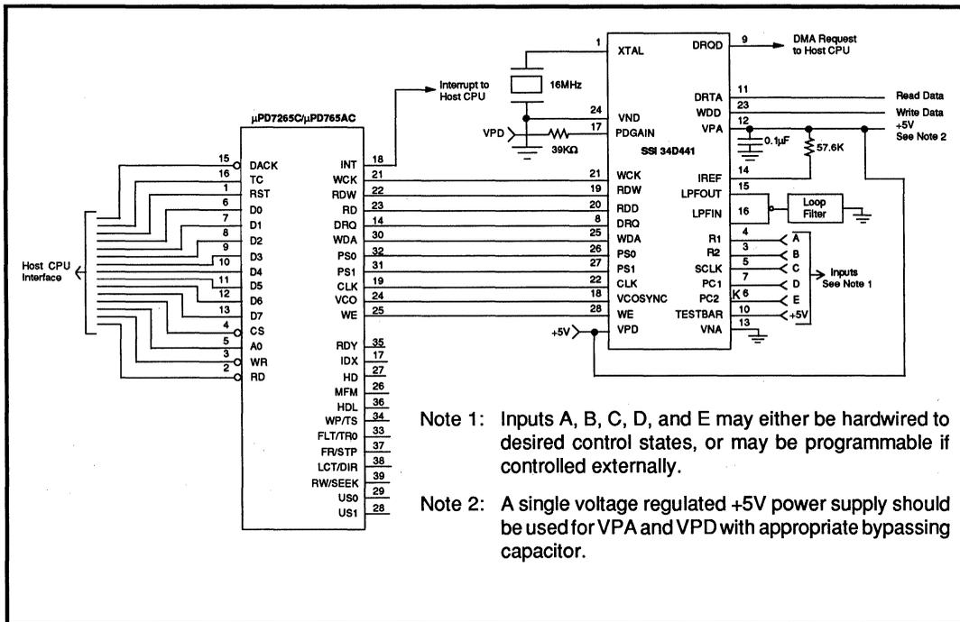
FIGURE 5: Application Diagram
