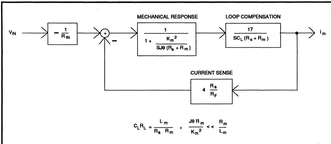
**FIGURE 4(B): SIMPLIFIED TRANSFER FUNCTION OF SSI 32H569
