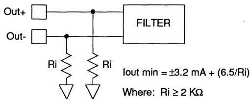
One filter for both amplitude (DIN+/- input) and time (CIN+/- input) channels, or a separate filter for each may be used. If two filters are used, attention must be paid to time delays so that each channel is timed properly. A multi-pole Bessel filter is typically used for its linear phase or constant group delay characteristics.
