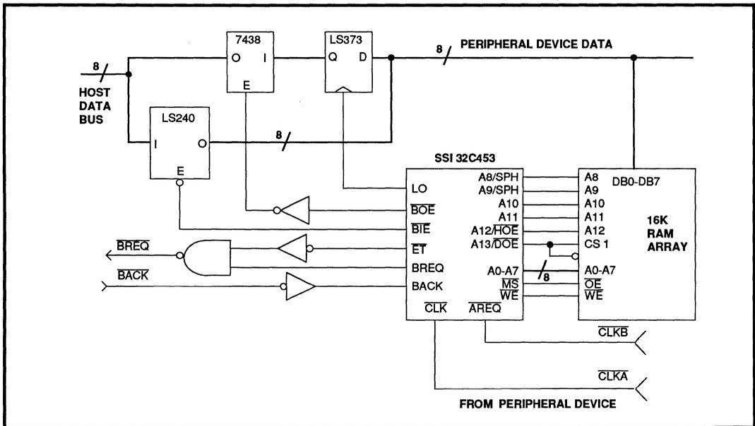
FIGURE 9: Direct Addressing Mode Example - 14 Address Lines
