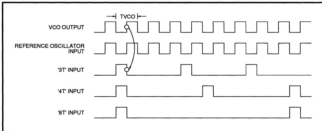
**FIGURE 12: RELATIONSHIP OF VCO OUTPUT TO PHASE DETECTOR INPUT**
