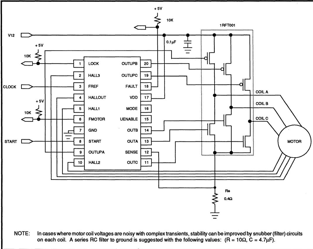
**TYPICAL THREE-PHASE, 4-POLE, BIPOLAR,
