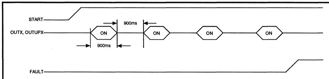
FIGURE 2: Jammed Platter Sequence
