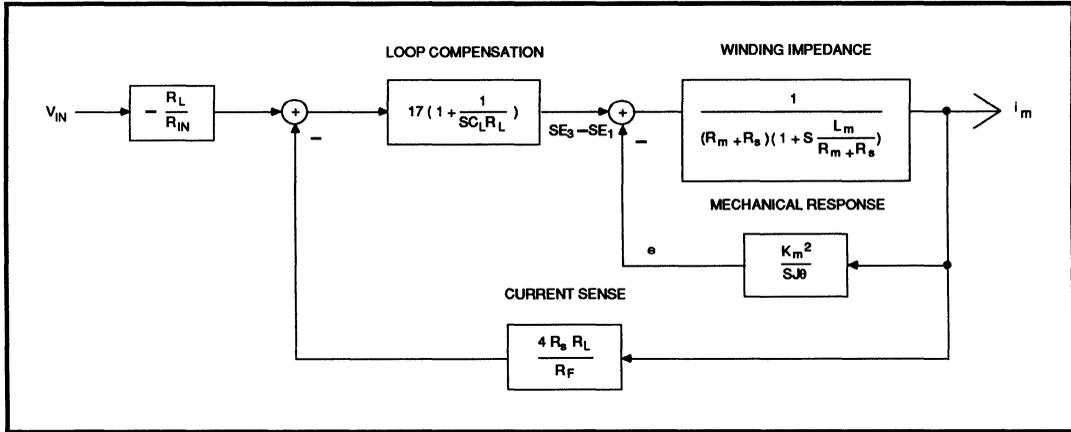
**FIGURE 4(A): TRANSFER FUNCTION OF SSI 32H569
