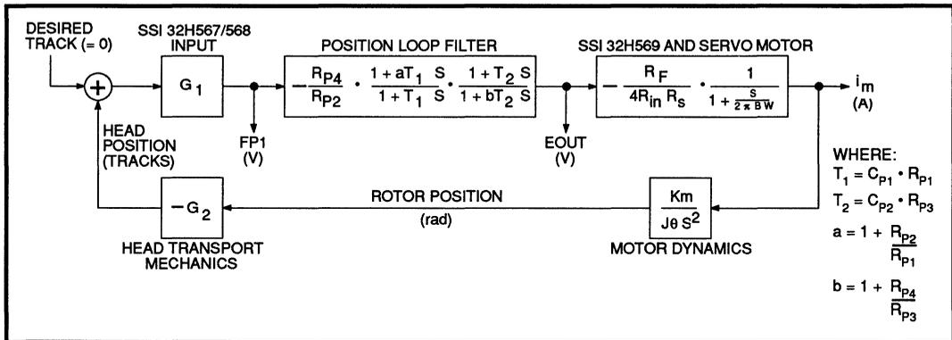
FIGURE 8(a): SYSTEM TRANSFER FUNCTION IN TRACK MODE
