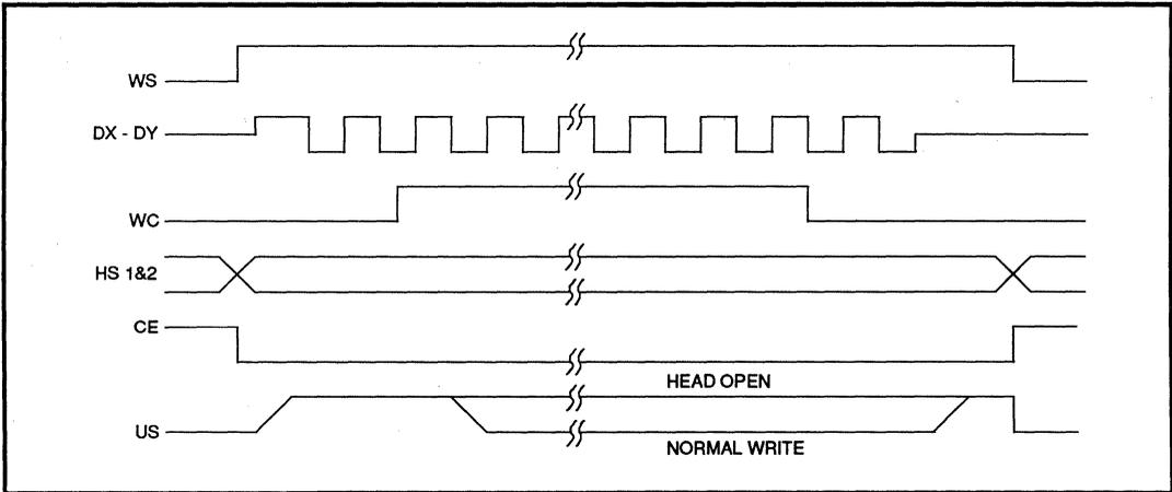
**FIGURE 1: Write Mode Timing System**
