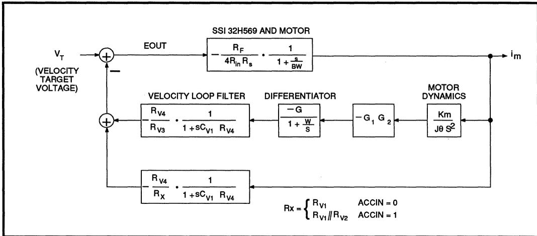
FIGURE 10(a): TRANSFER FUNCTION OF SSI 32H568 IN SEEK MODE
