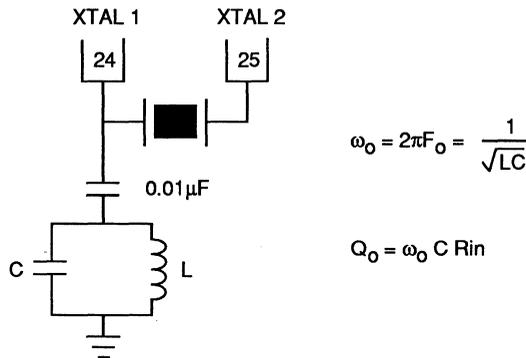
The typical input impedance looking into XTAL1 is approximately  $R_{in} = 250\Omega$ . It is recommended to design the value of  $Q_0$  at approximately 10 to 15. Therefore, a resonant frequency of  $F_0 = 20\text{MHz}$  would result in  $L \cong 0.16\mu\text{H}$  and  $C \cong 380\text{pF}$ .
