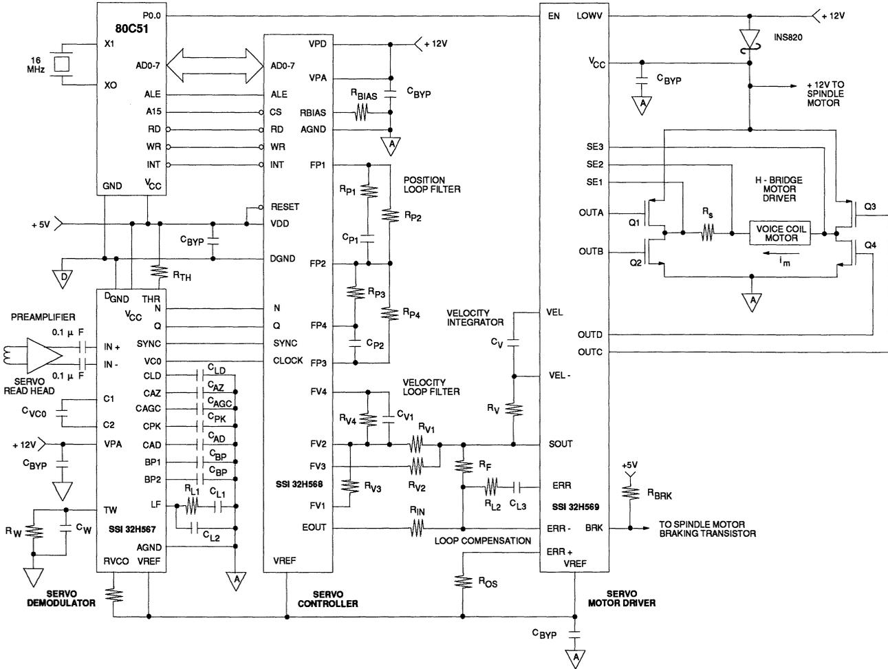
FIGURE 7: COMPLETE EXAMPLE OF SERVO PATH ELECTRONICS USING SSI 32H567/568/569 CHIP SET
