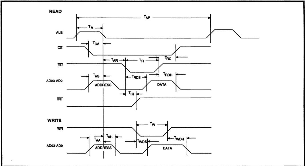
**FIGURE 8: MICROPROCESSOR INTERFACE TIMING**
