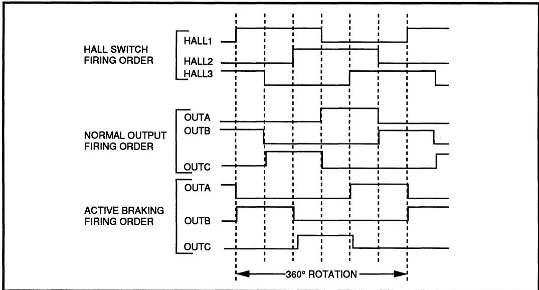
FIGURE 1: HALL Switch/Driver Timing Relationship
