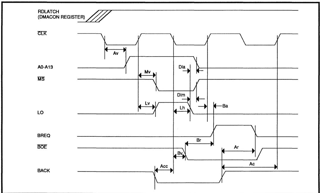
FIGURE 2: Buffer toHost Interface Timing
