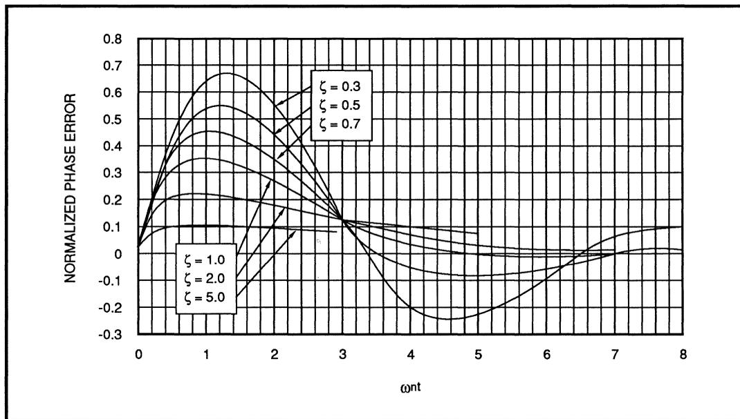
FIGURE 15: TRANSIENT PHASE ERROR  $\theta_e(t)$  DUE TO A STEP IN FREQUENCY  $\Delta\omega$
