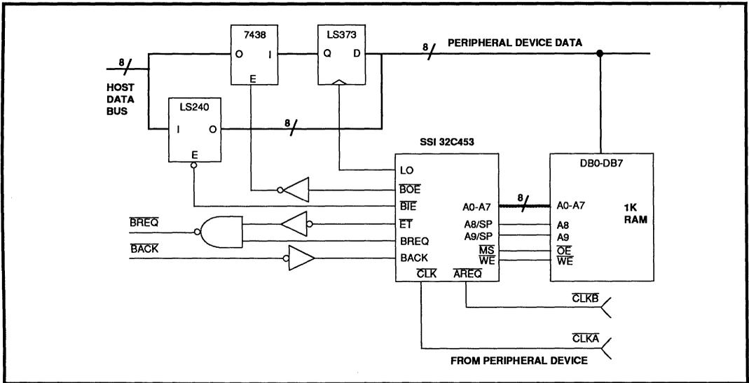
FIGURE 8: Direct Address Mode Example - 10 Address Lines
