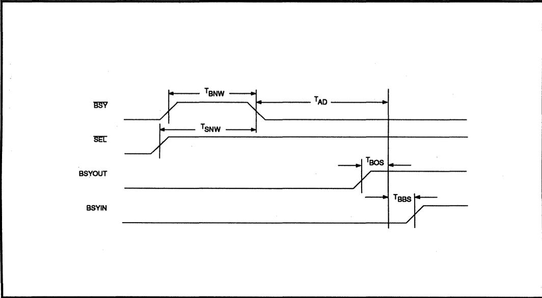
FIGURE 6: BSYIN AND BSYOUT TIMING - SSI 32B450A AND OTHER SCSI DEVICES ARBITRATING
