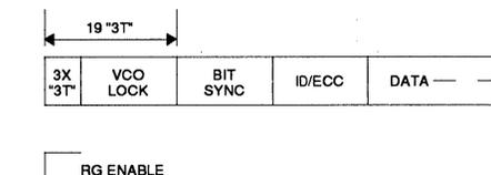
In hard sector operation a low AMENB disables the SSI 32D537's Address Mark Detection circuitry and AMD remains inactive. A hard sector read operation does not require an address mark search but starts with a preamble search as with soft sector and sequences identically. In all respects, with exception to the address mark search sequence, hard sector read operation is the same as soft sector read.
