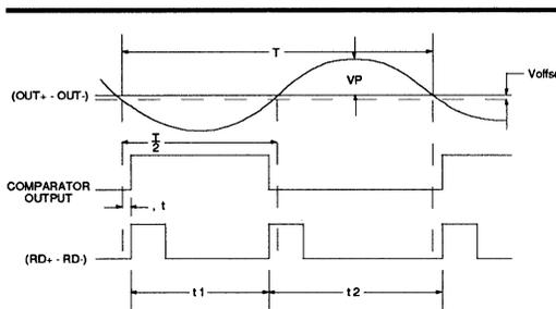
FIGURE 4: Effect of Comparator Offset on Output Waveform
