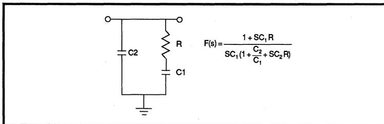
FIGURE 6 : Loop Filter Example
