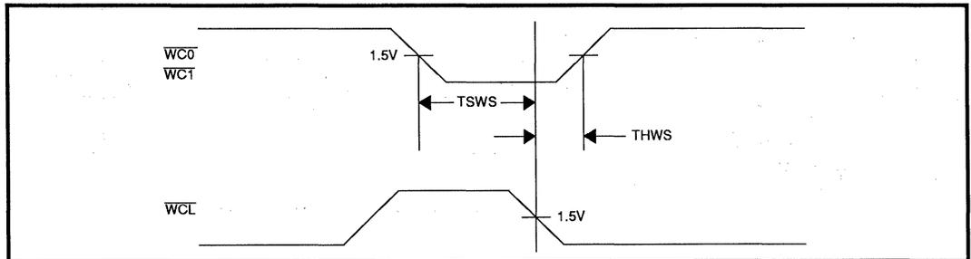
FIGURE 5: Control Timing
