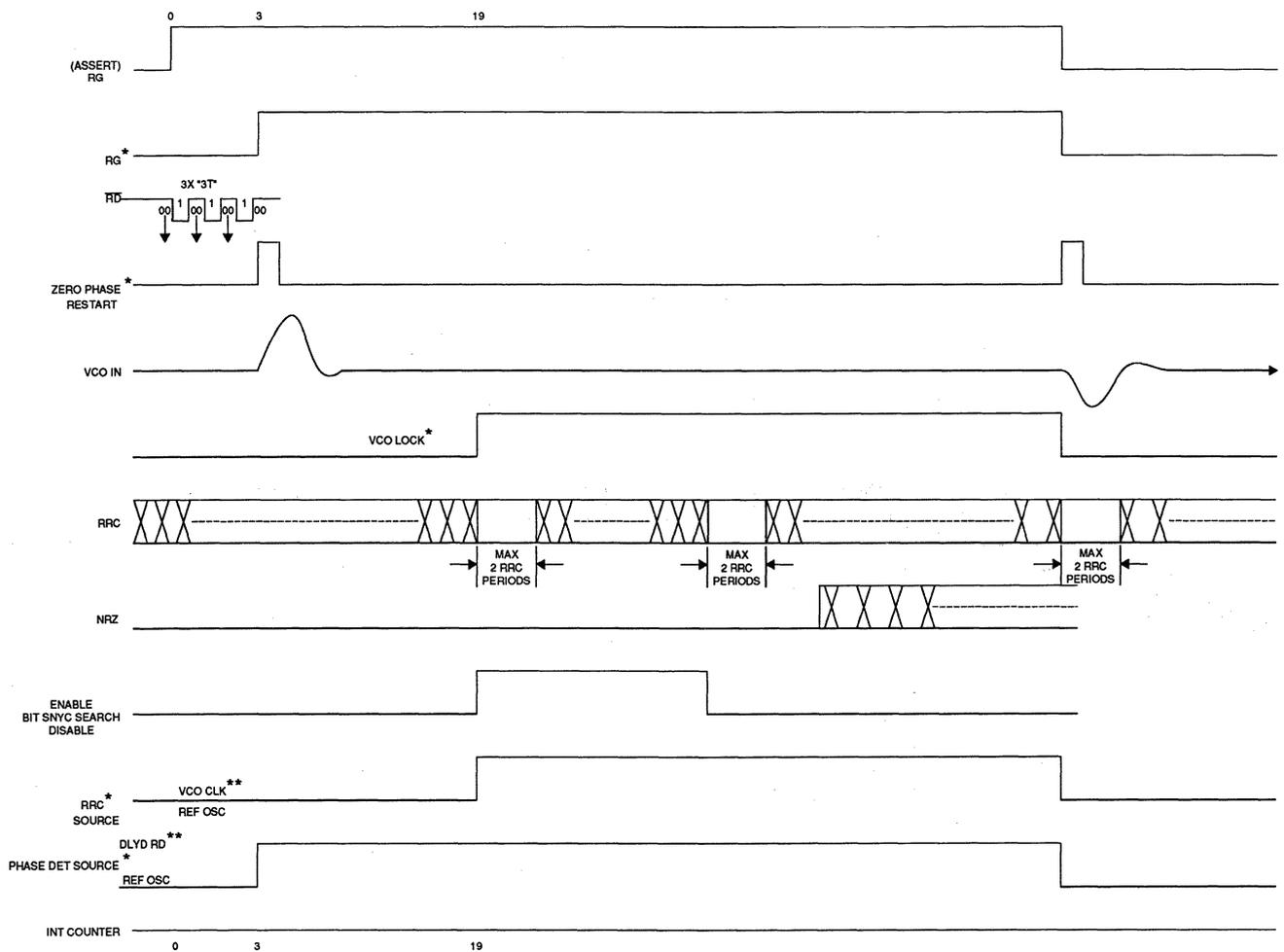
**FIGURE 7: Read Mode Locking Sequence (Soft and Hard Sector)**
