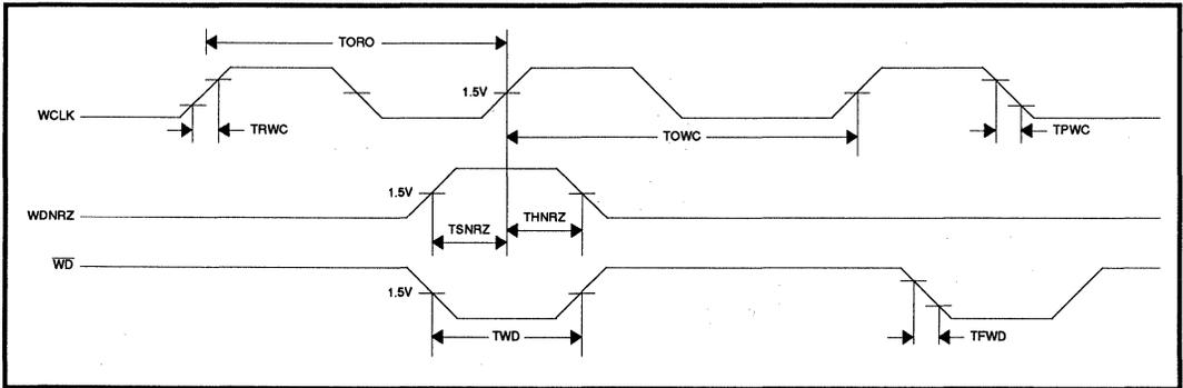
FIGURE 4: Write Timing
