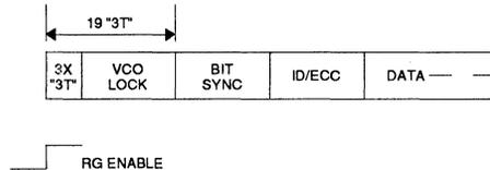
In hard sector operation a low AMENB disables the SSI 32D5362's Address Mark Detection circuitry and AMD remains inactive. A hard sector read operation does not require an address mark search but starts with a preamble search as with soft sector and sequences identically. In all respects, with exception to the address mark search sequence, hard sector read operation is the same as soft sector read.
