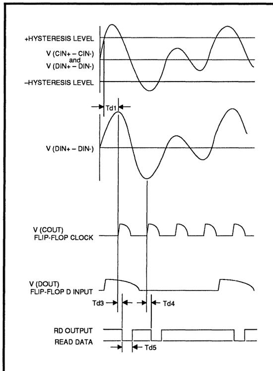
FIGURE 2: Timing Diagram
