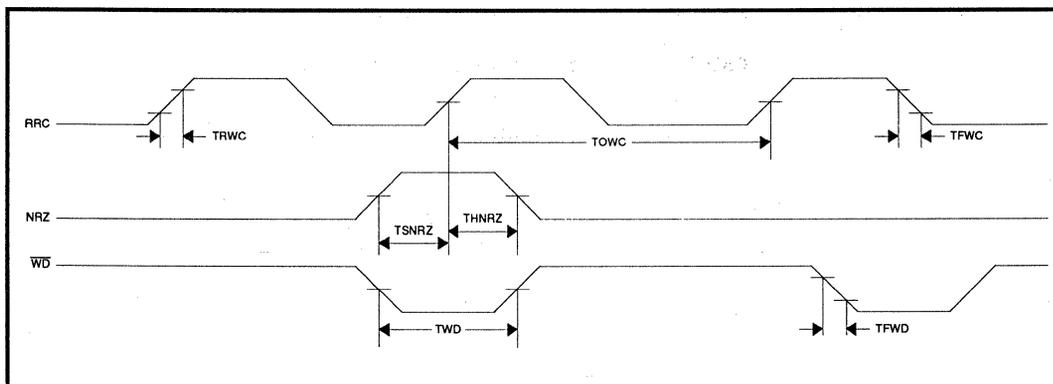
FIGURE 12: Write Timing
