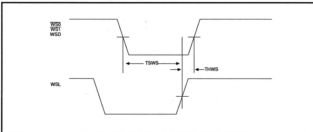
**FIGURE 11: Control Timing**
