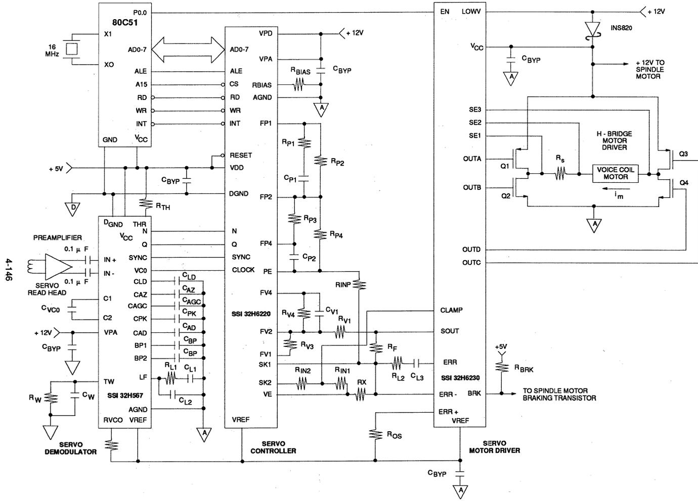
FIGURE 8: Complete Example of Servo Path Electronics Using the SSI 32H567/6220/6230 Chip Set
