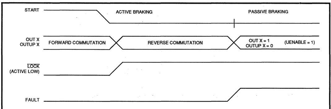
FIGURE 3: Active Braking Sequence
