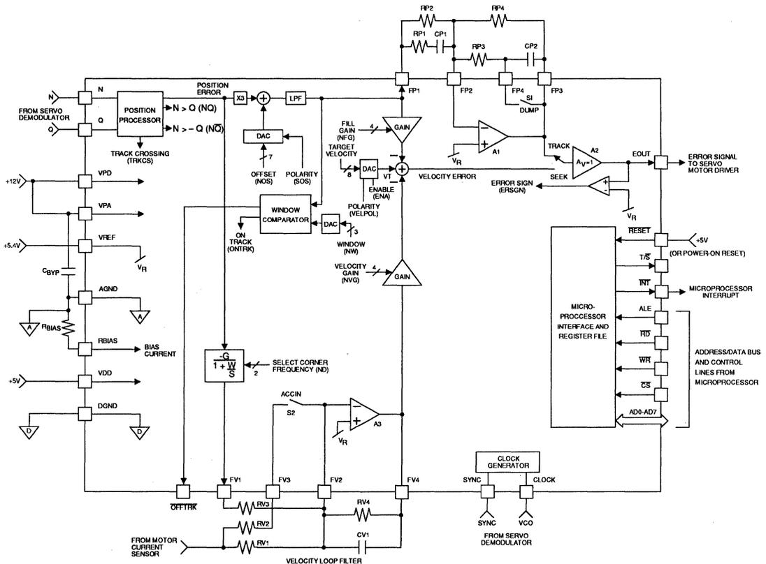
FIGURE 2: SSI 32H568 Typical Application
