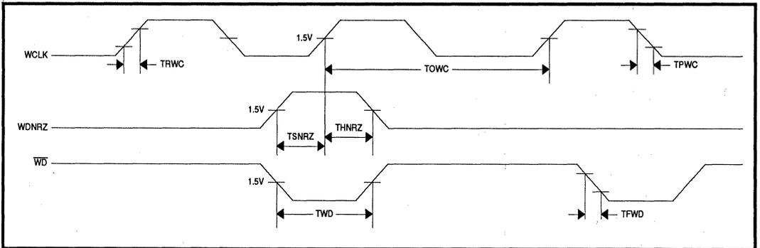
FIGURE 4: Write Timing
