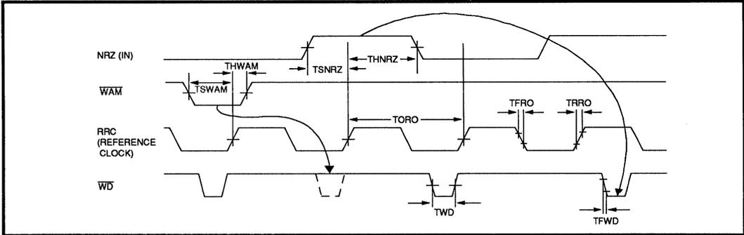
**FIGURE 9: Write Timing**
