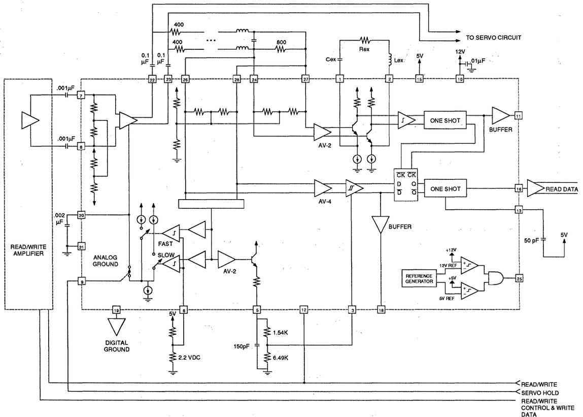
NOTE: Circuit traces for the 12V bypass capacitor and the AGC Hold capacitor should be as short as possible with both capacitors returned to the Analog Ground Pin. Component values, where given, are for a 5Mbit/s system.
