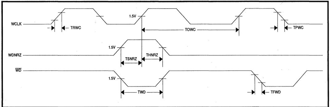
FIGURE 4: Write Timing
