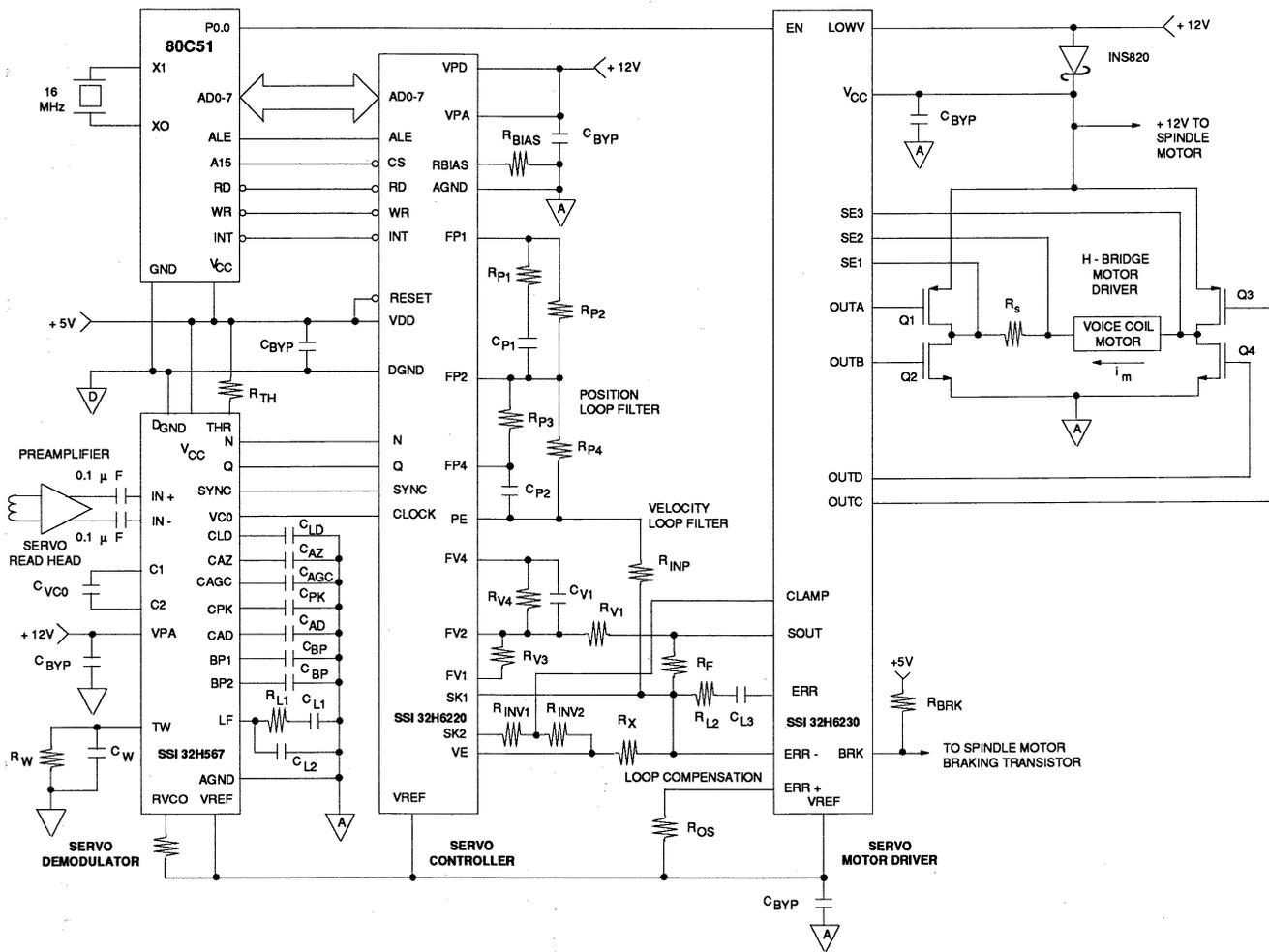
FIGURE 9: Complete Example of Servo Path Electronics Using SSI 32H567/6220/6230 Chip Set
