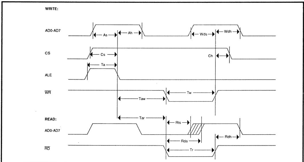
**FIGURE 4: Microprocessor Interface**
