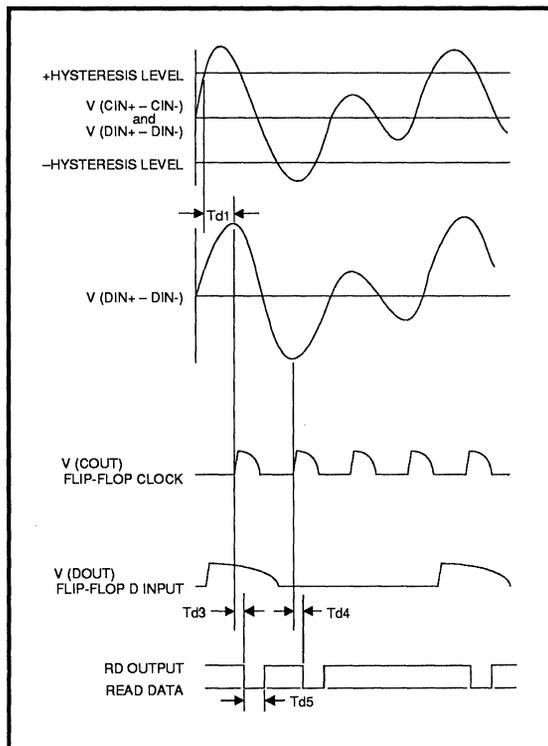
**FIGURE 2: Timing Diagram**
