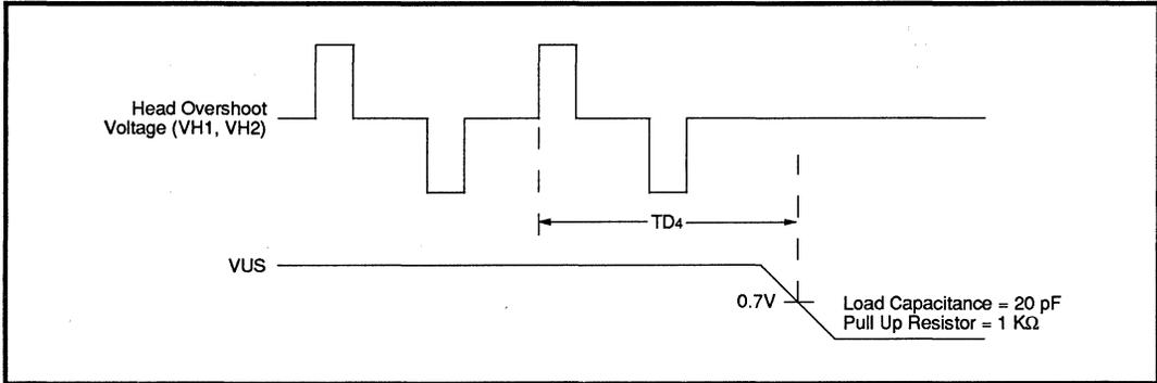
FIGURE 2B: Safe to Unsafe Timing
