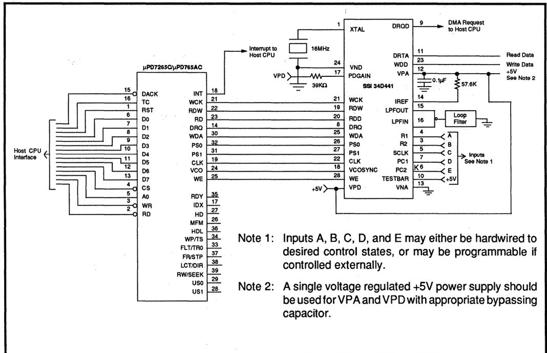
FIGURE 5: Application Diagram
