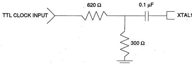
The signal amplitude into XTAL1 should be attenuated to approximately 1.0 Vp-p; this will insure that the transients associated with TTL switching characteristics won't couple into the SSI 32D5321/22 and degrade performance.
