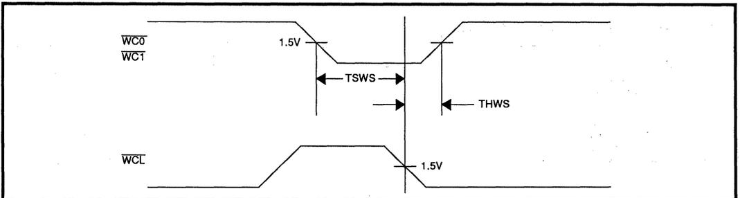
FIGURE 5: Control Timing
