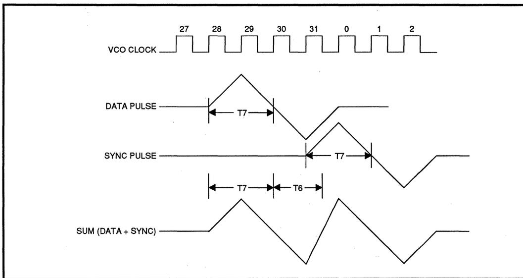
FIGURE 6 : Servo Writer Data-Sync Pulse Generation
