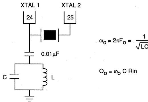
The typical input impedance looking into XTAL1 is approximately  $R_{in} = 250\Omega$ . It is recommended to design the value of  $Q_0$  at approximately 10 to 15. Therefore, a resonant frequency of  $F_0 = 20\text{MHz}$  would result in  $L \cong 0.16\mu\text{H}$  and  $C \cong 380\text{pF}$ .
