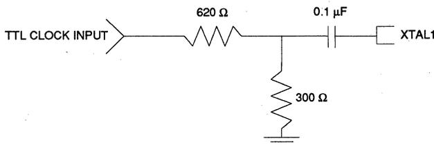
The signal amplitude into XTAL1 should be attenuated to approximately 1.0 V<sub>p-p</sub>; this will insure that the transients associated with TTL switching characteristics won't couple into the SSI 32D536 and degrade performance.
