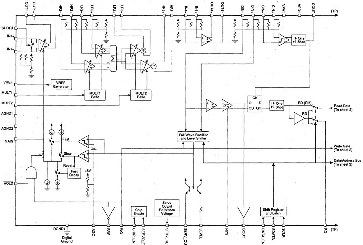
SSI 32P4620 Block Diagram - Sheet 1
