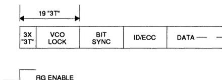
In hard sector operation a low AMENB disables the SSI 32D536's Address Mark Detection circuitry and  $\overline{AMD}$  remains inactive. A hard sector read operation does not require an address mark search but starts with a preamble search as with soft sector and sequences identically. In all respects, with exception to the address mark search sequence, hard sector read operation is the same as soft sector read.
