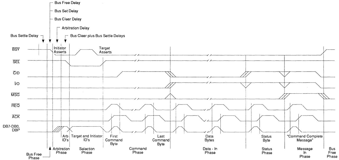
FIGURE 7: SCSI Signal Sequence Example
