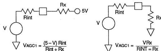
$V$  = Voltage at AGC1 with pin open (2.2V, nom.)
