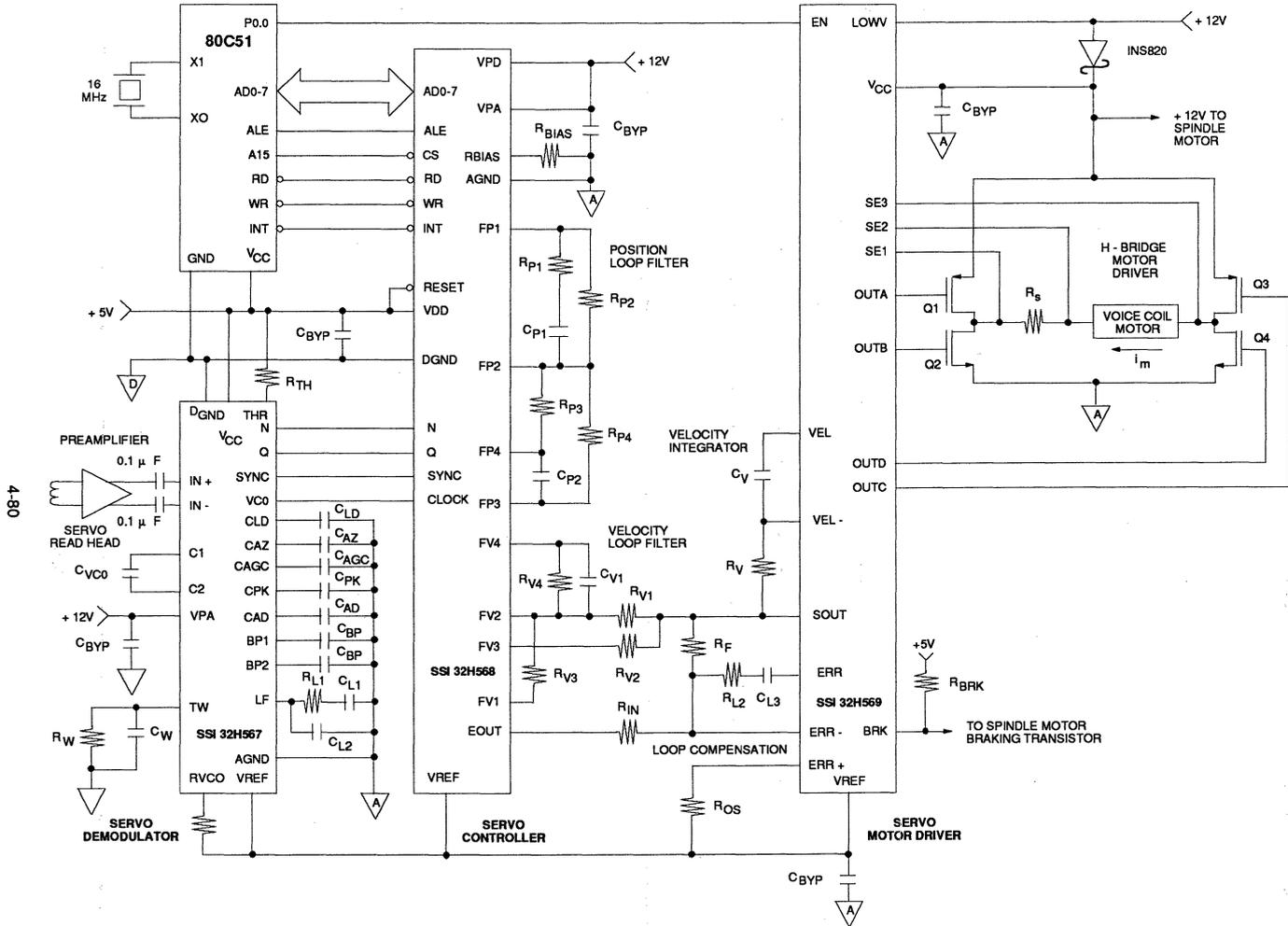
FIGURE 10: Complete Example Of Servo Path Electronics Using The SSI 32H567/568/569 Chip Set
