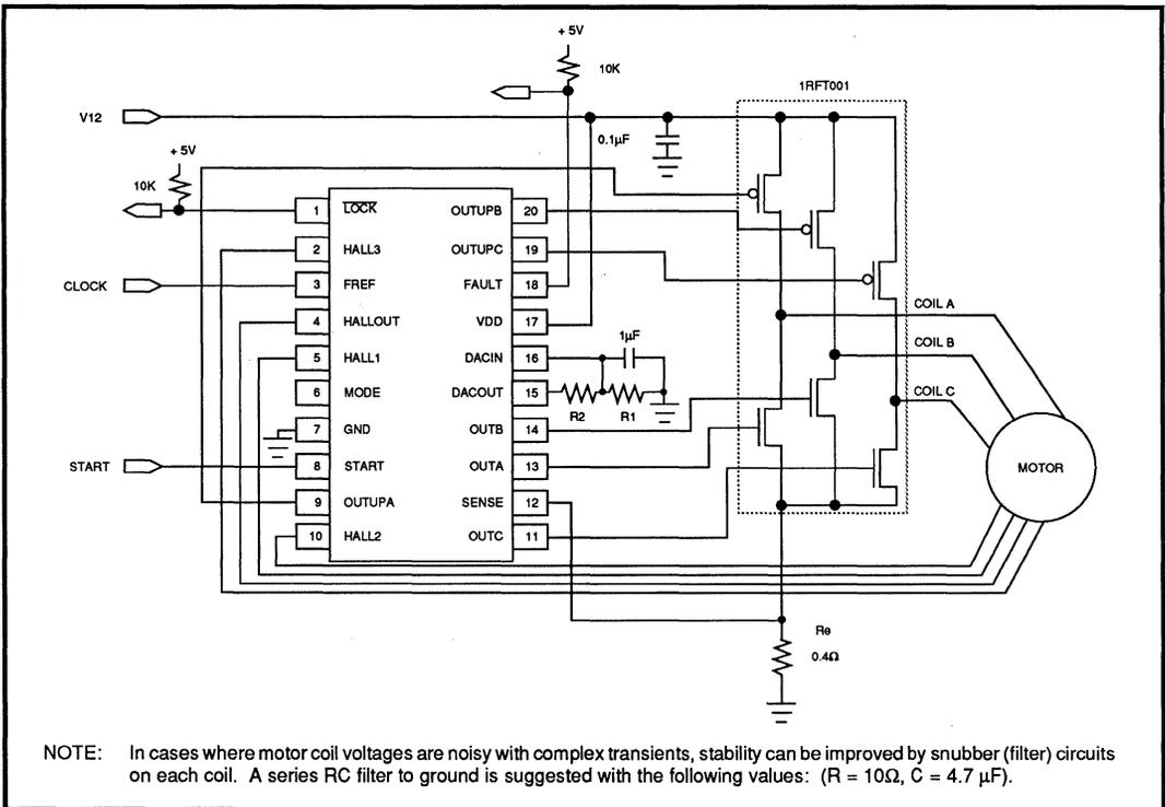
**Typical Three-Phase, 4-Pole, Bipolar,
