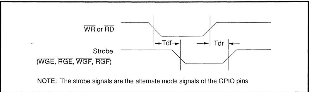
FIGURE 7: Address Decode 6E and 6F Timing
