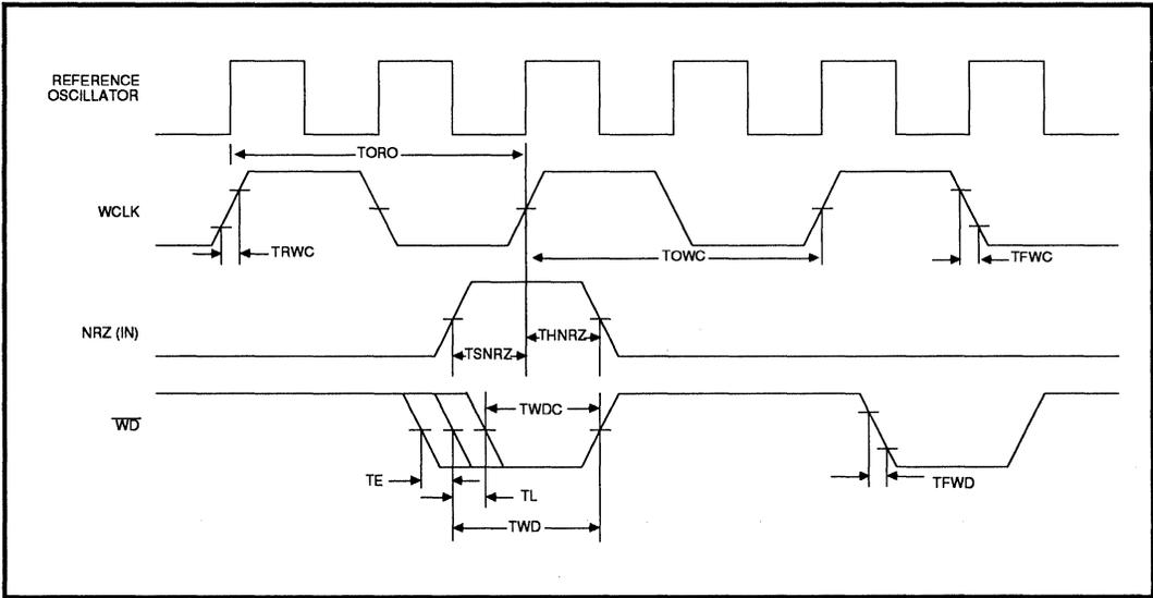
**FIGURE 10: Write Timing**
