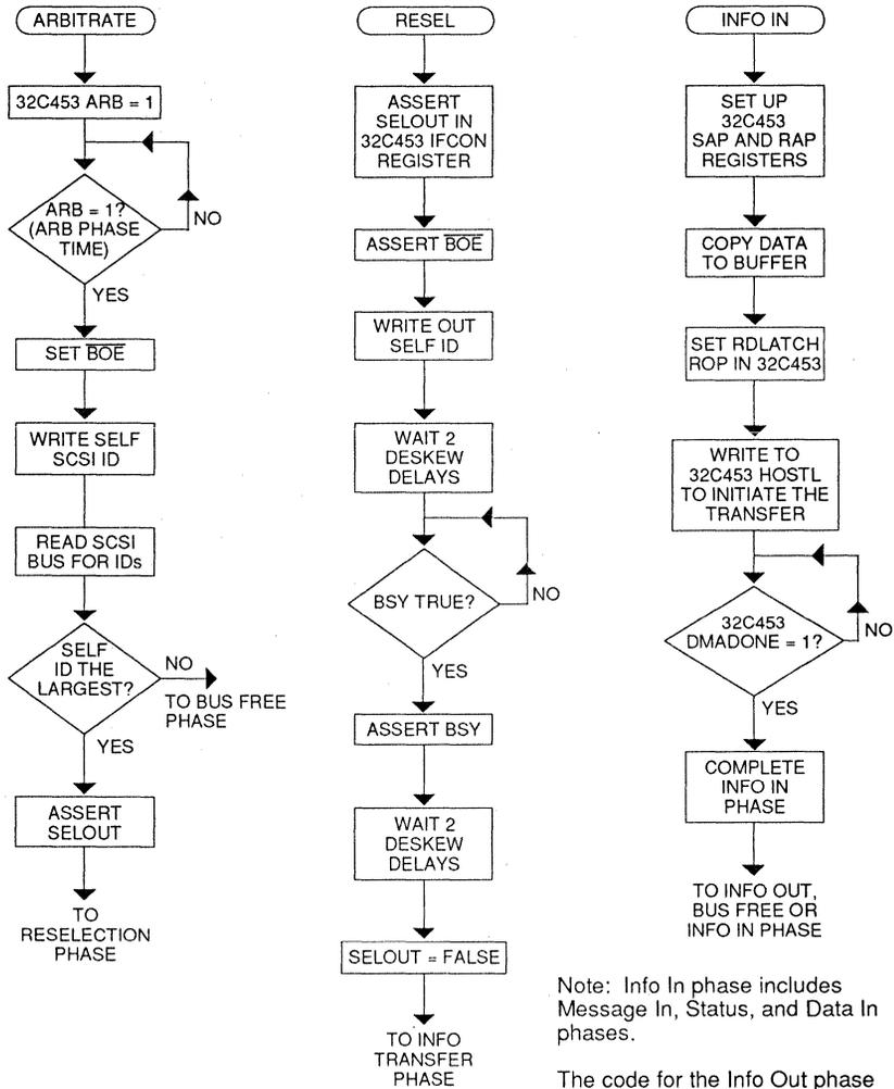
FIGURE 8: Flow Charts for Various SSI 32B451 Routines
