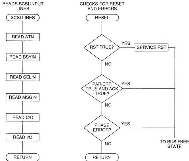
FIGURE 9: SCSI Background Routines Using SSI 32B451
