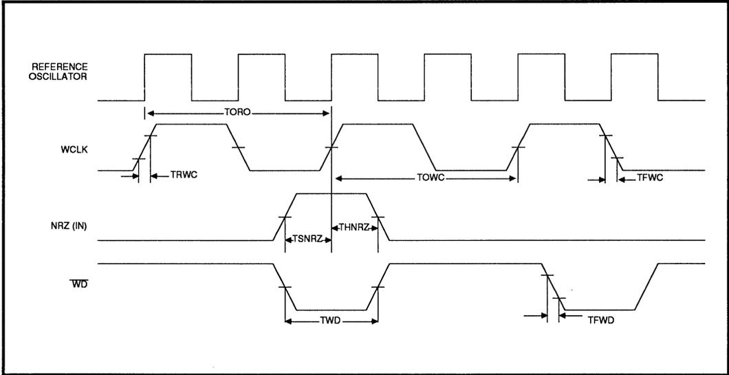
FIGURE 10: Write Timing
