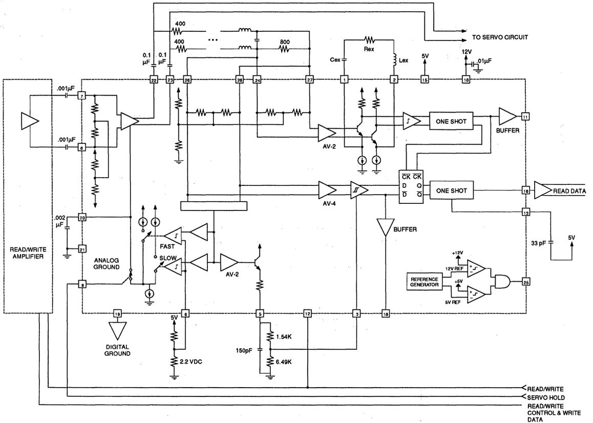
NOTE: Circuit traces for the 12V bypass capacitor and the AGC Hold Capacitor should be as short as possible with both capacitors returned to the Analog Ground Pin. Component values, where given, are for a 24 Mbit/s System. Above pin numbers are for the 28-pin PLCC package.
