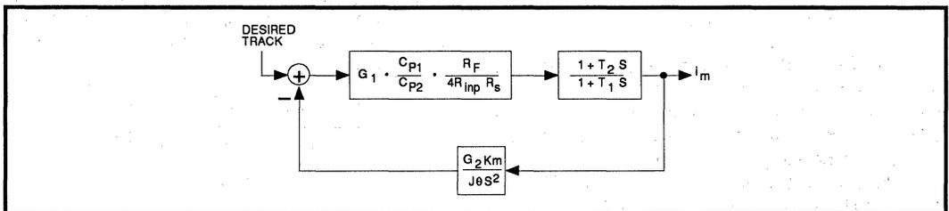
FIGURE 8(b): Simplified Track Mode Transfer Function
