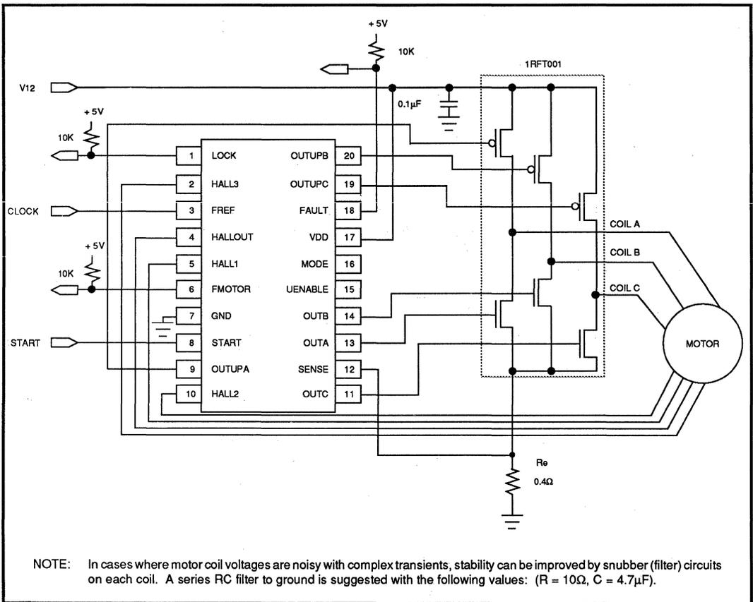
**Typical Three-Phase, 4-Pole, Bipolar,
