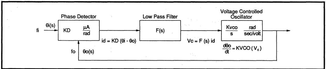
FIGURE 5 : Phase Locked Loop
