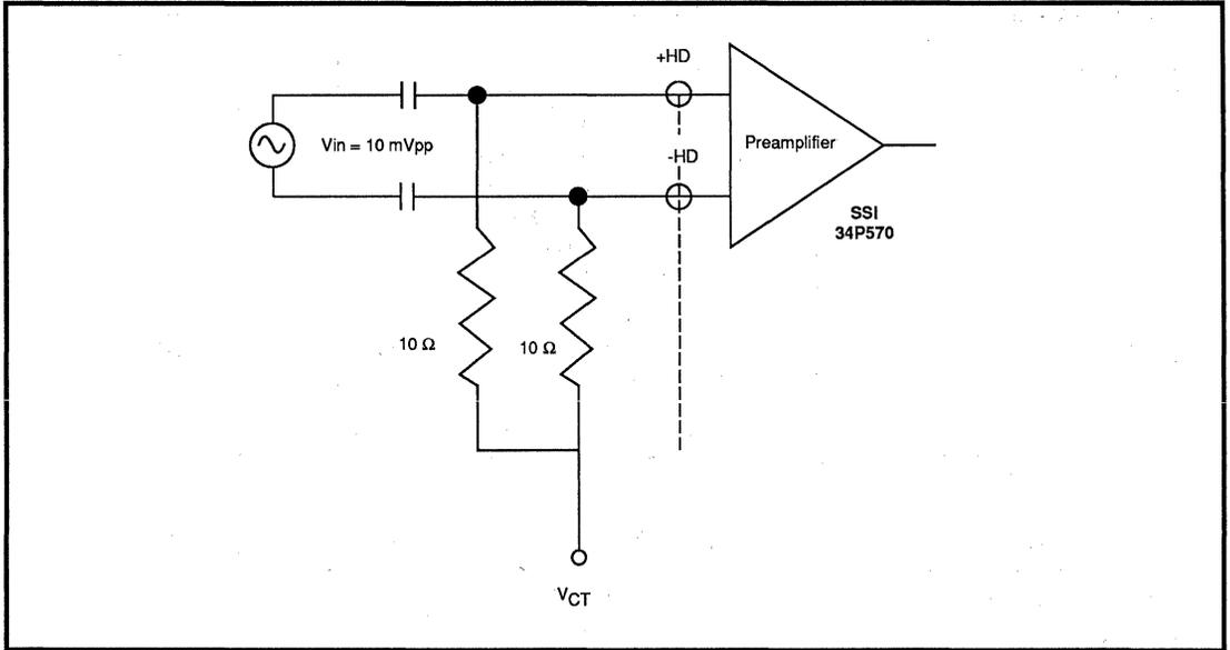
FIGURE 1: Preamplifier Characteristics
