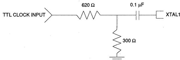
The signal amplitude into XTAL1 should be attenuated to approximately 1.0 Vp-p; this will insure that the transients associated with TTL switching characteristics won't couple into the SSI 32D535/5351 and degrade performance.
