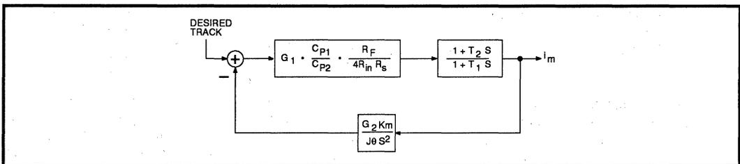
FIGURE 8(b): Simplified Track Mode Transfer Function
