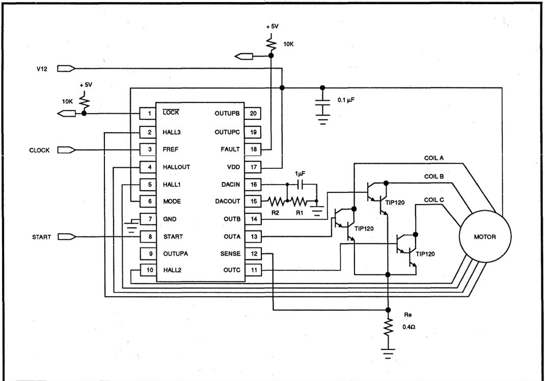
**Typical Three-Phase, 8-Pole, Unipolar,
