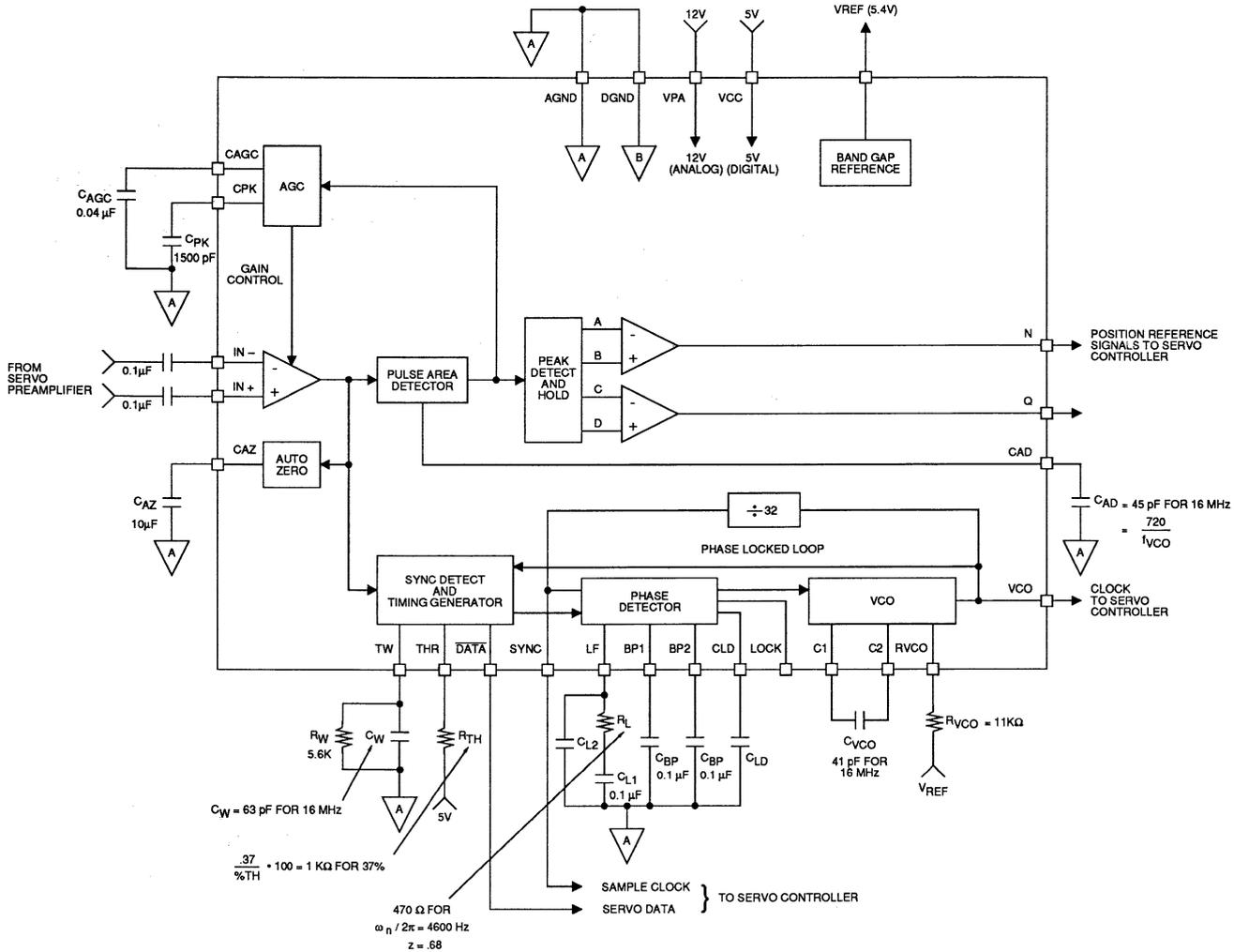
FIGURE 7: Design Example for 500 KHz Frame Rate
