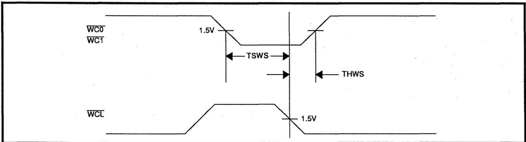
FIGURE 5: Control Timing
