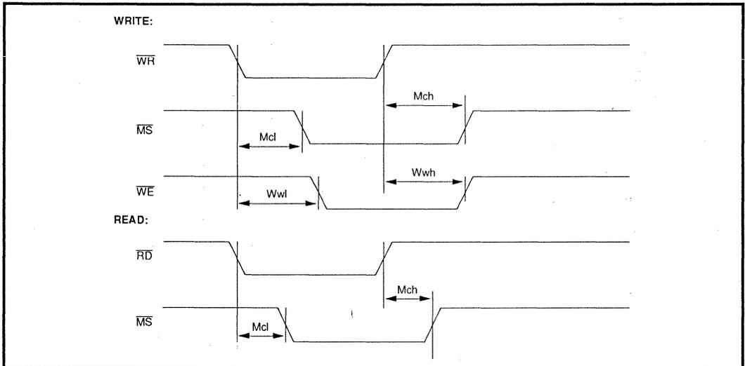
FIGURE 5: Register 70 Timing
