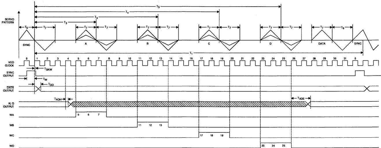
FIGURE 4: Timing Diagram
