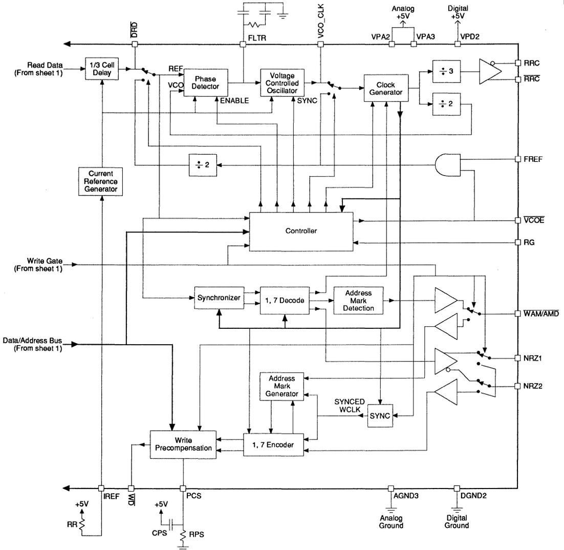
FIGURE 5b: Circuit Block Diagram - Differential Output Data Version - Sheet 2
