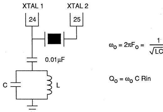
The typical input impedance looking into XTAL1 is approximately  $R_{in} = 250\Omega$ . It is recommended to design the value of  $Q_0$  at approximately 10 to 15. Therefore, a resonant frequency of  $F_0 = 20$  MHz would result in  $L \cong 0.16 \mu\text{H}$  and  $C \cong 380 \text{ pF}$ .
