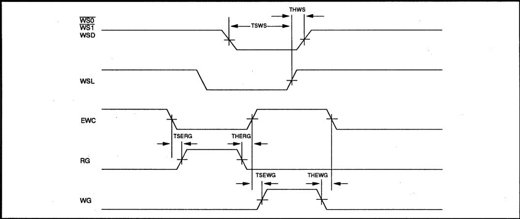
**FIGURE 7: Control Timing**
