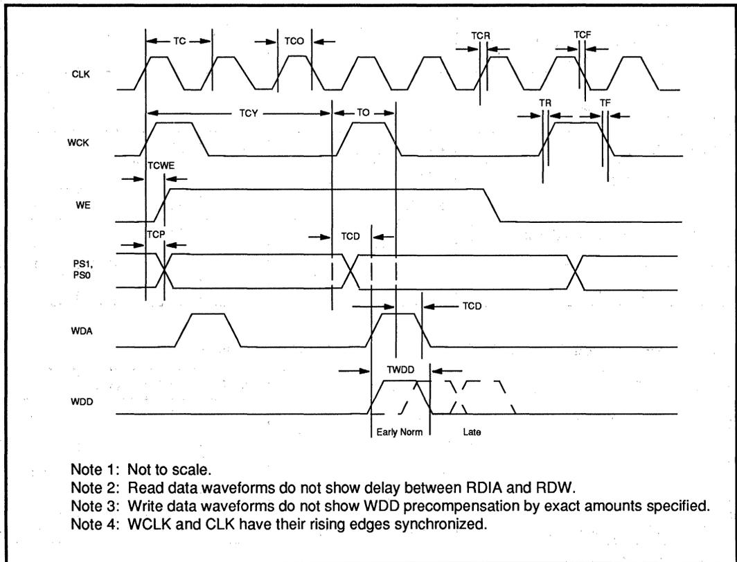
FIGURE 3: Switching Characteristics
