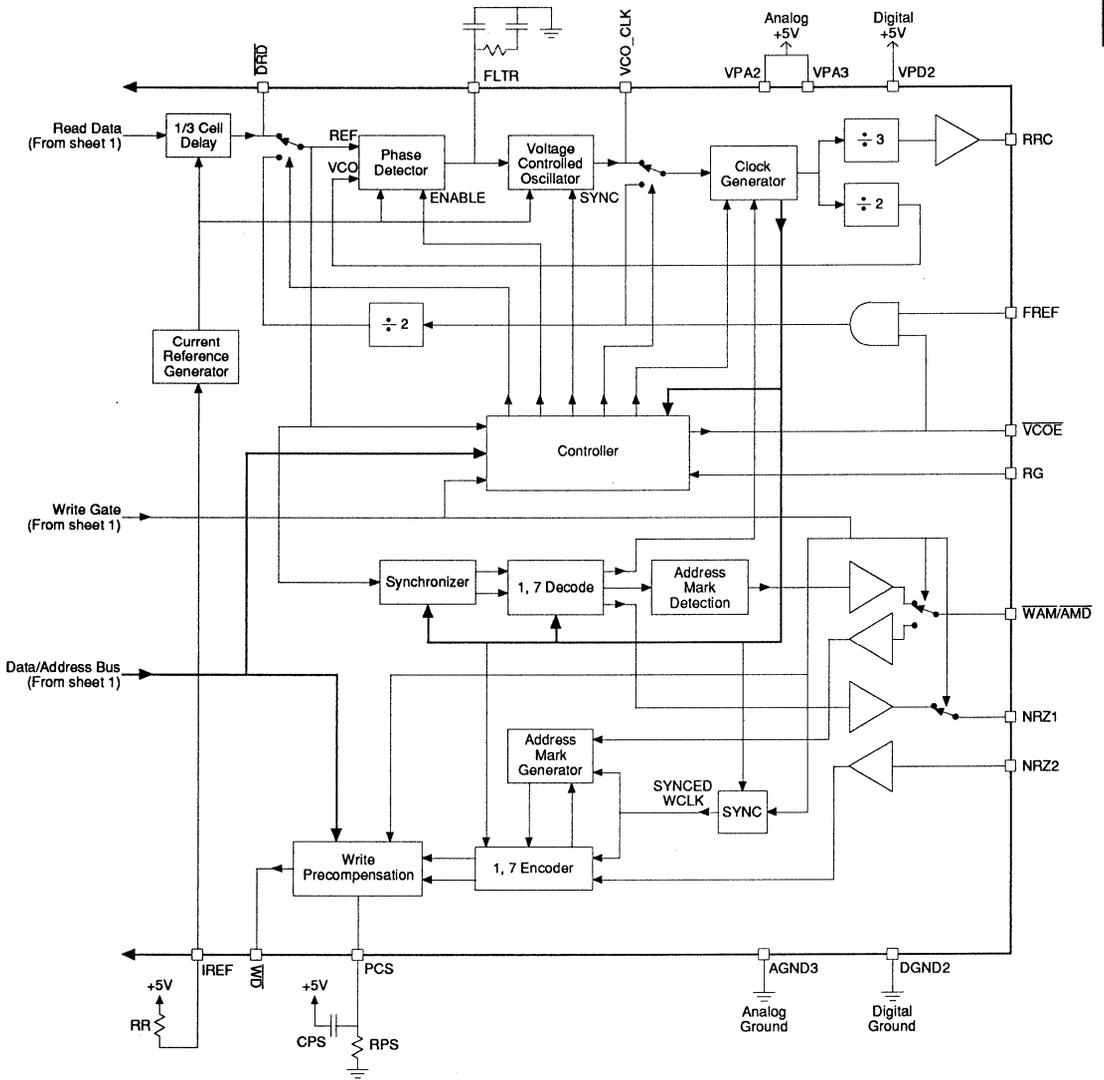
FIGURE 6b: Circuit Block Diagram - Single Ended Output Data Version - Sheet 2
