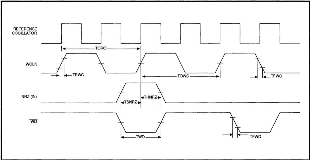
FIGURE 10: Write Timing
