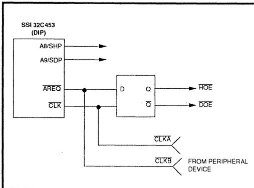
FIGURE 11: Extended Mode Address Strobes for DIP Package
