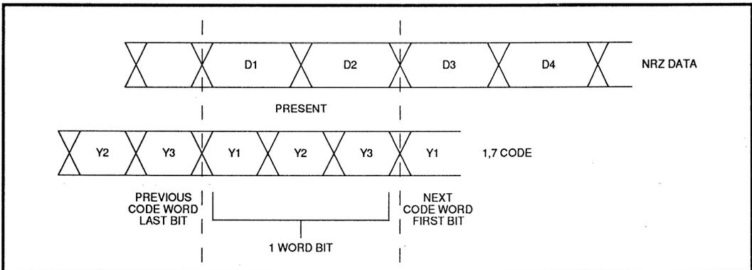
FIGURE 10: NRZ Data Word Comparison to 1, 7 Code Word Bit
