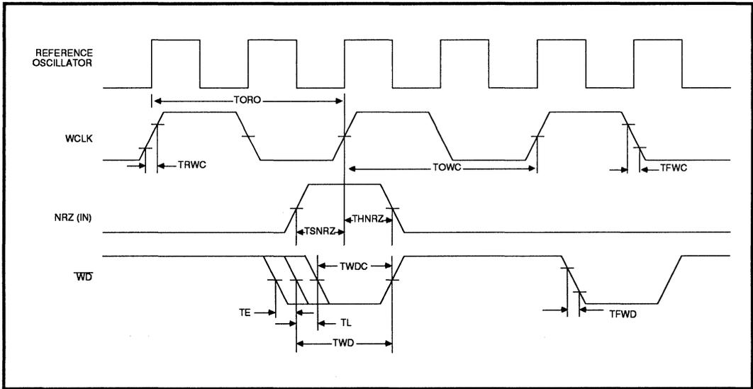
**FIGURE 10: Write Timing**
