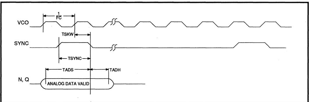
FIGURE 5: Analog Timing
