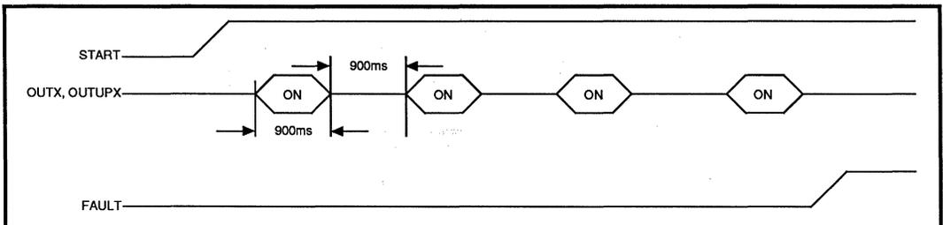
FIGURE 2: Jammed Platter Sequence
