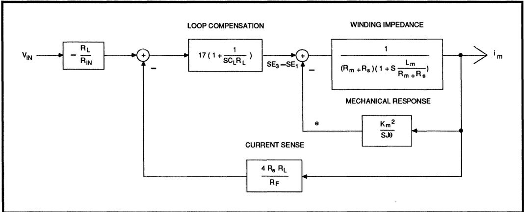
**FIGURE 4(A): Transfer Function Of SSI 32H569
