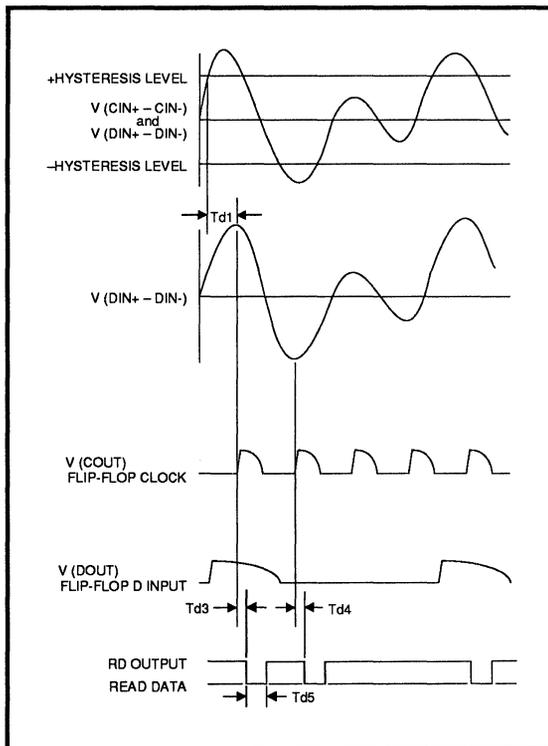
**FIGURE 2: Timing Diagram**
