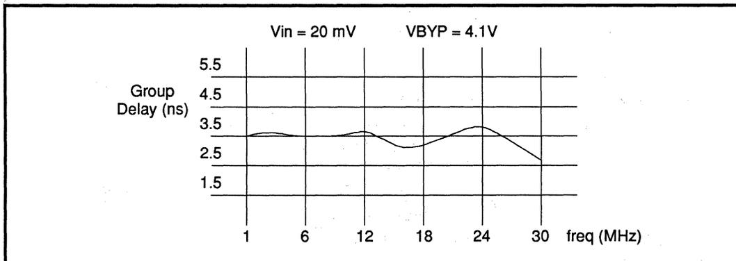
FIGURE 1: AGC Amplifier - Typical Group Delay Variation
