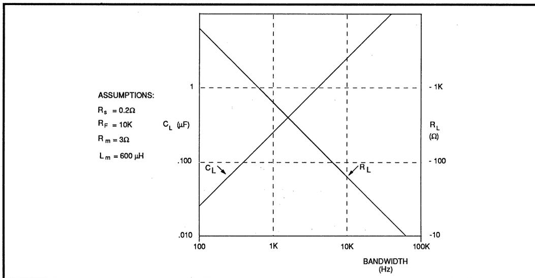
**FIGURE 6: Typical Motor Driver Compensation**
