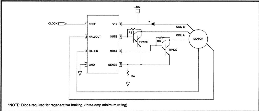
\*NOTE: Diode required for regenerative braking, (three amp minimum rating)
