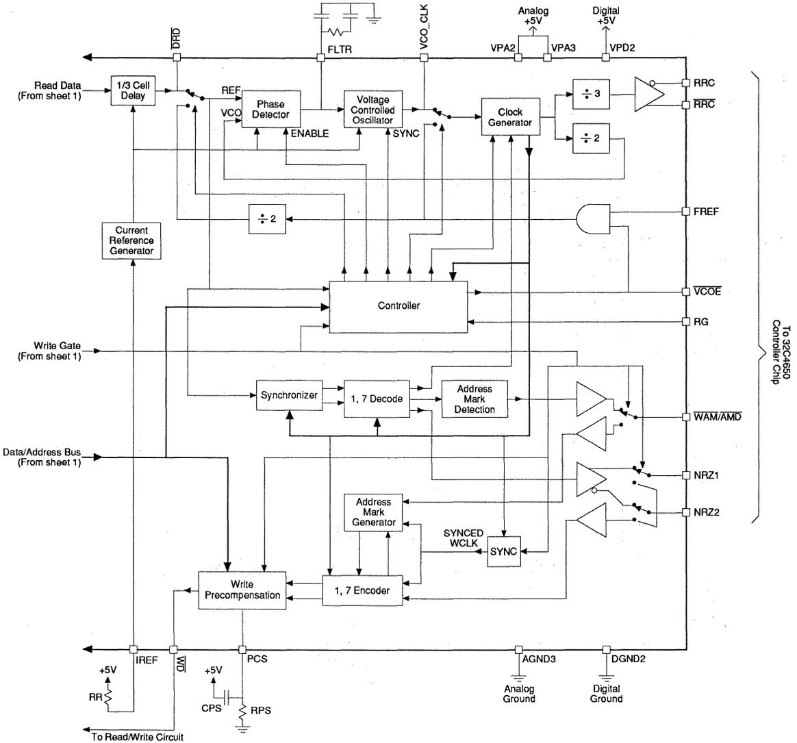
FIGURE 17b: System Configuration - Sheet 2
