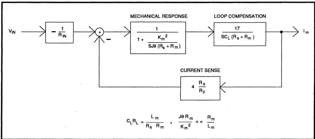
**FIGURE 4(B): Simplified Transfer Function Of
