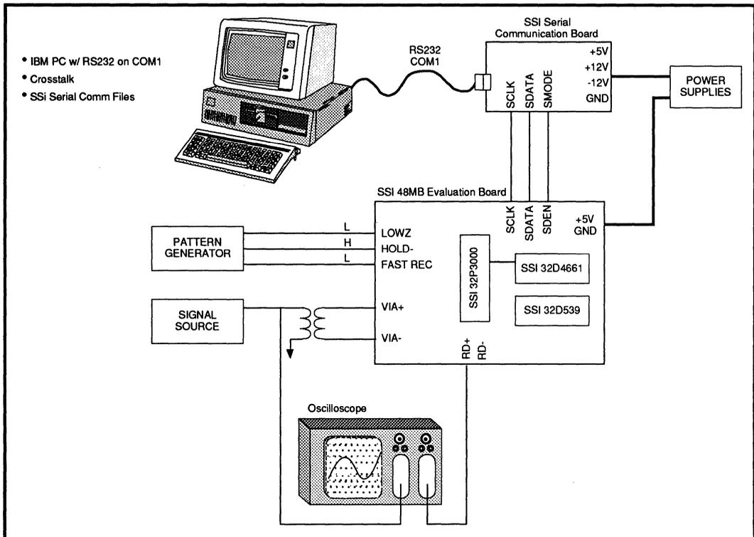
Figure 2: SSI 32P3000 Evaluation Board General Setup
