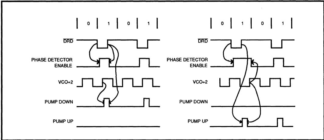
FIGURE 4.4.2: SSI 32P4730/4731 Data Separator Phase Detector Data Locking Mechanism
