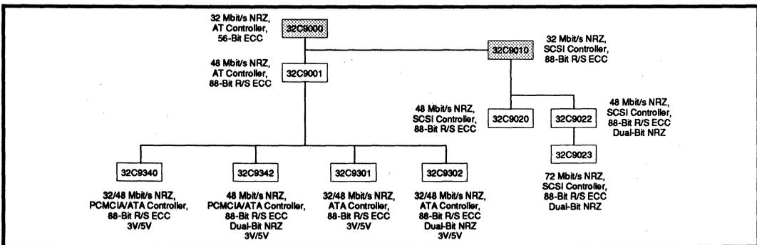
FIGURE 1: Silicon Systems' Disk Controller Chip Hierarchy
