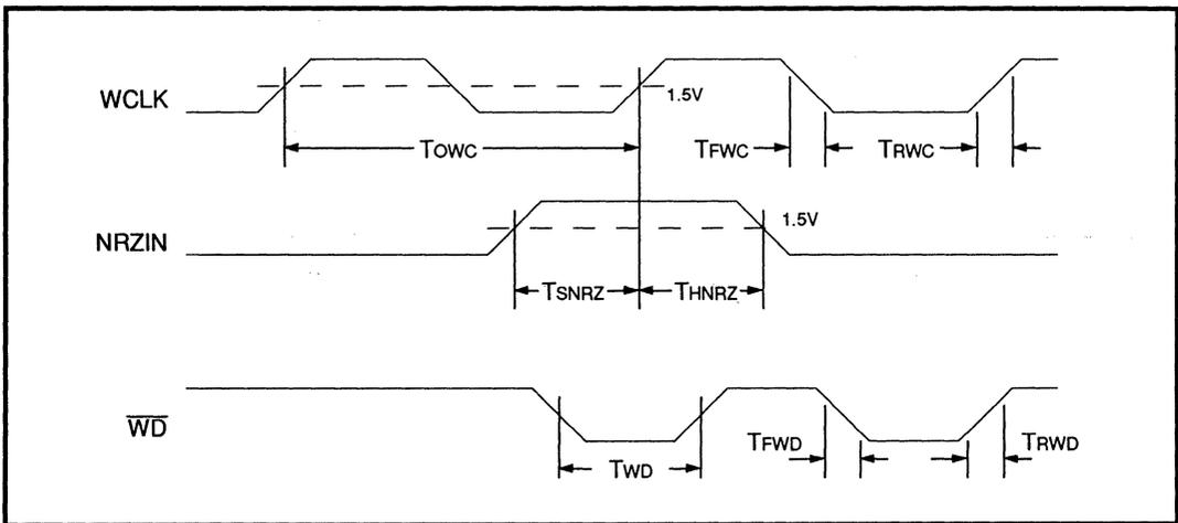
FIGURE 4:  $\overline{WD}$  and NRZ Write Timing
