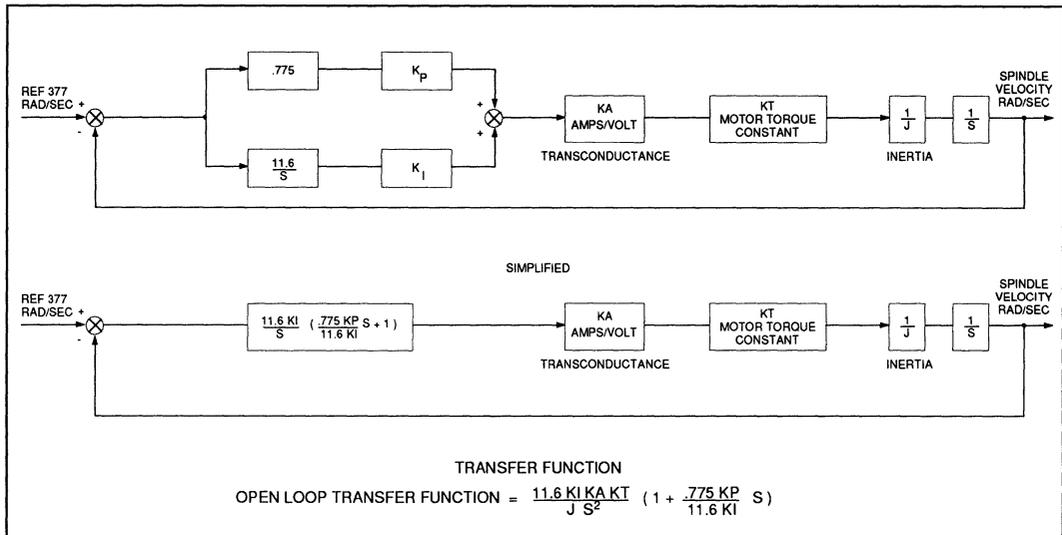
**FIGURE 1: Motor Speed Control Linearized Block Diagram**
