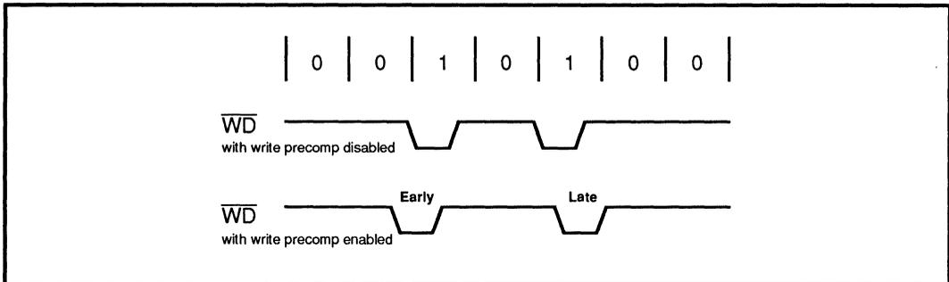
**FIGURE 6.2.1: Write Precomp Effect on  $\overline{WD}$**
