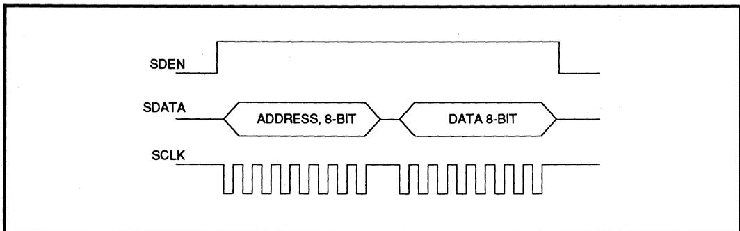
FIGURE 1: Serial Port Data Transfer Format
