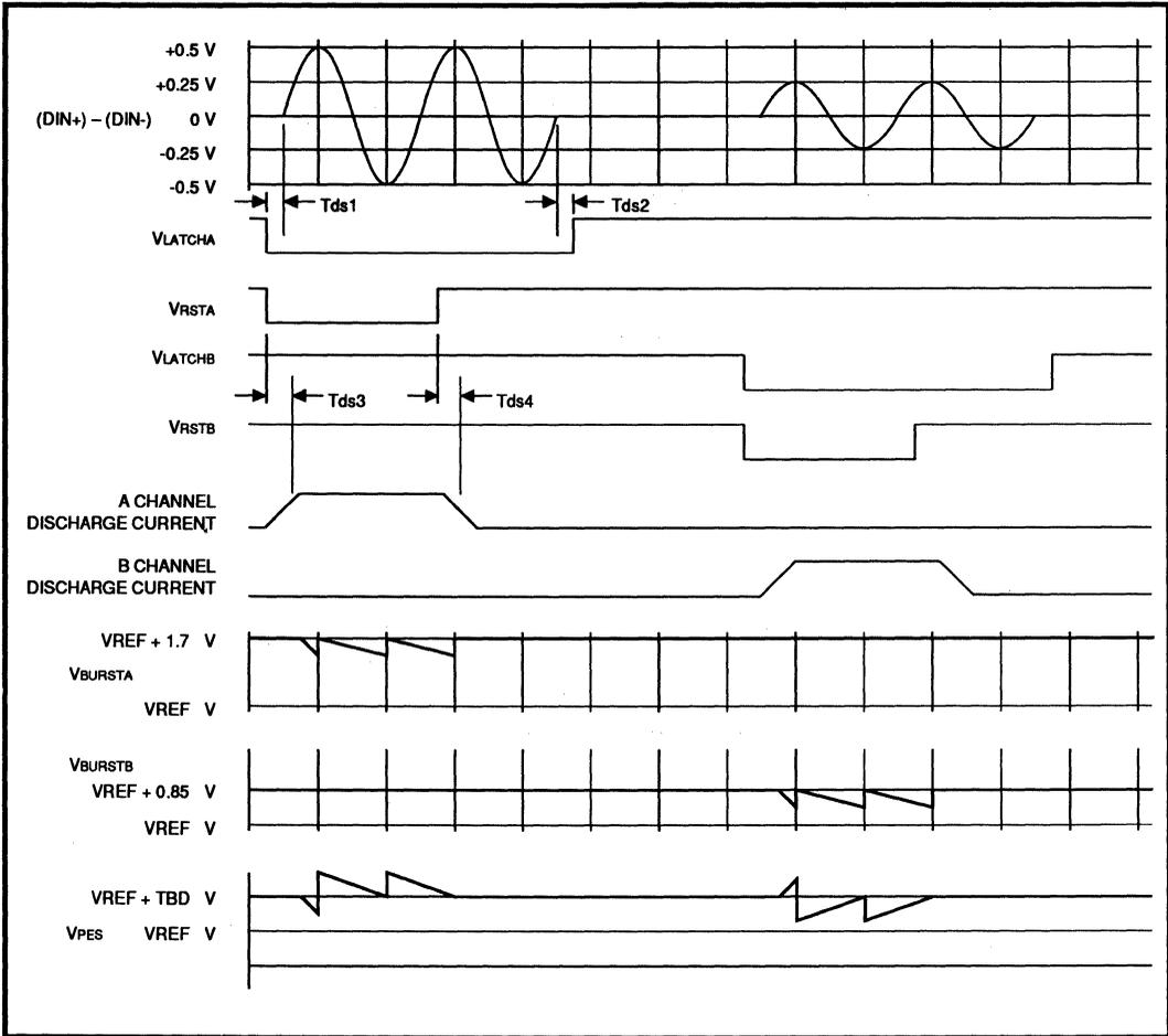
FIGURE 4: Servo Read Mode II Timing Diagram
