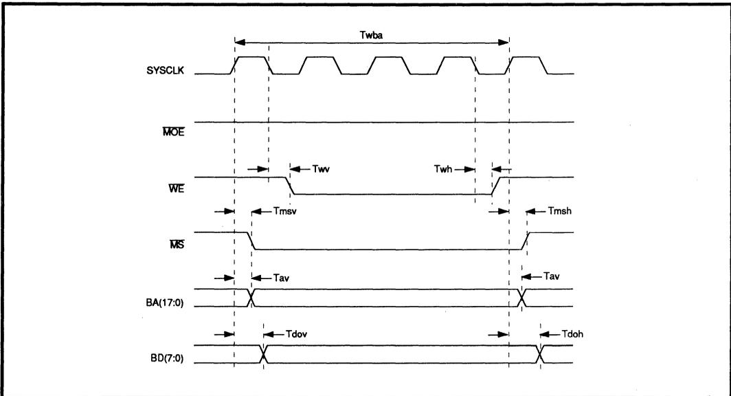
**FIGURE 10: SRAM Write Timing**
