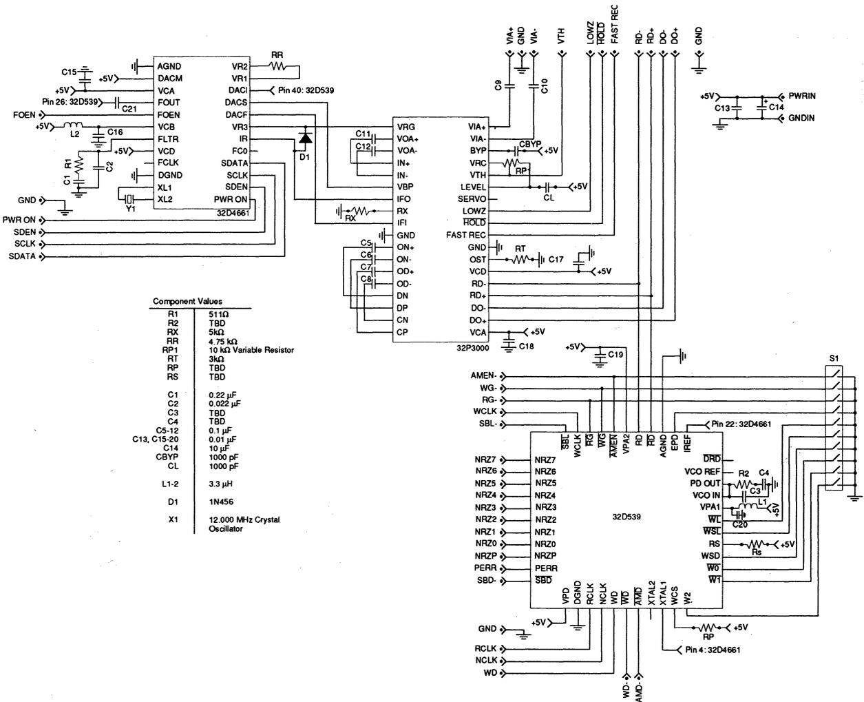
FIGURE 12: 32P3000 / 32D539 / 32D4661 Evaluation Board Schematic
