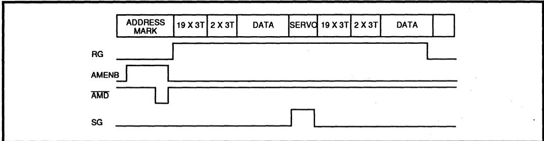
FIGURE 7: Split Field Servo Operation
