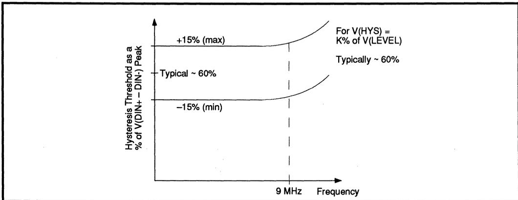
FIGURE 5: Percentage Threshold Versus Frequency
