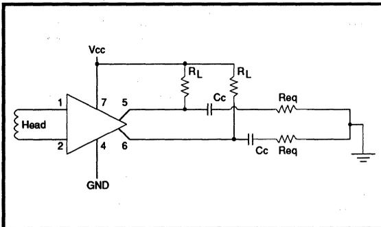
FIGURE 1: Connection Diagram
