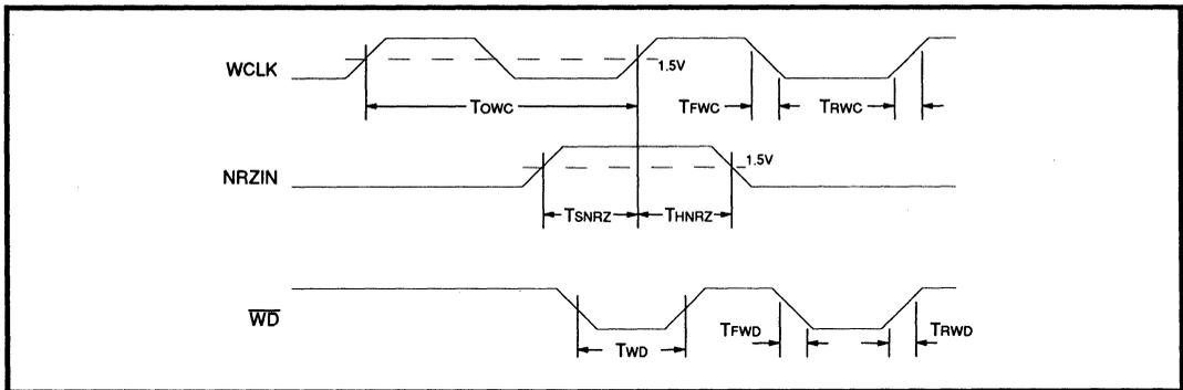
FIGURE 9:  $\overline{WD}$  and NRZ Write Timing
