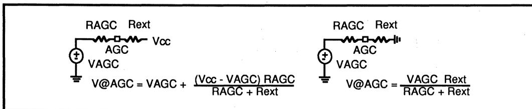
FIGURE 2: AGC Loop Reference Adjustment
