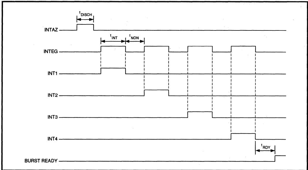
FIGURE 1: Embedded Servo Burst Processor Timing Diagram
