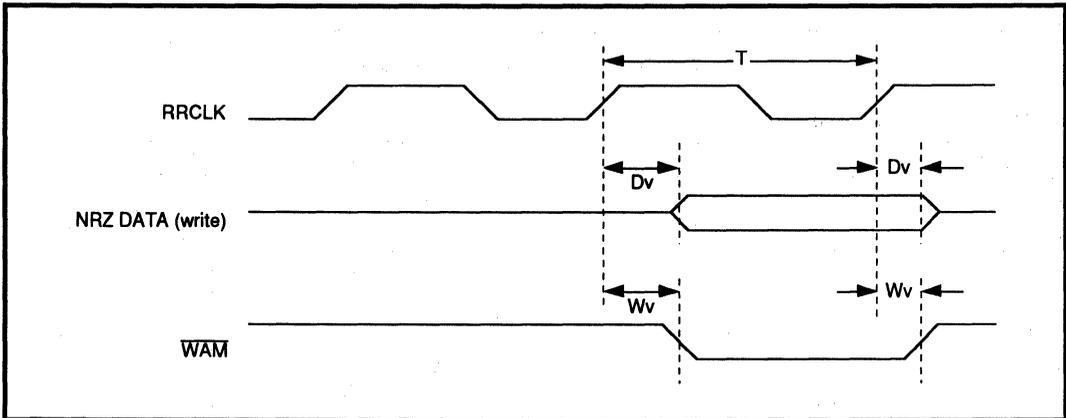
**FIGURE 8: Disk Write Timing**
