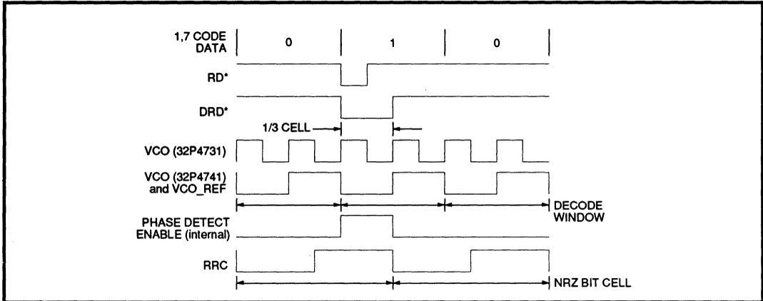
**FIGURE 5: Data Synchronization Waveform**
