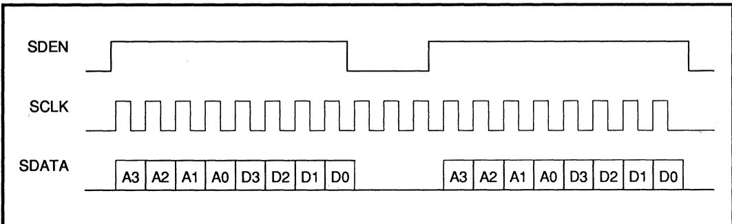
FIGURE 2: Serial Port Timing, Multiple Transfers
