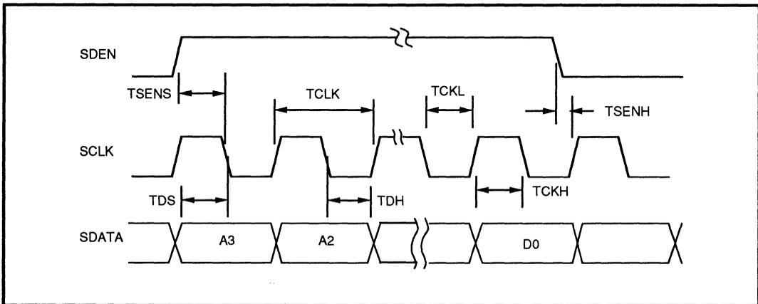
**FIGURE 2: Serial Port Timing**
