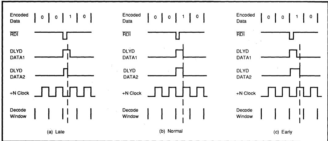
**FIGURE 6: Decode Window & Window Shift Directions**
