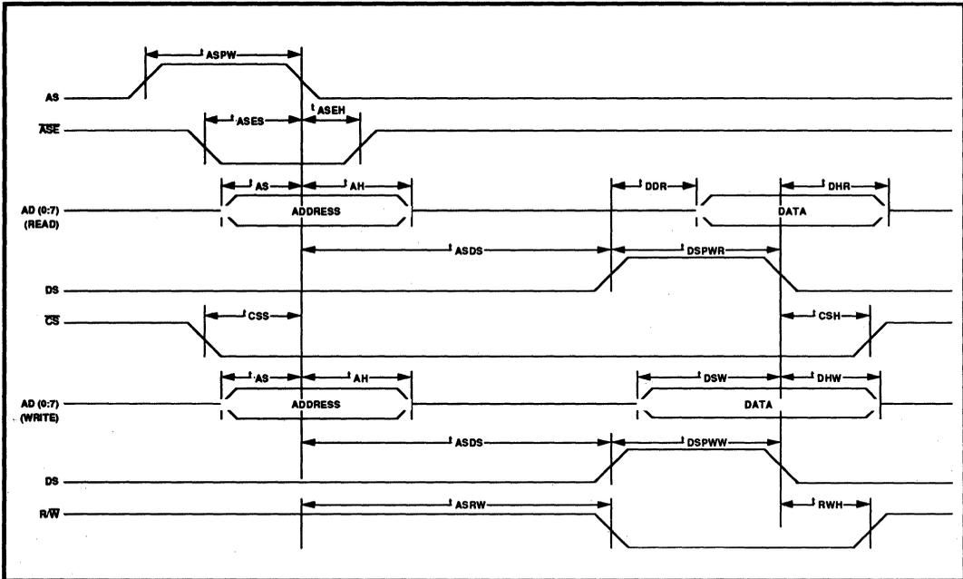
FIGURE 12: Motorola Microprocessor Bus Interface Timing Diagram
