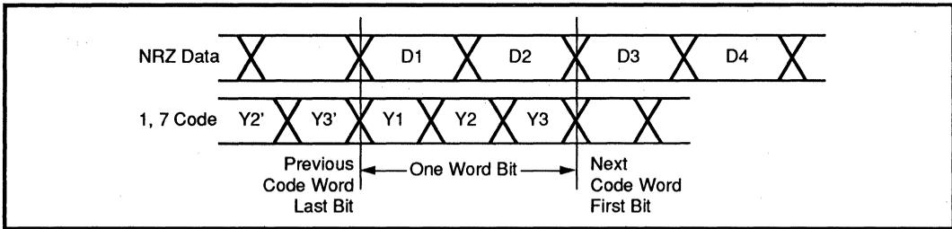
**FIGURE 4: NRZ Data Word Comparison to 1, 7 Code Word Bit**
