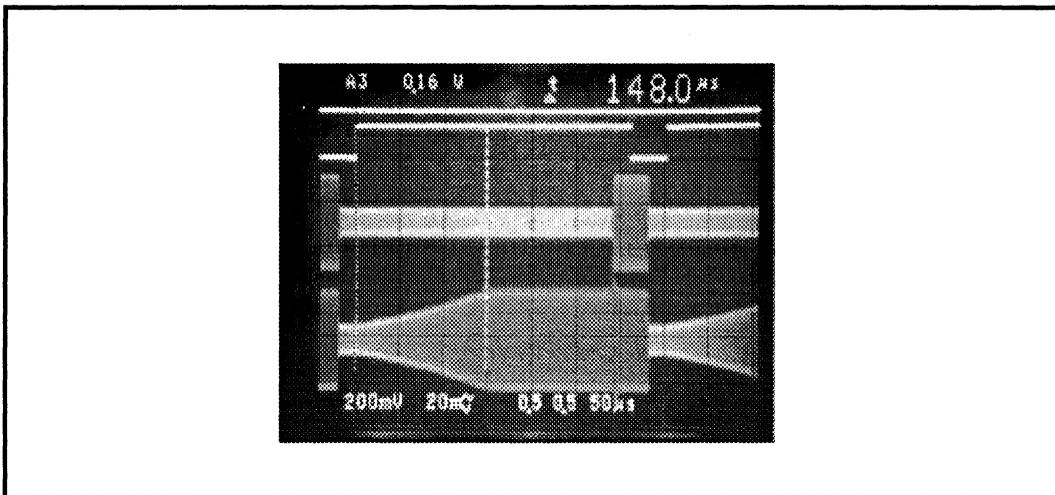
**Figure 10: AGC Recovery Without Using FAST REC**
