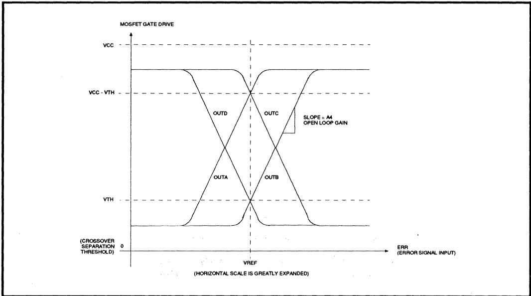
**FIGURE 5: Simplified Transfer Function of SSI 32H6230
