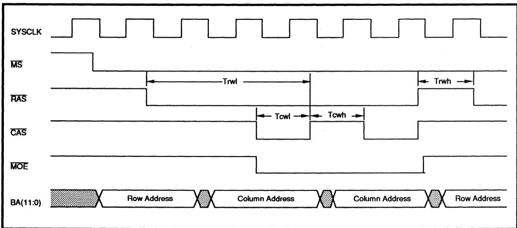
**FIGURE 14: DRAM Timing (Showing the Relationship of RWL, RWH, CWL and CWH to overall timing)**
