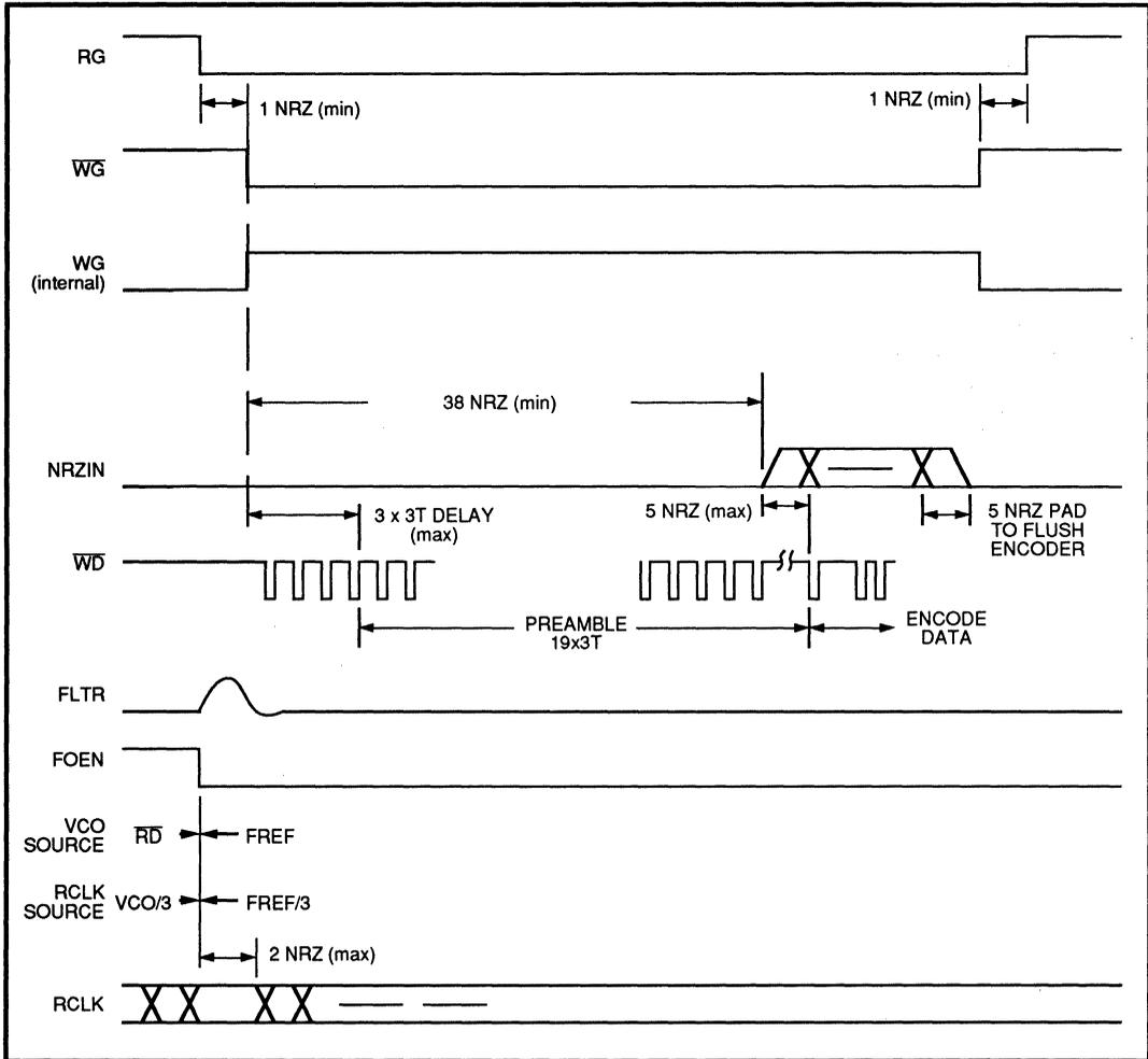
**FIGURE 7: Write Data Operation**
