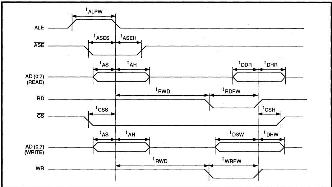
FIGURE 2: Intel Microprocessor Bus Interface Timing Diagram
