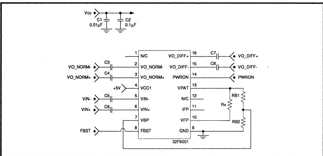
FIGURE 3: The 32F8001 Setup as a Fixed Response Filter
