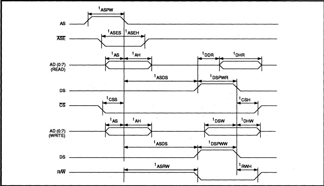
FIGURE 3: Motorola Microprocessor Bus Interface Timing Diagram
