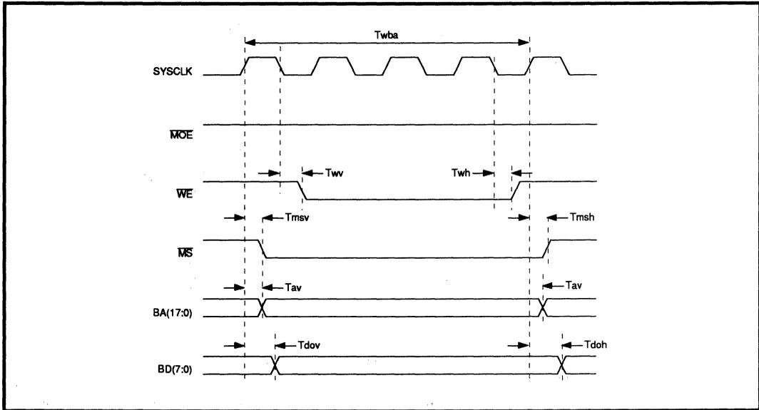
**FIGURE 10: SRAM Write Timing**
