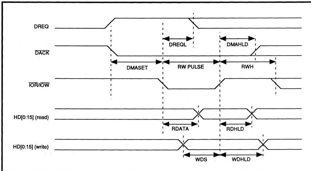
FIGURE 17: Host DMA 8/16-Bit Interface Timing (Demand Mode)
