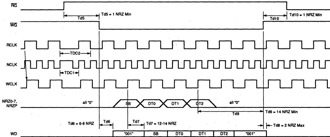
**FIGURE 13: Write Mode NRZ Timing**
