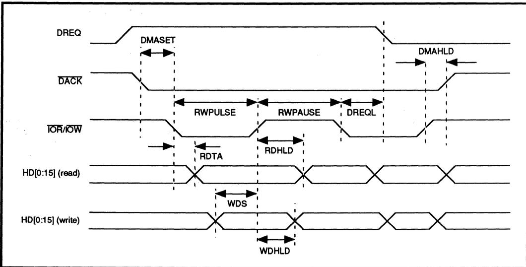
**FIGURE 16: Host DMA 8/16-Bit Interface Timing (Demand Mode)**
