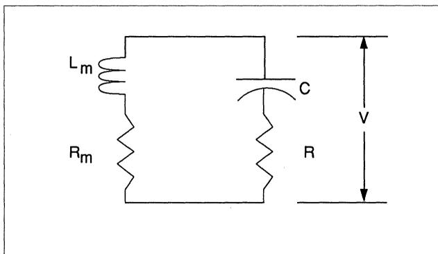
Figure 1: Motor and Snubber Circuit Equivalent Circuit
