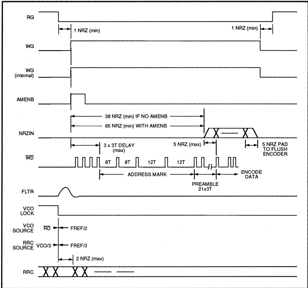
**FIGURE 12: Write Data Operation (Hard and Soft Sector)**
