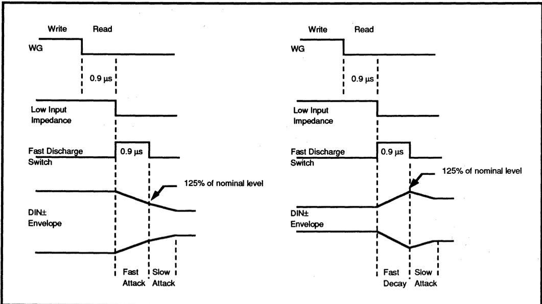
**FIGURE 3: AGC Action Timing in Write-to-Read Recovery**
