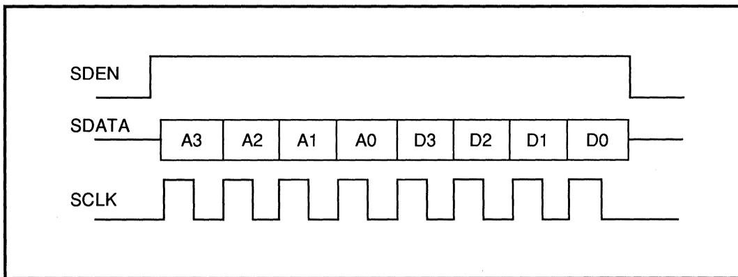
FIGURE 1: Serial Port Data Transfer Format
