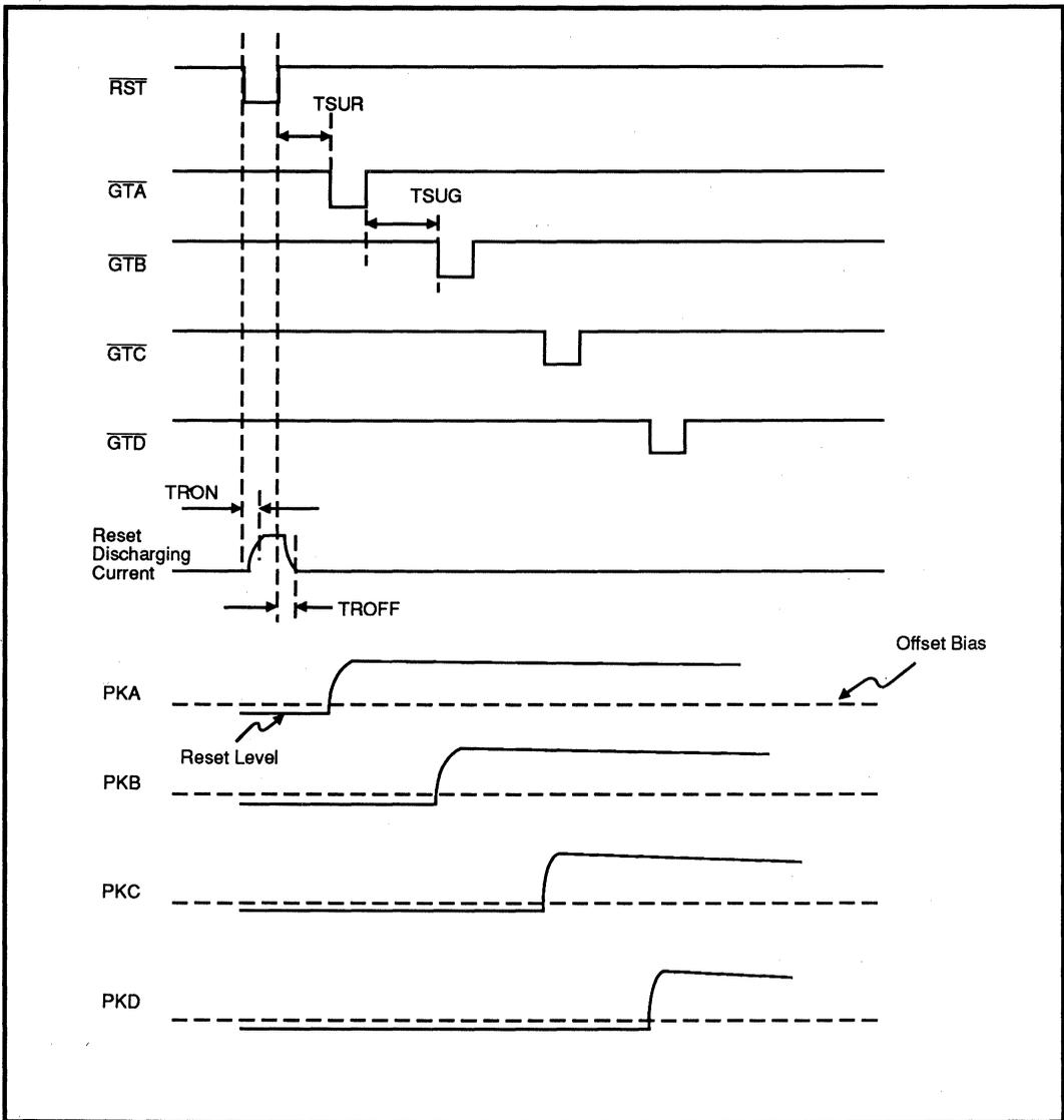
FIGURE 2: Servo Capture Timing Sequence
