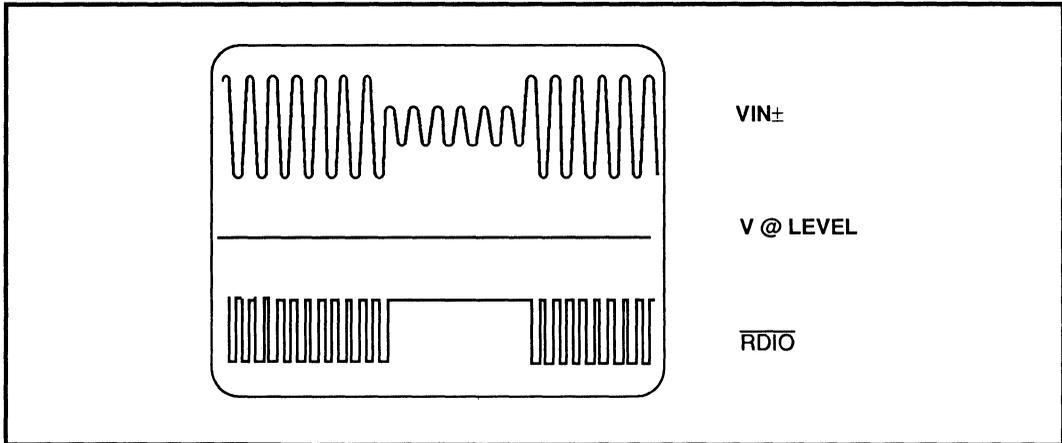
PHOTO 4.1.1: Qualification threshold at 50%; 0.033  $\mu$ F from LEVEL to VPA. Input changes from 100 mVppd to 40 mVppd. Large qual threshold time constant  $\gg$  Missing  $\overline{RDIO}$  pulses.
