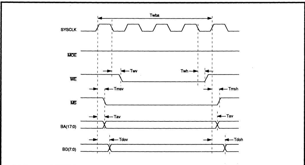
**FIGURE 10: SRAM Write Timing**
