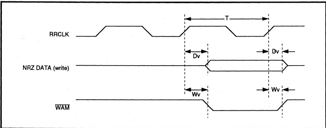
FIGURE 8: Disk Write Timing
