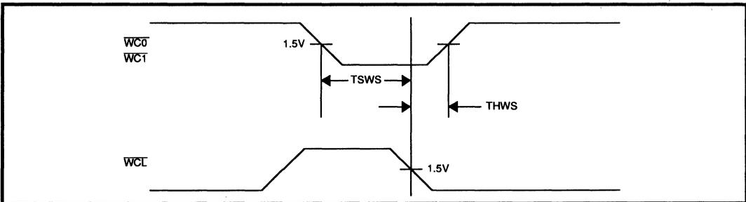
**FIGURE 5: Control Timing**
