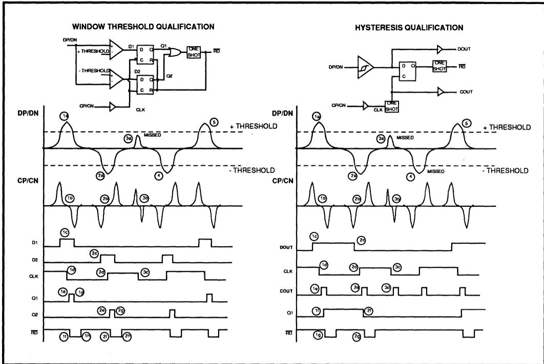
FIGURE 4.1.3: Window Threshold Qualification & Hysteresis Qualification
