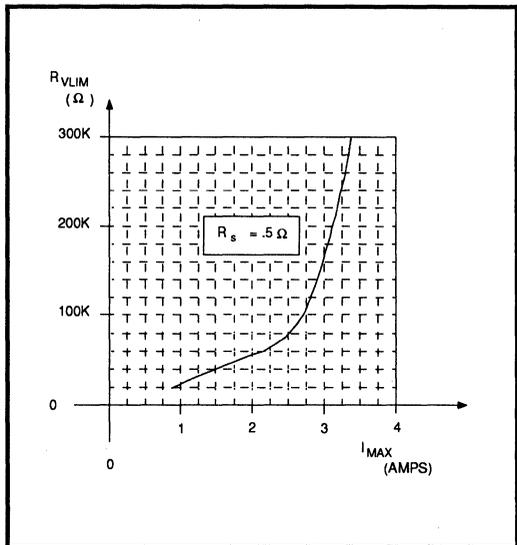
**FIGURE 7: RVLIM To VREF Typical Motor Current Limit**
