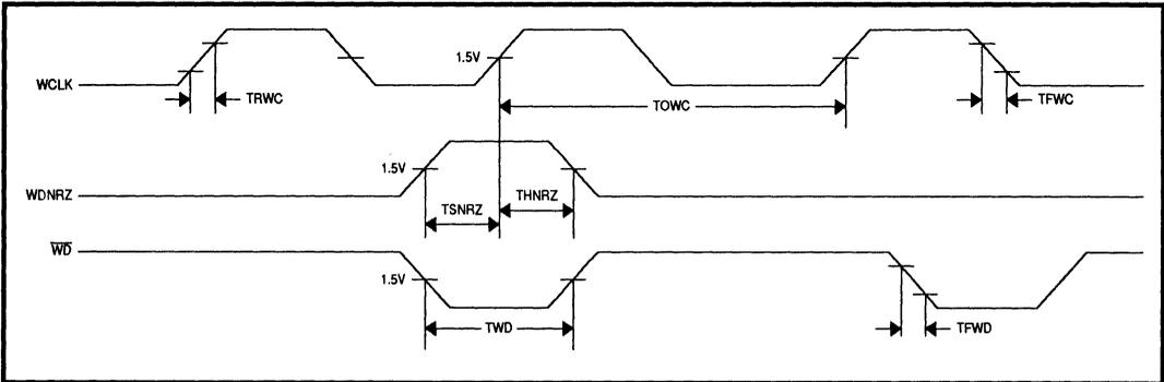
**FIGURE 4: Write Timing**
