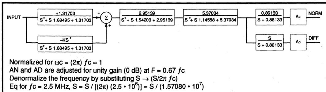
FIGURE 1: Normalized Transfer Function of the SSI 32F8130/8131
