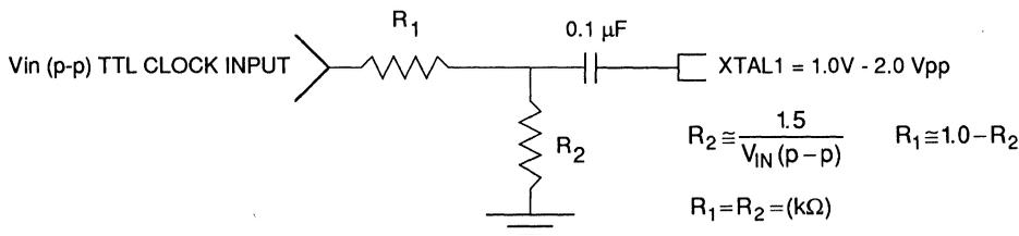
The signal amplitude into XTAL1 should be attenuated to approximately 1.0 to 2.0 Vp-p; this will insure that the transients associated with TTL switching characteristics won't couple into the data synchronizer and degrade performance.
