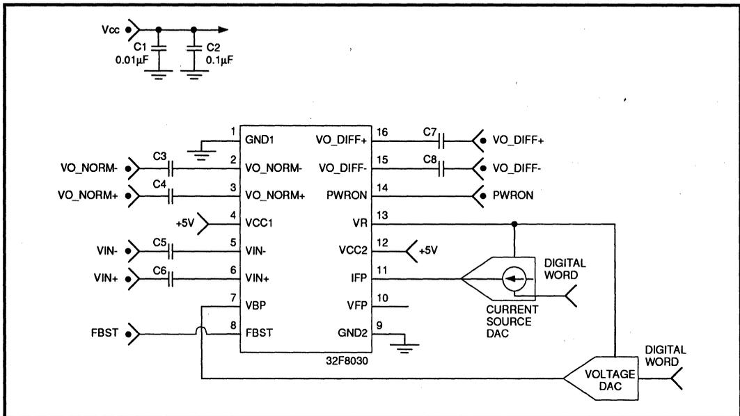
FIGURE 4: The SSI 32F8030 Setup Schematic Using a Current Source DAC for Cutoff Frequency Control
