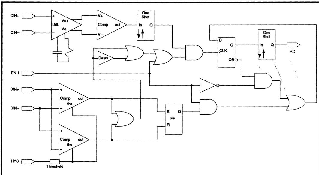
**FIGURE 3: ENH Provides Two Pulse Qualification Modes.**
