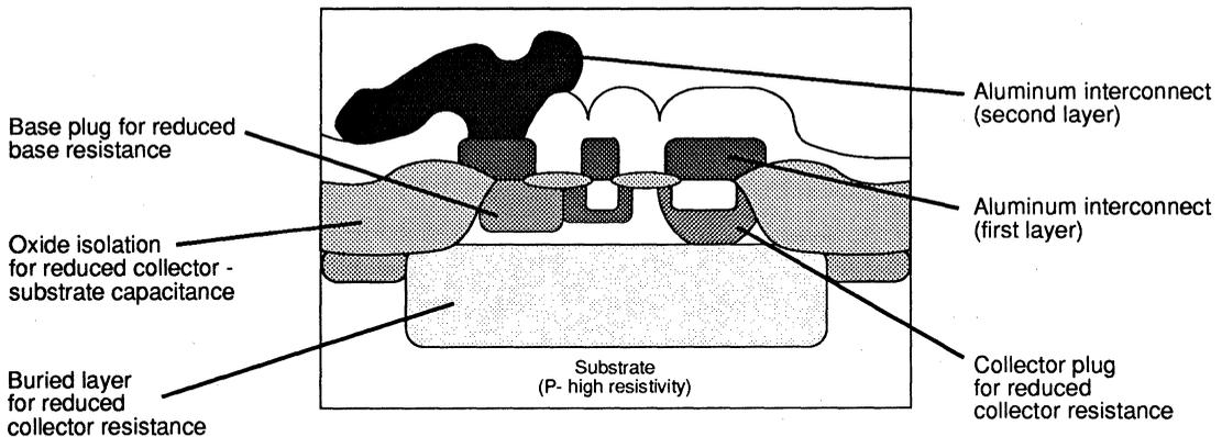
**FIGURE 2: BN Bipolar Process NPN Transistor**
