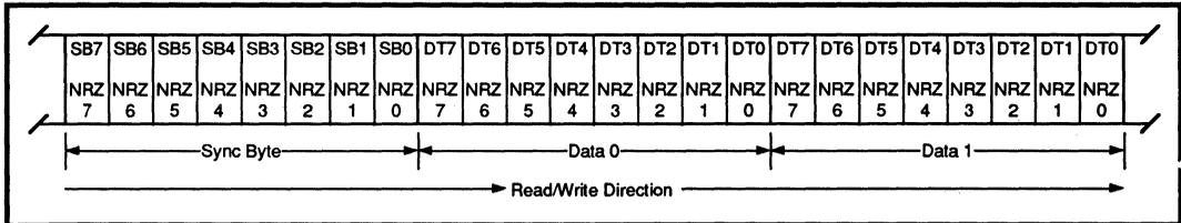
**FIGURE 14: Parallel/Serial Conversion Format**
