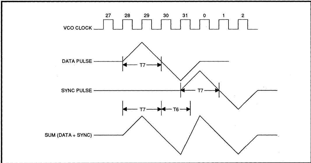
FIGURE 7 : Servo Writer Data-Sync Pulse Generation
