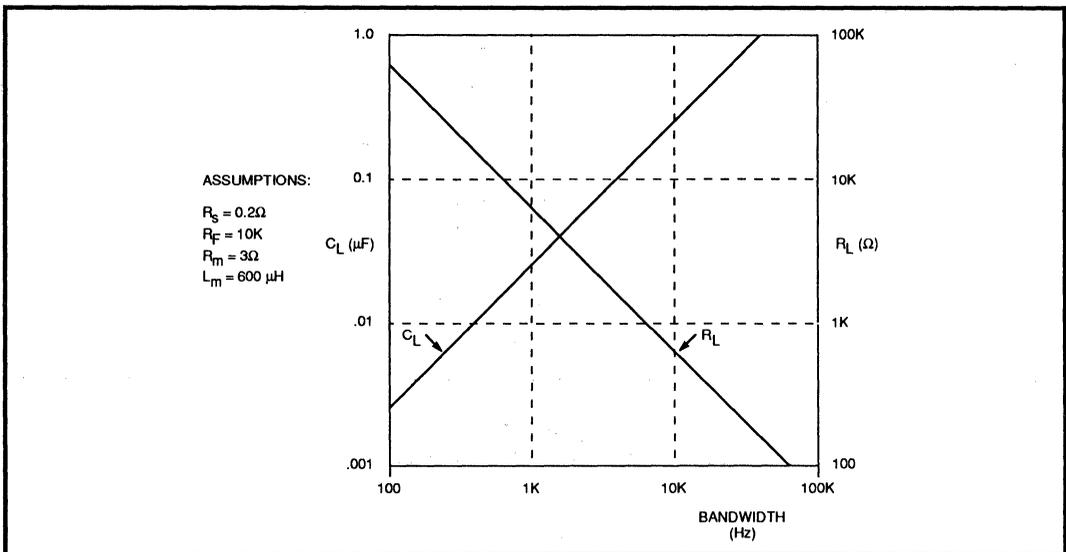
**FIGURE 6: Typical Motor Driver Compensation**
