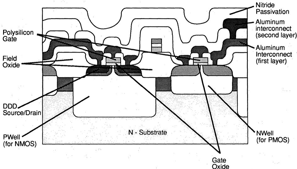
FIGURE 1: CG CMOS Process Transistor
