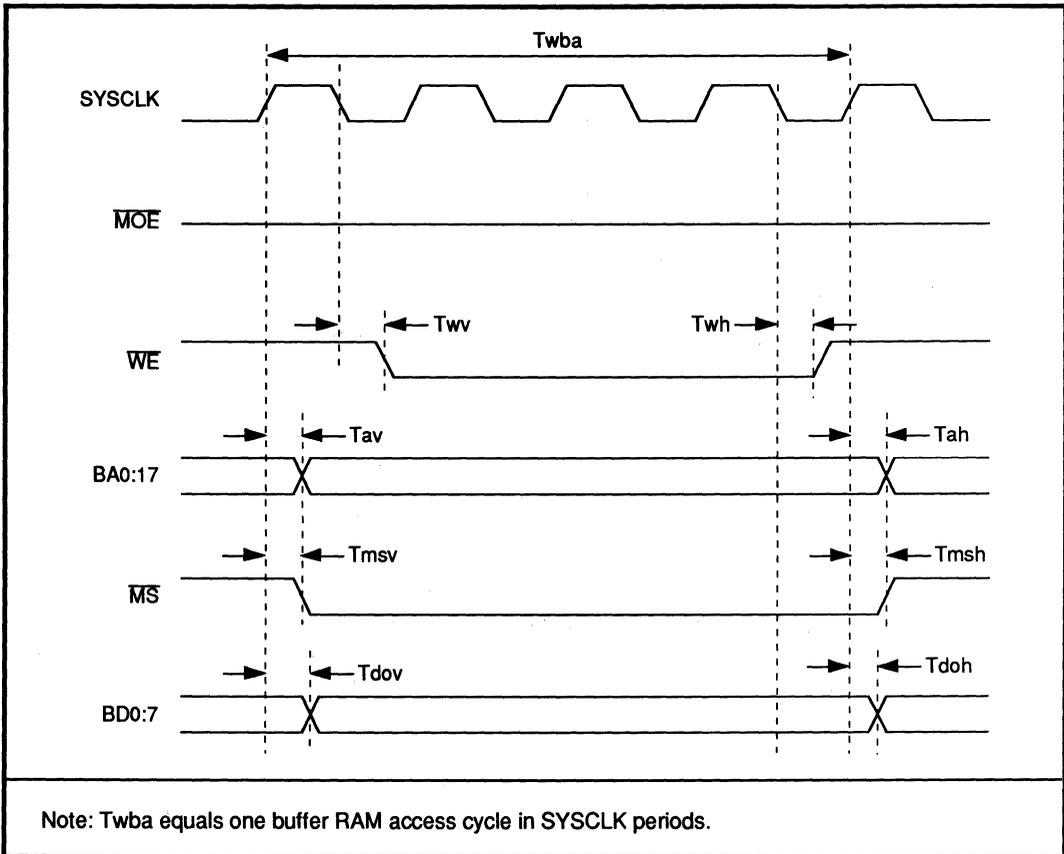
**FIGURE 10: SRAM Write Timing**
