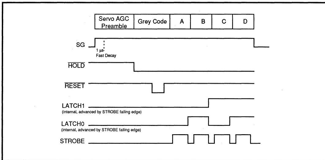
FIGURE 5.2.1: SSI 32P4731 Servo Control Sequence
