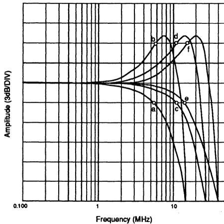
**FIGURE 4: 32F8011/8012 Normal Low Pass Output Response (VO\_NORM)**
