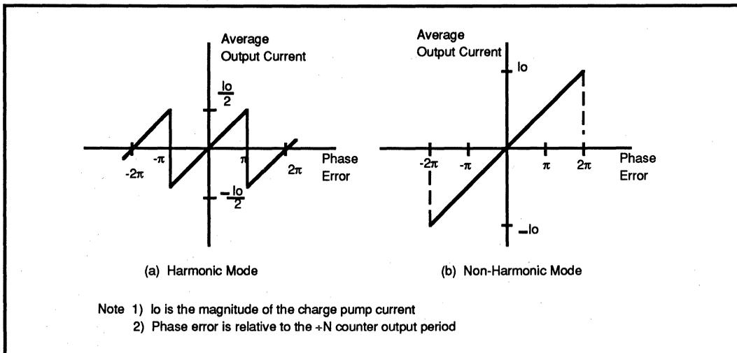
FIGURE 5: Phase Detector Transfer Function
