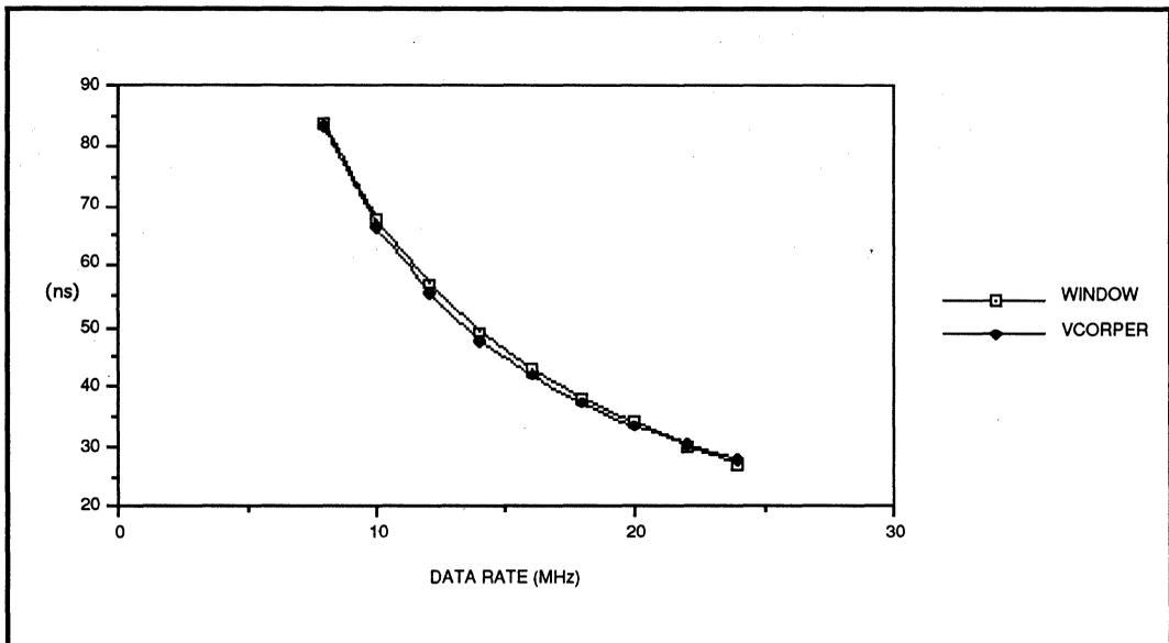
FIGURE 4.4.4: SSI 32P4730/4731 1/3 Delay Cell & VCO Period Matching
