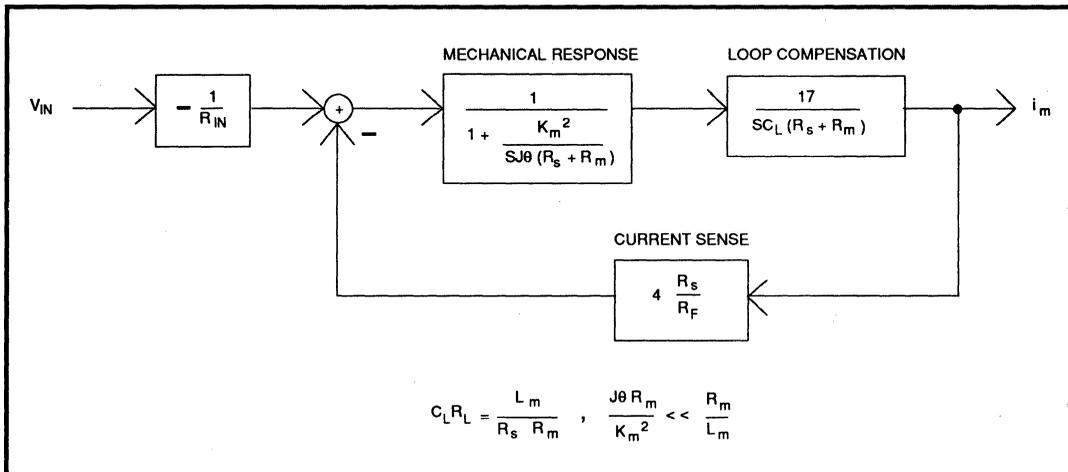
FIGURE 4(B): Simplified Transfer Function Of
