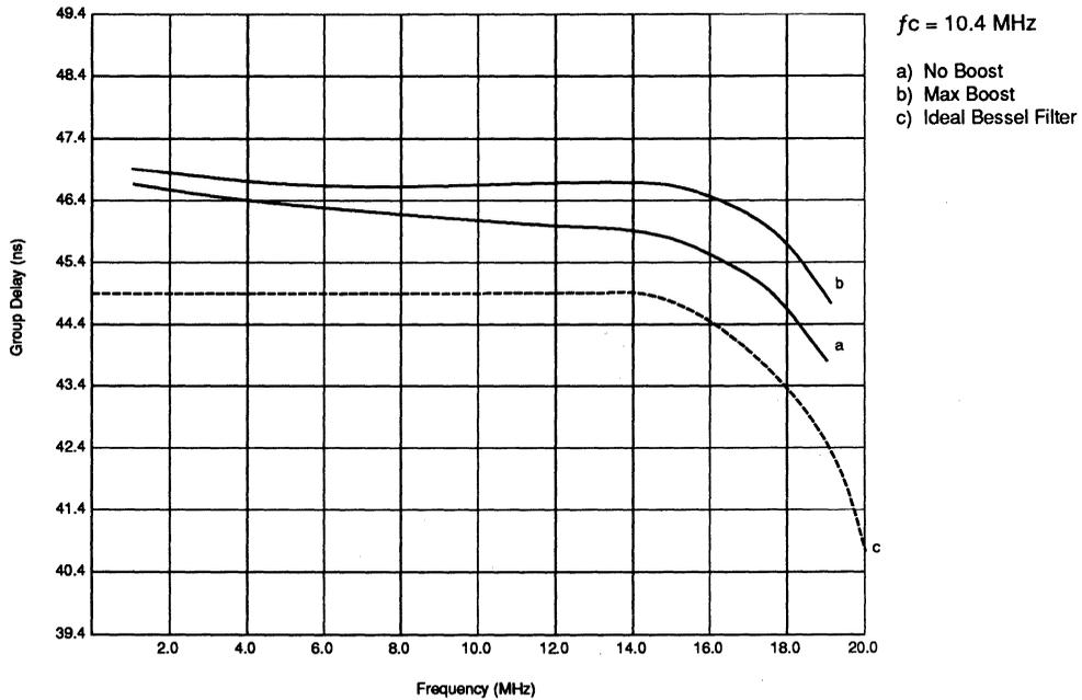
**FIGURE 3: 32F8011/8012 Typical Group Delay Variation (Differentiated Output)**
