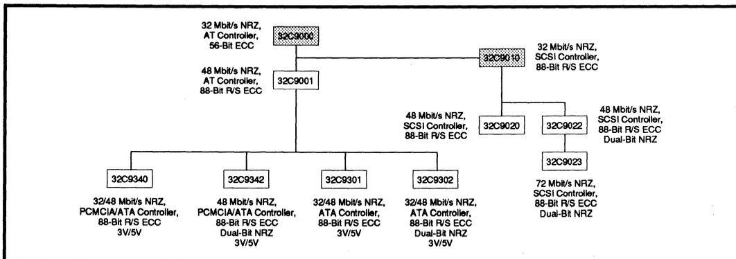
**FIGURE 1: Silicon Systems' Disk Controller Chip Hierarchy**
