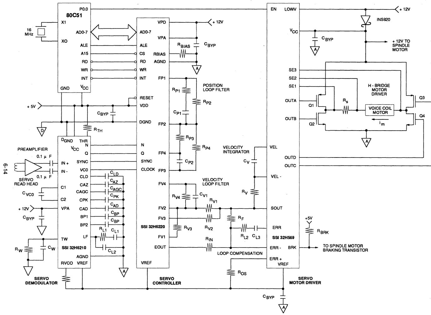
FIGURE 10: Complete Example of Servo Path Electronics Using the SSI 32H6210/ 6220/ 569
