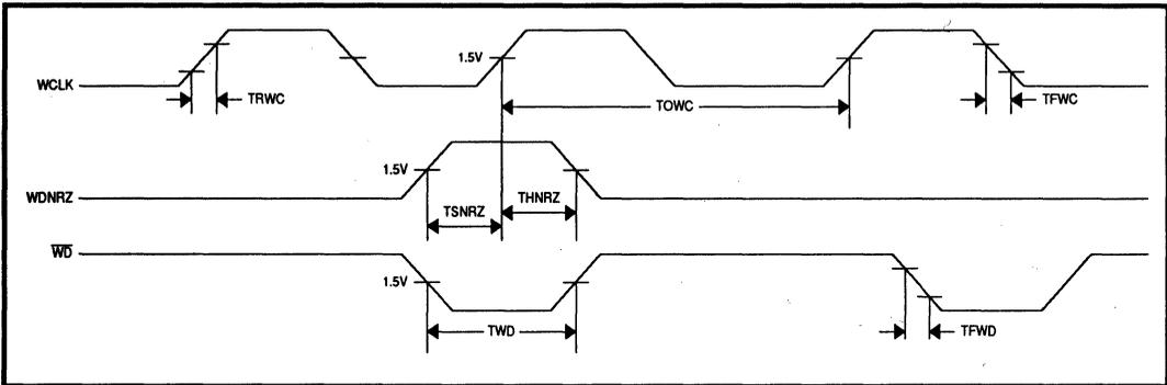
**FIGURE 4: Write Timing**
