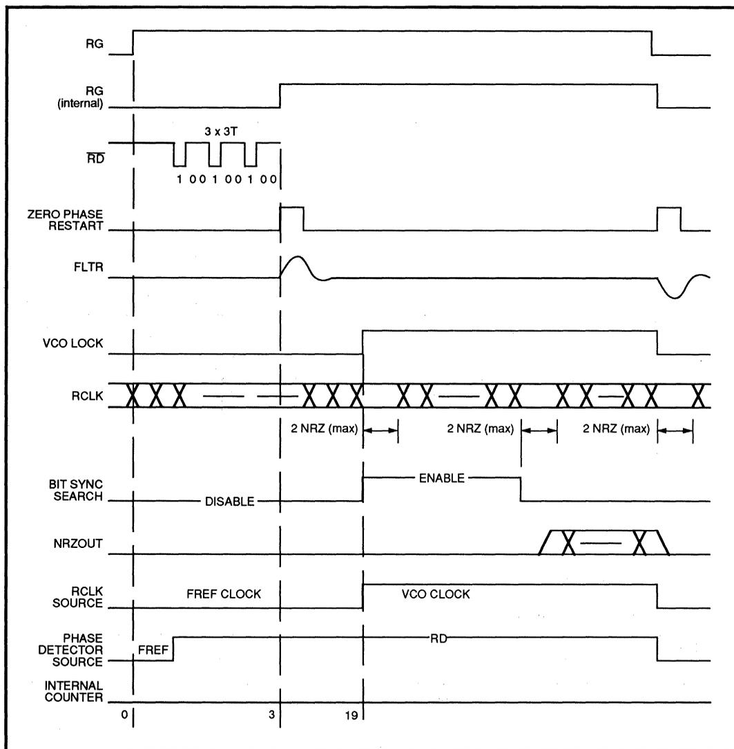
FIGURE 8: Read Mode Locking Sequence
