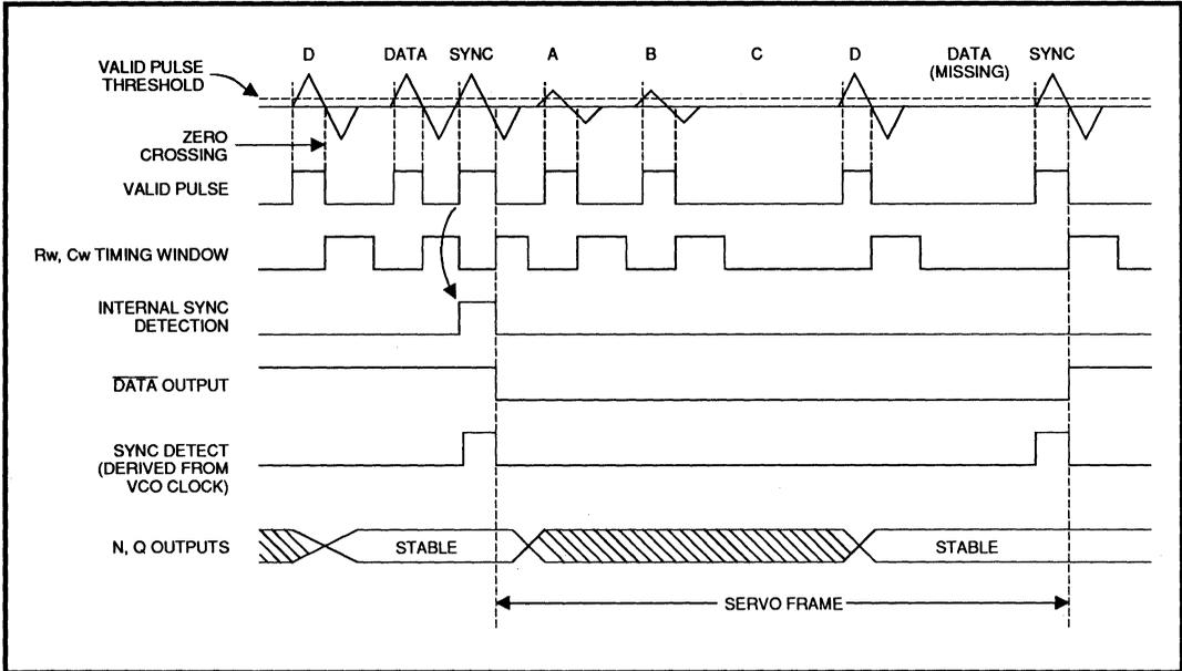
FIGURE 6 : Sync and DATA Pulse Detection
