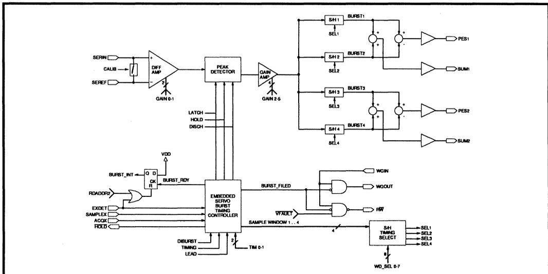
FIGURE 3: Embedded Servo Burst Amplitude Processor & Timing Controller
