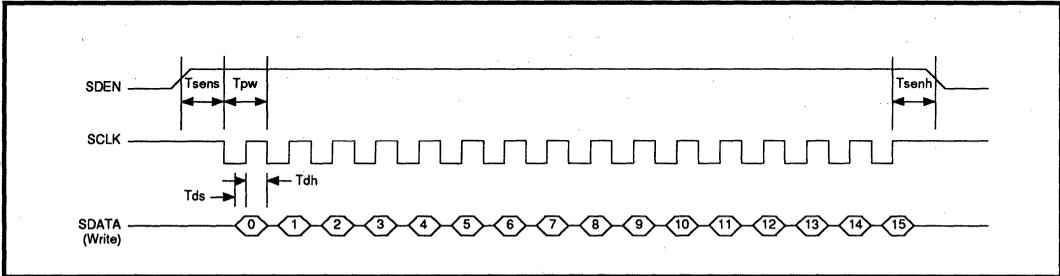
FIGURE 2: SSI 32H6811 Serial Interface Timing Diagram
