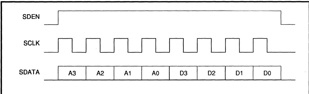
FIGURE 1: Serial Port Timing
