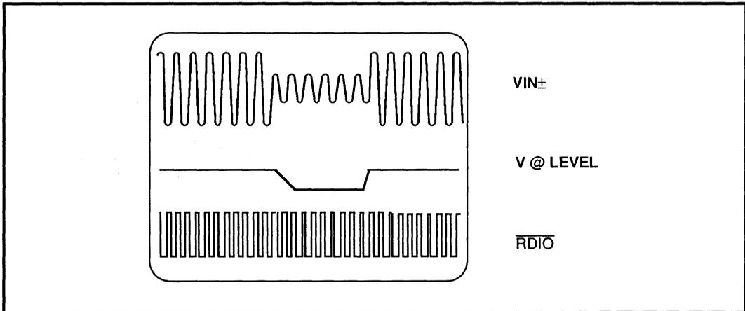
PHOTO 4.1.2: Qualification threshold at 50%; 330 pF from LEVEL to VPA. Input changes from 100 mVppd to 40 mVppd. Proper qual threshold time constant  $\gg$  All  $\overline{RDIO}$  pulses present.
