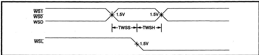
**FIGURE 9: Window Symmetry Control Timing**
