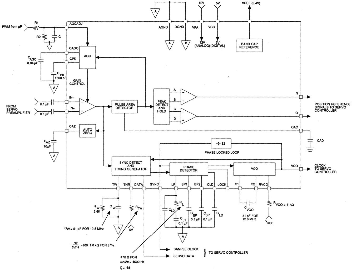
FIGURE 8: Design Example for 400 kHz Frame Rate
