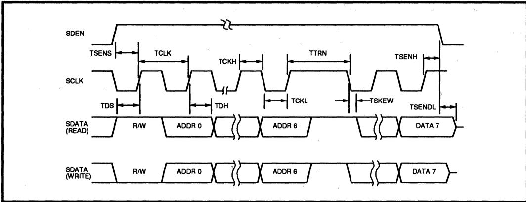
FIGURE 13(b): Serial Port Timing Information
