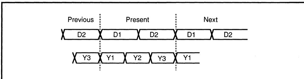
FIGURE 8.3.1: Definition of Y1-3 & D1-2 in Encode Table
