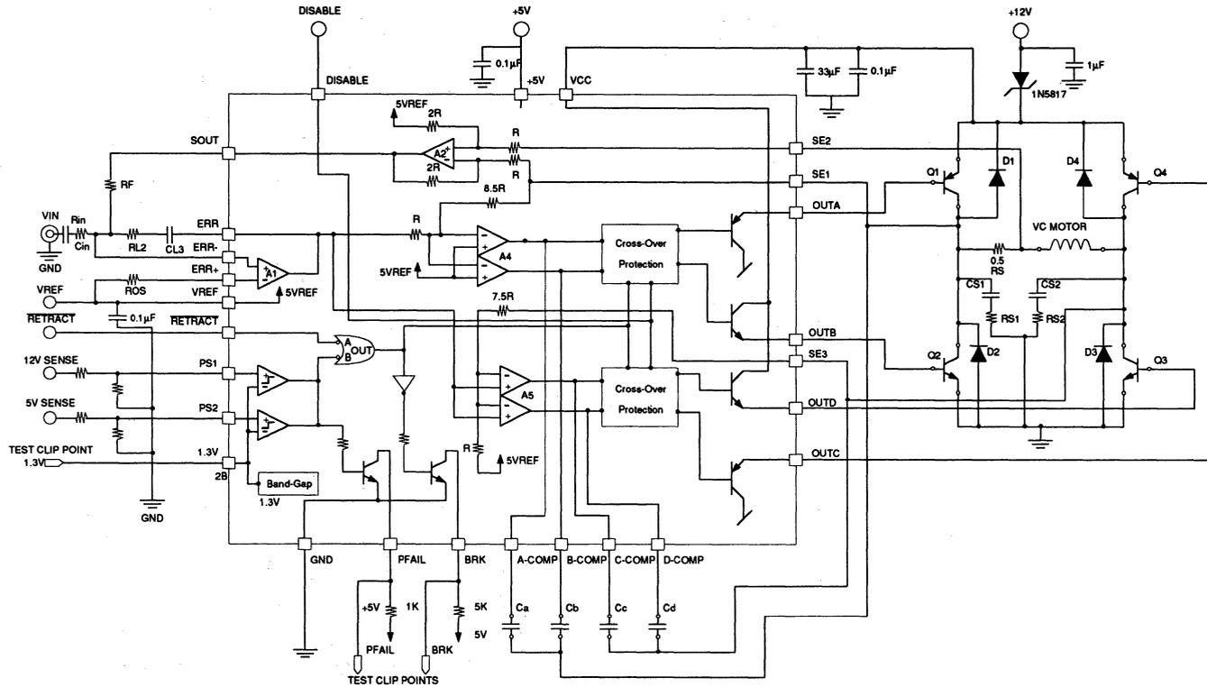
FIGURE 2: SSI 32H6240 Typical Application
