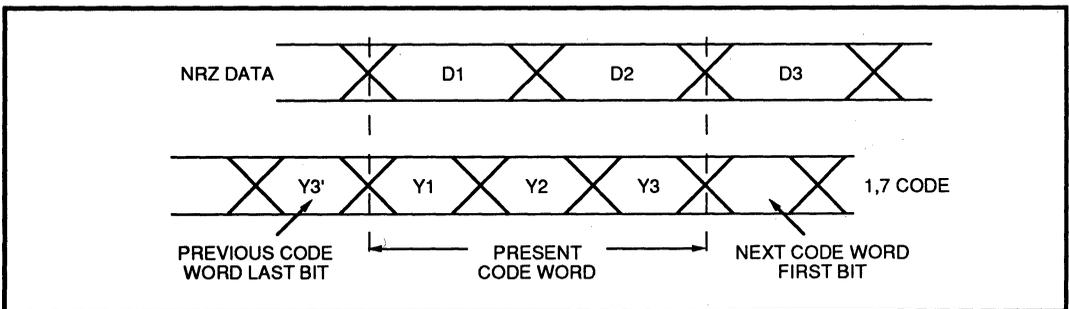
**FIGURE 6: NRZ Data Word to 1,7 Code Word Bit Comparison**
