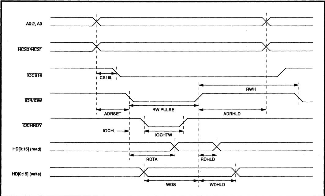
**FIGURE 16: Host Programmed I/O 8-16 Bit Timing**
