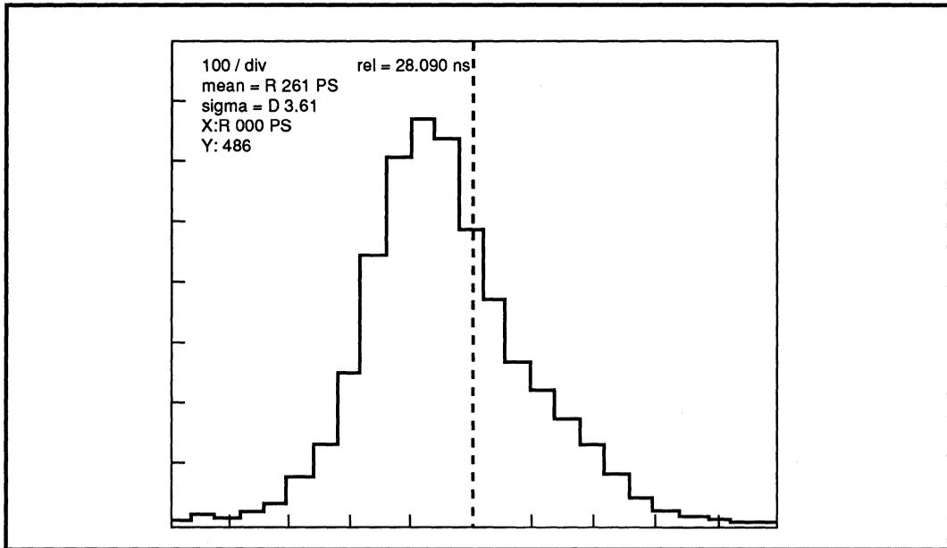
Figure 5: Histogram of RD Periods with 18 MHz Sinusoidal Input
