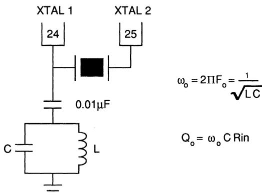
The typical input impedance looking into XTAL1 is approximately  $R_{in} = 250\Omega$ . It is recommended to design the value of  $Q_0$  at approximately 10 to 15. Therefore, a resonant frequency of  $F_0 = 20$  MHz would result in  $L \cong 0.16 \mu H$  and  $C \cong 380$  pF.
