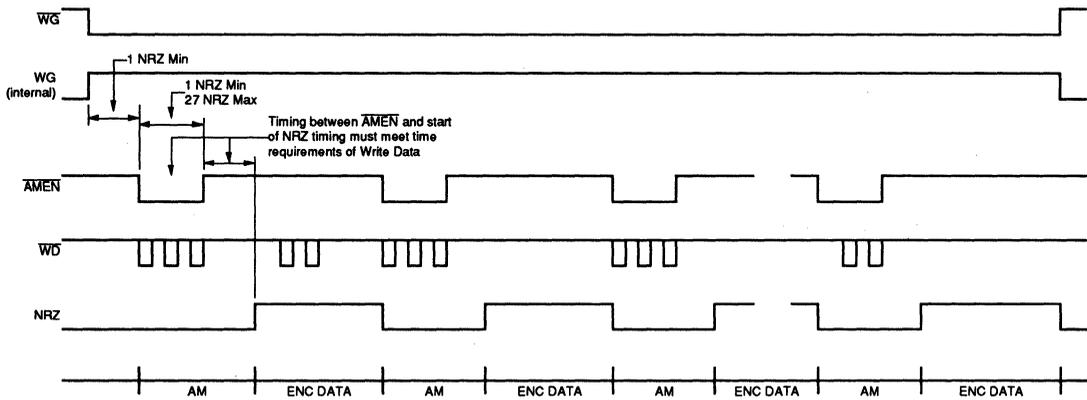
**FIGURE 11: Multiple Address Mark Write**
