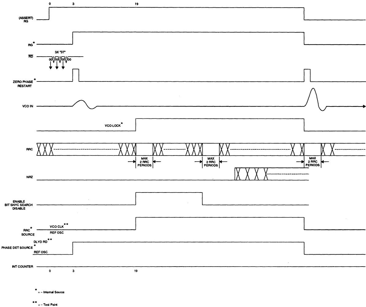
**FIGURE 8: Read Mode Locking Sequence (Soft and Hard Sector)**
