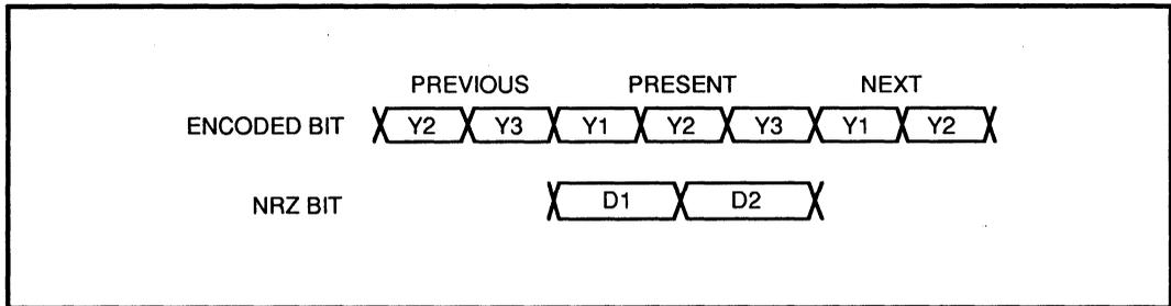
**FIGURE 14: Definition of Y1-3 & D1-2 for Decode Table**
