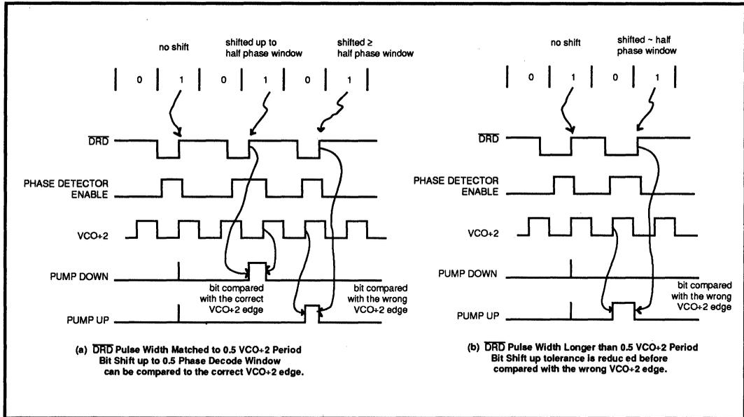
FIGURE 4.4.3: SSI 32P4730/4731 Data Separator Phase Decode Window Asymmetry causes bit shift tolerance reduction.
