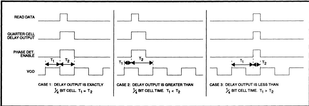
**FIGURE 15B: Timing of Phase Detector Enable Logic.** The read data input pulse can shift to the left by  $T_1$  and to the right by  $T_2$  before an error occurs in the phase detector output polarity. If the quarter cell delay output is not exactly  $\frac{1}{4}$  bit cell wide, then  $T_1 \neq T_2$ , as shown in cases 2 and 3.
