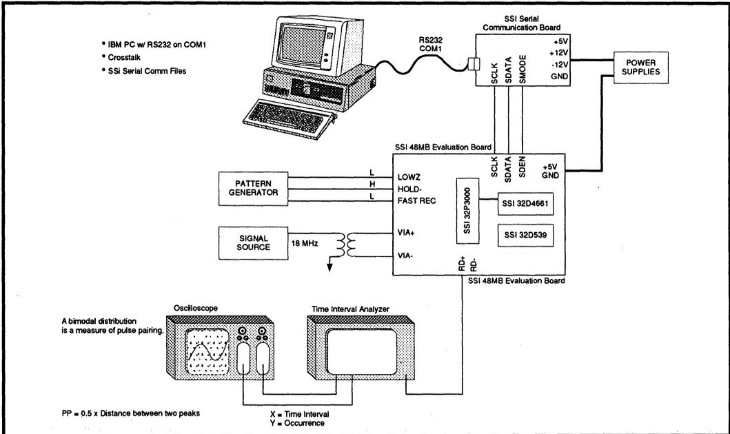
Figure 4: SSI 32P3000 Evaluation Board Pulse Pairing Setup
