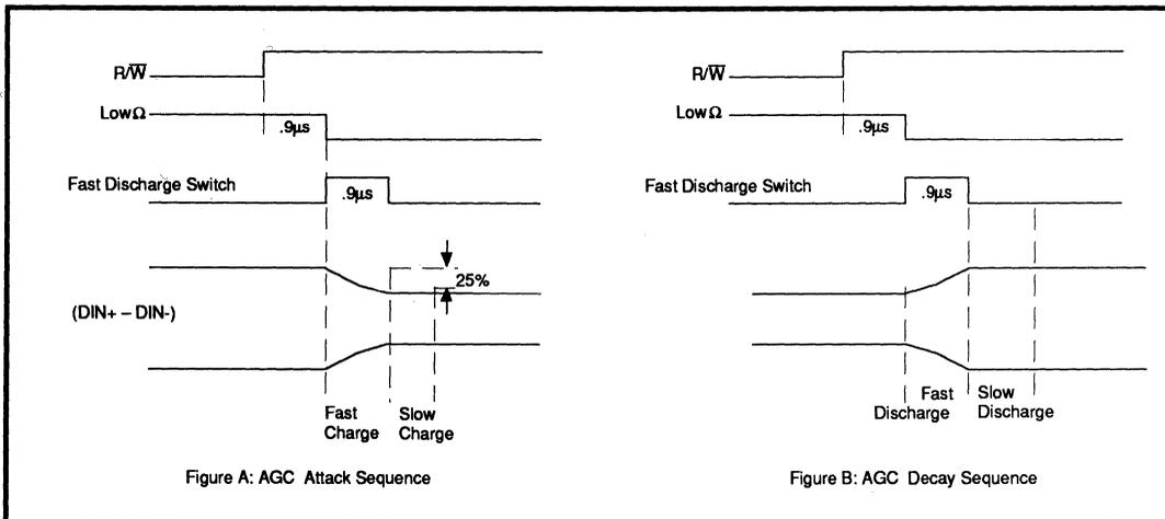
**FIGURE 6: AGC Timing Diagram**
