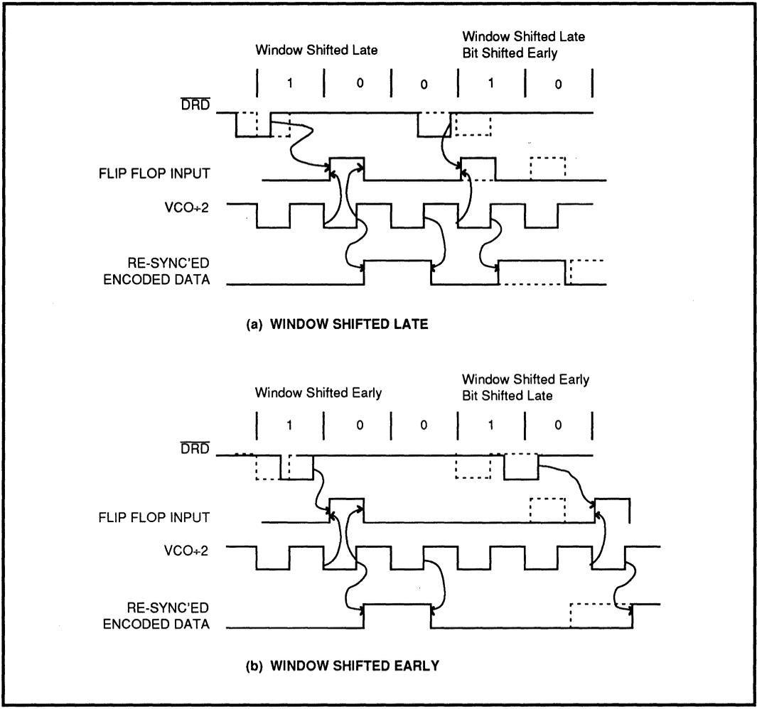
FIGURE 4.8.1: Window Shift Function Illustration
