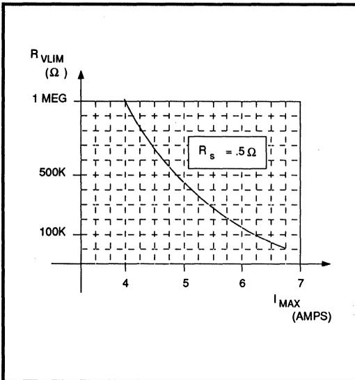
**FIGURE 6: RVLIM To Ground Typical Motor Current Limit**
