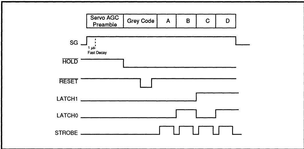
**FIGURE 5.1.1: SSI 32P4730 Servo Control Sequence**
