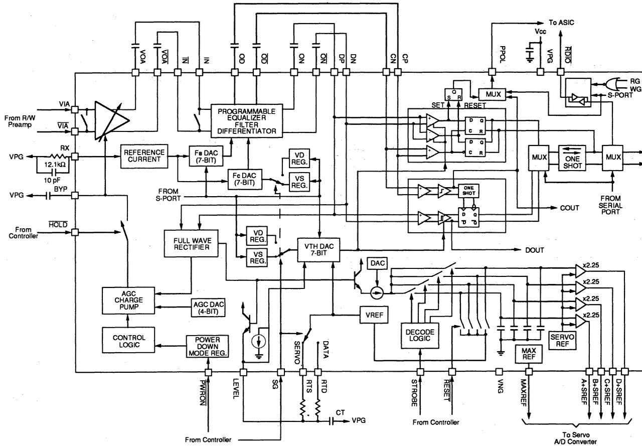
**FIGURE 15A: 32P4731/41 Application Diagram**
