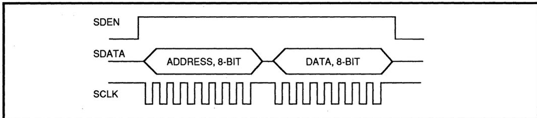
**FIGURE 13(a): Serial Port Data Transfer Format**
