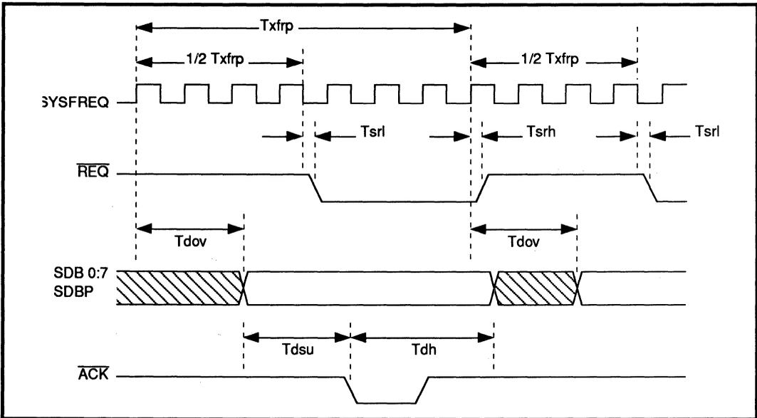
**FIGURE 17: Odd Number of SYSFREQ Cycles/SCSI Transfer Period**
