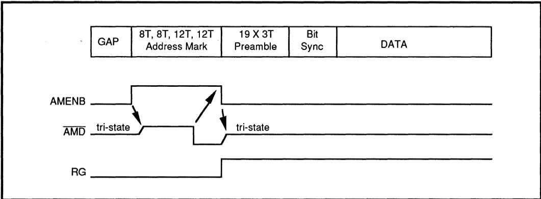
FIGURE 4.7.1: Read Mode Soft Sector Timing
