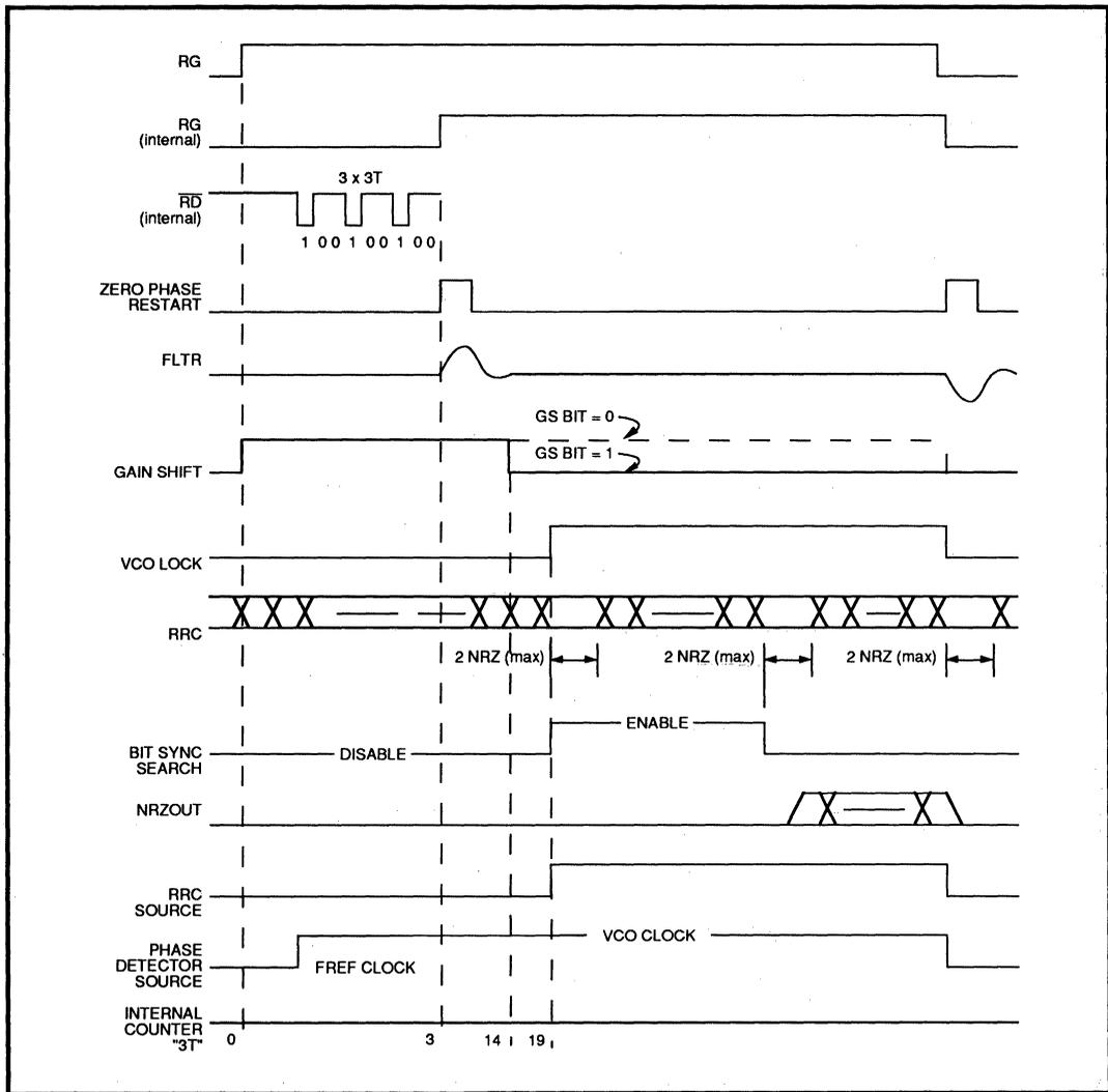
FIGURE 11: Read Mode Locking Sequence (Hard and Soft Sector)
