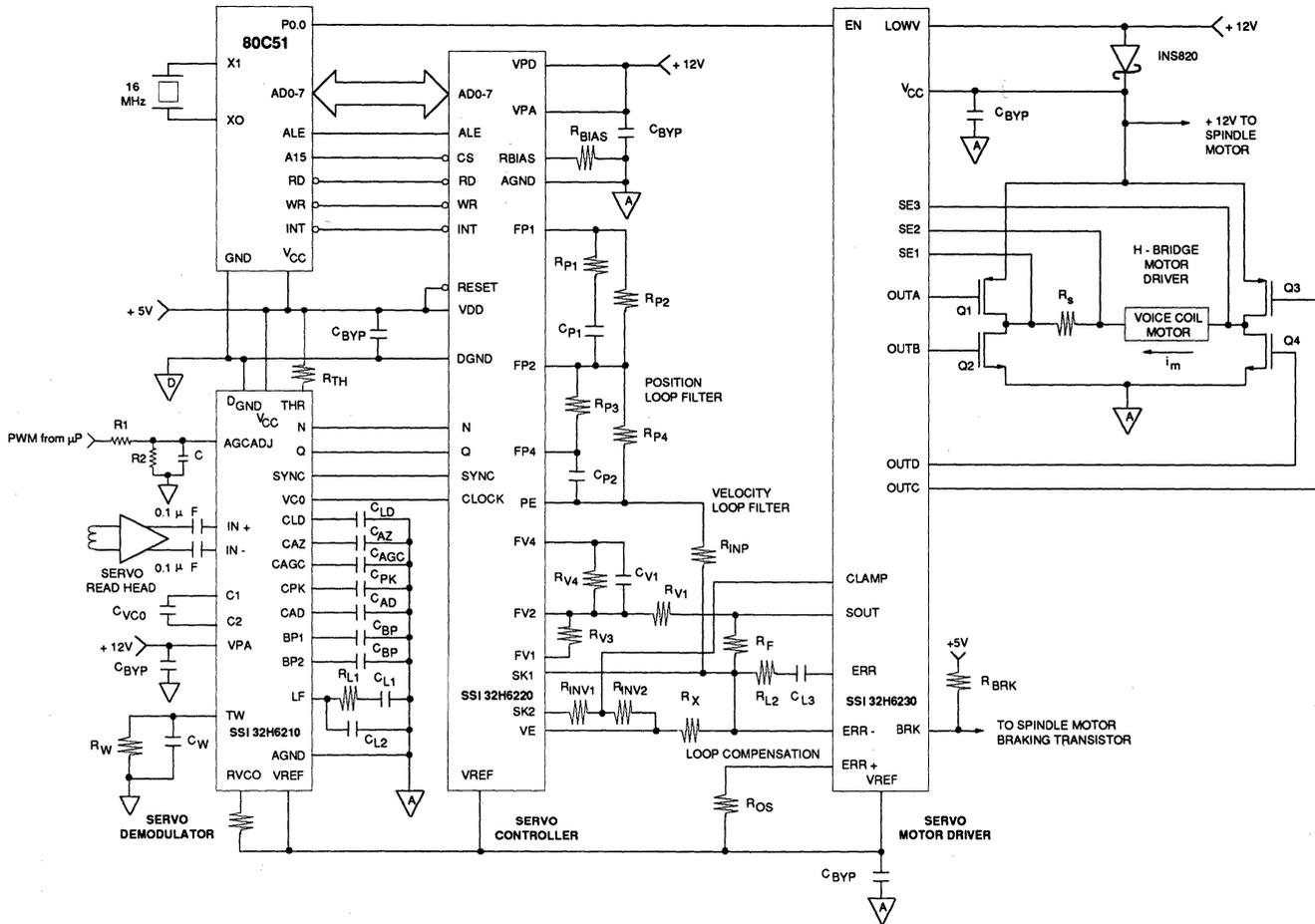
FIGURE 9: Complete Example of Servo Path Electronics Using SSI 32H6210/6220/6230 Chip Set
