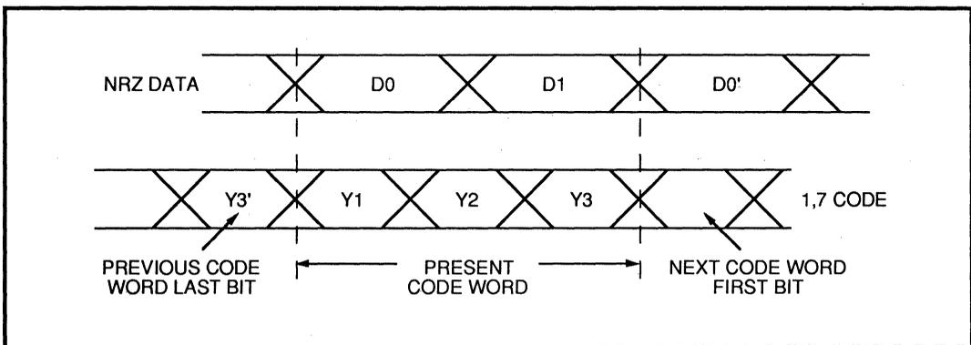
**FIGURE 6: NRZ Data Word to 1,7 Code Word Bit Comparison**
