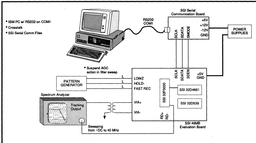
Figure 6: SSI 32P3000 Evaluation Board Filter Characteristic Setup
