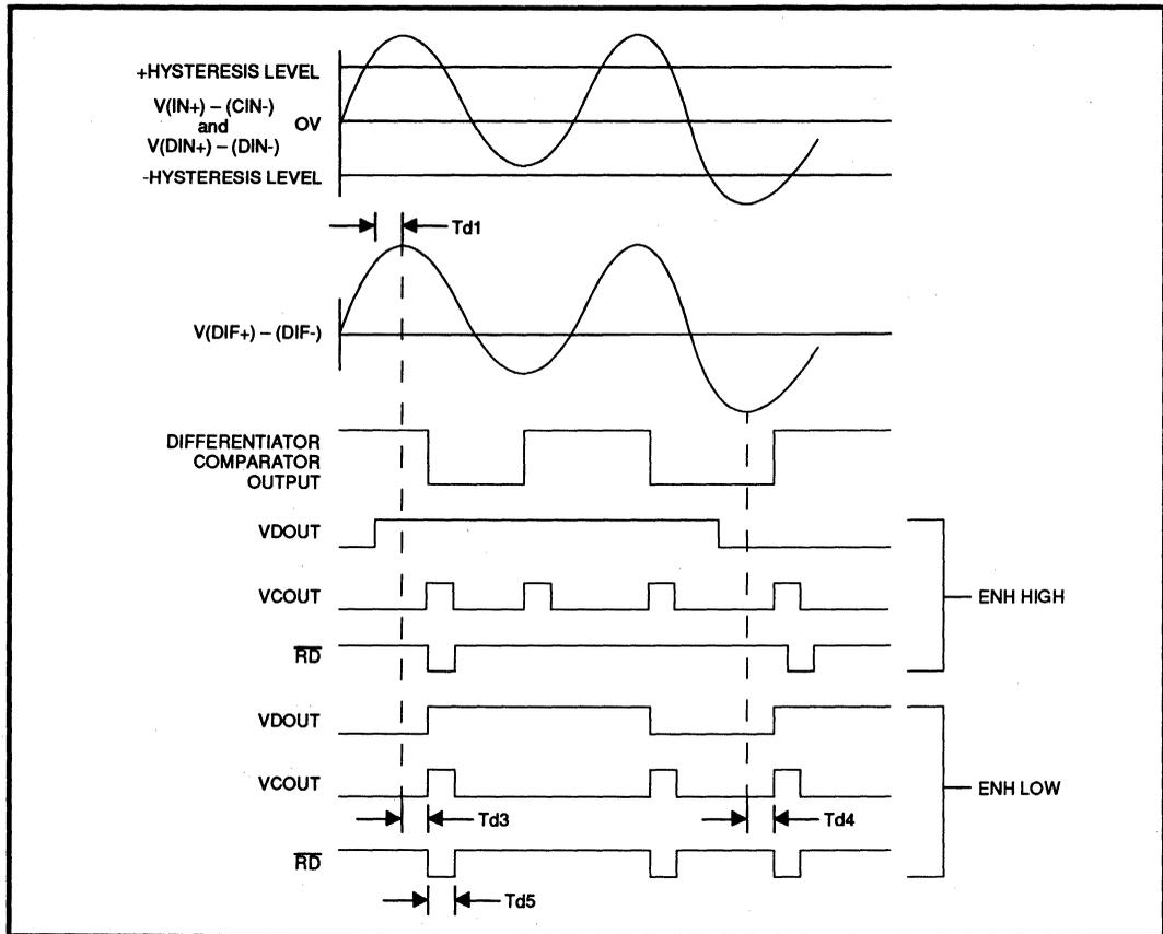
FIGURE 7: Read Mode Digital Section Timing Diagram
