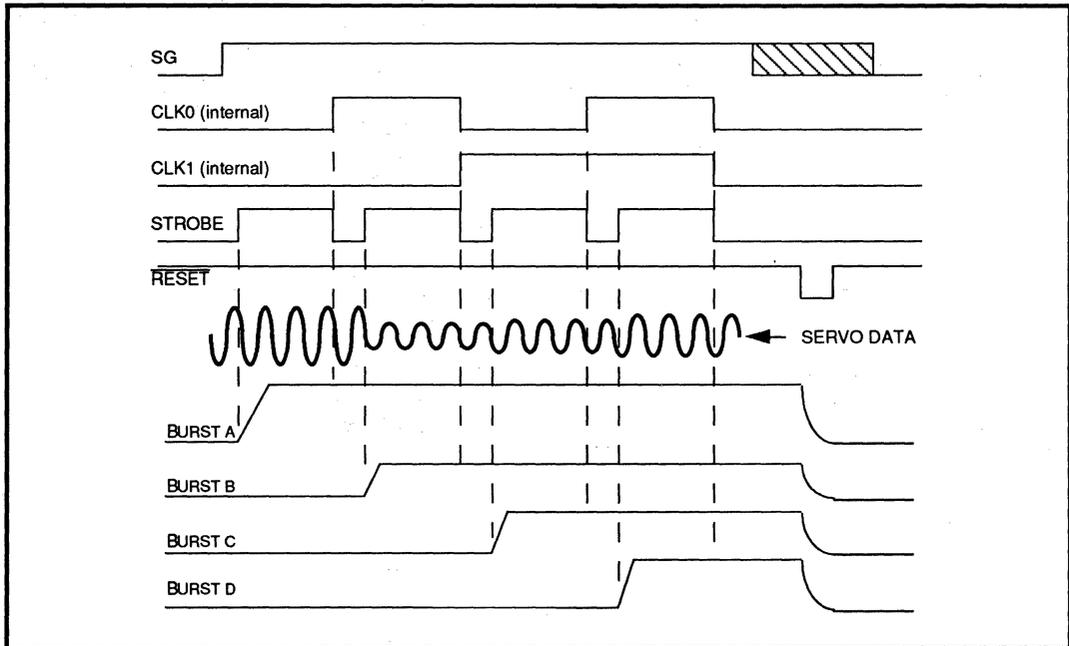
FIGURE 3: Servo Capture Timing
