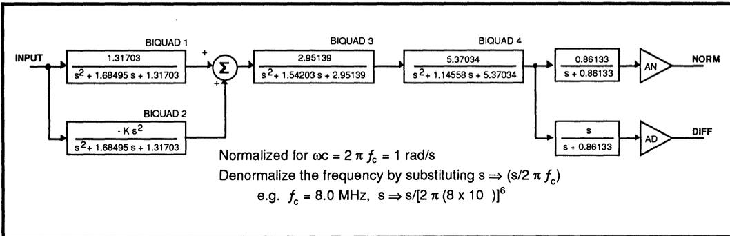
FIGURE 4.2.1: Programmable Filter Normalized Transfer Function
