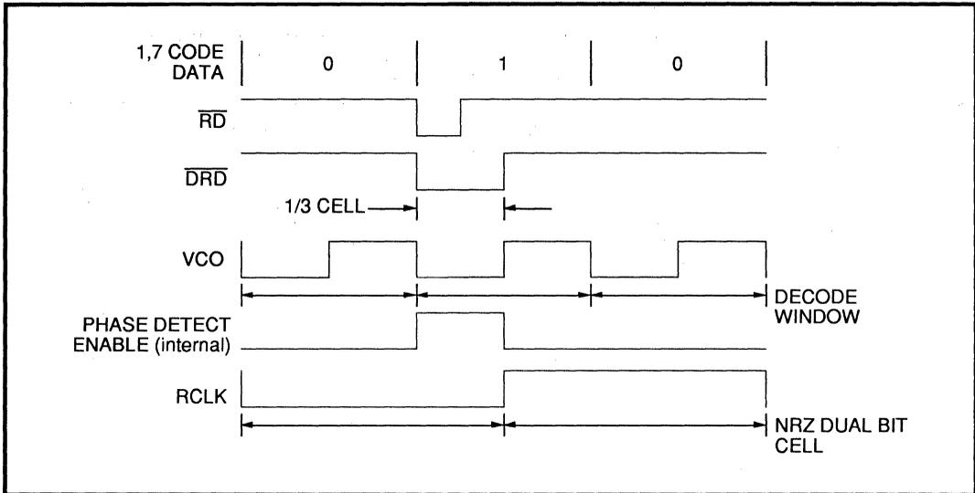
**FIGURE 5: Data Synchronization Waveform**
