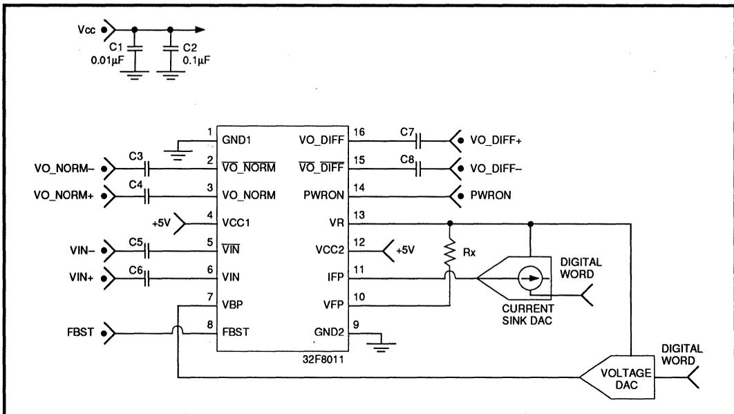
FIGURE 4: The SSI 32F8011 Setup Schematic Using a Current Source DAC for Cutoff Frequency Control
