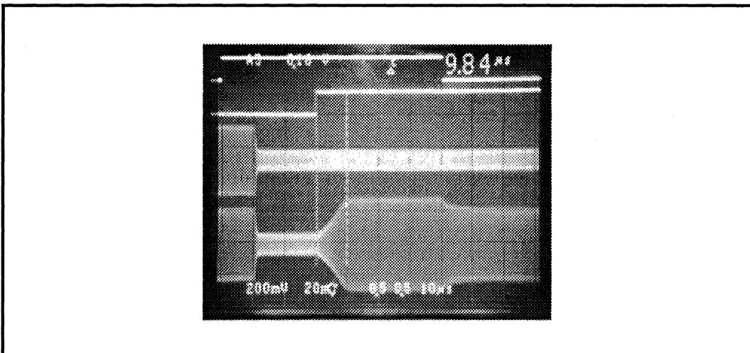
**Figure 11: AGC Recovery With FAST REC**
