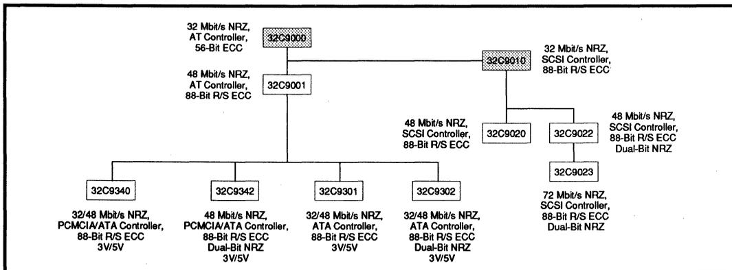
FIGURE 1: Silicon Systems' Single Chip Controller Hierarchy
