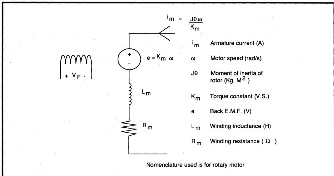
FIGURE 3: Equivalent Circuit For Fixed Field DC Motor
