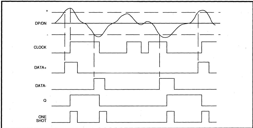
FIGURE 2(a): Dual Comparator Timing Diagram
