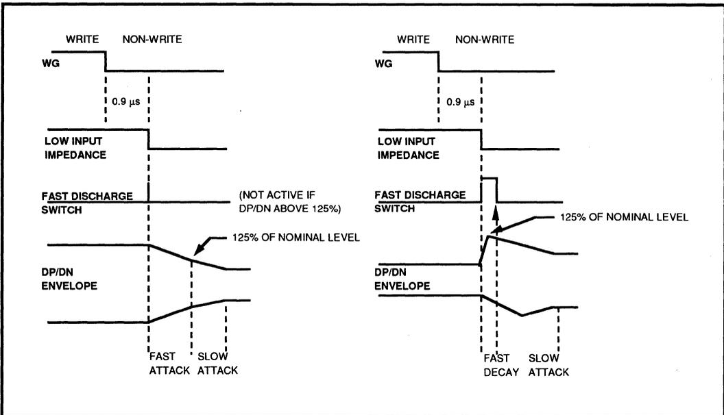
FIGURE 4.1.1: AGC Action Timing in Write-to-Read Recovery
