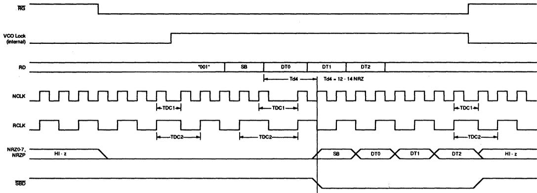
**FIGURE 10: Read Mode NRZ Data Timing**
