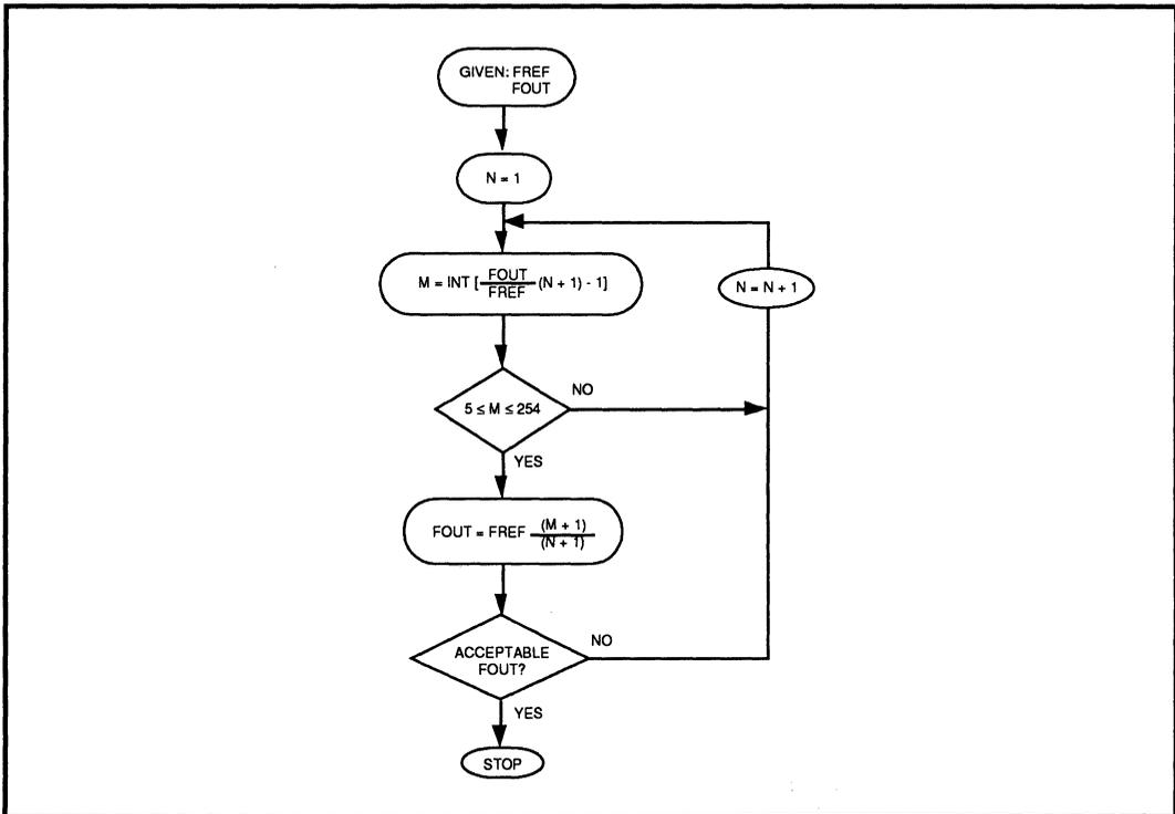
FIGURE 4.3.2: M & N Codes for Time Base Generator
