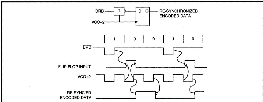
**FIGURE 4.4.5: Data Resynchronization Timing**
