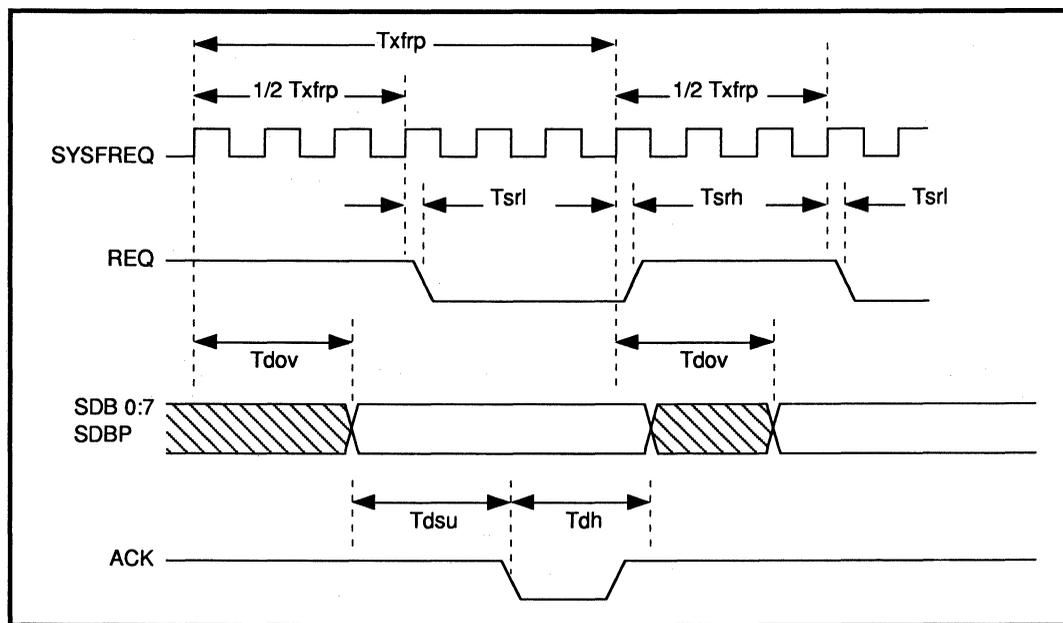
FIGURE 16: Even Number of SYSFREQ Cycles/SCSI Transfer Period
