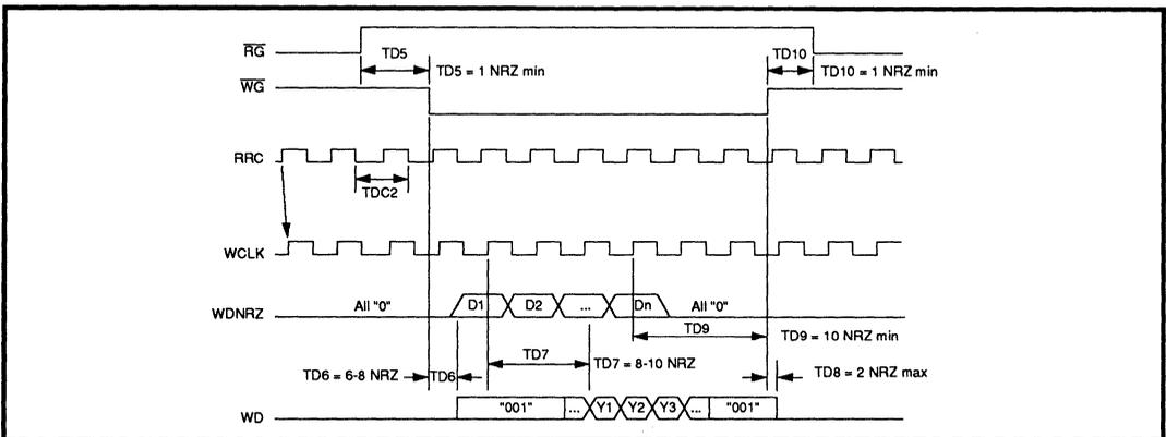
**FIGURE 6: Write Mode NRZ Data Timing**
