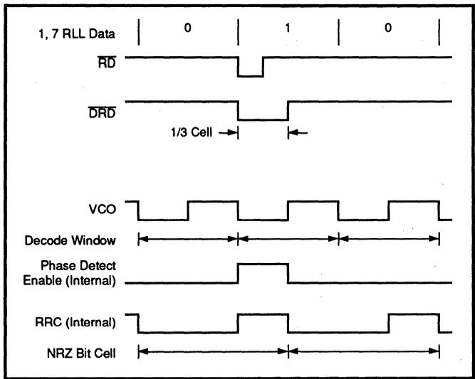
**FIGURE 3: Data Synchronization Waveforms**
