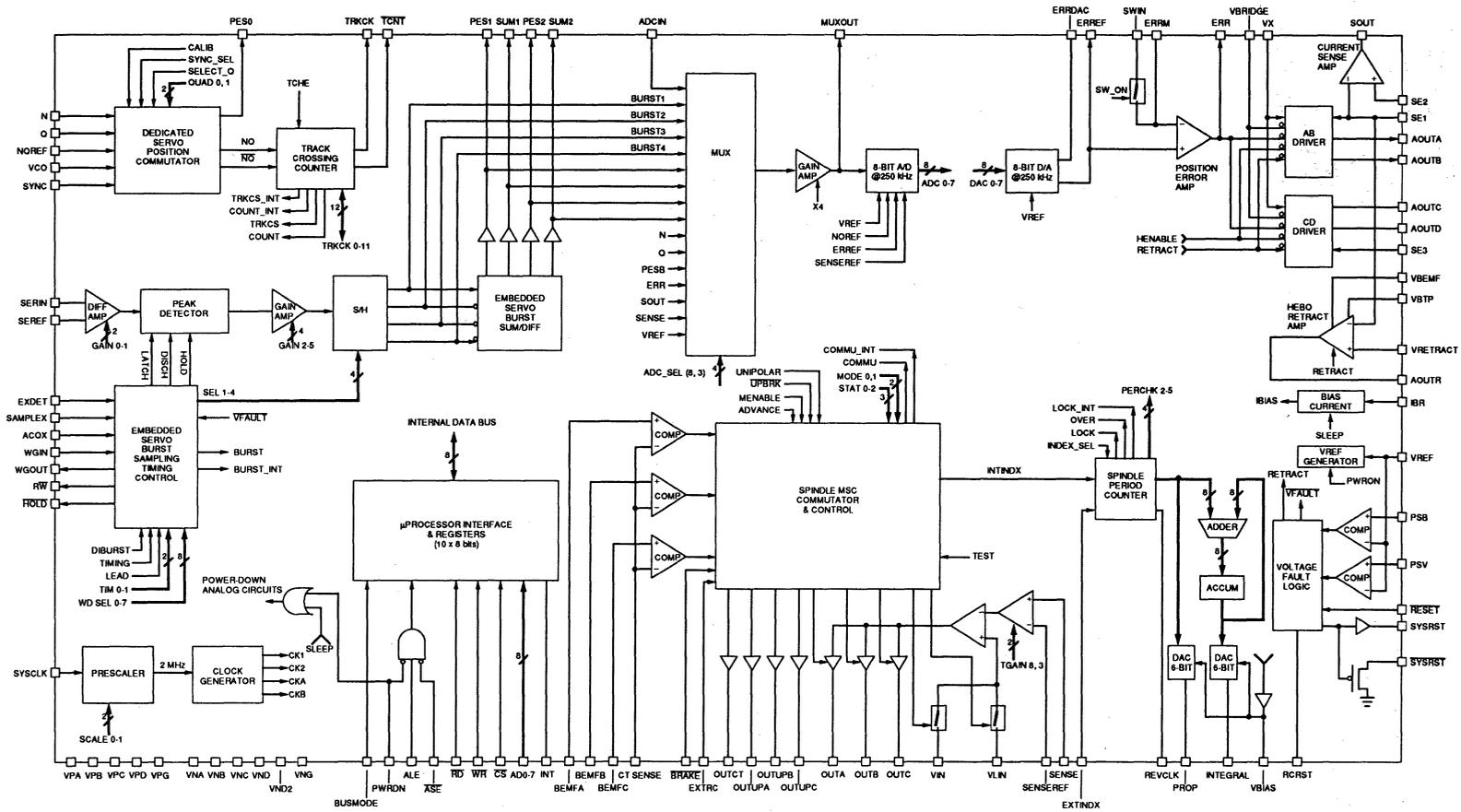
FIGURE 1: SSI 32H4633 Block Diagram
