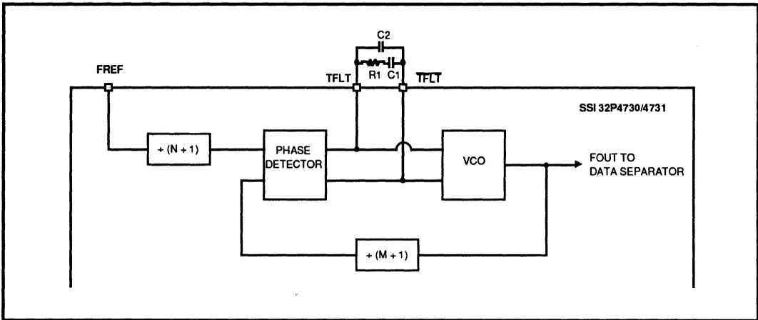
FIGURE 4.3.1: Time Base Generator Functional Model
