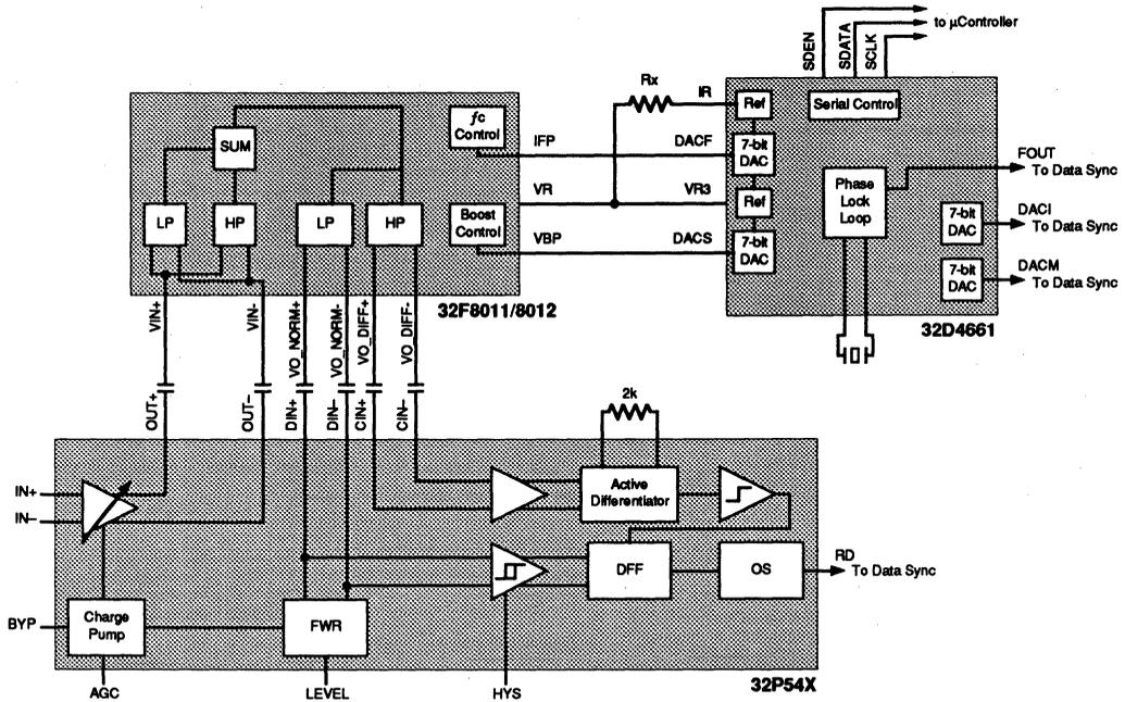
**FIGURE 2: Applications Setup, Constant Density Recording
