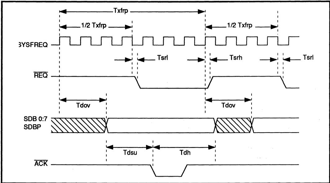
**FIGURE 18: Odd Number of SYSFREQ Cycles/SCSI Transfer Period**
