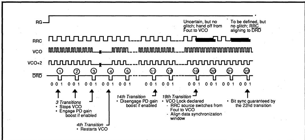
FIGURE 4.4.1: SSI 32P4730/4731 Regeneration Process
