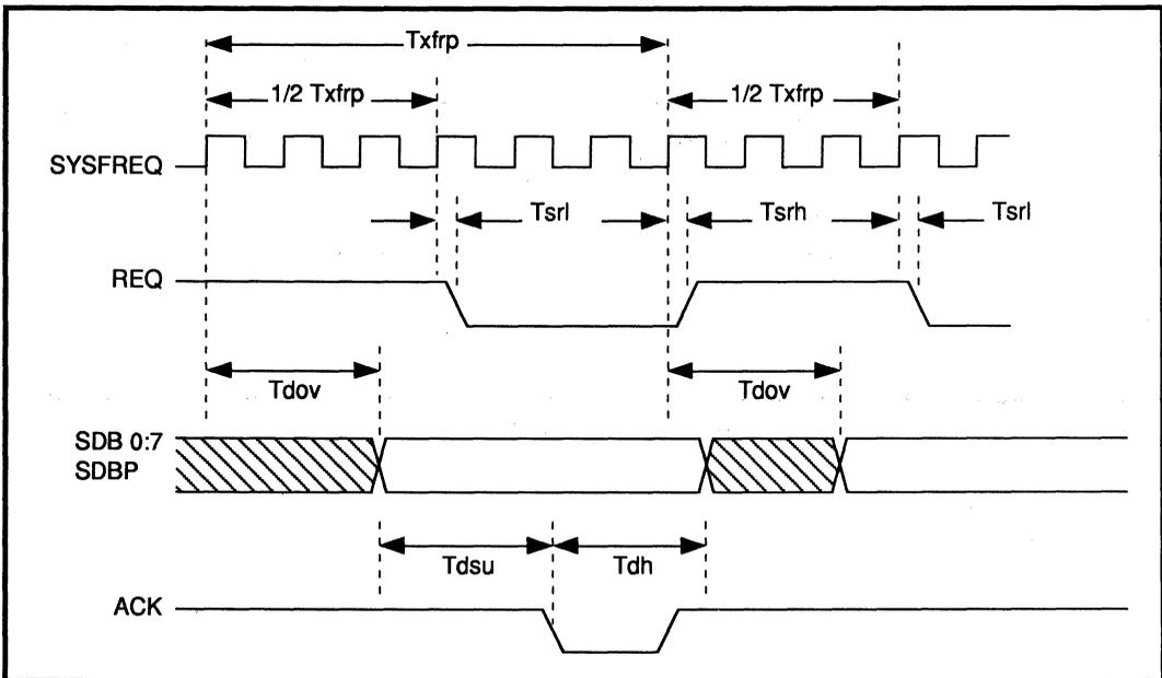
FIGURE 17: Even Number of SYSFREQ Cycles/SCSI Transfer Period
