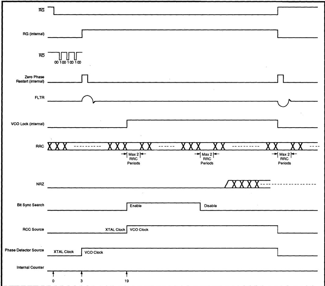
FIGURE 9: Read Mode Locking Sequence (Soft and Hard Sector)
