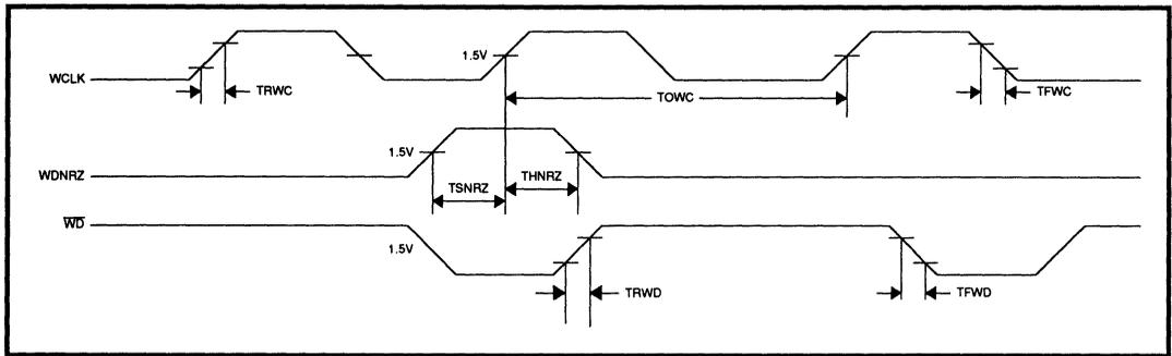
**FIGURE 6: Write Timing**
