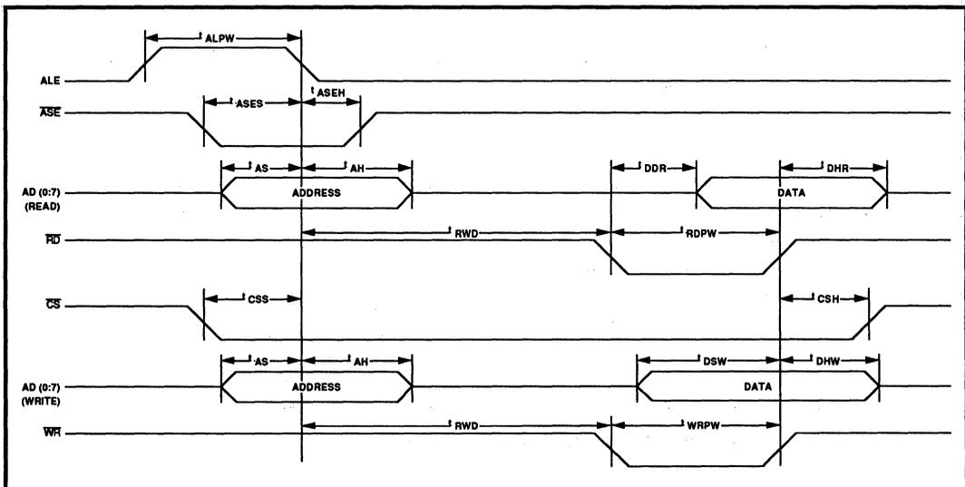
FIGURE 11: Intel Microprocessor Bus Interface Timing Diagram
