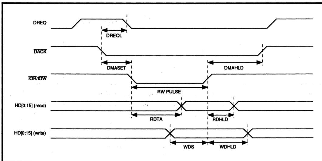
FIGURE 15: Host DMA 8/16-Bit Interface Timing
