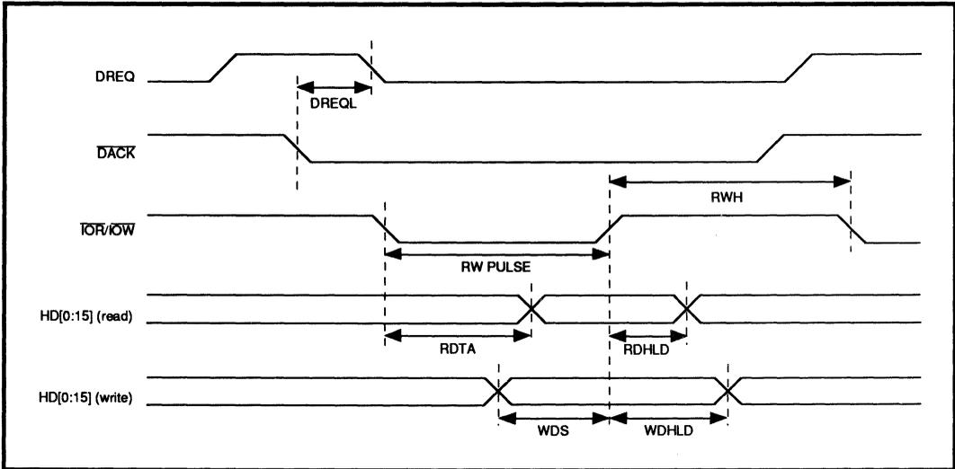
**FIGURE 15: Host DMA 8-16 Bit Interface Timing (Non-demand mode)**
