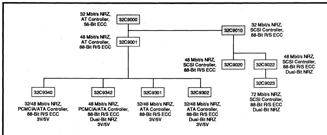
FIGURE 1: Silicon Systems's Disk Controller Chip Hierarchy
