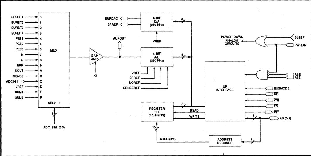
FIGURE 7: Data Acquisition & Microprocessor Bus Interface
