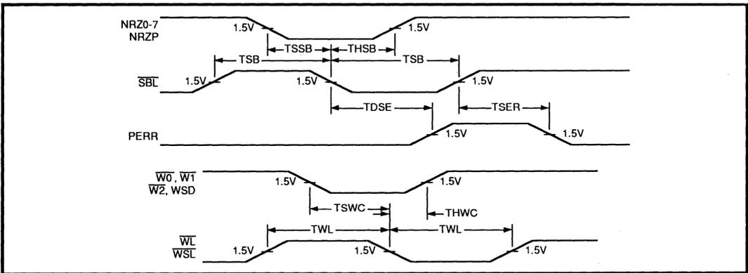
FIGURE 7: Control Timing
