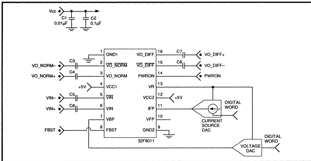
**FIGURE 5: The SSI 32F8011 Setup Schematic Using a Current Sink DAC for Cutoff Frequency Control**
