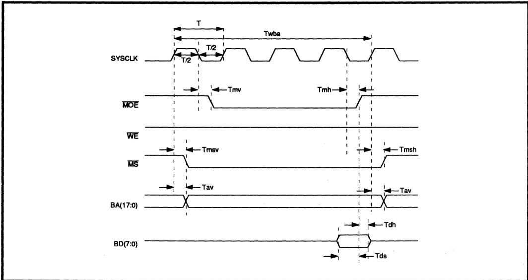
Note: Twba is a functional parameter that gives the duration of one RAM data buffer access cycle in SYSCLK periods. The value is programmed in bits 1-0 of register 54H. These examples show Twba = 4T.
