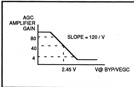
FIGURE 1: AGC Amplifier Gain vs  $V@BYP/VEGC$  Voltage
