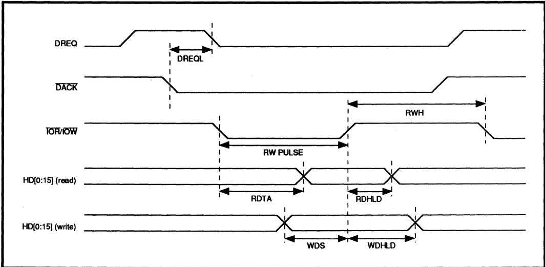
**FIGURE 15: Host Programmed I/O 8-16 Bit Timing**
