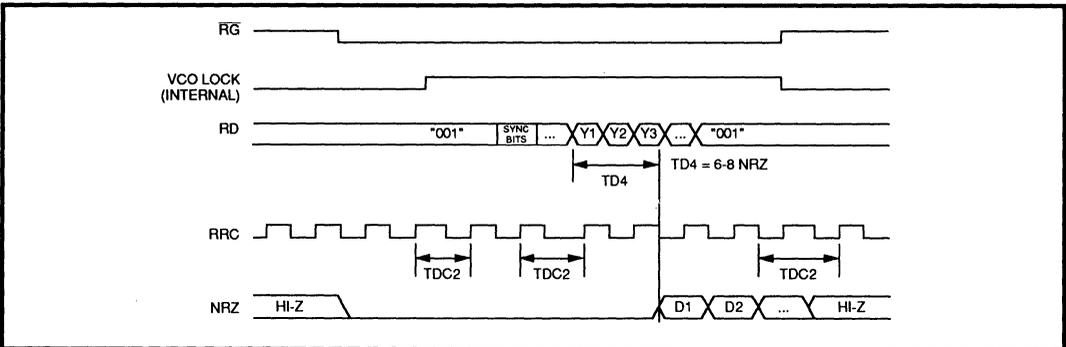
**FIGURE 5: Read Mode NRZ Data Timing**
