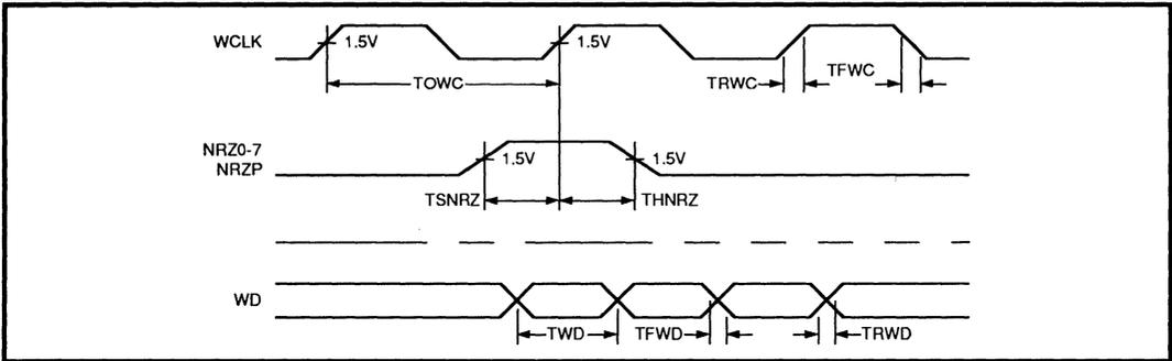
FIGURE 6: Write Timing
