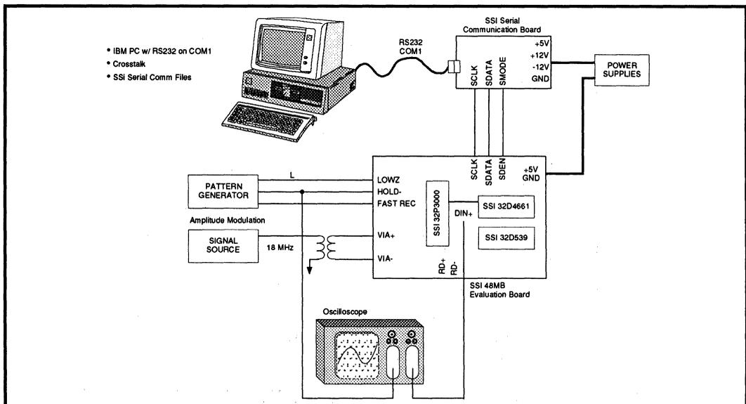
Figure 9: SSI 32P3000 Evaluation Board AGC Recovery Setup
