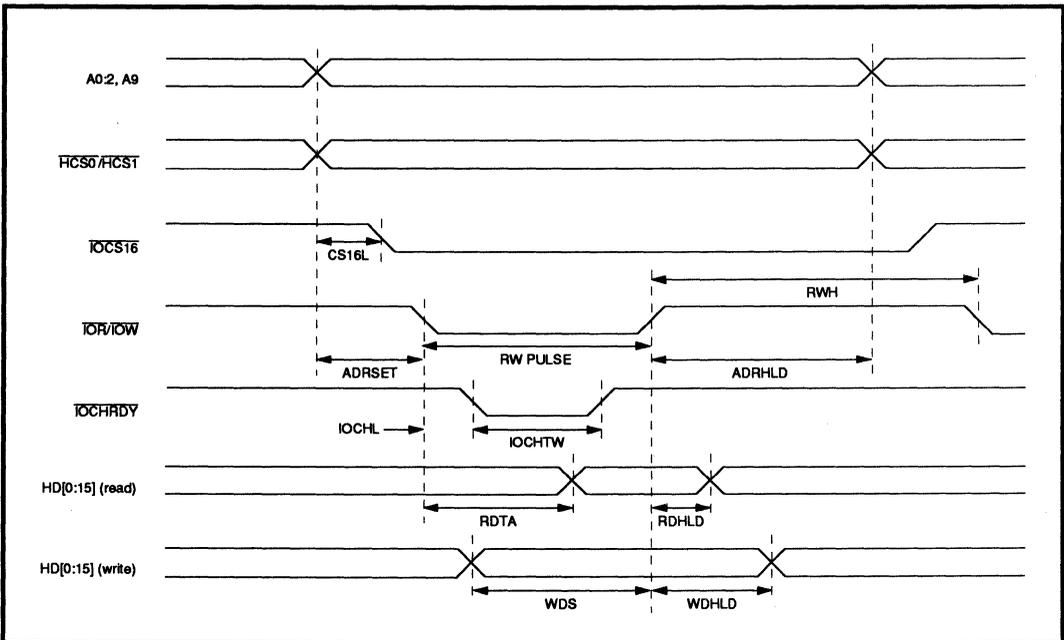
**FIGURE 16: Host DMA 8-16 Bit Interface Timing (Non-demand mode)**
