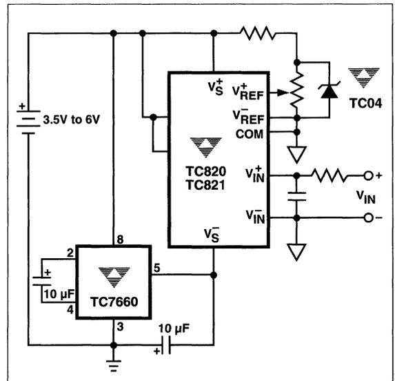
Figure 13. Powering the TC820/821 From a Low-Voltage Battery
