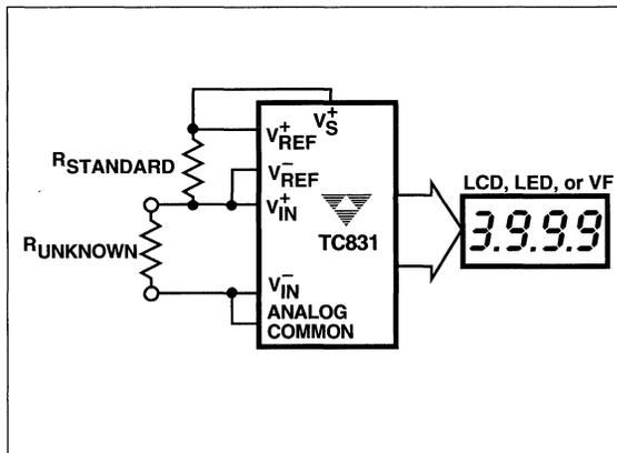
Figure 15. Low Parts Count Ratiometric Resistance Measurement
