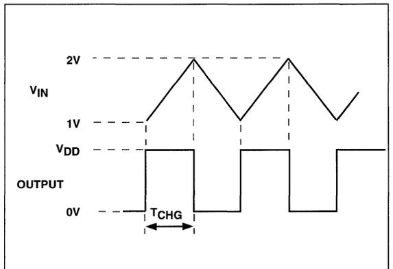
**Figure 3  $V_{IN}$  and Output Waveform**
