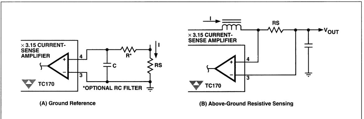
Figure 2 Resistive Sensing
