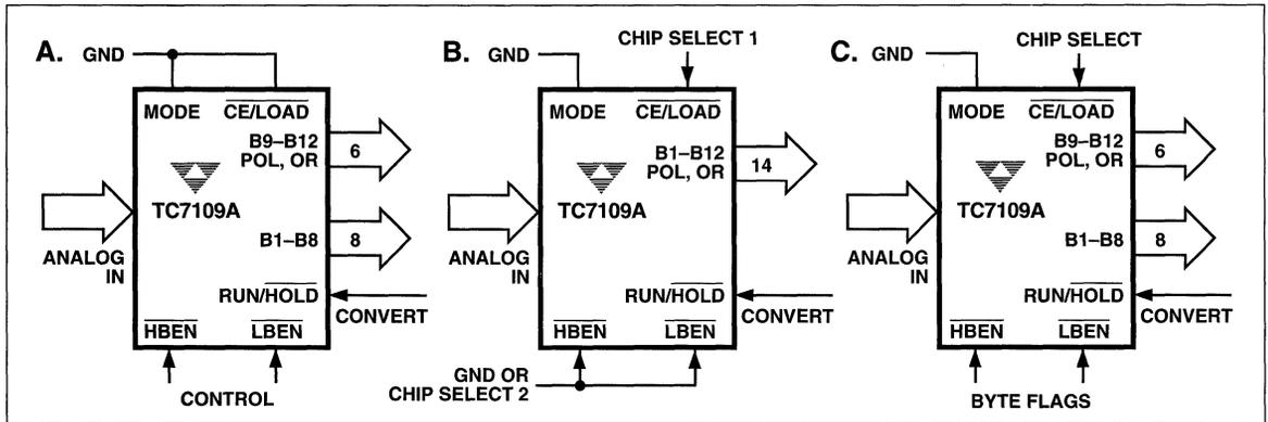
Figure 12 Direct Mode Chip and Byte Enable Combinations
