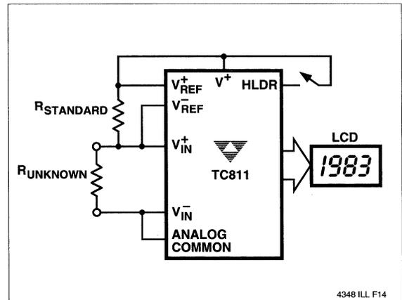
Figure 11 Low Parts Count Ratio Metric Resistance Measurement
