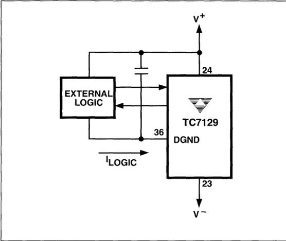
Figure 5 External Logic Referenced Directly to DGND
