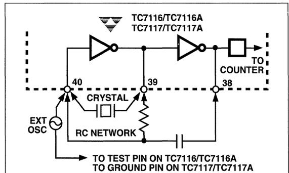
Figure 7 Clock Circuits
