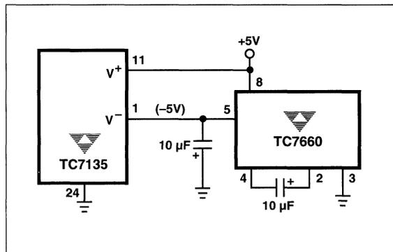
Figure 9. Negative Supply Voltage Generator
