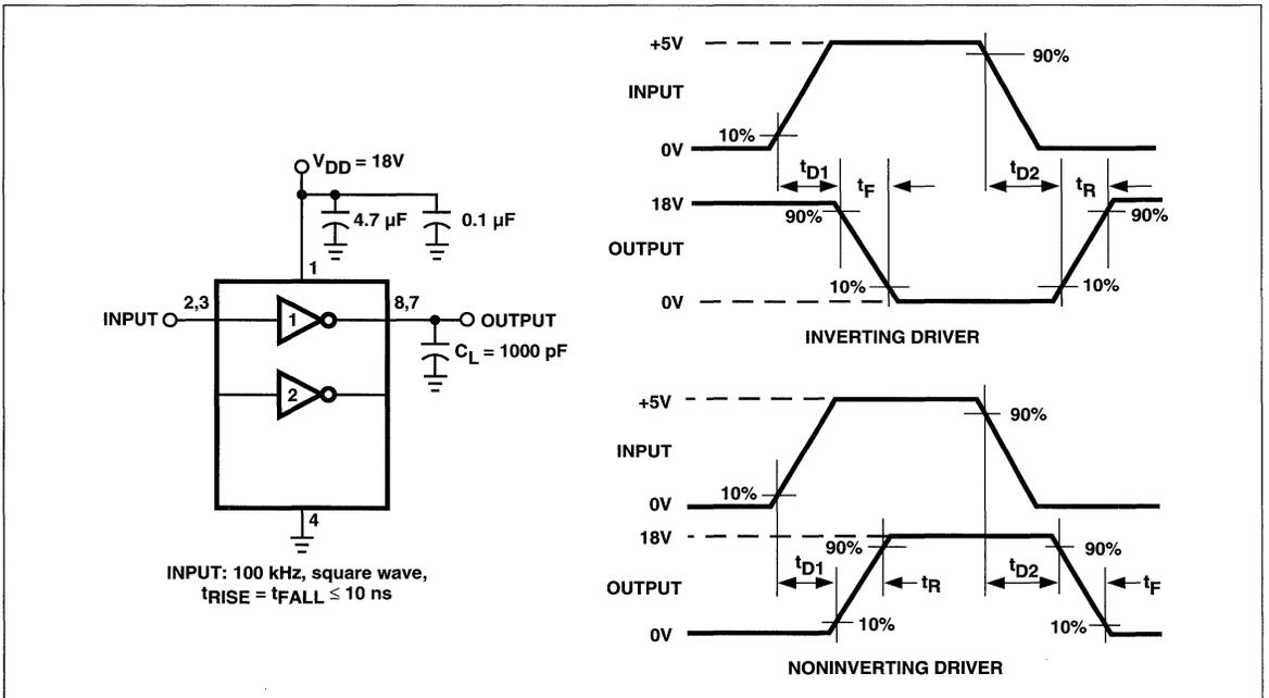
Figure 1 Switching Time Test Circuit
