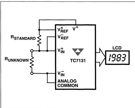
Figure 11 Low Parts Count Ratiometric Resistance Measurement
