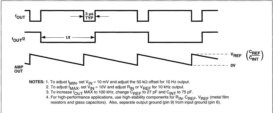
Figure 2 Output Waveforms
