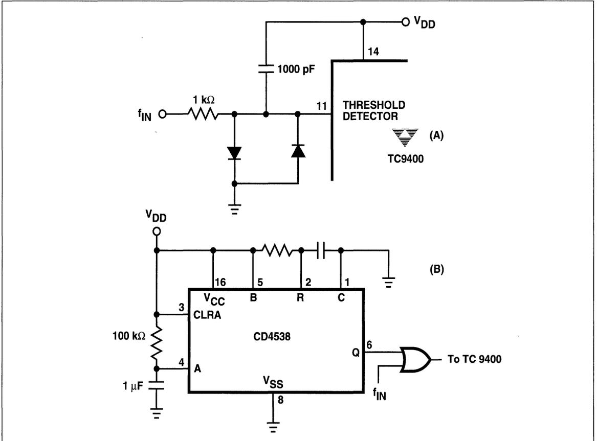
Figure 11 Power-On Operation/Reset
