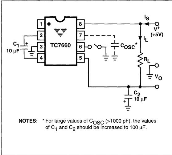
Figure 1. TC7660 Test Circuit
