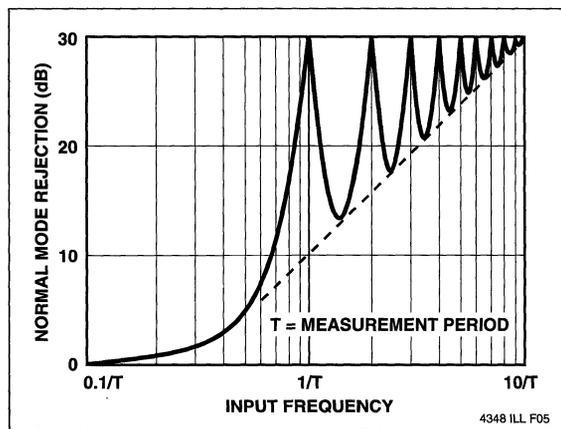
Figure 3 Normal-Mode Rejection of Dual Slope Converter
