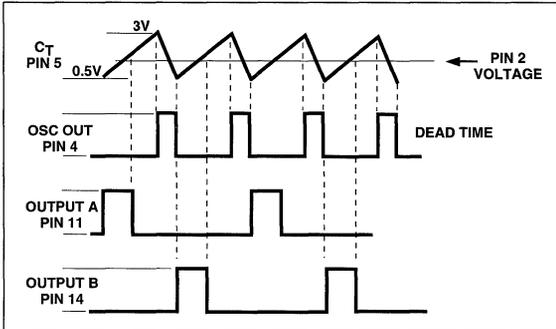
The 5K potentiometer sets a reference voltage at pin 2. When ramp voltage of pin 5 reaches this reference voltage, output drive pulse is active ON. Varying the discharge resistor will vary the dead time. Increasing the discharge resistor will effect an increase in the dead time.
