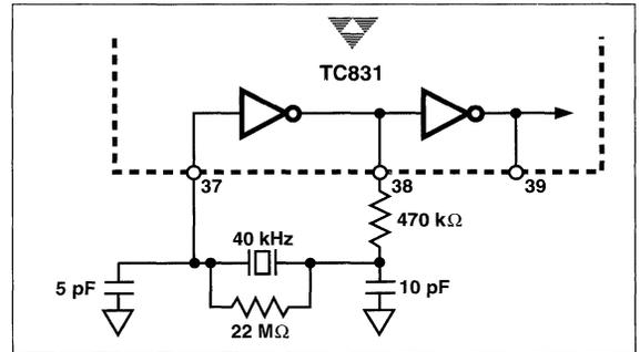
Figure 11. Suggested Crystal Oscillator Circuit
