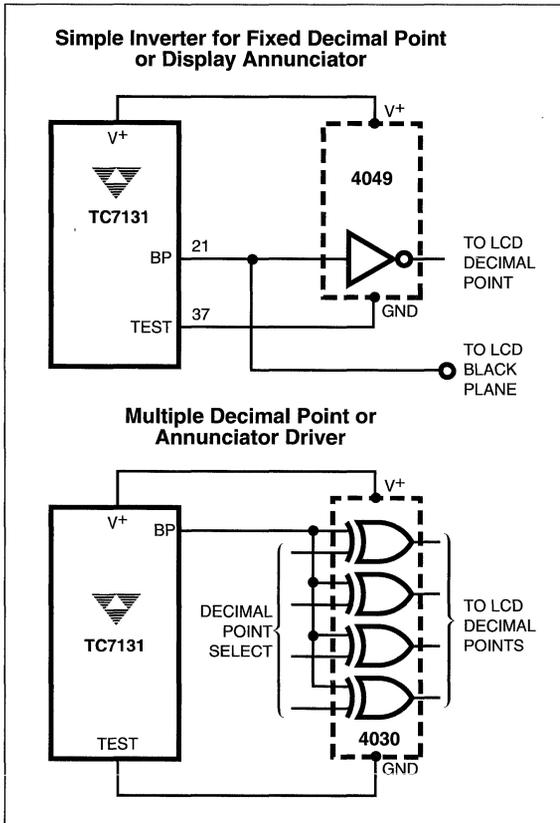
Figure 10 Decimal Point and Annunciator Drives
