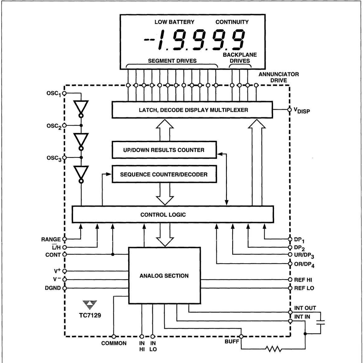
Figure 12 Functional Diagram
