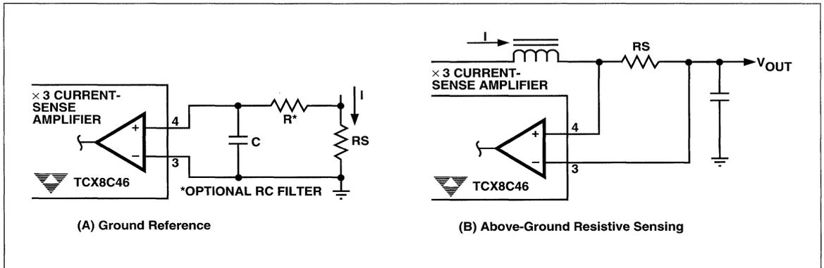
Figure 2 Resistive Sensing
