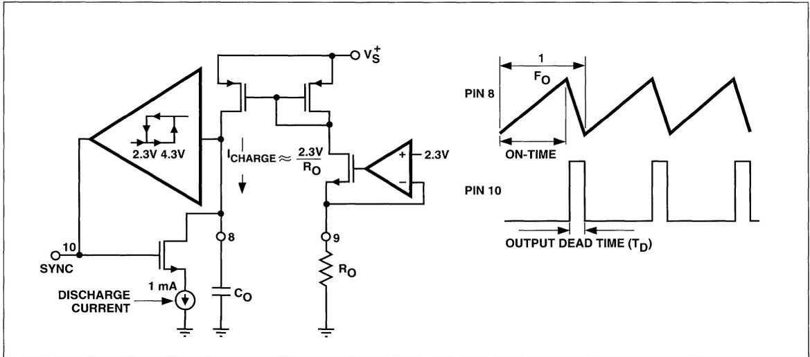
Figure 6 Oscillator Circuit
