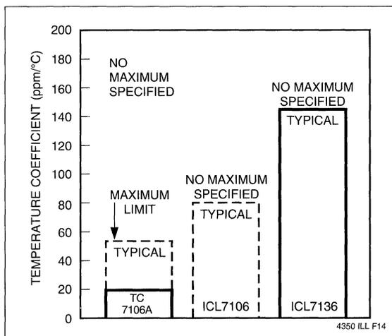
Figure 10 Analog Common Temperature Coefficient
