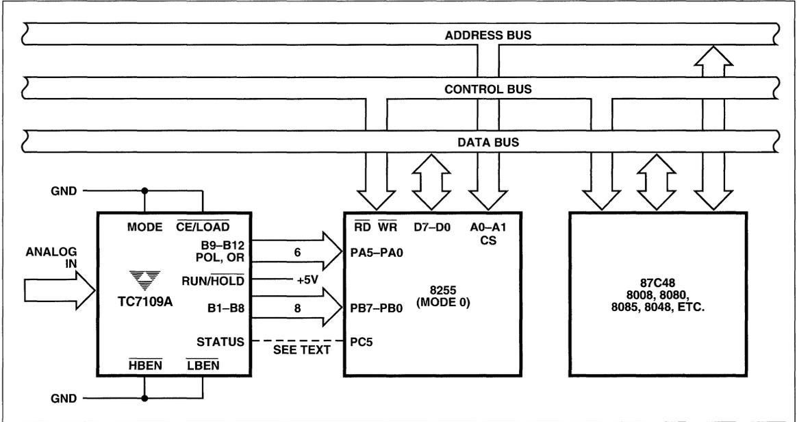
Figure 14 Full-Time Parallel Interface to MCS-48, -80, -85 Microcomputers
