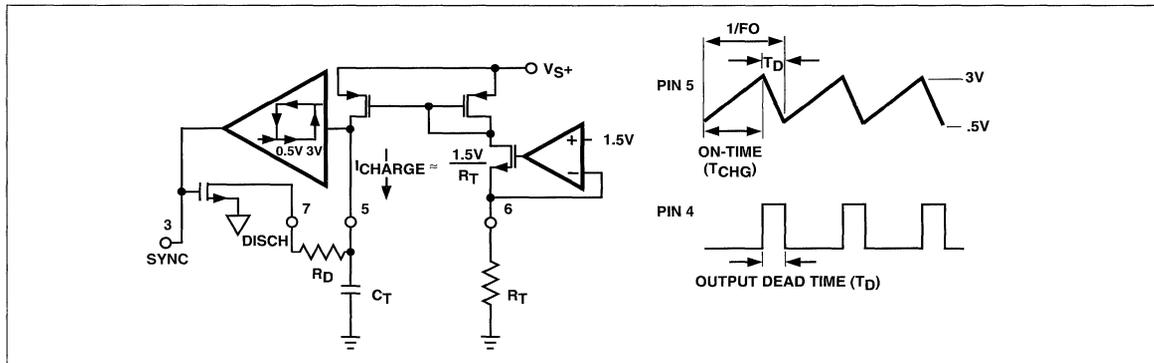
$$\text{The oscillator frequency } (F_0) = \frac{1}{T_{\text{CHG}} + T_D}$$
