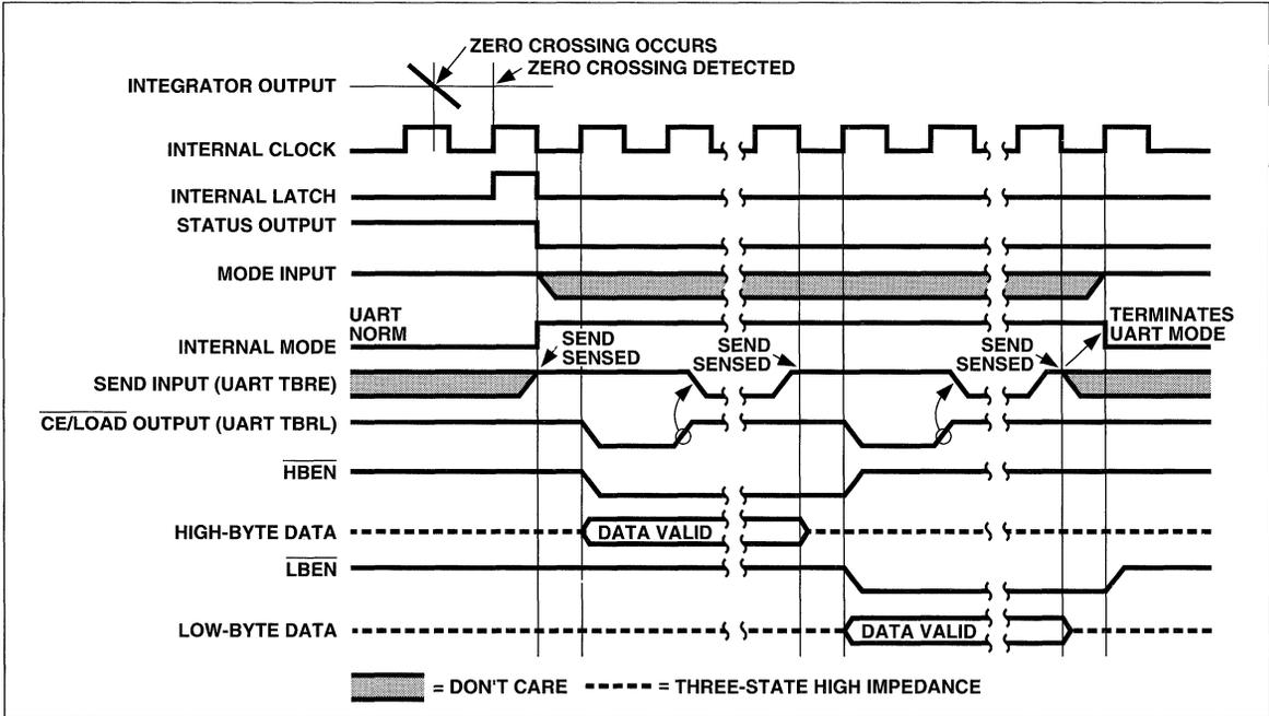
Figure 8 TC7109A Handshake — Typical UART Interface Timing
