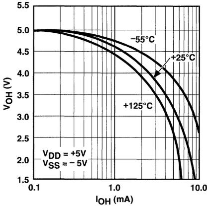
**Output Source Current vs Supply Voltage**
