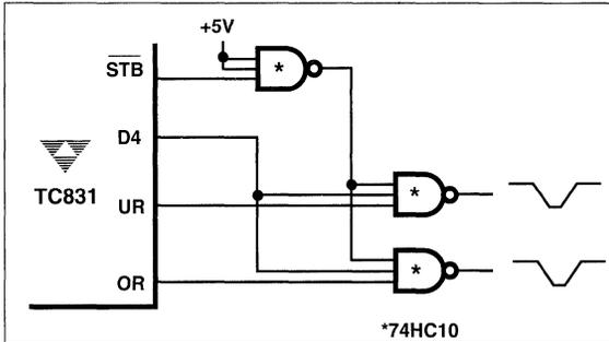
Figure 10. Generating Underrange and Overage Pulses
