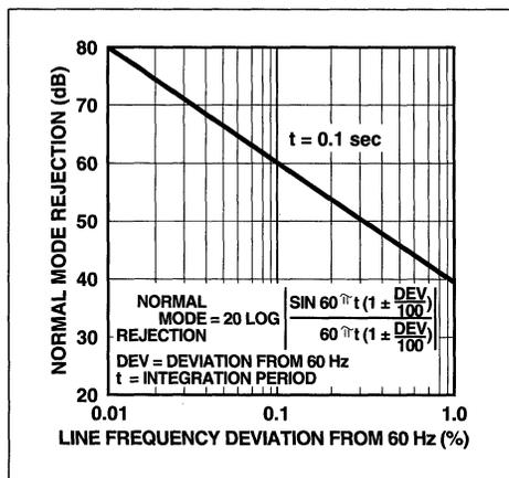
Figure 3. Normal Mode Rejection vs Input Frequency
