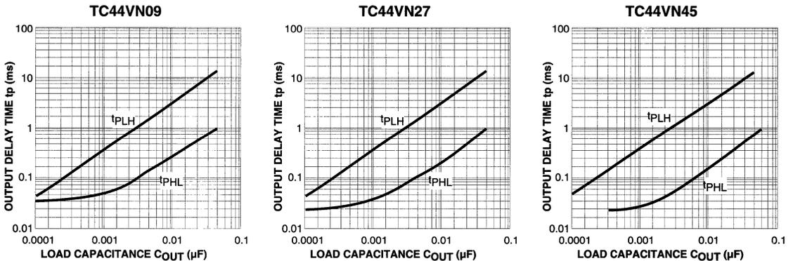
6) Output Delay vs. Input Capacitance (External)
