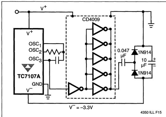
Figure 12 Generating Negative Supply From +5 V
