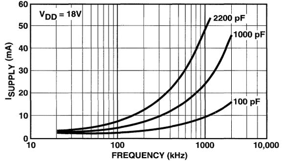
Supply Current vs Capacitive Load
