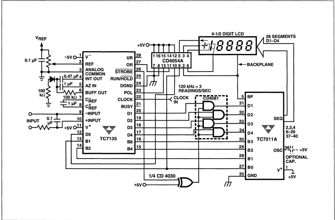
Figure 4: 4-1/2 Digit ADC Interfaced to LCD
