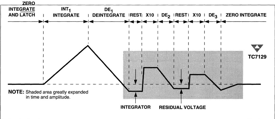
Figure 11 Integrator Waveform
