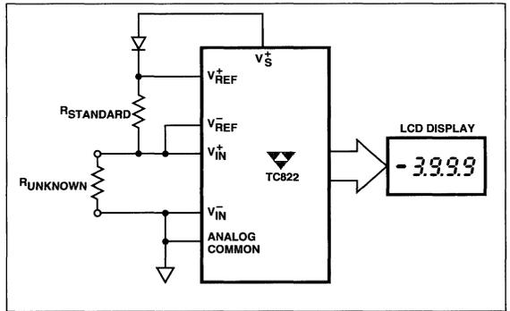
Figure 10 Low Parts Count Ratiometric Resistance Measurement
