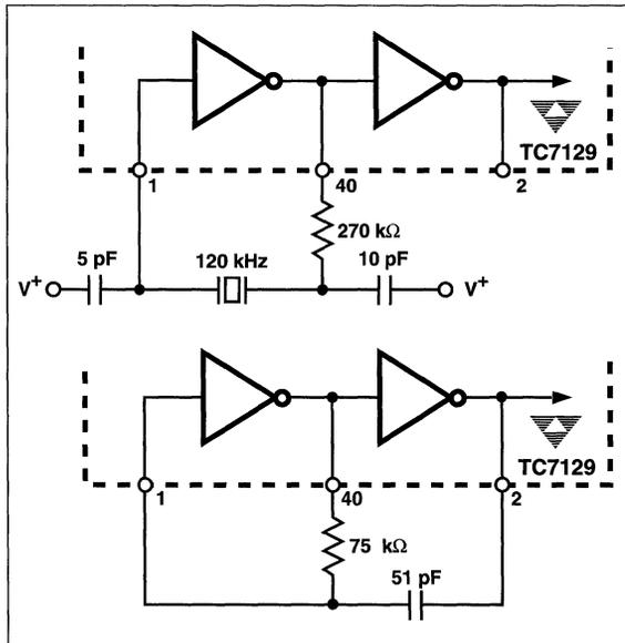
Figure 8 Oscillator Circuits
