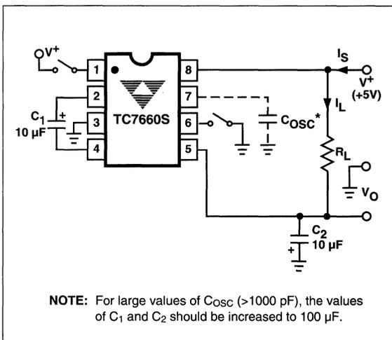
Figure 1. TC7660S Test Circuit
