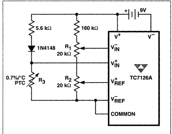
Figure 13 Positive Temperature Coefficient Resistor Temperature Sensor
