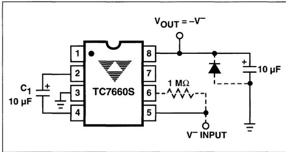
Figure 10. Positive Voltage Multiplier
