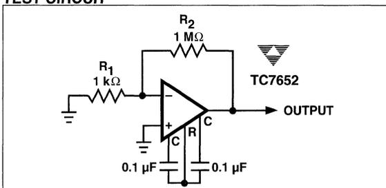
If the TC7652's output saturates, error voltages on the external capacitors will slow overload recovery. This condition can be avoided if a strobe signal is available. The strobe signal is applied to EXT CLK IN and the overload signal is applied to the amplifier while the strobe is LOW. In this case, neither capacitor will be charged. The low leakage of the capacitor pins allow long measurements to be made with negligible errors (typical capacitor drift is 10  $\mu$ V/sec).
