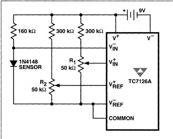
Figure 12 Temperature Sensor
