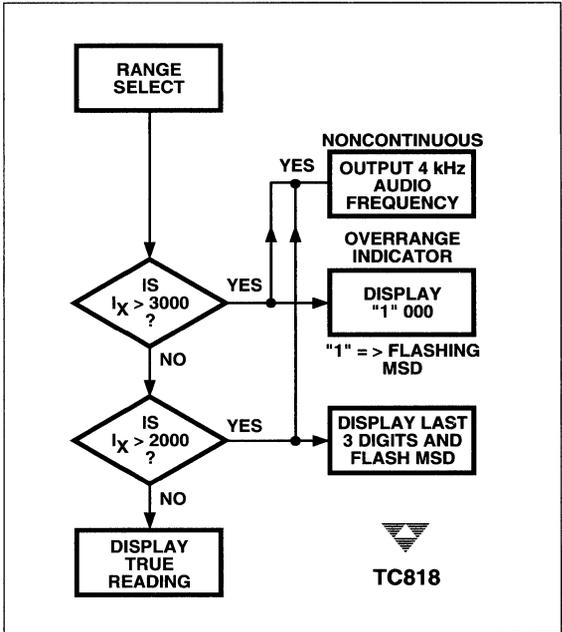
Figure 7 Manual Range Selection; Current Measurement
