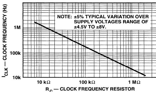
Figure 5. Typical Clock Frequency vs Resistor ( $R_C$ )
