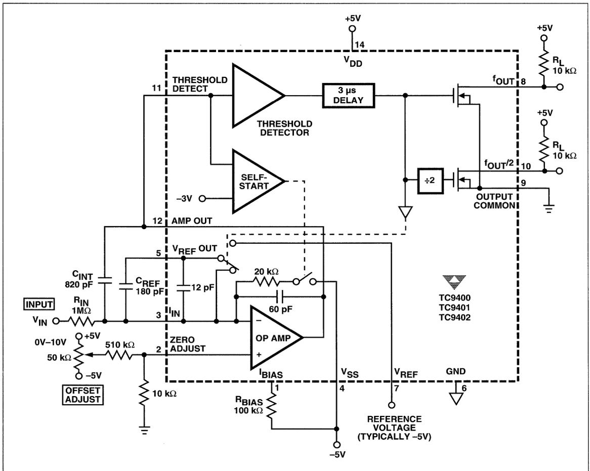
Figure 1 10 Hz to 10 kHz V/F Converter
