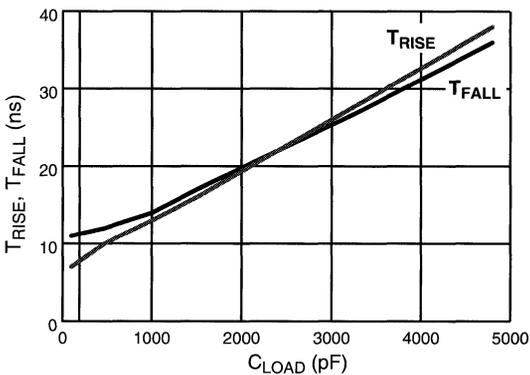
**Propagation Delays vs. Capacitive Load**
