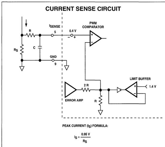
Shutdown can be accomplished by either pulling  $I_{SENSE}$  above 1 volt or pulling COMP, pin 1 to GND. This will set the PWM latch so that the output will remain low until the next clock pulse after the shutdown condition is removed.
