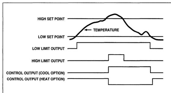
TC620/621 Input vs. Output Logic
