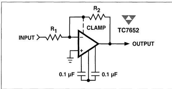
Figure 2 Inverting Amplifier With Optional Clamp
