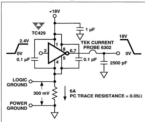
Figure 2 Switching Time Degradation Due to Negative Feedback
