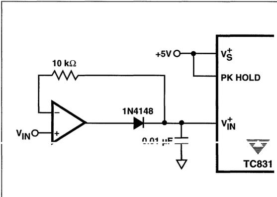
Figure 17. External Peak Detector
