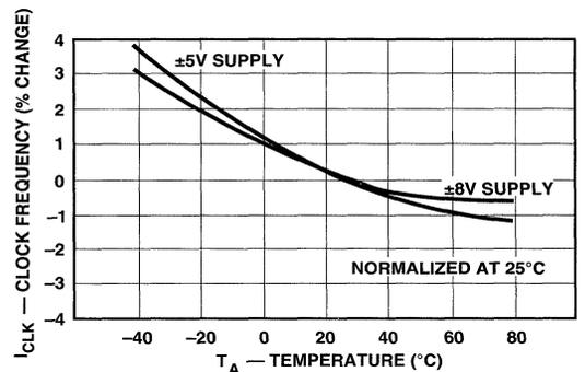
Figure 6. Typical % Change of Clock Frequency vs Temperature
