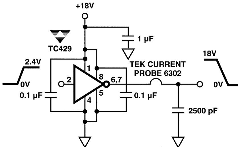
Figure 3 Peak Output Current Test Circuit
