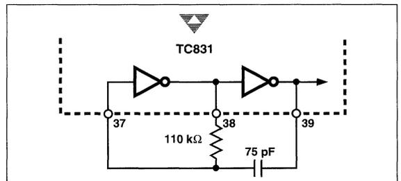
Figure 12. R-C Oscillator Circuit
