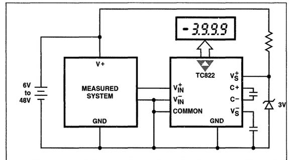
**Figure 4 DC-to-DC Converter Permits Ground Referenced Measurements**
