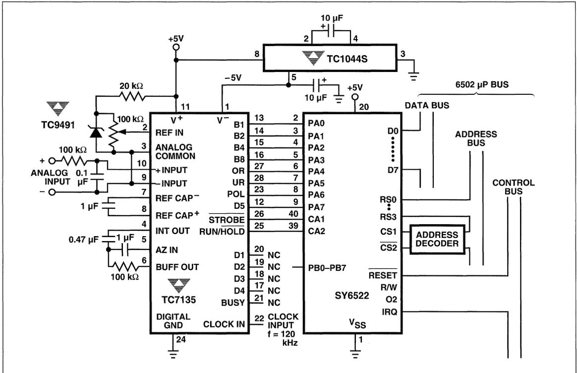
Figure 13. TC1044S Supplies -5V for Converters in Microprocessor-Controlled Data Acquisition Systems
