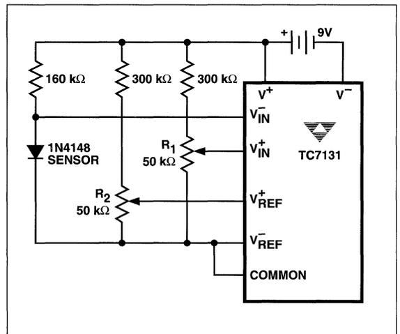
Figure 12 Temperature Sensor
