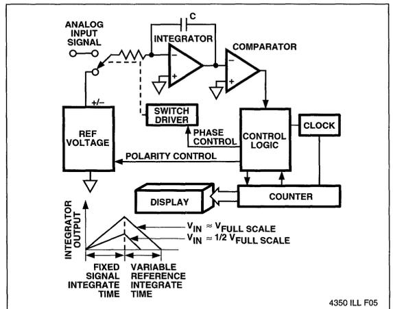
Figure 2A Basic Dual Slope Converter
