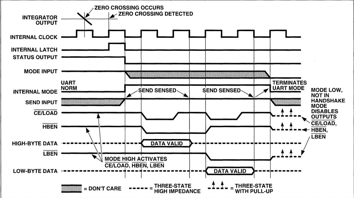
Figure 7 TC7109A Handshake With SEND INPUT Held Positive
