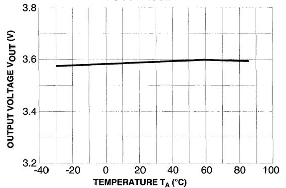
9) Detector Threshold vs. Temperature
