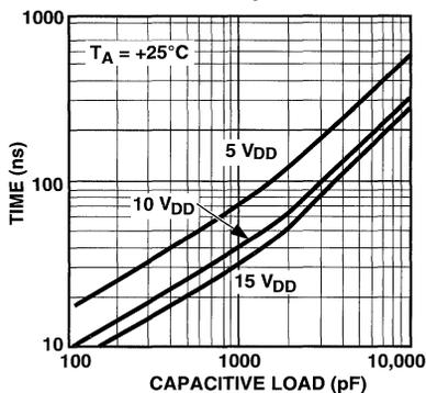
Fall Time vs Capacitive Load
