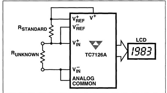
Figure 10 Low Parts Count Ratiometric Resistance Measurement
