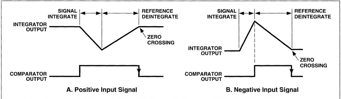
Figure 1. Comparator Output
