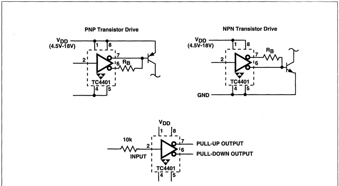
At turn-ON,  $R_B$  limits the base current in the transistor. The output that does the turn-OFF does not require a limiting resistor.
