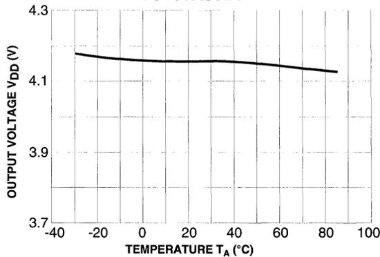
8) Output Voltage  $V_{OUT}$  vs. Temperature
