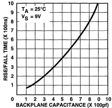
Figure 11 Backplane Driver Rise/Fall Time vs. Capacitance
