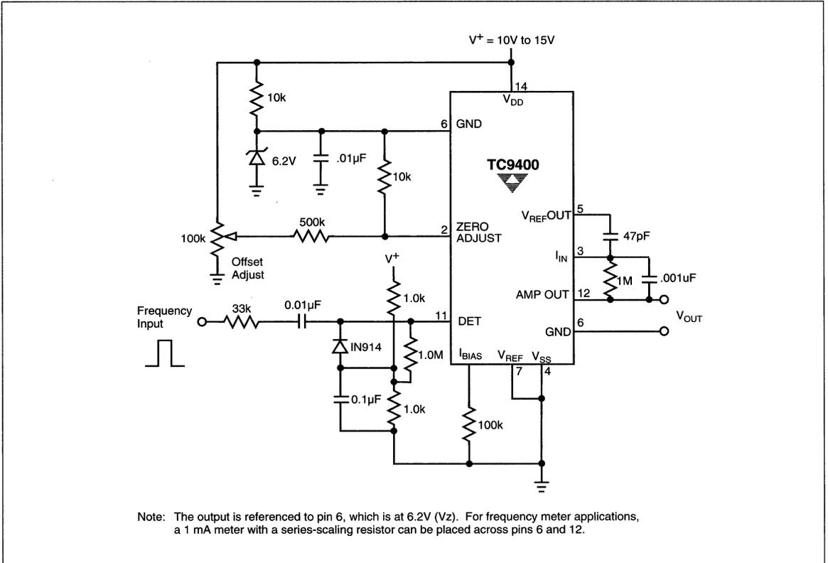
Figure 9 F/V Single Supply F/V Converter
