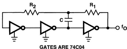
$$1. f_o \approx \frac{1}{2 C [0.41 R_P + 0.70 R_1]}, R_P = \frac{R_1 R_2}{R_1 + R_2}$$
