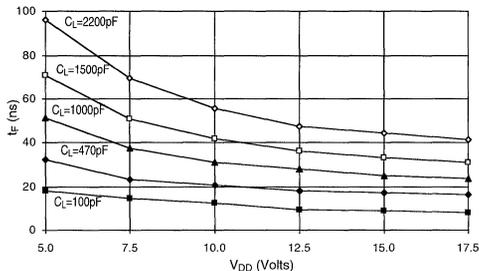
**Effect of Input Amplitude on Delay**
