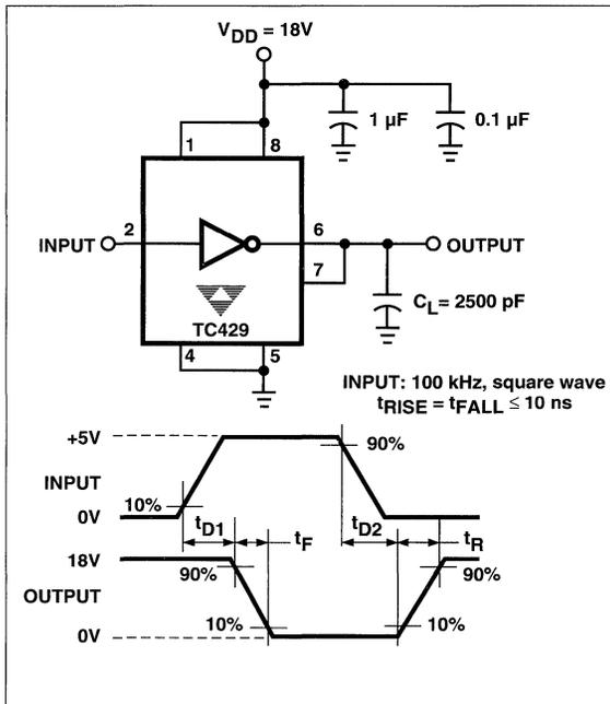
Figure 1 Inverting Driver Switching Time Test Circuit
