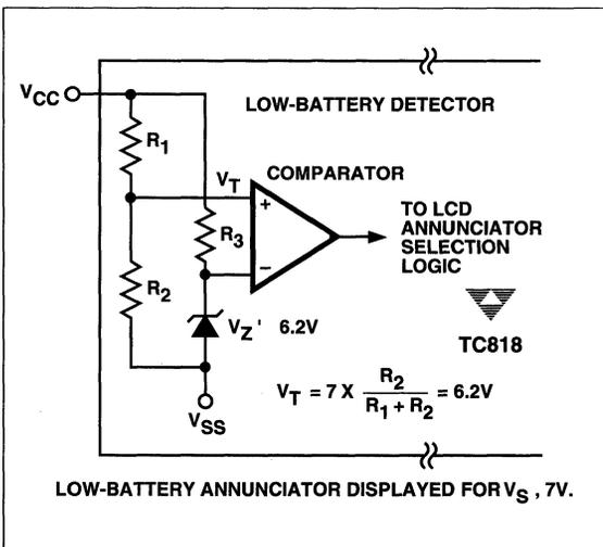
Figure 11 Low-Battery Detector
