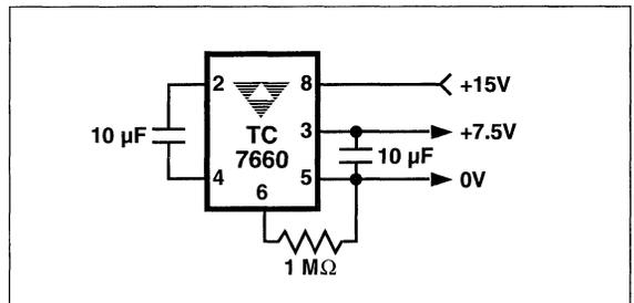
Figure 6 Splitting +15V With the 7660 at >95% Efficiency
