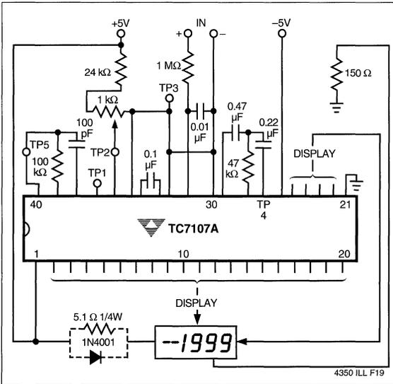
Figure 15 Diode or Resistor Limits Package Power Dissipation
