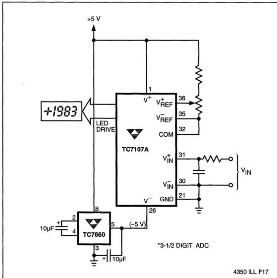
Figure 13 Negative Power Supply Generation with TC7660
