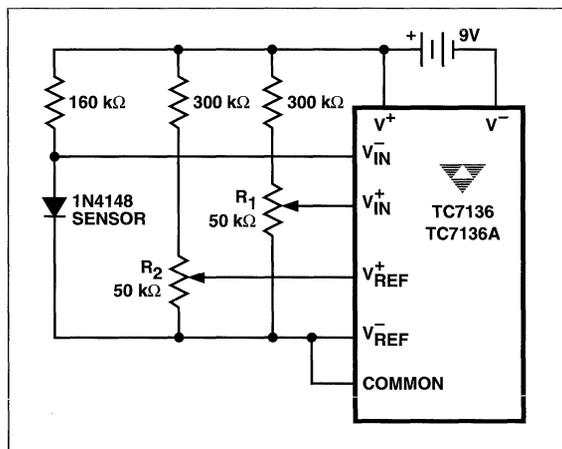
Figure 13 Temperature Sensor
