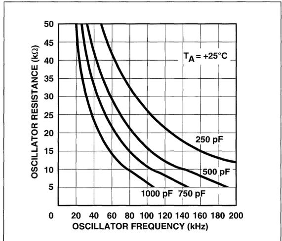
Figure 7 Oscillator Frequency vs Oscillator Resistance
