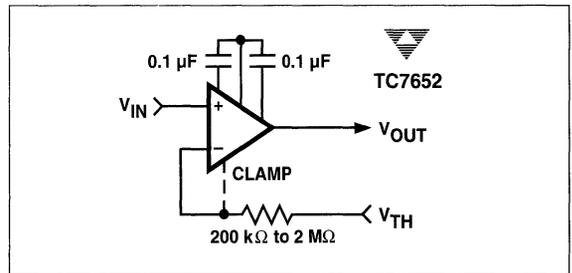
Figure 4 Low Offset Comparator
