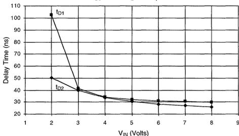
**Propagation Delay Time vs. Supply Voltage**
