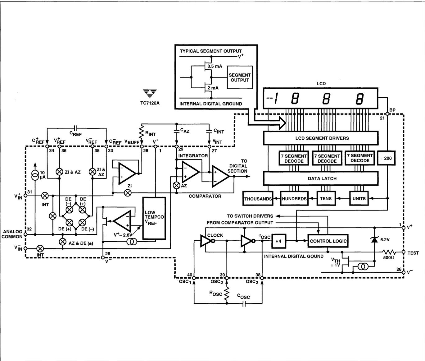
Figure 3 TC7126A Block Diagram
