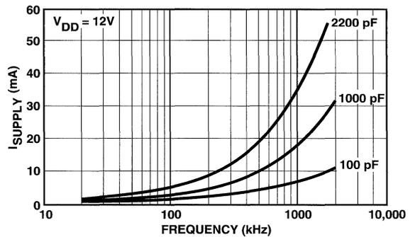
Supply Current vs Capacitive Load
