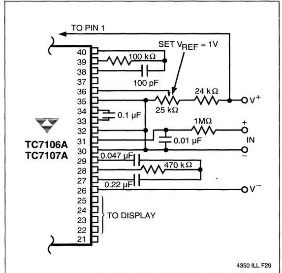
Figure 25 TC7106A/TC7107A: Recommended Component Values for 2.00 V Full-Scale
