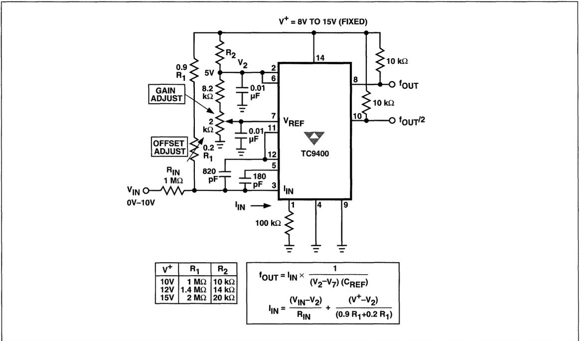
Figure 4 Fixed Voltage — Single Supply Operation
