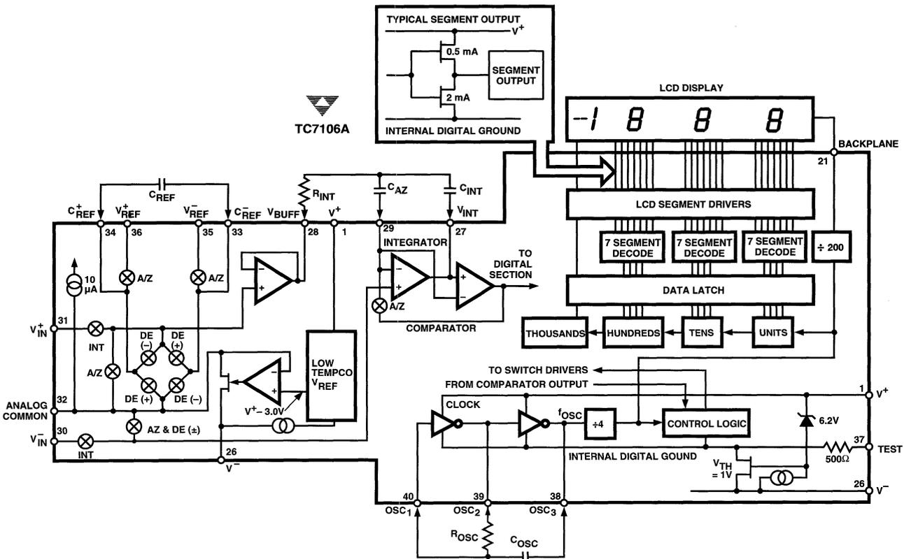
Figure 3 TC7106A Block Diagram
