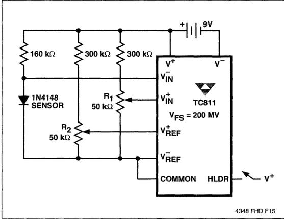
Figure 12 Temperature Sensor
