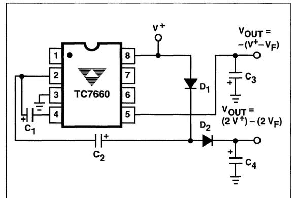
Figure 9. Combined Negative Converter and Positive Multiplier
