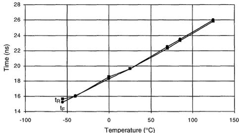
**Propagation Delay Time vs. Temperature**
