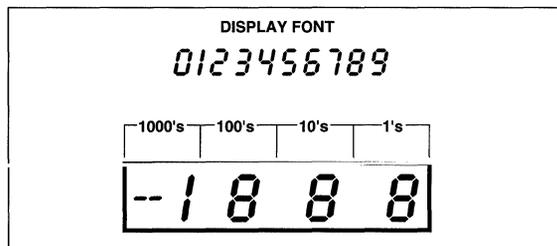
Figure 6 Display FONT and Segment Assignment
