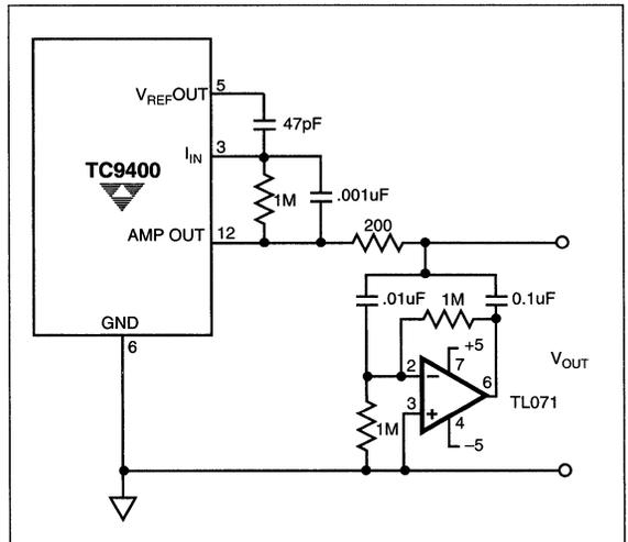
Figure 10 Ripple Filter
