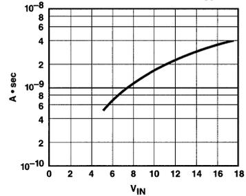
**NOTE:** The values on this graph represent the loss seen by both drivers in a package during one complete cycle. For a single driver, divide the stated values by 2. For a single transition of a single driver, divide the stated value by 4.
