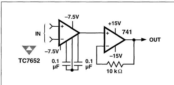
Figure 3 Using 741 to Boost Output Drive Capability
