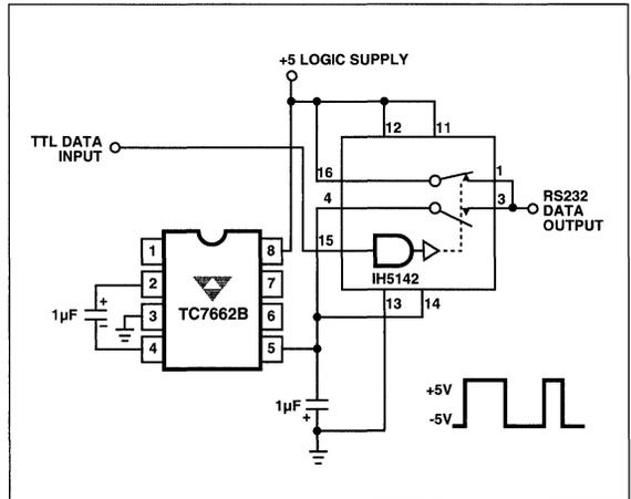
Figure 13. RS232 Levels from a Single 5V Supply
