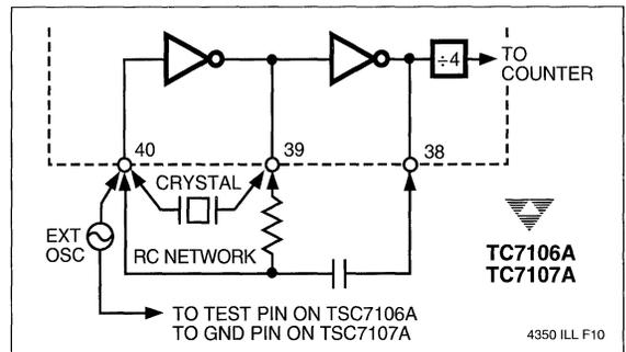
Figure 6 Clock Circuits
