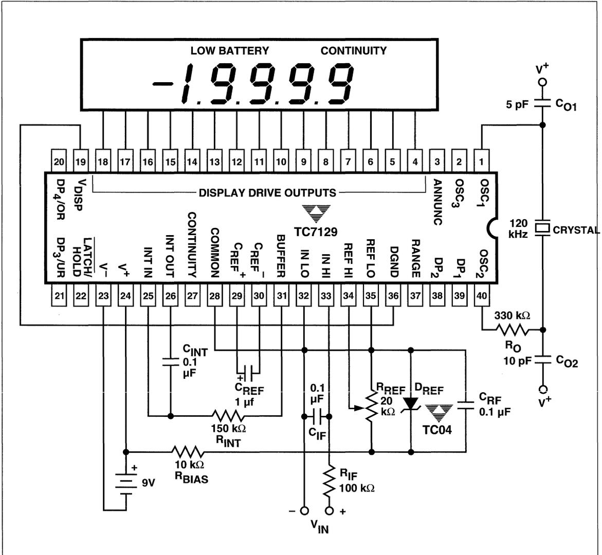
Figure 1 Standard Circuit
