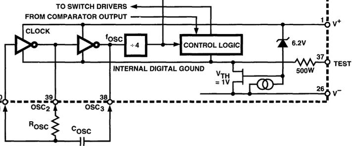
Figure 3 TC7136A Block Diagram
