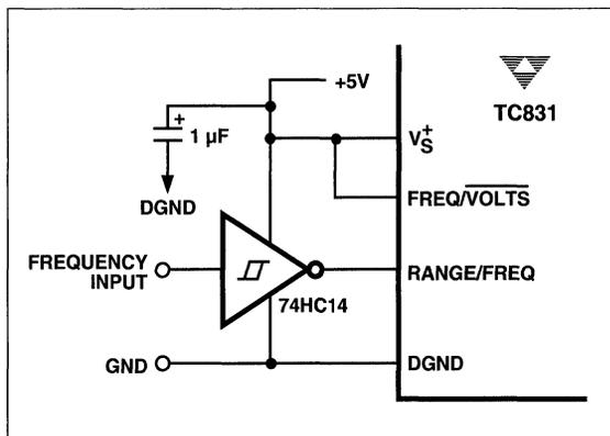
Figure 16. Frequency Counter External Buffer
