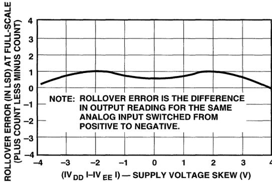
Figure 1. Typical Rollover Error vs Power Supply Skew
