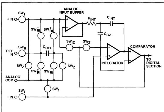
Figure 3A. Internal Analog Switches
