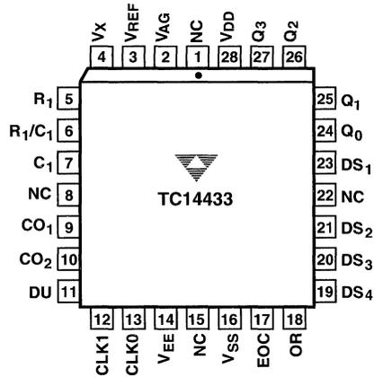
$$R_1 = \frac{V_X(\text{max})}{C_1} \cdot 3 \cdot \frac{T}{\Delta V}$$
