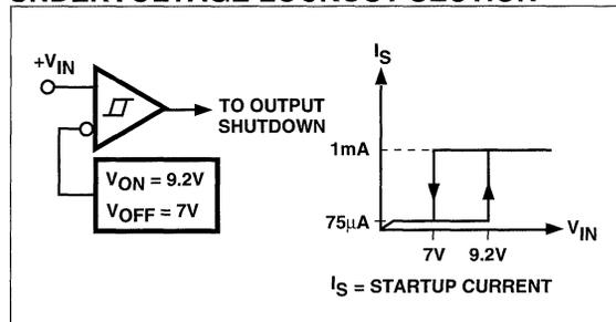
The typical turn on threshold is 9.2 V for operation of this family of PWM Controllers. When supply voltage at pin 15 drops below 7 V, after normal operation above 9.2 V, lockout occurs and both output drives to pin 11 and 14 are terminated.
