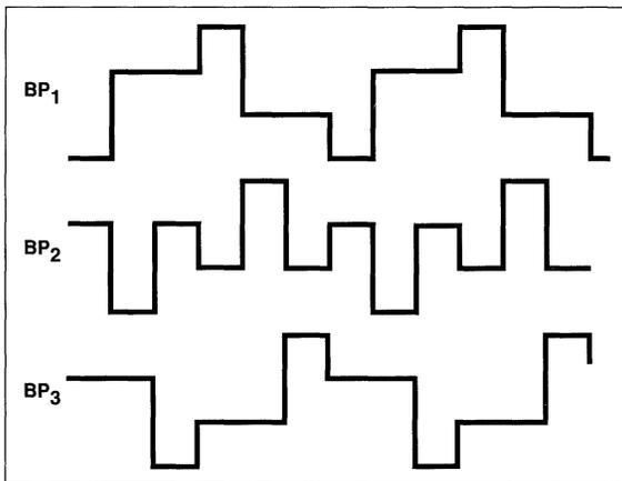
Figure 18 Backplane Waveforms
