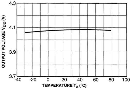
8) Output Voltage  $V_{OUT}$  vs. Temperature
