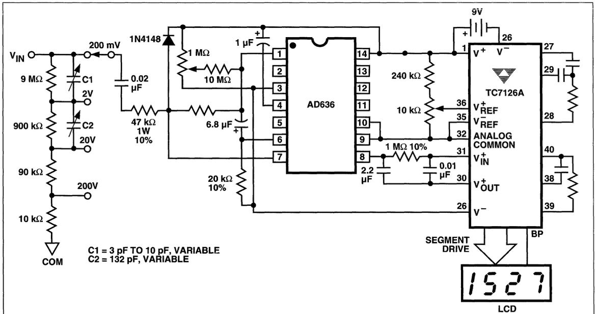
Figure 11 3-1/2 Digit True RMS AC DMM
