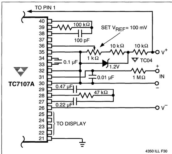
Figure 26 TC7107A With a 1.2 V External Band-Gap Reference. ( $V_{IN}$  Tied to Common.)
