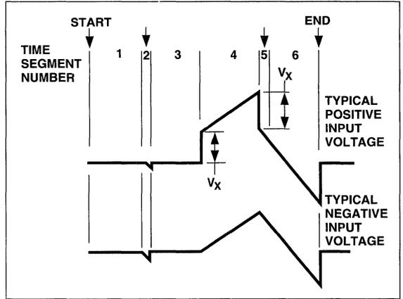
Figure 7. Integrator Waveforms at Pin 6
