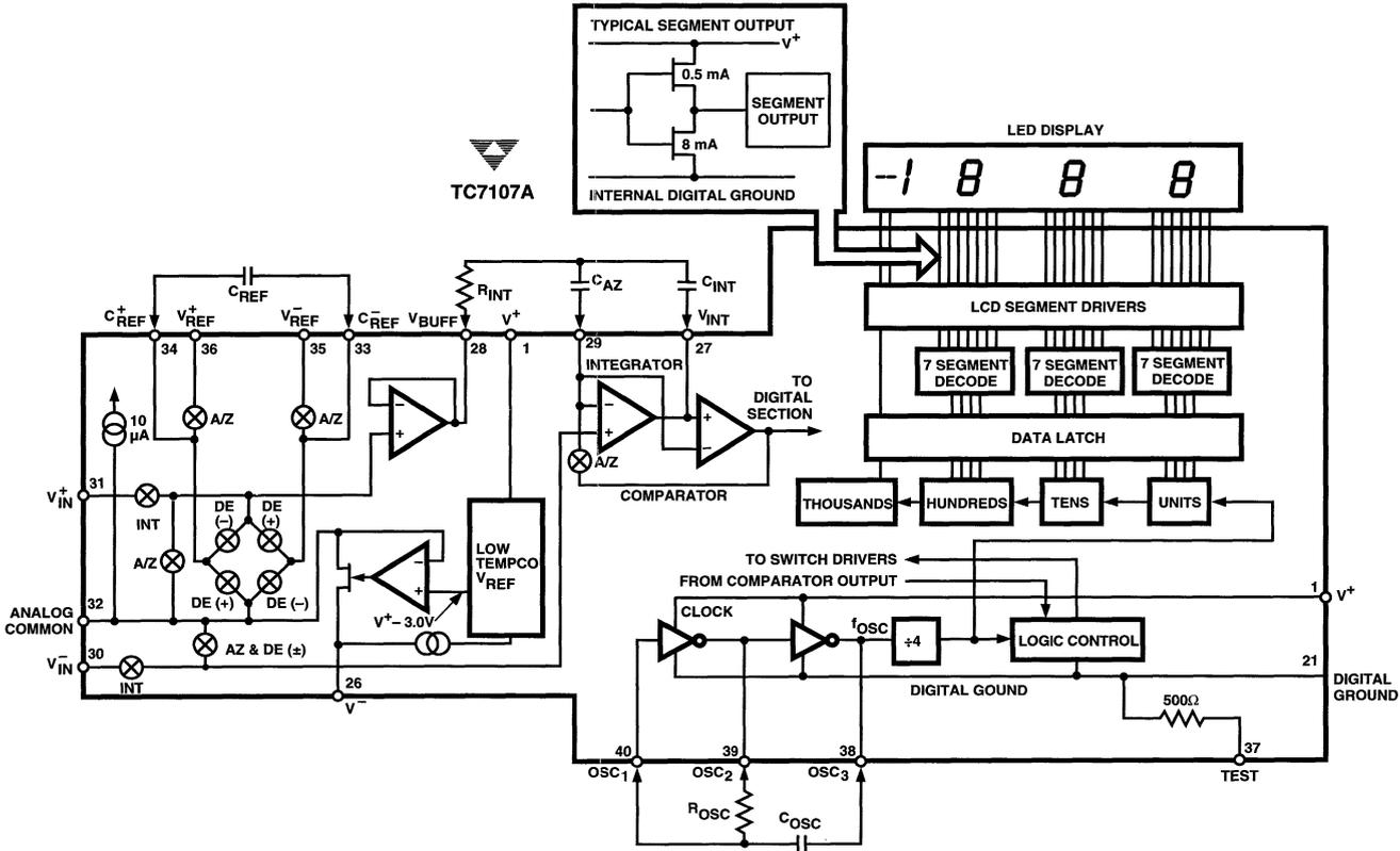
Figure 5 TC7107A Block Diagram
