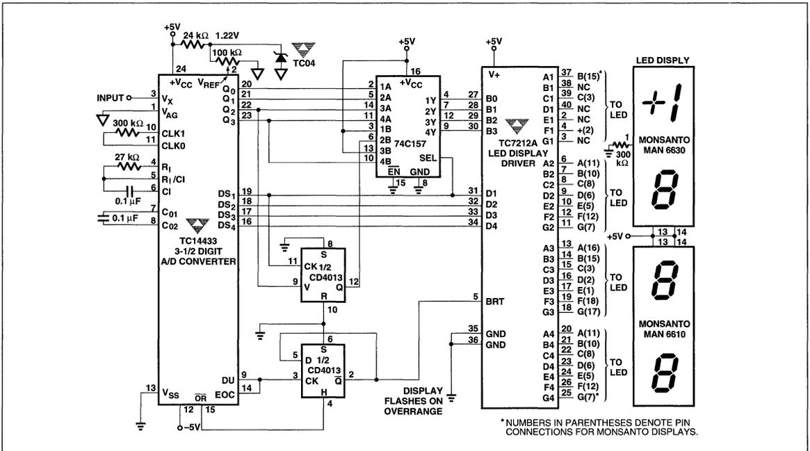
Figure 15. TC7212A Interface to TC14433 3-1/2 Digit ADC
