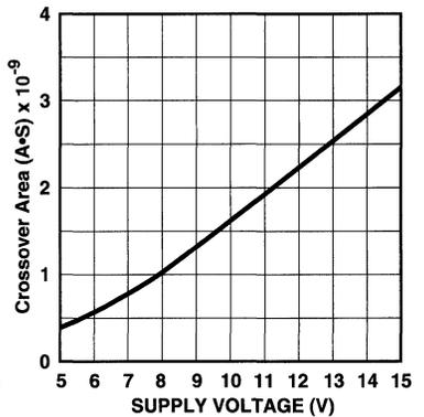
\* The values on this graph represent the loss seen by the driver during one complete cycle. For a single transition, divide the value by 2.
