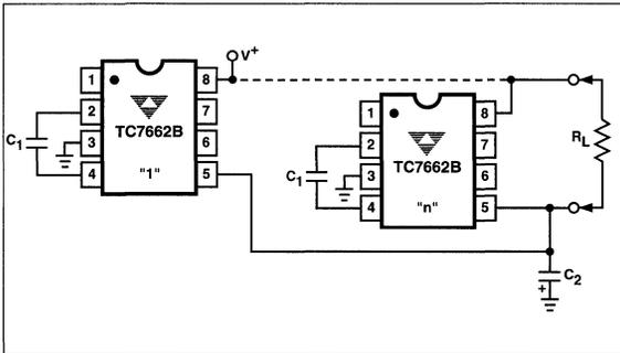
Figure 5. Paralleling Devices
