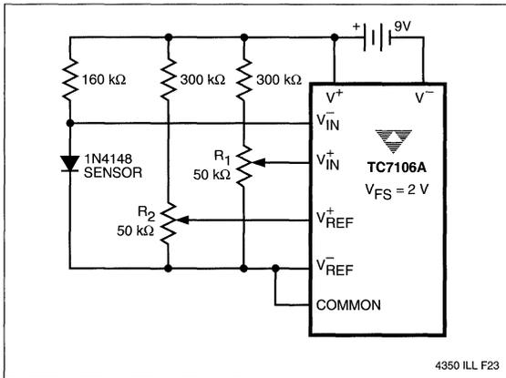
Figure 19 Temperature Sensor
