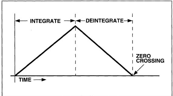
Figure 9 Dual-Slope Conversion
