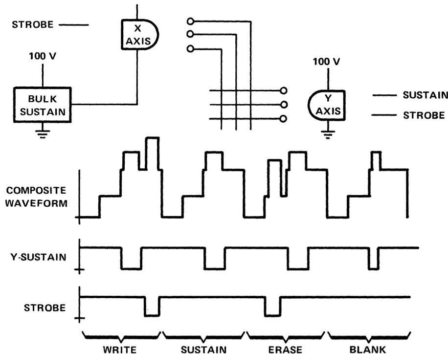
Figure 8-35. Control Signal Timing
