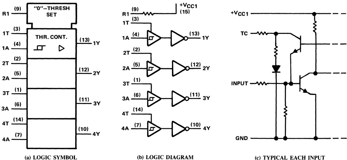
Figure 9-61. SN75154 Quad Data Line Receiver
