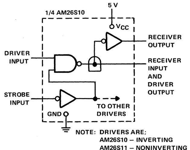
Figure 9-21. AM26S10 Functional Diagram
