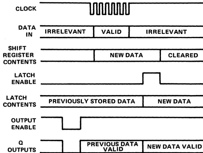
Figure 8-22. SN75581 Typical Operating Sequence
