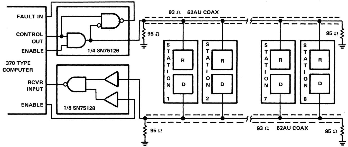
Figure 9-131. Typical IBM 370 Interface Application
