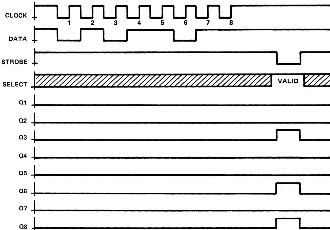
Figure 8-39. Typical Operating Sequence — SN75500A
