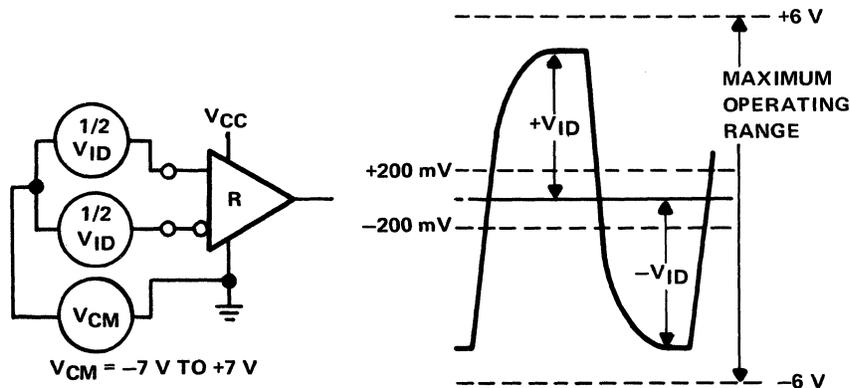
**Figure 9-74. Receiver Input Sensitivity Test**
