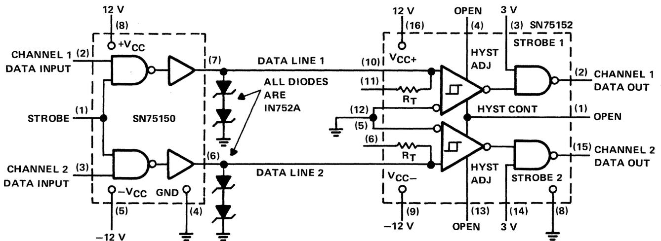
Figure 9-59. MIL-STD-188C Dual Channel Application with SN75150 and SN75152
