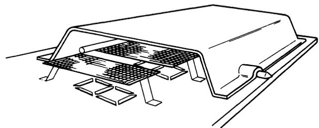
Figure 8-52. Vacuum Fluorescent Display Construction
