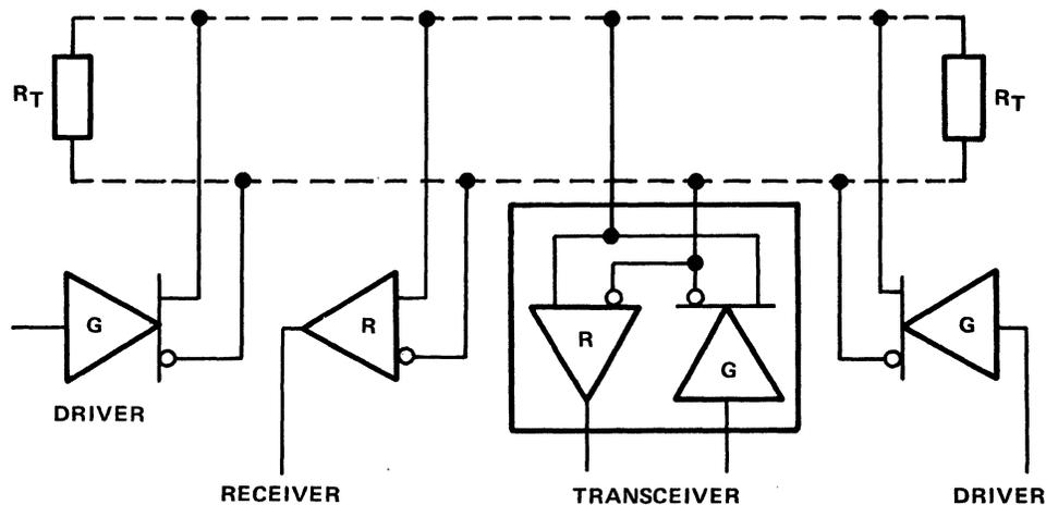
Figure 9-84. Multipoint Balanced Digital Interface
