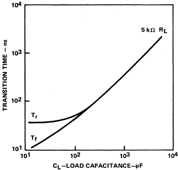
Figure 9-68. Output Transition Times Versus Total Load Capacitance
