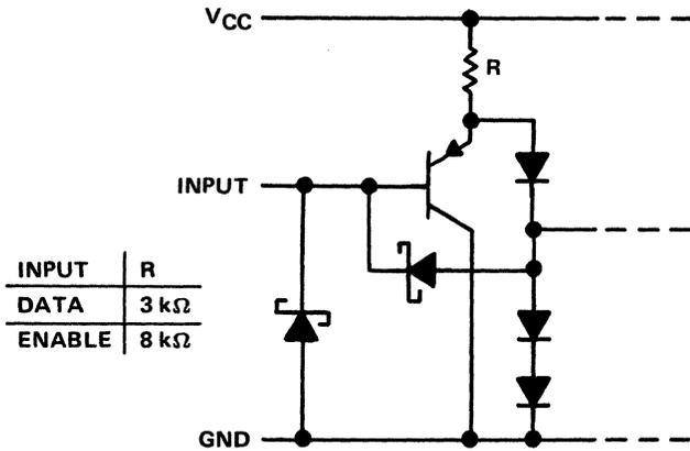
Figure 9-89. Equivalent Driver Input Circuit
