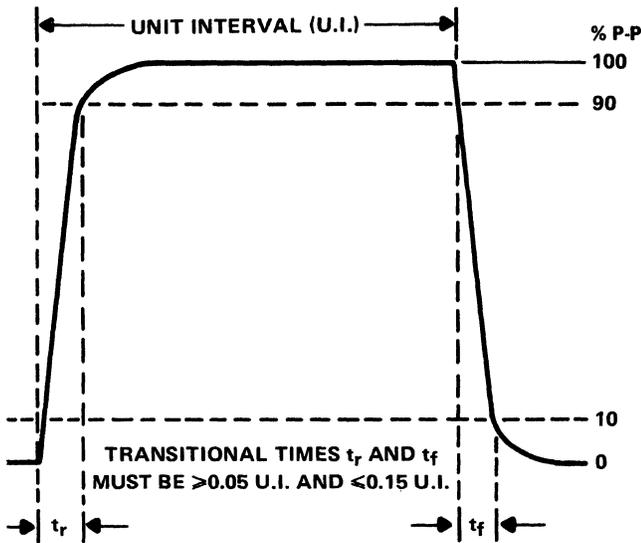
Figure 9-60. MIL-STD-188C Wave Shape Requirements
