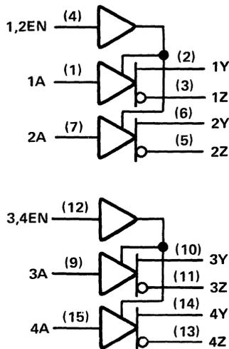
**Figure 9-87. Quad Differential Line Driver MC3487 and SN75174B**
