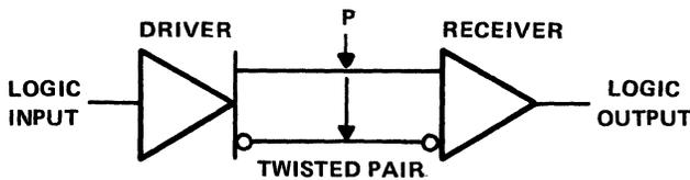
Figure 9-5. Balanced (Differential) Driven Twisted Pair
