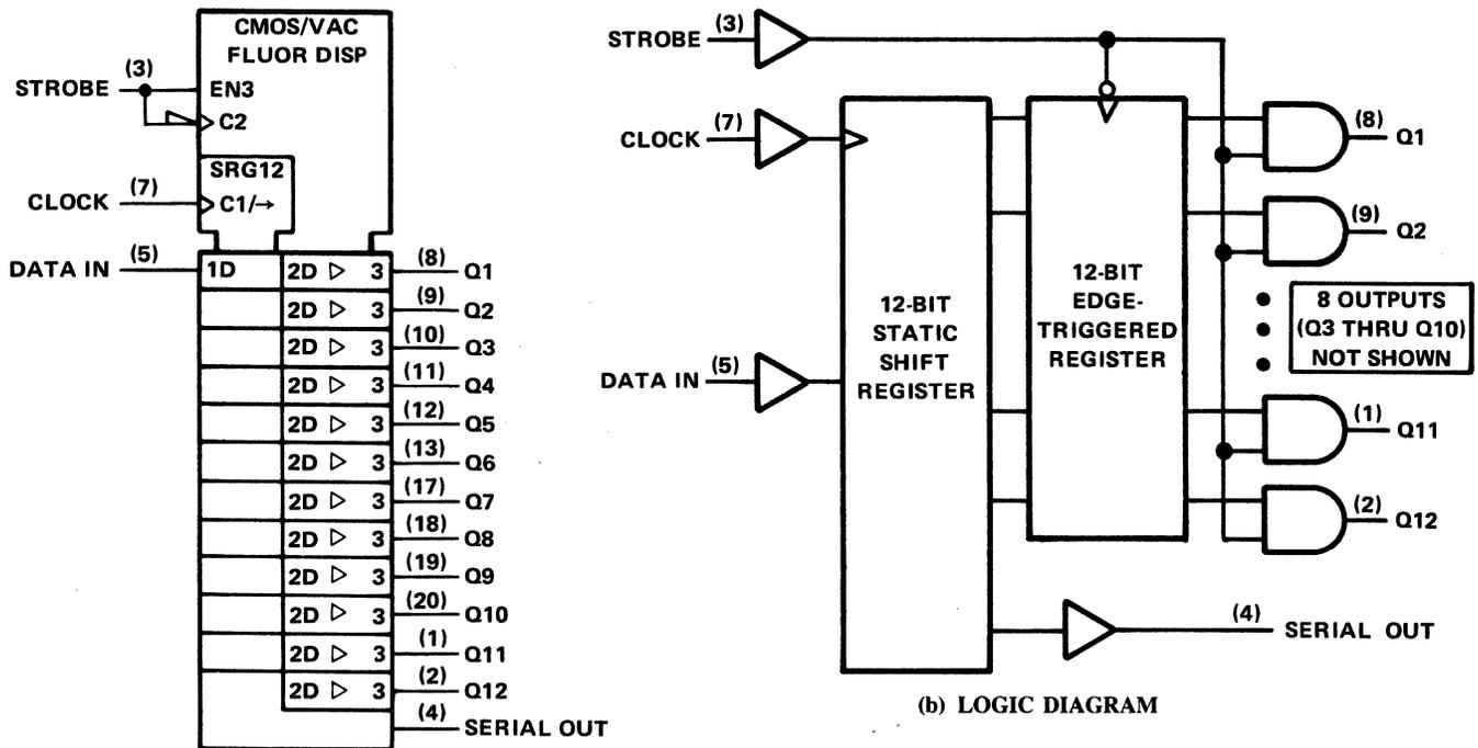
Figure 8-61. SN75514 12-Bit VFD Driver
