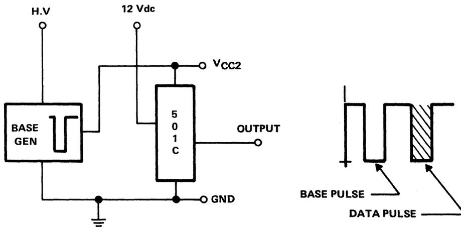
Figure 8-44. SN75501C with Pulsed  $V_{CC2}$
