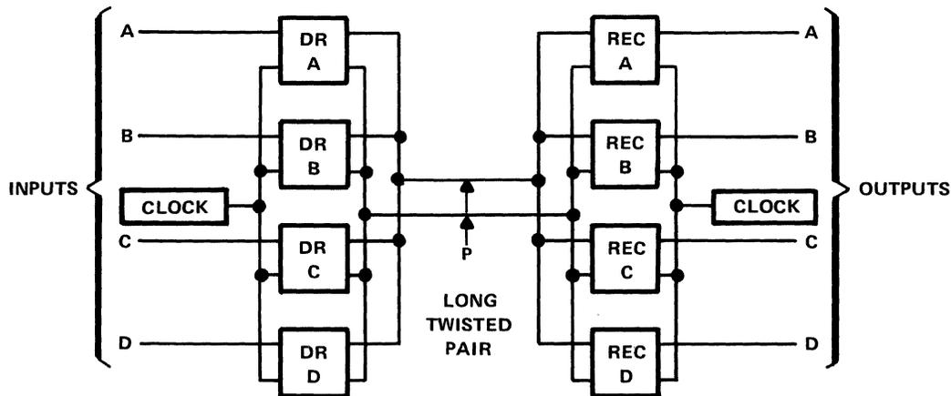
Figure 9-42. Conceptual Diagram of Four Transmission Channels Sharing the Same Party Line
