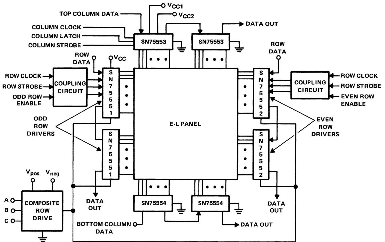
Figure 8-82. Display Block Diagram
