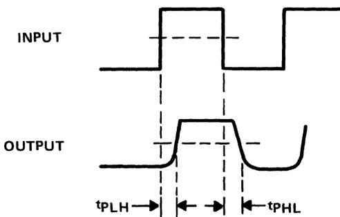
Figure 9-96. Receiver Propagation Delays
