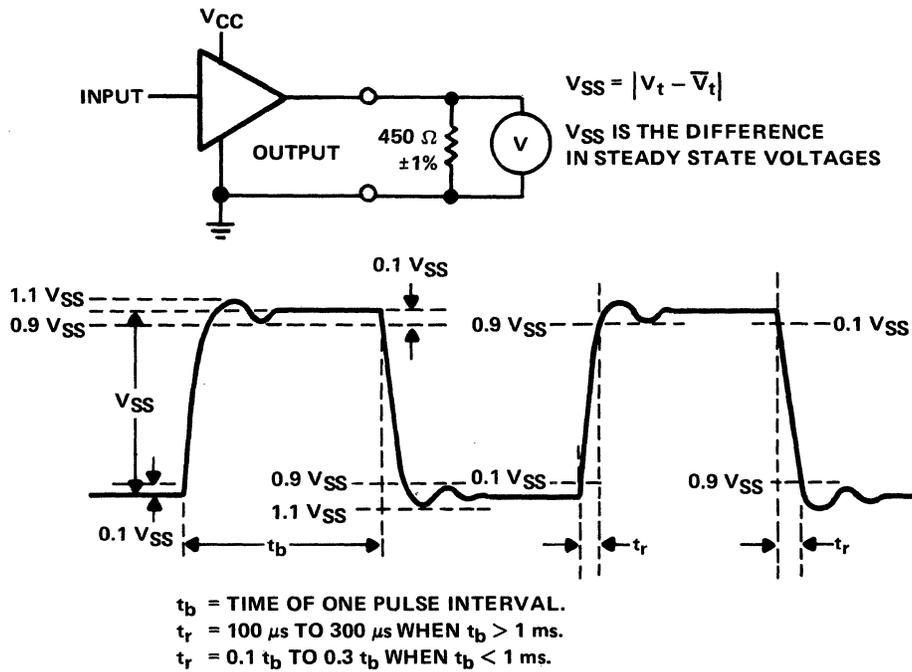
Figure 9-72. Signal Wave Shaping Requirement
