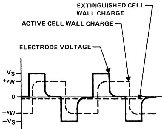
Figure 8-29. Cell Waveforms
