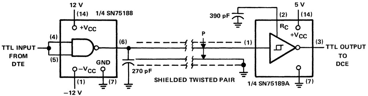
Figure 9-69. Typical EIA RS-232-C Interface Using SN75188 and SN75189A
