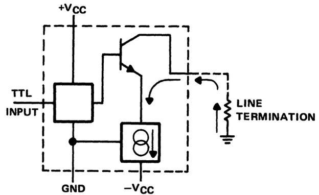
Figure 9-18. Current-Mode Configuration
