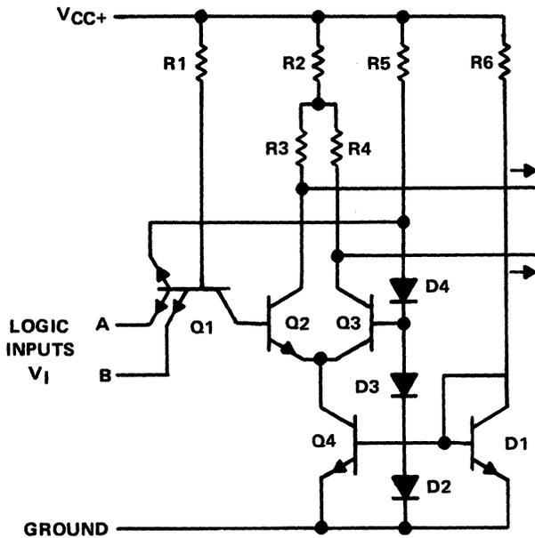
Figure 9-29. Input Circuit
