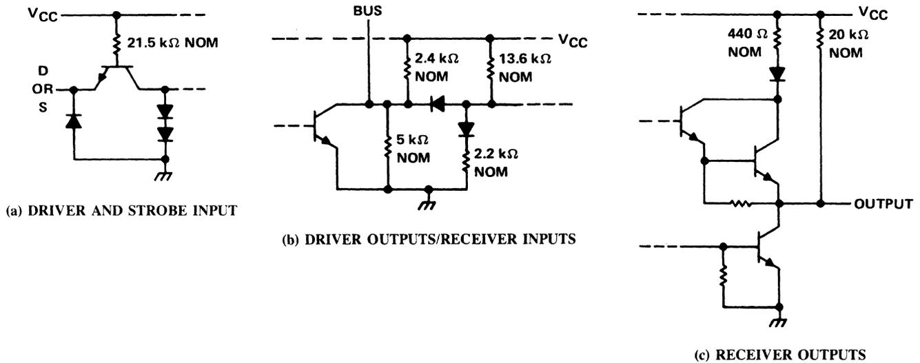
**Figure 9-117. MC3446 Input and Output Equivalent Circuits**
