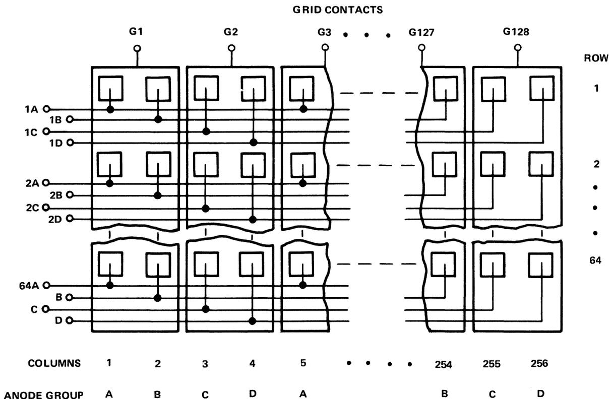
**Figure 8-68. A 256 × 64 Dot Matrix VFD Pinout**
