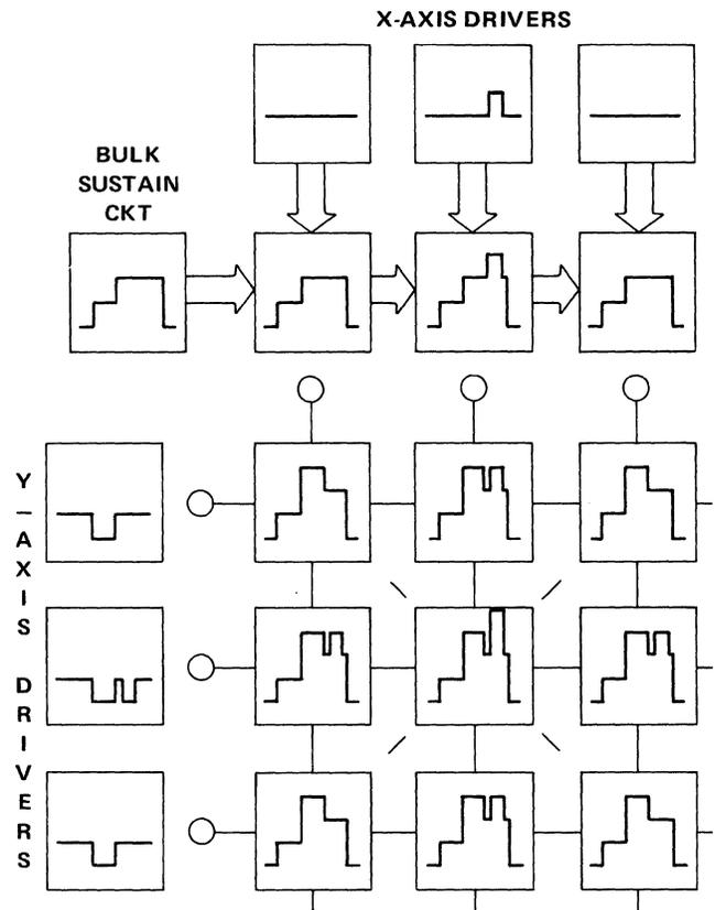
Figure 8-34. Write Waveform Array and Origin
