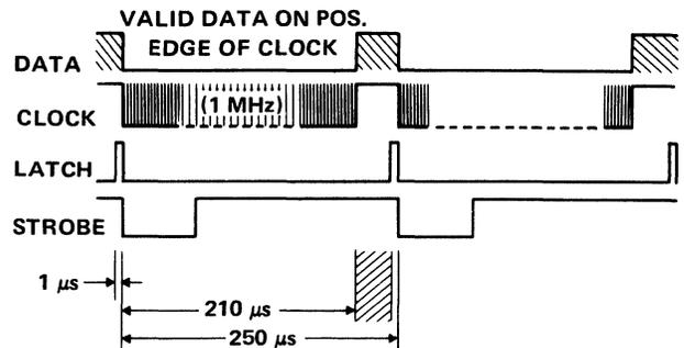
**Figure 8-67. Data Registration of an SN75512 12-Bit VFD with Latch**
