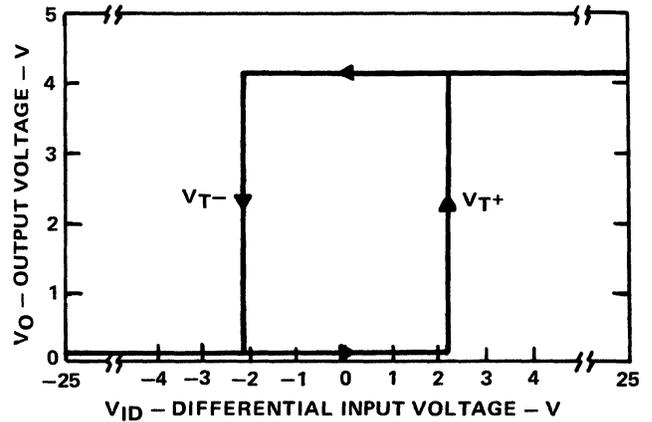
(b)  $V_{ID}$  VERSUS  $V_O$  in RS-232-C CONFIGURATION
