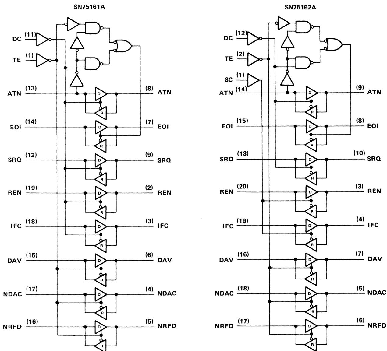
Figure 9-114. Logic Diagrams (Positive Logic) of SN75161A and SN75162A
