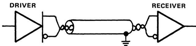
Figure 9-12. Shielded Twisted Pair Transmission
