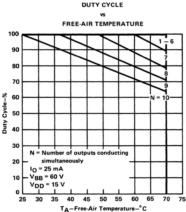
Figure 8-58. UCN4810A Operational Duty Cycle
