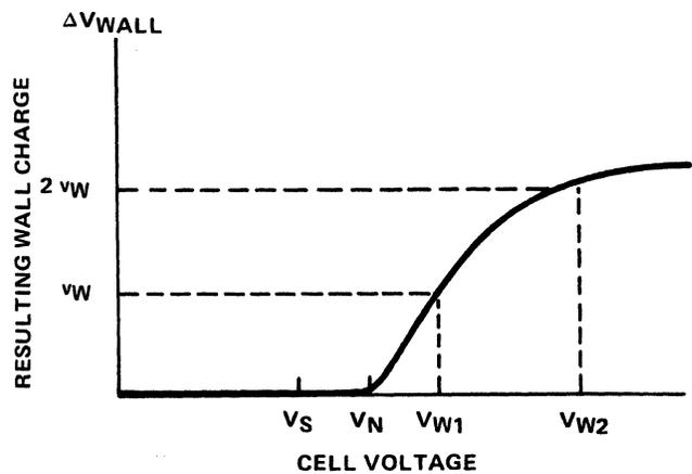
Figure 8-31. Charge Transfer Characteristics of AC Plasma Cell
