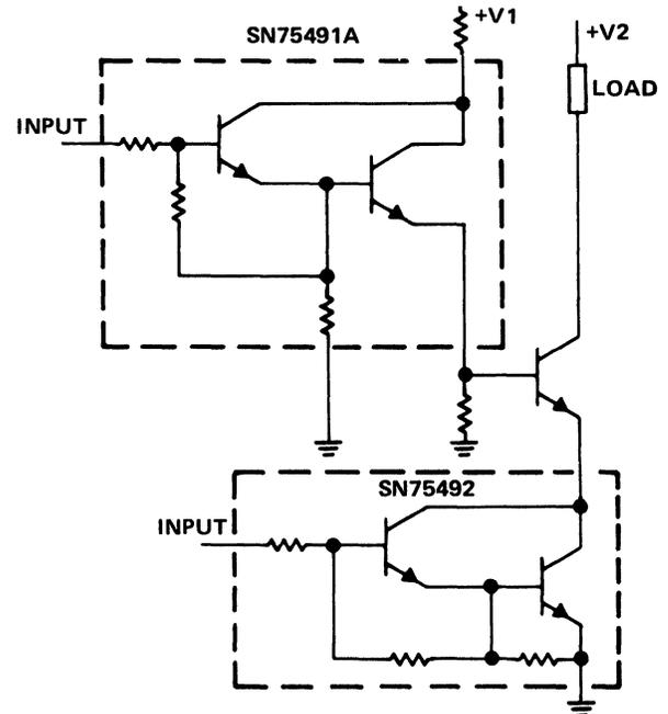
Figure 8-13. Base/Emitter Select N-P-N Transistor
