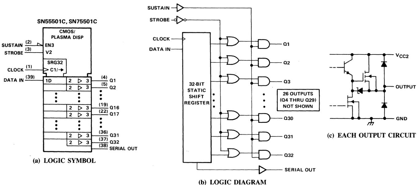
Figure 8-40. SN55501C and SN75501C
