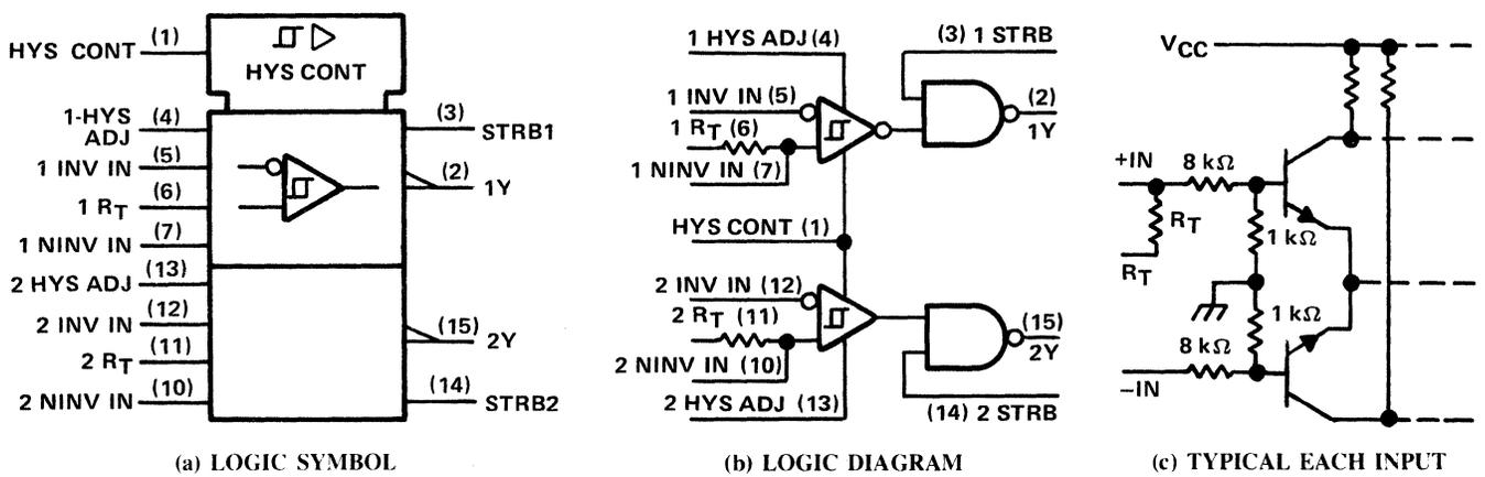
Figure 9-54. SN75152 Dual Line Receiver
