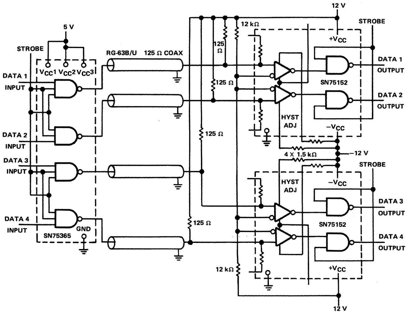
Figure 9-25. Quad Transmission System with High Noise Immunity
