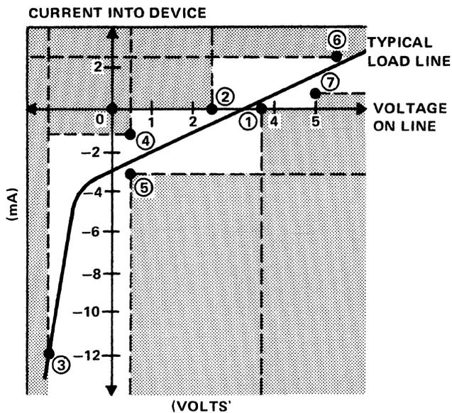
Figure 9-108. DC Load Line Permissible Operating Area
