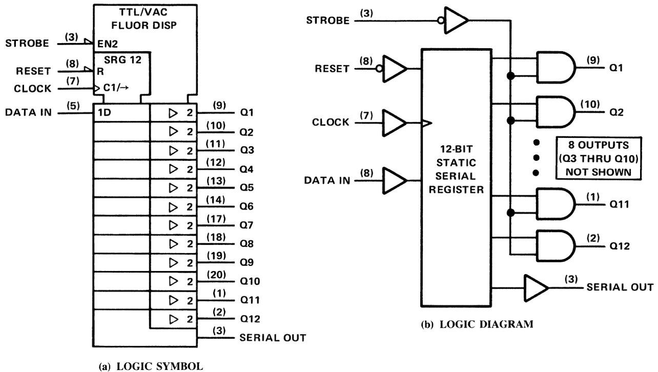
Figure 8-60. SN75513A 12-Bit VFD Driver
