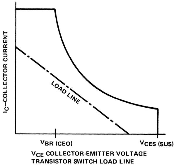
Figure 8-2. RBSOA Curve and Load Line
