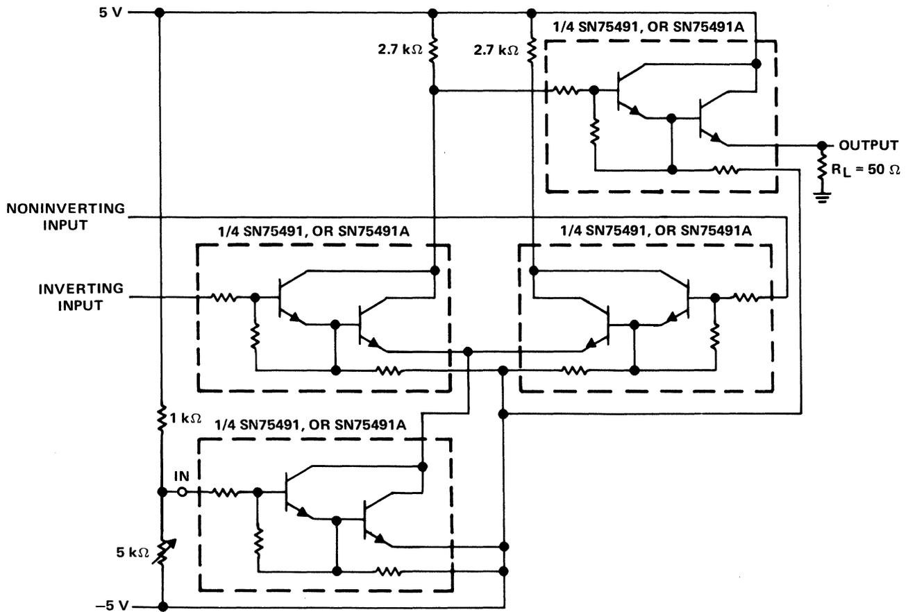
Figure 8-17. SN75491/SN75491A Used as an Interface Circuit Between the Balanced 30-MHz Output of an RF Amplifier and a Coaxial Cable
