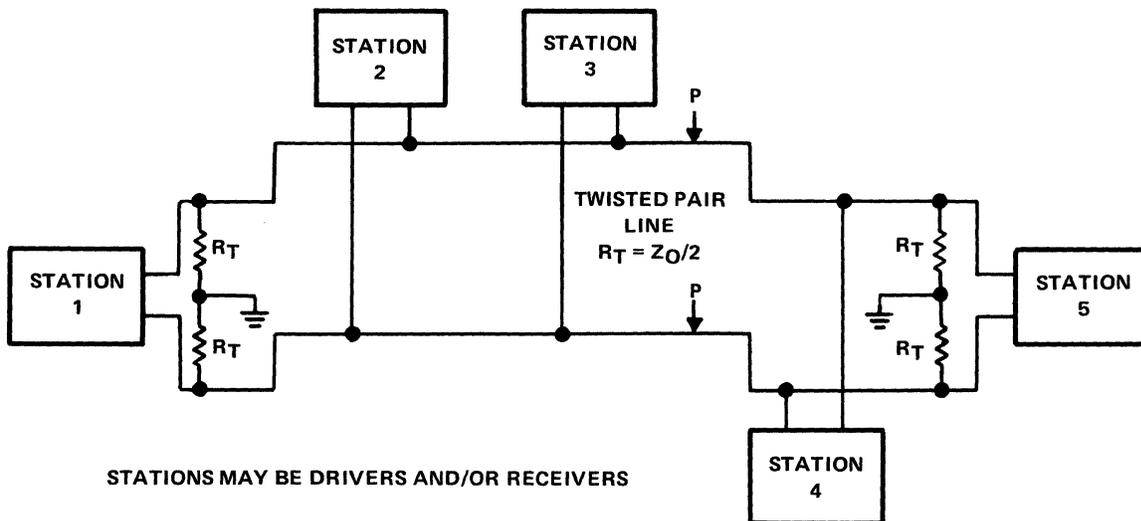
(c) MULTIPLE STATIONS; EACH LINE TERMINATED TO GROUND; TERMINATE EXTREME ENDS ONLY
