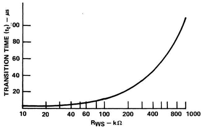
Figure 9-52. SN75156 Transition Time vs RWS
