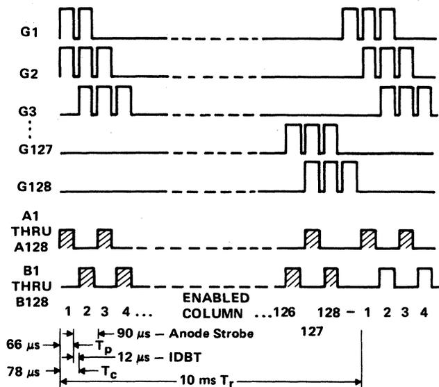
Figure 8-73. Timing Diagram for VFD of 128 x 128 Dot Matrix Pinout
