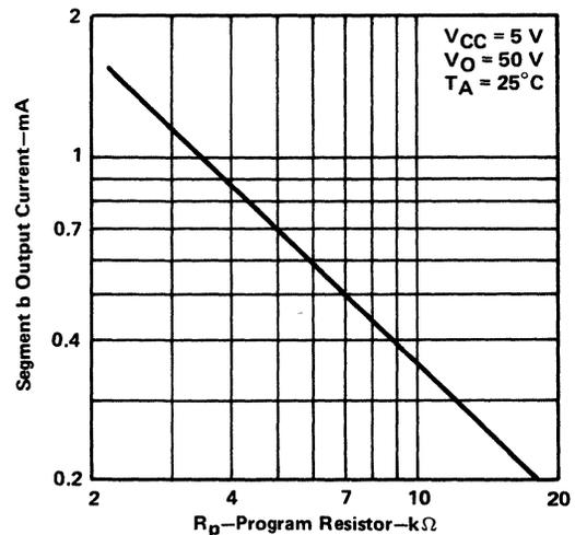
(c) SEGMENT OUTPUT CURRENT vs PROGRAMMING RESISTOR
