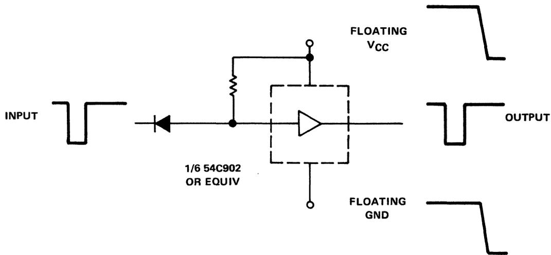
Figure 8-51. Negative Base Signal Data Buffer Circuit
