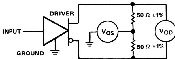
$V_{OD}$  = DIFFERENTIAL OUTPUT VOLTAGE
