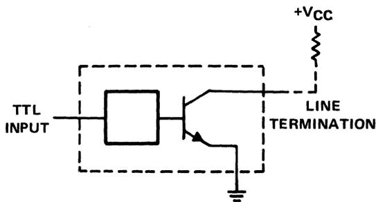
Figure 9-16. Active Pull-Down Configuration
