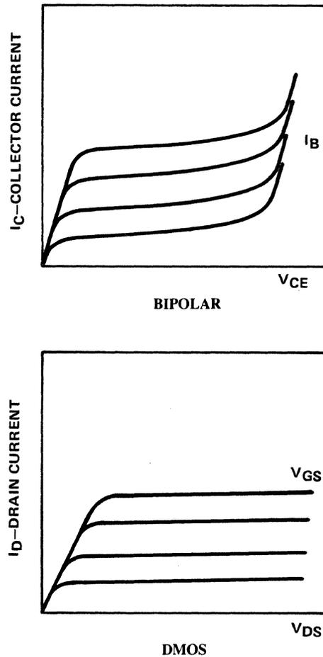
Figure 8-4. Characteristic Waveforms
