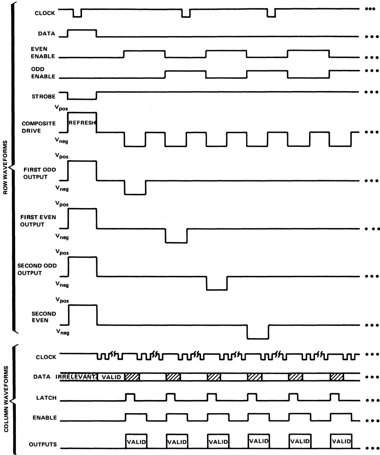
Figure 8-83. Refresh Operation Waveforms
