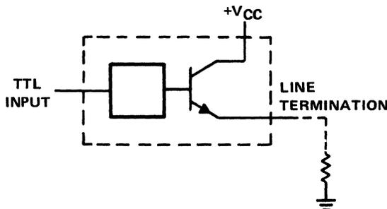
Figure 9-15. Active Pull-Up Configuration
