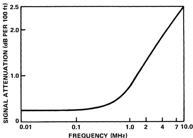
Figure 9-48. Signal Attenuation with Frequency in Twisted Pair Transmission Line (AWG 22 Solid Wire with 0.060-in Plastic Cover, Twisted 4.5 Times Per Foot)
