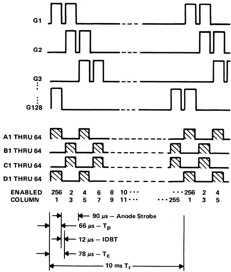
Figure 8-69. Timing Diagram for VFD of SN75512
