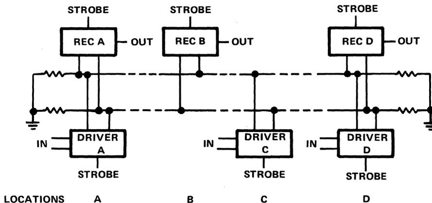
Figure 9-40. Simple Party-Line System with Driving and Receiving Stations Scattered Along the Receiving Stations Scattered Along the Line
