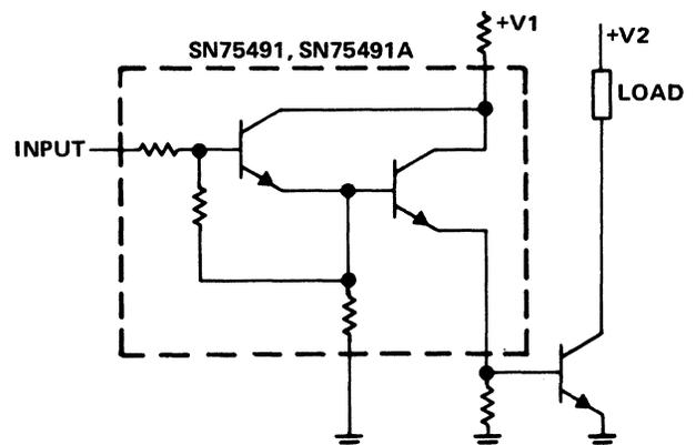
Figure 8-15. Quad High-Current N-P-N Transistor Driver
