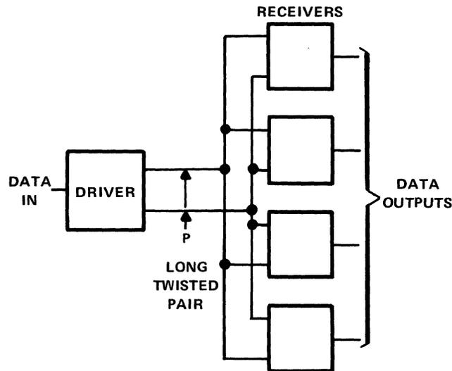
Figure 9-41. Party-Line Concept of One Driver Transmitting to One of Many Receivers
