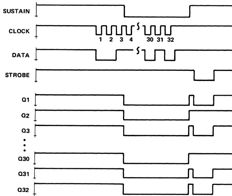
Figure 8-41. Typical Operating Sequence — SN75501C
