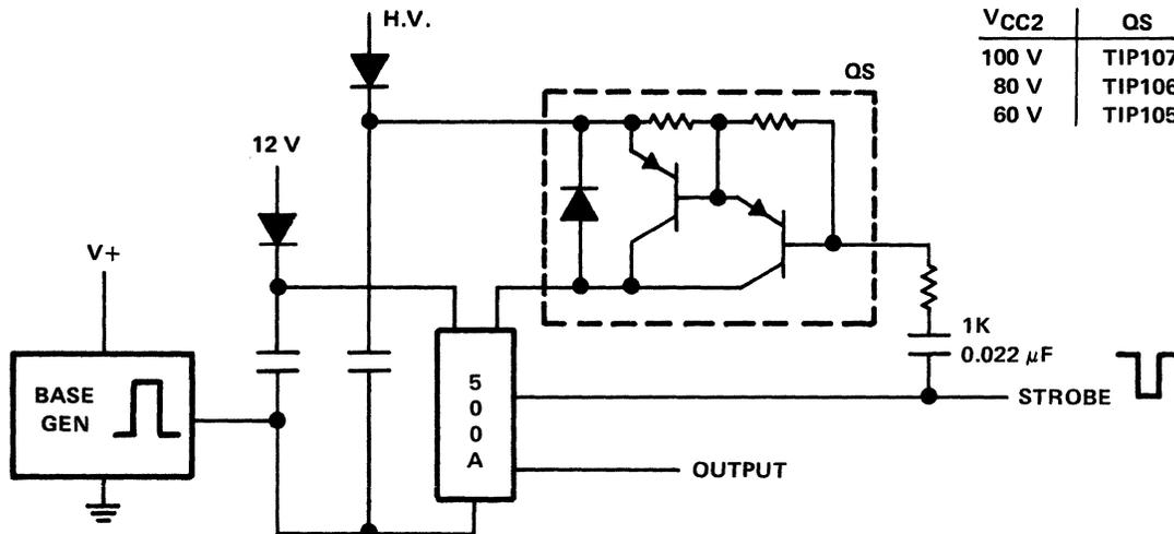
Figure 8-47. Floating SN75500A with Pulsed VCC2
