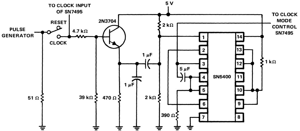
Figure 9-44. Detector Circuit for Clearing SN7495 Clock in Figure 9-43
