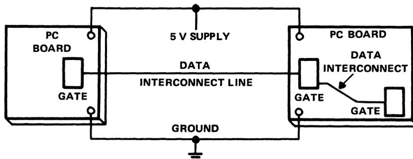
Figure 9-1. Single Wire and Ground Plane
