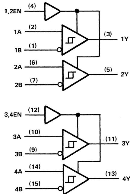
**Figure 9-88. Quad Differential Line Receiver MC3486 and SN75175A**
