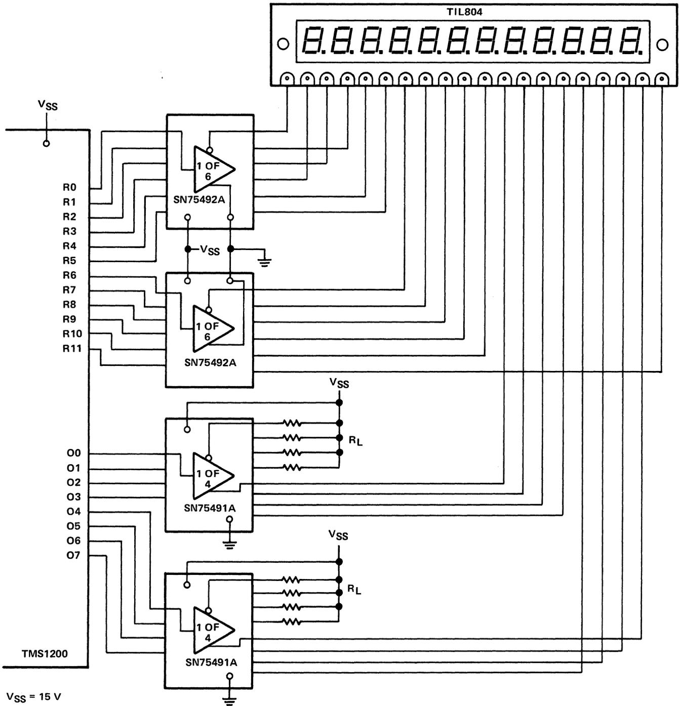
Figure 8-9. 12-Digit LED Numeric Display and Drive
