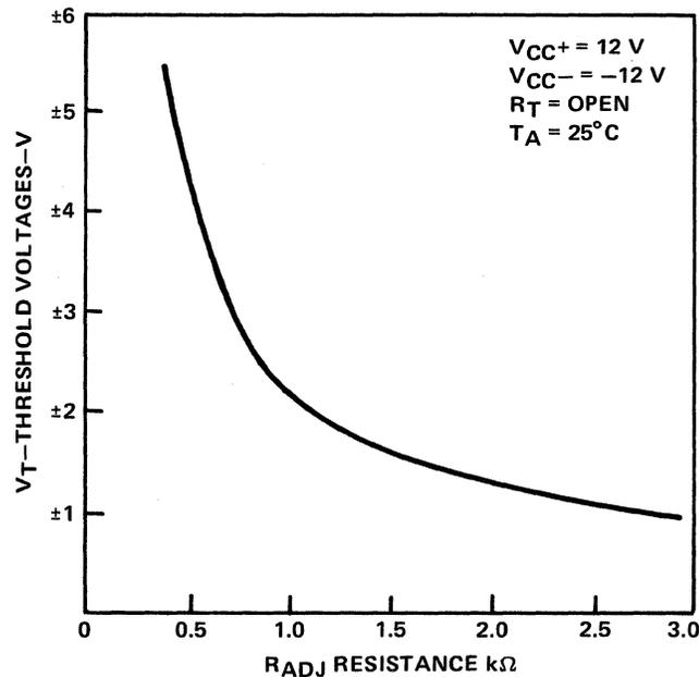
Figure 9-58. Threshold Voltage Versus Hysteresis Adjust Resistance
