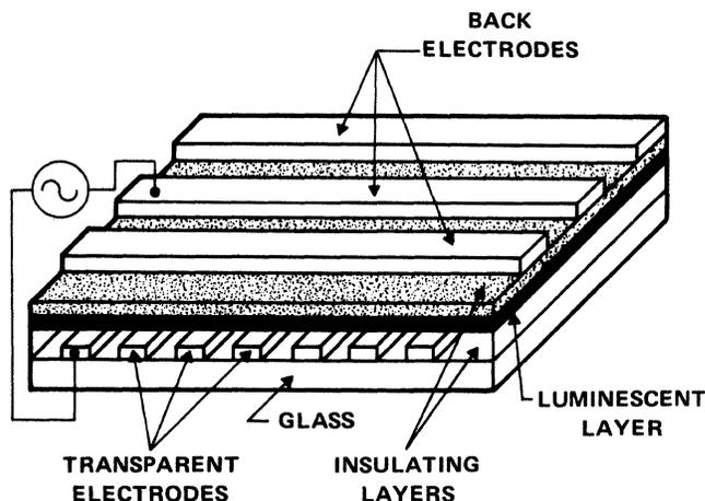
Figure 8-74. TFEL Construction
