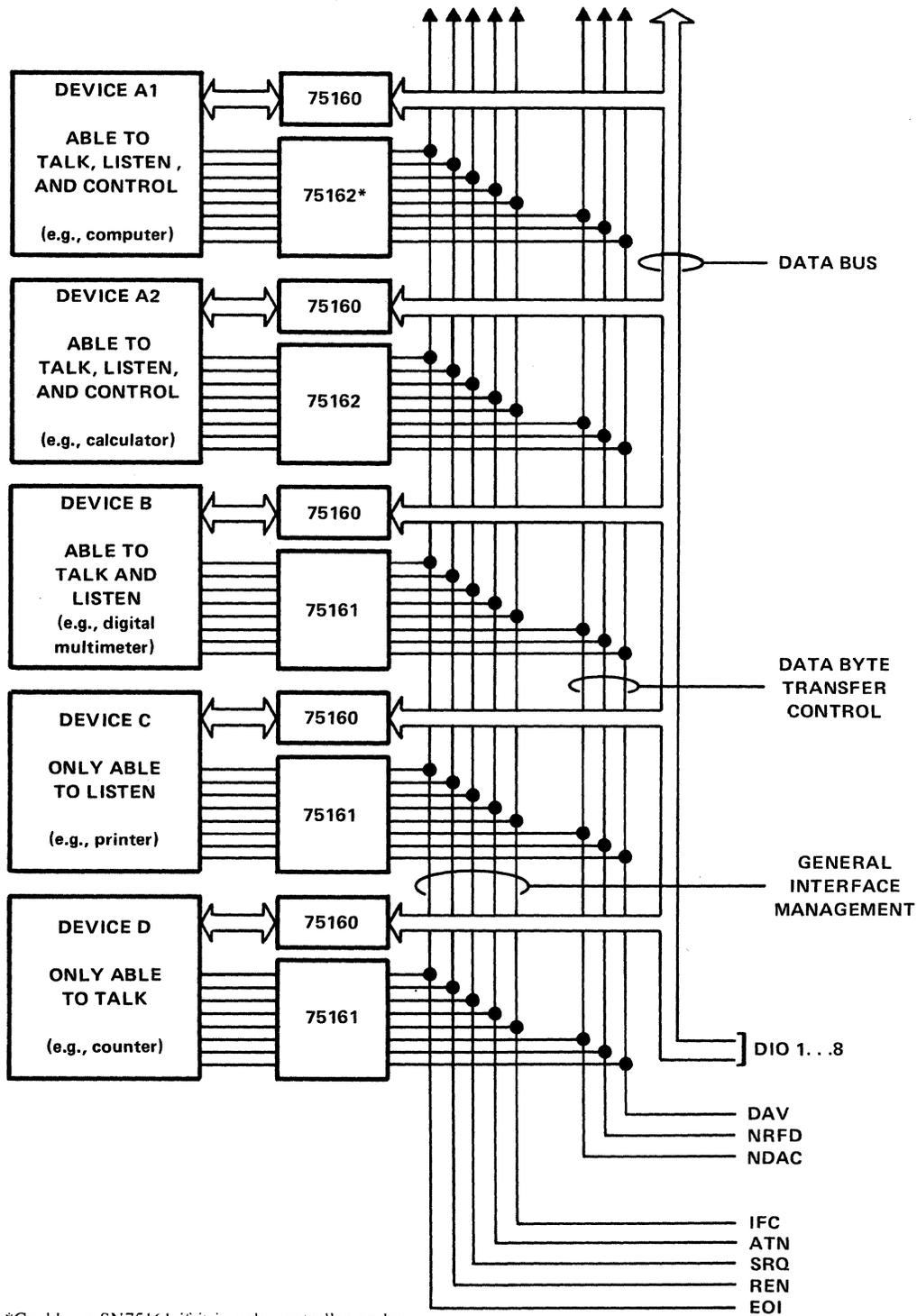
Figure 9-104. Typical IEEE-488 Interface System
