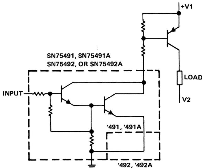
Figure 8-12. Quad or Hex High-Current P-N-P Transistor Driver
