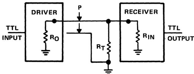
Figure 9-7. Basic, Single Ended, Line Terminations
