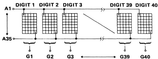
Figure 8-64. A 40: 5 x 7 Dot Character VFD Configuration
