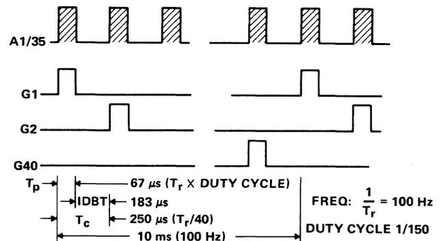
**Figure 8-66. A 40 Character VFD Timing Diagram**
