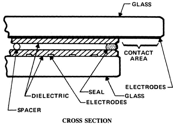
Figure 8-28. Panel Construction
