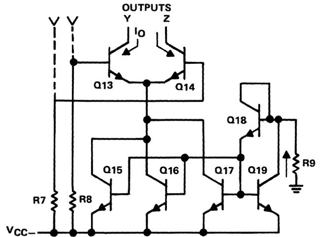
Figure 9-30. Output Circuit
