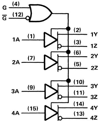
**Figure 9-85. Quad Differential Line Driver AM26LS31 and SN75172B**
