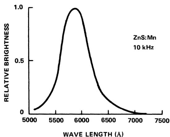
Figure 8-75. TFEL Emission Spectrum
