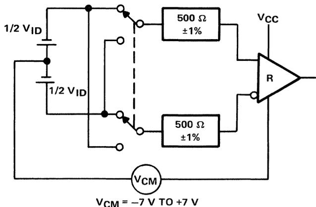
Figure 9-75. Receiver Input Balance Test
