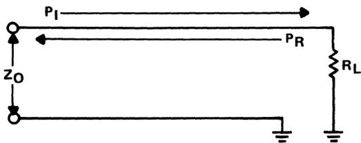
Figure 9-6. Line Incident ( $P_I$ ) and Reflected ( $P_R$ ) Power
