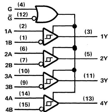
**Figure 9-86. Quad Differential Line Receiver AM26LS32A and SN75173A**
