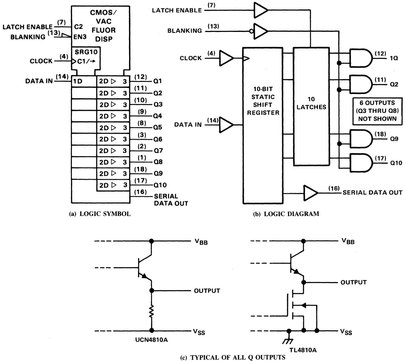
Figure 8-57. UCN4810A and TL4810A VFD Display Drivers
