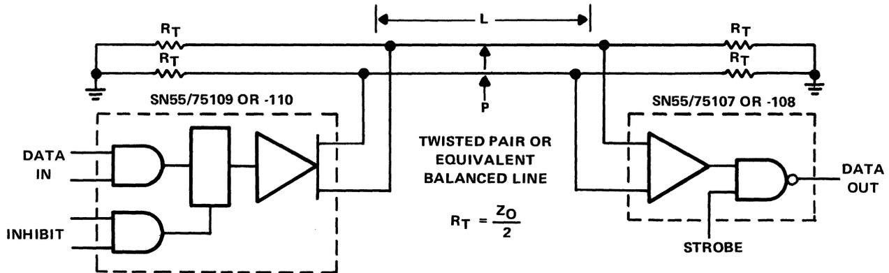
Figure 9-39. Use of SN55107 Series Devices in a Typical Single-Driver, Single-Receiver Transmission System
