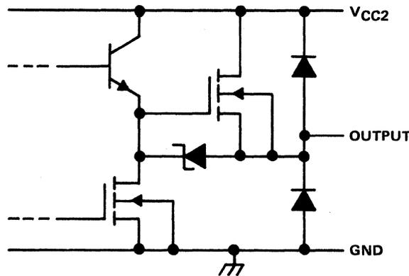
Figure 8-63. SN75501C VFD Driver
