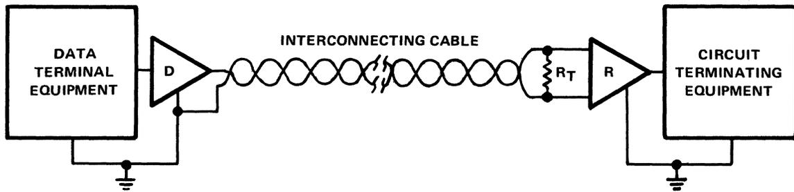
Figure 9-71. Basic RS-423-A Unbalanced Digital Interface
