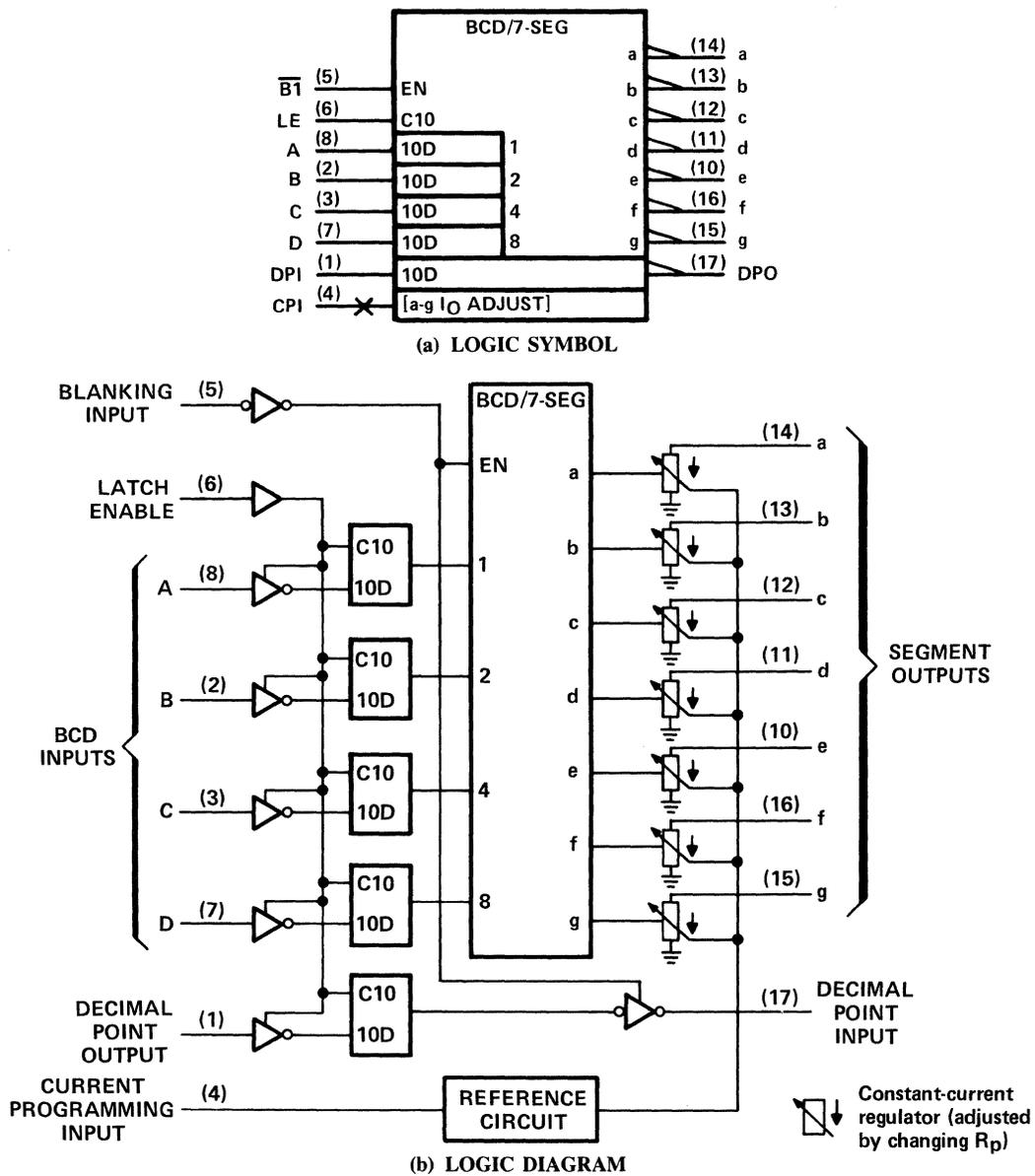
Figure 8-24. SN75584A DC Plasma Segment Driver
