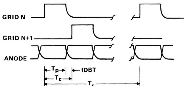
**Figure 8-56. VFD Timing Diagram**
