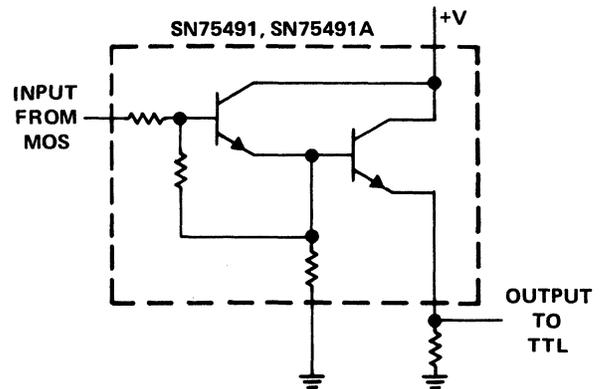
Figure 8-14. MOS to TTL Level Shifter
