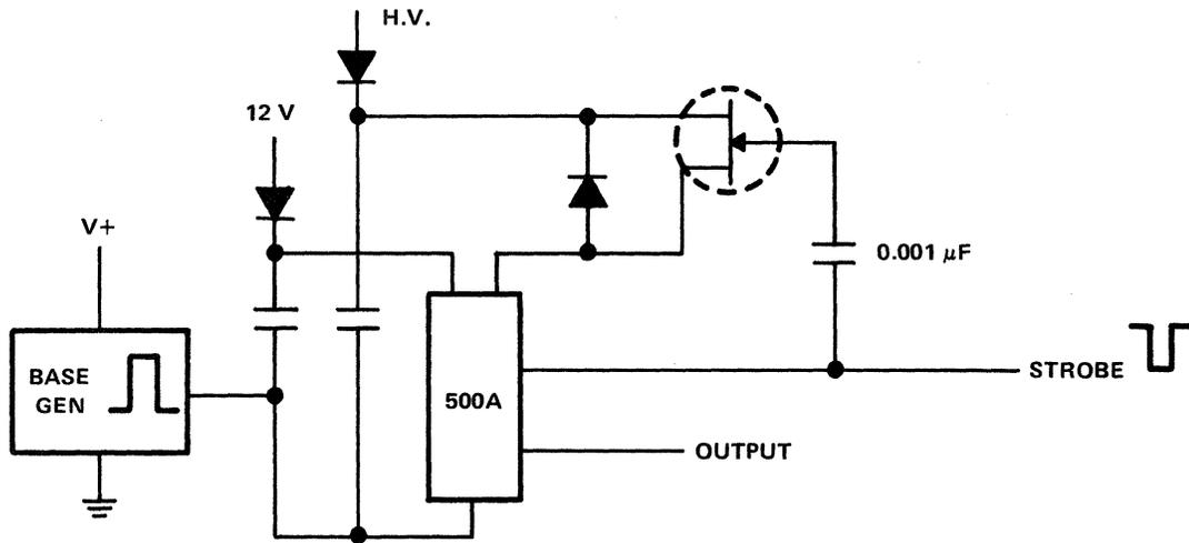
Figure 8-48. Floating SN75500A with FET Pulsed  $V_{CC2}$
