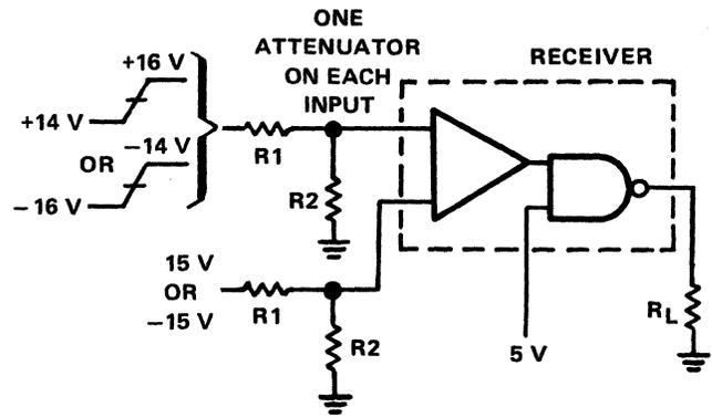
**Figure 9-35. Common-Mode Circuit for Testing Input Attenuators**
