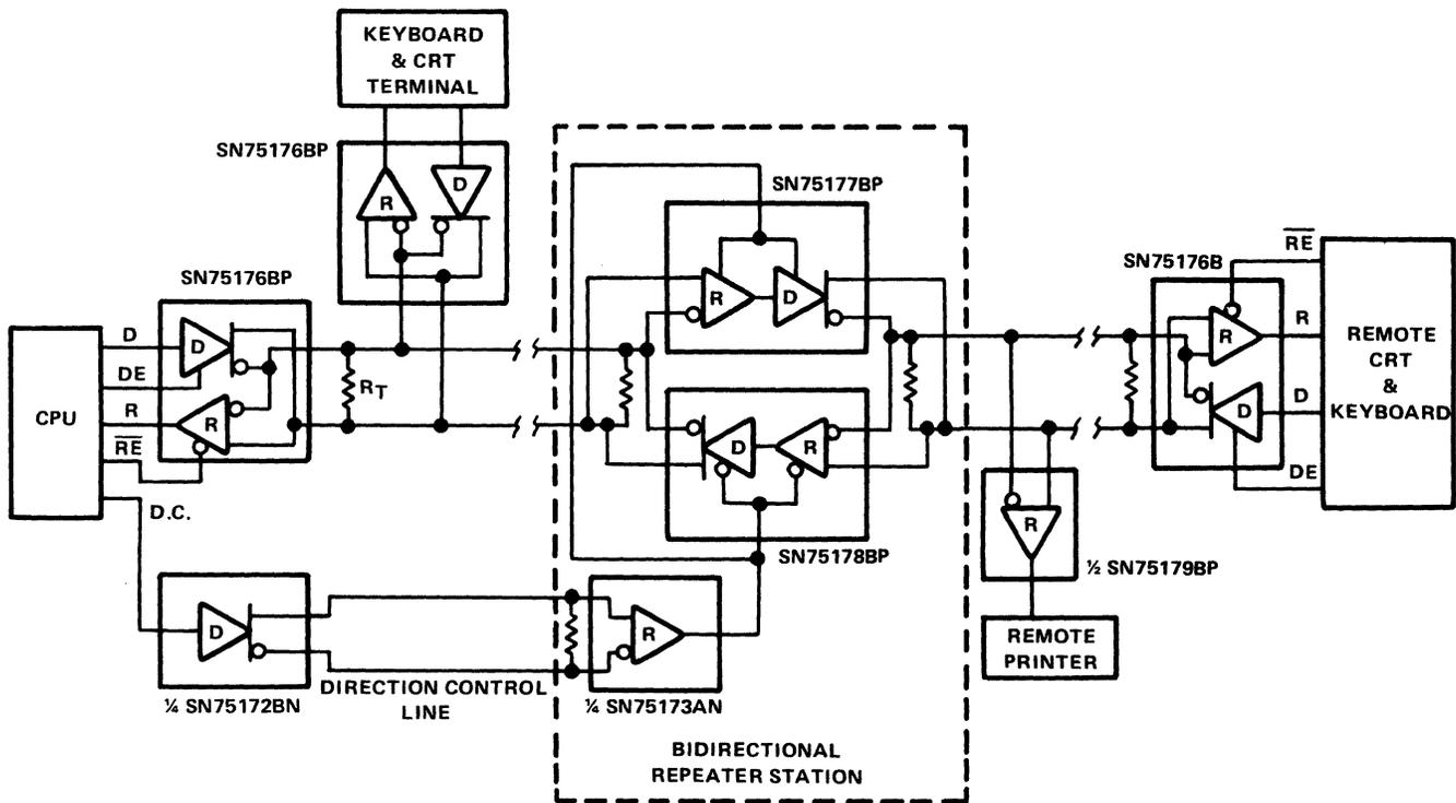
Figure 9-102. SN75177B and SN75178B Allow Bidirectional Long Line Communication
