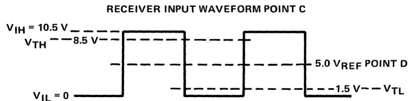
Figure 9-20. Single-Ended Transmission with Receiver Adjusted for High Noise Immunity
