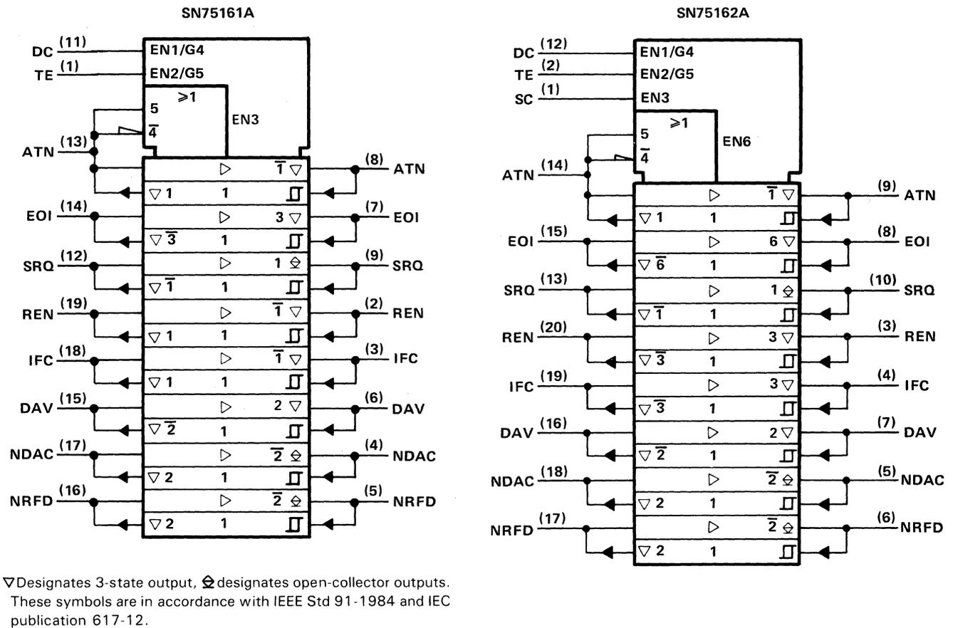
Figure 9-113. Logic Symbols for SN75161A and SN75162A
