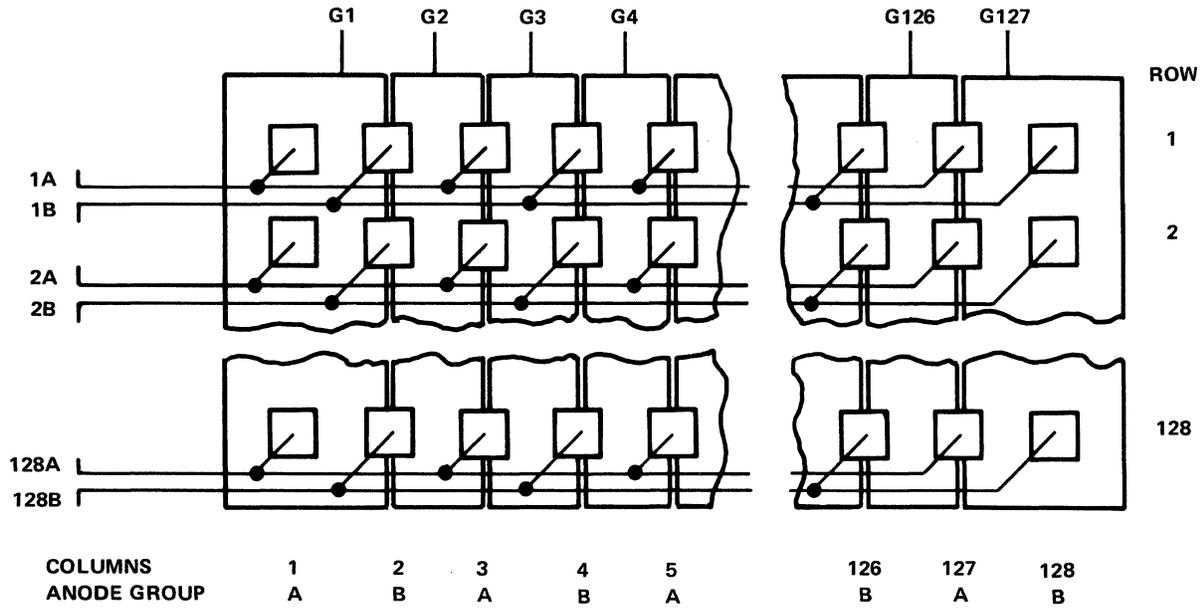
Figure 8-70. A 128 x 128 Dot Matrix VFD Pinout
