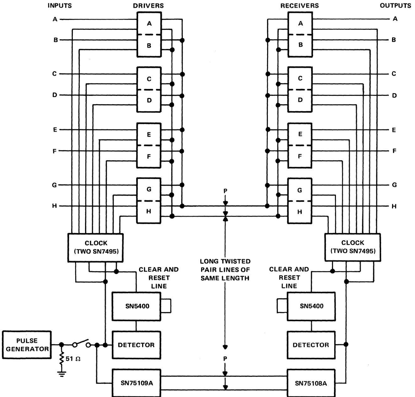
Figure 9-43. A Multi-Channel System with Clocking
