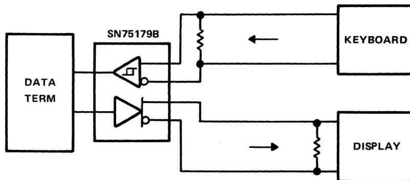
Figure 9-103. SN75179B Independent Driver and Receiver
