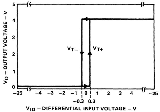
(b)  $V_{ID}$  VERSUS  $V_O$  in MIL-STD-188C CONFIGURATION
