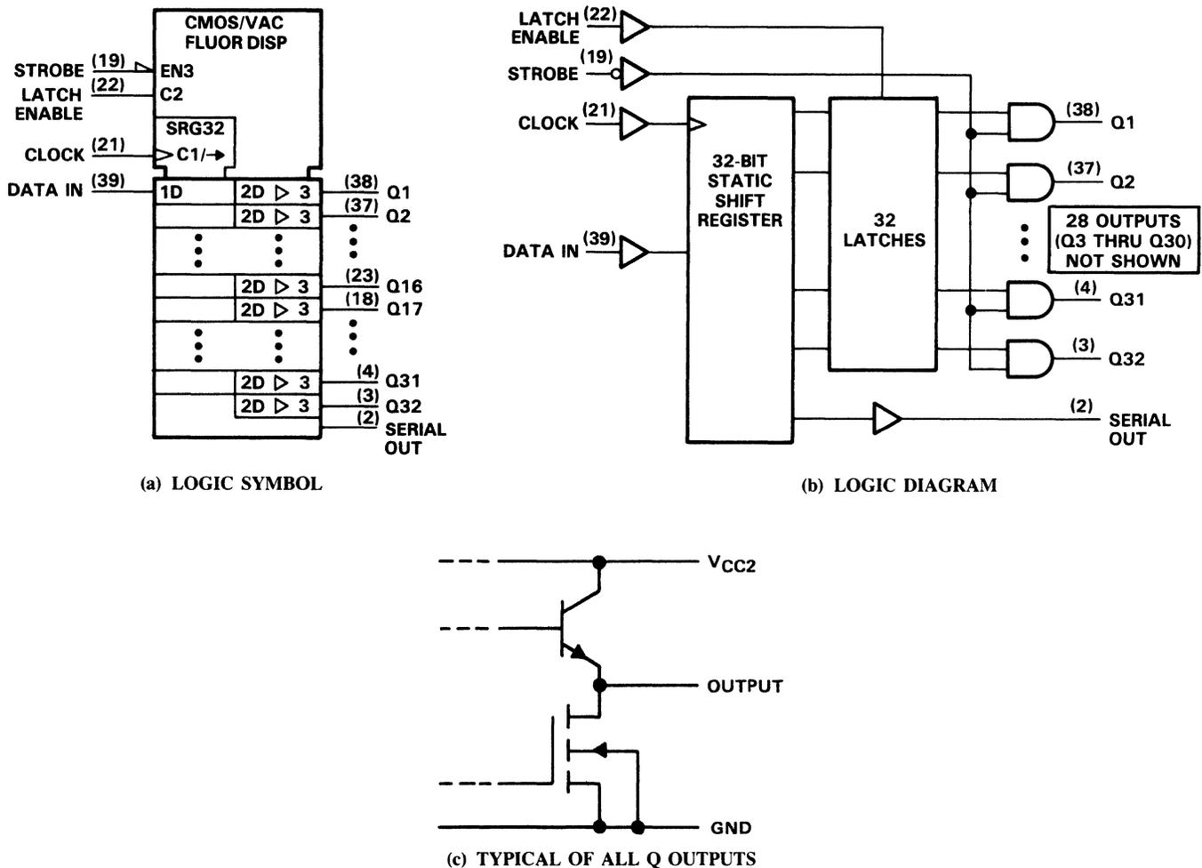
Figure 8-62. SN75518 VFD Driver
