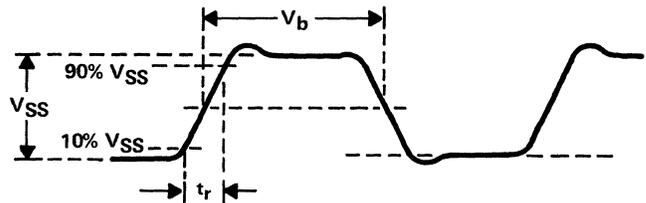
$V_{SS}$  = difference in steady-state voltage levels
