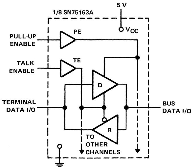
Figure 9-22. SN75163A Functional Diagram
