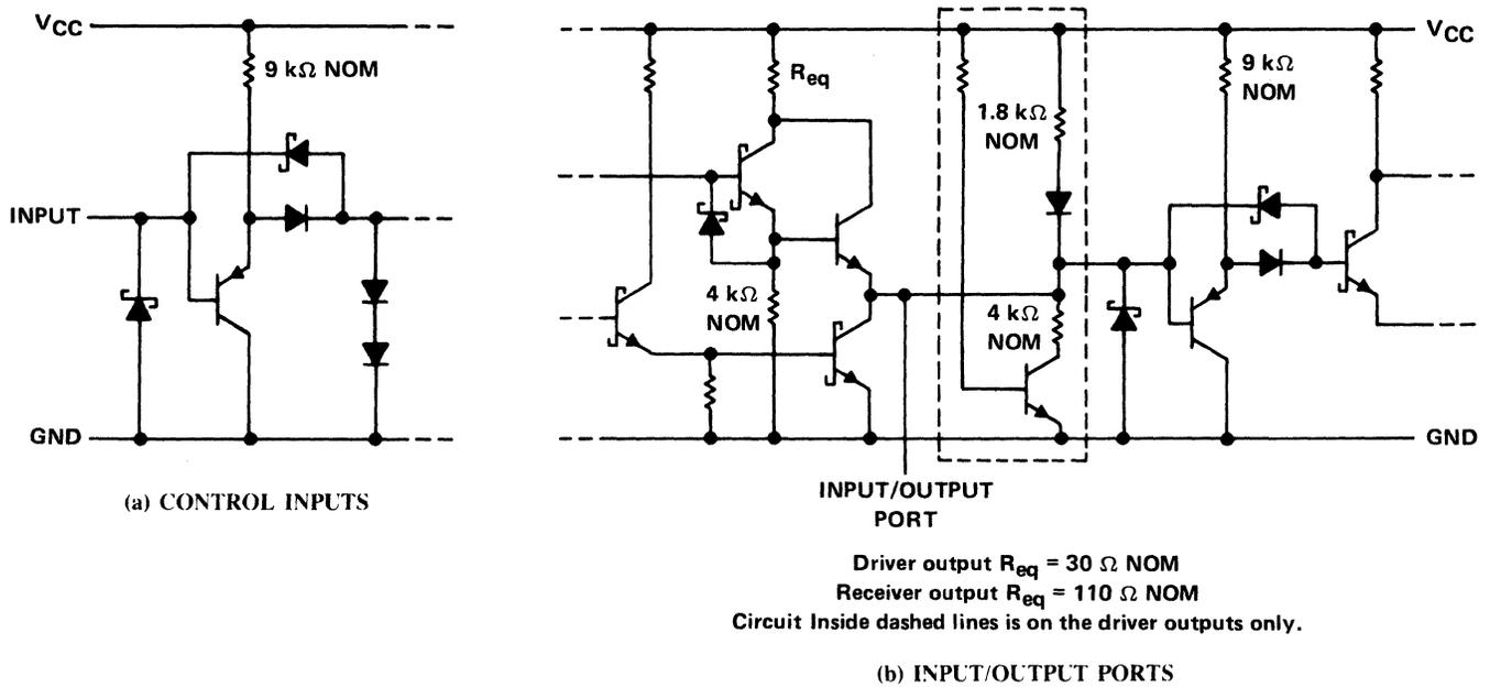
Figure 9-111. Equivalent Schematics of SN75160A Input and Output Sections
