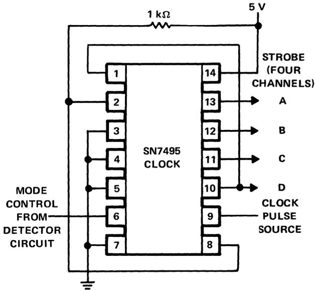
NOTE: IF MORE THAN FOUR CHANNELS ARE NEEDED, USE ADDITIONAL SN7495's CONNECT "D" (PIN 10) TO THE SERIAL INPUT (PIN 1) OF THE SECOND CLOCK AND THE "D" (PIN 10) OUTPUT OF THE LAST CLOCK BACK TO PIN 1 OF THE FIRST CLOCK.
