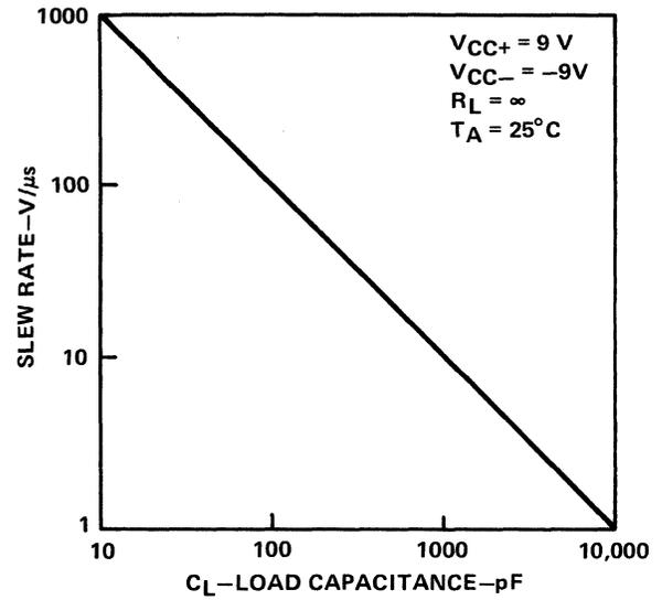
Figure 9-70. Slew Rate Versus Load Capacitance
