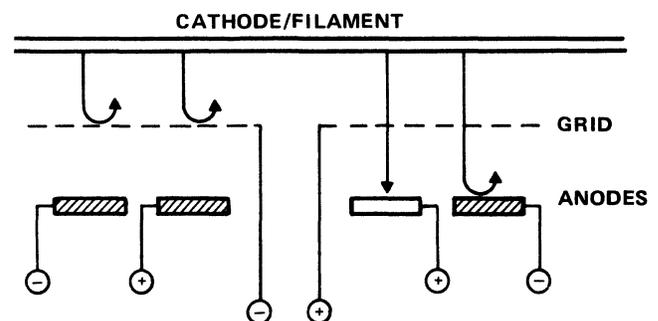
Figure 8-53. Vacuum Fluorescent Display Electron Flow
