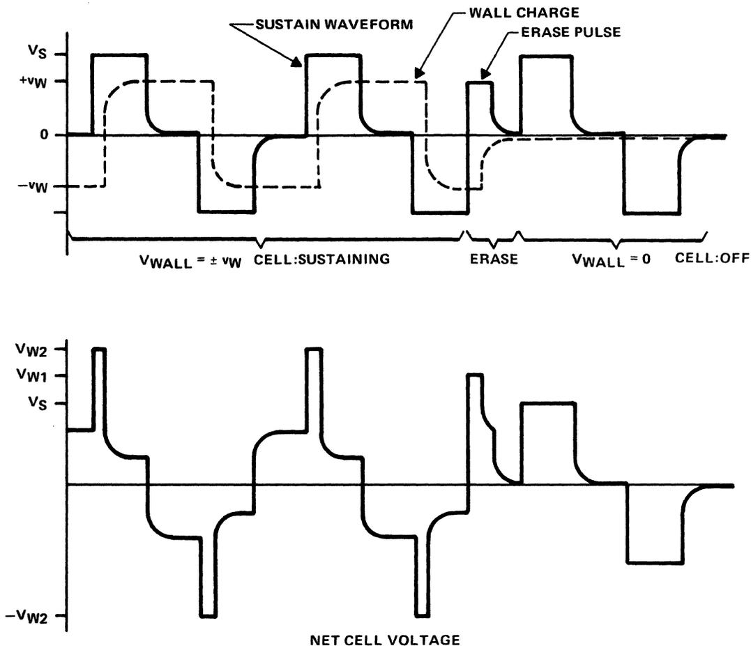
Figure 8-32. Sustain-Erase Cycle Cell Waveforms
