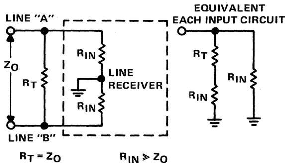
Figure 9-10. Line-to-Line Termination
