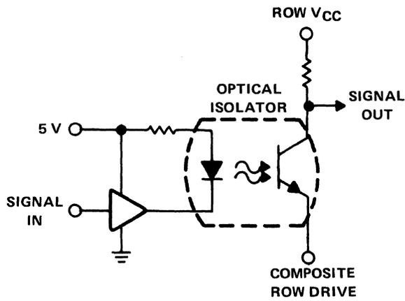
Figure 8-84. Coupling Circuit
