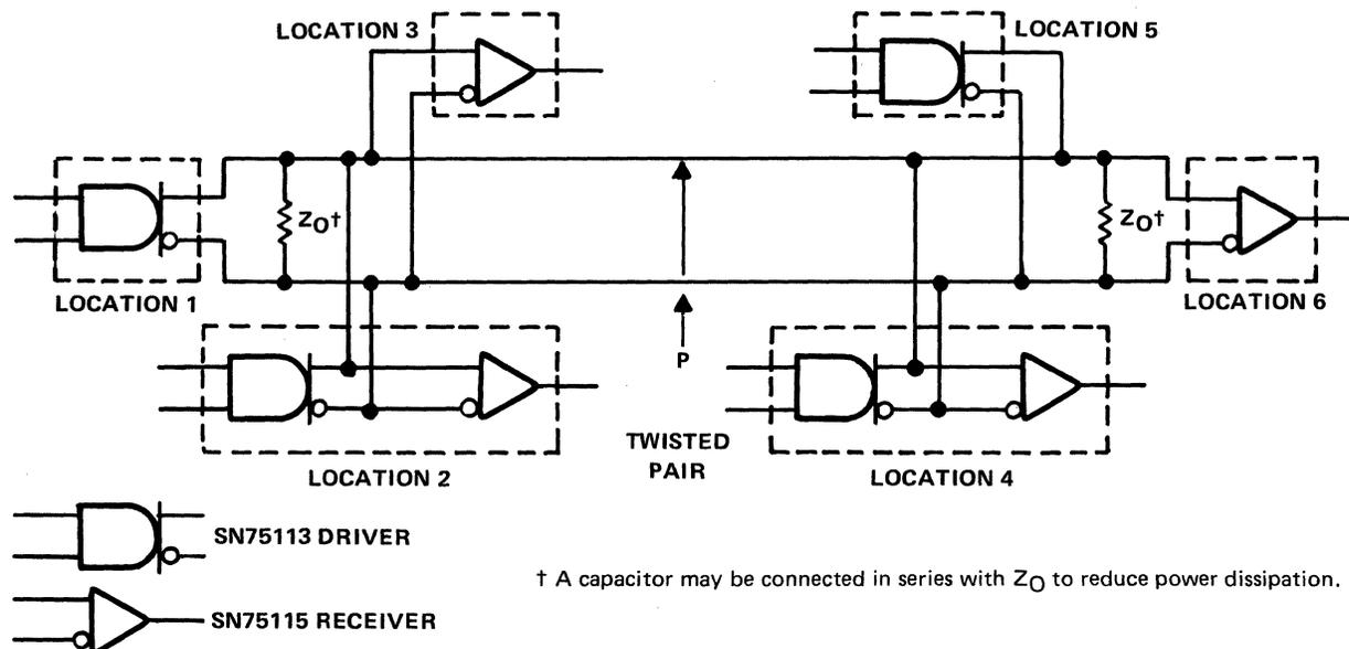
Figure 9-47. Basic Party-Line Differential Data Transmission
