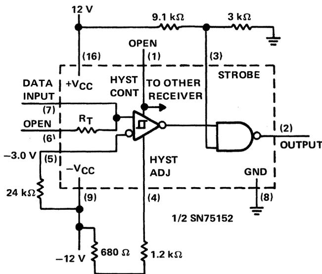
(a) -3 V THRESHOLD,  $\pm 1.5$  V HYSTERESIS CIRCUIT CONFIGURATION
