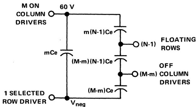
Figure 8-89. Panel Equivalent Circuit
