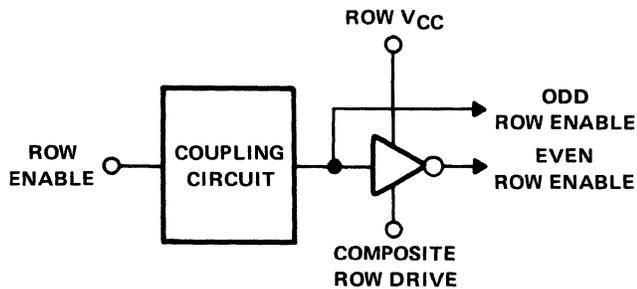
Figure 8-85. Odd and Even Enable Circuits
