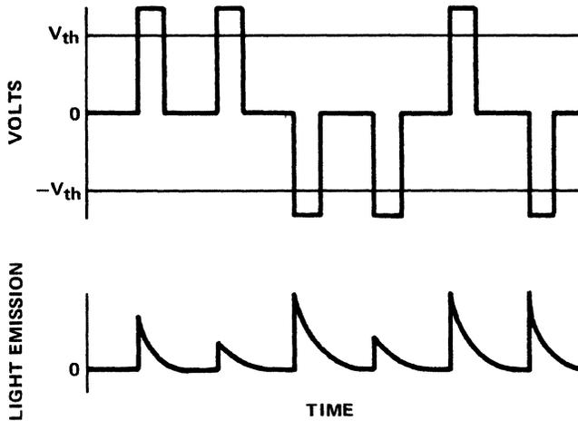
**Figure 8-76. Brightness Dependence on Polarity**
