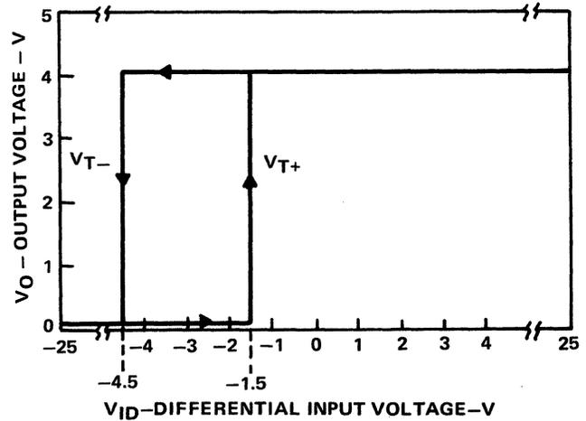
(b) RESULTING  $V_{ID}$  VERSUS  $V_O$
