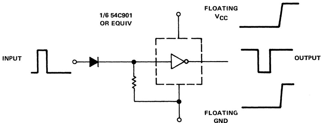
Figure 8-50. Positive Base Signal Data Buffer Circuit
