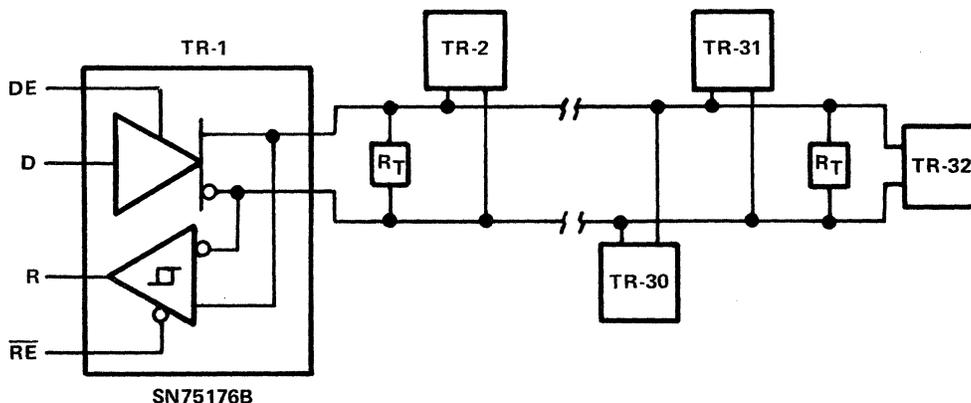
Figure 9-101. SN75176B Transceivers on Multi-Station Bus
