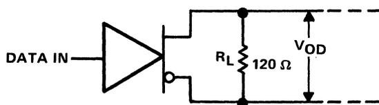
Figure 9-91. Line-to-Line Termination
