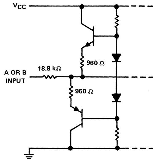
Figure 9-94. Equivalent Receiver A or B Input
