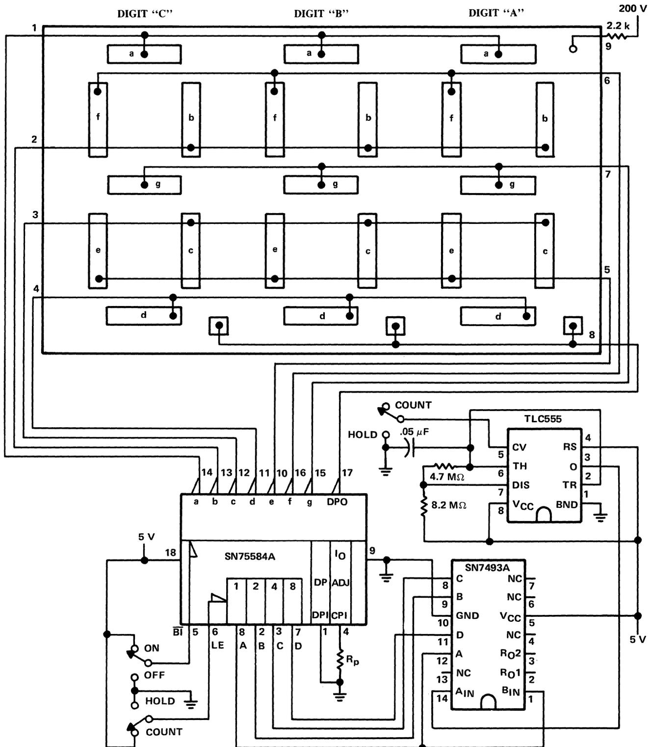
Figure 8-27. Three-Digit Display Driver Application
