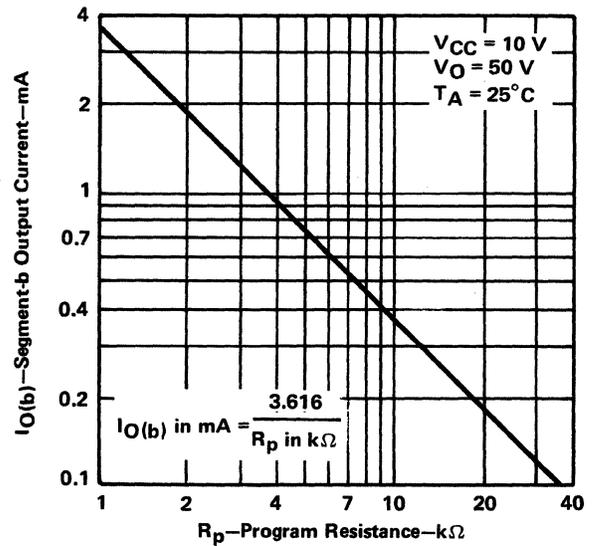
Figure 8-25. SN75584A Segment Output Current vs Program Resistance
