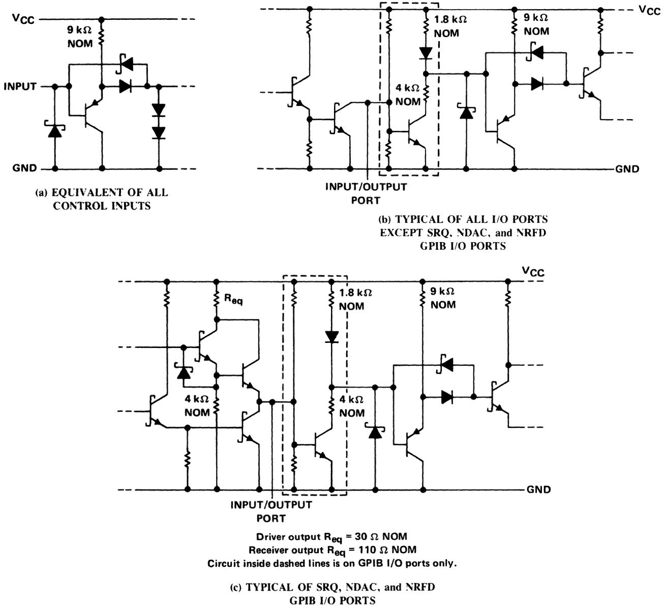
Figure 9-115. Input/Output Sections of SN75161A and SN75162A
