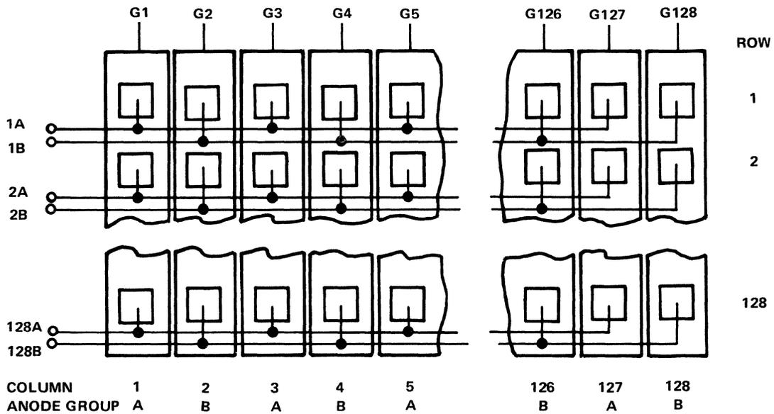
Figure 8-72. A 128 x 128 Dot Matrix VFD Pinout
