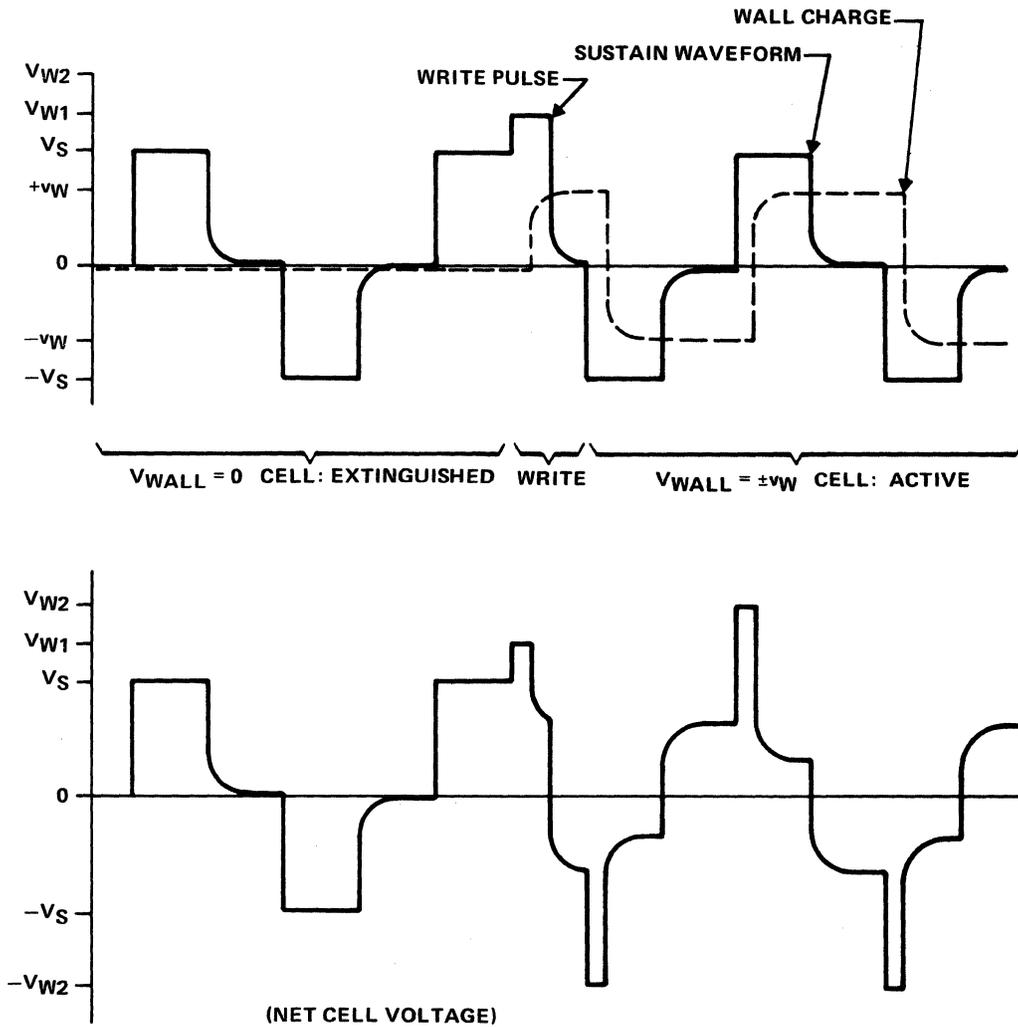
Figure 8-30. Write-Sustain Cycle Cell Waveforms
