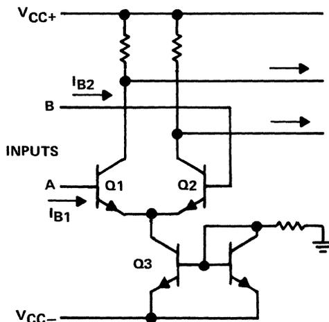
Figure 9-33. Receiver Input Stage, Input Current Source, and Bias Circuit
