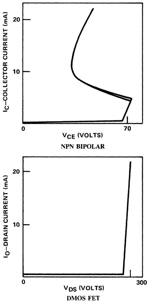
Figure 8-3. Breakdown Characteristics
