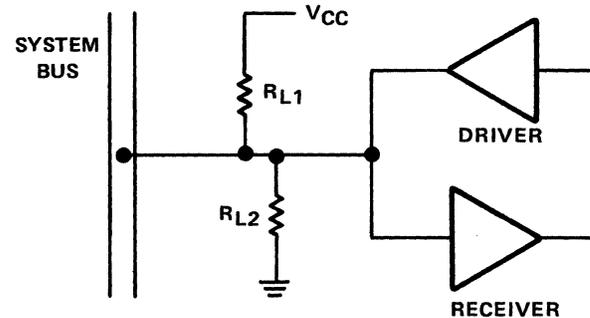
Figure 9-107. Typical Signal Line I/O Circuit
