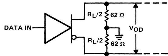
Figure 9-92. Line-to-Ground Termination
