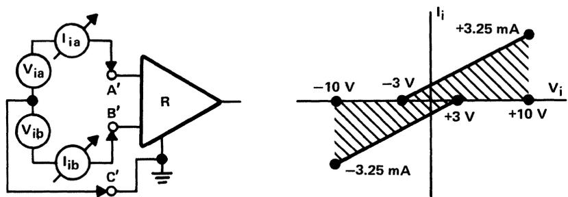
Figure 9-73. Receiver Input Current-Voltage Measurement
