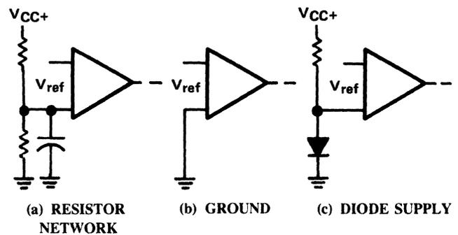
**Figure 9-36. Some Methods of Referencing Receiver Inputs**
