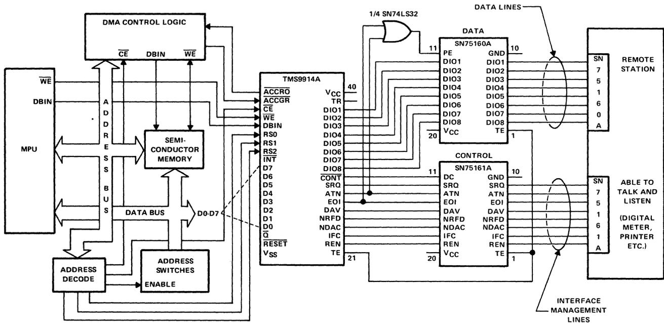
Figure 9-119. Typical IEEE-488 System Application
