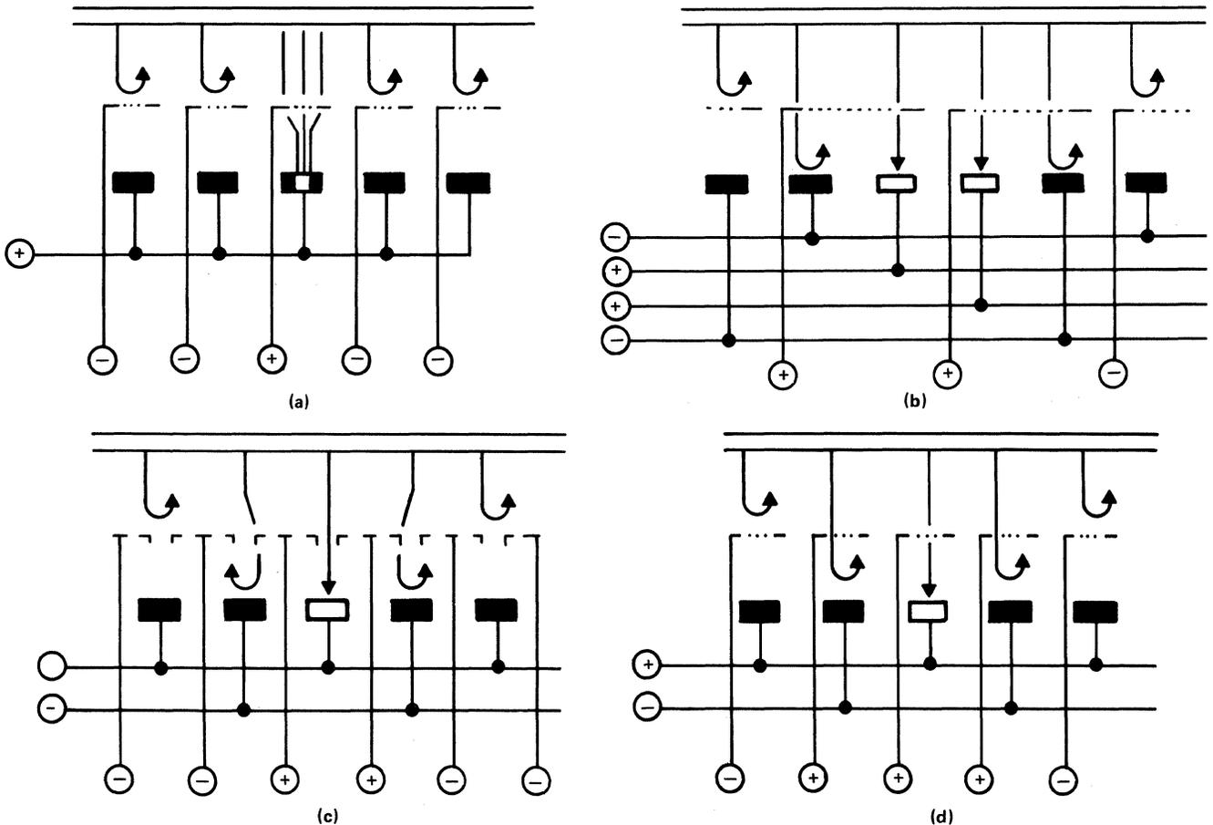
**Figure 8-55. Grid-Anode Configurations of Dot Matrix VFDs**
