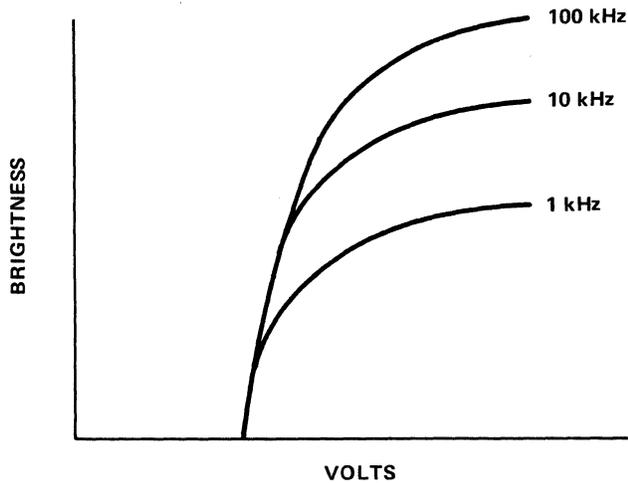
Figure 8-78. Brightness Dependence on Frequency
