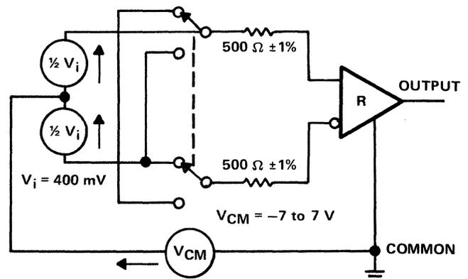
Figure 9-81. Receiver Input Balance Test
