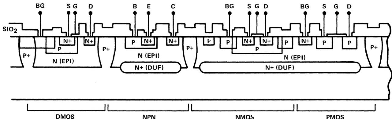
Figure 8-1. BIDFET Cell Cross Section
