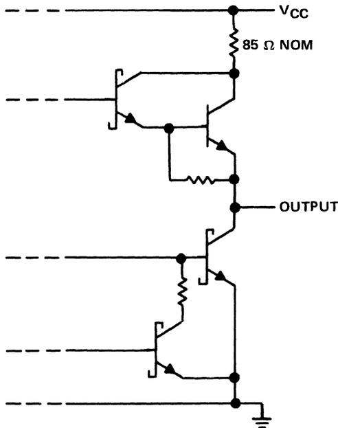
Figure 9-95. Equivalent Receiver Output
