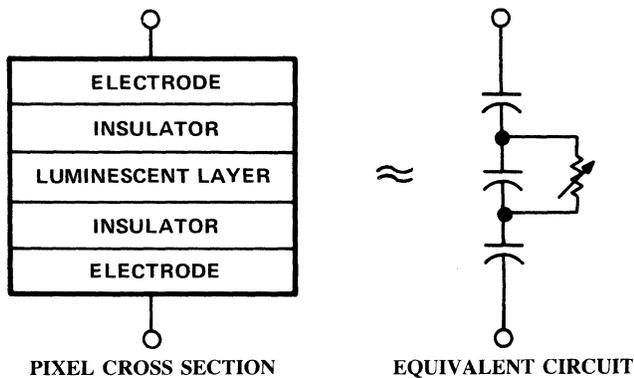
Figure 8-79. Pixel Equivalent Circuit
