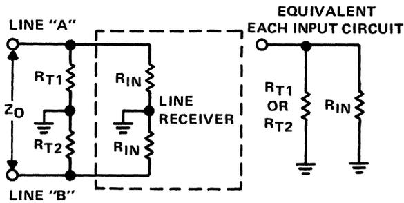
Figure 9-11. Termination to Ground
