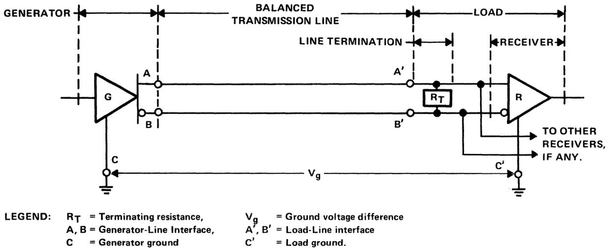
Figure 9-78. Balanced Digital Interface
