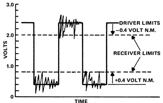
Figure 9-14. TTL Gate Noise Margins
