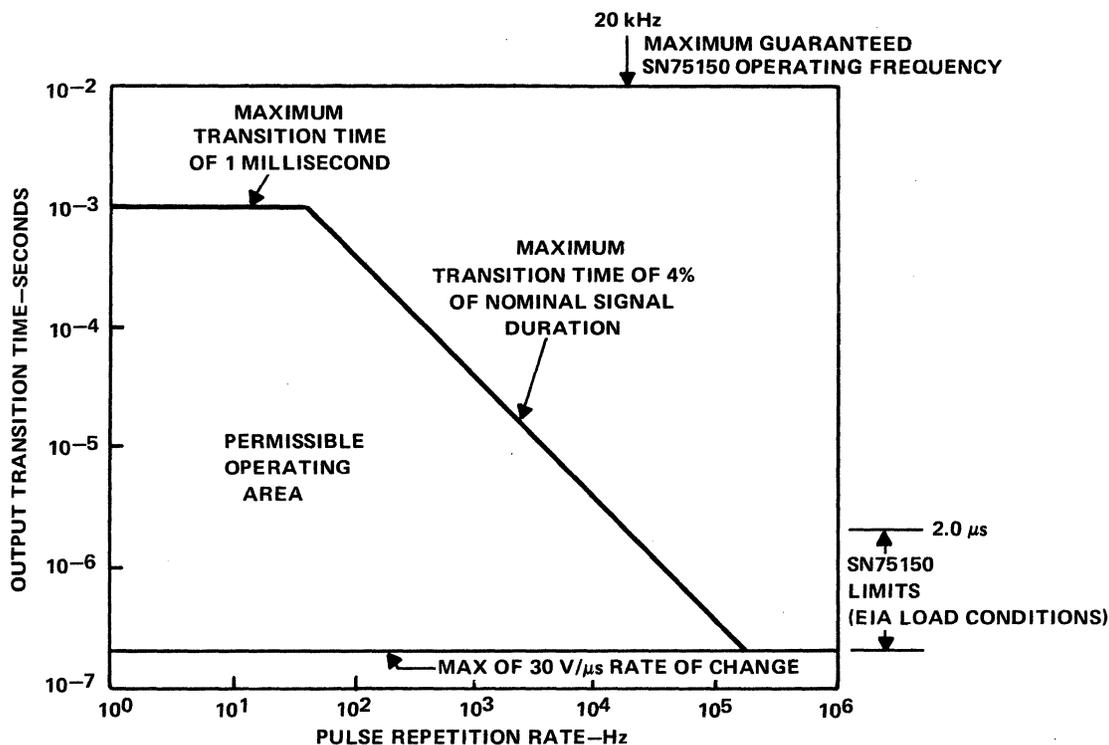
Figure 9-67. Pulse Repetition Rate Versus Output Transition Time of SN75150
