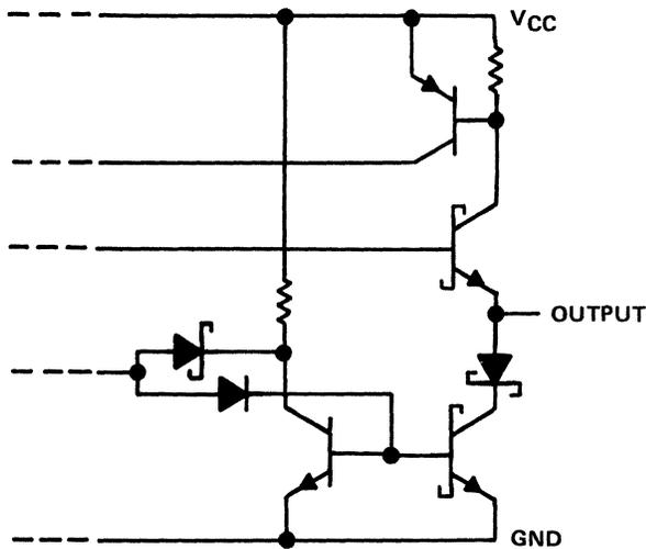
Figure 9-90. Equivalent Each Driver Output
