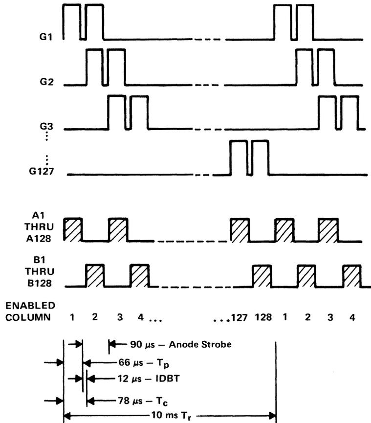
Figure 8-71. Timing Diagram for VFD 1128 x 128 Dot Matrix
