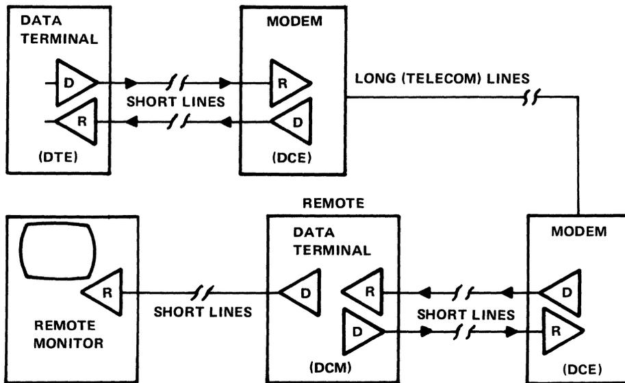
Figure 9-49. RS-232-C Drivers and Receivers in a Basic Data Communications System
