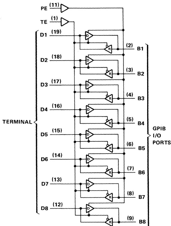
Figure 9-110. SN75160A Logic Symbol and Logic Diagram (Positive Logic)
