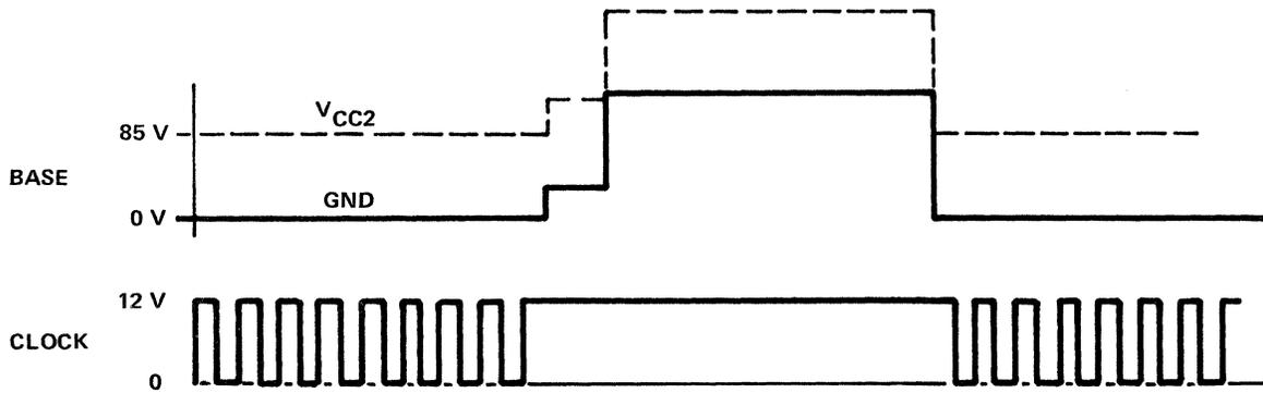
Figure 8-49. Gated Clock for Floating Applications
