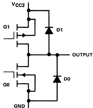
Figure 8-42. SN75500A and SN75501C Output Structure
