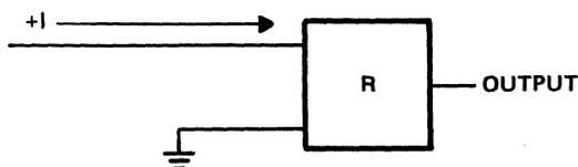
Figure 9-122. Receiver Input Current Polarity
