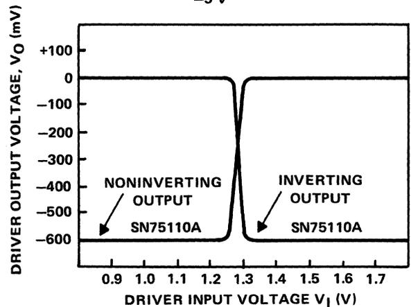
Figure 9-31. Typical Voltage Plot for SN75110A Driver
