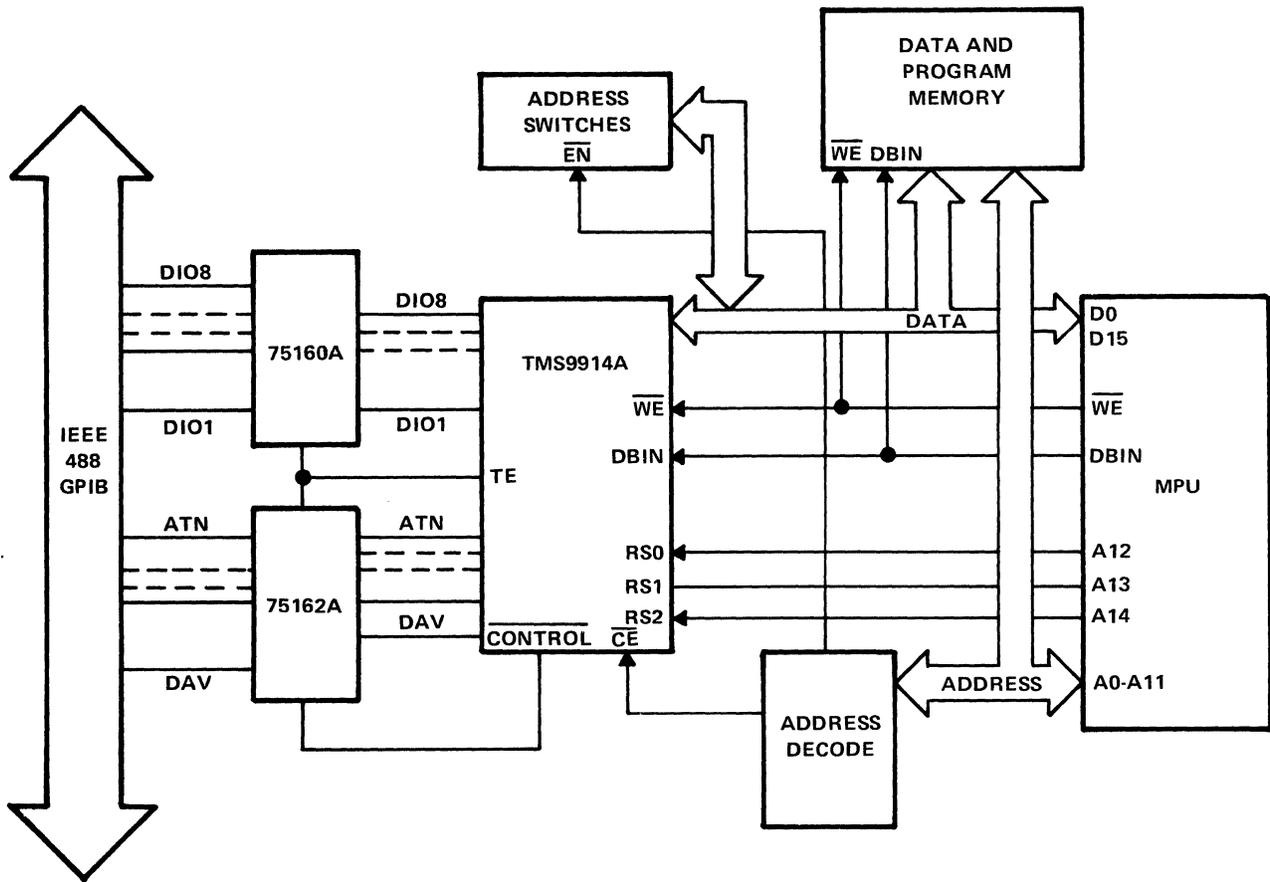
Figure 9-118. Typical TMS9914A Application Block Diagram
