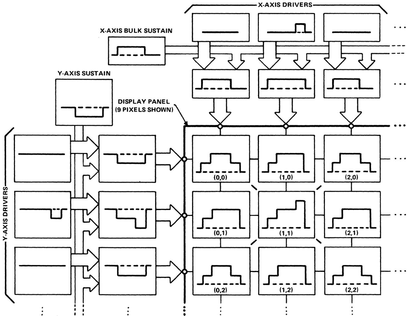
Figure 8-37. Write Waveform Array and Origin Split Axis Sustain — Blanking Select
