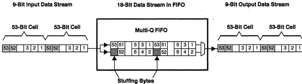
**Figure 5. Data Stream With Odd Cell Size**
