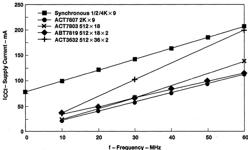
Figure 8. Active  $I_{CC}$  Versus Frequency
