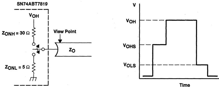
**Figure 4. Shelf Voltage When Switching a Transmission Line**
