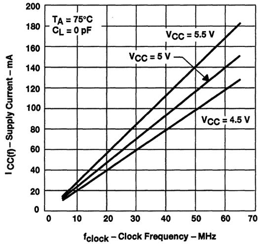
Figure 4. SN74ACT7803 Supply Current Versus Clock Frequency
