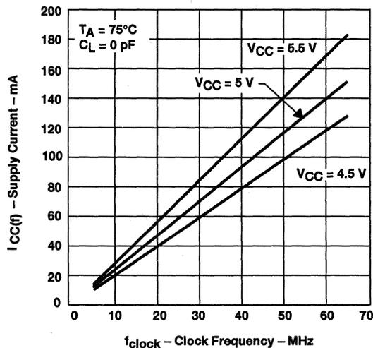
Figure 2. SN74ACT7806 Supply Current Versus Clock Frequency
