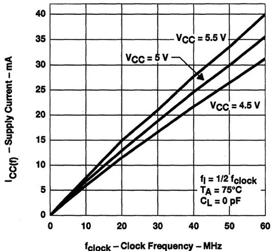
Figure 2. SN74ACT2227 and SN74ACT2229 Single FIFO Supply Current Versus Clock Frequency
