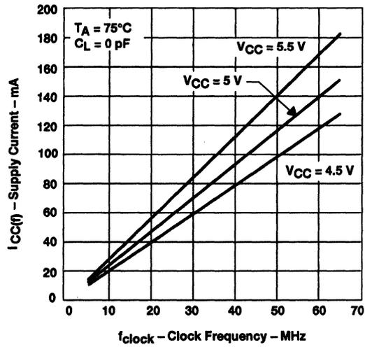
Figure 7. SN74ACT7813 Supply Current Versus Clock Frequency
