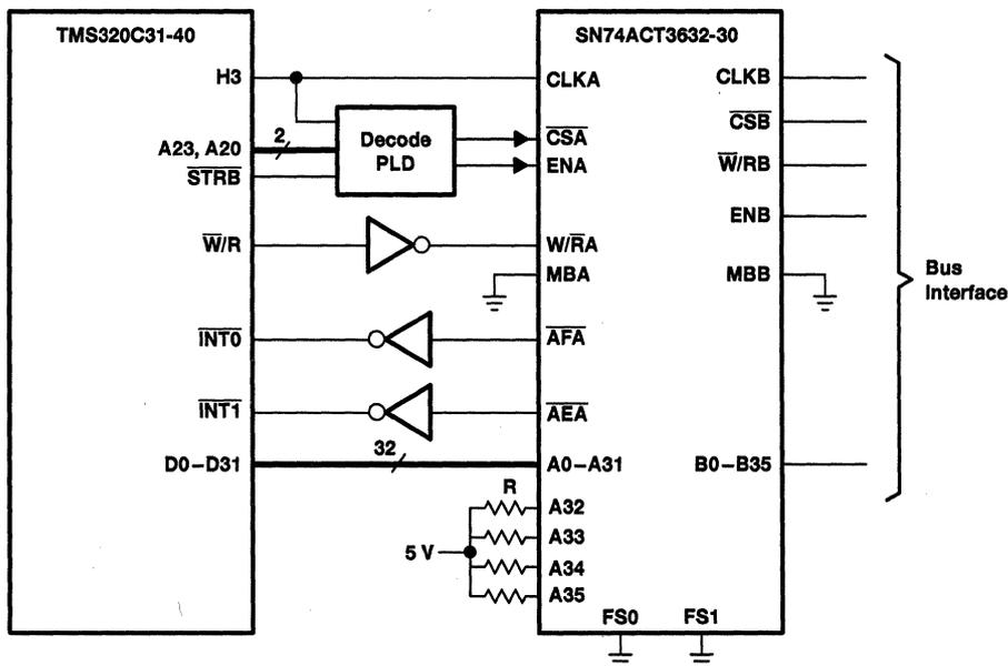
Figure 11. TMS320C31-40 Interface to an SN74ACT3632-30 FIFO
