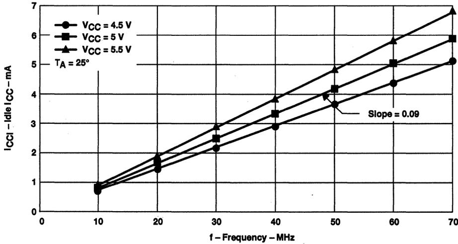
Figure A-7. SN74ACT7807 Idle  $I_{CC}$  With RDCLK Switching, Other Inputs at 0 or  $V_{CC} - 0.2\text{ V}$  and Outputs Disconnected
