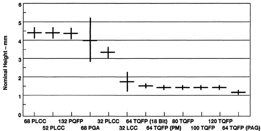
Figure 7. Typical Package Height Versus Height Variance
