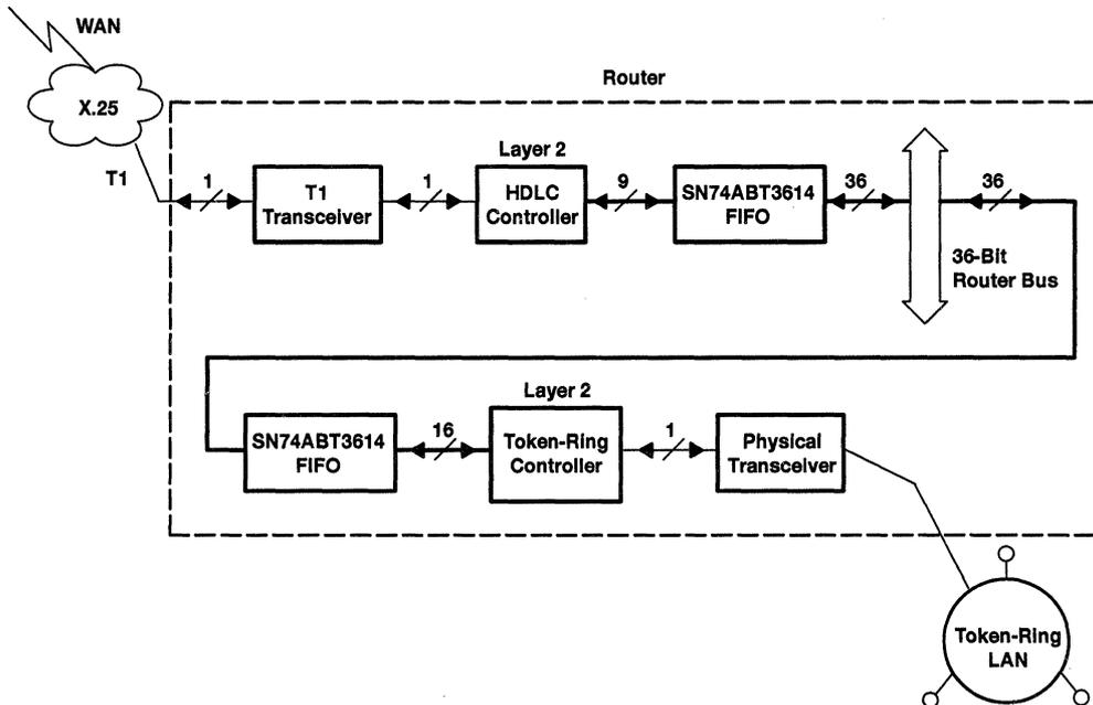
Figure 17. WAN to Token-Ring Router Using SN74ABT3614 FIFO
