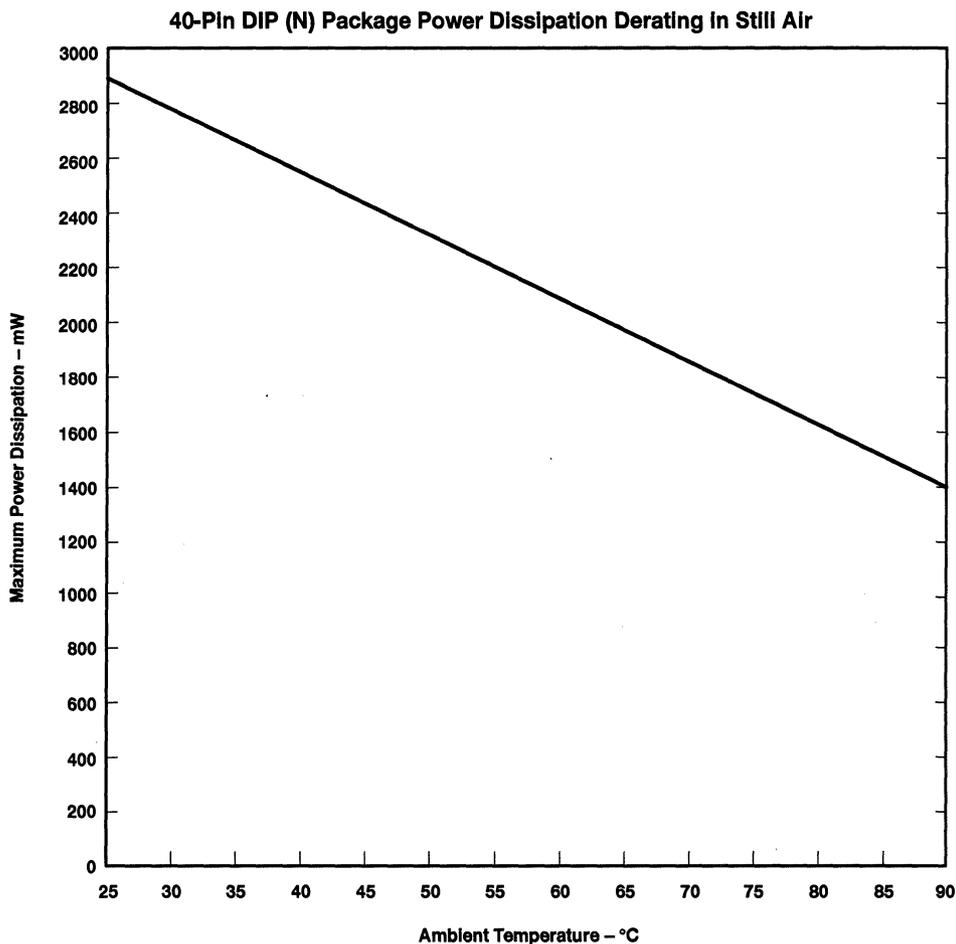
**Thermal Resistance ( $\theta$ ) Measurements†**
