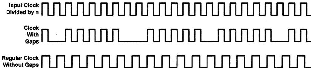
Figure 15. Clock Signals at the Receiver
