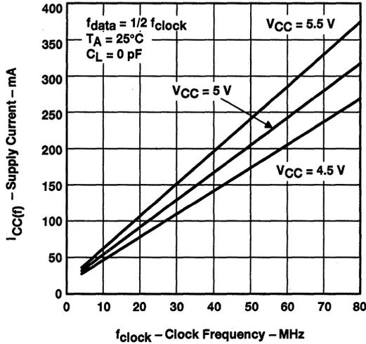
Figure 1. SN74ABT3611 Supply Current Versus Clock Frequency
