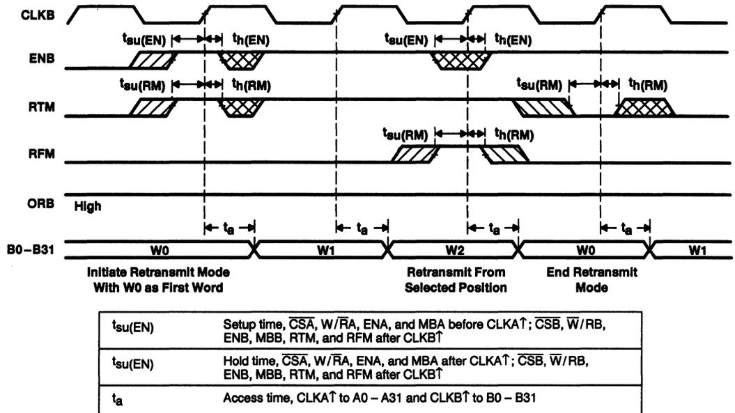
Figure 2. FIFO1 Retransmit Timing Diagram Showing Minimum Retransmit Length
