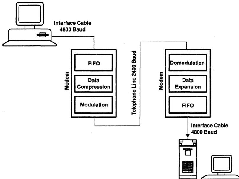
**Figure 16. Data Transmission by Modem With Data Compression**
