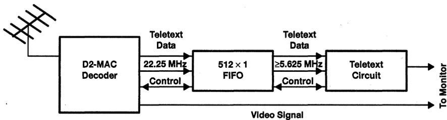
**Figure 21. Teletext Decoder With 1 × 512 FIFO Block Diagram**
