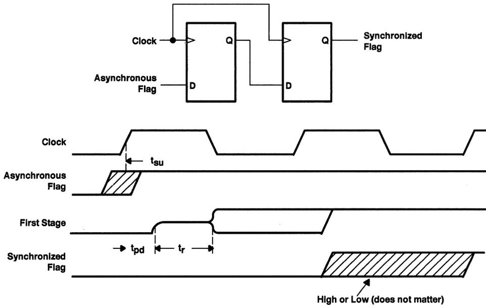
**Figure 3. Two-Stage Synchronizer**
