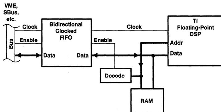
**Figure 3. Bidirectional Clocked FIFO Used for Bus-Speed Matching**
