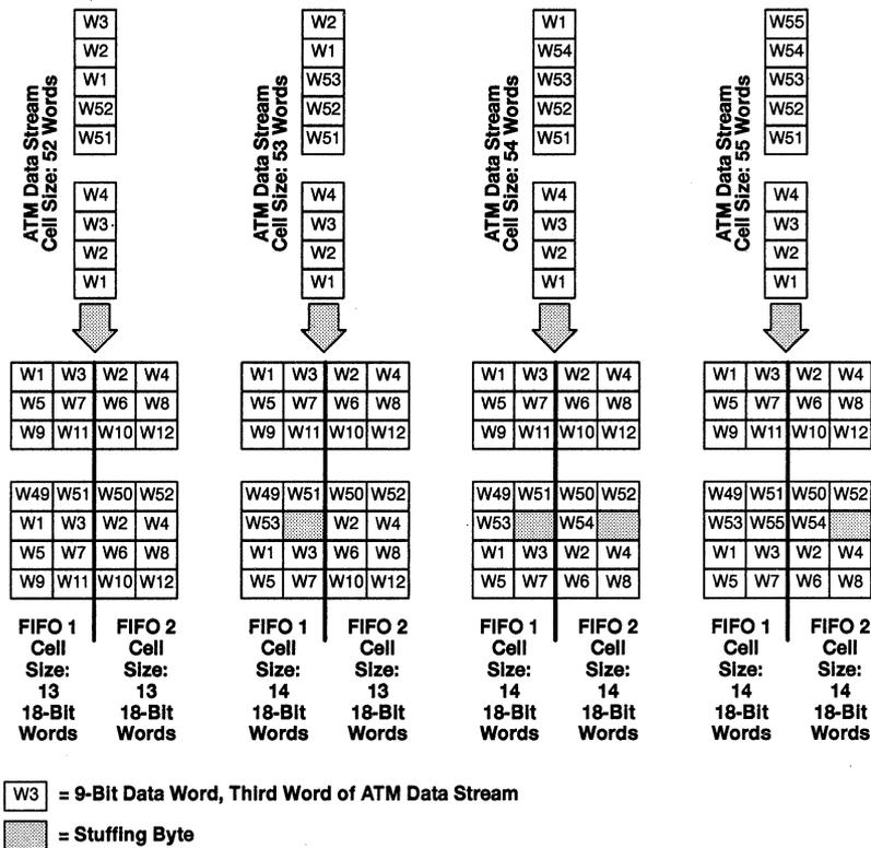
NOTE A: Two Multi-Q FIFOs are connected as a 36-bit-wide FIFO with 9-bit data access.
