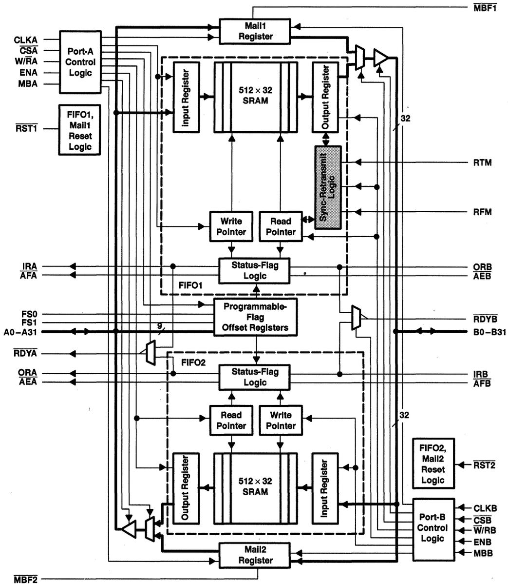
Figure 1. SN74ACT3638 Functional Block Diagram
