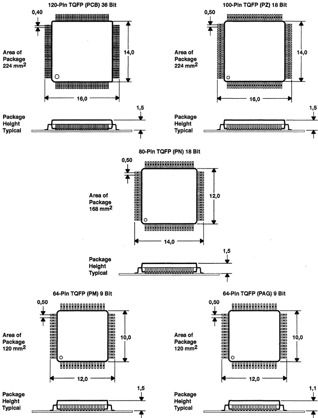
NOTE: Dimensions are in millimeters.
