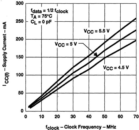
Figure 1. SN74ACT3632 Supply Current Versus Clock Frequency
