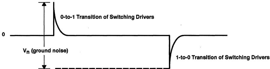
Figure 3. Example of Ground-Bounce Waveform<sup>2</sup>
