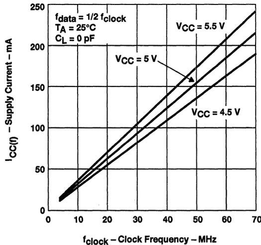
Figure 2. SN74ACT3638 Supply Current Versus Clock Frequency
