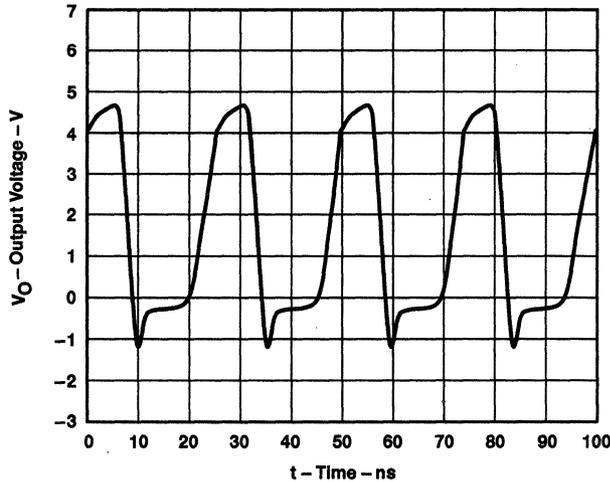
Figure 2. Output Waveform at 80-MHz Clock ( $C_L = 50$  pF)
