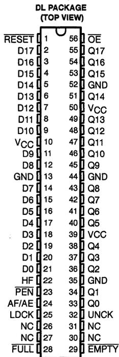
**Figure 4. SN74ACT7814 FIFO With Multiple GND Pins**
