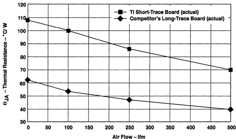
**Figure 1. Competitor Versus TI K-Factor Board (52-pin MQFP)**
