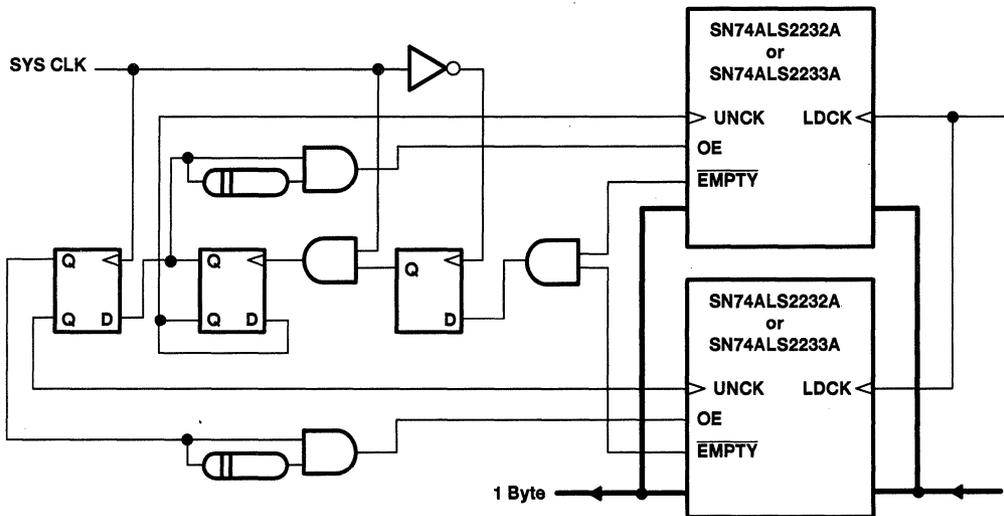
Figure 7. Bus-Folding Logic
