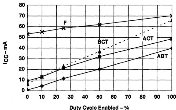
Figure 5.  $I_{CC}$  Versus Duty Cycle Enabled (25 MHz)
