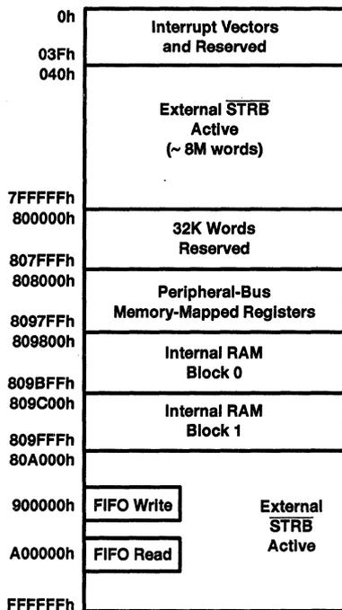
**Figure 6. TMS320C31 Memory Map in Microprocessor Mode**
