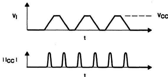
**Figure 3. Current Waveform When Switching Frequency Is Doubled**
