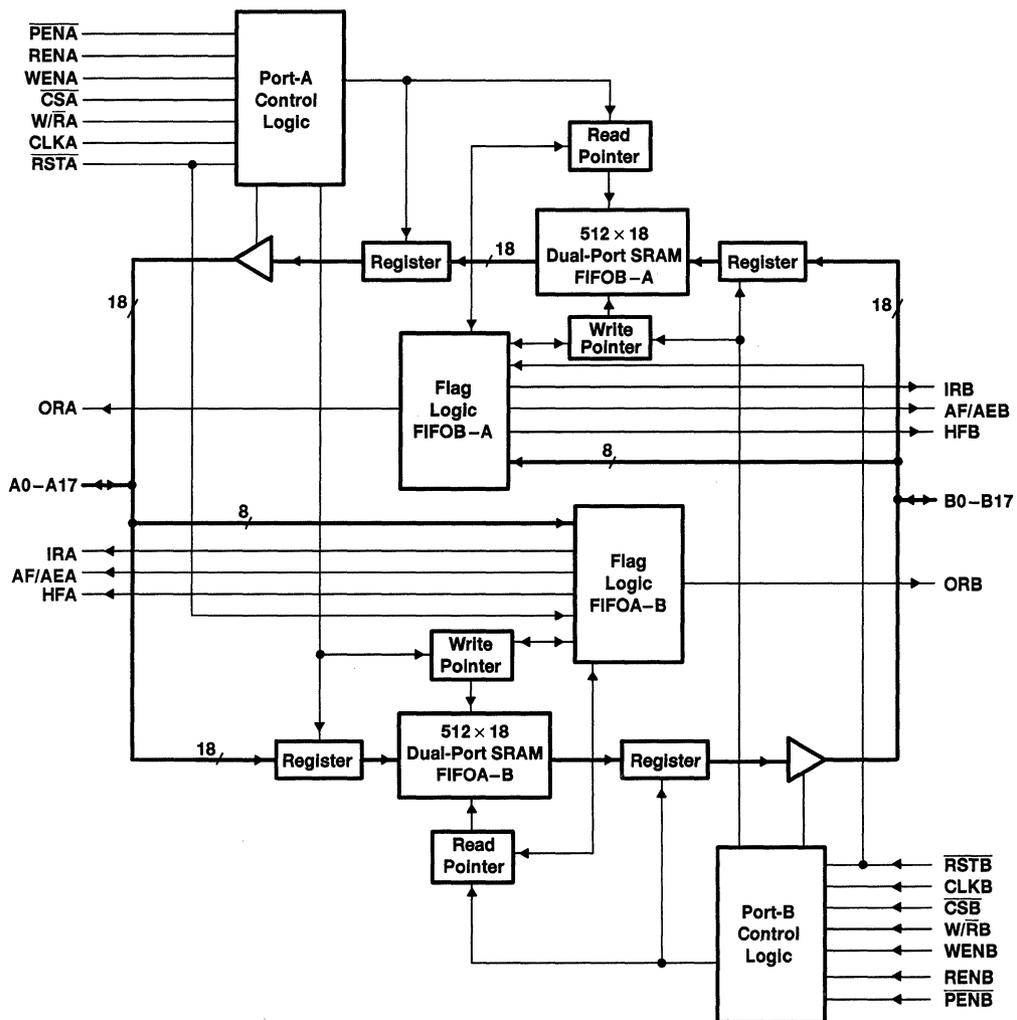
Figure 1. SN74ABT7819 Block Diagram
