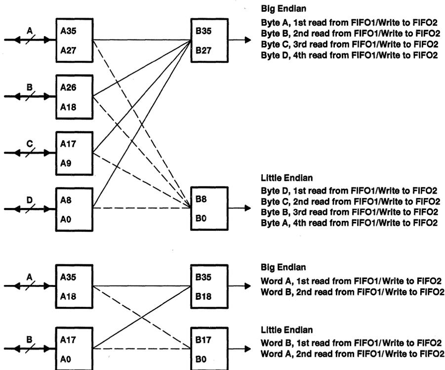
**Figure 4. Port-B Bus-Matching Configurations**
