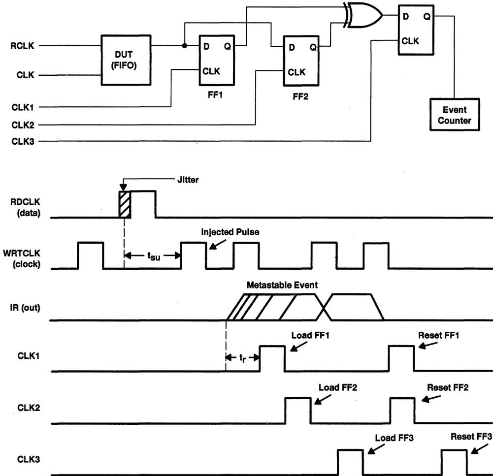
Figure 4. Metastable Event Counter and Input Waveforms
