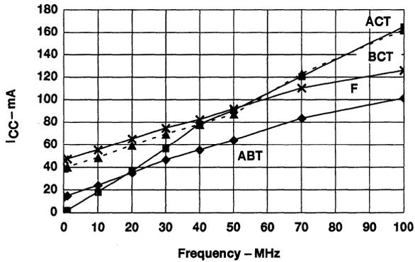
Figure 3.  $I_{CC}$  Versus Frequency (All Outputs Switching)
