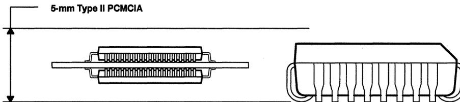
Figure 5. TQFP Package Height
