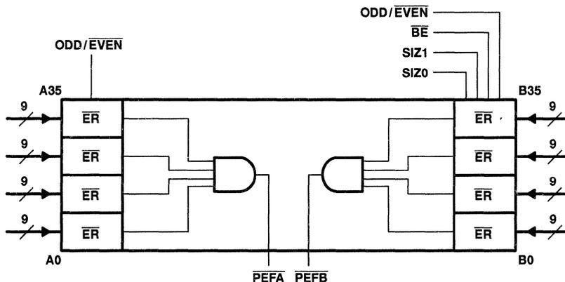
Figure 13. Parity-Checking Block Diagram
