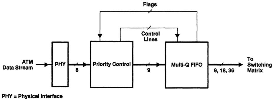
Figure 15. ATM-Exchange Receiving Unit
