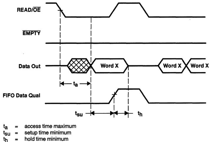
Figure 1. FIFO Read Control With READ/OE Logic
