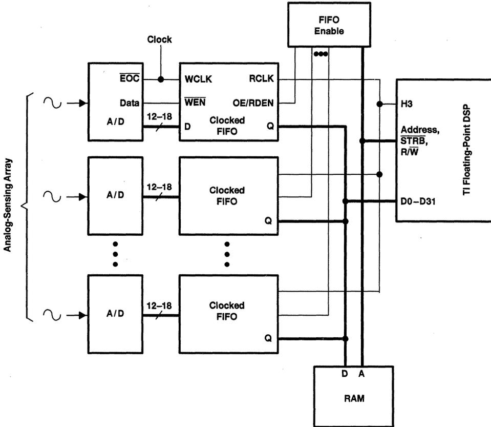
**Figure 1. Clocked FIFOs Used for High-Speed Data Acquisition**
