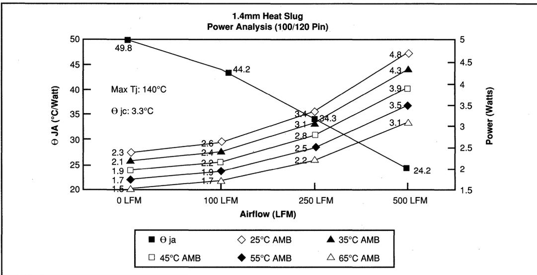
**Figure 8. Power Dissipation at Scheduled Ambient Temperatures.**
