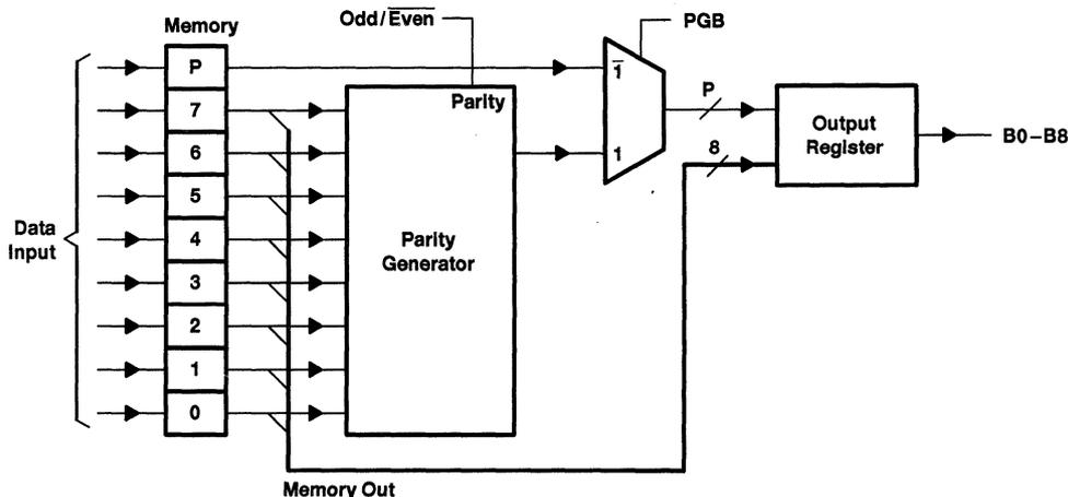
Figure 1. Parity-Generate Circuit
