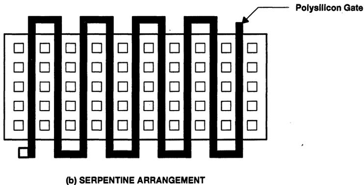
Figure 5. CMOS-Transistor-Gate Layout
