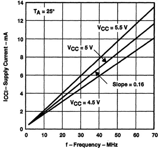
Figure 5. SN74ACT3641 Idle Current With CLKB Switching
