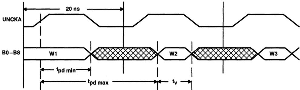
For SN74ACT2235-20:  $t_{pd \text{ min}} = 12 \text{ ns}$ ,  $t_{pd \text{ max}} = 25 \text{ ns}$ ,  $t_v = 7 \text{ ns}$
