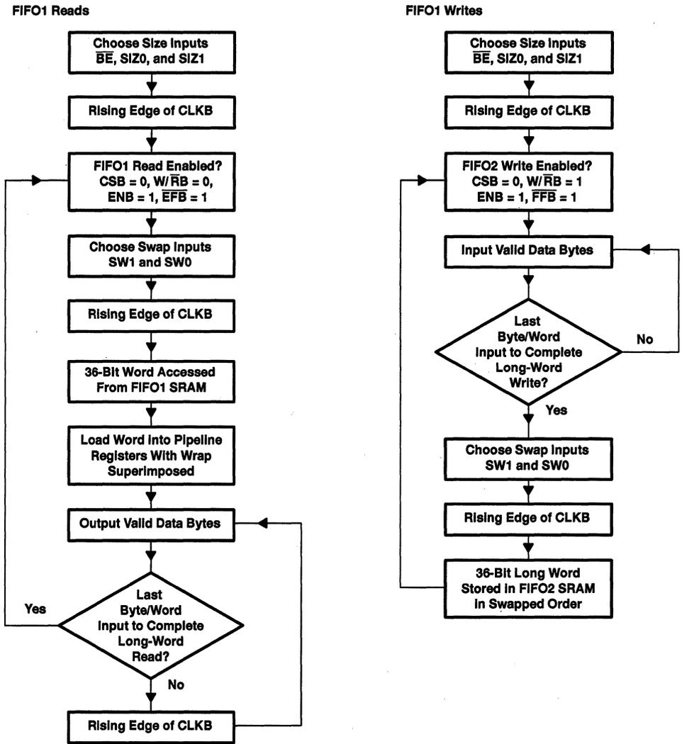
Figure 12. FIFO1 Data-Read and FIFO2 Data-Write Sequence During Simultaneous Bus-Sizing and Byte-Swapping Operations
