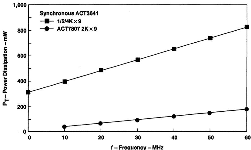
Figure 9. Multiple 9-Bit Solution Versus Single 36-Bit FIFO
