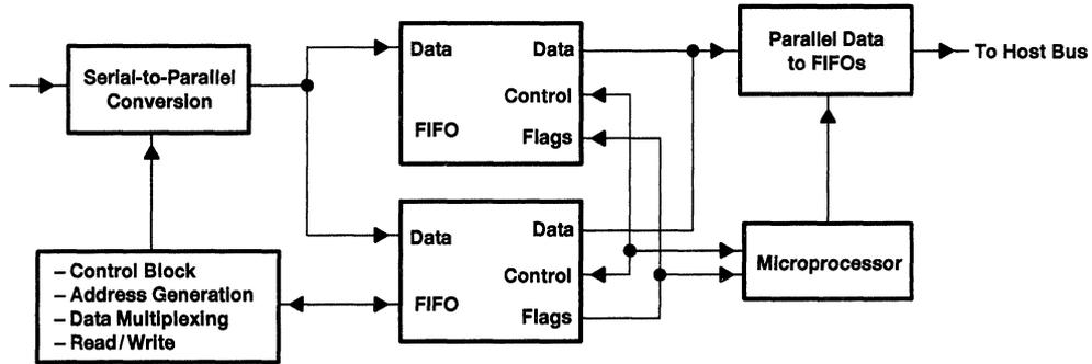
Figure 16. Implementation of a Bridge Using FIFOs
