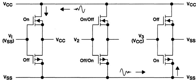
Figure 1. Power/Ground Noise Coupling Through a dc-on Driver to External Circuitry<sup>1</sup>
