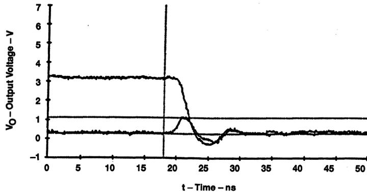
$V_1 = 250 \text{ mV}$ ,  $V_2 = 1.12 \text{ V}$ ,  $V_D = 875 \text{ mV}$
