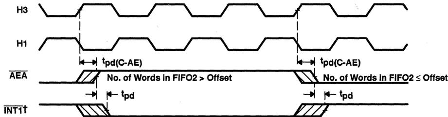
† Low level on  $\overline{INT1}$  indicates an available FIFO2 packet space.
