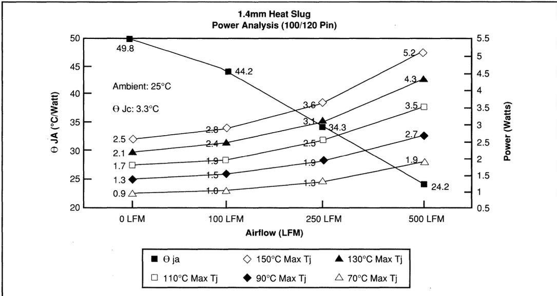
Figure 9. Power Dissipation at Selected Maximum Junction Temperatures.
