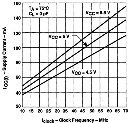
Figure 2. SN74ABT7820 Supply Current Versus Clock Frequency
