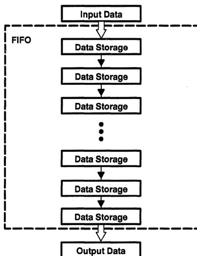
Figure 1. First-In, First-Out Data Flow
