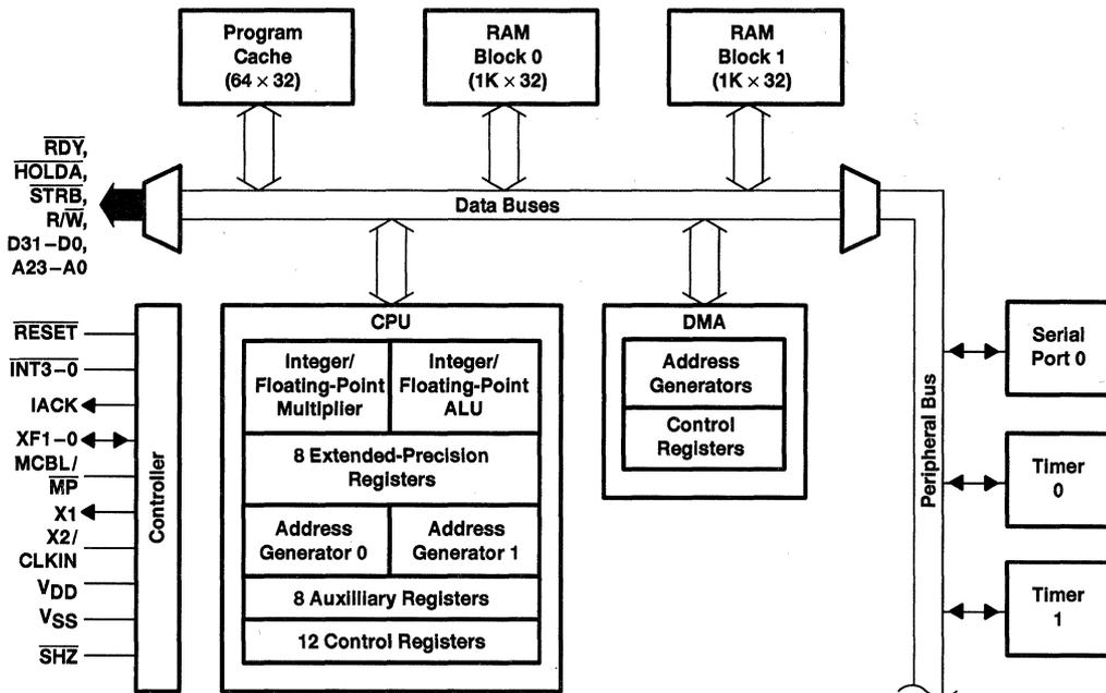
Figure 4. TMS320C31 DSP Block Diagram
