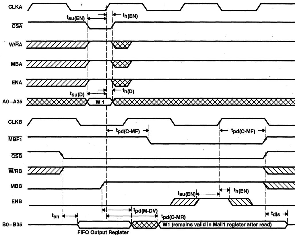
Figure 2. Timing Diagram for Mail1 Register and  $\overline{MBF1}$  Status Flag
