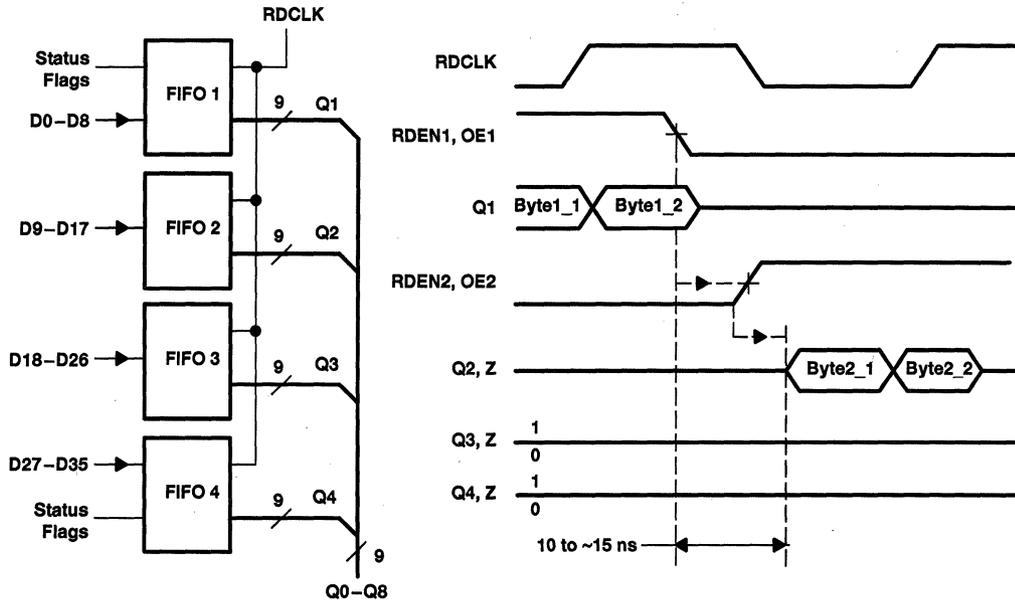
Figure 2. Data-Read Cycle for 36-Bit to 9-Bit Bus Matching
