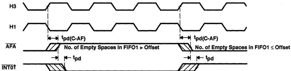
† Low level on  $\overline{INT0}$  indicates an available FIFO1 packet space.
