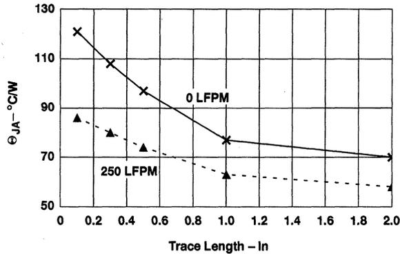
**Figure 6. 48-Pin SSOP  $\Theta_{JA}$  Versus Trace Length**
