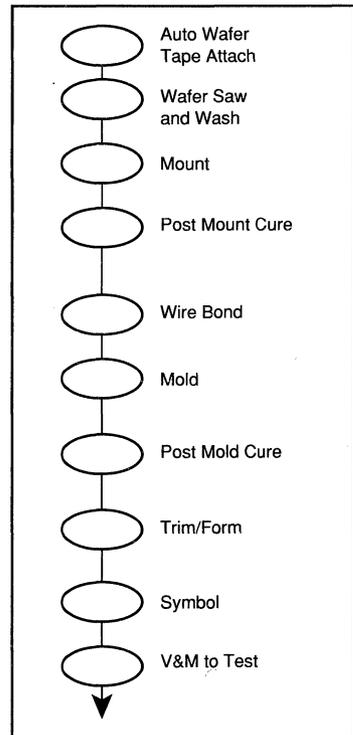
Figure 7. Assembly Process Flow.
