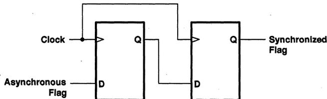
**Figure 2. Two-Stage Synchronizer**
