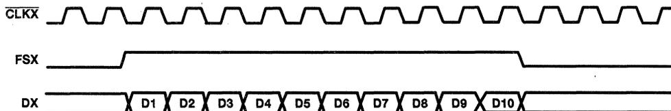
Figure 18. Serial-Port Data-Transmission Protocol With Inverted Signals
