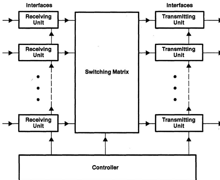
Figure 2. ATM Telecommunications Exchange System Block Diagram
