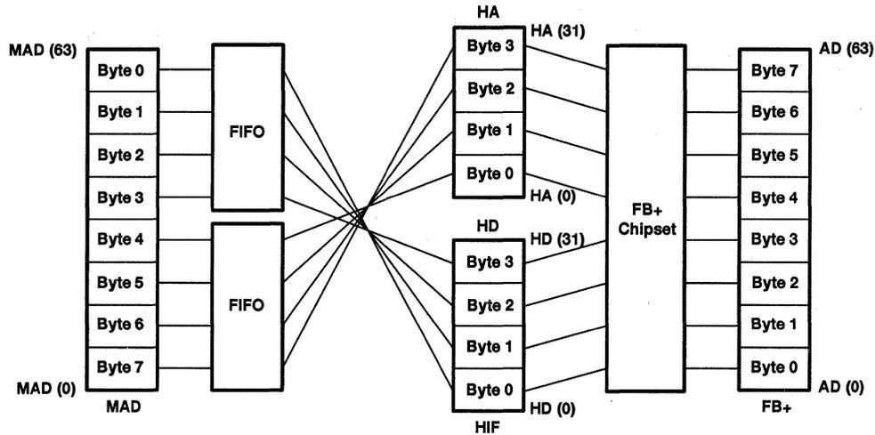
Figure 4. Byte-Lane Mapping for a 64-Bit-Only System
