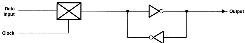
Figure 1. A Simple CMOS Latch
