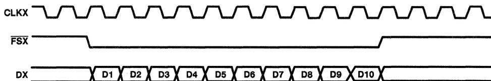
Figure 17. Serial-Port Data-Transmission Protocol of a TMS320CXX
