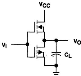
Figure 1. Gate Model of a CMOS Inverter
