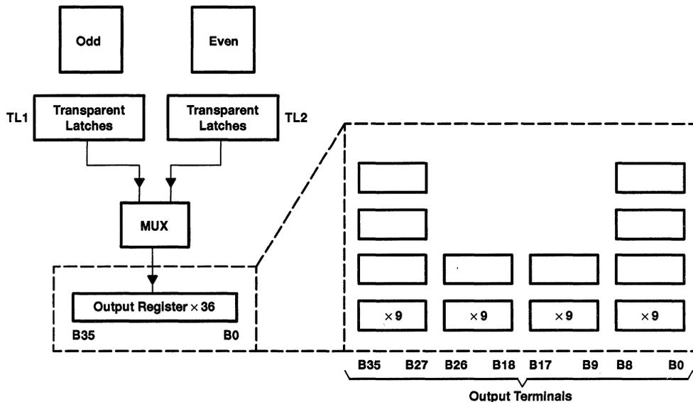
**Figure 5. Pipeline Registers**
