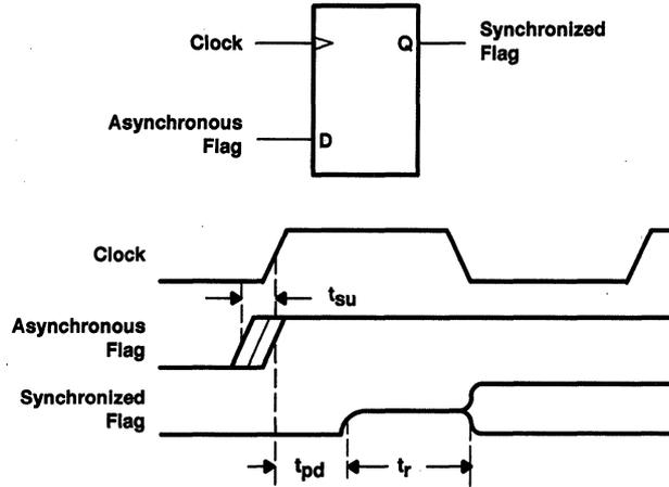
Figure 2. Single-Stage Synchronizer
