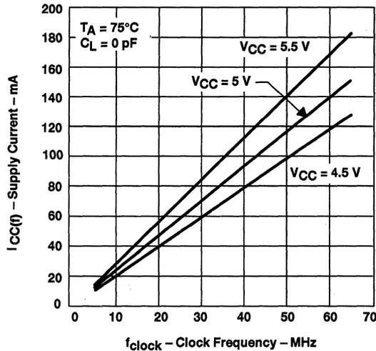
Figure 1. SN74ACT7804 Supply Current Versus Clock Frequency
