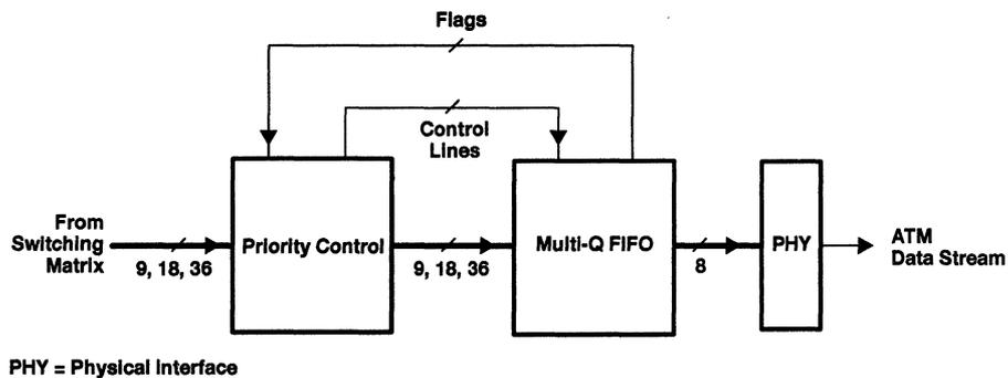
Figure 16. ATM-Exchange Transmitting Unit
