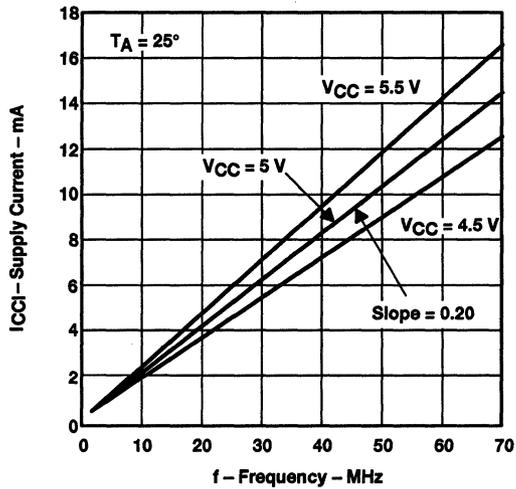
Figure 4. SN74ACT3641 Idle Current With CLKA Switching
