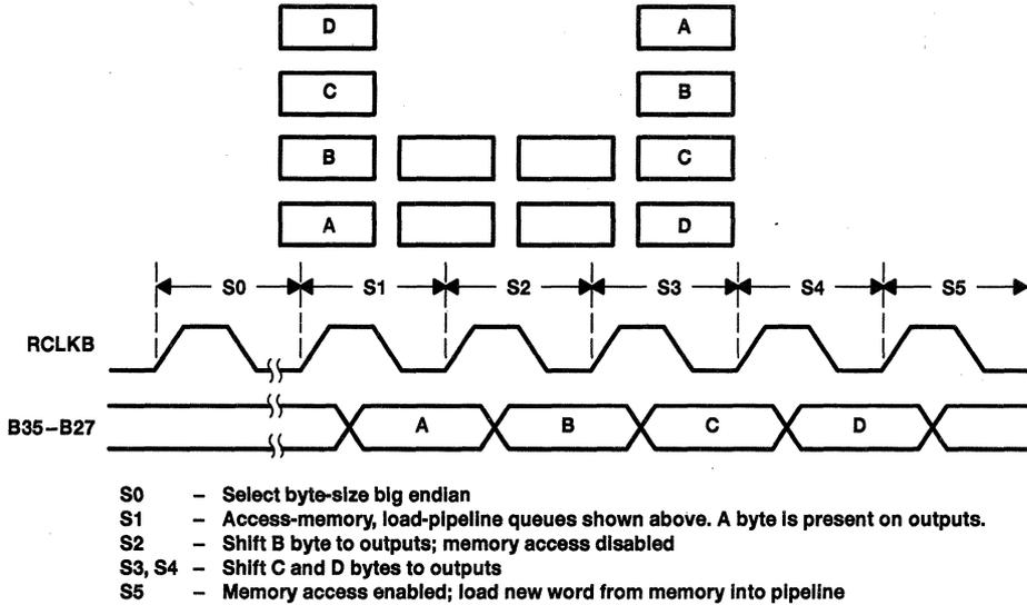
**Figure 6. Read Access During Byte-Size, Big-Endian Configuration**
