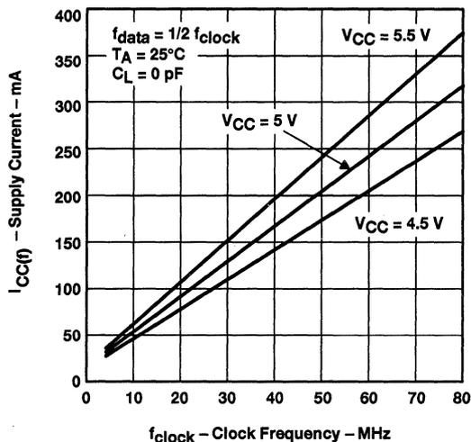
Figure 3. SN74ABT3613 Supply Current Versus Clock Frequency
