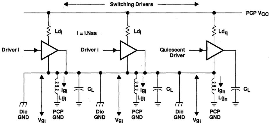
Figure 2. Simultaneous Switching<sup>2</sup>
