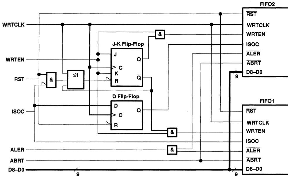
**Figure 13. Extension of Word With 9-Bit Input Data**
