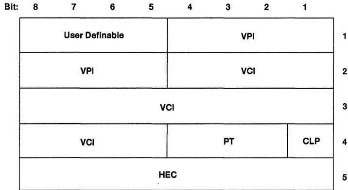
**Figure 3. ATM-Header Structure**
