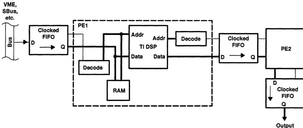
**Figure 2. Clocked FIFOs Used in Pipelined Image-Processing Systems**
