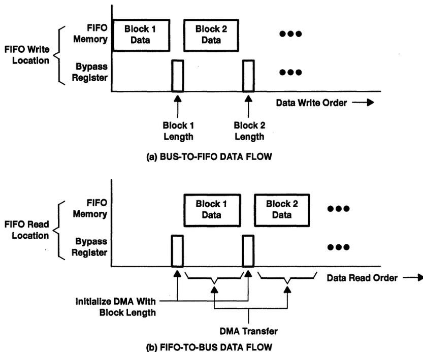
Figure 6. Using Mailbox-Bypass Registers to Initialize DMA Control
