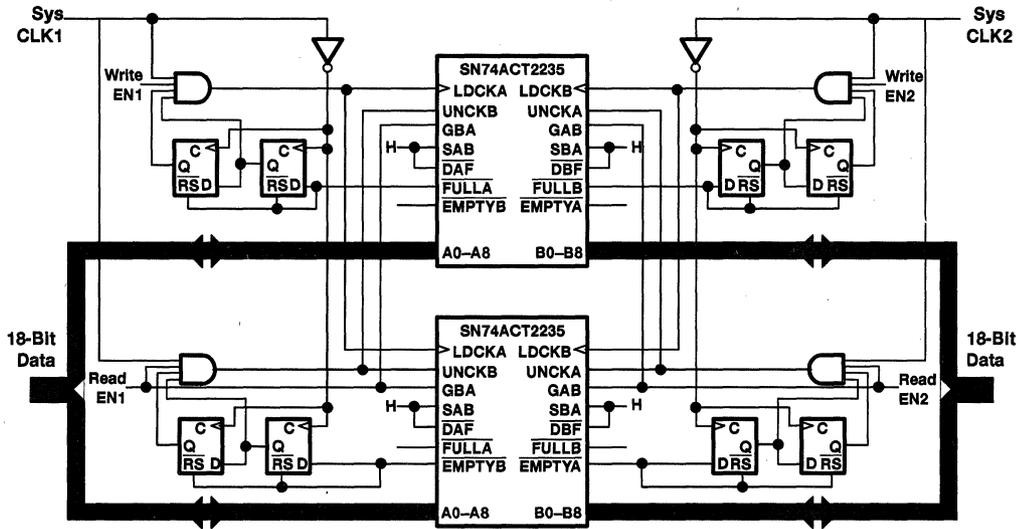
NOTE: Two devices are used for 18-bit width expansion.
