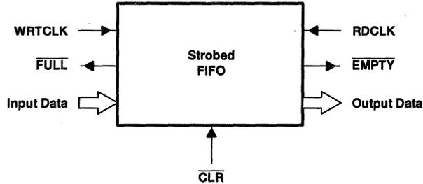
Figure 2. Connections of a Strobed FIFO
