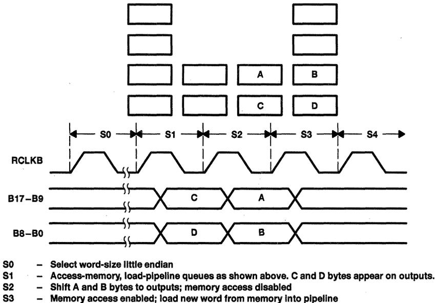
**Figure 7. Read Access During Word-Size, Little-Endian Configuration**
