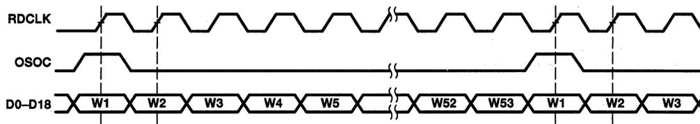
Figure 9. Reading Cells Out of the FIFO
