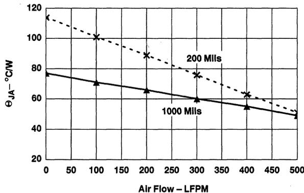
**Figure 7. 48-Pin SSOP  $\Theta_{JA}$  Versus Air Flow**
