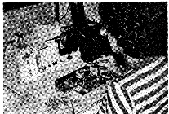
Figure 2B. Hand Mount Station \approx 100 units/hour
