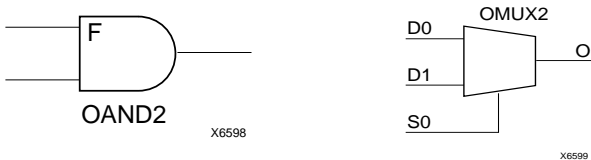
Figure 7: AND & MUX Symbols in Spartan-XL IOB
