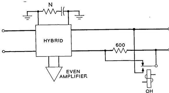
Fig. 9 — 1A echo suppressor modified for greater suppression.
