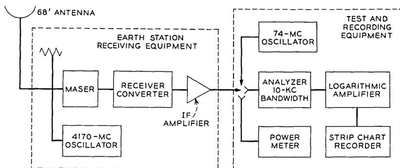
Fig. 4 — Test setup.
