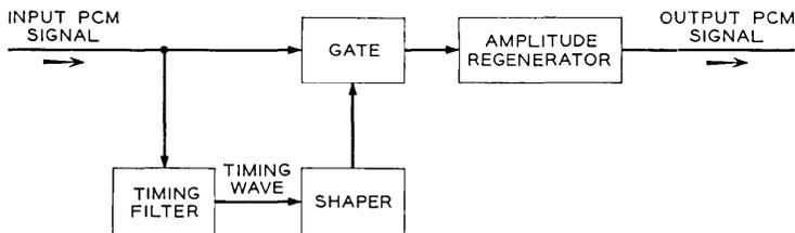
Fig. 1 — Block diagram of a self-timed forward acting regenerator.
