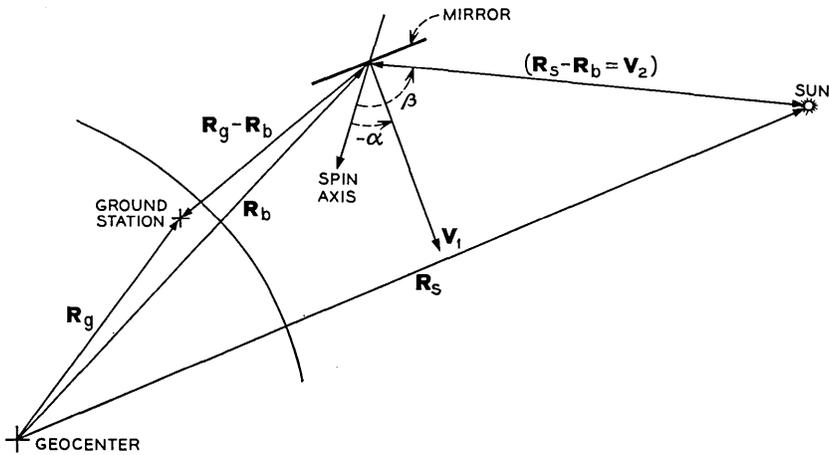
Fig. 3 — Reference frame for calculations from mirror flashes.
