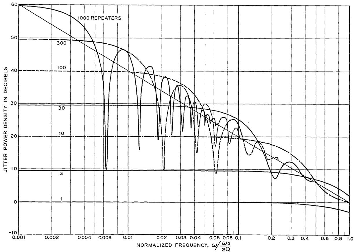
Fig. 3 — Jitter spectrum due to a random pattern (computed from the model).
