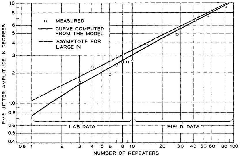
Fig. 14 — Root-mean-square jitter due to a random pattern (10-----) versus the number of repeaters in the chain, measured and calculated.
