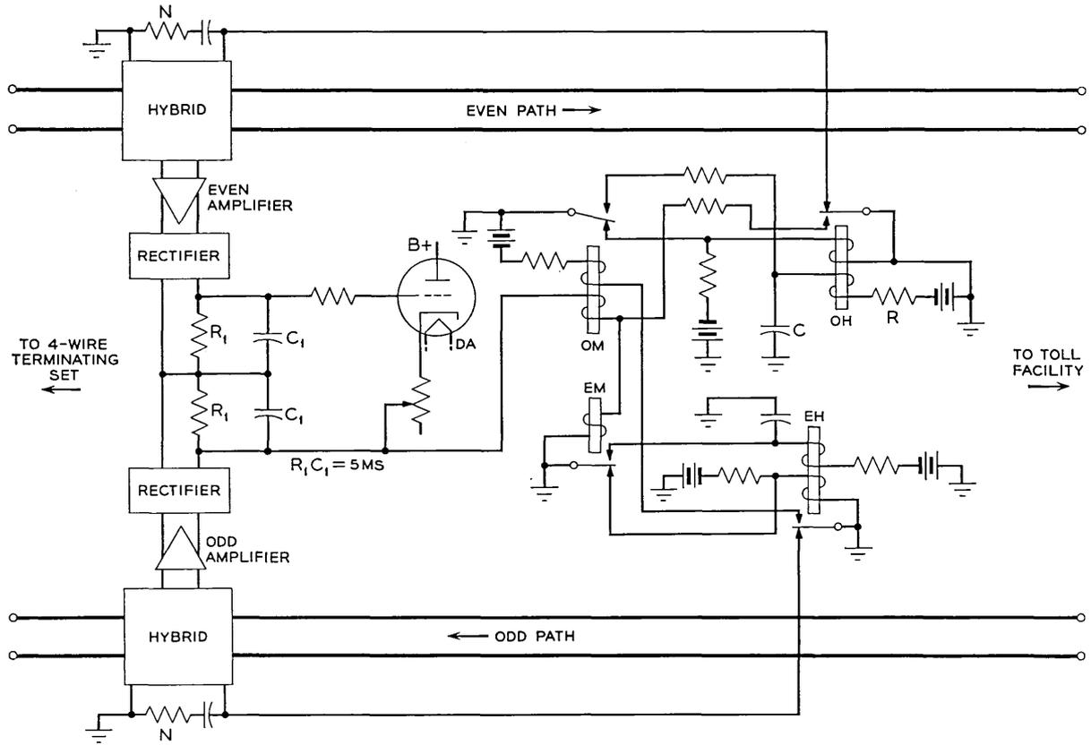
Fig. 8 — Simplified schematic of 1A echo suppressor.
