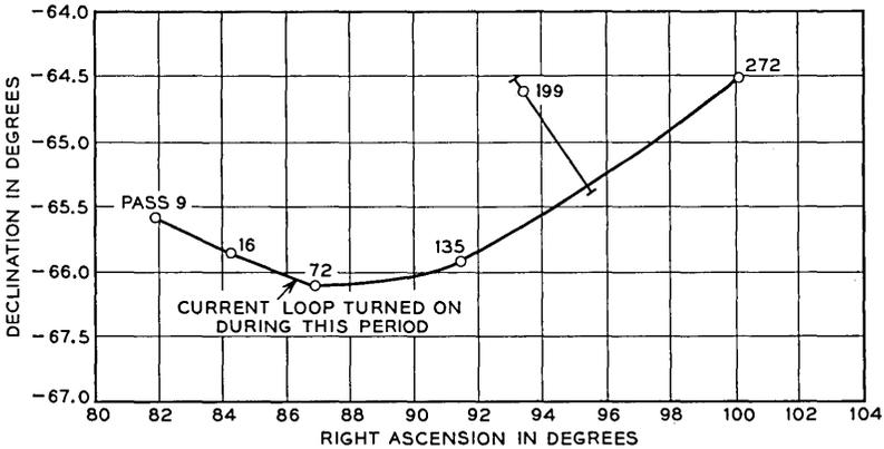
Fig. 5 — Motion of spin axis in geocentric coordinates.
