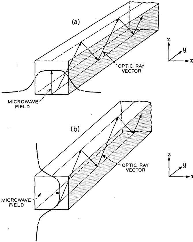
Fig. 2 — Relative orientation of modulating electric field and optical plane of incidence in the two zigzag modulator configurations: (a) 0° modulator; (b) 90° modulator.
