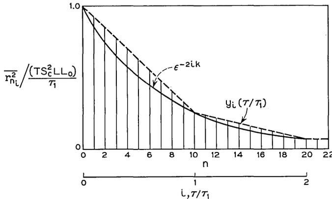
Fig. 3 — For periodically placed mode filters of  $k$  nepers differential attenuation each, the envelope of the equivalent echoes consists of a straight-line approximation  $y_i(\tau/\tau_1)$  to the exponential  $\epsilon^{-2ik}$ .
