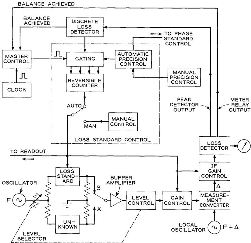
Fig. 8 — Simplified block diagram — loss measuring circuit.
