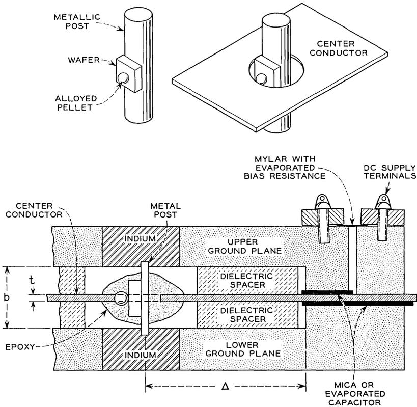
Fig. 1 — Tunnel diode mounted in balanced strip transmission line.
