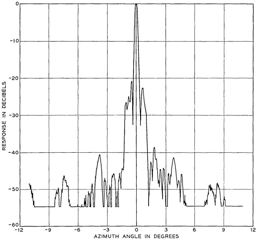
Fig. 7 — Antenna directivity in horizontal plane.
