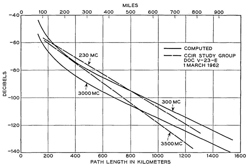
Fig. 3 — Transhorizon transmission loss for widebeam antenna.
