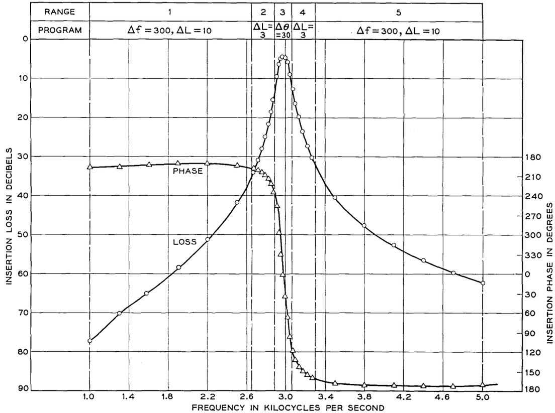
Fig. 14 — Automatic data selection — bandpass filter.
