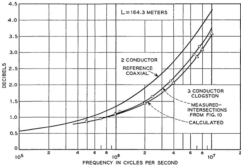
Fig. 14 — Attenuation of three-conductor Clogston transmission line compared with a two-conductor line of like dimensions.
