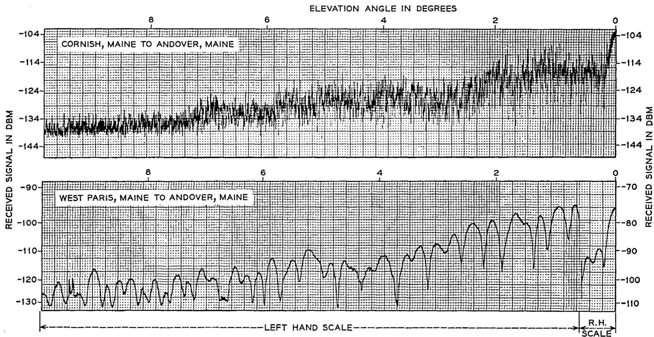
Fig. 18 — Elevation scans (elevation angles are in degrees above that for maximum signal in each case; azimuth angles are fixed at value giving maximum signal at reference elevation in each case; elevation scan rate is  $0.043^\circ$  per second).
