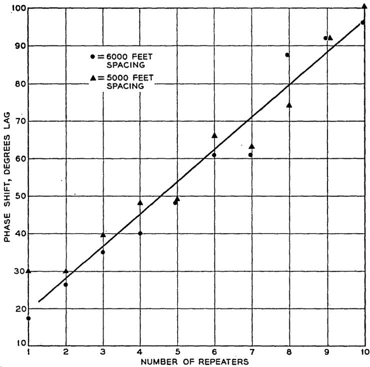
Fig. 10 — Measurement of the effect of repeater spacing.
