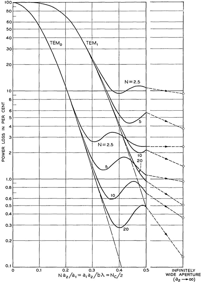
Fig. 2 — Power loss per transit for the two lowest-order modes of an aperture-limited concentric interferometer. The abscissa is the half width of the aperture normalized to  $a_1/N$ . (Both  $a_1$  and  $N$  should be regarded as constants.) The dashed curves are for the “comparable” confocal interferometer.
