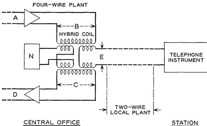
Fig. 4 — Occurrence of echo in two-wire local plant.
