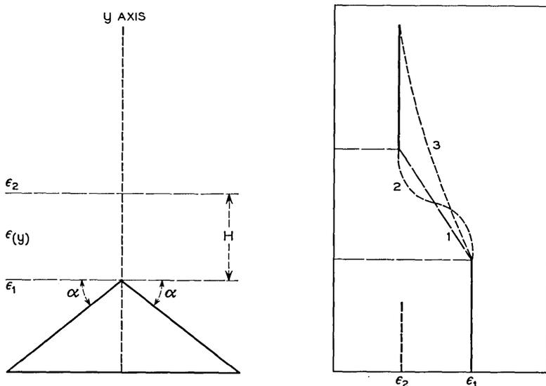
Fig. 5 — Idealized geometry for reflection from stratified media.
