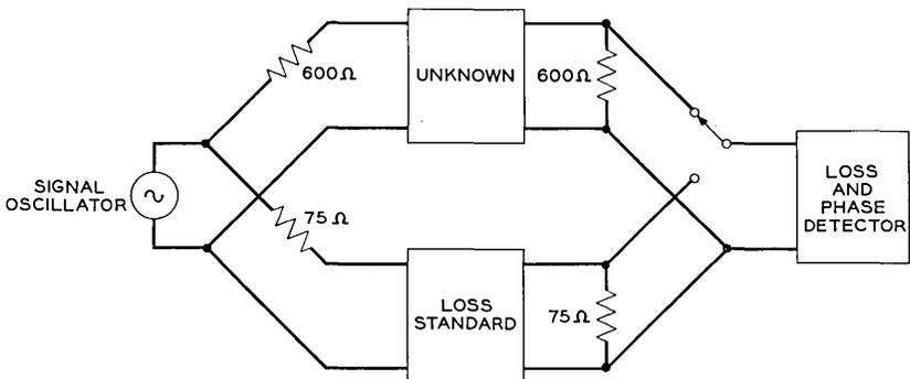
Fig. 11 — Comparison circuit.
