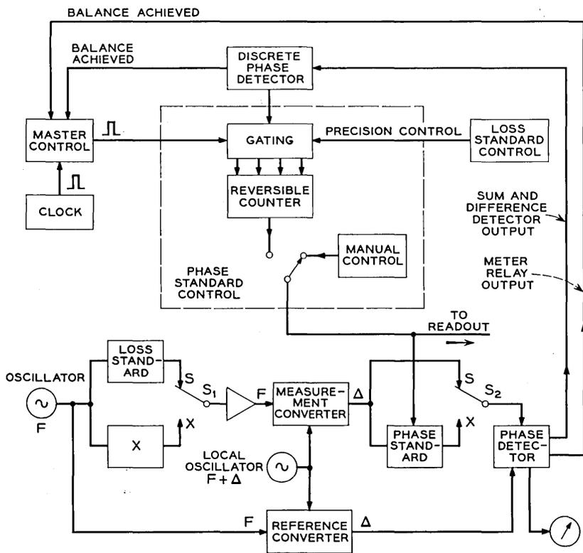
Fig. 9 — Simplified block diagram — phase measuring circuit.
