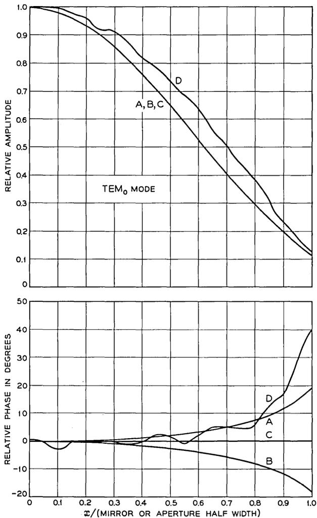
Fig. 3 — Relative amplitude and phase distributions of the lowest-order ( $\text{TEM}_0$ ) mode. Both A and B are for an aperture-limited concentric interferometer with  $N = 10$  and  $a_2/a_1 = 0.0325$ ; A is the field distribution over the mirror and B is the field distribution over the aperture. C is for the “comparable” confocal interferometer with a Fresnel number of 0.65. D is for a concentric interferometer with  $N = 10$  and  $a_2 \rightarrow \infty$ .
