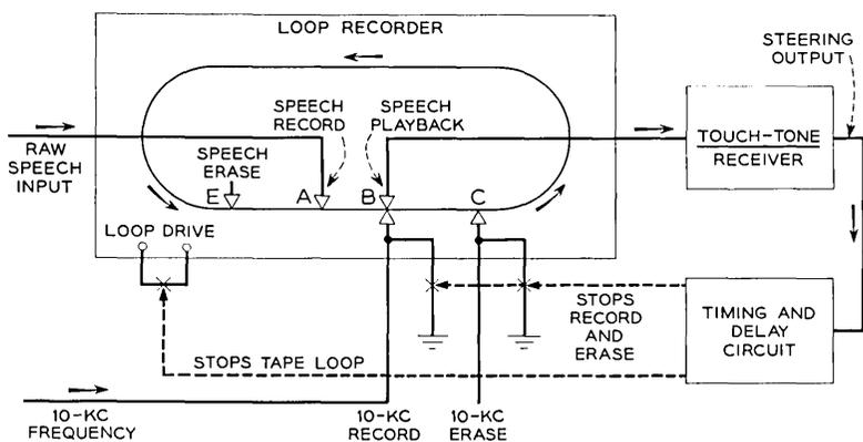
Fig. 1 — Apparatus for recording digit-simulating speech segments.
