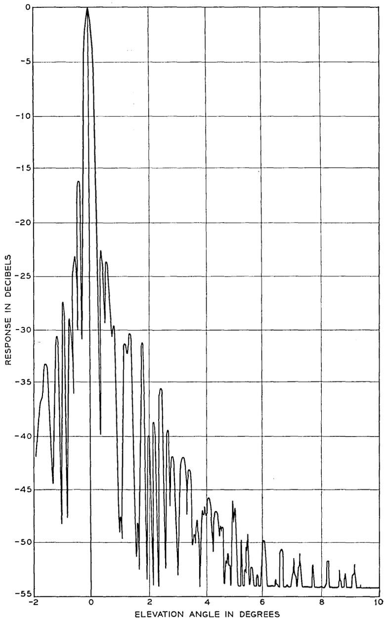
Fig. 6 — Antenna directivity in vertical plane.
