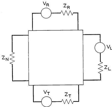
Fig. B1 — General prototype of hybrid terminations.
