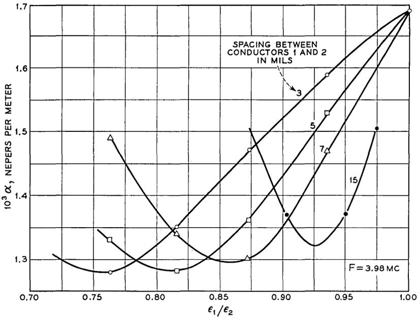
Fig. 4 — Calculated attenuation of three-conductor Clogston line.
