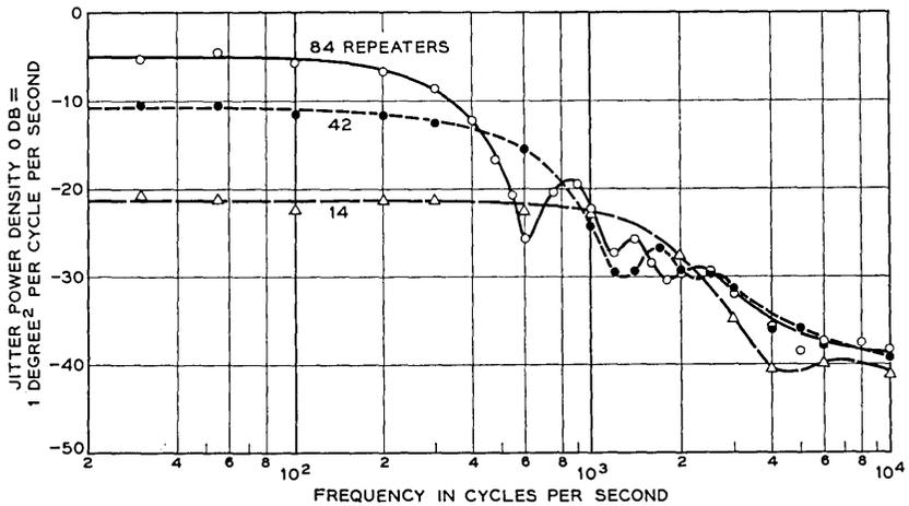
Fig. 11 — Measured spectral distributions for a random pattern (10-----).
