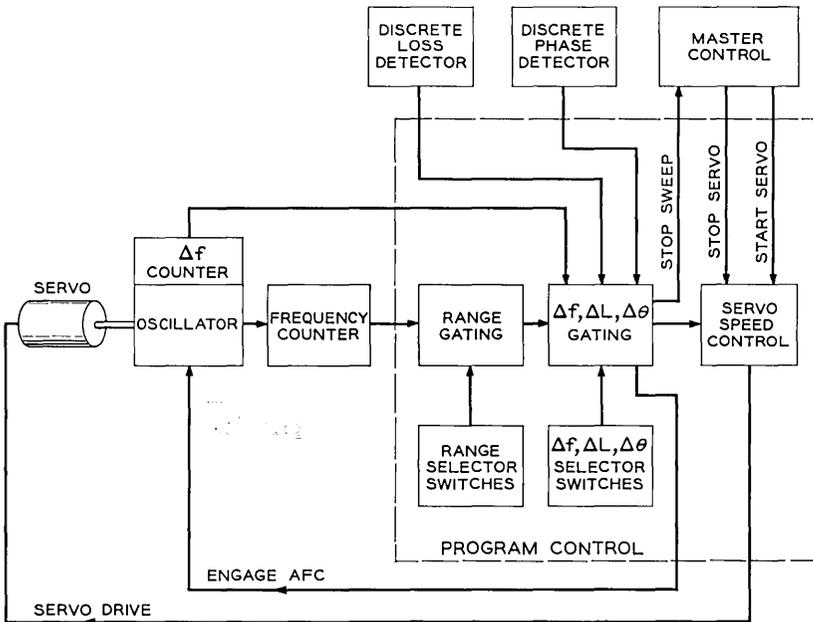
Fig. 10 — Simplified block diagram — programming circuits.
