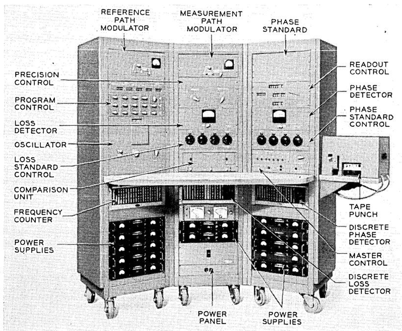
Fig. 5 — Console arrangement of transmission measuring set.
