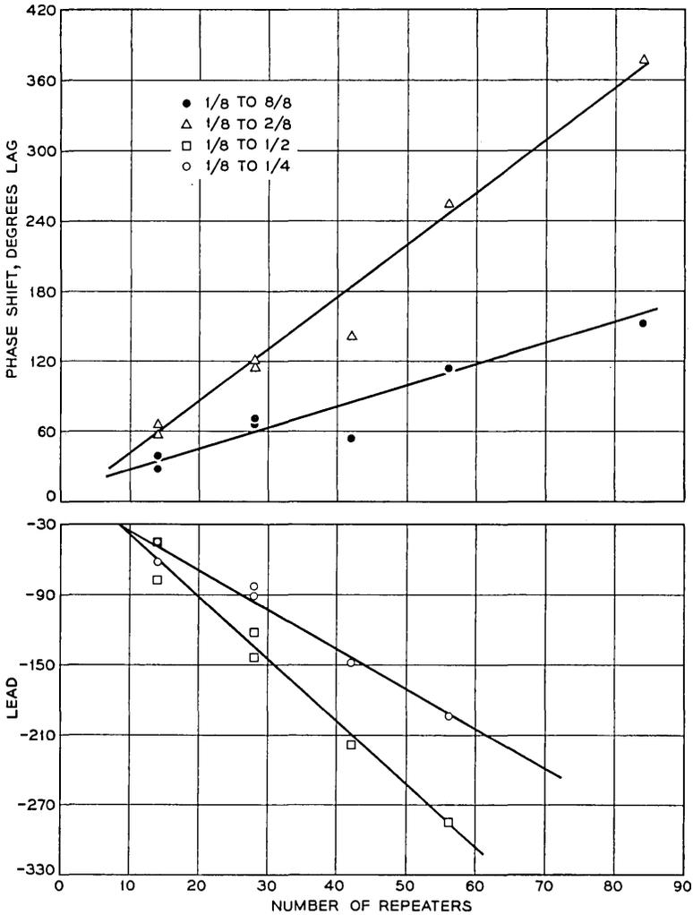
Fig. 8 — Steady-state phase shift between fixed patterns.
