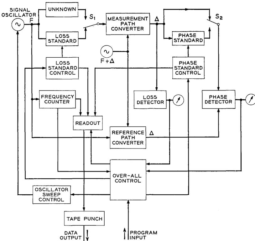
Fig. 4 — Simplified block diagram — measuring and control circuits.
