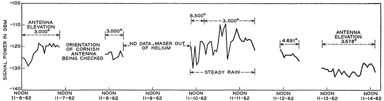
Fig. 19 — Hourly median received signal at Andover from Cornish (elevation angles are referred to that for maximum received signal, i.e., 2.433° above the horizontal).
