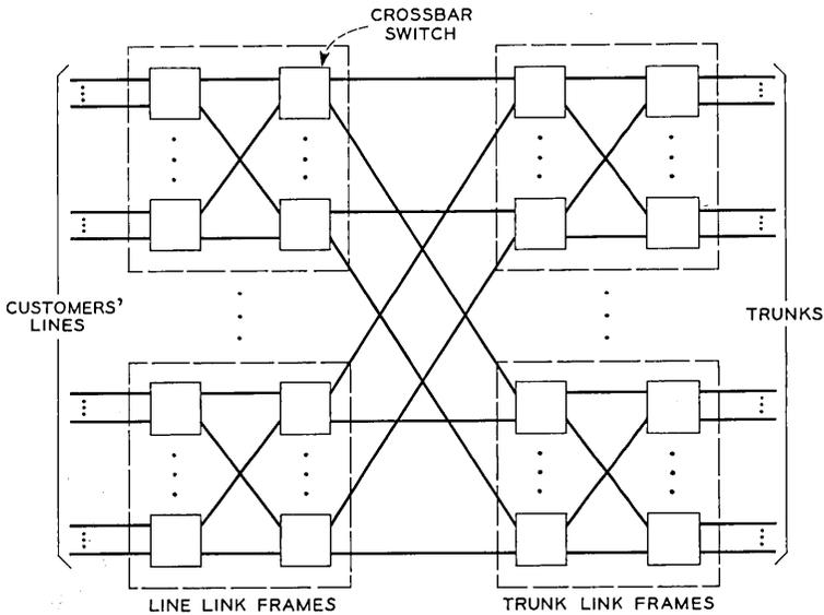
Fig. 1 — Structure of No. 5 Crossbar network.
