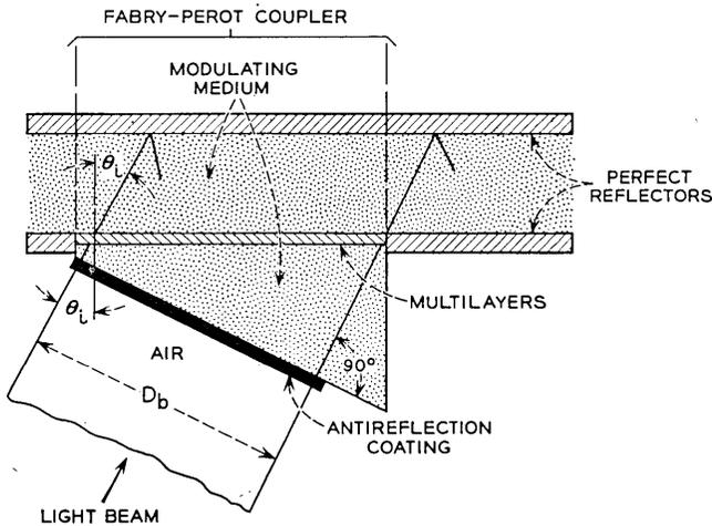
Fig. 11 — Modified coupling arrangement used when  $n_0^2/\sqrt{\kappa'} > 1$ .
