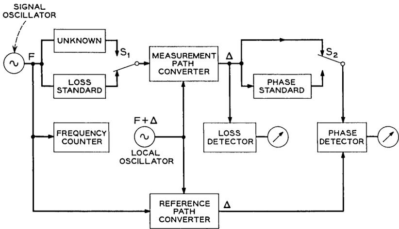
Fig. 3 — Simplified block diagram — measuring circuit.
