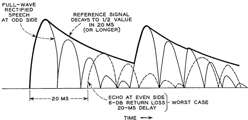
Fig. 5 — Typical waveforms appearing in rectified speech break-in detector.
