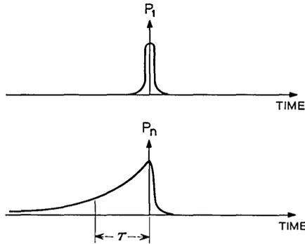
FIG. 2 — Signal impulse ( $P_1$ ) and reconversion echo wave ( $P_n$ ) versus time after transmission through a multimode line with mode conversion.
