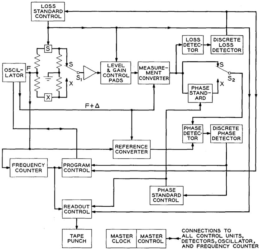
Fig. 6 — Simplified block diagram — measuring and control circuits.
