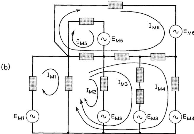
Fig. 3 — Node and mesh currents and voltages: (a) node analysis; (b) mesh analysis.
