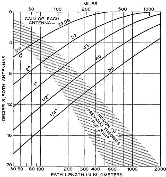
Fig. 4 — Loss in effective antenna gain.
