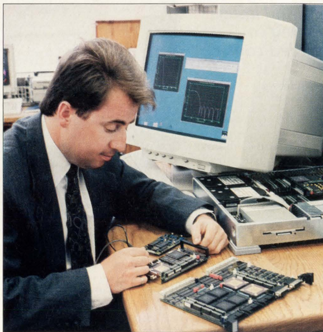
Spectrum Signal Processing's Ross Mitchell looks at one of the company's latest signal processing boards. The company pioneered VME DSP boards, but it now offers a broad selection of boards in a variety of formats, including SBUS.
