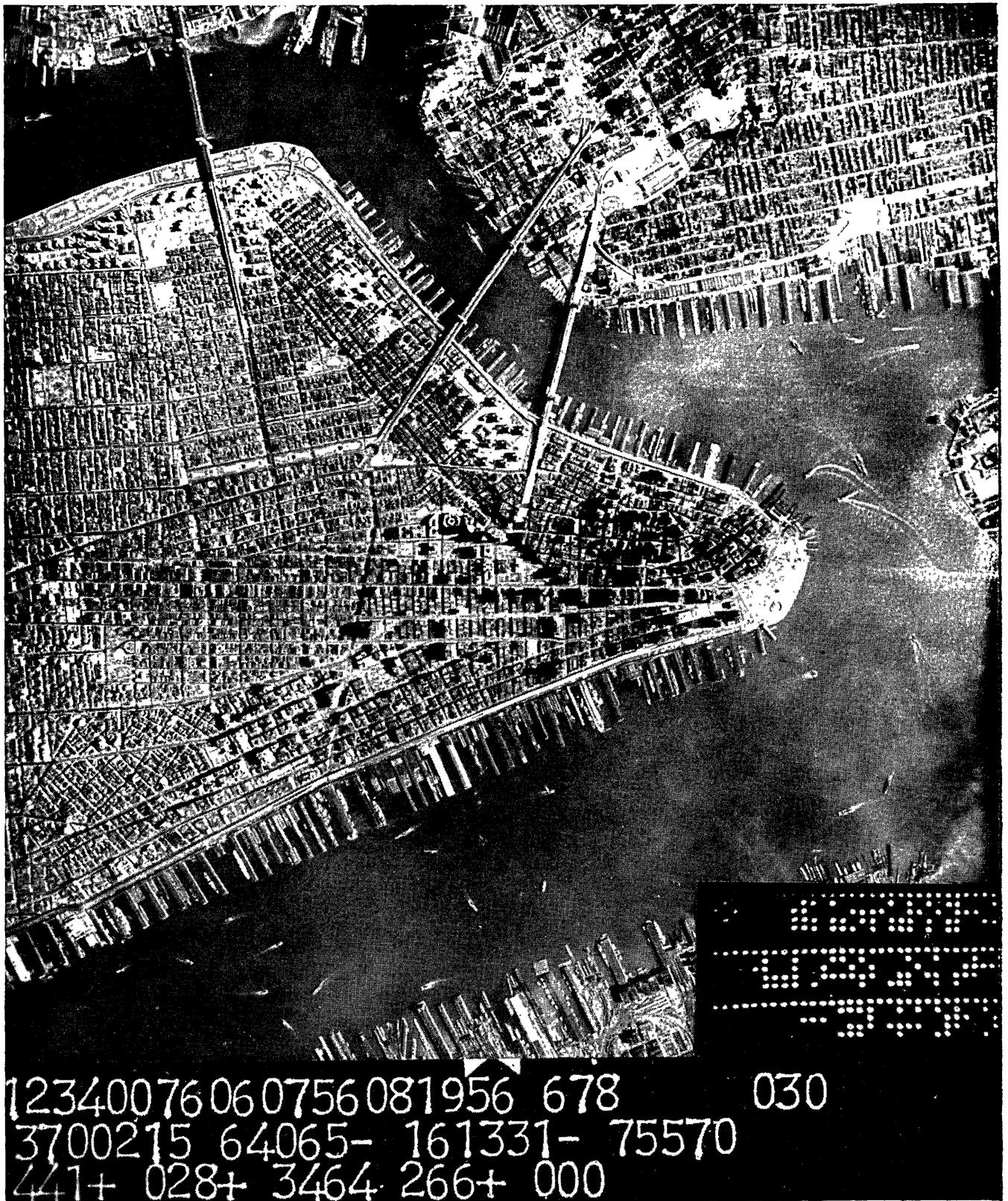
Position, altitude and other pertinent data necessary to U.S. Air Force reconnaissance may be recorded automatically on photographs with a device produced by International Telephone and Telegraph Laboratories, Nutley, N.J., research division of International Telephone and Telegraph Corp. The device, known as the Digital Data Recording Device, records all information in coded-dot form (lower-right) directly on the photograph. During development of the film, a ground-based reader decodes and prints the data beneath the picture (bottom). Commercial applications envisaged for various portions of the Recording Device range from library cataloguing to industrial automation. (Note: This photograph of lower Manhattan has no relation to the coded information shown, which is simply illustrative.)
