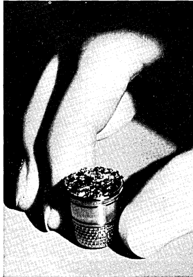
— Integrated circuits for three computers fit into a thimble.
