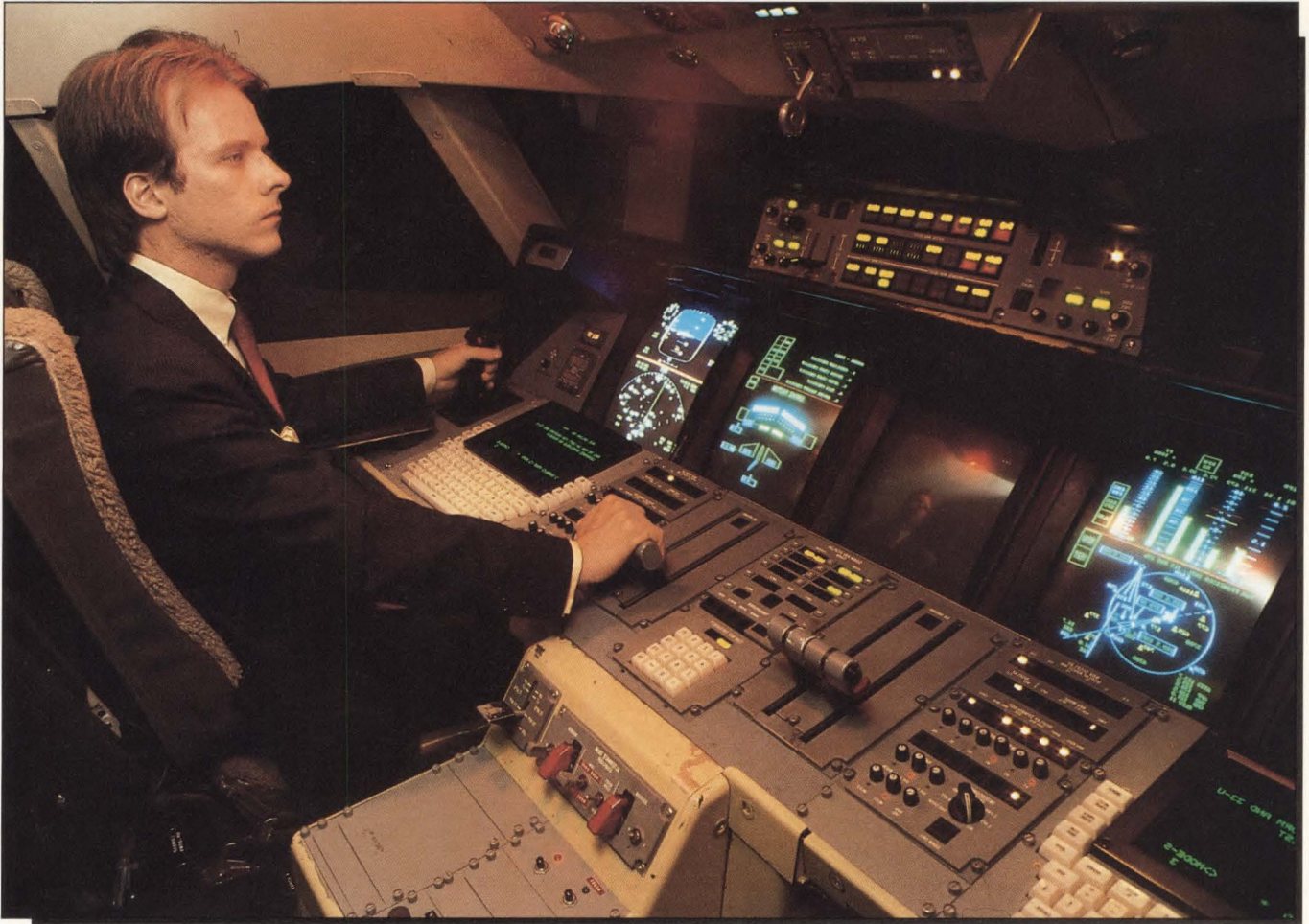
The Advanced Concepts night flying cockpit simulation. The red illumination helps pilots maintain their night vision.
