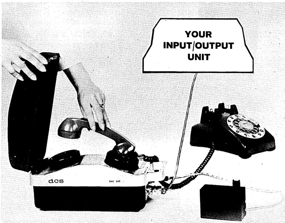
The DAC 347, originate-answer model, or the DAC 337, originate model, couplers readily connect any conventional telephone line to your input and/or output terminal device.
