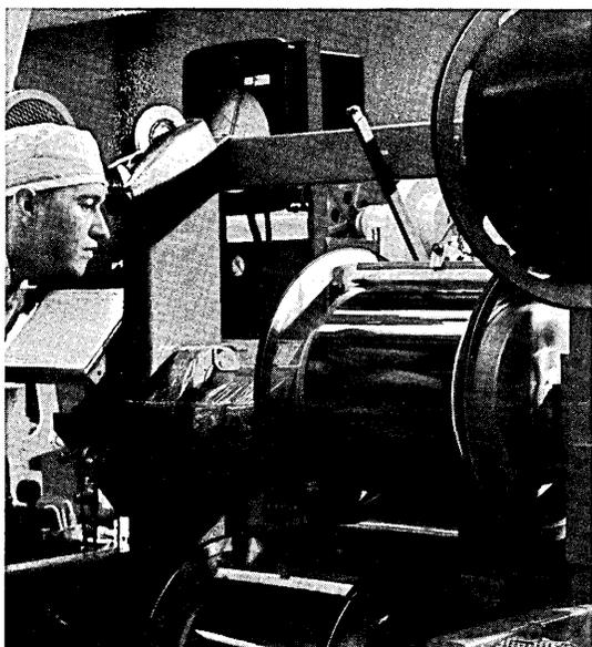
Ampex CATT computer tape is subjected to precisely controlled heat and pressure—ultra finished—to give it a non-abrasive, super-smooth surface.
