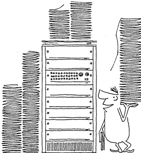
And that means more of it faster, and with less cost, work and worry. Raytheon Computer's \$15,000 703 has system characteristics built-in... 1.75 usec cycle time... 16-bit word... memory expandable to 32K... byte and word manipulation... real-time priority interrupt... options like direct memory access, multiply/divide, expandable I/O bus.
