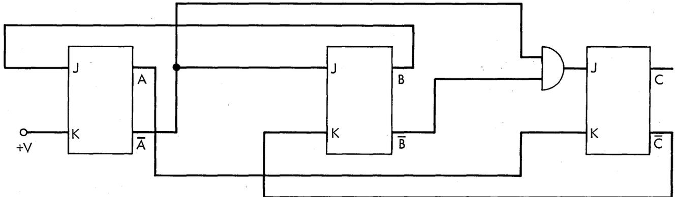
Fig. 14 (below). Logical schematic as in Fig. 13, but providing clock inputs.
