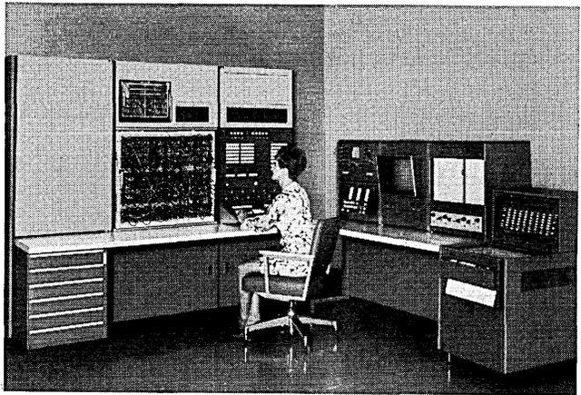
by adding plug-in modules. The console also has centralized master control and monitoring, central overload-indicator panel and automatic program hold. Computing components include a five-digit digital voltmeter, two-input electronic comparators, digitally controlled attenuators, gp registers and gp logic gates (AND, NAND, OR and NOR).
