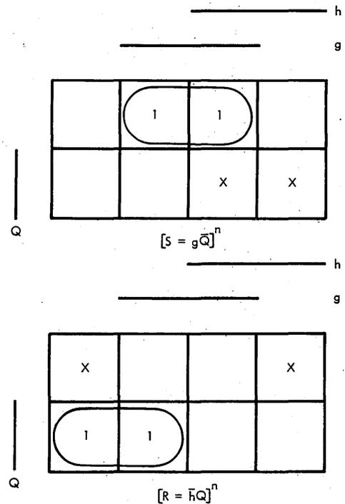
Fig. 6 Minimaps for the R-S flip-flop characteristic application equations.
