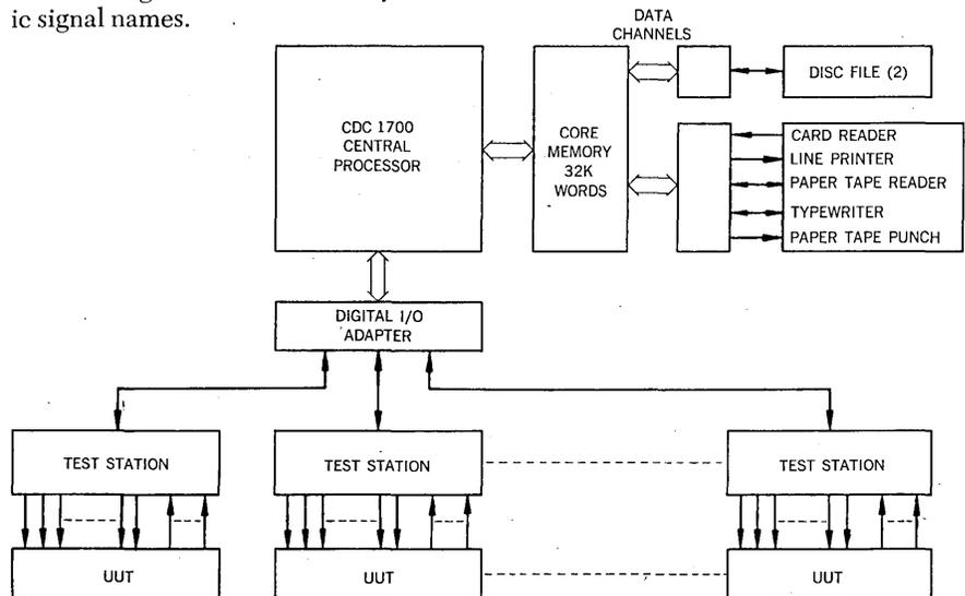
Production test system block diagram (above).
