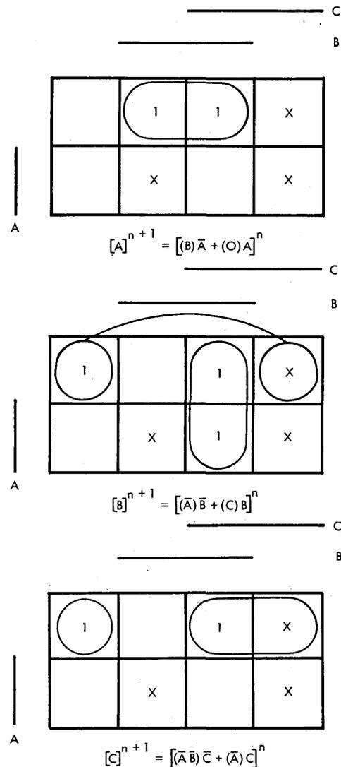
Fig. 11 Minimaps for the application of flip-flops A, B and C.
