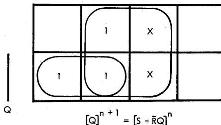
Fig. 2 Minimap for the R-S flip-flop characteristic equation.
