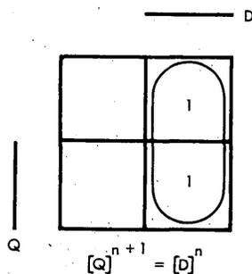
Fig. 5 Minimap for the D flip-flop characteristic equation.
