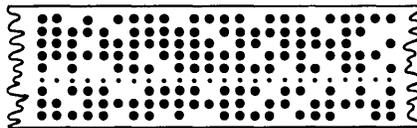
You can store ten characters on an inch of punched tape. You can store up to 800 characters on an inch of magnetic tape. That's 80 times more data per inch!
