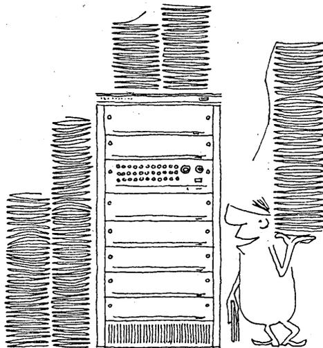
And that means more of it faster, and with less cost, work and worry. Raytheon Computer's \$15,000 703 has system characteristics built-in... 1.75 usec cycle time... 16-bit word... memory expandable to 32K...byte and word manipulation... real-time priority interrupt... options like direct memory access, multiply/divide, expandable I/O bus.
