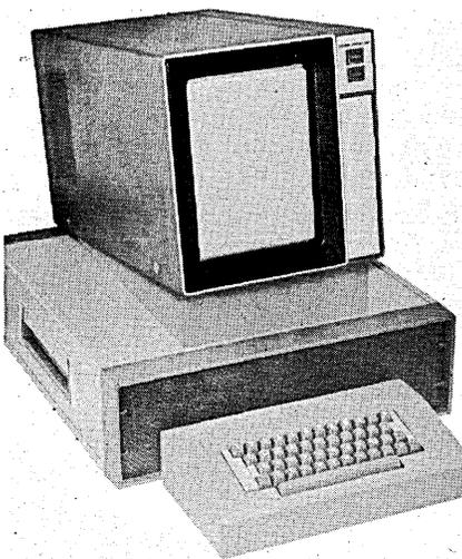
stand-alone display terminals which feature a curve generator for graphics that enables curves to be drawn directly rather than approximated by straight-line segments. The 400 mod 20, first in the series, includes a storage
