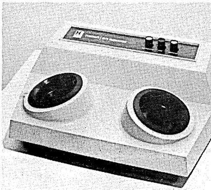
with EIA interface. The unit also has a magnetic receiver which eliminates interference from local room noise. It will operate in either full- or half-duplex mode; transmission rates are 300 baud. For information:
