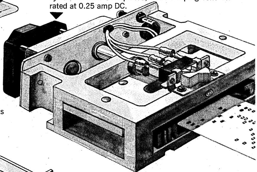
**Behind-panel reader.** Model 2981A. Industrial full 80-column card reader. Complete alphanumeric coding and 160 six-bit word capability with only 160 diodes. Can be bussed by column, by split column, or by row. Gold-plated contacts take 0.25 amp.
