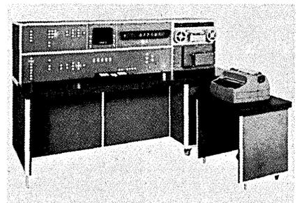
ors from one production batch to another. The system, given console inputs or measuring color directly through a special sensing instrument, selects a combination of colorants considering both cost and quality of color matches. The size of a production batch is considered too, so that production personnel receive information from the computer regarding the ac-
