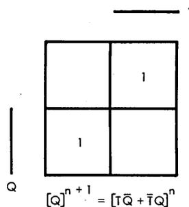
Fig. 3 Minimap for the T flip-flop characteristic equation.
