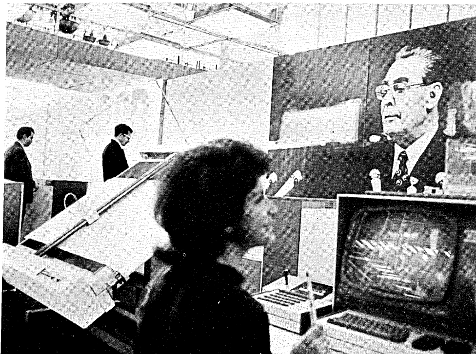
Fig. 3. A Soviet crt unit with light pen and joystick operates beneath a photograph of party secretary Leonid Brezhnev.
