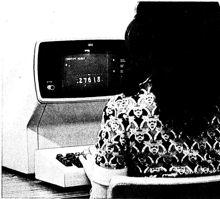
At an IBM 3277 terminal, an operator corrects a handprinted number which was previously rejected as unreadable by a 3886 optical character reader.
