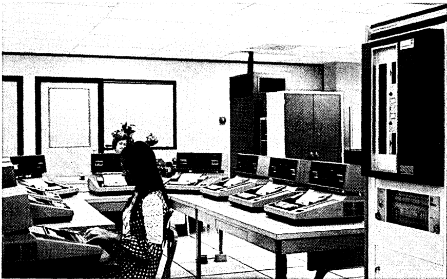
Model 700 TPS Terminal Polling System links the TI 960 Series minicomputer with "Silent 700" terminals for a complete data network.
