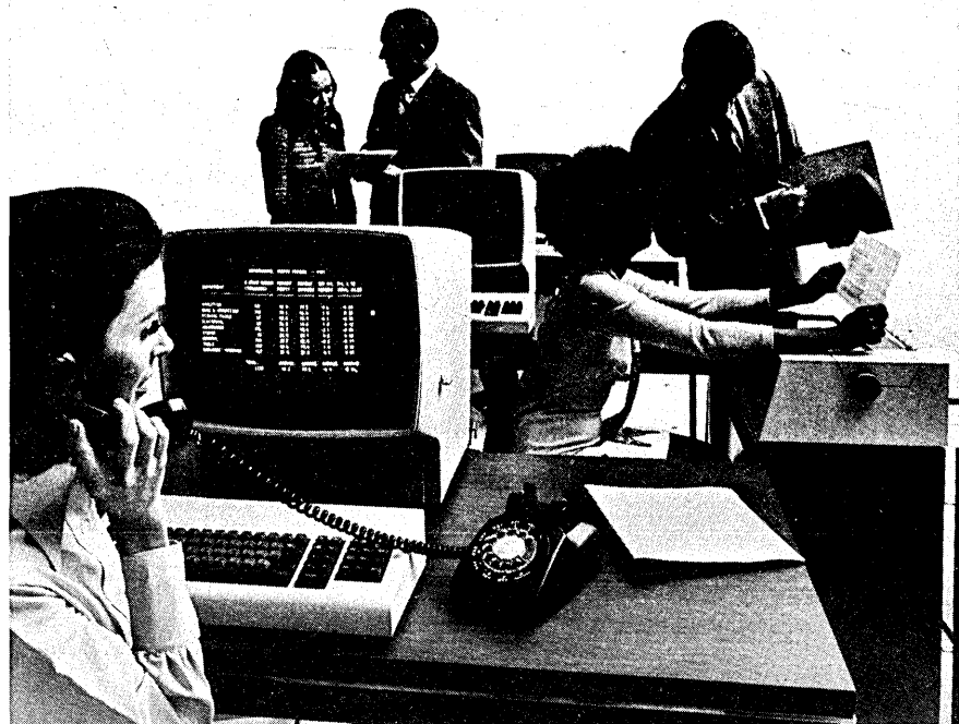
IBM is expected to tie terminals closely into networks involving IBM host processors, thus ensuring for itself a large share of the growing terminals market. A "cluster" of IBM 3270 keyboard/displays is shown.
