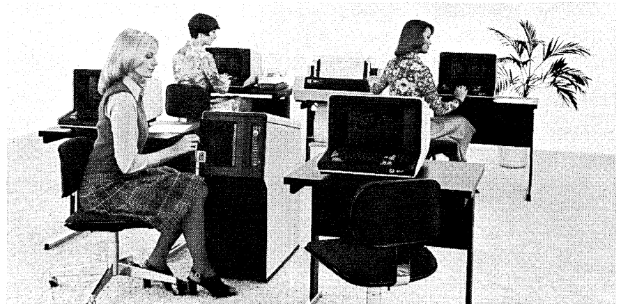
The Sycor 440 is a clustered processing system. It is available with cassette or diskette interchange, up to 20mb of storage and eight video display terminals.
