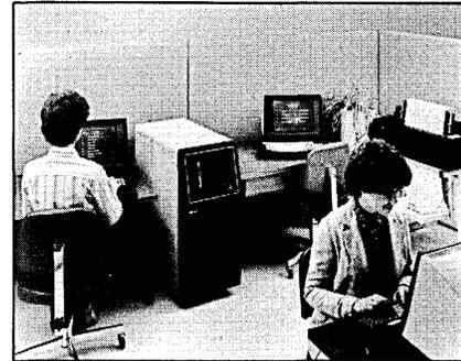
lengthy make/buy study, Northern Telecom went ahead and developed its own eight-inch Winchester disk for the 585. The disk is made in 11MB and 22MB (formatted) capacities, and includes an integral 15MB cartridge tape for backup.
