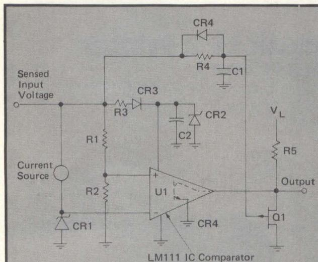
Fig 7 Precise voltage level detector, powered by the sensed potential, contains two principal circuit components, U1 and Q1. U1 is a high gain differential IC comparator, such as LM11, which has an open collector output and is able to operate over a wide range of supply voltage. Q1 is a p-channel JFET with a pinch-off threshold lower than the sensed input,  $V_I$  minus  $V_L$ , that controls the output by clamping it to ground level, until the LM111 has had time to stabilize after power ON.
