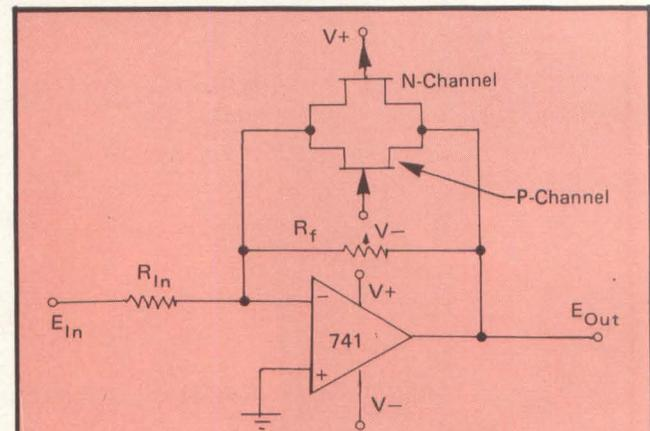
Fig 9 Two normally-ON JFETs connected in parallel across the feedback of the 741 op amp clamp the output to zero and provide a nearly zero feedback impedance. The FETs can also absorb high discharge current from charged up capacitors.
