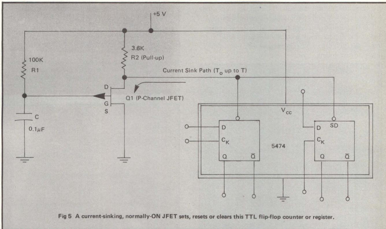
Fig 5 A current-sinking, normally-ON JFET sets, resets or clears this TTL flip-flop counter or register.
