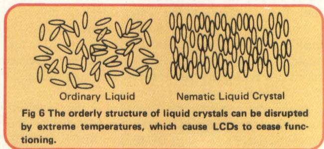
Fig 6 The orderly structure of liquid crystals can be disrupted by extreme temperatures, which cause LCDs to cease functioning.
