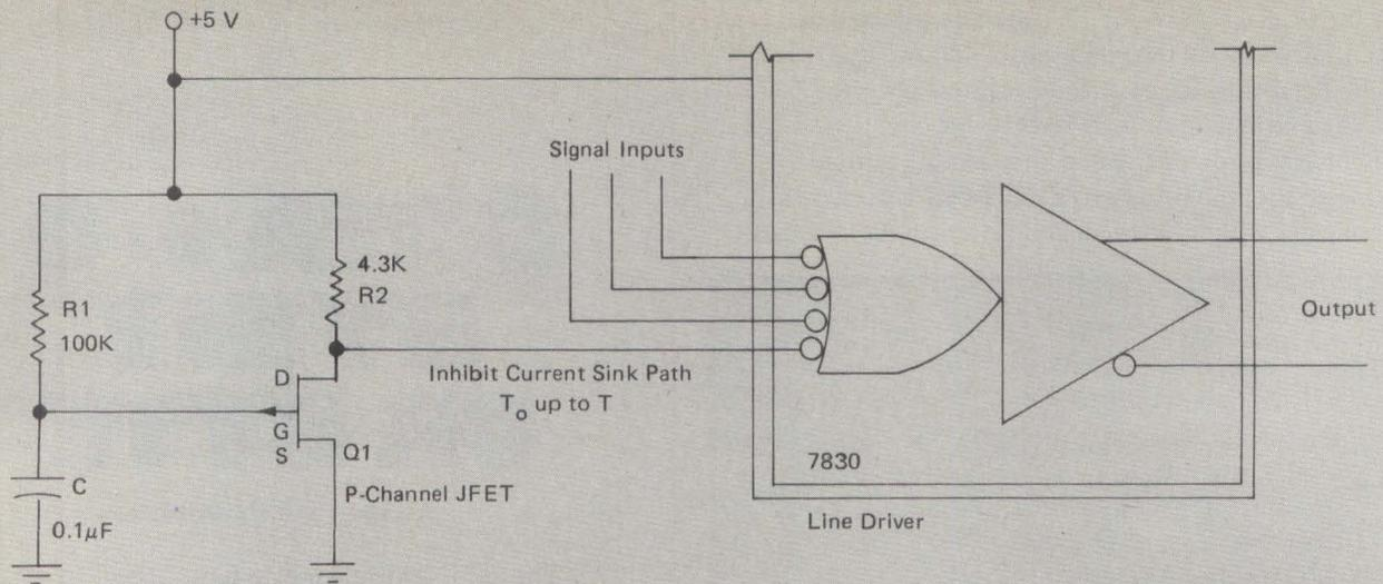
Fig 4 In this line driver inhibit circuit, R1 and C1 determine the duration of the inhibit signal and R2 serves as the pull-up when Q1 begins to cut off.
