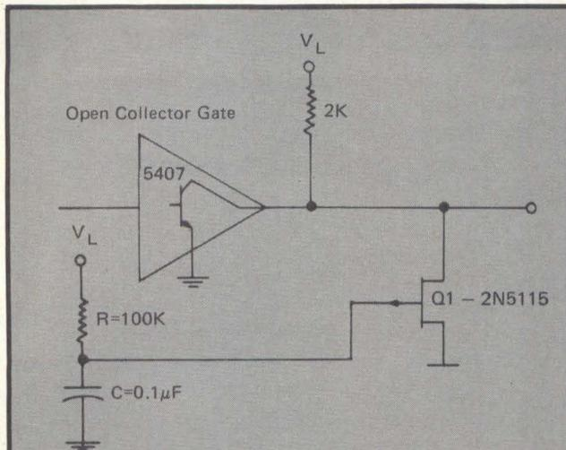
Fig 6 A normally-ON JFET, in parallel with open collector gates or drivers, guarantees a known, low-level start-up state.
