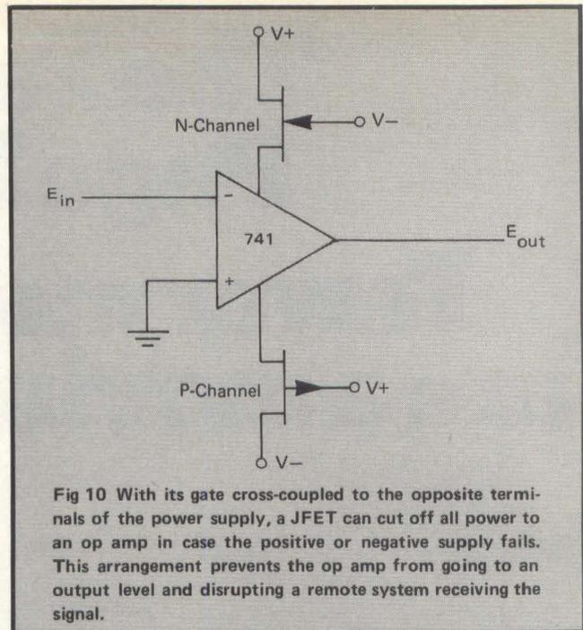
**Fig 10** With its gate cross-coupled to the opposite terminals of the power supply, a JFET can cut off all power to an op amp in case the positive or negative supply fails. This arrangement prevents the op amp from going to an output level and disrupting a remote system receiving the signal.
