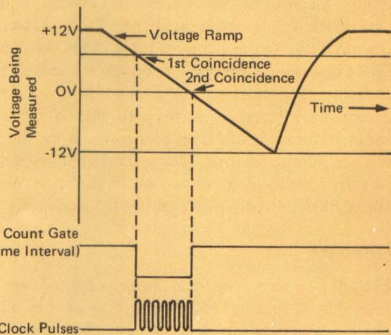
Fig 4 Ramp conversion is used in low-resolution, low-accuracy DPMs. Errors can come from the ramp voltage and the clock.
