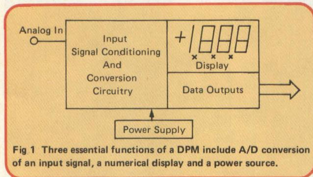
Fig 1 Three essential functions of a DPM include A/D conversion of an input signal, a numerical display and a power source.
