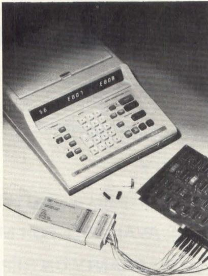
instrument requests the trigger word or address and any following delay, 0 to 65,535 clock-intervals before the data-trace, may be specified. The clip-on probe set plugs into a standard edge connector on the probe. The HP-IB option makes the 1602A totally key-programmable and able to dump its 64-word memory onto the bus on command for analysis by the computing controller. Price is \$1800. Hewlett Packard, 1501 Page Mill Rd., Palo Alto, CA 94304. (415) 493-1501. **Circle 164**
