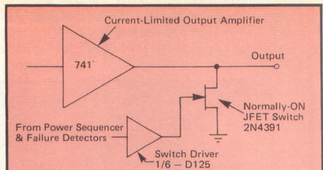
Fig 8 Although this typical basic amplifier output clamp uses a 741 current-limited output amplifier, one-sixth of a D125 switch driver and a 2N4391 JFET as a switch, the designer can configure his own circuit with other components.
