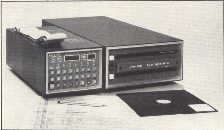
**MuPro-80 Microprocessor Development System:** This system supports real time emulation of 8080 programs. The control panel on the right hand unit permits the programmer to debug his code without worrying about final system timing problems.
