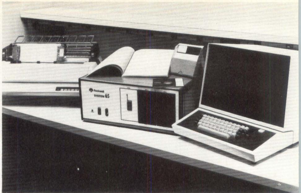
**Fig 8** Rockwell System 65 development system supports R6500 microcomputer system development with dual minifloppy disk drives, 16K bytes of static RAM plus ROM-based resident system software, monitor, text editor and assembler.
