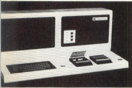
**Fig 7** Information Control Microcommand System™ supports development of 8080 and Z-80 microprocessor-based systems with light pen, editor, assembler, monitor, up to 64K RAM and up to 2 Kbytes ROM, dual floppy disks, EPROM programmer, keyboard, CRT and optional In-Circuit Debugger.™
