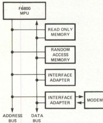
Fig 1 Microcomputer consists of micro-processor (in this case Fairchild 6800), ROM, RAM and I/O.
