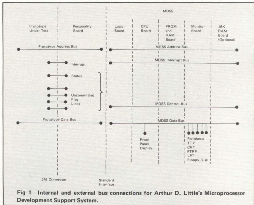
ADL's Microprocessor Development Support System (MDSS) is the capability to monitor and control the prototype in real-time. Curtis points out that many development systems that use emulation techniques cannot run in realtime; they incorporate an external
