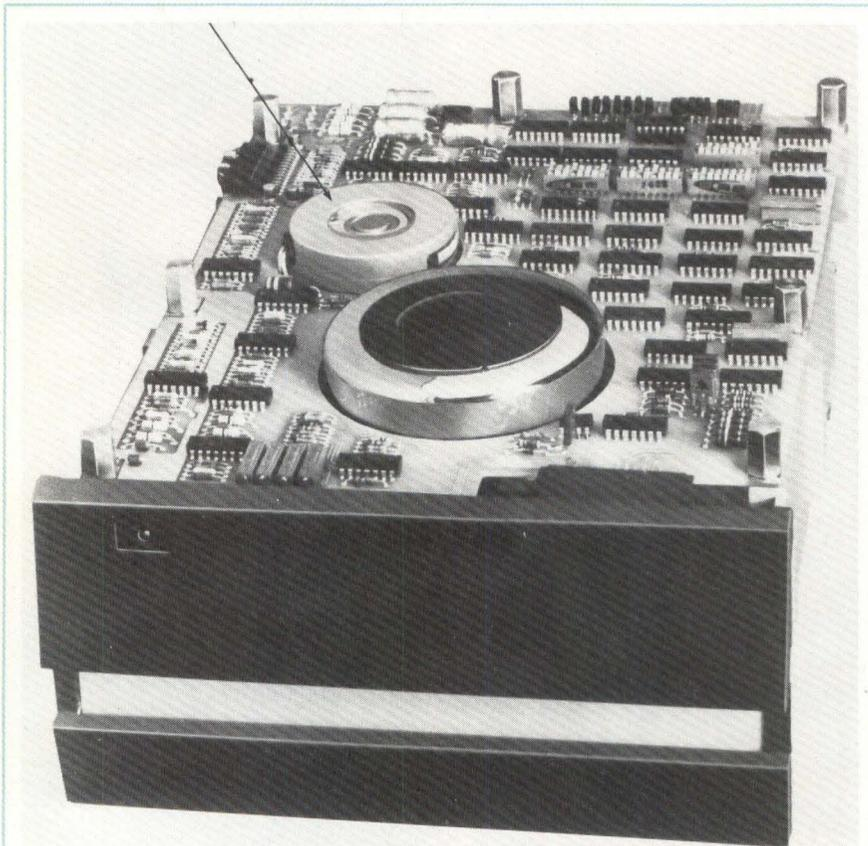
Fig 1 Top view of the 800 diskette drive shows central location of the stepper motor.
