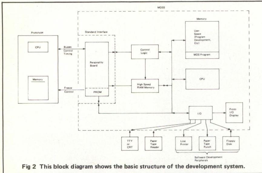
**Fig 2** This block diagram shows the basic structure of the development system.
