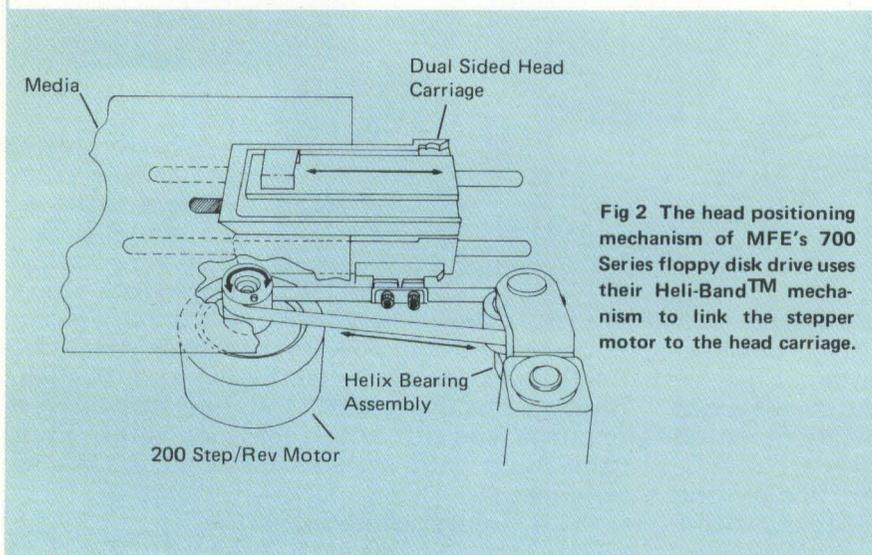
Fig 2 The head positioning mechanism of MFE's 700 Series floppy disk drive uses their Heli-Band™ mechanism to link the stepper motor to the head carriage.
