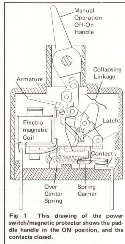
**Fig 1** This drawing of the power switch/magnetic protector shows the paddle handle in the ON position, and the contacts closed.
