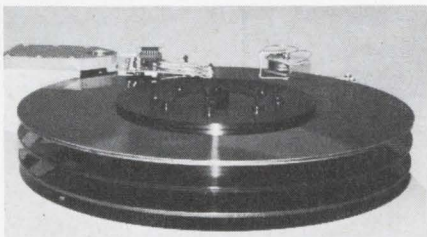
Figure 1: Alpha Data's Atlas 14" Winchester uses three platters and 72 heads in a sealed, maintenance-free chamber. Storage capacity for the $6K drive is 80 Mbytes to 100 Mbytes, with average access times of under 20ms.
