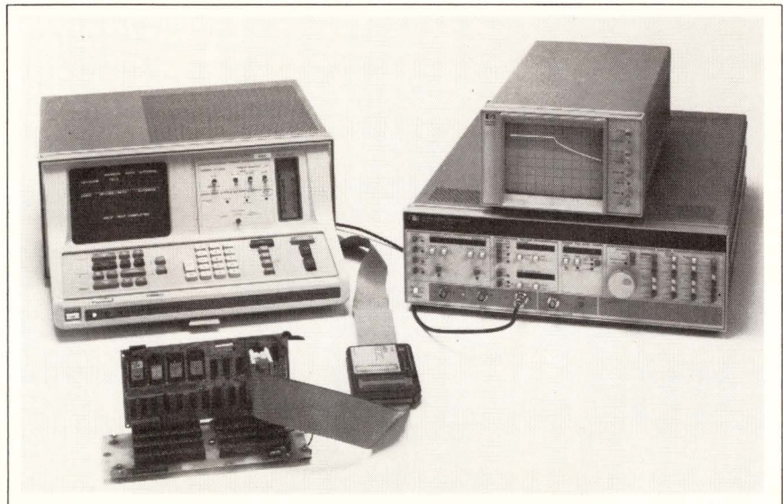
Figure 1: A typical equipment set-up using the 5180A Waveform Recorder with a HP1611A Logic Analyzer.
