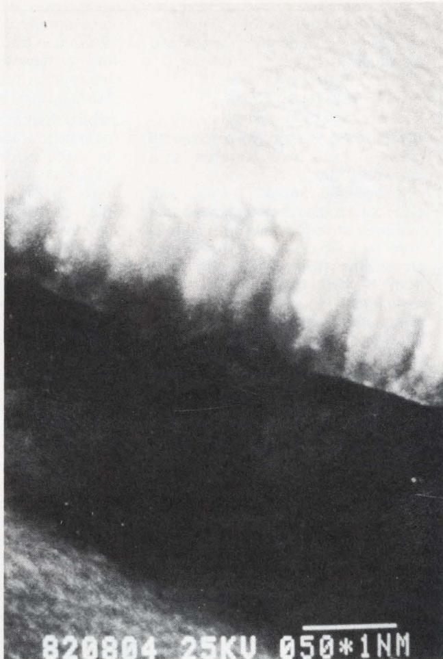
Figure 8: A cross-section view shows how cobalt-chromium forms crystals perpendicular to the diskettes surface.
