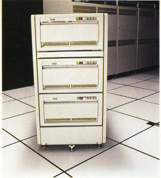
The RA81 disk subsystem from DEC. Shown in the background is a VAX 11/780.
