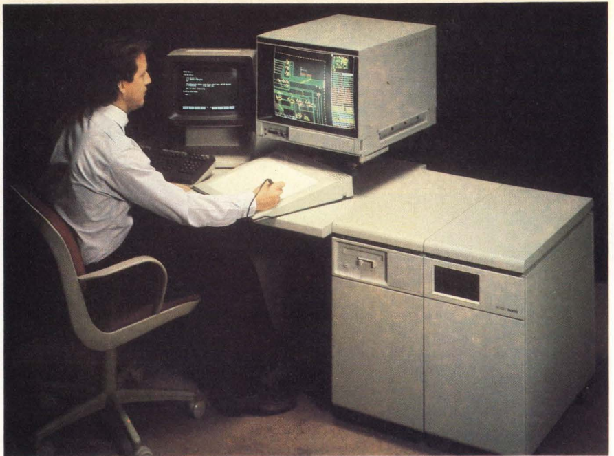
Figure 4: Hewlett-Packard's 9000 series model 540 workstation can be configured with three processors, runs HP-UX, supports up to six users and each I/O processor adds 8 DMA-capable I/O slots.
