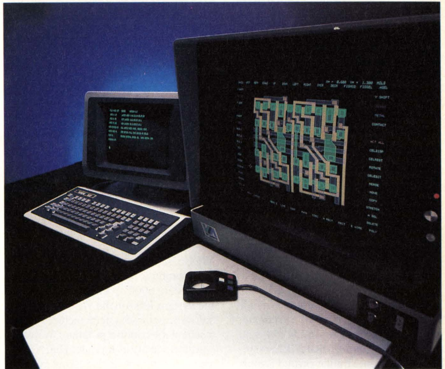
Figure 1: VIA Systems' workstation is based on DEC's 11/73 processor, includes a 330 Mbyte Winchester disk and runs VIA's VLSI design and layout software.
