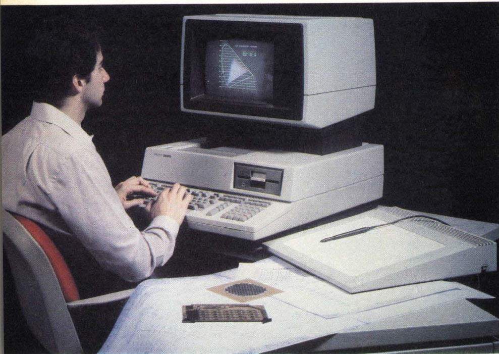
Figure 3: Hewlett-Packard's 9000 series Model 520 desktop workstation has a 5¼" floppy disk, can accommodate up to 5 Mbytes of RAM and runs HP-UX.
