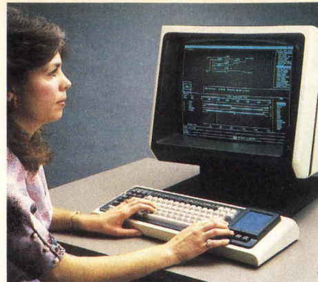
Based on Apollo's DOMAIN Computers, Calma's TEGASStation includes schematic capture, netlist extraction, logic simulation and fault simulation.
