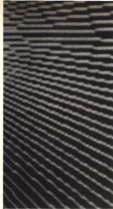
Megatek's proprietary antialiasing technique reduces jaggies appearing on lines and polygon boundaries in traditional raster display systems. These actual screen photos of the same image on the same monitor demonstrate the increase in addressable points to 3072 \times 2304 achieved using the technique (left) on the Merlin 9200.
