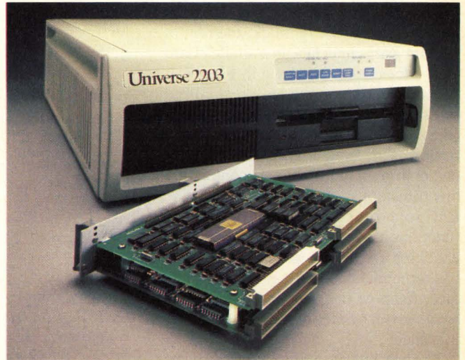
Figure 1: The 2203 is a seven-slot VMEbus backplane with Winchester and backup designed for 32-bit operation.
