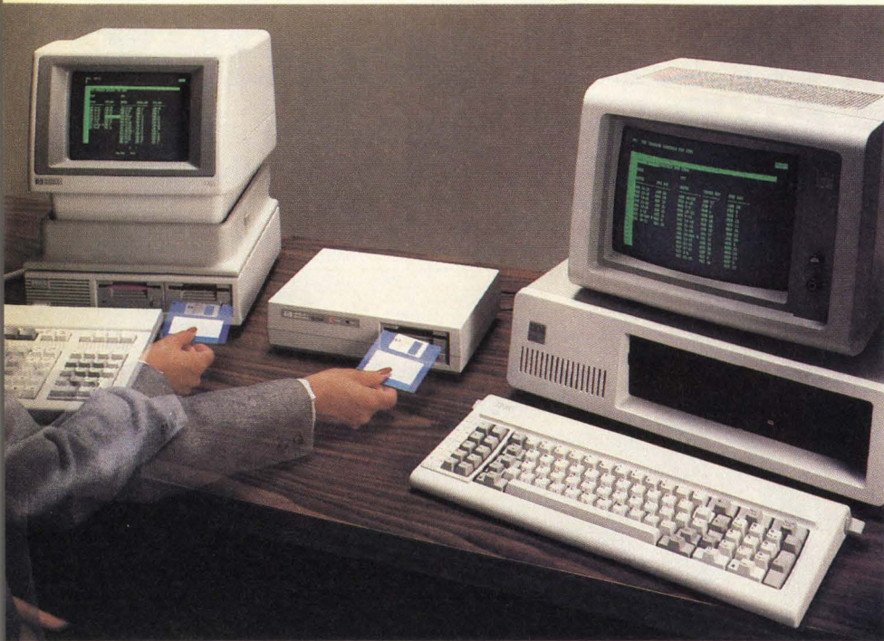
The first systems announced to use microfloppies were Hewlett-Packard's Personal Computers; HP now offers a line of microfloppy drives that can also be used with IBM PCs.
