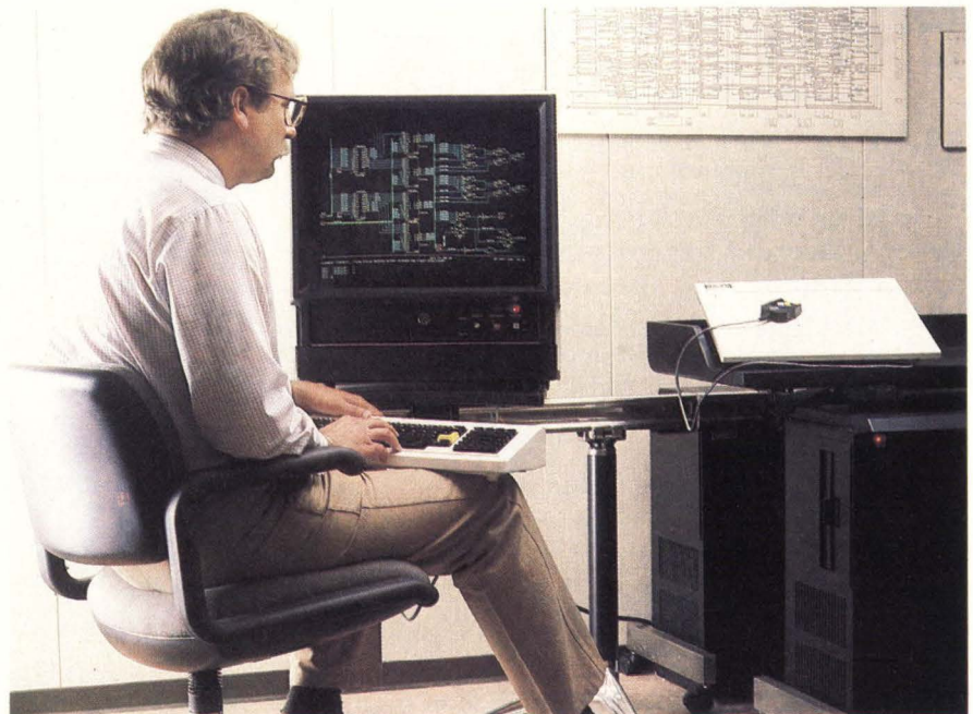
Figure 5: Daisy's Megalogician is a completely integrated workstation with capabilities ranging from schematic capture and gate array place-and-route to hardware simulation and physical modeling.
