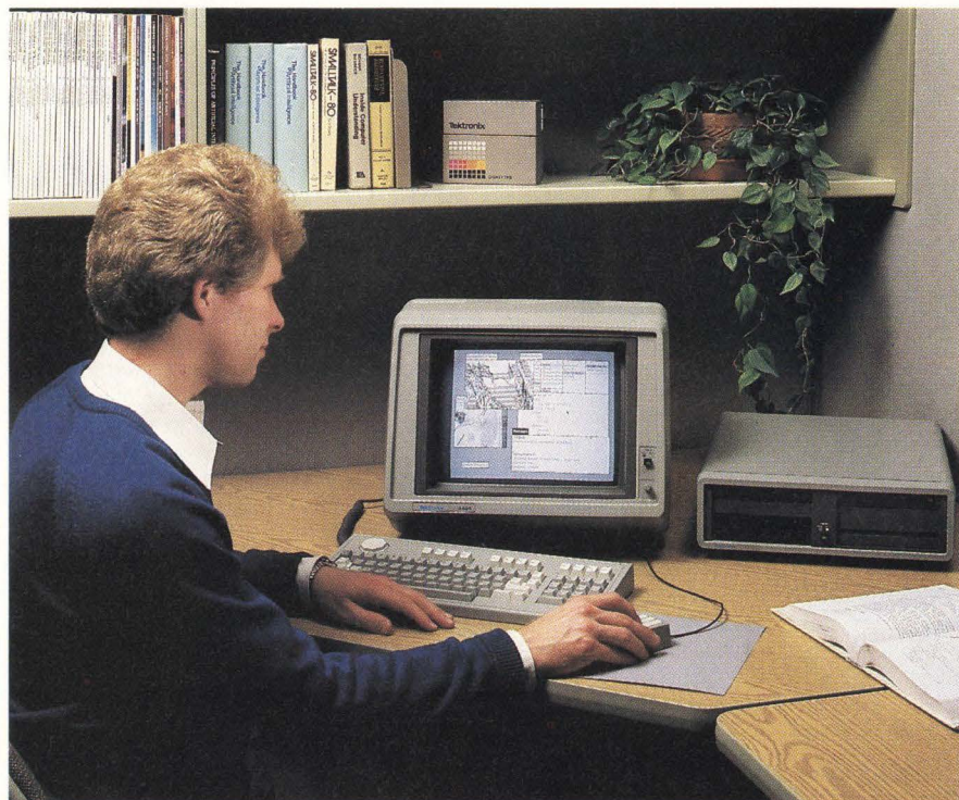
The standard Tektronix 4404 Artificial Intelligence System features a monochrome bit-mapped display; keyboard; mouse; 32-bit microprocessor with virtual memory management; hardware floating point; 1 Mbyte RAM; and a 20-Mbyte hard disk with a single 5 1/4" floppy disk.
