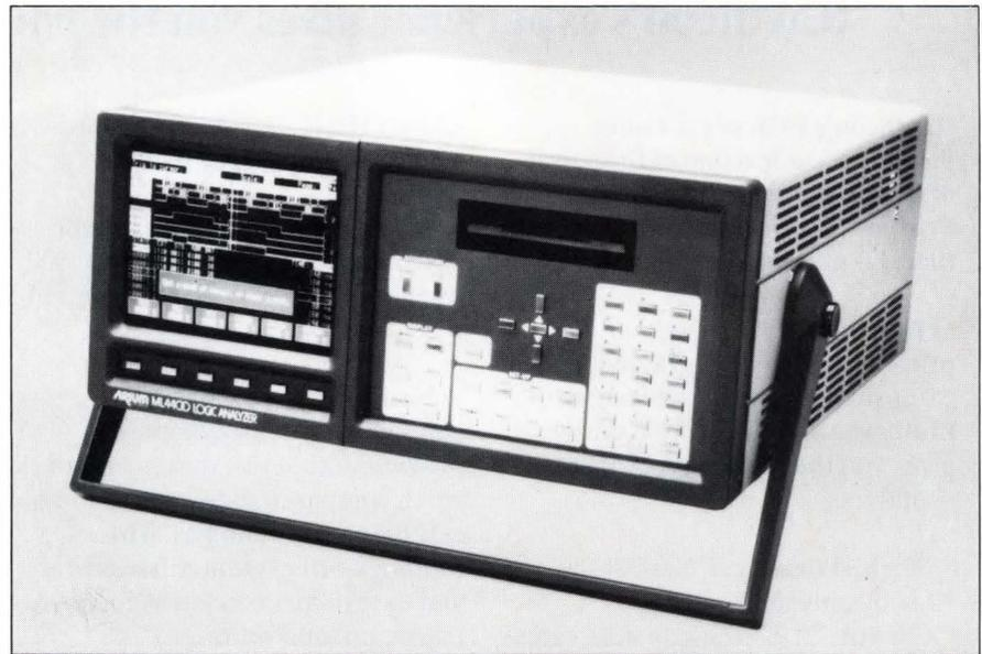
*Providing a good blend of channel width and speed in a moderately priced portable logic analyzer, the ML4400 from Arium supports 320 channels at 25 MHz, 160 channels at 50 MHz, and other configurations to as many as 16 channels at 400 MHz. It supports histograms and other time-measurement features found on many of the higher-priced systems.*
