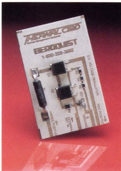
**Fig 4—Single-layer board solutions** such as Berquist's Thermal Clad can be used in SMT applications and as a mounting surface for power hybrids.
