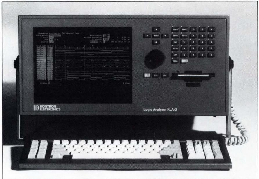
*Designed for high-performance applications, the KLA/2 from Kontron supports 192 channels at 50 MHz plus additional high-speed modules that are capable of 2-GHz clock rates. The system is available both in a portable 10-MHz IBM PC/AT-compatible version (shown here) or as a separate computer-controlled mainframe with two additional card slots. The unit has built-in channel-deskewing capability. A hexadecimal display of the address and data buses is next to the timing display.*
