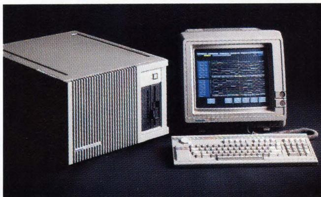
*The DAS 9200, now three years old, is still a top performer. This system still has the highest channel-count capacity at any clock rate from 20 MHz to 2 GHz. Tektronix continues to introduce new modules for this system.*
