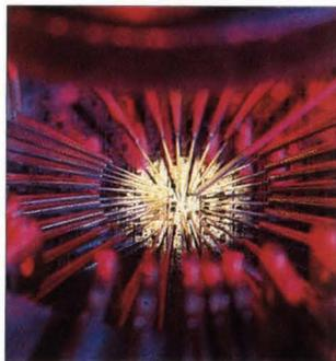
Advance water-level laser trimming assures maximum precision and stability for Burr-Brown op amps.
