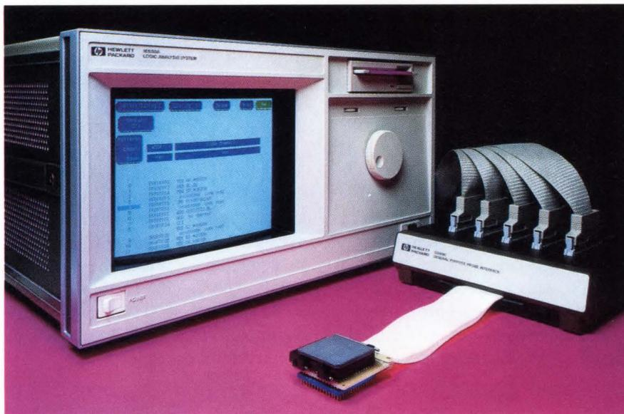
*Recently upgraded, the general-purpose logic-analysis modules for the 16500A from Hewlett-Packard now support 35-MHz synchronous clocking and a memory-compare capability. High-performance modules support clock rates reaching 1 GHz.*
